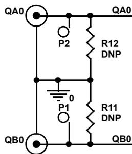
**FIGURE 10. QA/QB BNC COMPARATOR OUTPUTS**
