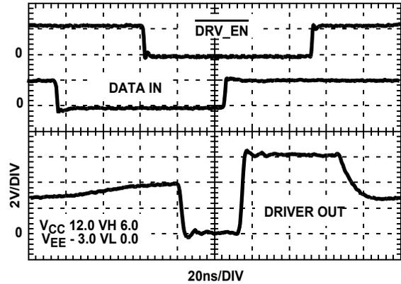
**FIGURE 12. DATA AND DRV\_EN CONTROL OF DRIVER OUT**
