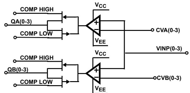
FIGURE 3. DIAGRAM OF ISL55100A/BEVAL3/3Z DRIVERS AND RECEIVERS
