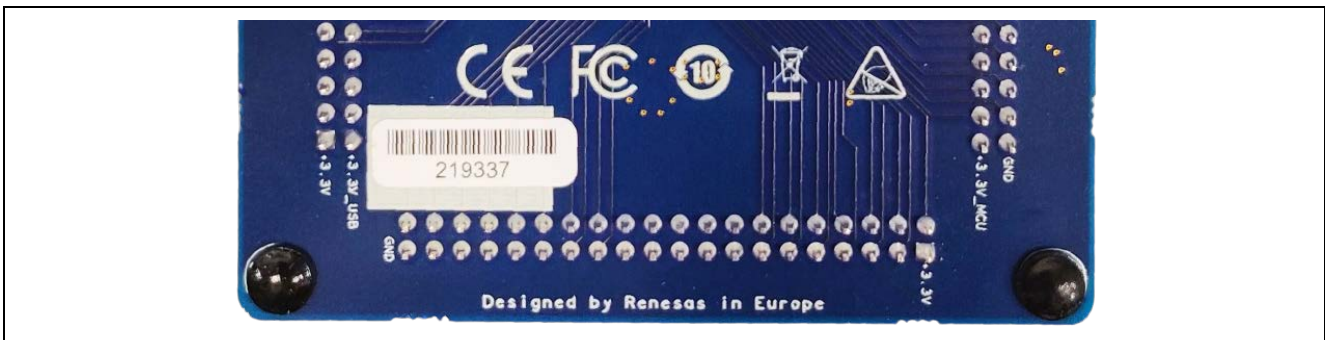
Figure 7. Identification of the Serial Number on the EK-RA4M3 Board
