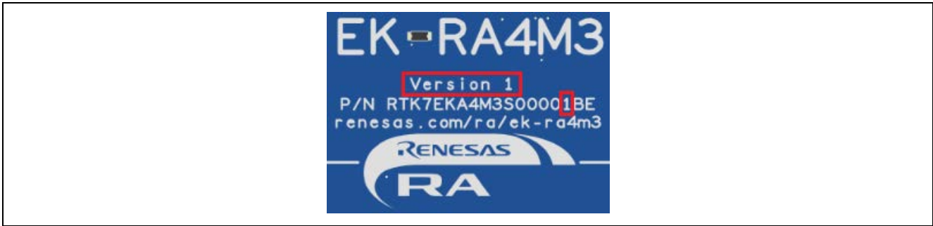
Figure 5. Identification of the Kit Version Number on the EK-RA4M3 Board
