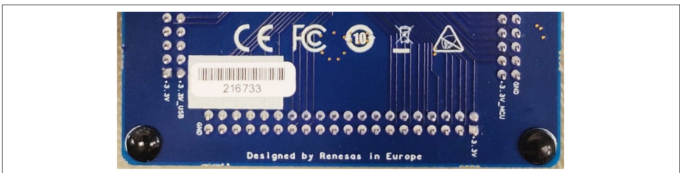
Figure 7. Identification of the Serial Number on the EK-RA4M2 Board
