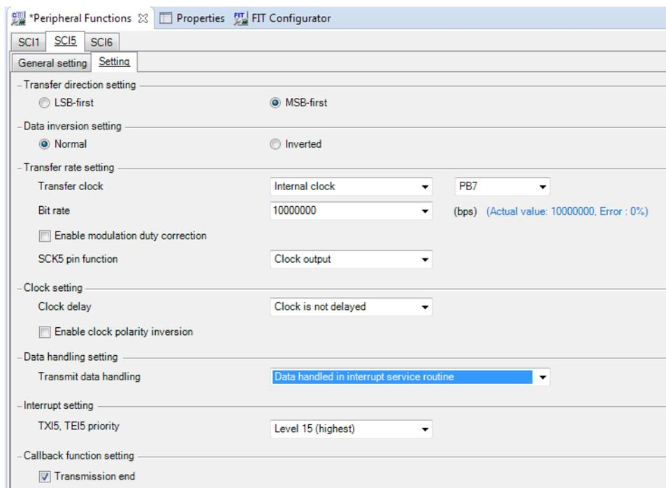
**Figure 4-11 SCI5 SPI Master Setting**
