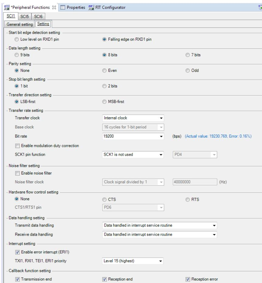
**Figure 4-13 SCI1 Asynchronous Setting**
