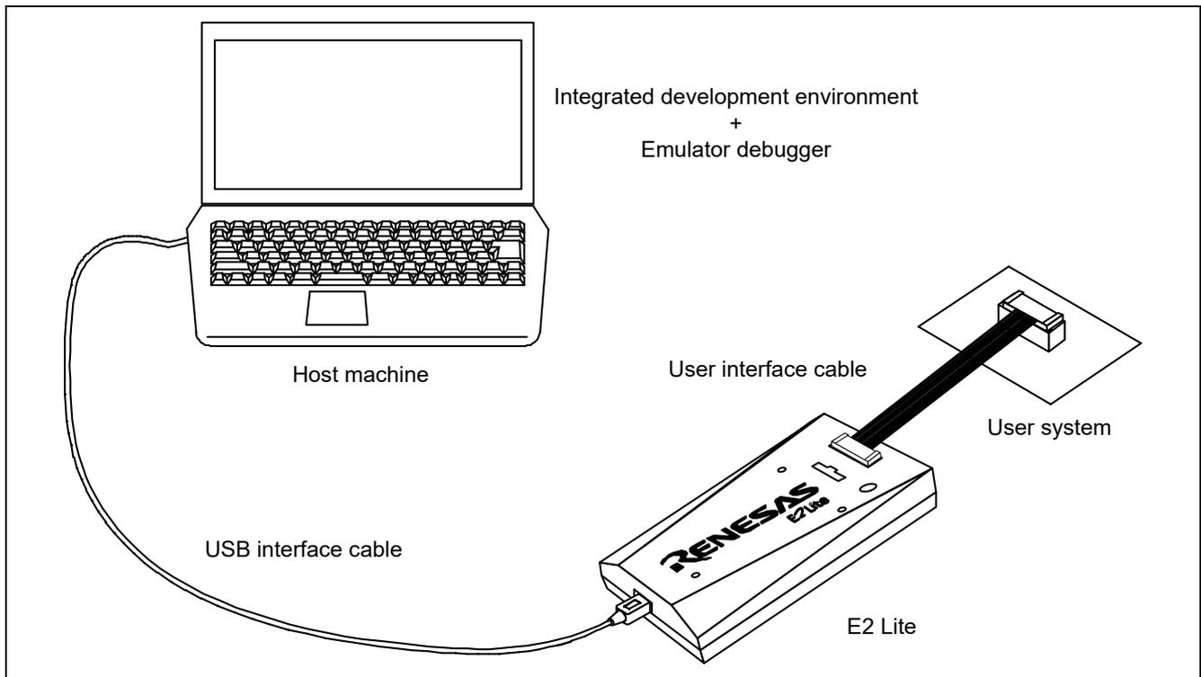
**Figure 1.1 System Configuration of the E2 Lite**
