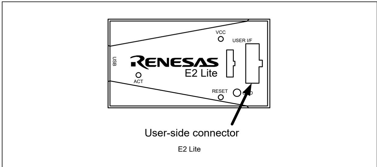
Figure 2.2 User-Side Connector on the E2 Lite
