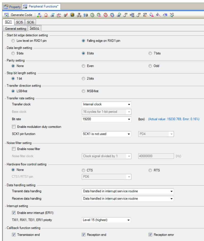
**Figure 4-12 SCI1 Asynchronous Setting**
