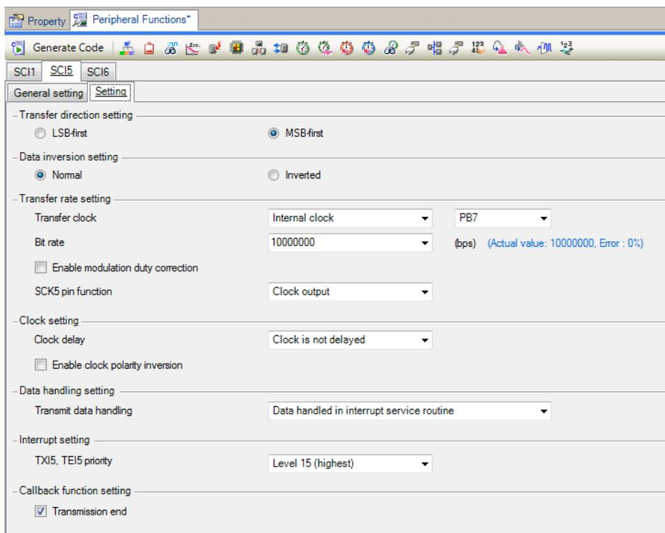
**Figure 4-10 SCI5 SPI Master Setting**
