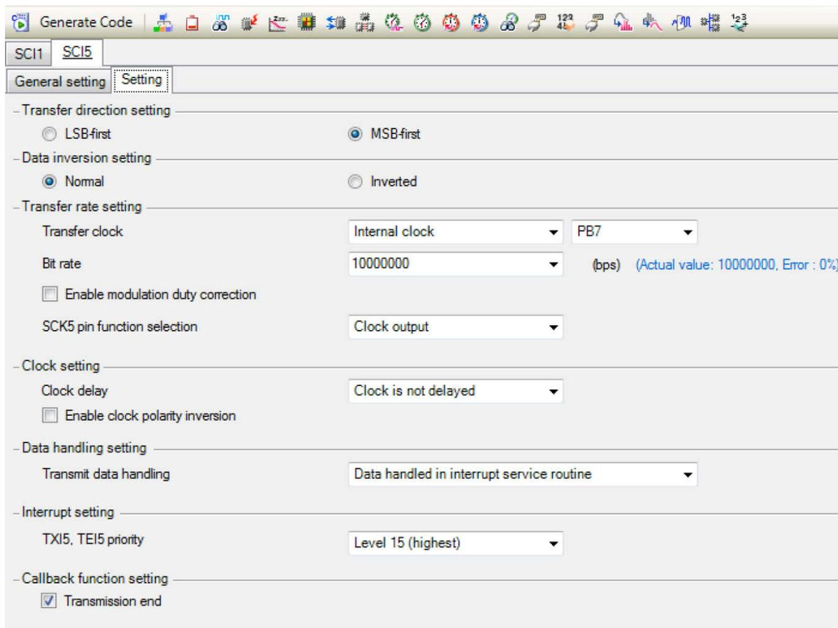
Figure 4-10 SCI5 SPI Master Setting
