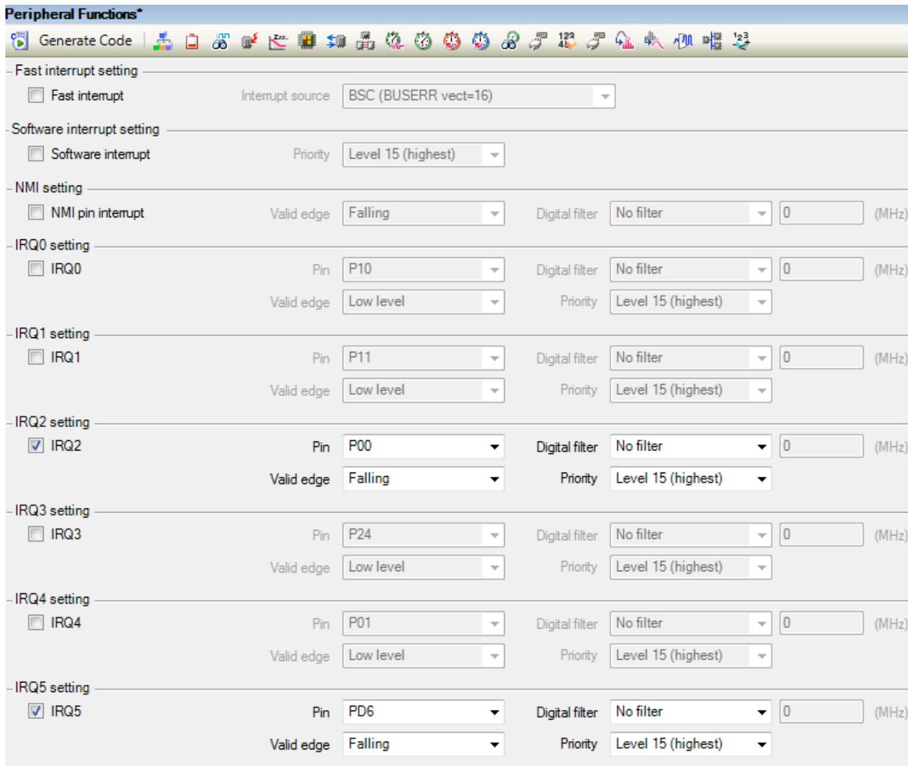
Figure 4-3 Interrupt Functions tab
