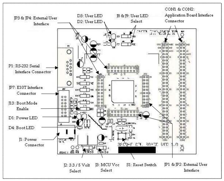
Figure 2.1 Names of Parts on CPU Board
