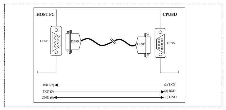
Figure 2.2 Serial Communication connections
