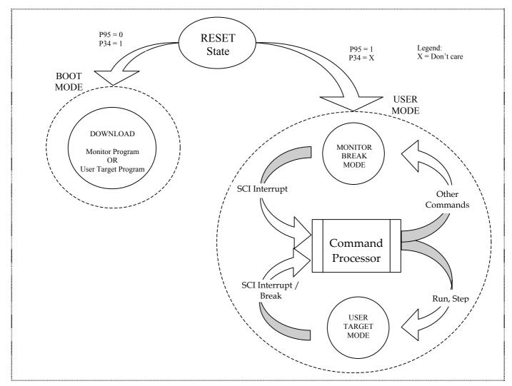
Figure 7.1 Mode Transition Diagram
