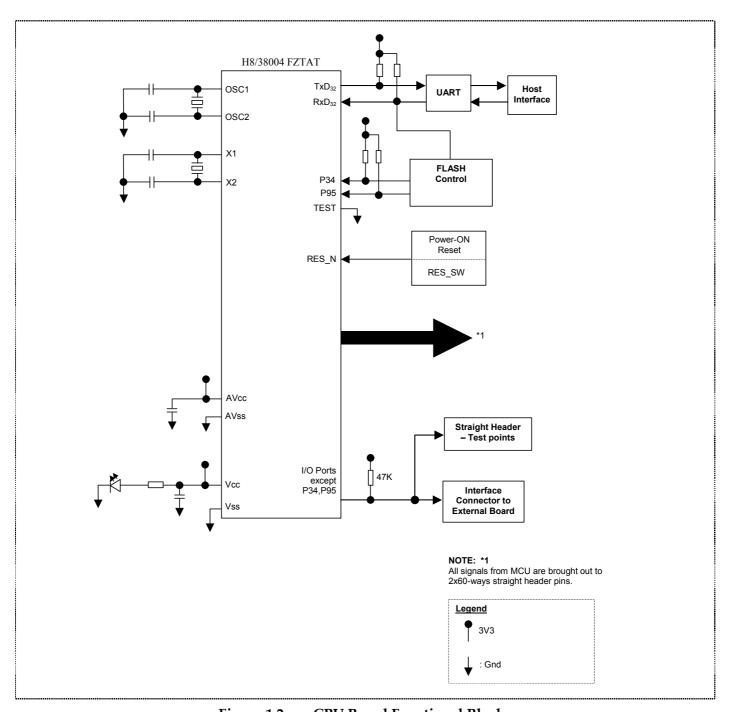
Figure 1.2 CPU Board Functional Blocks
