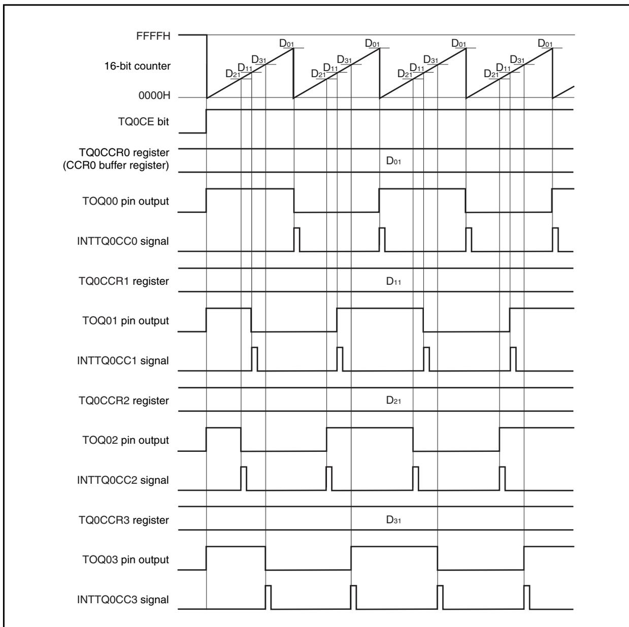
If the value of the TQ0CCRk register is greater than the value of the TQ0CCR0 register, the value of the 16-bit counter will not match the value of the TQ0CCRk register. Consequently, the INTTQ0CCk signal is not generated, nor is the output of the TOQ0k pin changed.
