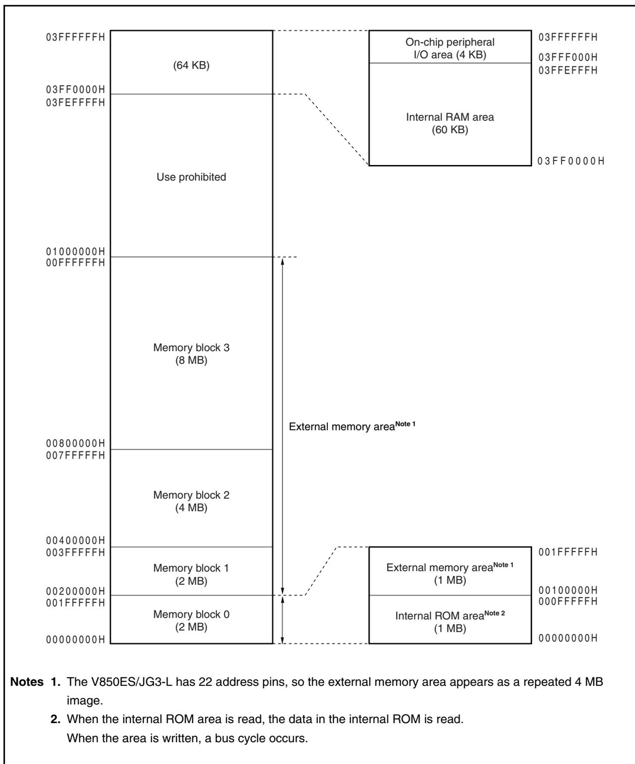
**Notes** 1. The V850ES/JG3-L has 22 address pins, so the external memory area appears as a repeated 4 MB image.
