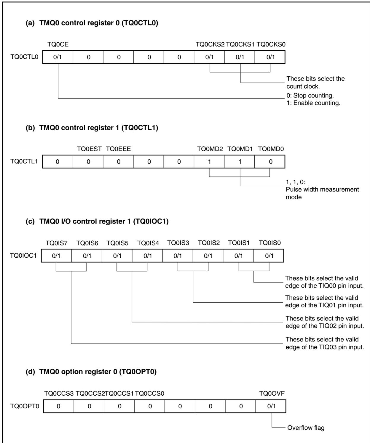
**Figure 8-67. Register Settings in Pulse Width Measurement Mode (2/2)****(e) TMQ0 counter read buffer register (TQ0CNT)**
