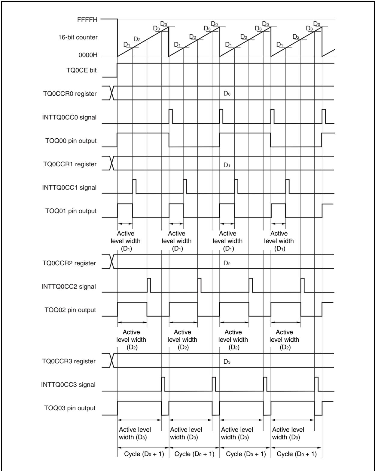
When the TQ0CE bit is set to 1, the 16-bit counter is cleared from FFFFH to 0000H, starts incrementing, and outputs a PWM waveform from the TOQ0k pin.
