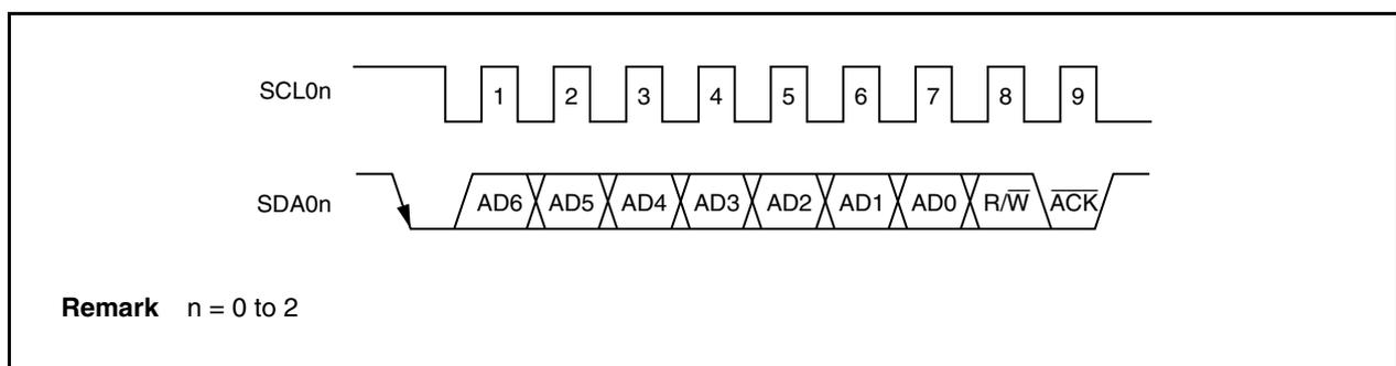
When the local address is received,  $\overline{\text{ACK}}$  is automatically generated regardless of the value of the ACKEn bit. No  $\overline{\text{ACK}}$  is generated if the received address is not a local address (NACK).
