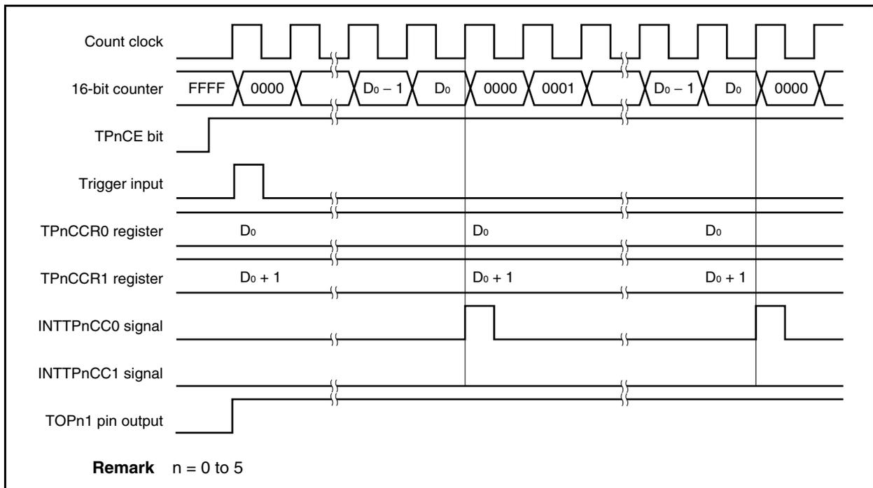
**(c) Detection of trigger immediately before or after INTTPnCC1 generation**
