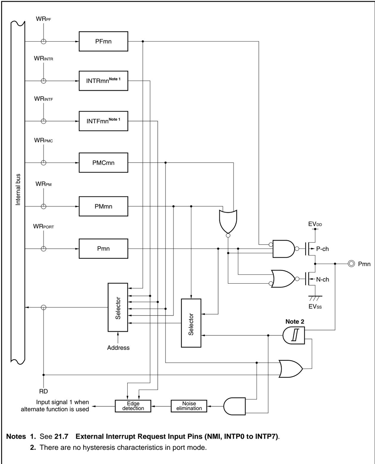
Figure 4-17. Block Diagram of Type N-1
