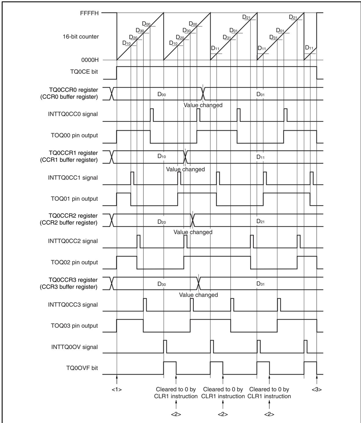
Figure 8-56. Timing and Processing of Operations in Free-Running Timer Mode (Compare Function) (2/2)
