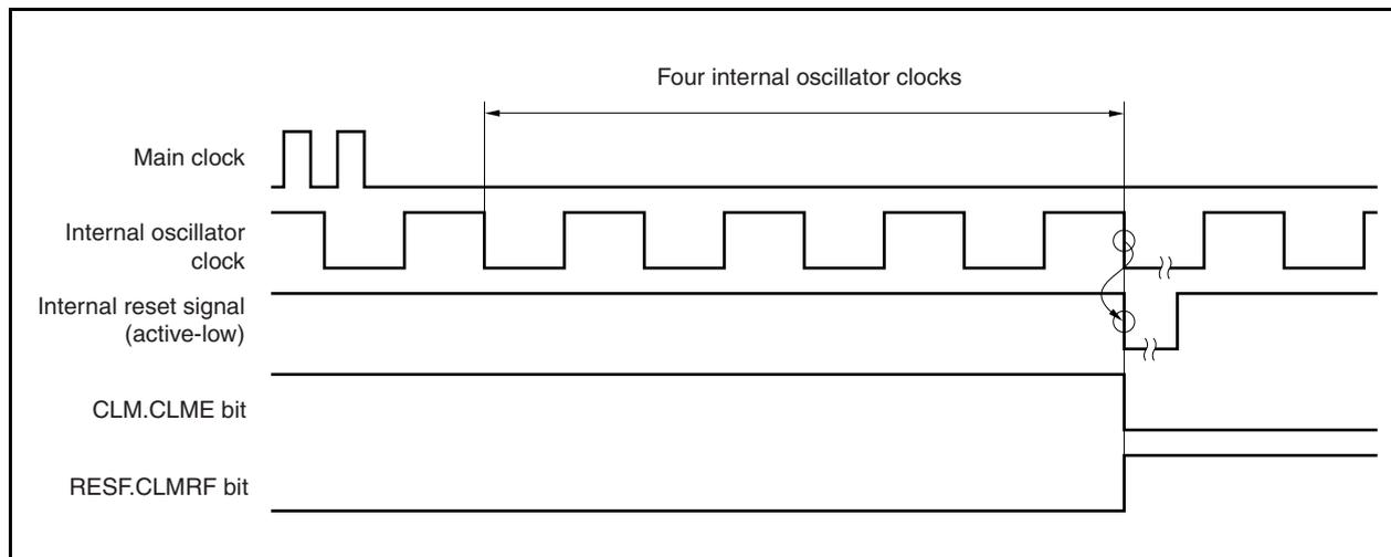
**(2) Clock monitor status after  $\overline{\text{RESET}}$  input**
