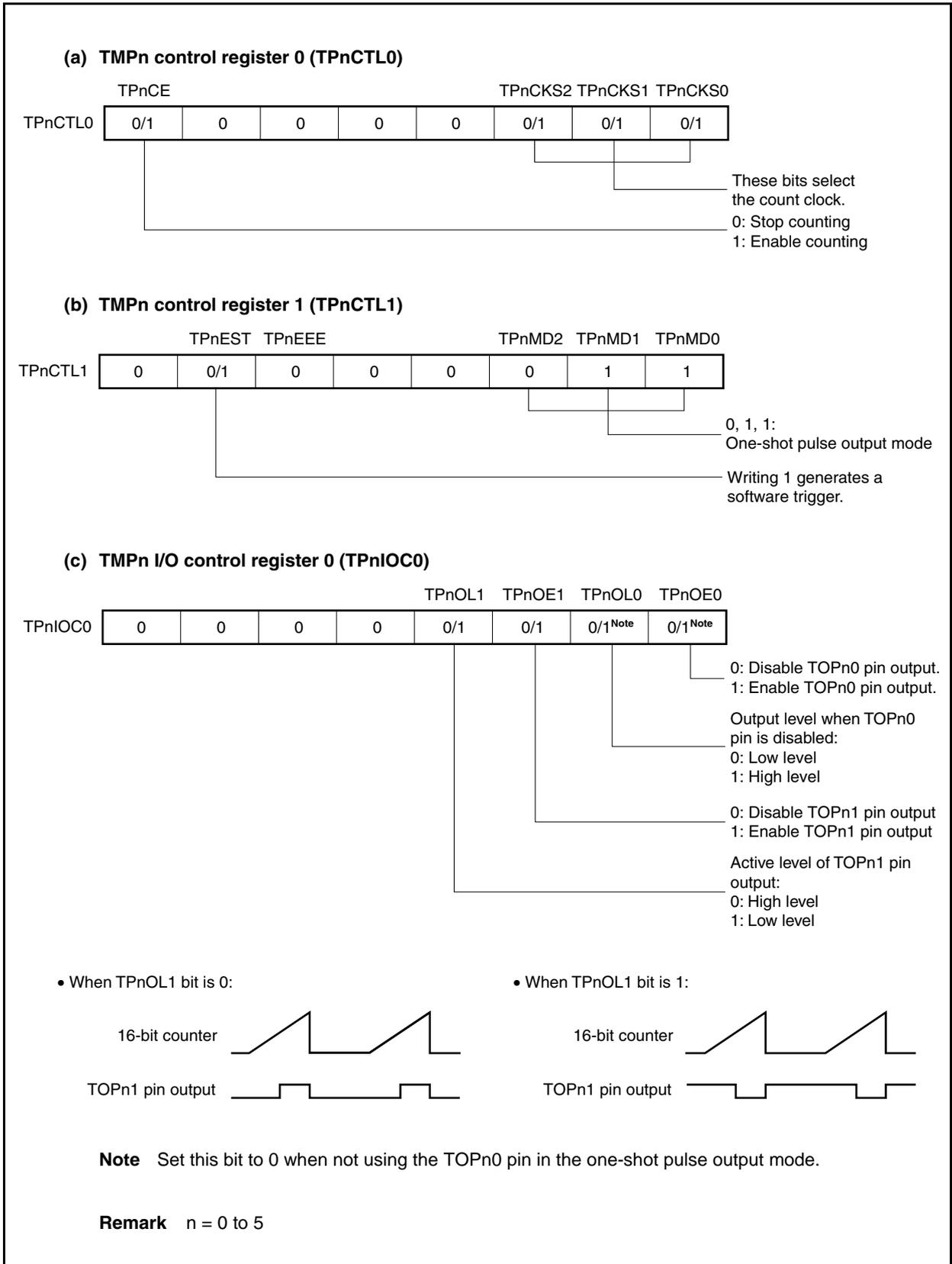
Figure 7-40. Register Settings in One-Shot Pulse Output Mode (2/2)
