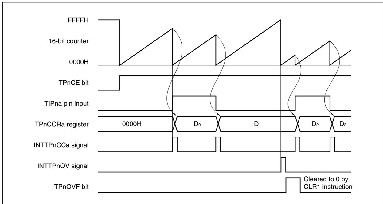
When the TPnCE bit is set to 1, the 16-bit counter starts incrementing. When it is subsequently detected that a valid edge has been input to the TIPna pin, the value of the 16-bit counter is stored in the TPnCCRa register, the 16-bit counter is cleared to 0000H, and a capture interrupt request signal (INTTPnCCa) is generated.
