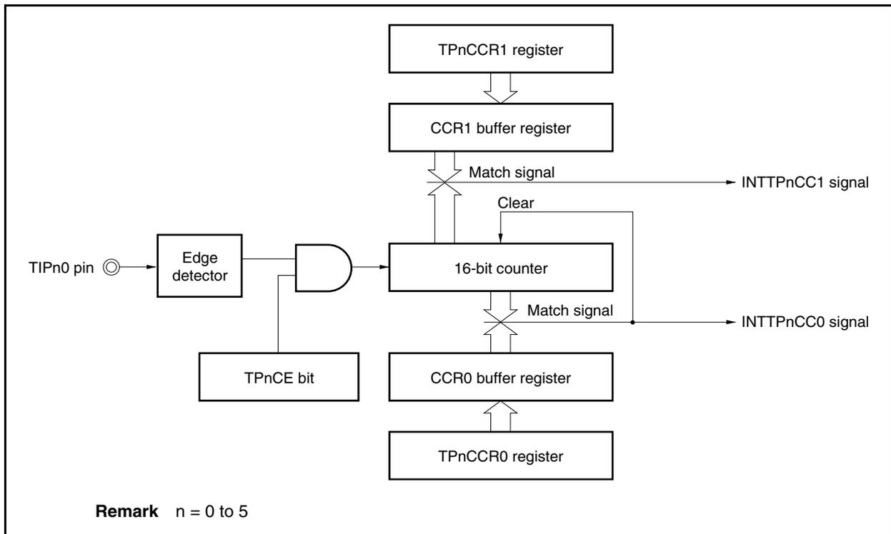
If the value of the TPnCCR1 register is less than or equal to the value of the TPnCCR0 register, the INTTPnCC1 signal is generated once per cycle.
