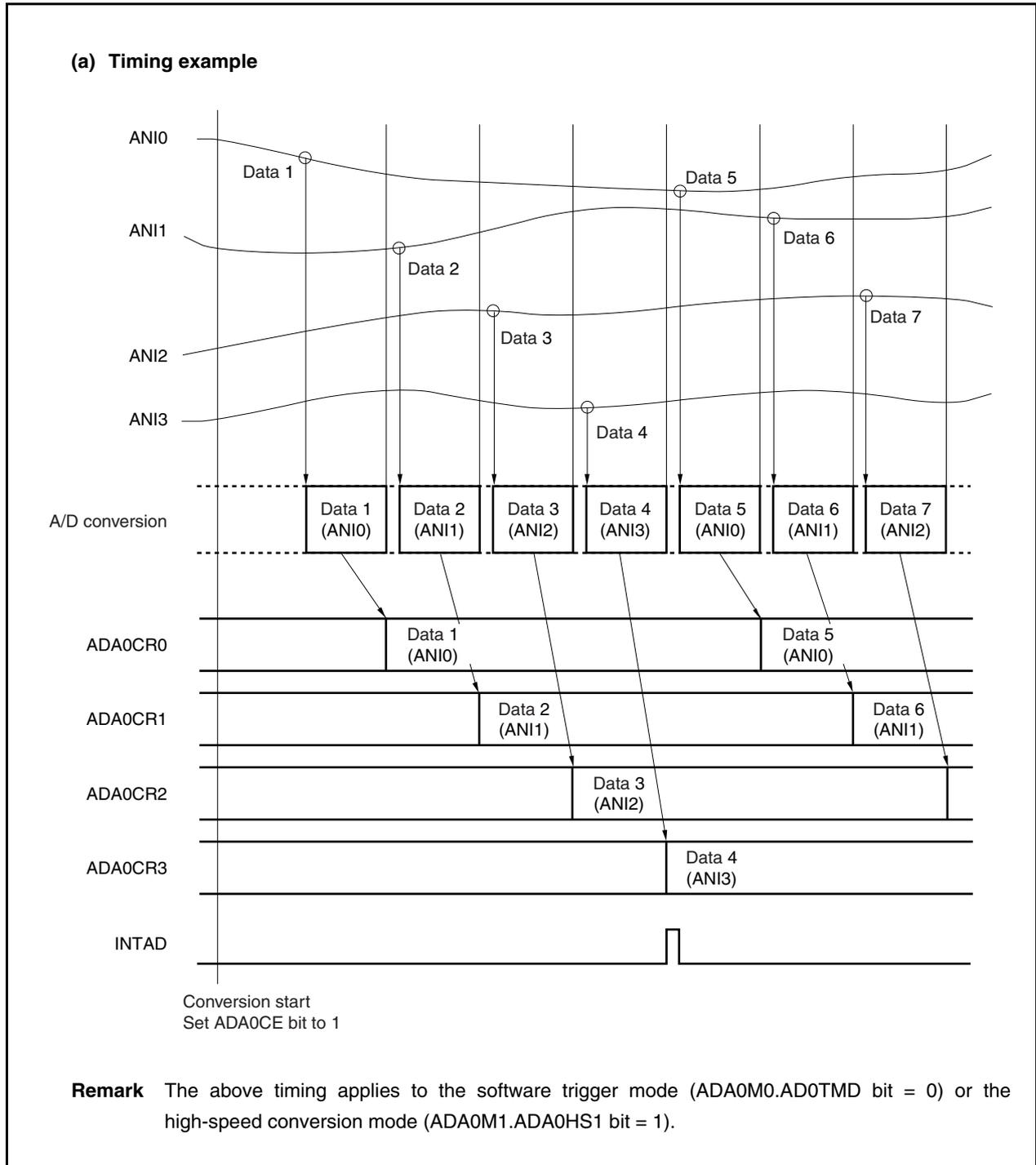
Figure 14-5. Example of Timing in Continuous Scan Mode (ADA0S Register = 03H) (2/2)
