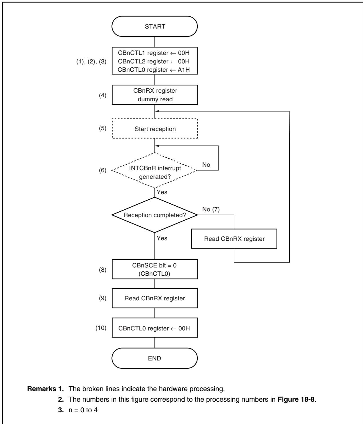
**Figure 18-8. Single Transfer Mode Operation Timing (Master Mode, Reception Mode)**
