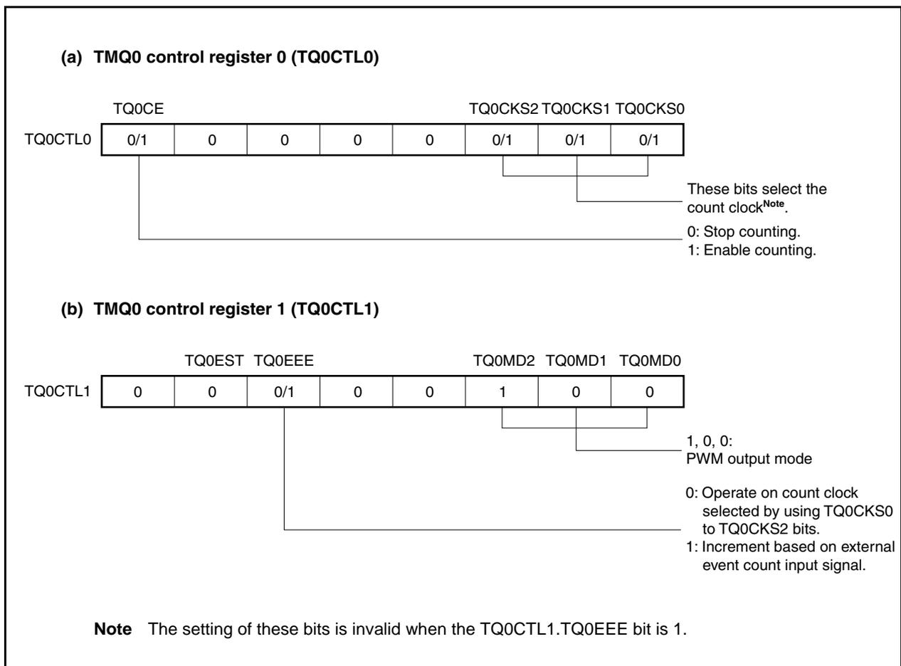
Figure 8-46. Register Settings in PWM Output Mode (2/3)
