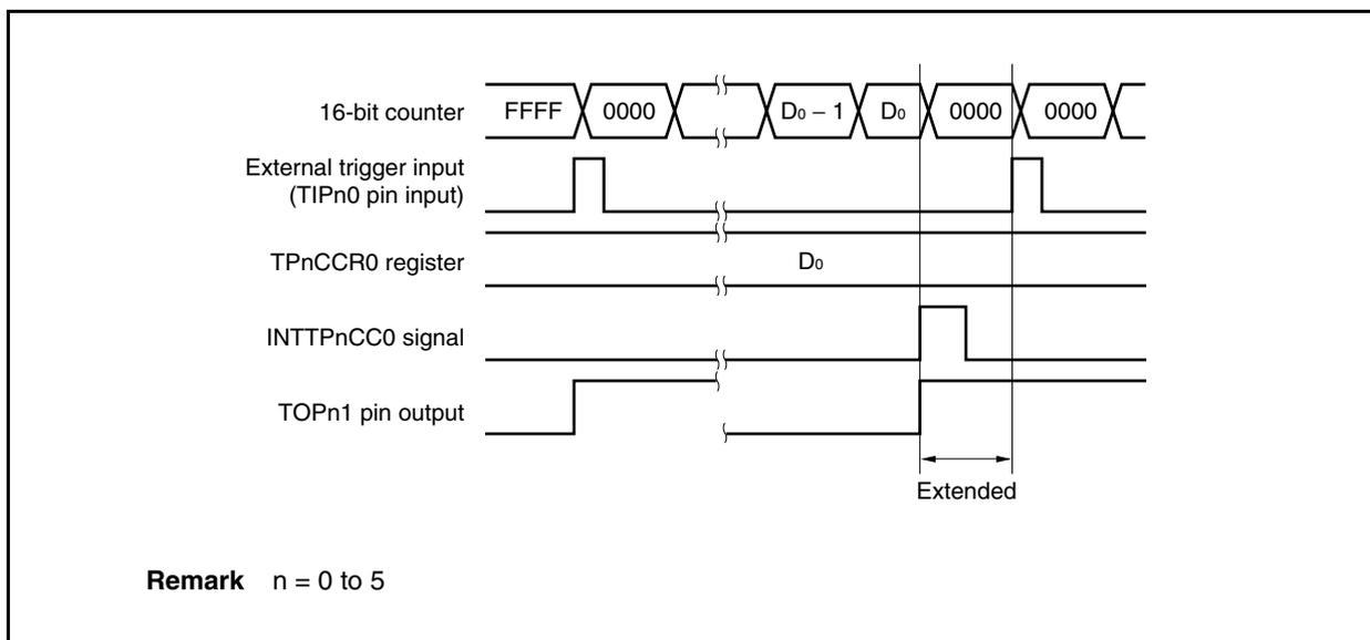
If the trigger is detected immediately before the INTTPnCC0 signal is generated, the INTTPnCC0 signal is not generated. The 16-bit counter is cleared to 0000H, the TOPn1 pin is set to the active level, and the counter continues incrementing. Consequently, the inactive period of the PWM waveform is shortened.
