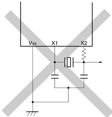
**Remark** For the subsystem clock, read X1 and X2 as XT1 and XT2. Note that a resistor must be inserted in series on the XT2 side.
