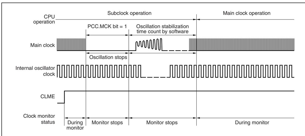
**(5) Operation while CPU is operating on internal oscillator clock (CCLS.CCLS bit = 1)**
