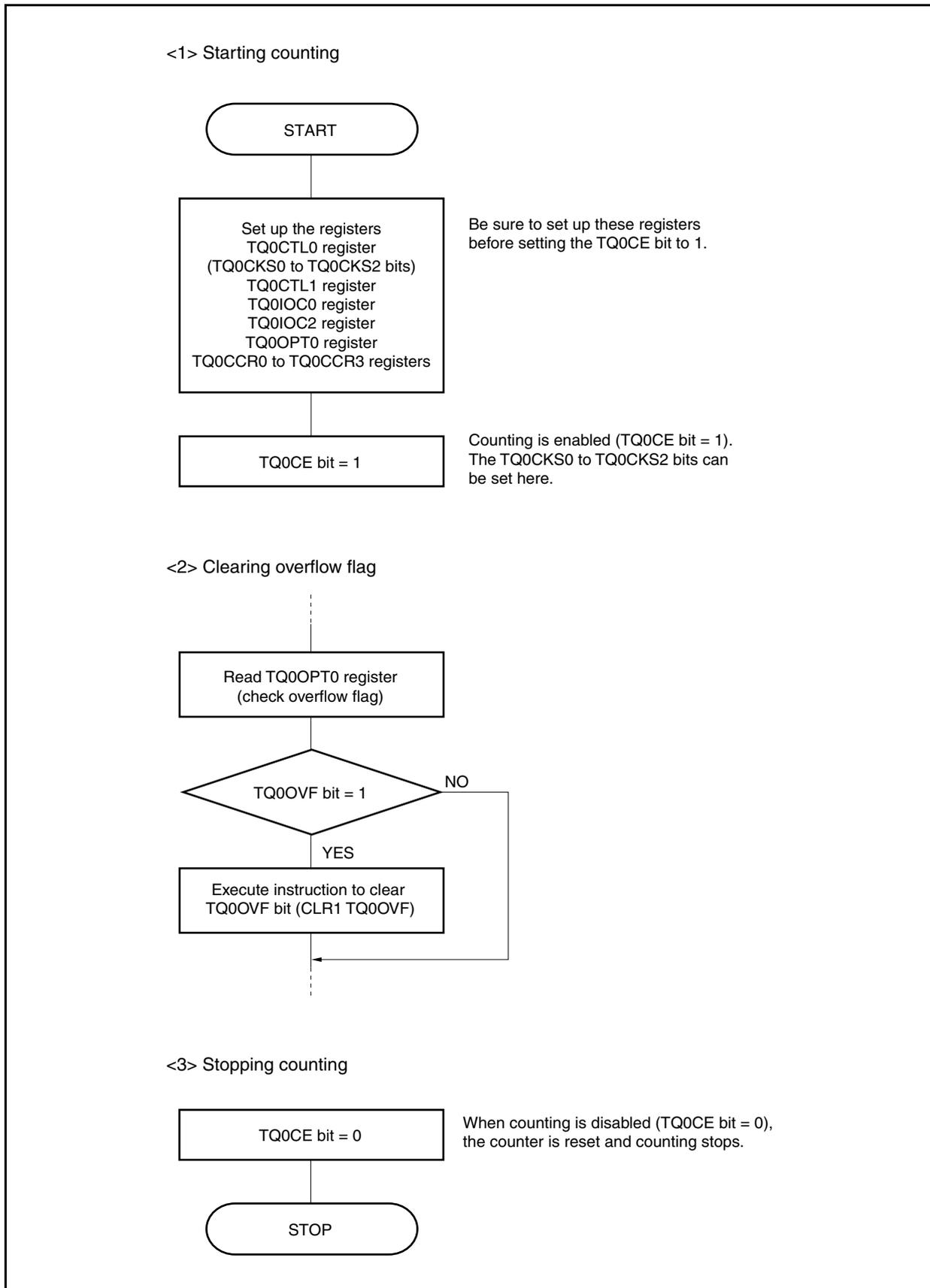
(b) Using a capture/compare register as a capture register
