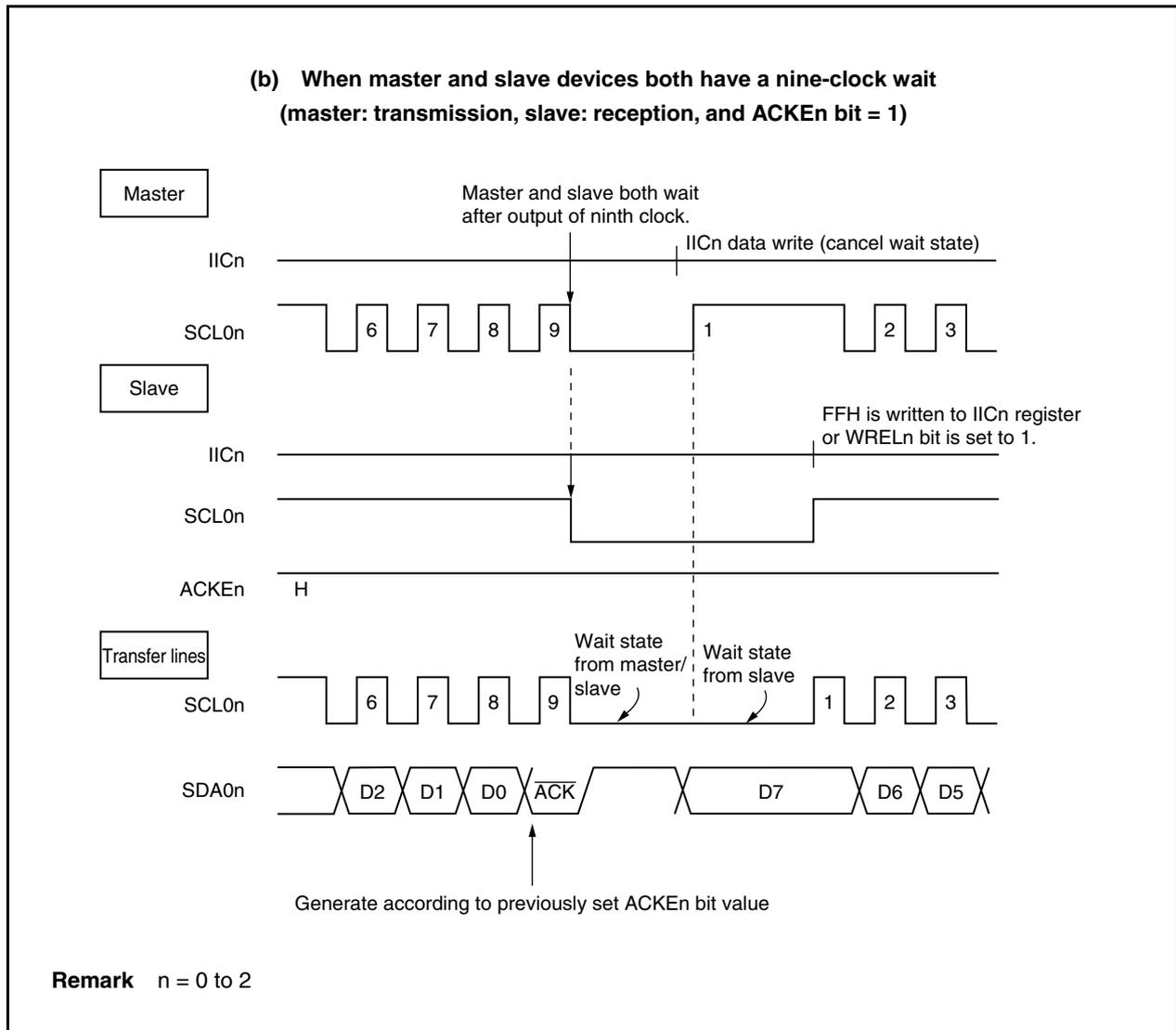
A wait state may be automatically generated depending on the setting of the IICn.WTIMn bit (n = 0 to 2). Normally, when the IICn.WRELn bit is set to 1 or when FFH is written to the IICn register on the receiving side, the wait state is canceled and the transmitting side writes data to the IICn register to cancel the wait state. The master device can also cancel the wait state via either of the following methods.
