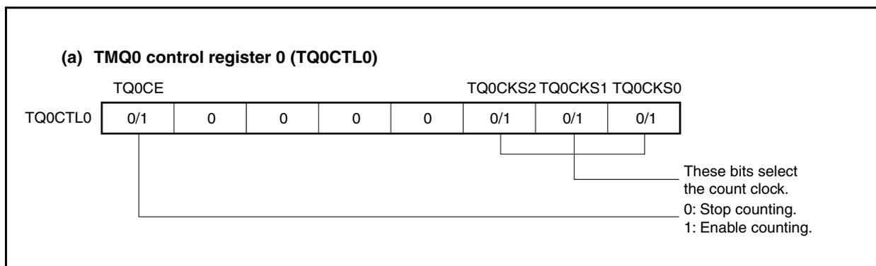
Figure 8-28. Register Settings in External Trigger Pulse Output Mode (2/3)
