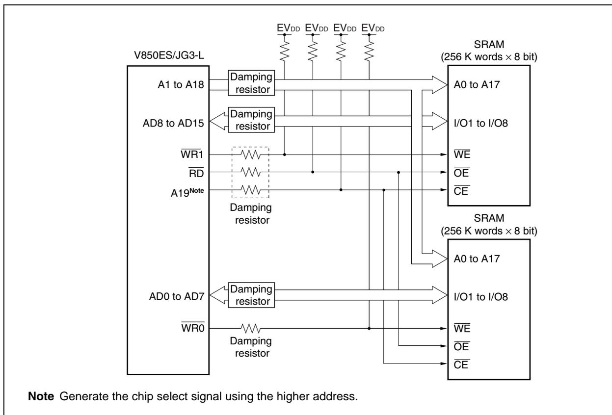
Figure 5-19. Connecting SRAM with 16-bit Data Bus to V850ES/JG3-L via 16-bit Bus
