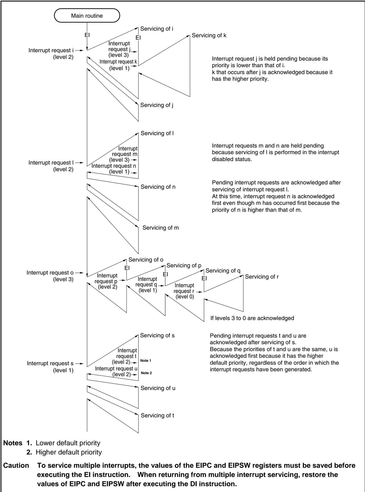
**Figure 21-8. Example of Servicing Interrupt Requests Generated Simultaneously**
