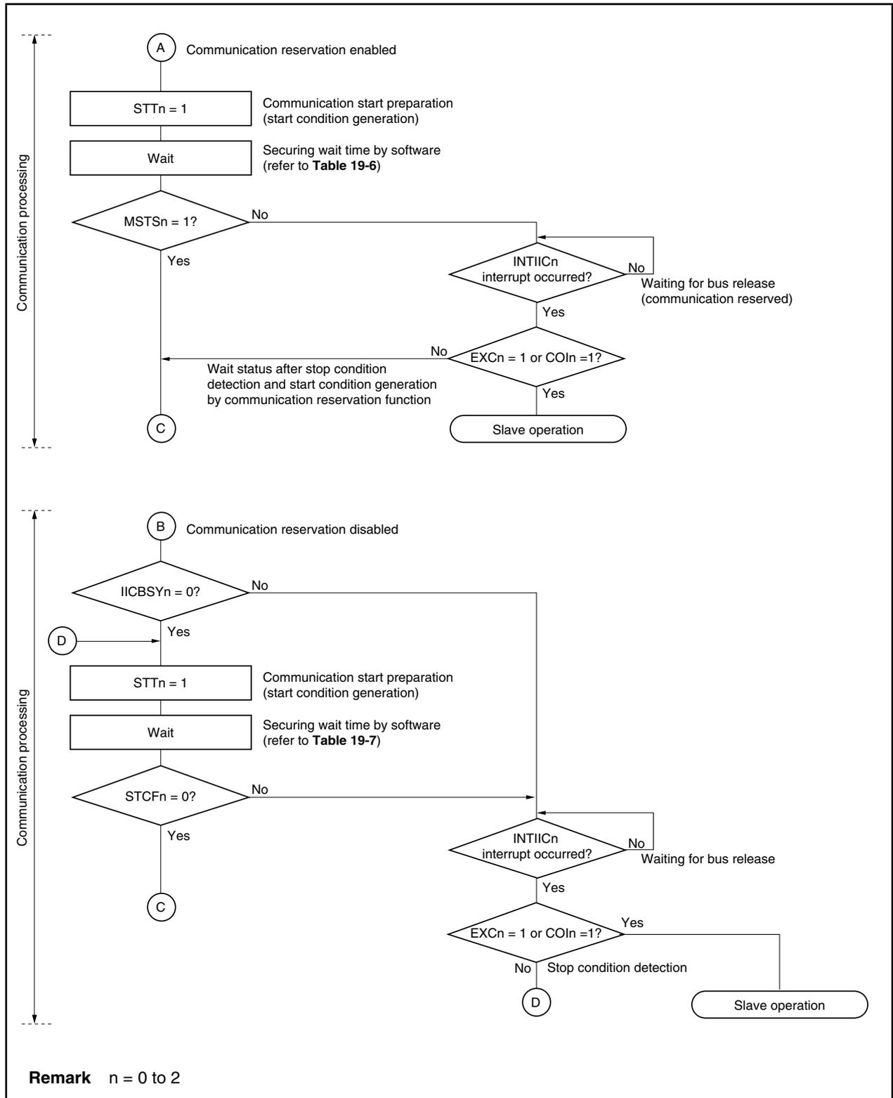
Figure 19-19. Master Operation in Multimaster System (3/3)
