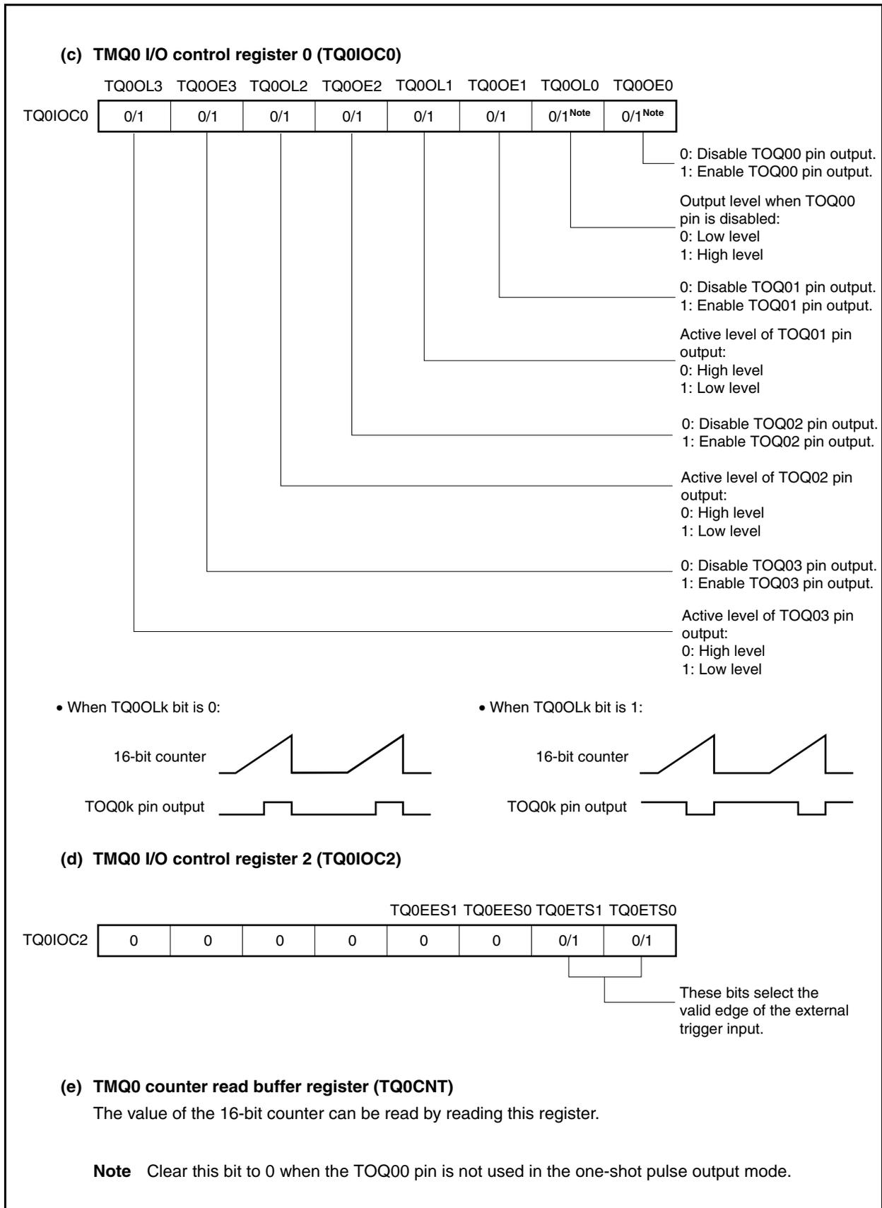
Figure 8-40. Register Settings in One-Shot Pulse Output Mode (3/3)
