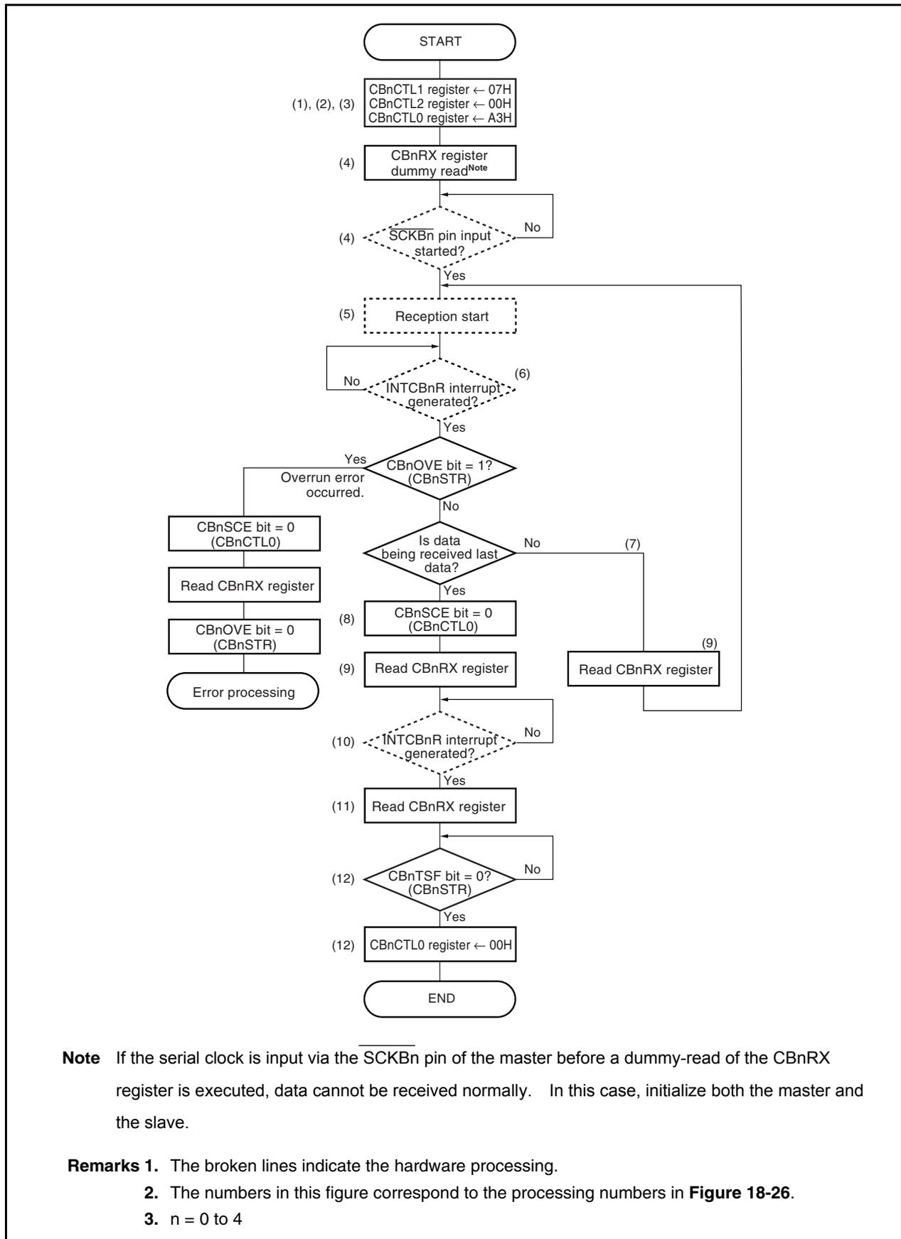
**Figure 18-26. Continuous Transfer Mode Operation Timing (Slave Mode, Reception Mode)**
