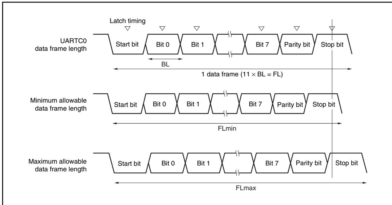
As shown in Figure 17-16, the receive data latch timing is determined by the counter set using the UC0CTL2 register following start bit detection. The transmit data can be received normally if up to the last data (stop bit) can be received in time for this latch timing.
