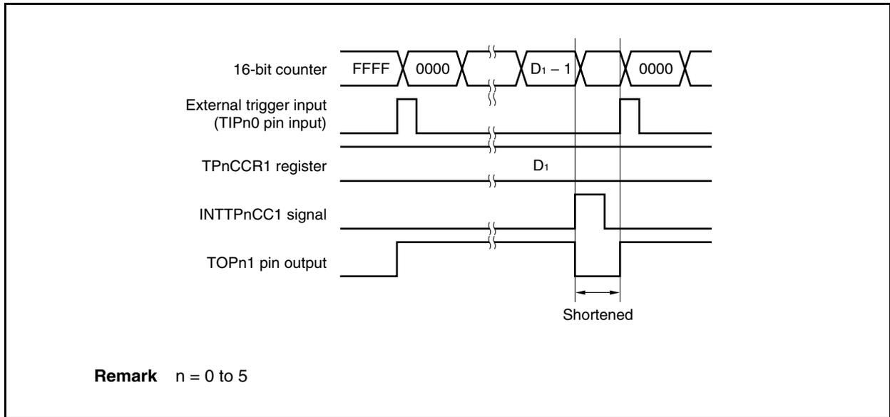
If the trigger is detected immediately before the INTTPnCC1 signal is generated, the INTTPnCC1 signal is not generated, and the 16-bit counter is cleared to 0000H and continues incrementing. The output signal of the TOPn1 pin remains active. Consequently, the active period of the PWM waveform is extended.
