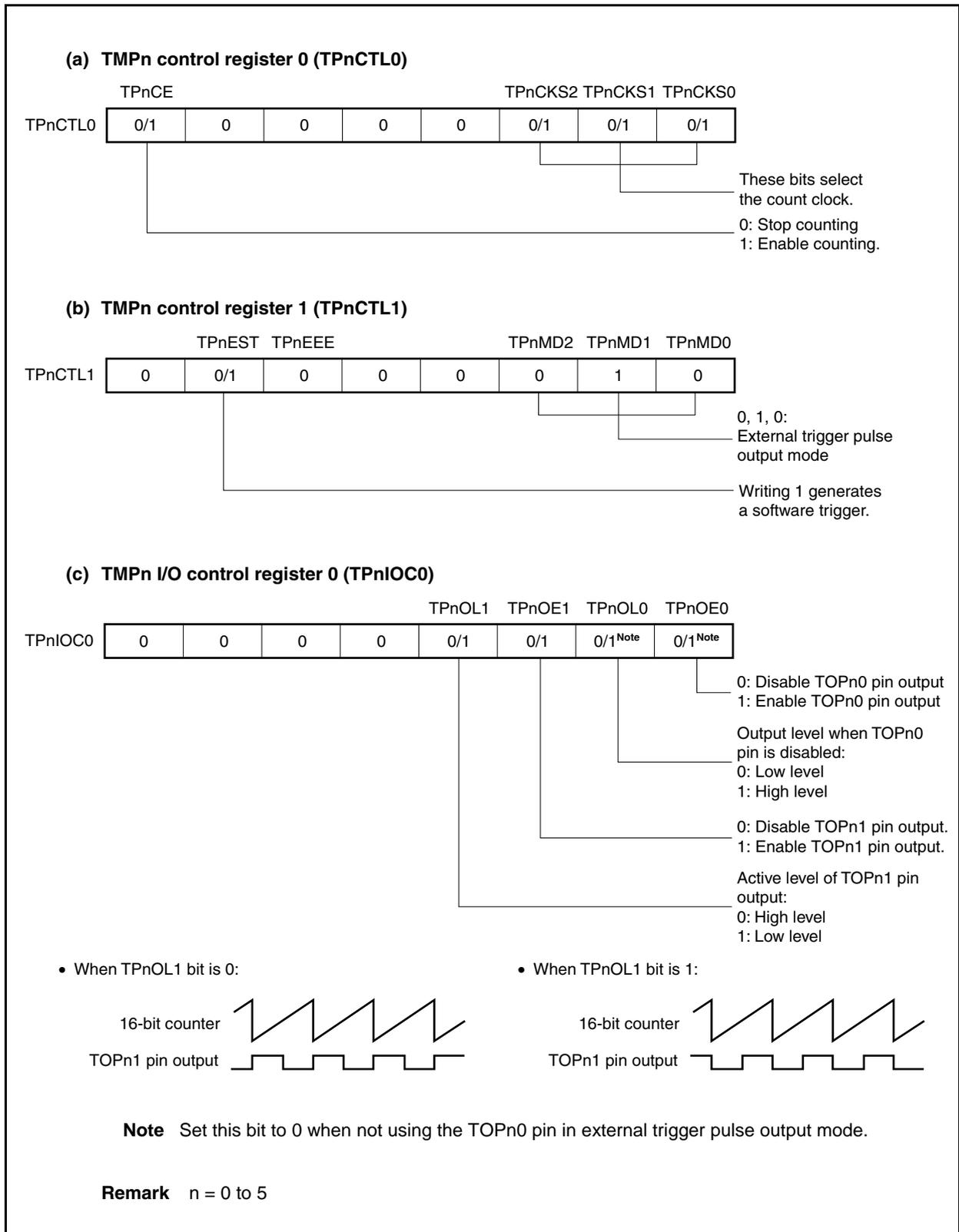
Figure 7-28. Register Settings in External Trigger Pulse Output Mode (2/2)
