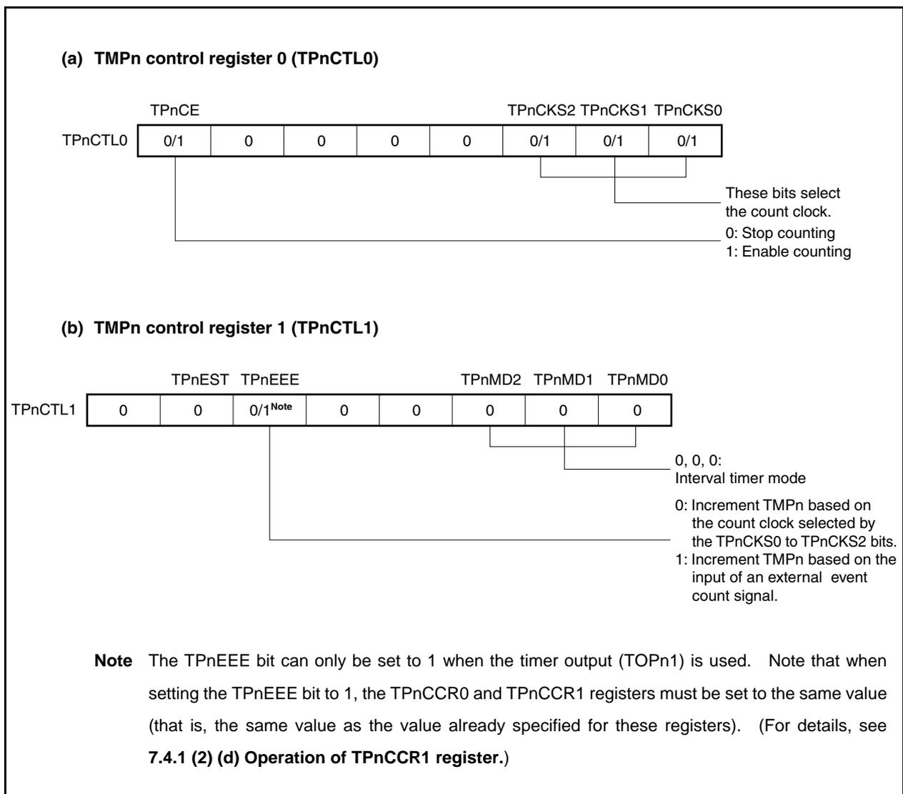
Figure 7-8. Register Settings in Interval Timer Mode (2/2)
