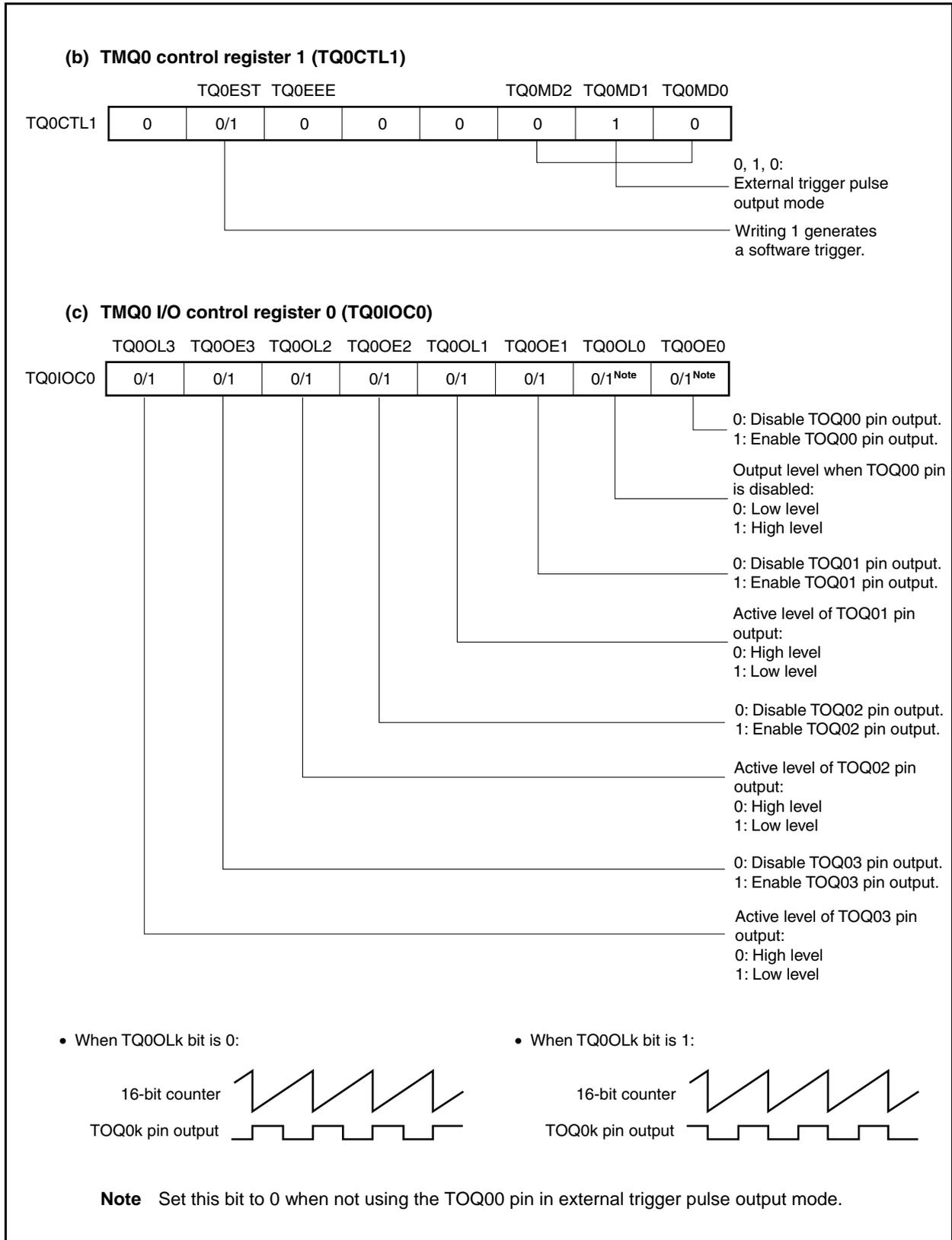
Figure 8-28. Register Settings in External Trigger Pulse Output Mode (3/3)
