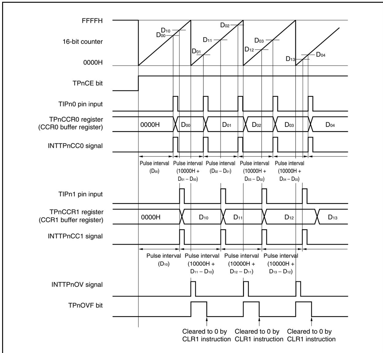
When executing pulse width measurement in the free-running timer mode, two pulse widths can be measured for one channel.
