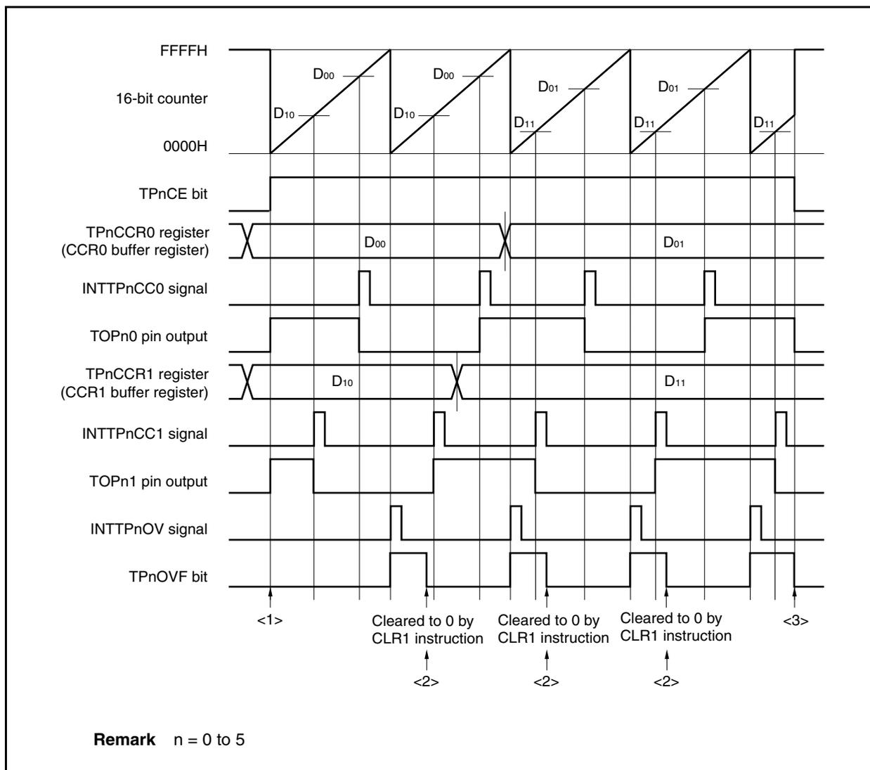
Figure 7-56. Timing and Processing of Operations in Free-Running Timer Mode (Compare Function) (2/2)
