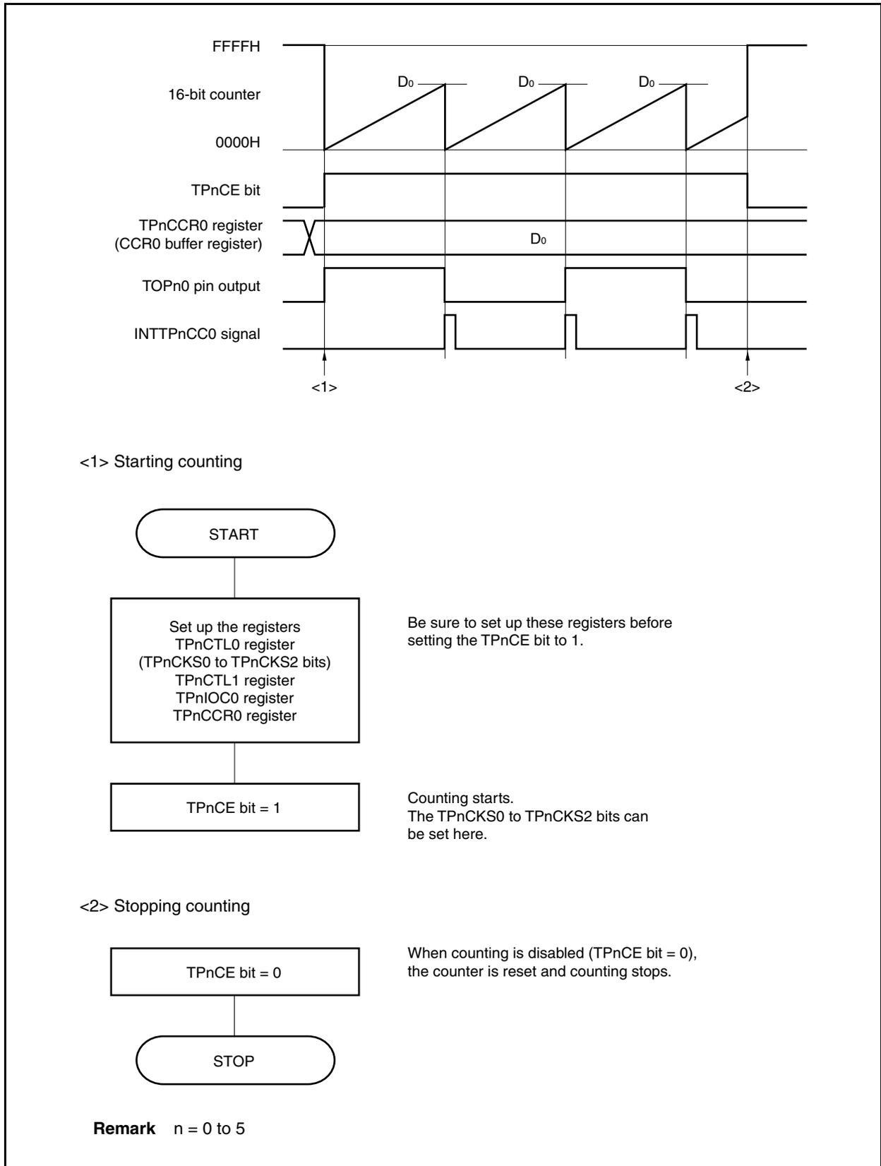
**(2) Using interval timer mode****(a) Operation when TPnCCR0 register is set to 0000H**
