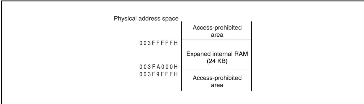
The initial settings for the expanded internal RAM are shown below.
