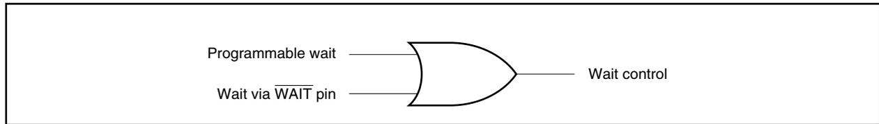
For example, if the timing of the programmable wait and the  $\overline{\text{WAIT}}$  pin signal is as shown in the Figure 5-4, three wait states will be inserted in the bus cycle. If wait insertion is controlled by the  $\overline{\text{WAIT}}$  pin, wait states might not be inserted at the expected timing. In this case, adjust the insertion timing by specifying a programmable wait value.
