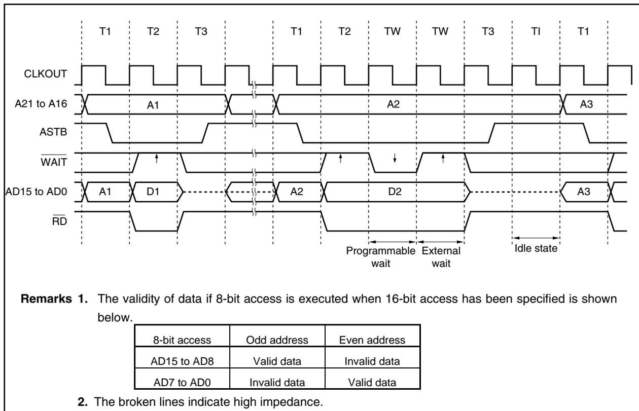
Figure 5-6. Multiplexed Bus Read Timing (Bus Size: 8 Bits)
