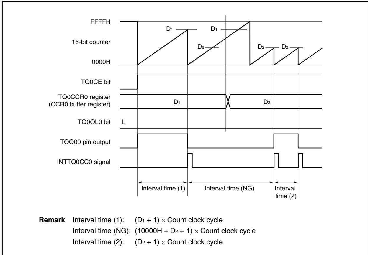
If the value of the TQ0CCR0 register is changed from  $D_1$  to  $D_2$  while the counter value is greater than  $D_2$  but less than  $D_1$ , the TQ0CCR0 register value is transferred to the CCR0 buffer register as soon as the register has been rewritten. Consequently, the value that is compared with the 16-bit counter value is  $D_2$ .
