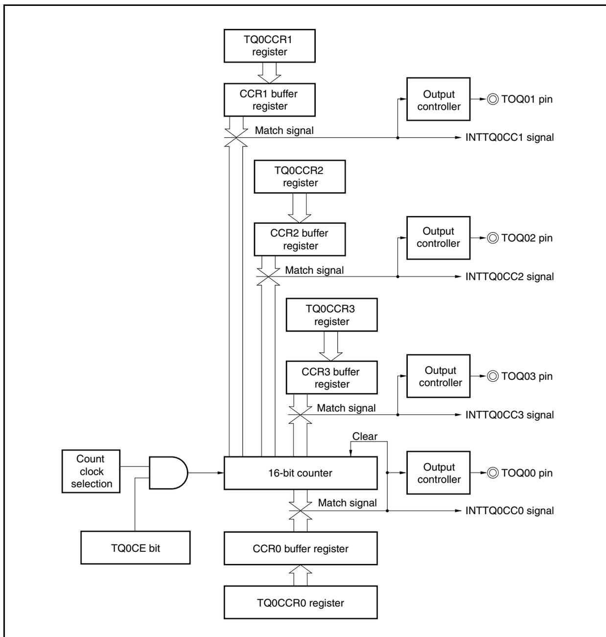
If the value of the TQ0CCRk register is less than or equal to the value of the TQ0CCR0 register, the INTTQ0CCk signal is generated once per cycle. At the same time, the output of the TOQ0k pin is inverted.
