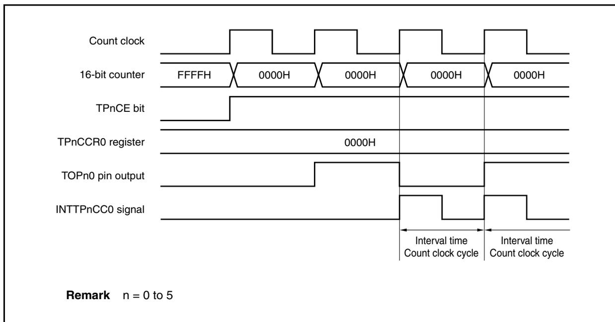
**(b) Operation when TPnCCR0 register is set to FFFFH**
