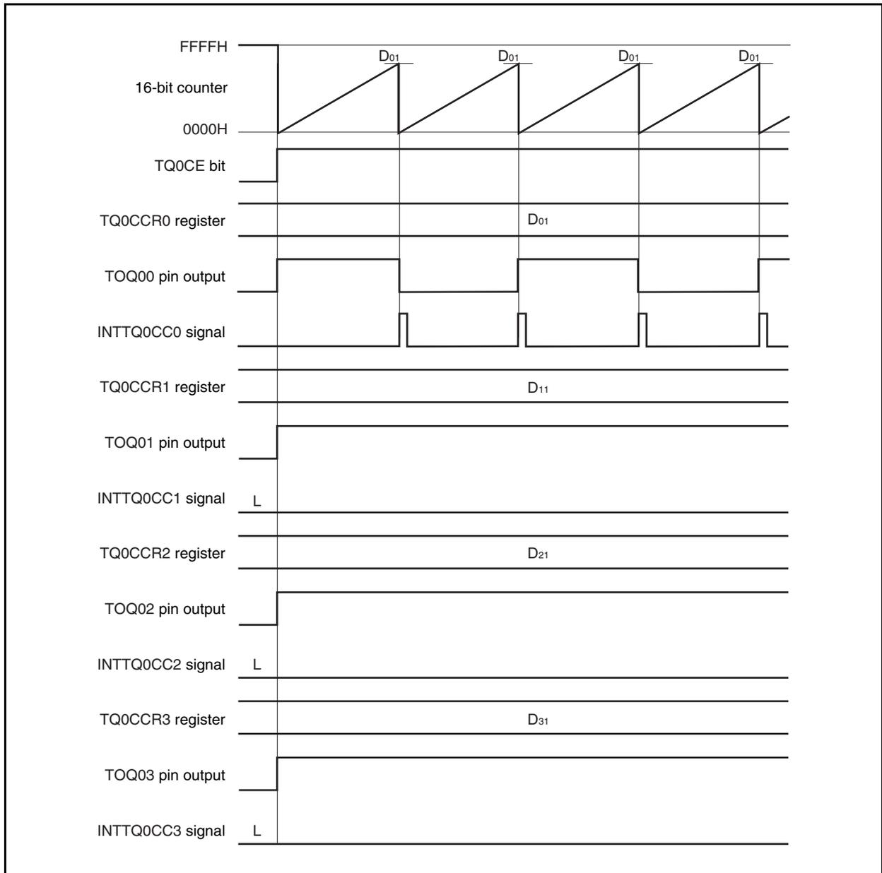
(3) Operation of interval timer based on input of external event count
