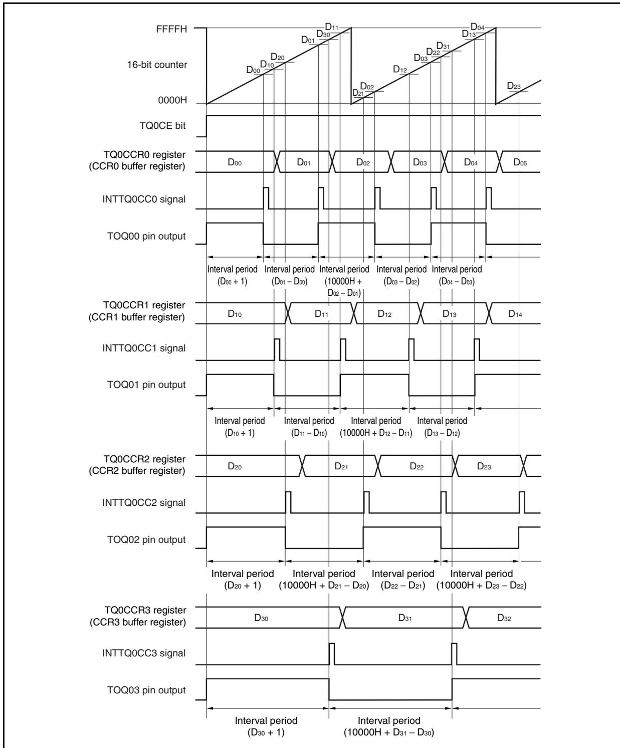
When performing an interval operation in the free-running timer mode, four intervals can be set for one channel.
