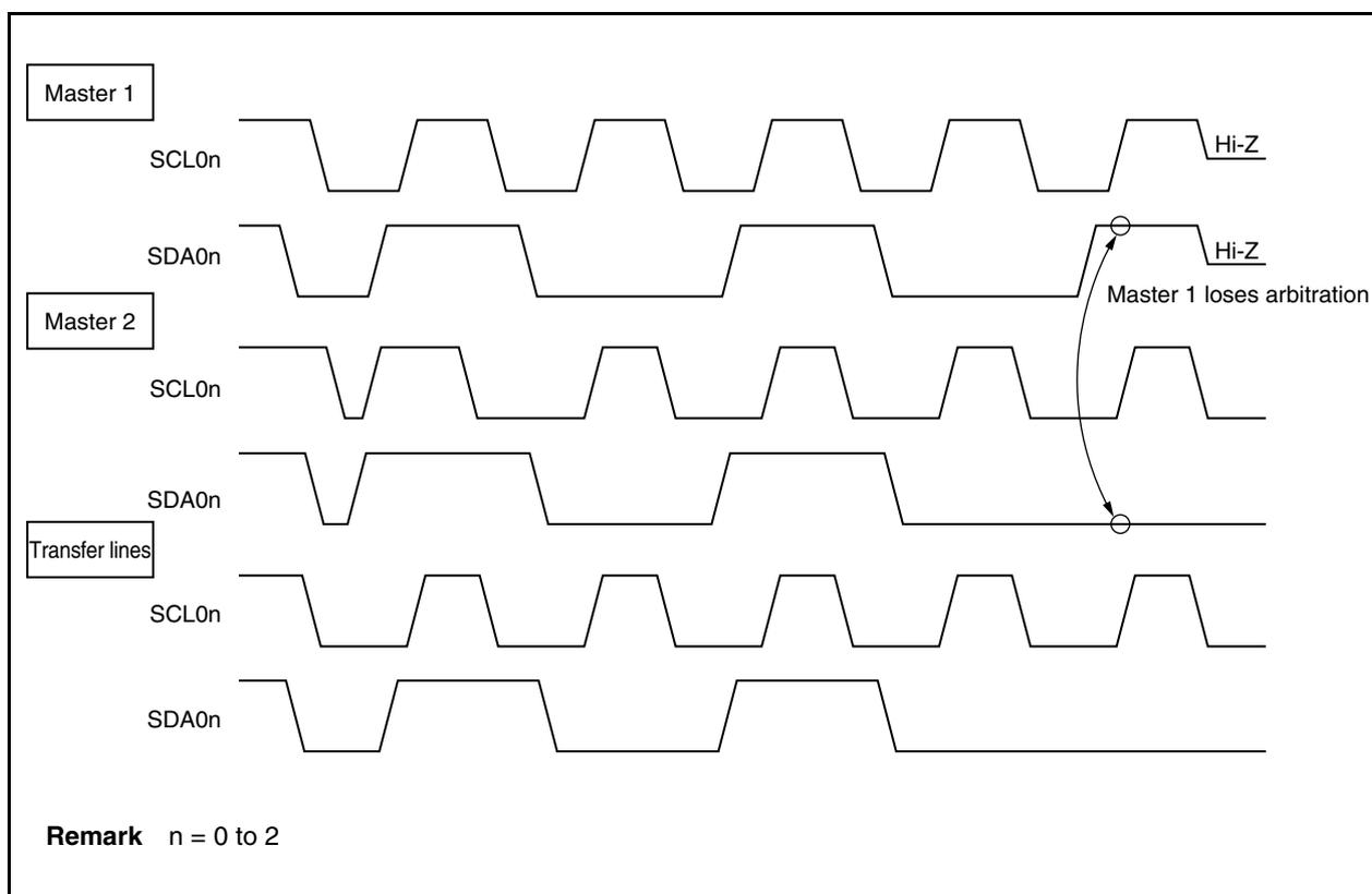
**Table 19-5. Status During Arbitration and Interrupt Request Signal Generation Timing**
