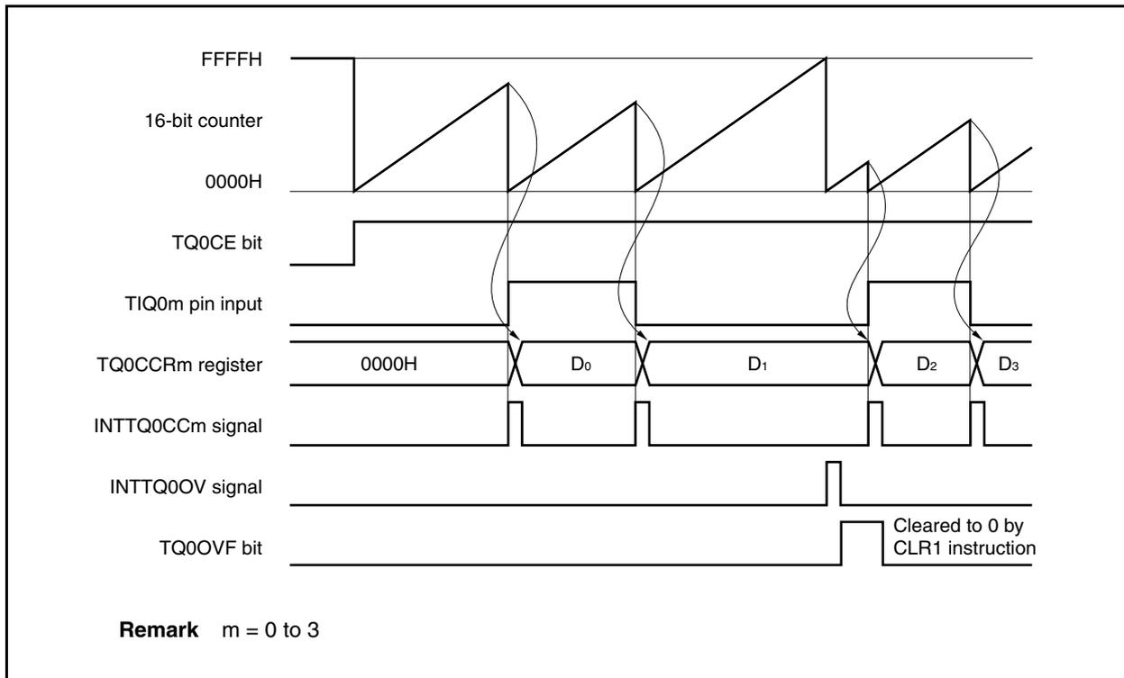
When the TQ0CE bit is set to 1, the 16-bit counter starts incrementing. When it is subsequently detected that a valid edge has been input to the TIQ0m pin, the value of the 16-bit counter is stored in the TQ0CCRm register, the 16-bit counter is cleared to 0000H, and a capture interrupt request signal (INTTQ0CCm) is generated.
