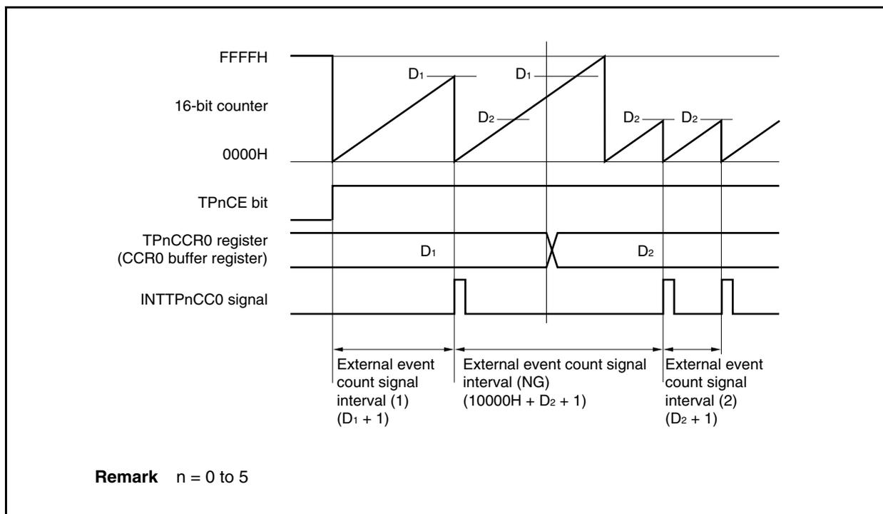
If the value of the TPnCCR0 register is changed from  $D_1$  to  $D_2$  while the counter value is greater than  $D_2$  but less than  $D_1$ , the TPnCCR0 register value is transferred to the CCR0 buffer register as soon as the register has been rewritten. Consequently, the value that is compared with the 16-bit counter value is  $D_2$ .
