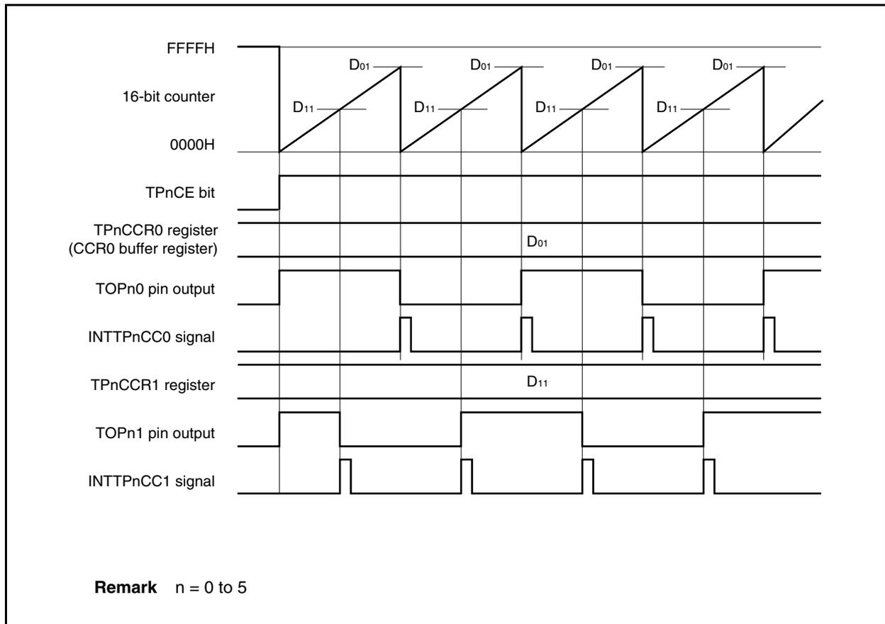
If the value of the TPnCCR1 register is greater than the value of the TPnCCR0 register, the value of the 16-bit counter will not match the value of the TPnCCR1 register. Consequently, the INTTPnCC1 signal is not generated, nor is the output of the TOPn1 pin changed.
