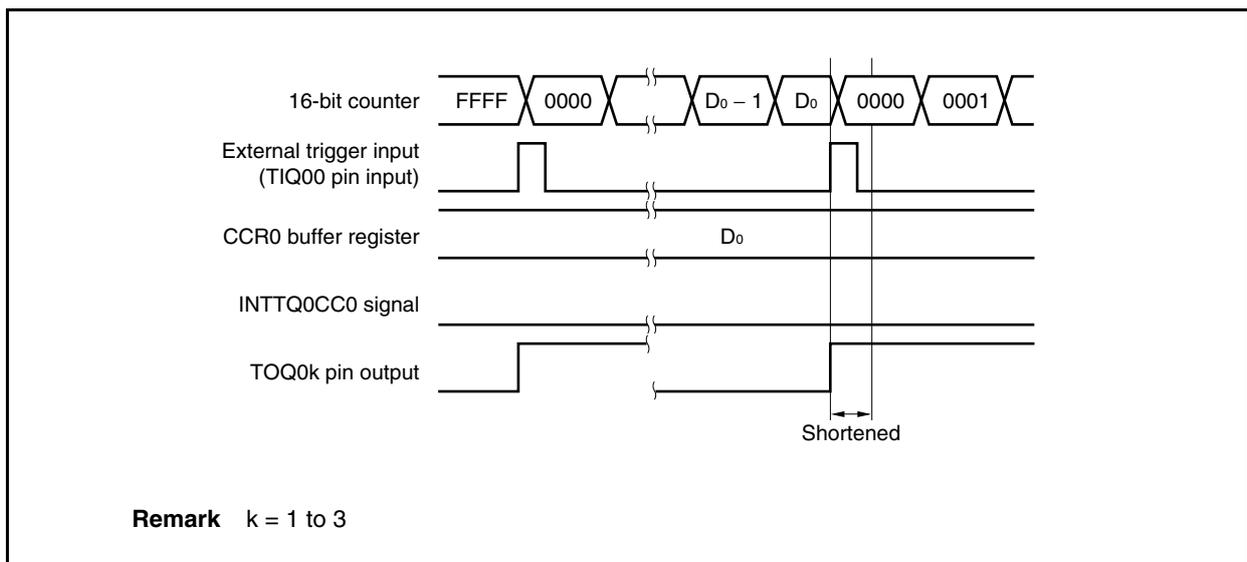
**(e) Timing of generating the compare match interrupt request signal (INTTQ0CCK)**
