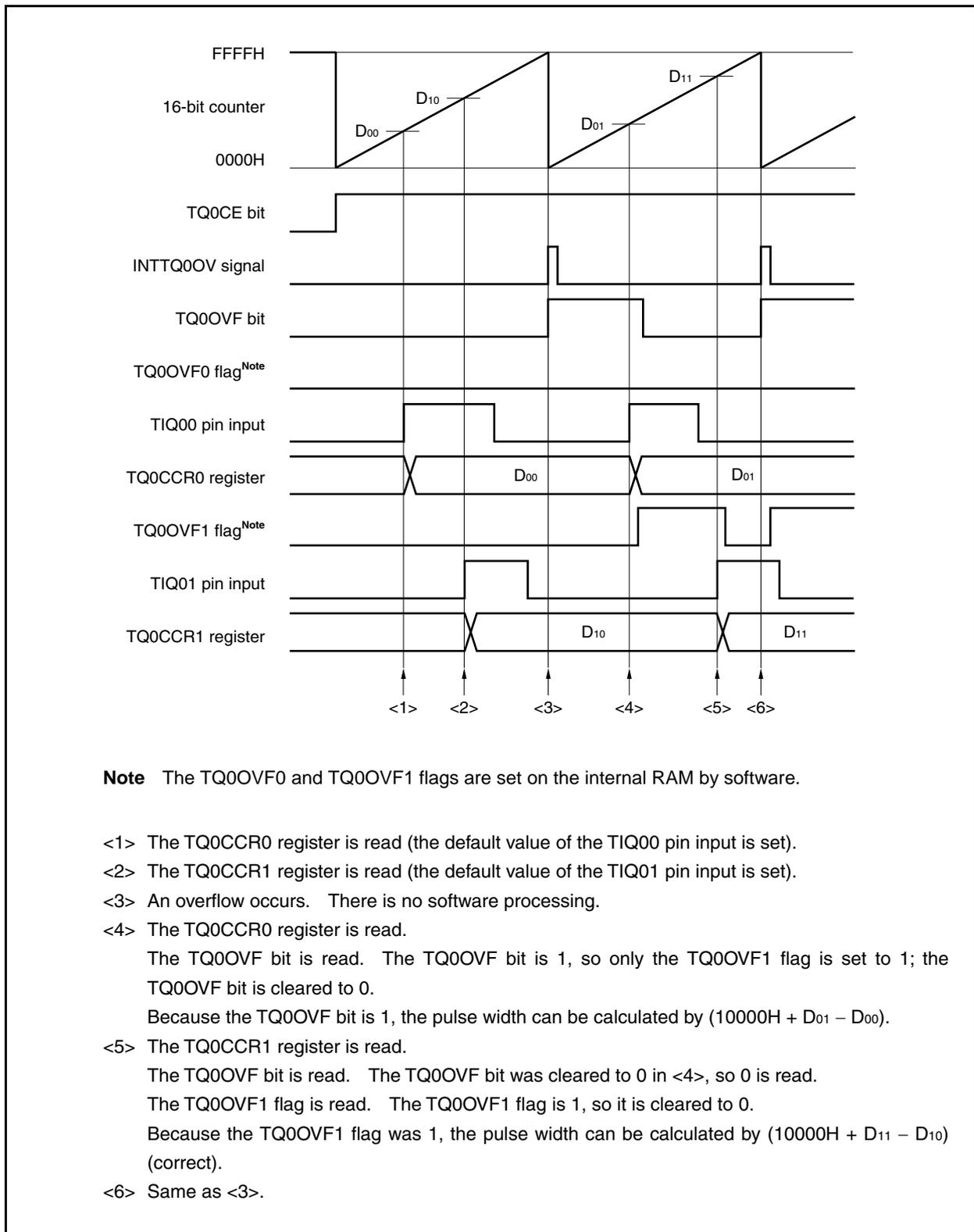
**(d) Processing of overflow if capture trigger interval is long**
