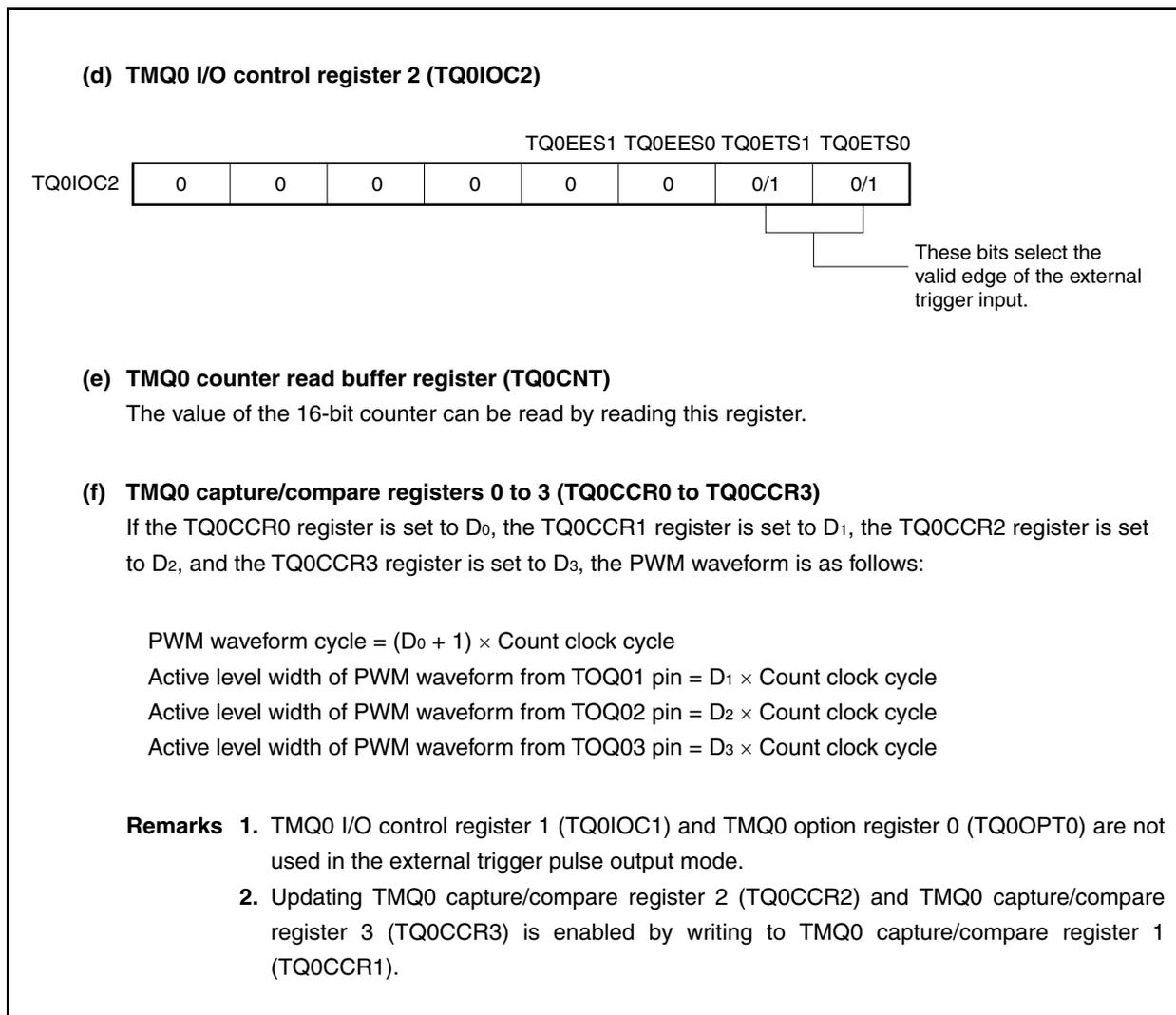
(1) Operations in external trigger pulse output mode
