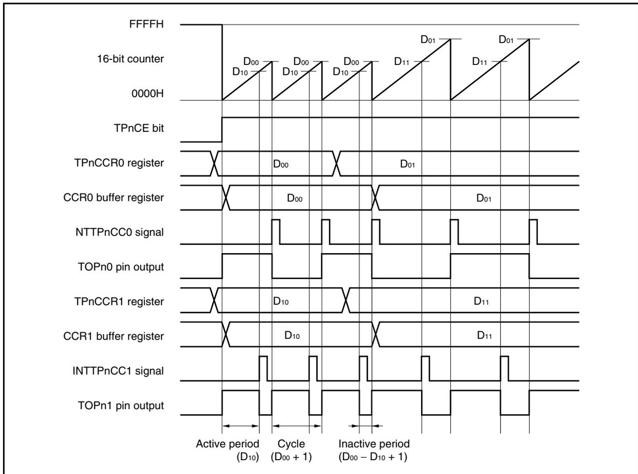
When the TPnCE bit is set to 1, the 16-bit counter is cleared from FFFFH to 0000H, starts incrementing, and outputs a PWM waveform from the TOPn1 pin.
