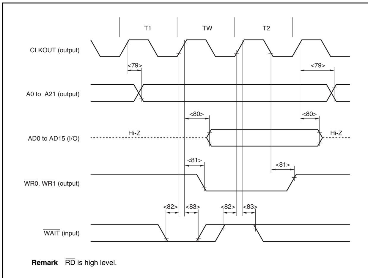
**(3) Bus hold****(a) Asynchronous to CLKOUT**
