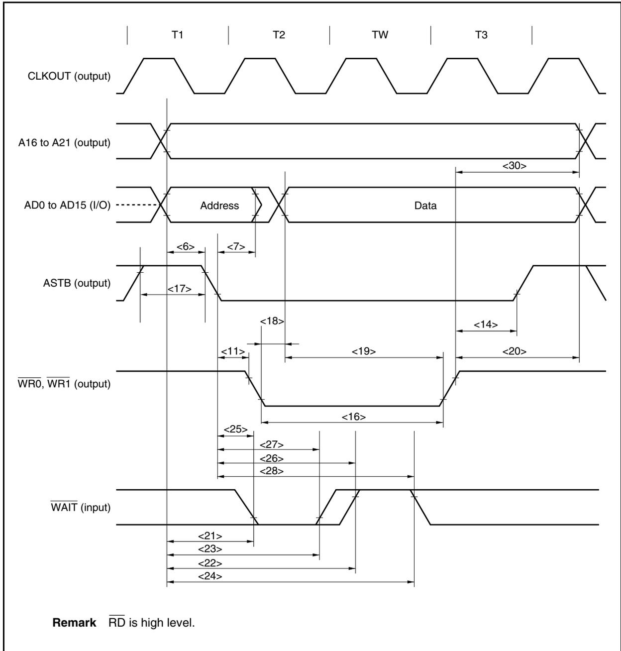
**(b) Read/write cycle (Synchronous with CLKOUT): In multiplexed bus mode**
