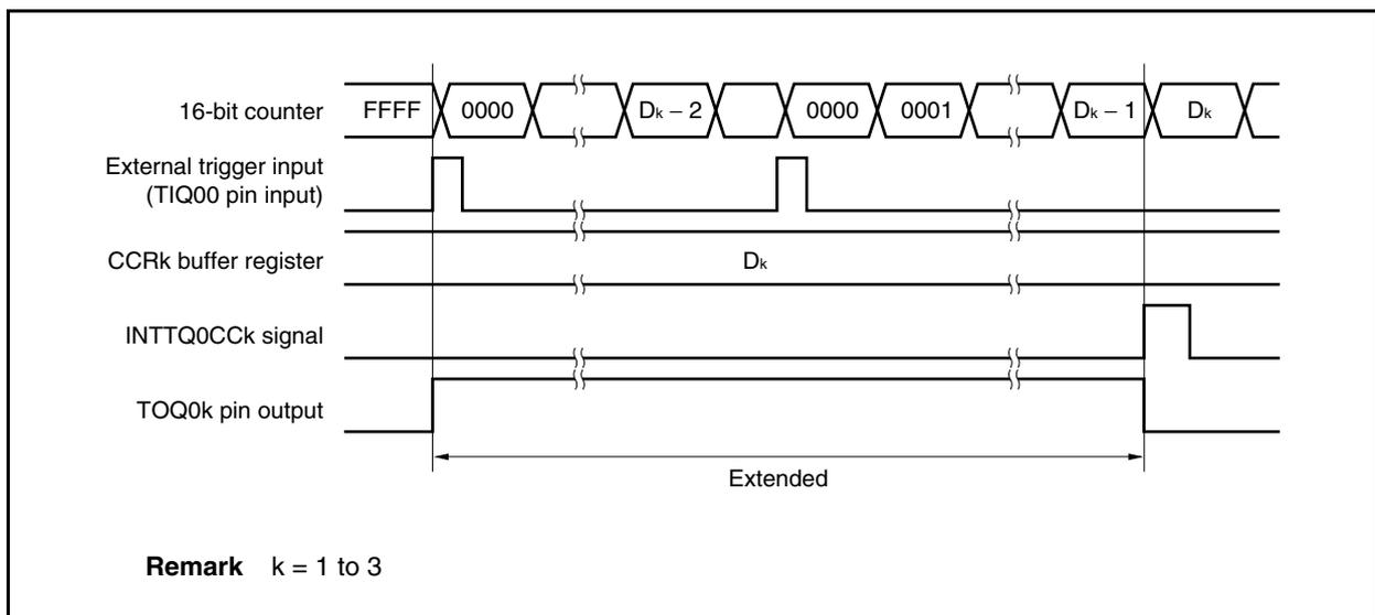
**(d) Detection of trigger immediately before or after INTTQ0CC0 generation**
