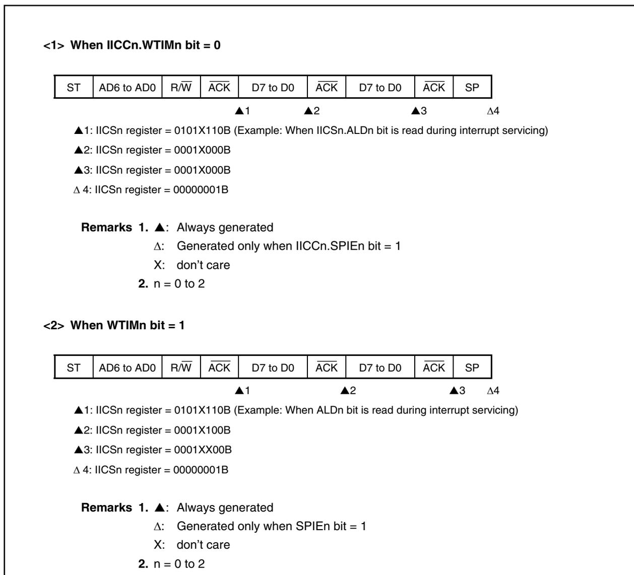
**(2) When arbitration loss occurs during transmission of extension code****<1> When WTIMn bit = 0**
