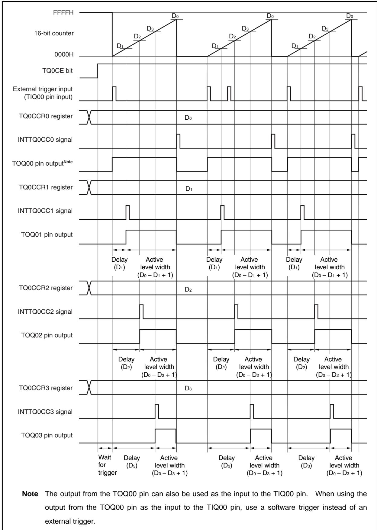
When the TQ0CE bit is set to 1, TMQ0 waits for a trigger. When the trigger is generated, the 16-bit counter is cleared from FFFFH to 0000H, starts incrementing, and outputs a one-shot pulse from the TOQ0k pin. After the one-shot pulse is output, the 16-bit counter is set to 0000H, stops incrementing, and waits for a trigger. If a trigger is generated again while the one-shot pulse is being output, it is ignored.
