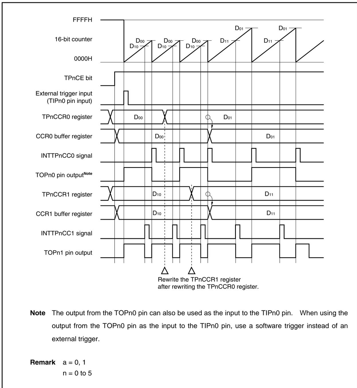
In order to transfer data from the TPnCCRa register to the CCRa buffer register, the TPnCCR1 register must be written.
