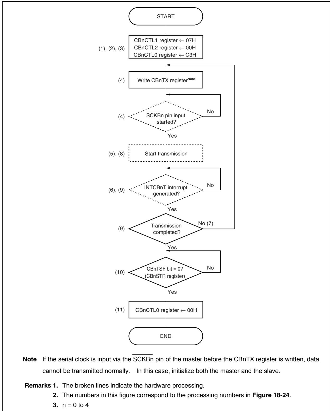
**Note** If the serial clock is input via the  $\overline{\text{SCKBn}}$  pin of the master before the CBnTX register is written, data cannot be transmitted normally. In this case, initialize both the master and the slave.
