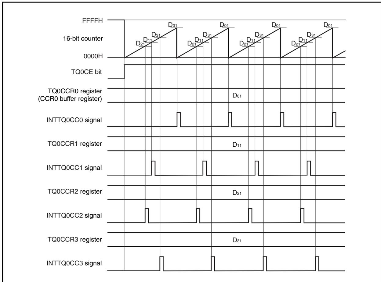
If the value of the TQ0CCRk register is greater than the value of the TQ0CCR0 register, the value of the 16-bit counter will not match the value of the TQ0CCRk register and the INTTQ0CCk signal will not be generated.
