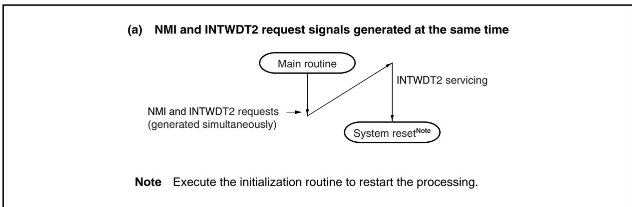
Figure 21-1. Non-Maskable Interrupt Request Signal Acknowledgment Operation (2/2)
