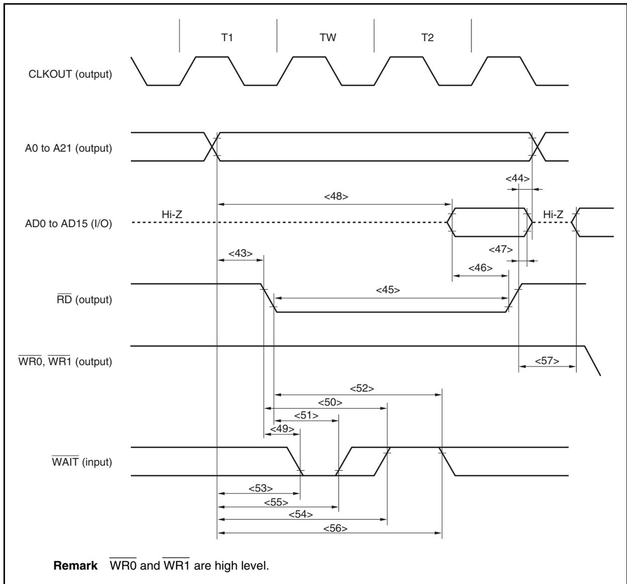
**(b) Write cycle (Asynchronous to CLKOUT): In separate bus mode**
