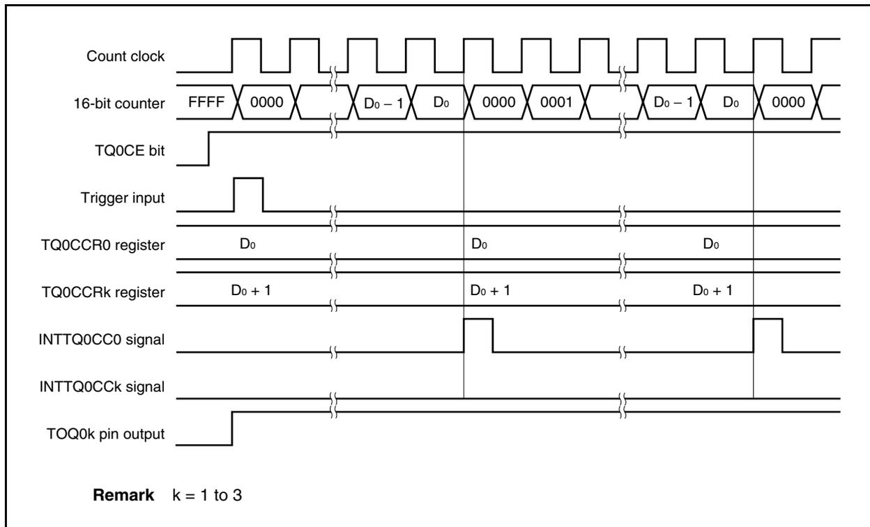
**(c) Detection of trigger immediately before or after INTTQ0CCK generation**
