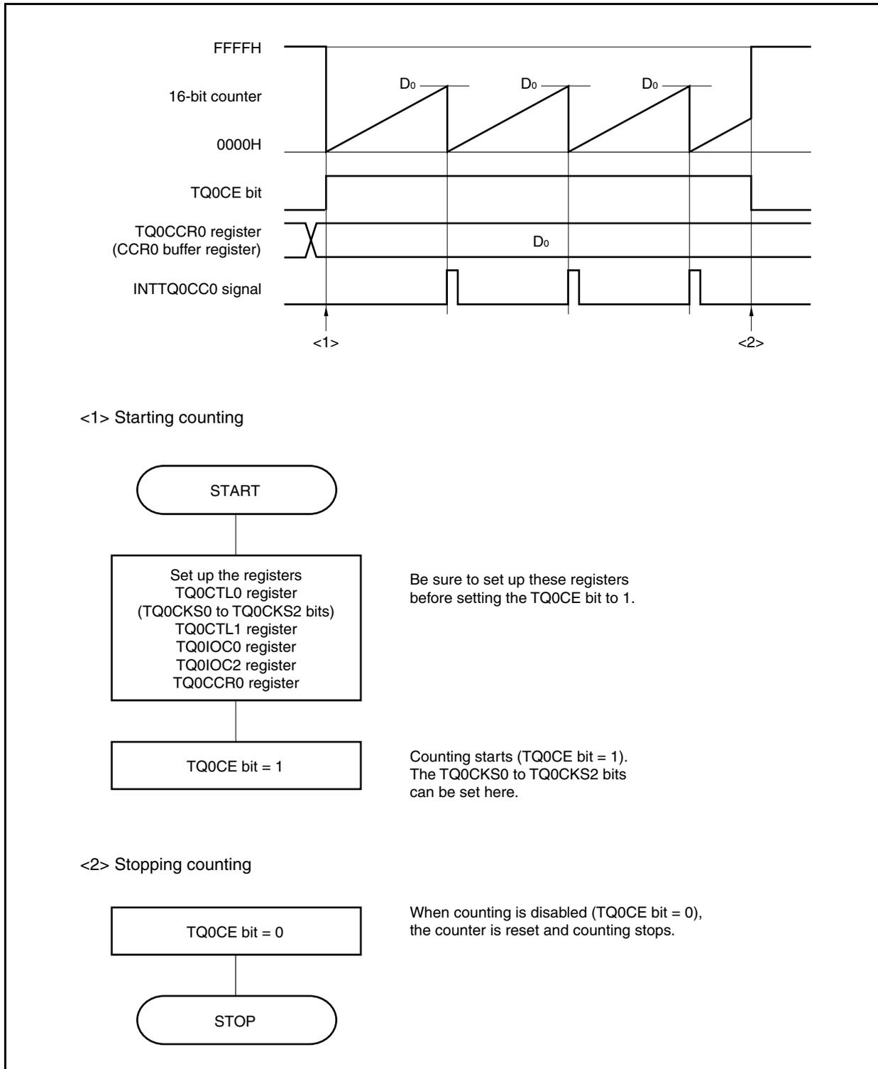
**(2) Using external event count mode****(a) Operation when TQ0CCR0 register is set to FFFFH**
