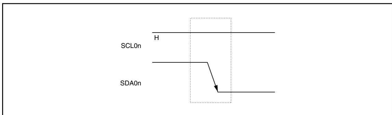
A start condition is output when the IICn.STTn bit is set (1) after a stop condition has been detected (IICn.SPDn bit = 1). When a start condition is detected, the IICn.STDn bit is set (1) ( $n = 0$  to 2).
