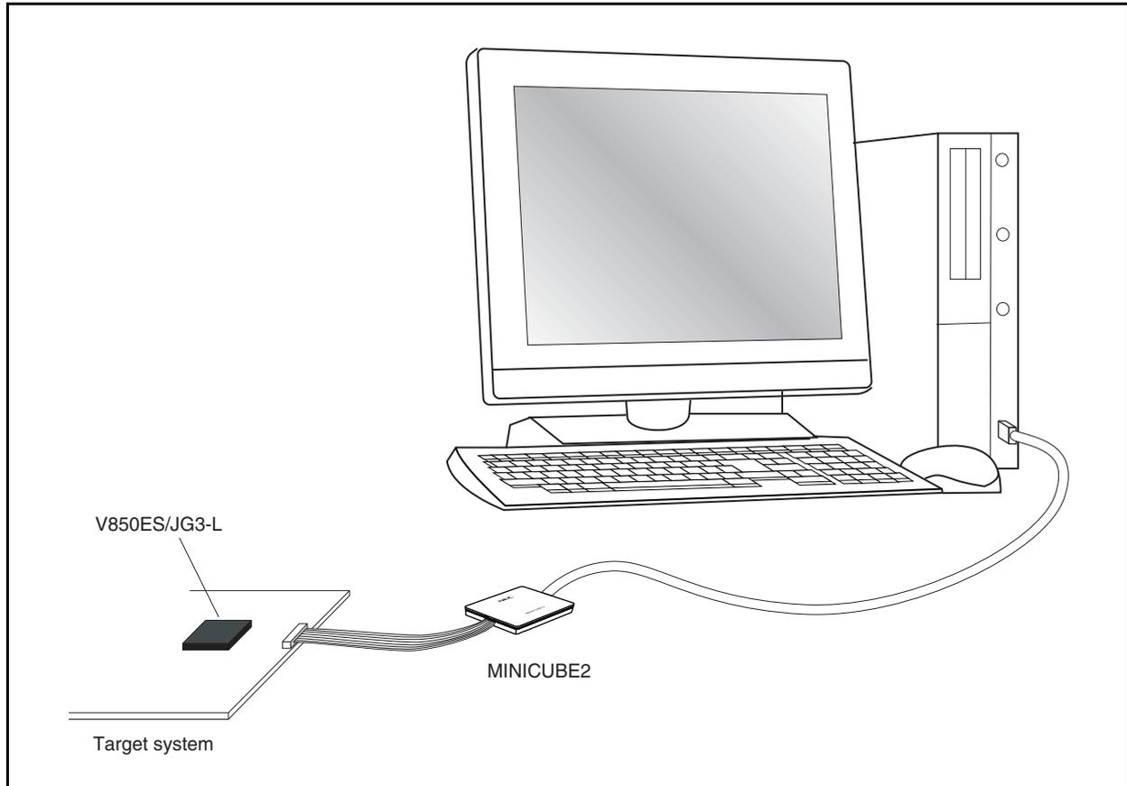
On-chip debugging can be performed for the V850ES/JG3-L by using the following two methods.
