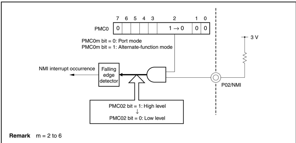
(2) In port mode, the PFn.PFn<sub>m</sub> bit is valid only in the output mode (PMn.PMn<sub>m</sub> bit = 0). In the input mode (PMn<sub>m</sub> bit = 1), the value of the PFn<sub>m</sub> bit is not reflected in the buffer.
