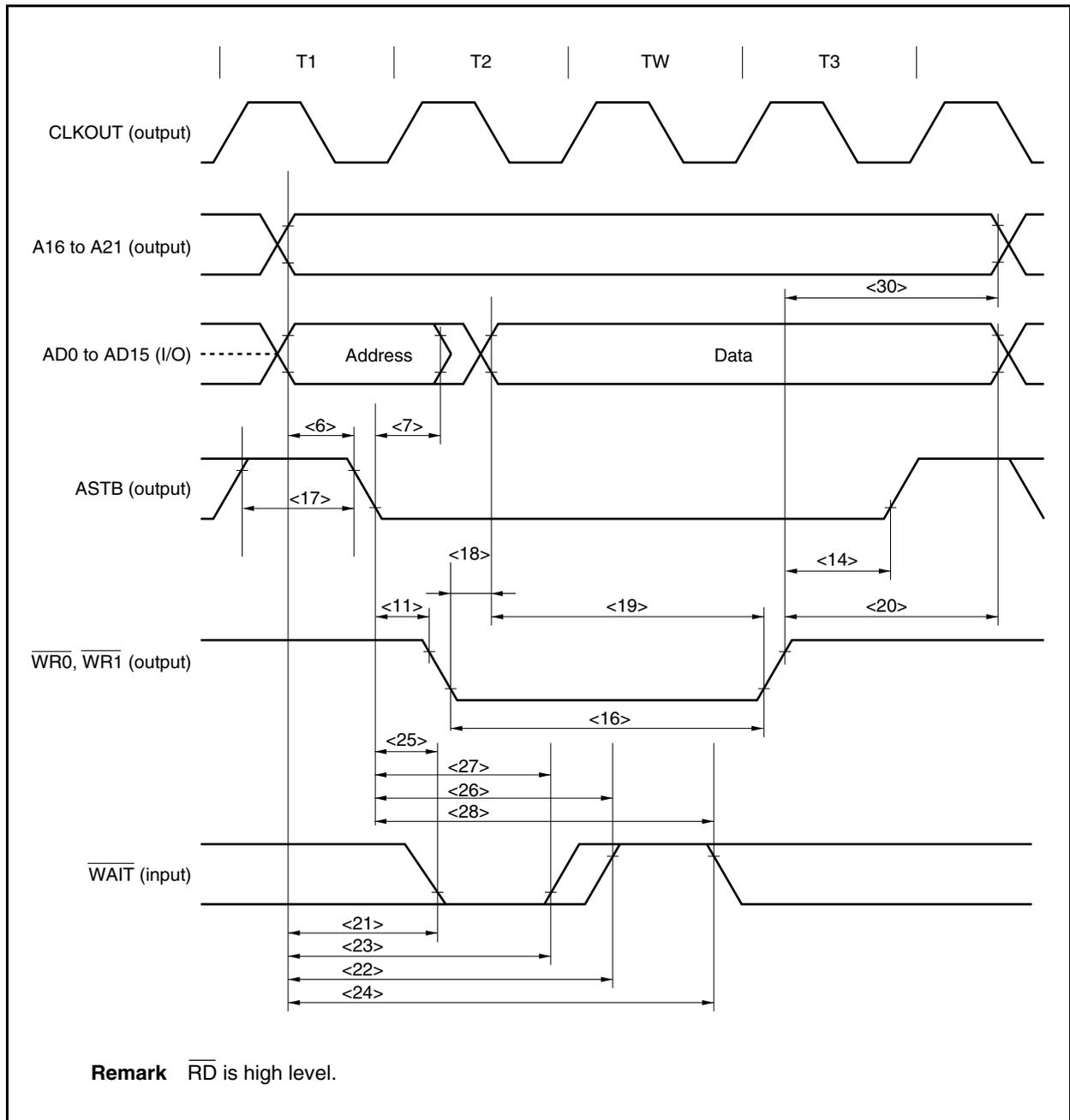
**(b) Read/write cycle (Synchronous with CLKOUT): In multiplexed bus mode****( $T_A = -40$  to  $+85^\circ\text{C}$ ,  $V_{DD} = EV_{DD} = AV_{REF0} = AV_{REF1} = 2.7$  to  $3.6$  V,  $V_{SS} = EV_{SS} = AV_{SS} = 0$  V,  $C_L = 50$  pF)**
