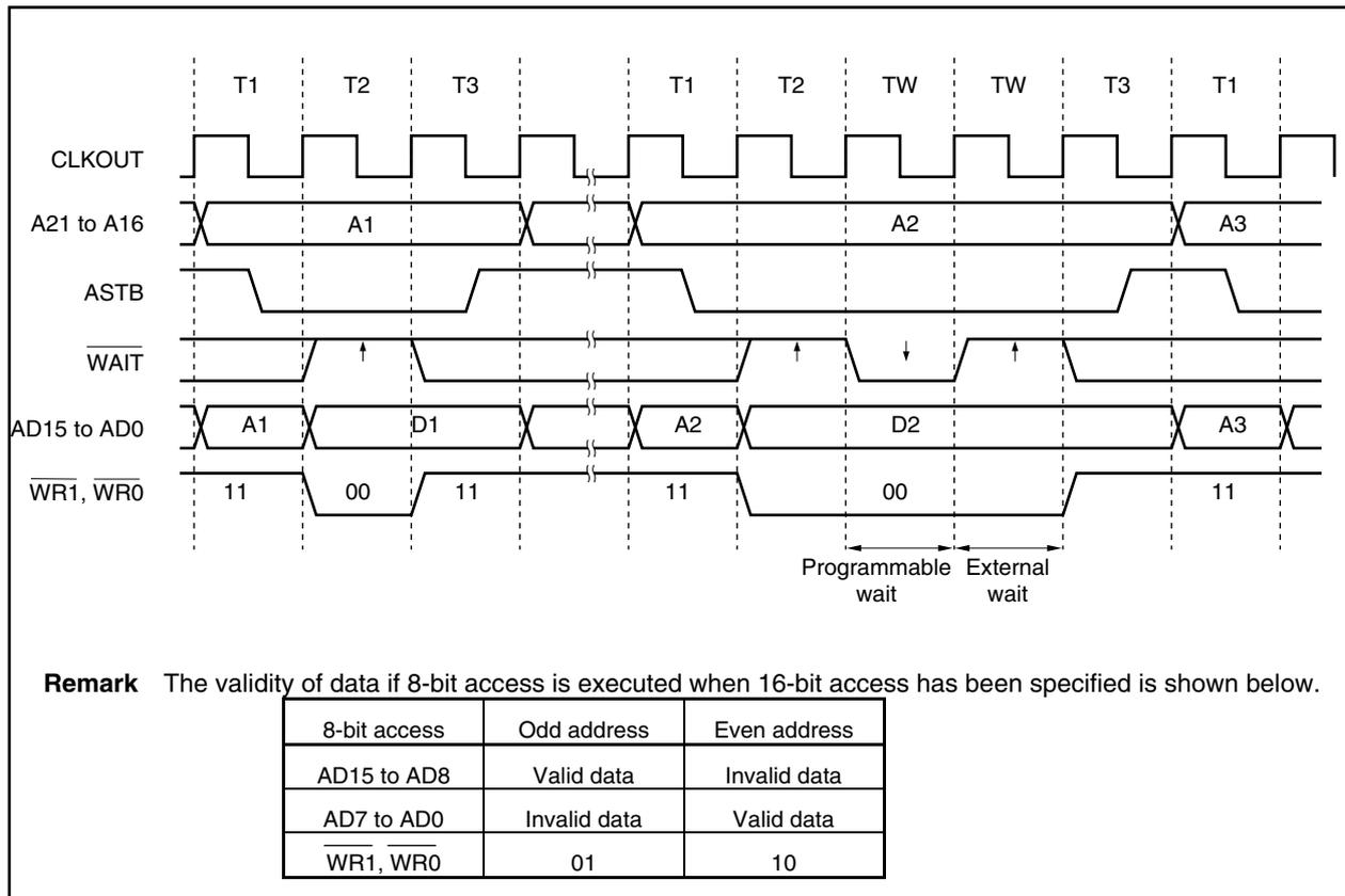
Figure 5-8. Multiplexed Bus Write Timing (Bus Size: 8 Bits)
