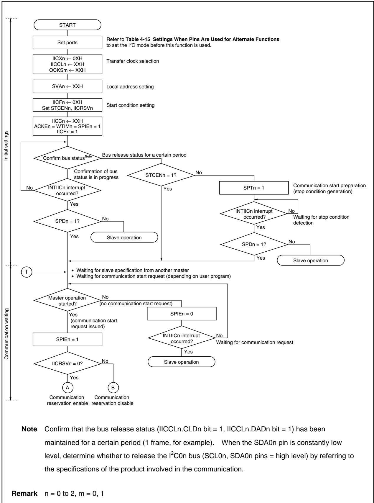
**Note** Confirm that the bus release status (IICCLn.CLDn bit = 1, IICCLn.DADn bit = 1) has been maintained for a certain period (1 frame, for example). When the SDA0n pin is constantly low level, determine whether to release the I<sup>2</sup>C0n bus (SCL0n, SDA0n pins = high level) by referring to the specifications of the product involved in the communication.
