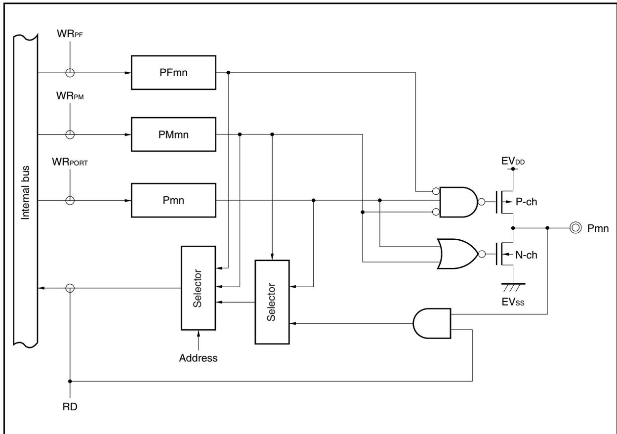
Figure 4-6. Block Diagram of Type D-1
