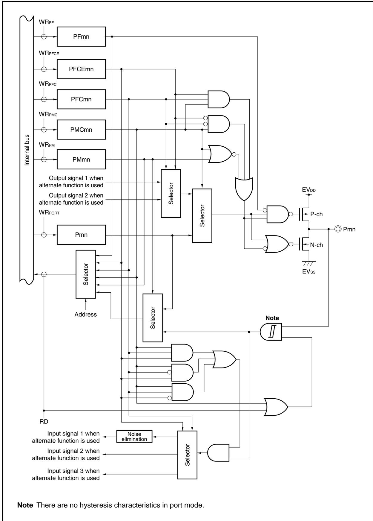
Figure 4-28. Block Diagram of Type U-12
