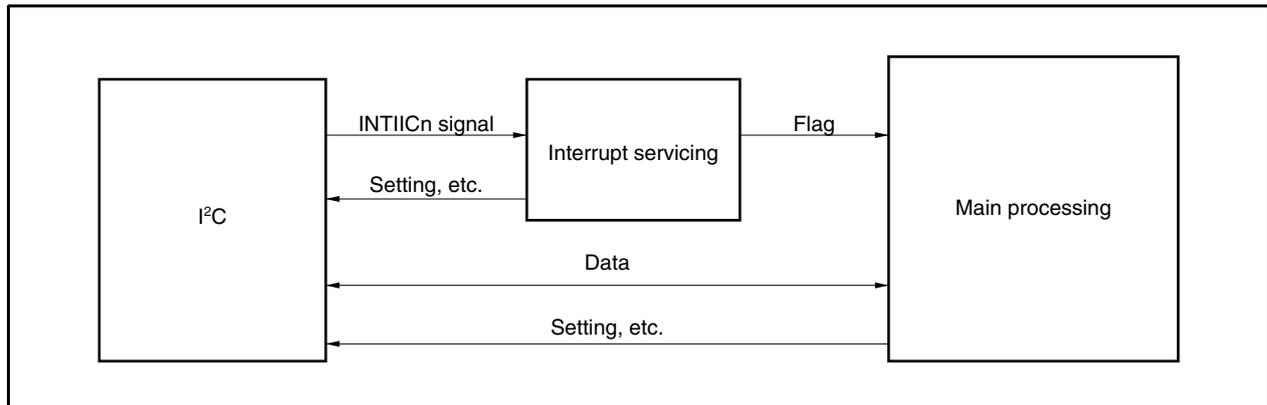
Therefore, the following three flags are prepared so that the data transfer processing can be performed by passing these flags to the main processing instead of INTIICn signal.
