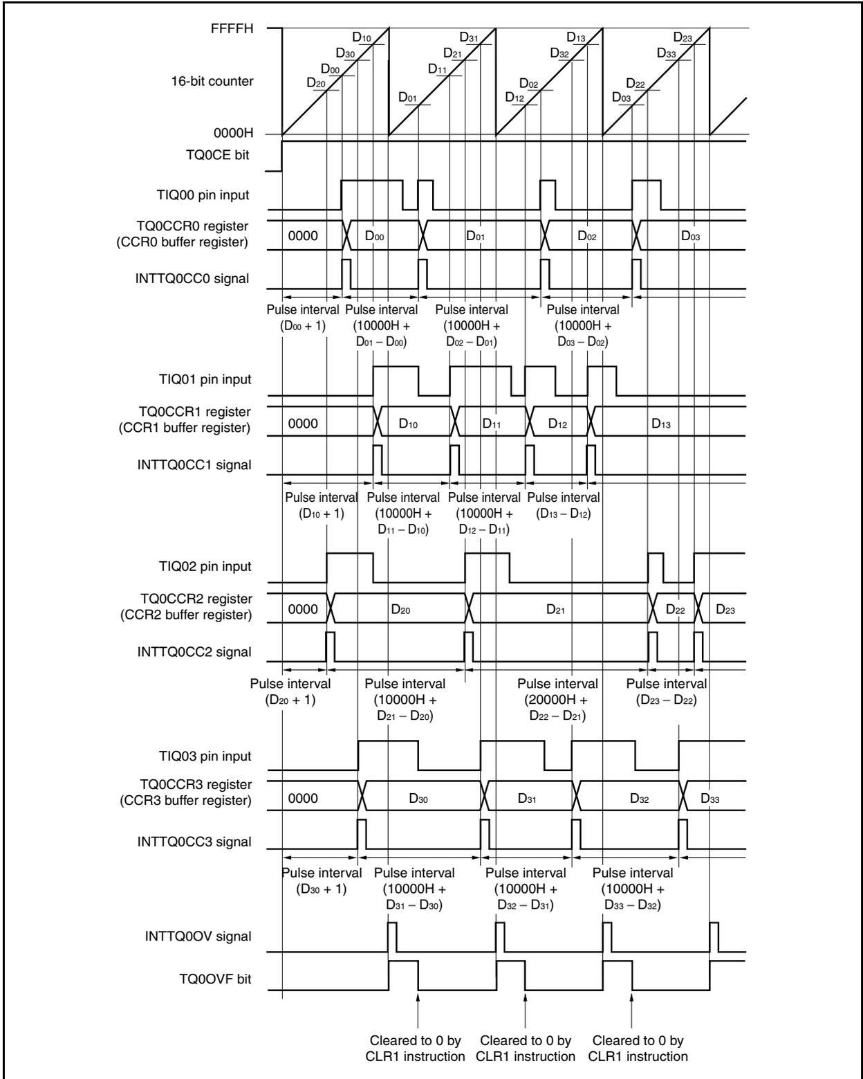
Four pulse widths can be measured in the free-running timer mode.
