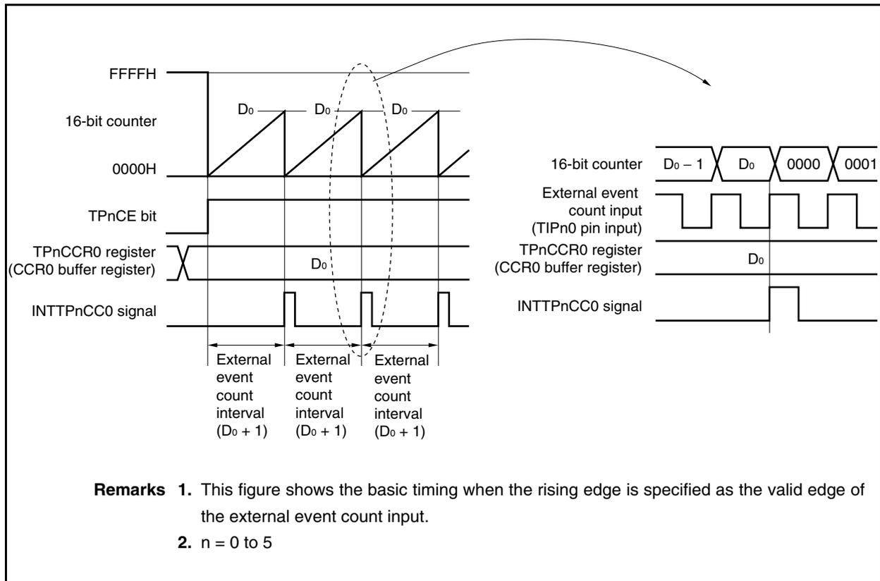
An example of the register settings when the external event count mode is used is shown in the figure below.
