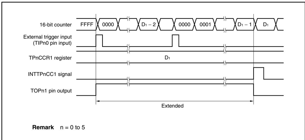
**(d) Detection of trigger immediately before or after INTTPnCC0 generation**
