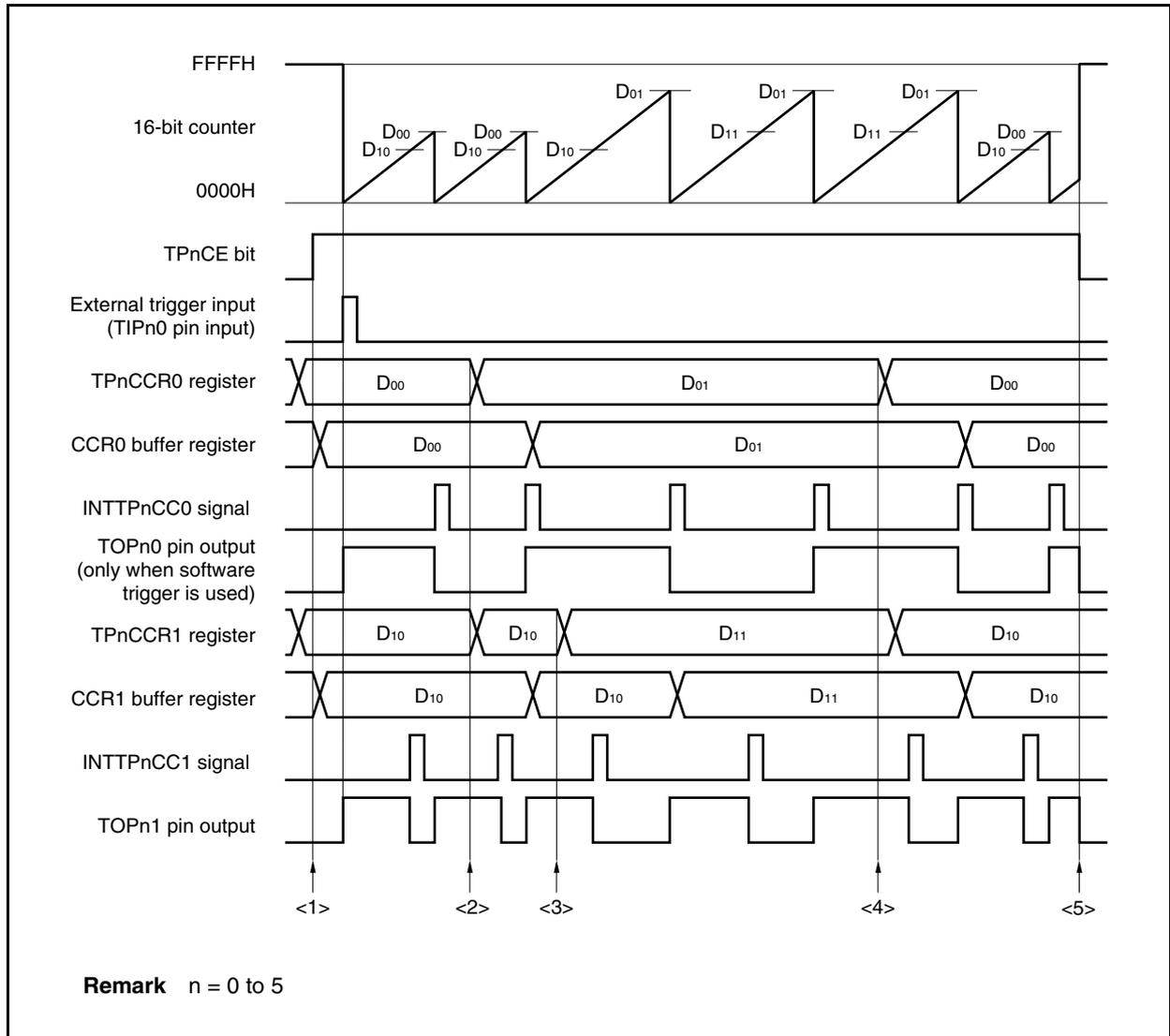
Figure 7-29. Timing and Processing of Operations in External Trigger Pulse Output Mode (2/2)
