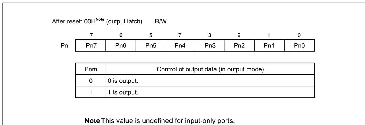
The operation when writing or reading the Pn register differs depending on the specified mode.
