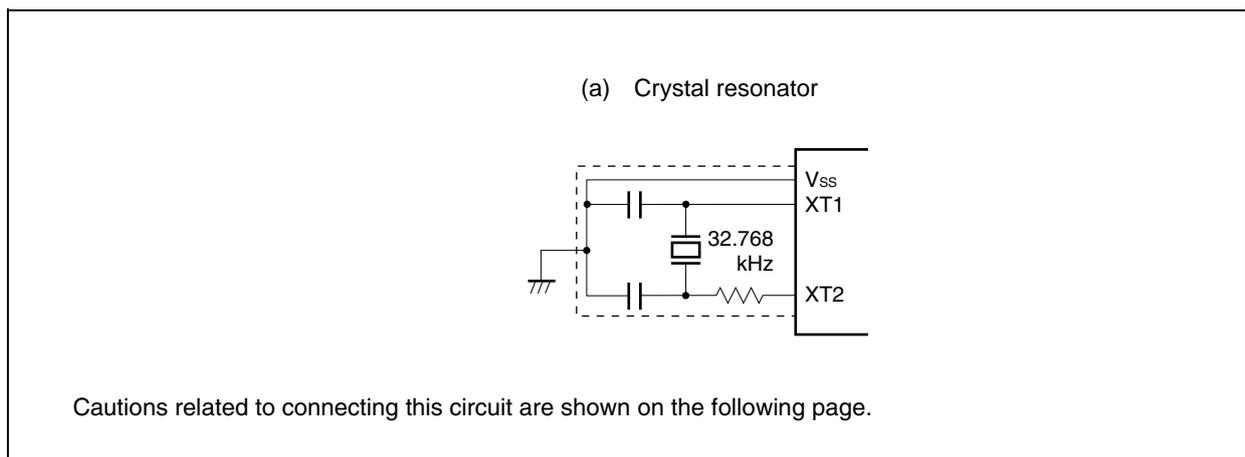
**Caution 1.** When using the main clock or subclock oscillator, wire as follows in the area enclosed by the broken lines in Figures 6-2 and 6-3 to avoid an adverse effect from wiring capacitance.
