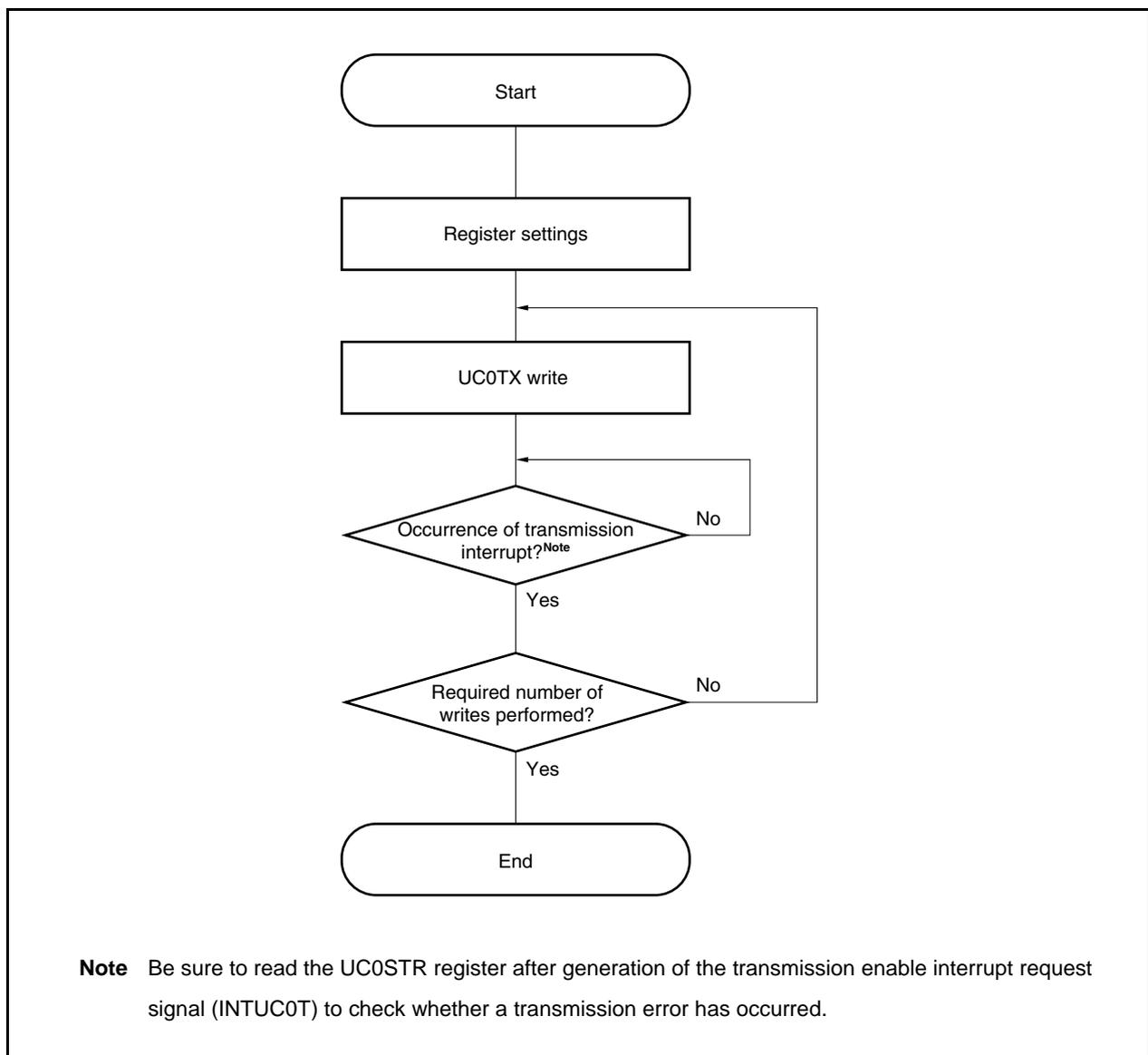
**Figure 17-6. Continuous Transmission Operation Timing**
