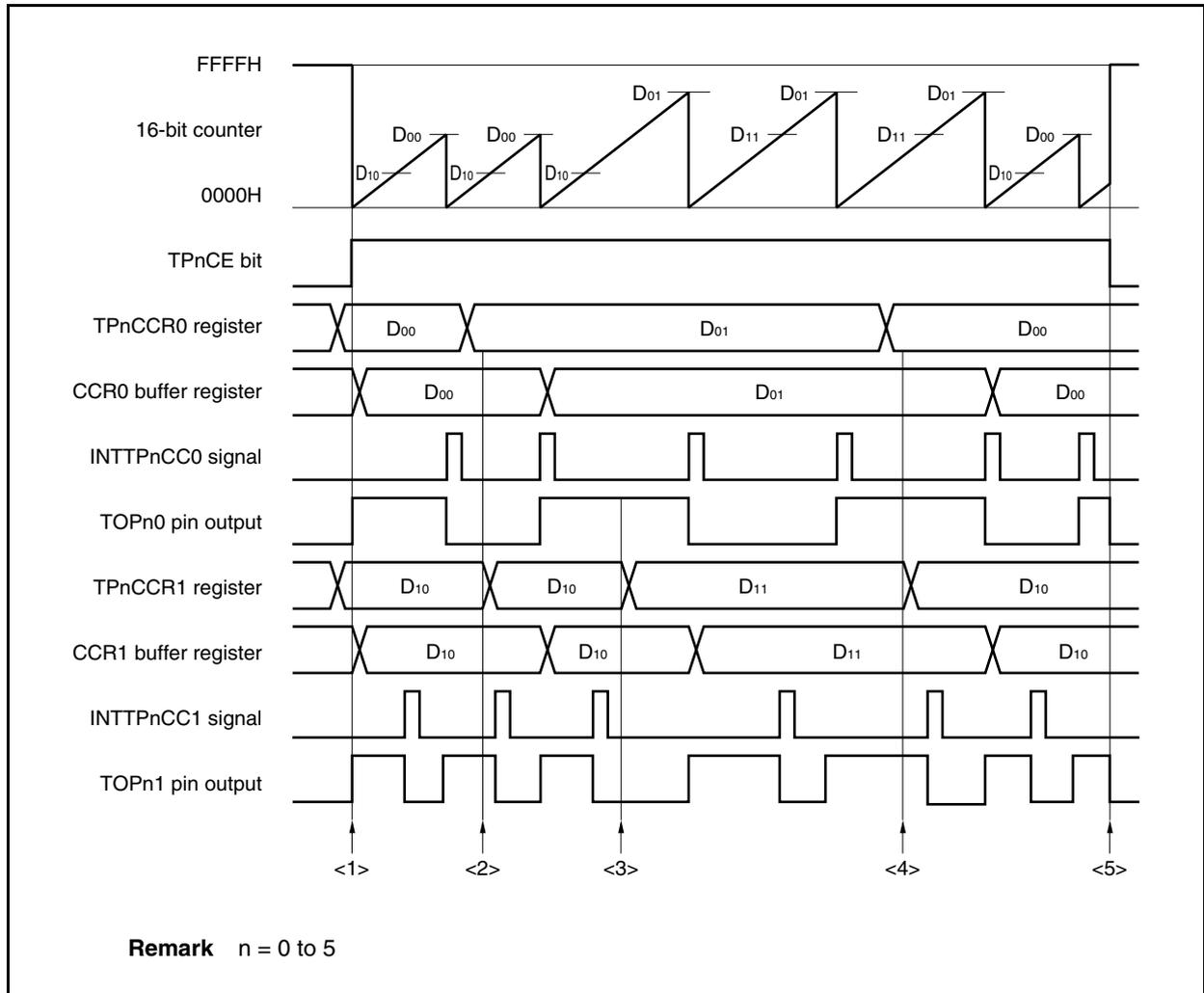
Figure 7-47. Timing and Processing of Operations in PWM Output Mode (2/2)
