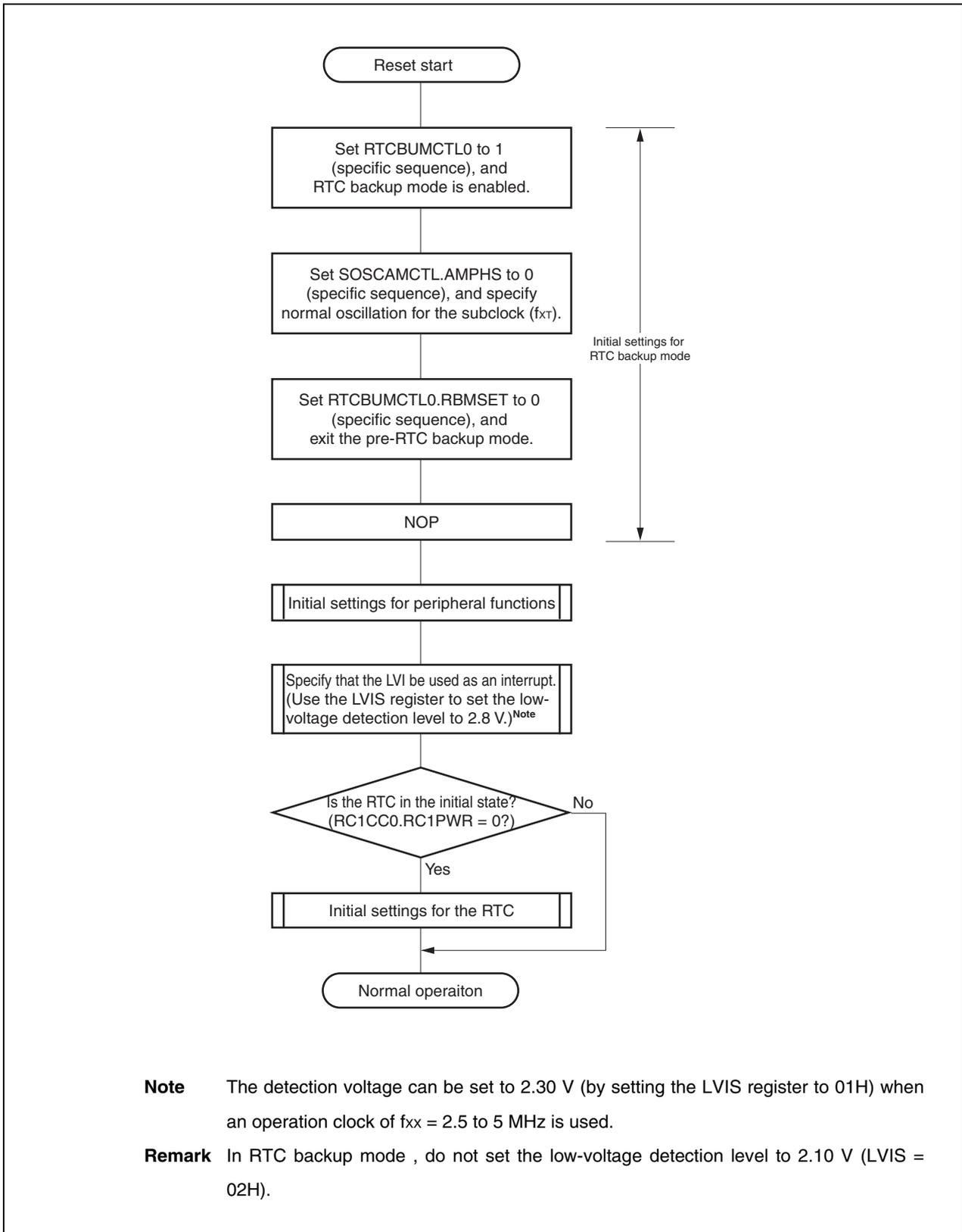
**Note** The detection voltage can be set to 2.30 V (by setting the LVIS register to 01H) when an operation clock of  $f_{xx} = 2.5$  to 5 MHz is used.
