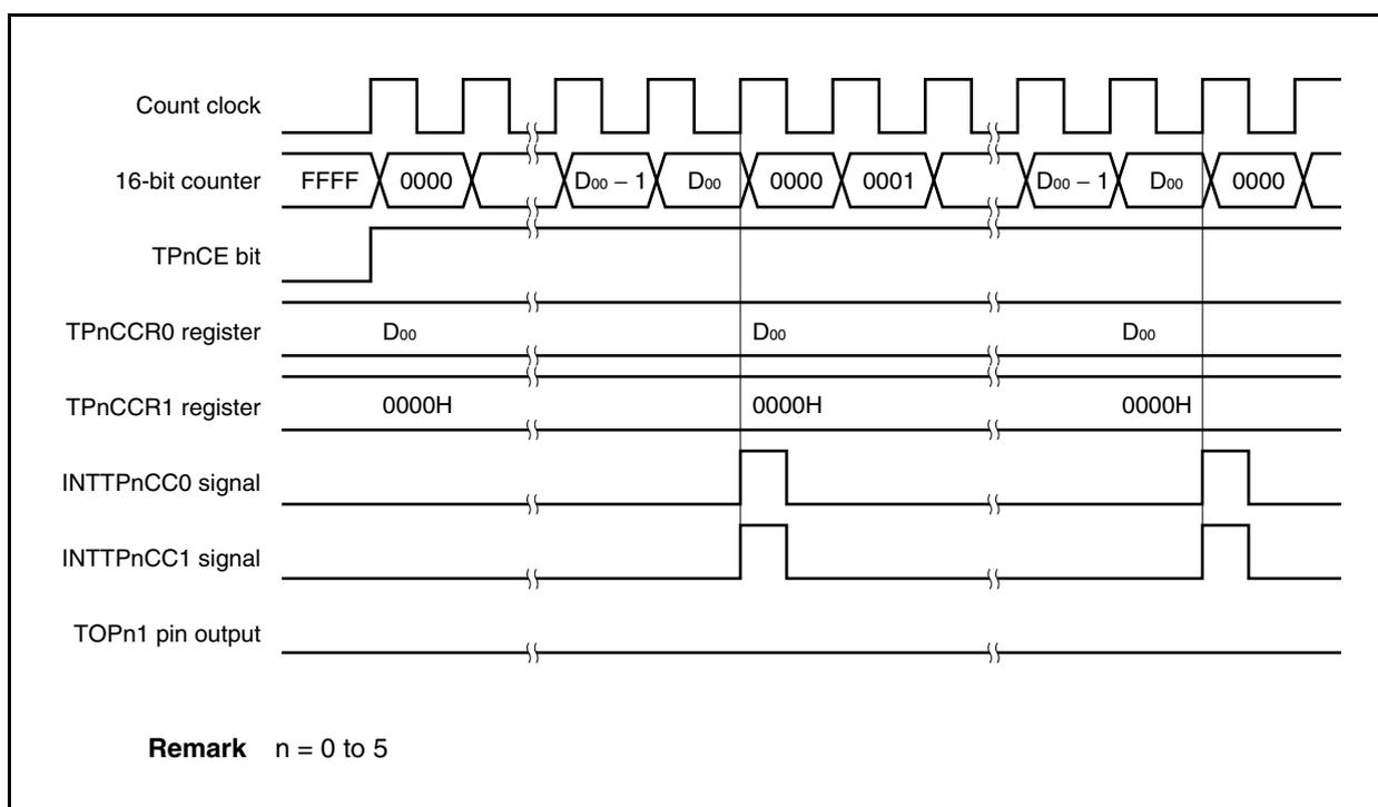
To output a 100% waveform, set the value of TPnCCR0 register + 1 to the TPnCCR1 register. If the value of the TPnCCR0 register is FFFFH, a 100% waveform cannot be output.
