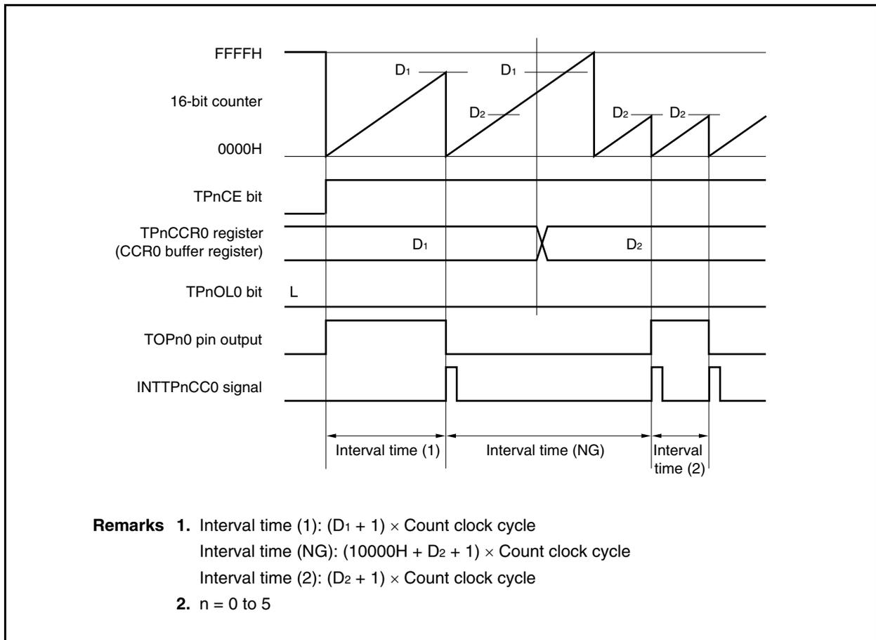
If the value of the TPnCCR0 register is changed from  $D_1$  to  $D_2$  while the counter value is greater than  $D_2$  but less than  $D_1$ , the TPnCCR0 register value is transferred to the CCR0 buffer register as soon as the register has been rewritten. Consequently, the value that is compared with the 16-bit counter value is  $D_2$ .
