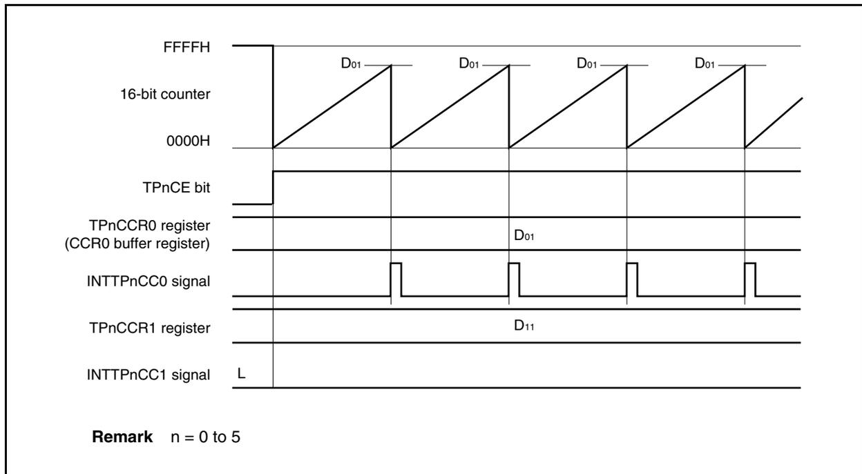
**7.4.3 External trigger pulse output mode (TPnMD2 to TPnMD0 bits = 010)**
