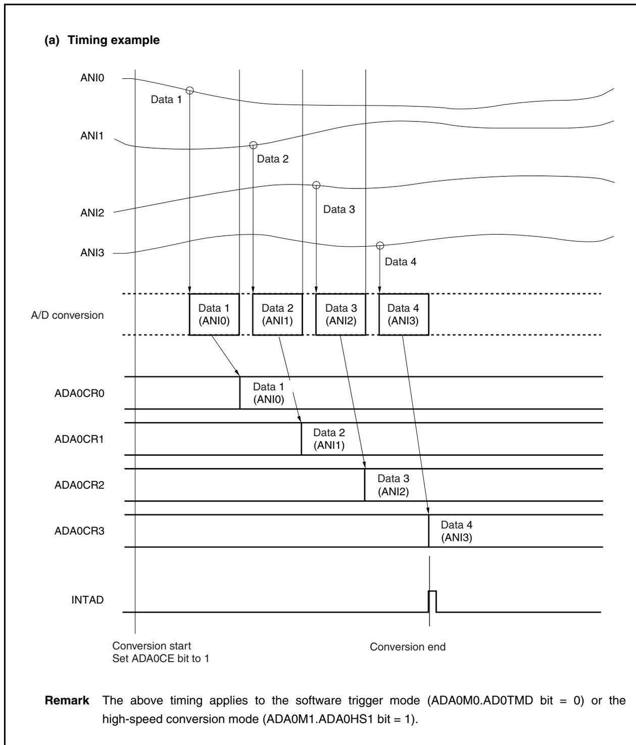
Figure 14-7. Example of Timing in One-Shot Scan Mode (ADA0S Register = 03H) (2/2)
