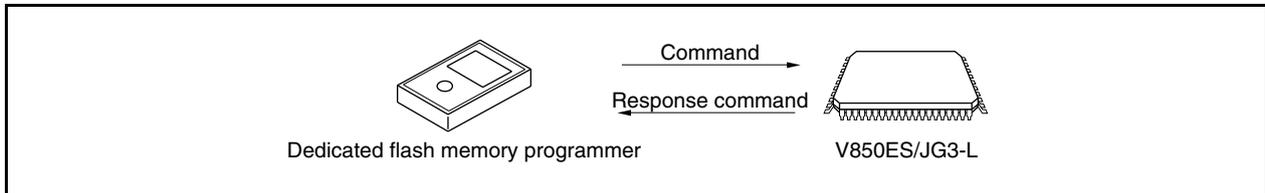
The following shows the commands for flash memory control in the V850ES/JG3-L. All of these commands are issued from the dedicated flash memory programmer, and the V850ES/JG3-L performs the processing corresponding to the commands.
