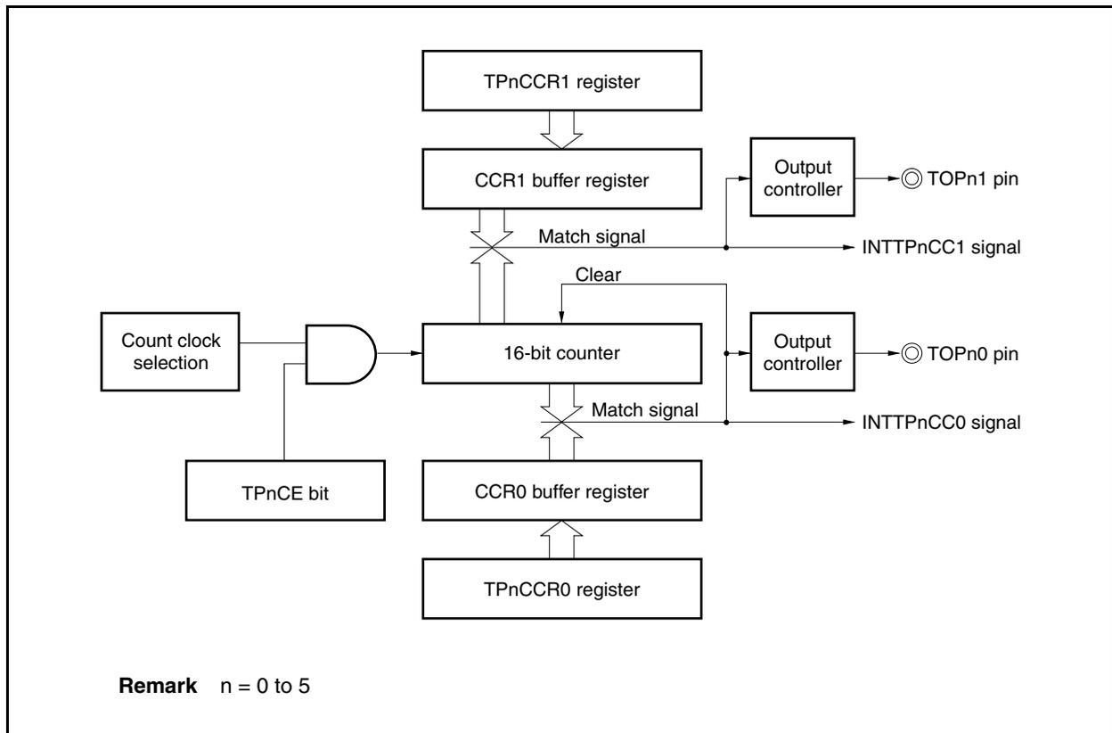
If the value of the TPnCCR1 register is less than or equal to the value of the TPnCCR0 register, the INTTPnCC1 signal is generated once per cycle. At the same time, the output of the TOPn1 pin is inverted.
