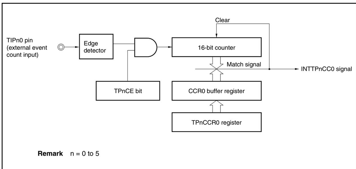
When the TPnCE bit is set to 1, the value of the 16-bit counter is cleared from FFFFH to 0000H. The counter increments each time the valid edge of the external event count input is detected, and the value of the TPnCCR0 register is transferred to the CCR0 buffer register.
