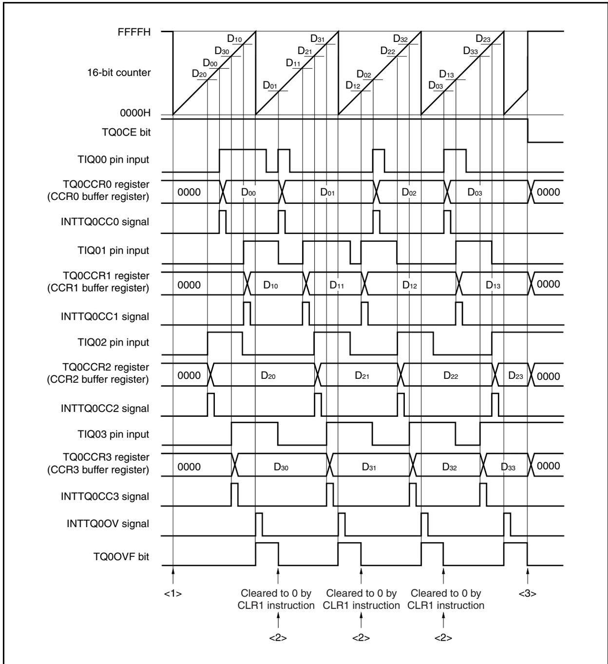
Figure 8-57. Timing and Processing of Operations in Free-Running Timer Mode (Capture Function) (2/2)
