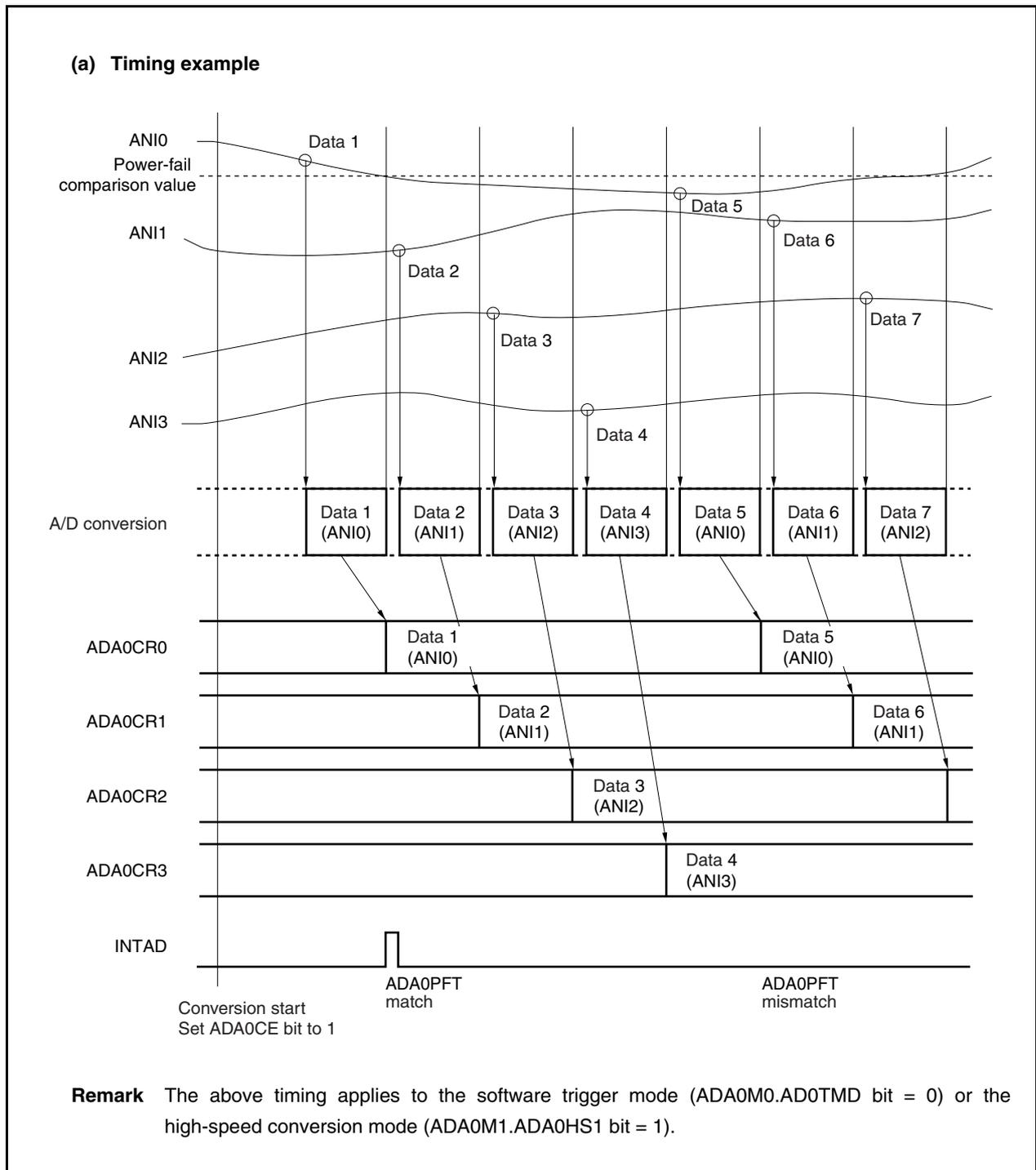
**Figure 14-9. Example of Timing in Continuous Scan Mode**
