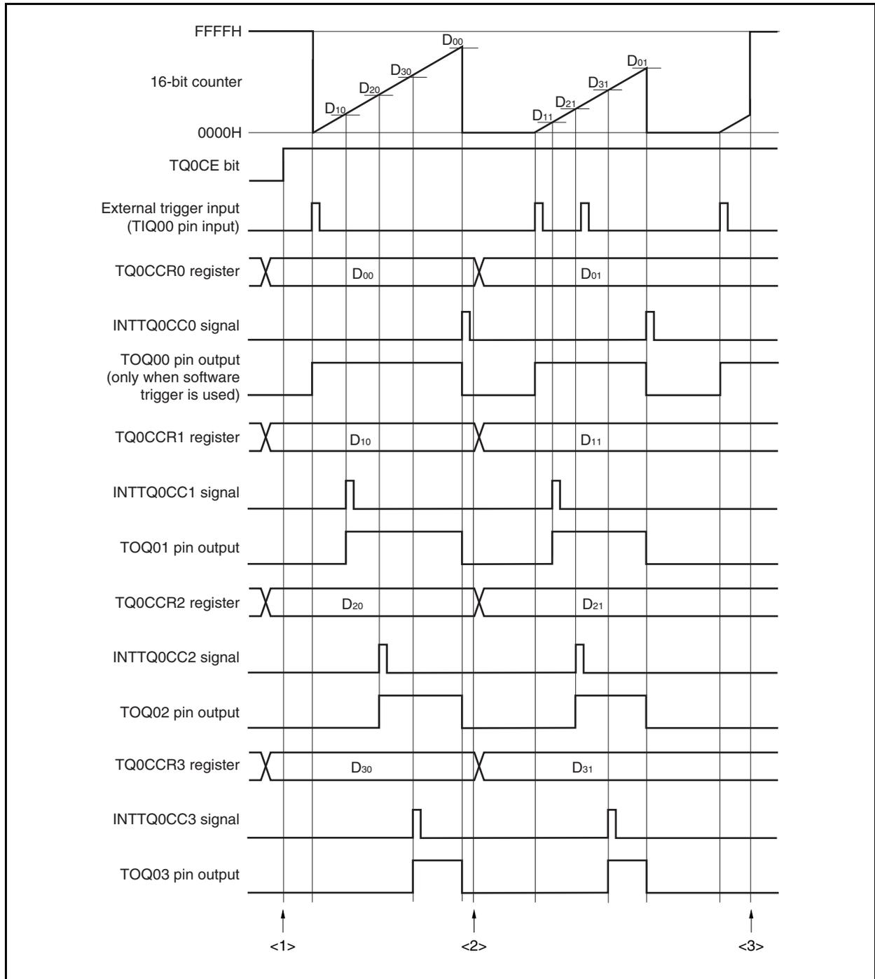
Figure 8-41. Timing and Processing of Operations in One-Shot Pulse Output Mode (2/2)
