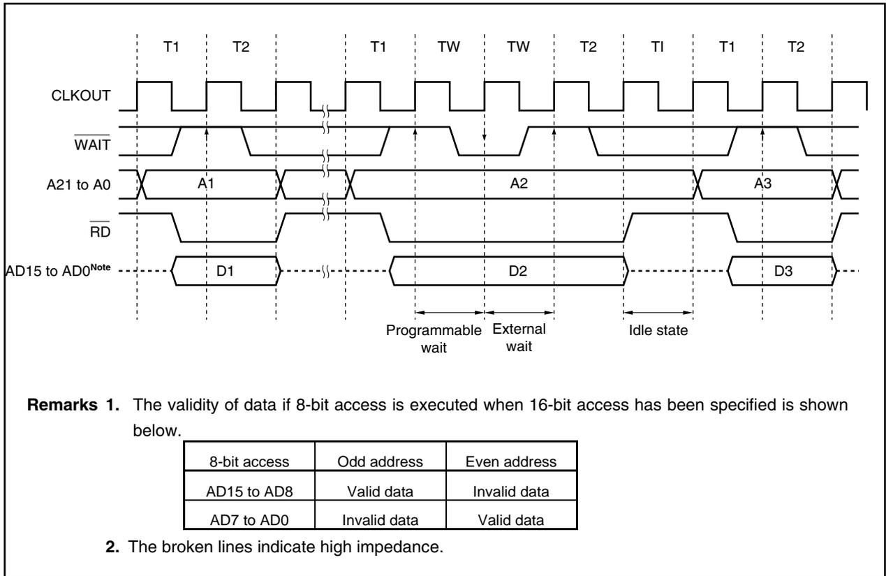
**Figure 5-12. Separate Bus Read Timing (Bus Size: 8 Bits)**
