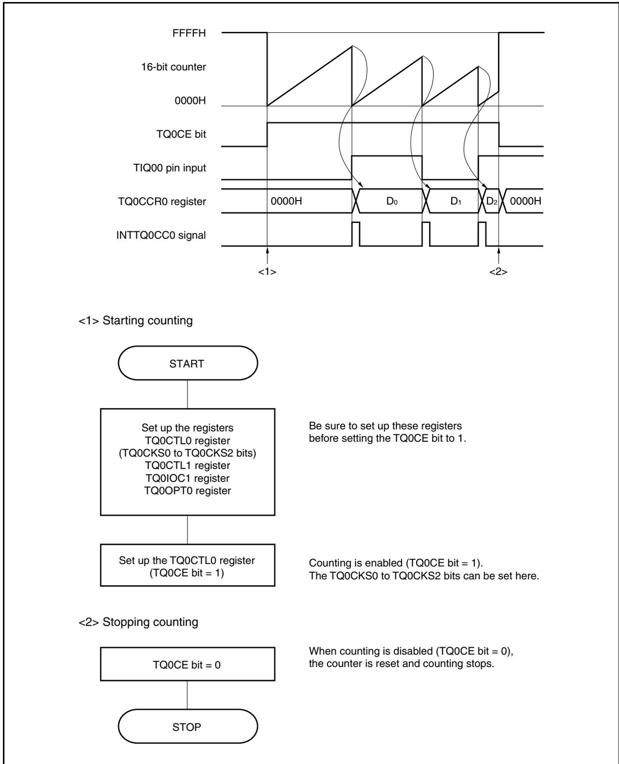
**(2) Using pulse width measurement mode****(a) Clearing the overflow flag (TQ0OVF)**
