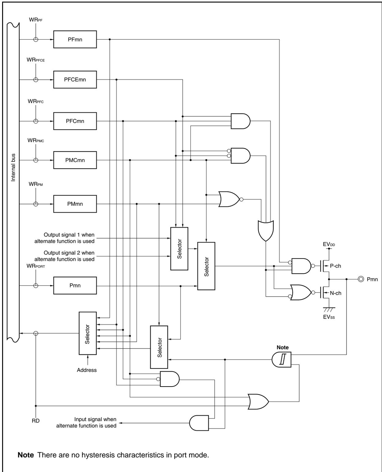
Figure 4-30. Block Diagram of Type U-14
