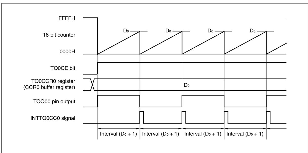
When the TQ0CE bit is set to 1, the value of the 16-bit counter is cleared from FFFFH to 0000H in synchronization with the count clock, and the counter starts incrementing. At this time, the output of the TOQ00 pin is inverted and the set value of the TQ0CCR0 register is transferred to the CCR0 buffer register.
