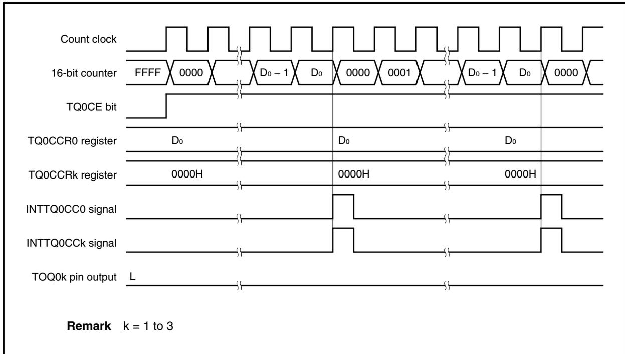
To output a 100% waveform, set the value of TQ0CCR0 register + 1 to the TQ0CCRk register. If the value of the TQ0CCR0 register is FFFFH, a 100% waveform cannot be output.
