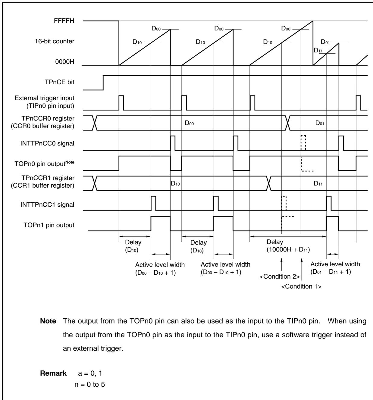
**(b) Timing of generating the compare match interrupt request signal (INTTPnCC1)**
