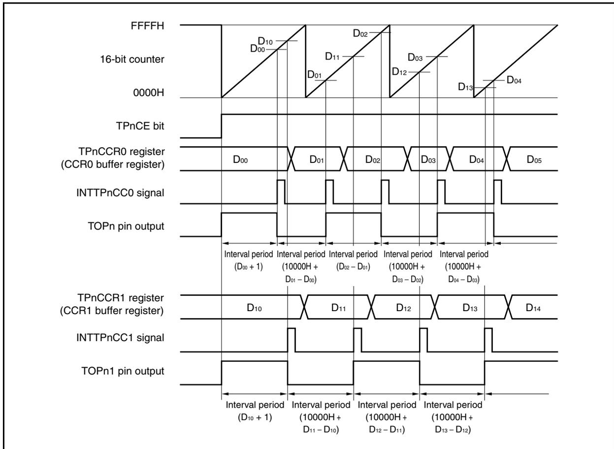
When performing an interval operation in the free-running timer mode, two intervals can be set for one channel.
