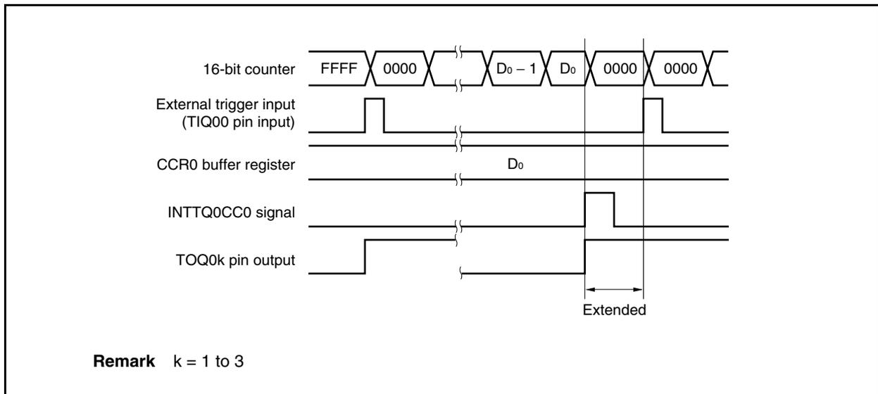
If the trigger is detected immediately before the INTTQ0CC0 signal is generated, the INTTQ0CC0 signal is not generated. The 16-bit counter is cleared to 0000H, the TOQ0k pin output is set to the active level, and the counter continues incrementing. Consequently, the inactive period of the PWM waveform is shortened.
