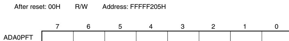
**Caution** In the following modes, write data to the ADA0PFT register while A/D conversion is stopped (ADA0M0.ADA0CE bit = 0), and then enable A/D conversion (ADA0CE bit = 1).
