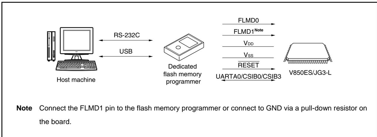
A host machine is required for controlling the dedicated flash memory programmer. In some cases, however, it can be used stand-alone. For details, see the user's manual of the dedicated flash memory programmer.
