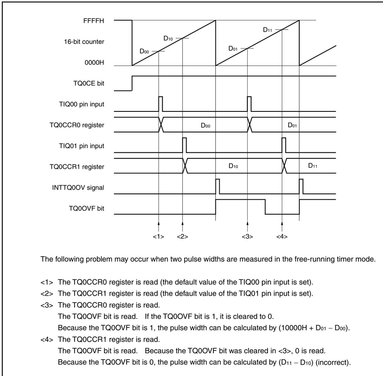
The following problem may occur when two pulse widths are measured in the free-running timer mode.
