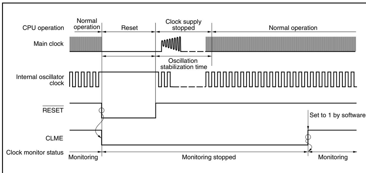
**(3) Operation in STOP mode or after STOP mode is released**
