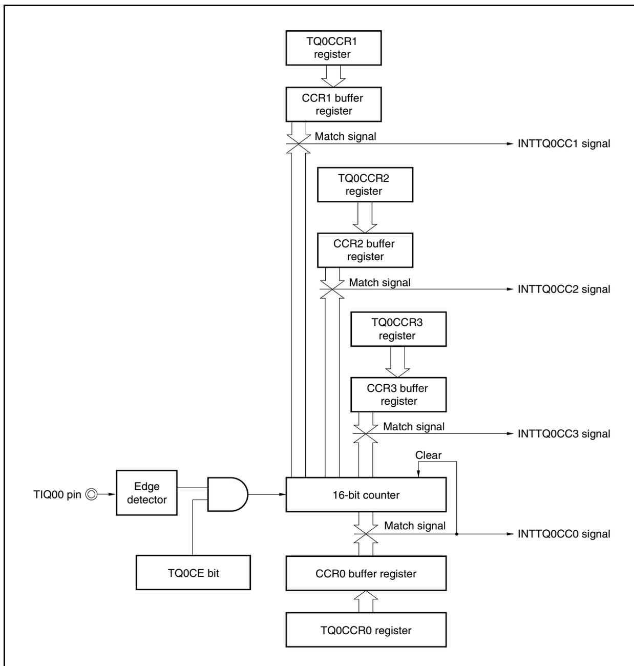
If the value of the TQ0CCRk register is less than or equal to the value of the TQ0CCR0 register, the INTTQ0CCk signal is generated once per cycle.
