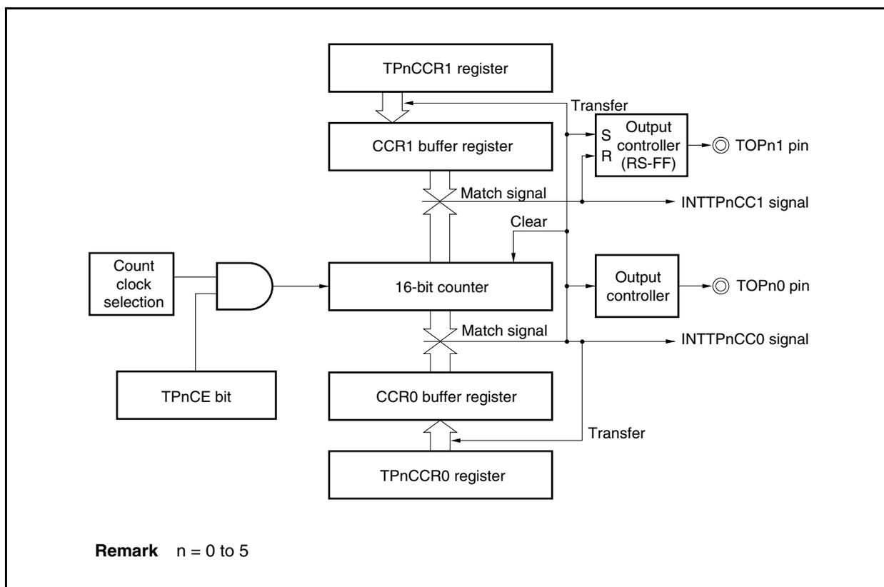
Figure 7-45. Basic Timing of Operations in PWM Output Mode
