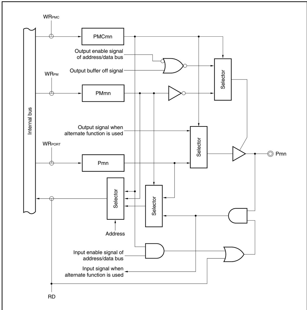
Figure 4-9. Block Diagram of Type E-3
