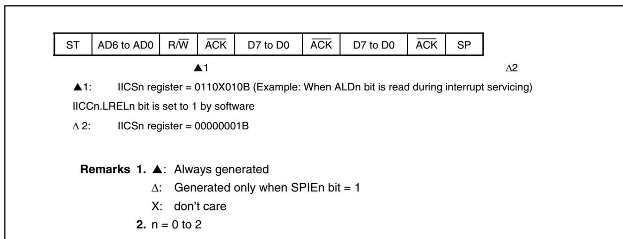
**(3) When arbitration loss occurs during data transfer****<1> When IICn.WTIMn bit = 0**
