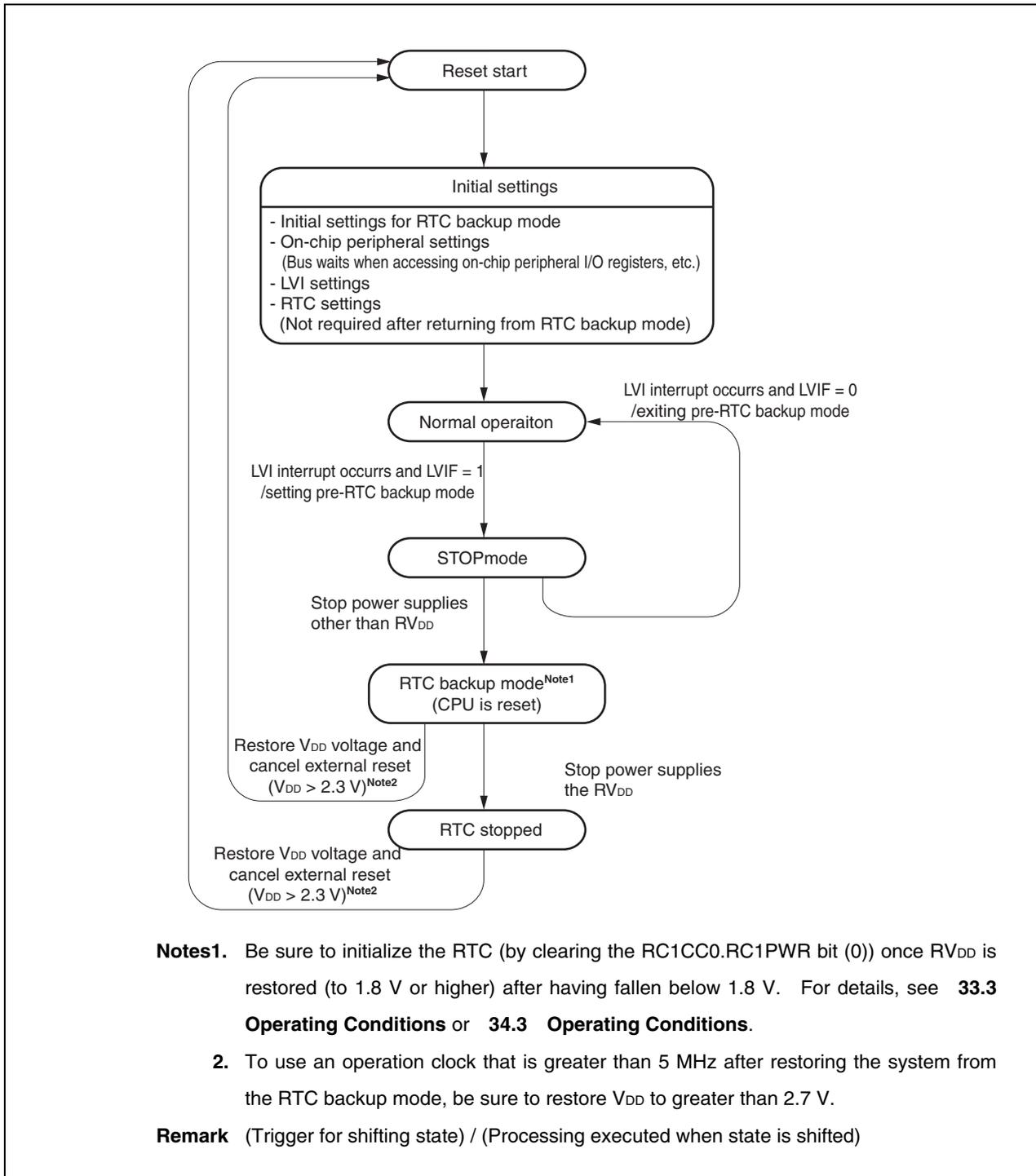
Figure 23-3. Setting the RTC backup mode (1/2)
