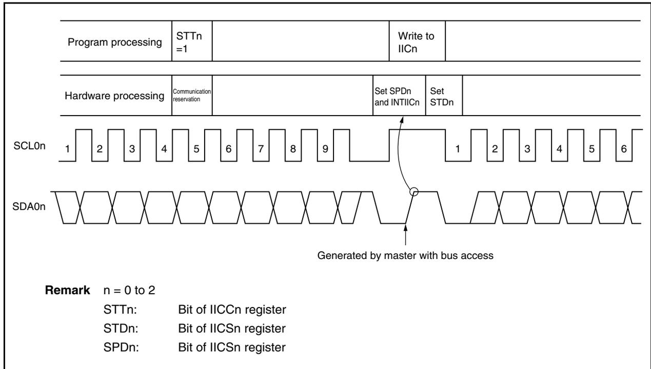
Communication reservations are accepted at the following timing. After the IICSn.STDn bit is set to 1, a communication reservation can be made by setting the IICCn.STTn bit to 1 before a stop condition is detected (n = 0 to 2).
