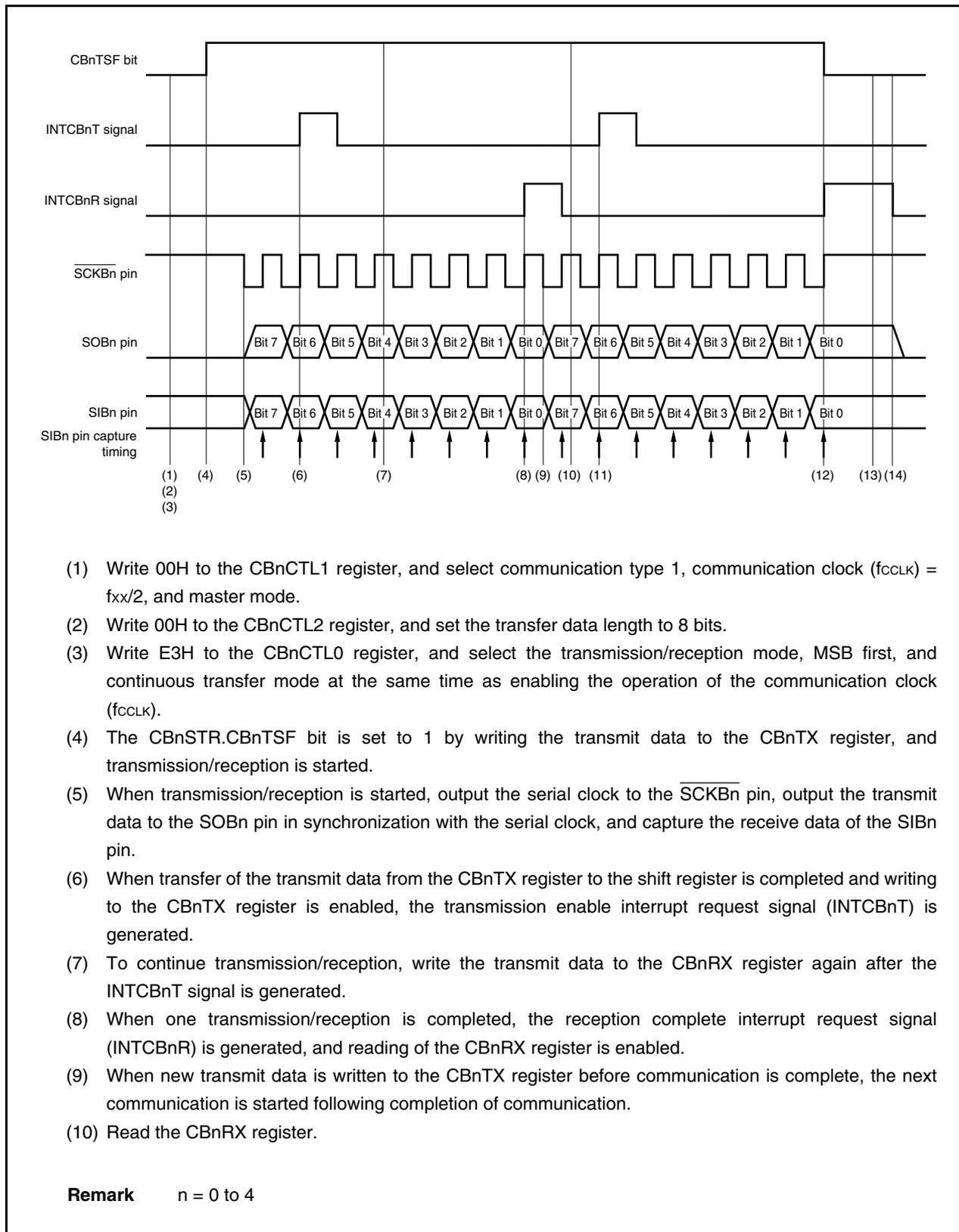
**Figure 18-22. Continuous Transfer Mode Operation Timing (Master Mode, Transmission/Reception Mode)**
