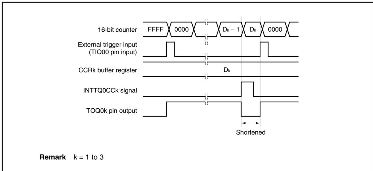
If the trigger is detected immediately before the INTTQ0CCK signal is generated, the INTTQ0CCK signal is not generated, and the 16-bit counter is cleared to 0000H and continues incrementing. The output signal of the TOQ0k pin remains active. Consequently, the active period of the PWM waveform is extended.
