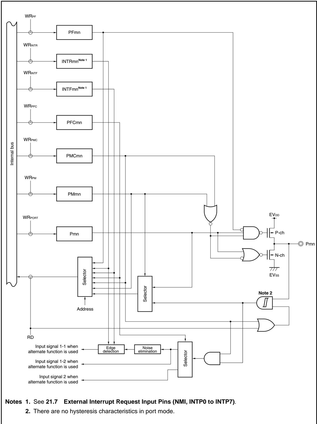
Figure 4-20. Block Diagram of Type U-1
