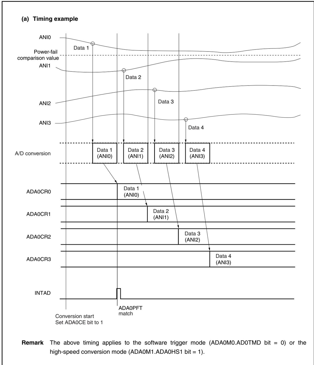
**Figure 14-11. Example of Timing in One-Shot Scan Mode**
