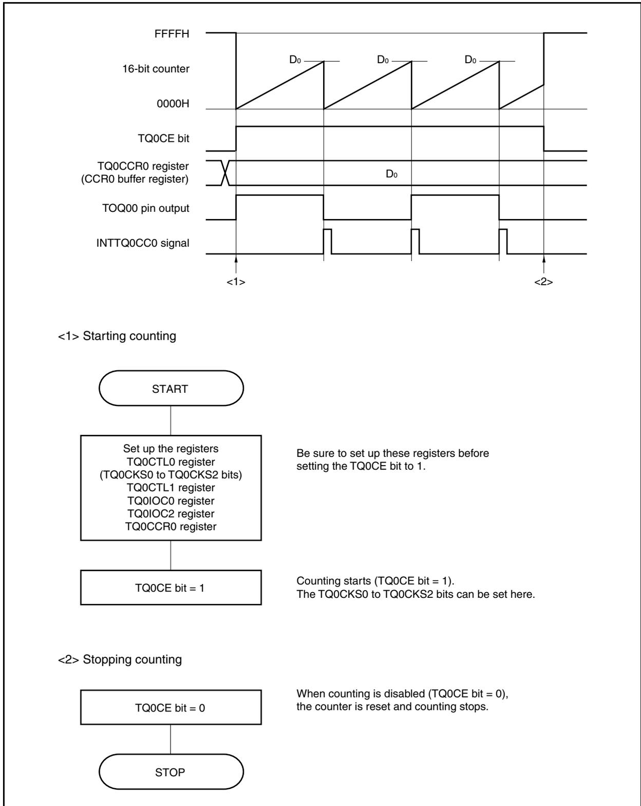
**(2) Using interval timer mode****(a) Operation when TQ0CCR0 register is set to 0000H**
