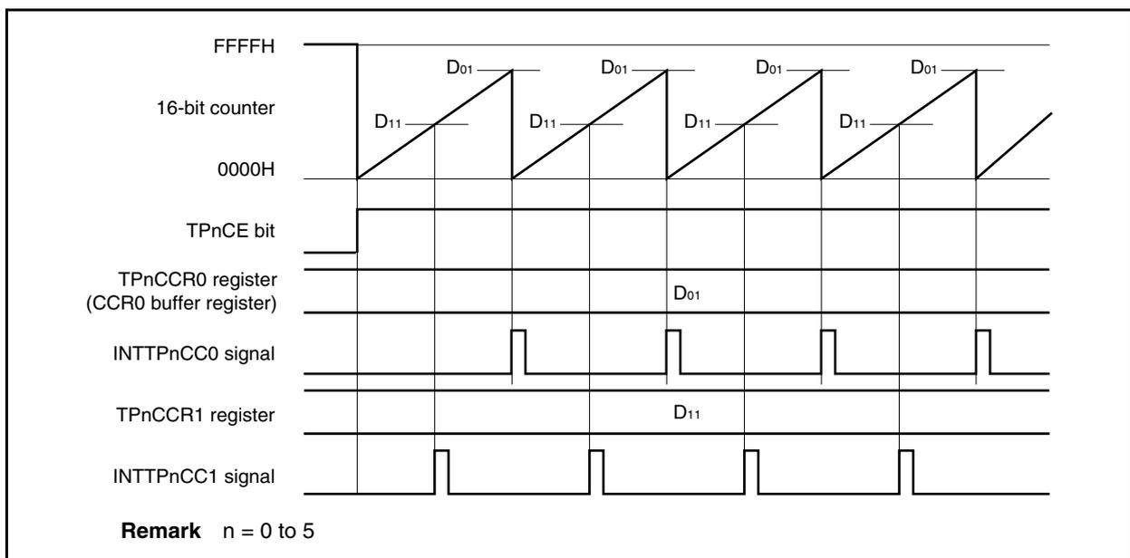
If the value of the TPnCCR1 register is greater than the value of the TPnCCR0 register, the value of the 16-bit counter will not match the value of the TPnCCR1 register and the INTTPnCC1 signal will not be generated.
