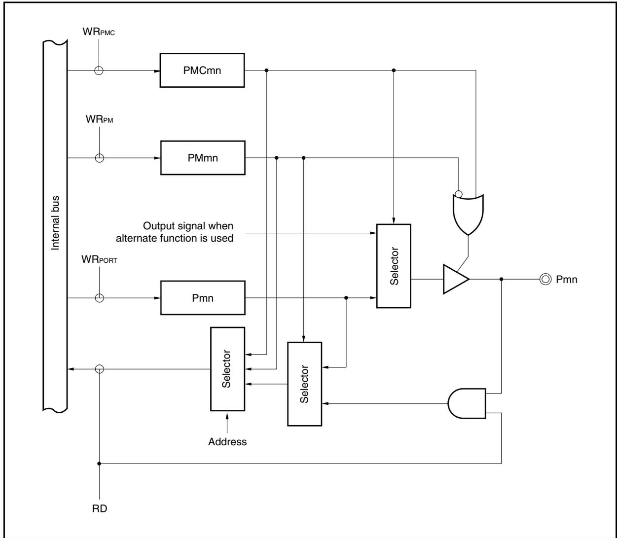
Figure 4-8. Block Diagram of Type D-3
