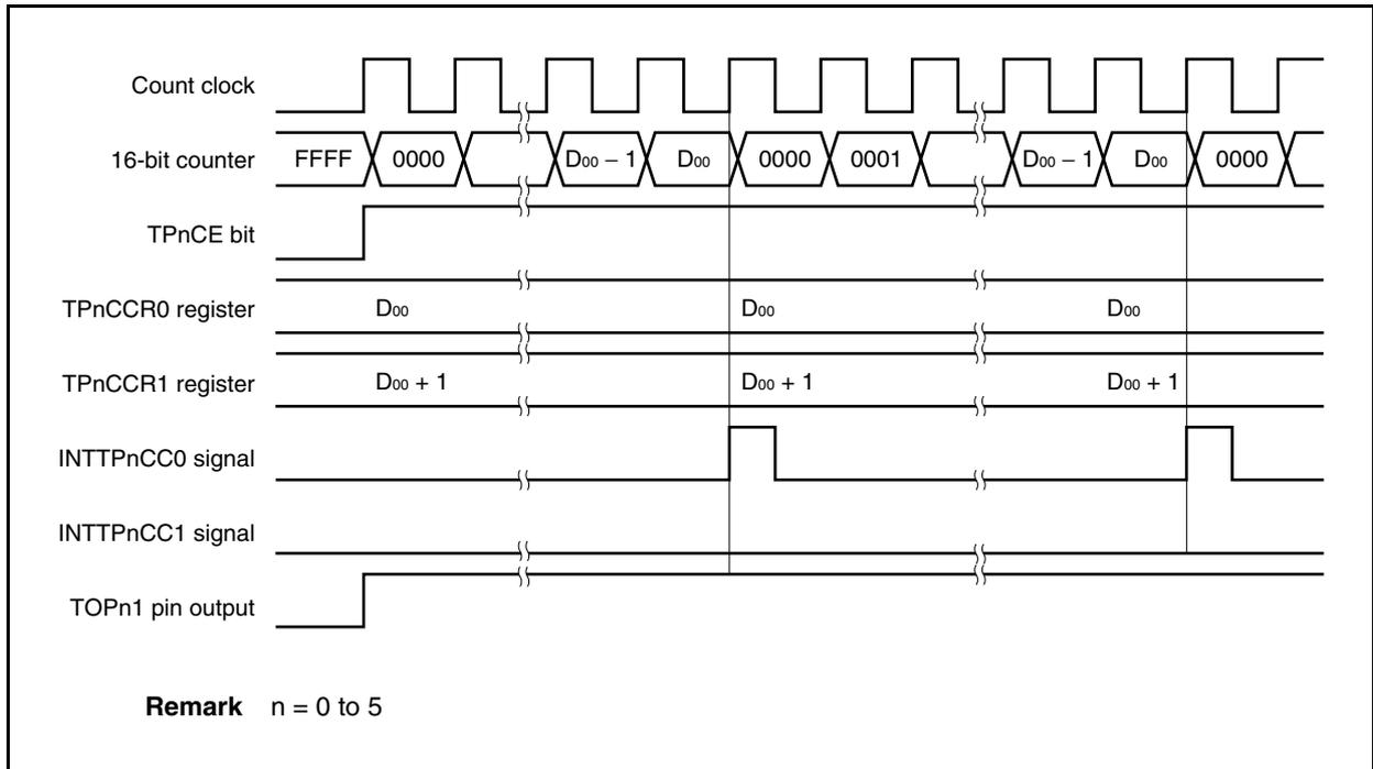
**(c) Timing of generating the compare match interrupt request signal (INTTPnCC1)**
