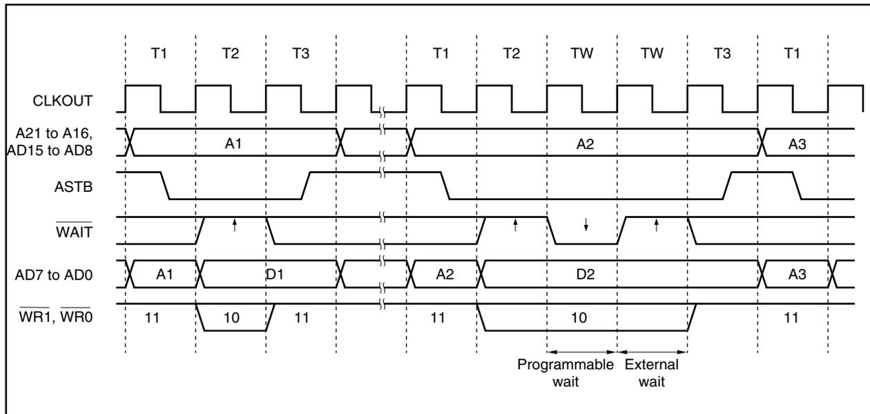
Figure 5-9. Multiplexed Bus Hold Timing (Bus Size: 16 Bits, 16-bit Access)
