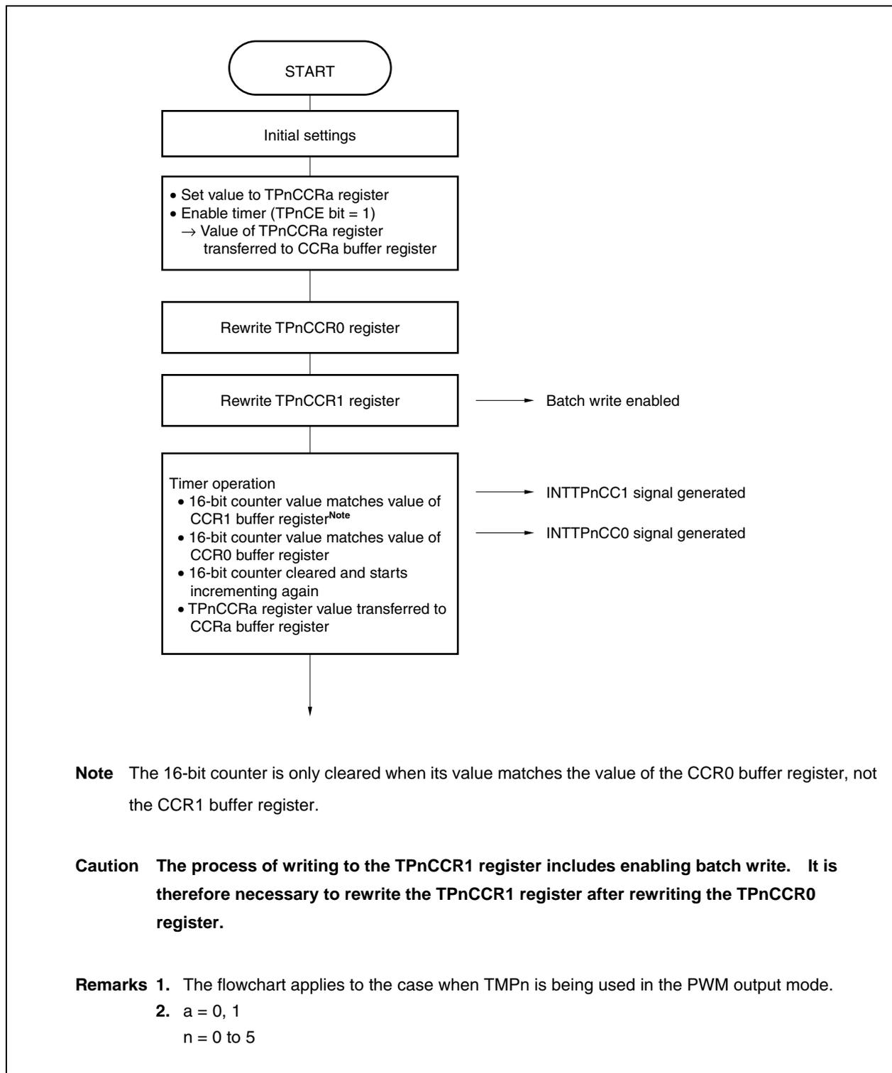
Figure 7-5. Batch Write Timing
