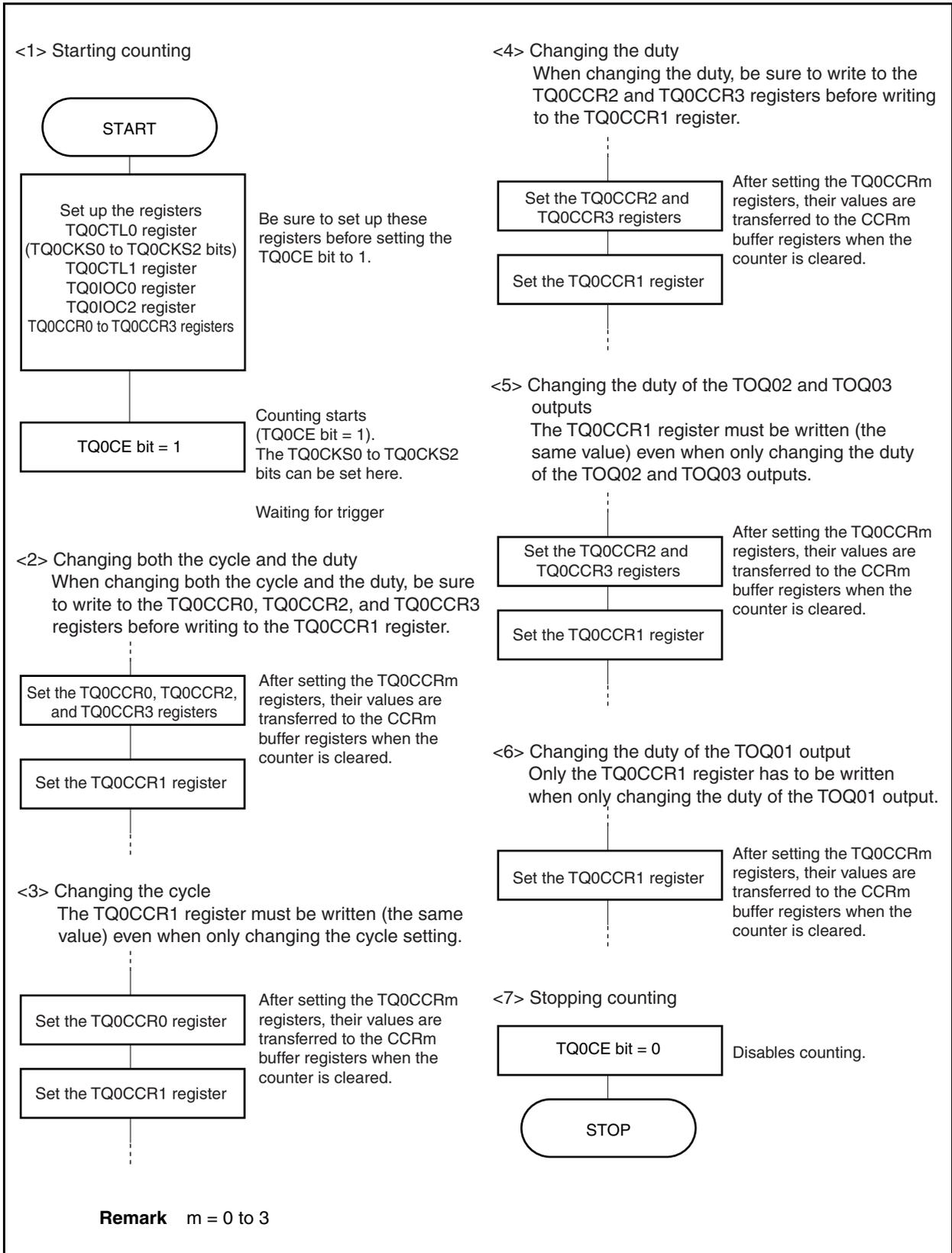
**(2) Using external trigger pulse output mode**
