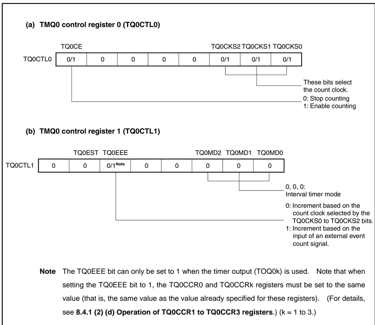
Figure 8-8. Register Settings in Interval Timer Mode (2/3)
