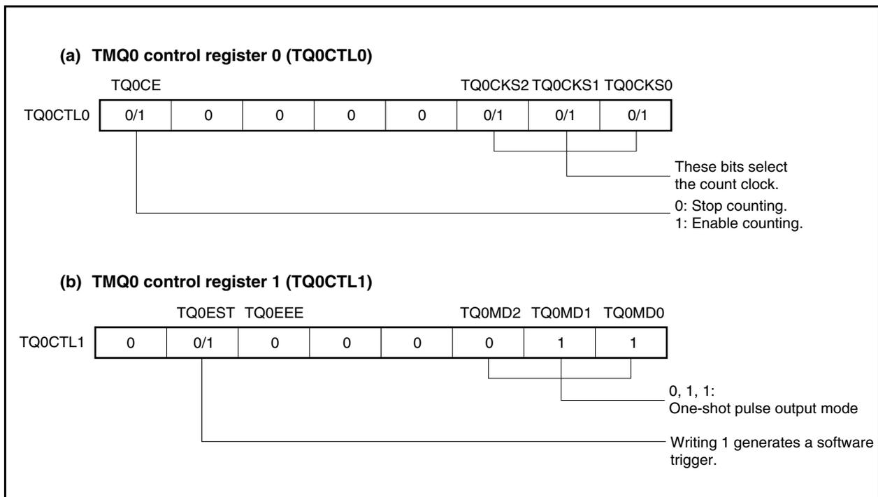
Figure 8-40. Register Settings in One-Shot Pulse Output Mode (2/3)
