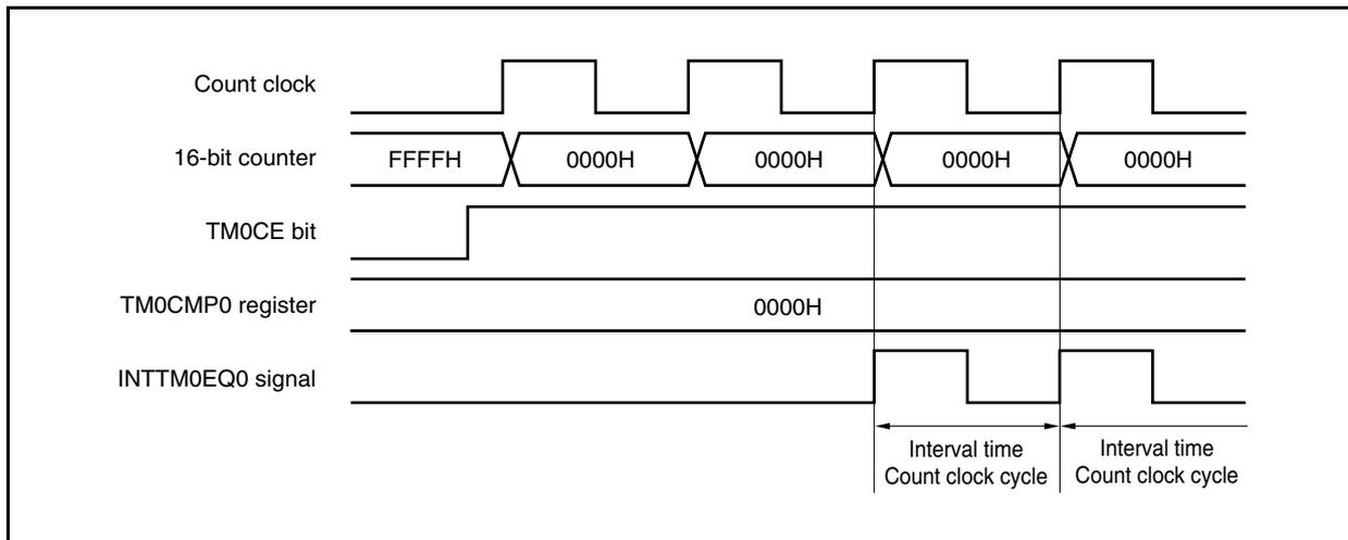
(b) Operation when TM0CMP0 register is set to N
