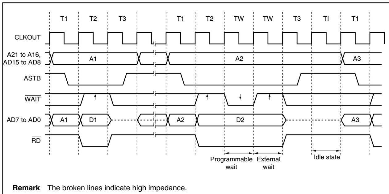
Figure 5-7. Multiplexed Bus Write Timing (Bus Size: 16 Bits, 16-bit Access)
