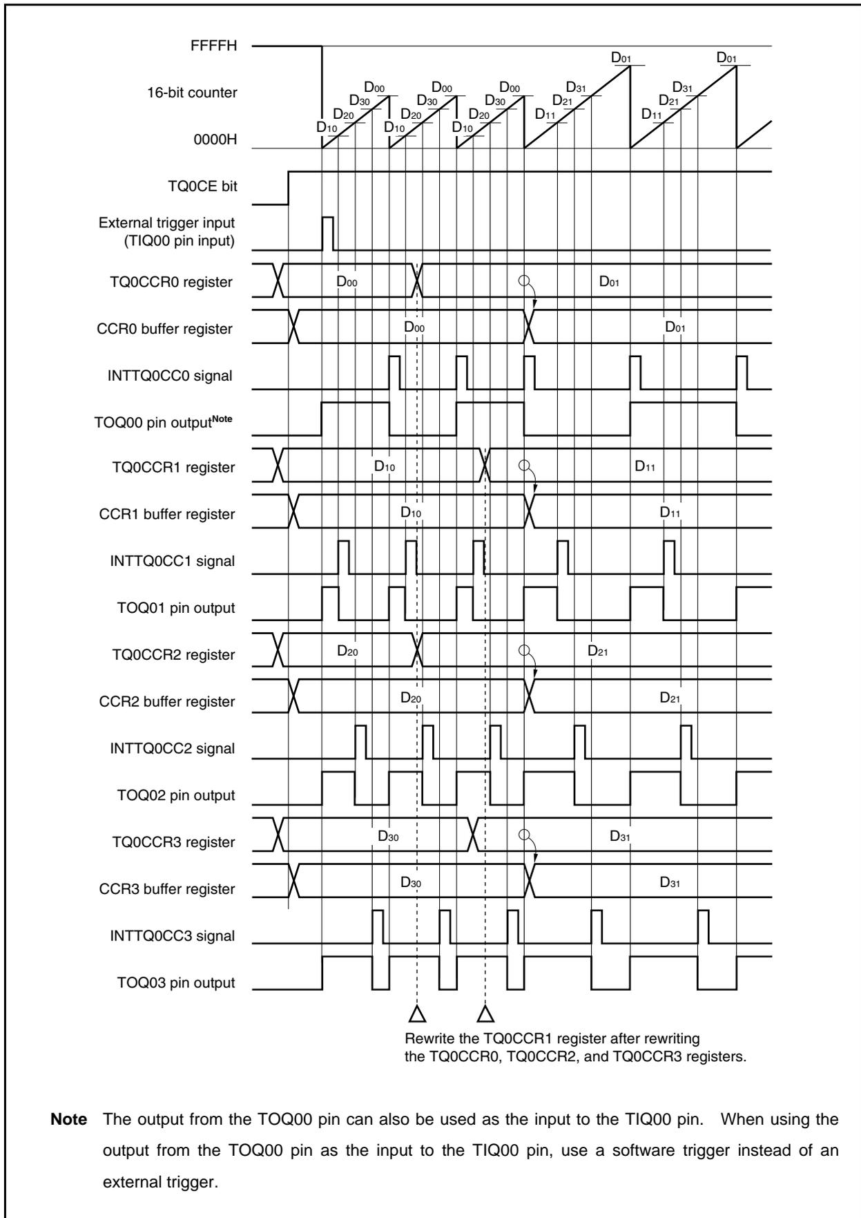
In order to transfer data from the TQ0CCRm register to the CCRm buffer register, the TQ0CCR1 register must be written.
