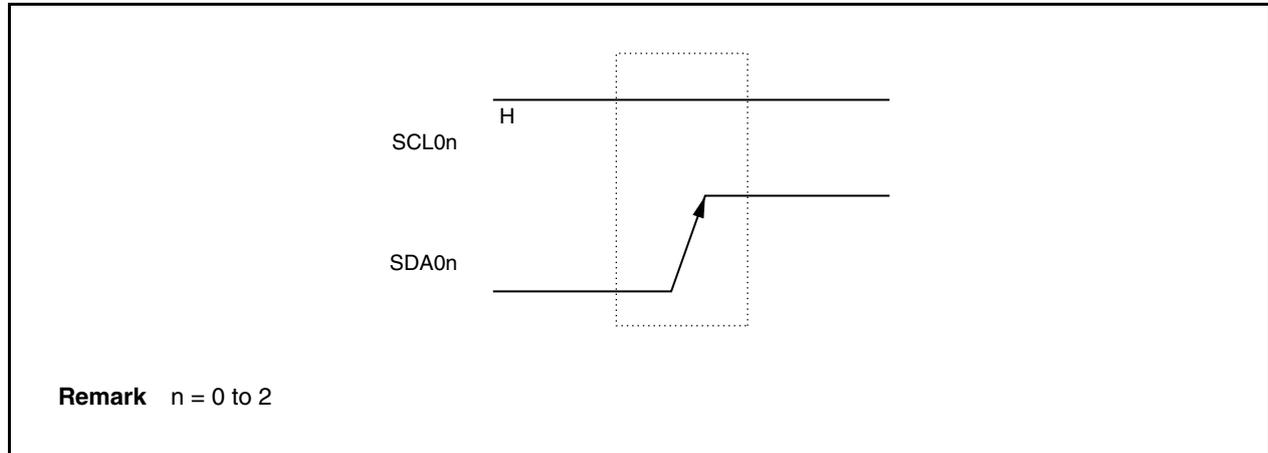
A stop condition is generated when the IICn.SPTn bit is set to 1. When the stop condition is detected, the IICn.SPDn bit is set to 1 and the interrupt request signal (INTIICn) is generated when the IICn.SPIEn bit is set to 1 (n = 0 to 2).
