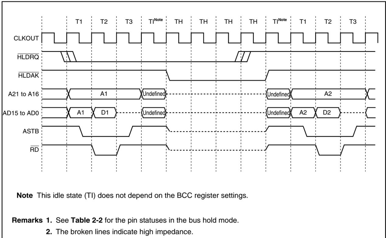
Figure 5-10. Address Wait Timing (Bus Size: 16 Bits, 16-bit Access)
