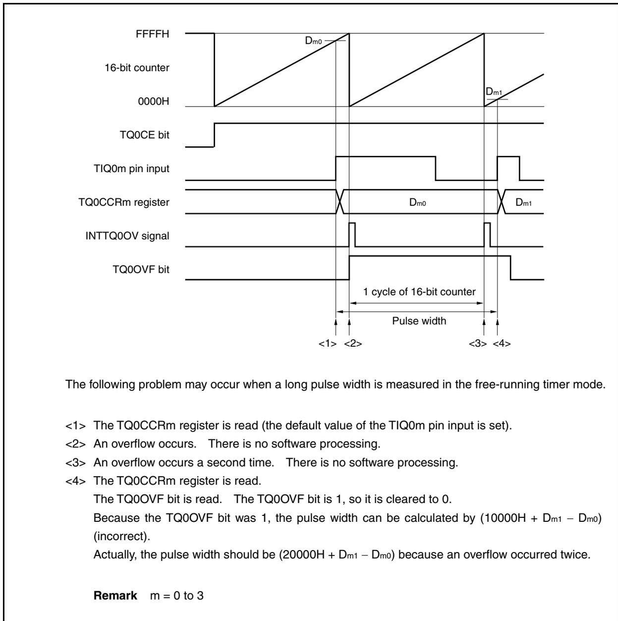
If an overflow occurs twice or more when the capture trigger interval is long, the correct pulse width may not be obtained.
