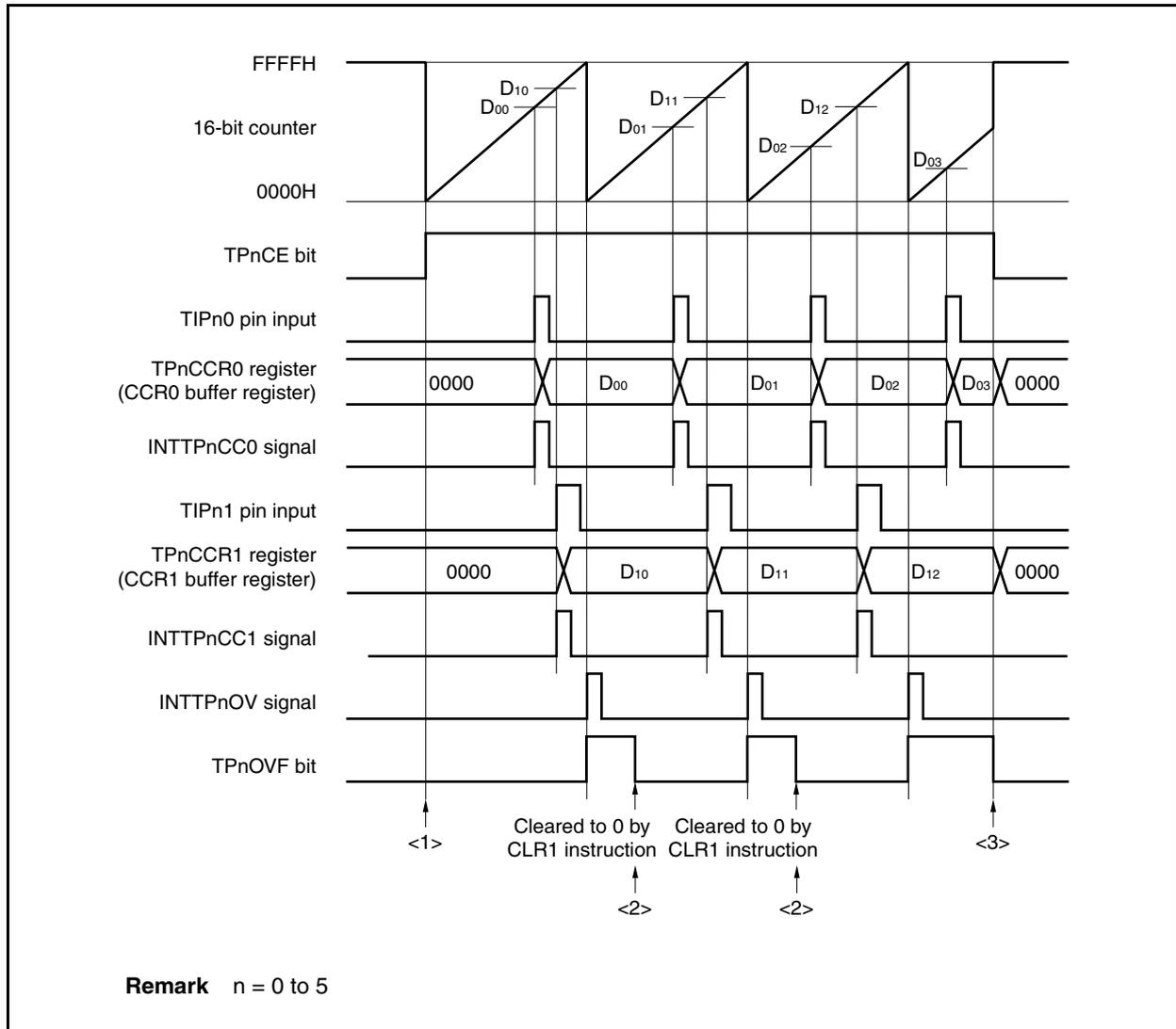
Figure 7-57. Timing and Processing of Operations in Free-Running Timer Mode (Capture Function) (2/2)
