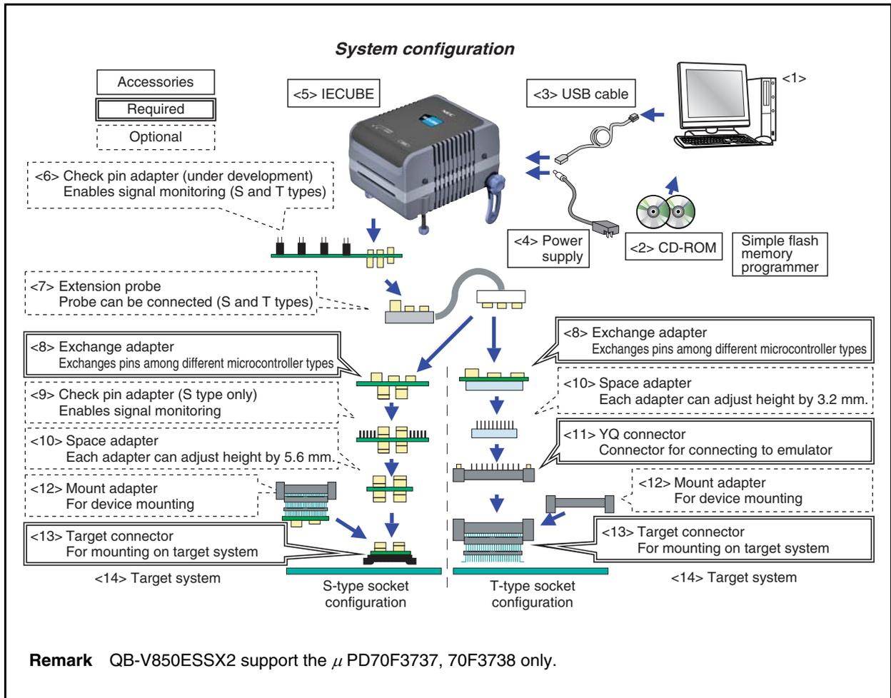
**Figure A-2. System Configuration (When Using QB-V850ESSX2, QB-V850ESJX3L) (2/2)**
