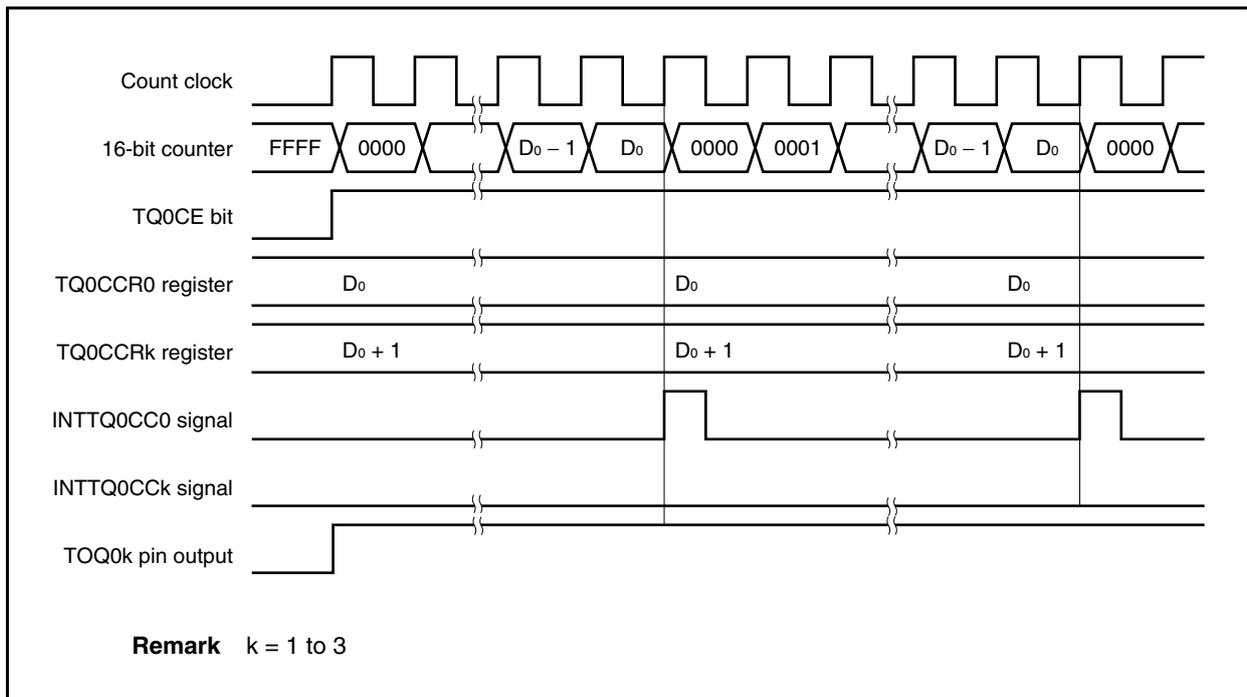
**(c) Timing of generating the compare match interrupt request signal (INTTQ0CCK)**
