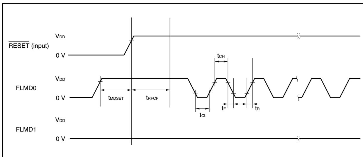
**(3) Programming characteristics****( $T_A = -40$  to  $+85^\circ\text{C}$ ,  $V_{DD} = EV_{DD} = AV_{REF0} = AV_{REF1} = 2.7$  to  $3.6$  V,  $V_{SS} = EV_{SS} = AV_{SS} = 0$  V,  $C_L = 50$  pF)**
