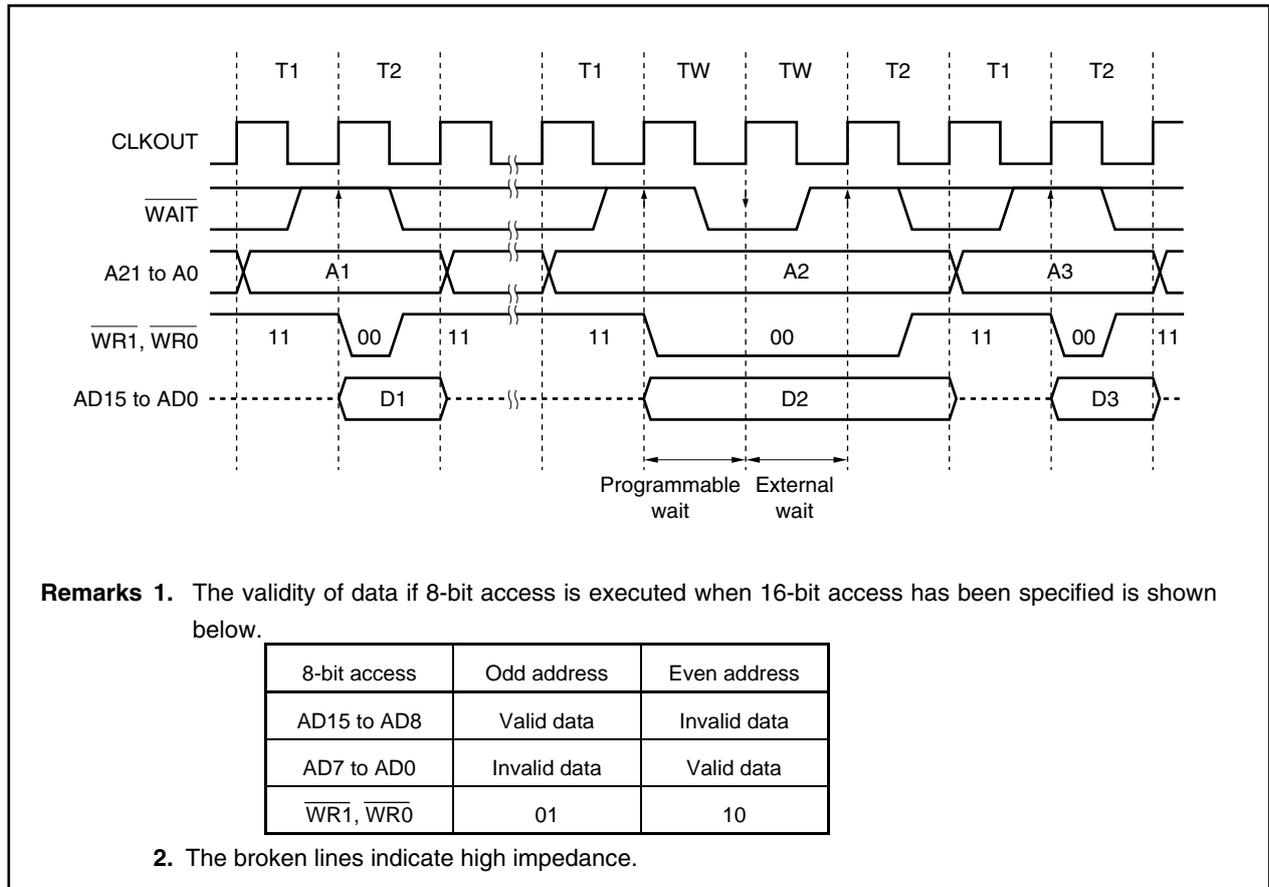
**Figure 5-14. Separate Bus Write Timing (Bus Size: 8 Bits)** ( $\mu$  PD70F3737, 70F3738, 70F3792, 70F3793 only)
