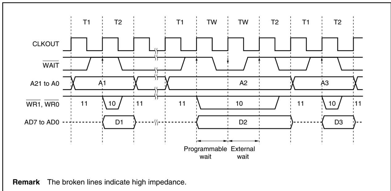
**Figure 5-15. Separate Bus Hold Timing (Bus Size: 8 Bits, Write)**
