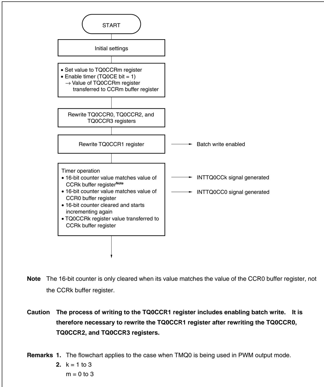
Figure 8-5. Batch Write Timing
