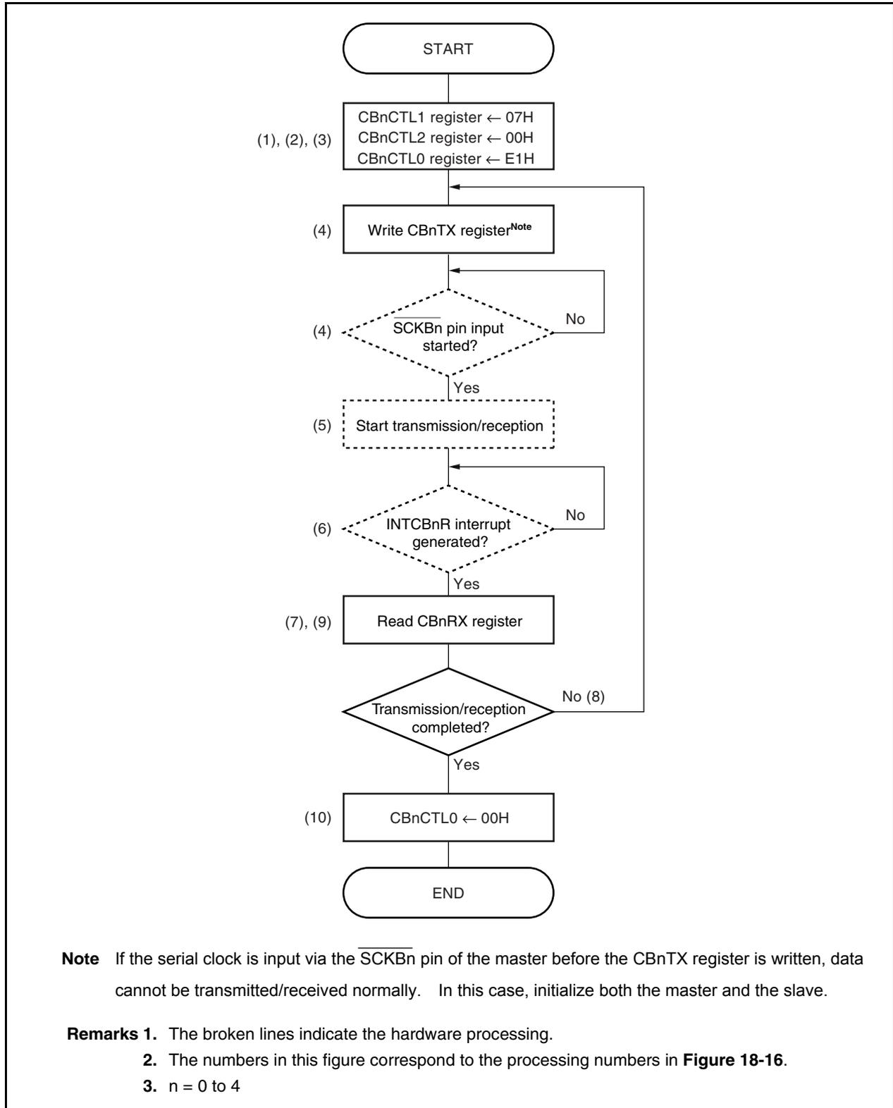
**Figure 18-16. Single Transfer Mode Operation Timing (Slave Mode, Transmission/Reception Mode)**
