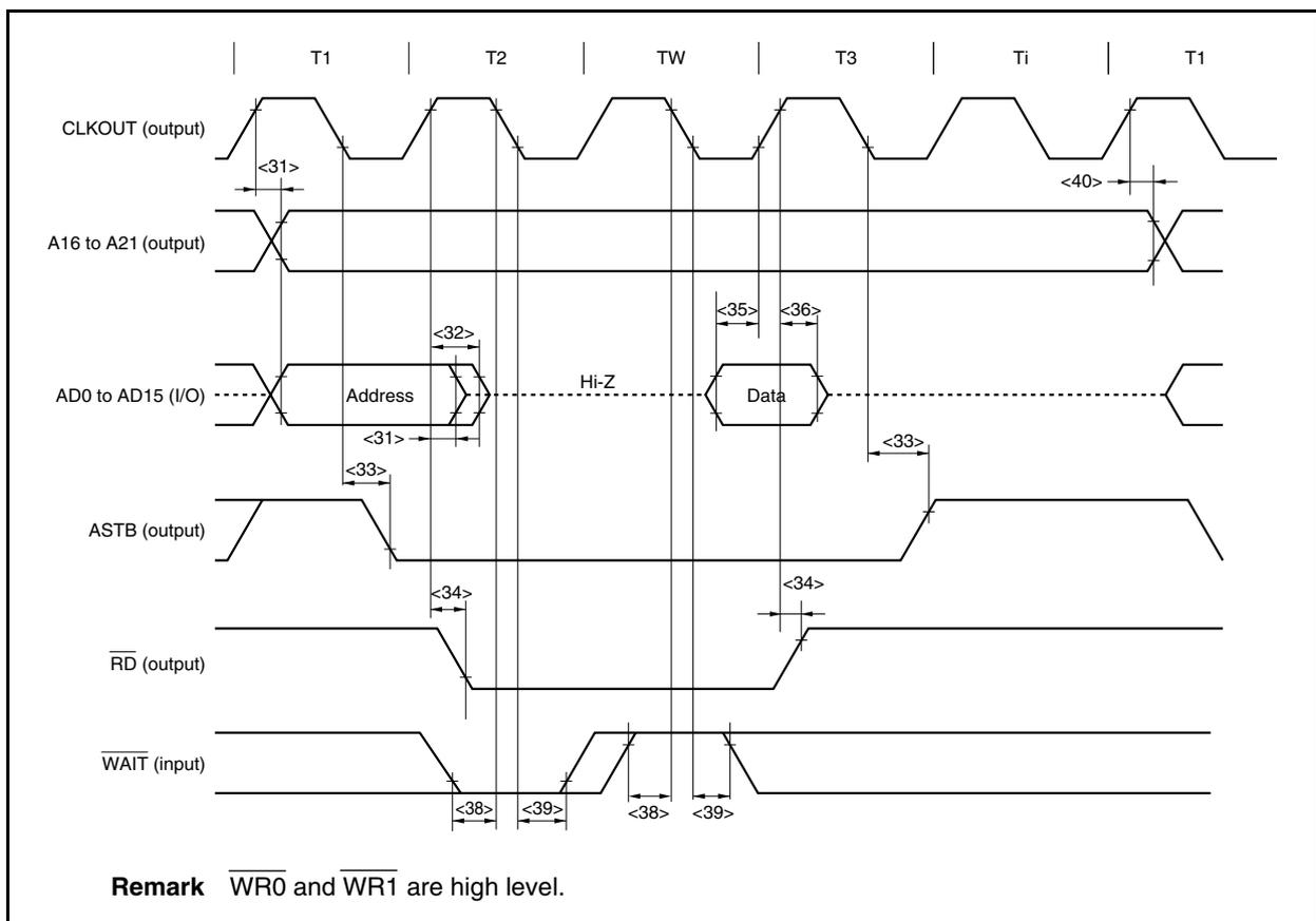
**Write Cycle (Synchronous with CLKOUT): In Multiplexed Bus Mode**
