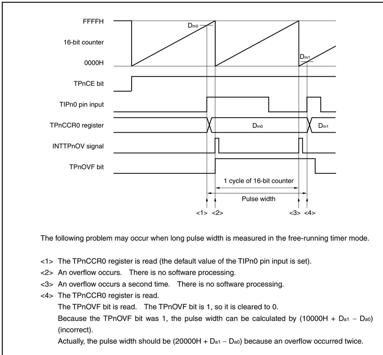
If an overflow occurs twice or more when the capture trigger interval is long, the correct pulse width may not be obtained.
