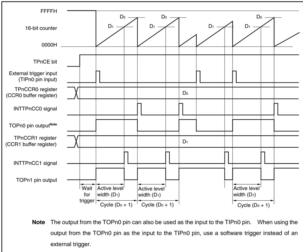
When the TPnCE bit is set to 1, TMPn waits for a trigger. When the trigger is generated, the 16-bit counter is cleared from FFFFH to 0000H, starts incrementing, and outputs a PWM waveform from the TOPn1 pin. If the trigger is generated again while the counter is incrementing, the counter is cleared to 0000H and restarts incrementing, and the output of the TOPn0 pin is inverted. (The TOPn1 pin outputs a high level signal regardless of the status (high/low) when a trigger occurs.)
