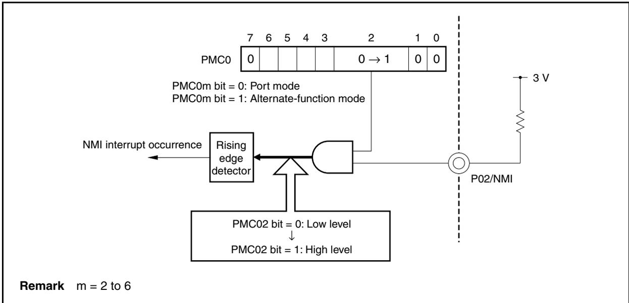
[Example 2] Switching from external pin (NMI) to general-purpose port pin (P02)
