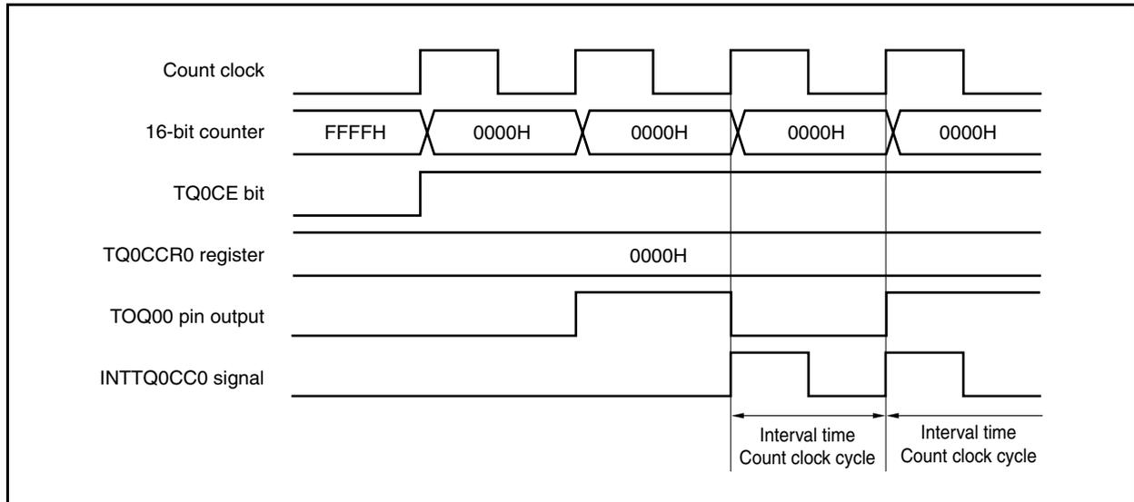
**(b) Operation when TQ0CCR0 register is set to FFFFH**
