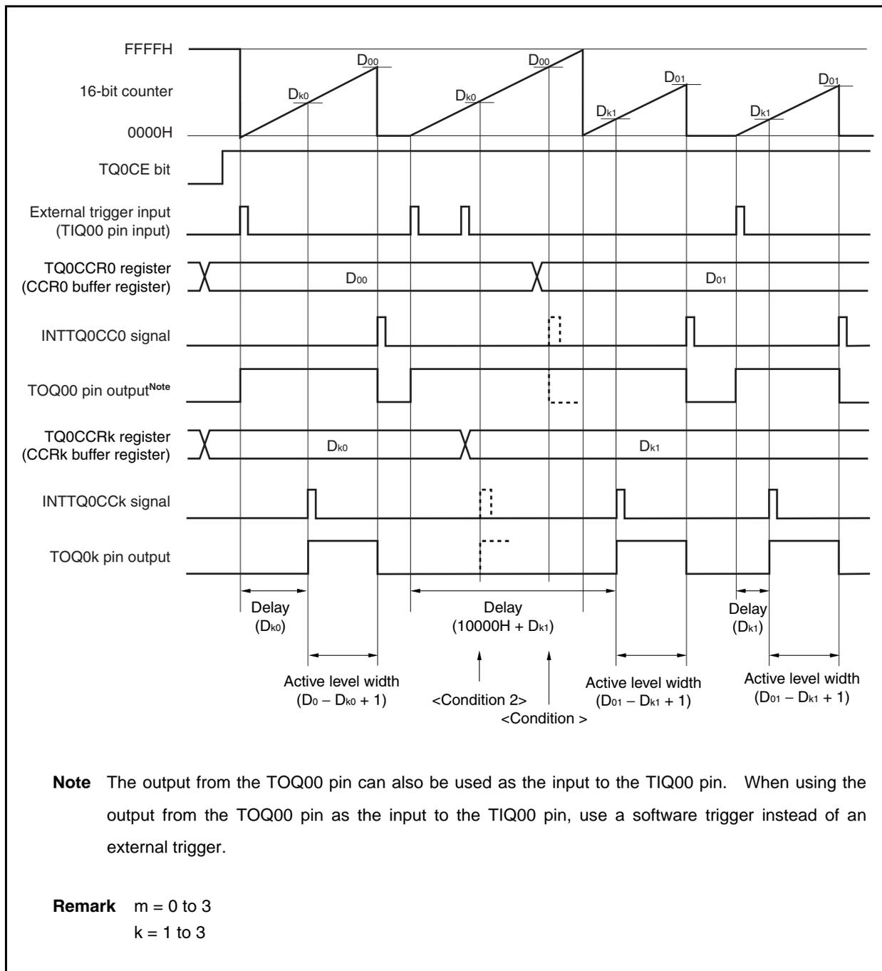
**(b) Timing of generating the compare match interrupt request signal (INTTQ0CCK)**
