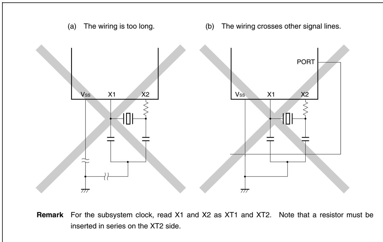
Figure 6-4. Examples of Incorrect Resonator Connections (2/2)
