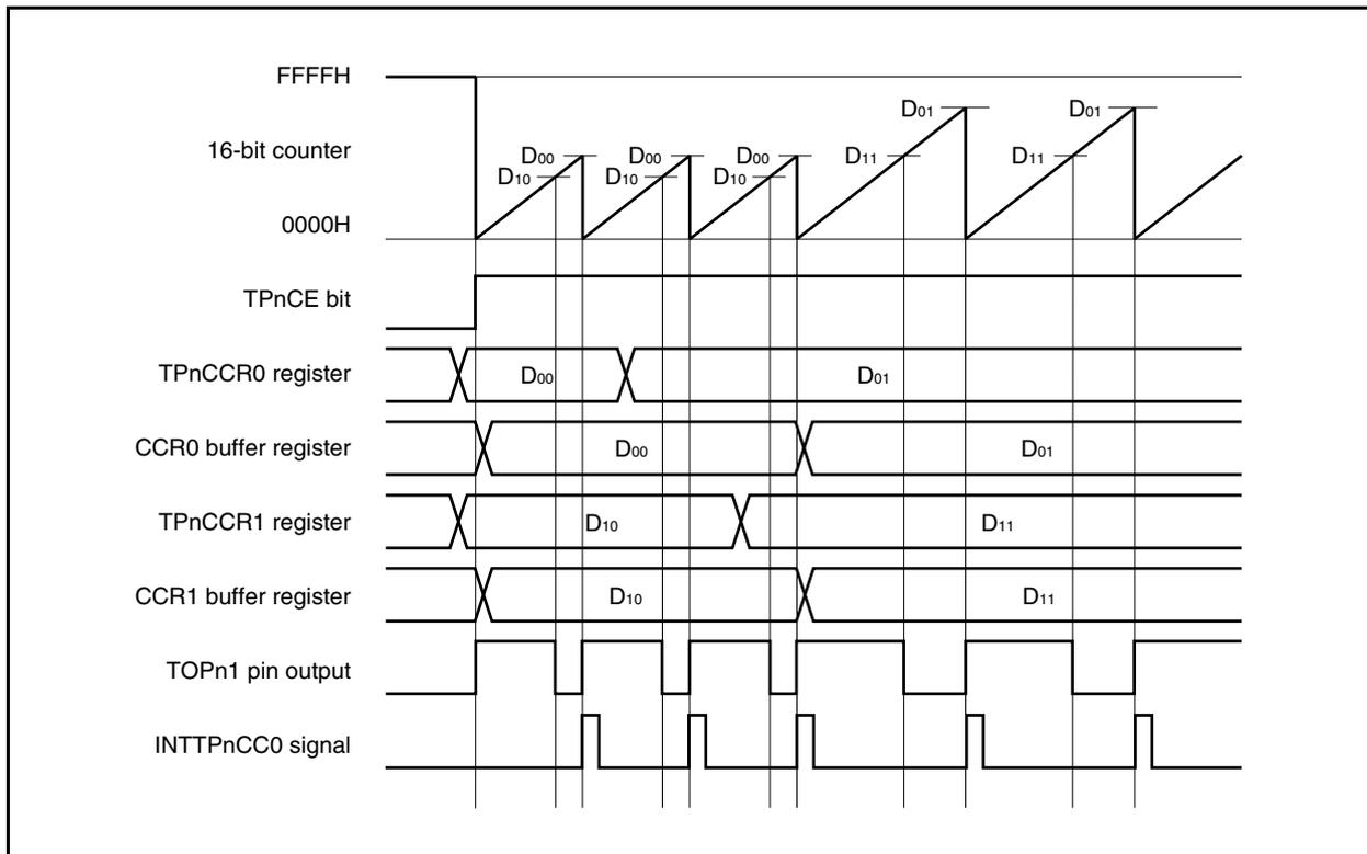
In order to transfer data from the TPnCCRa register to the CCRa buffer register, the TPnCCR1 register must be written.
