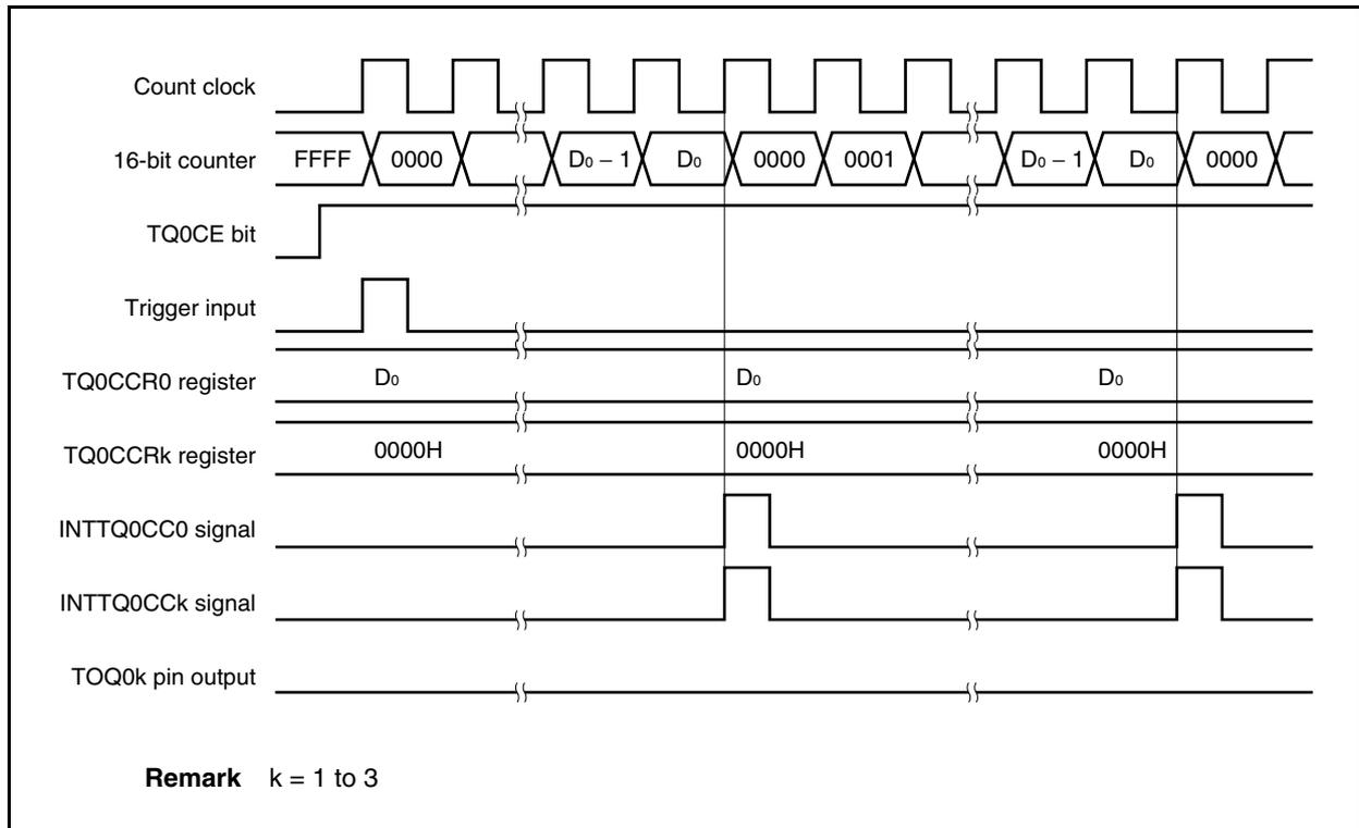
To output a 100% waveform, set the value of TQ0CCR0 register + 1 to the TQ0CCRk register.
