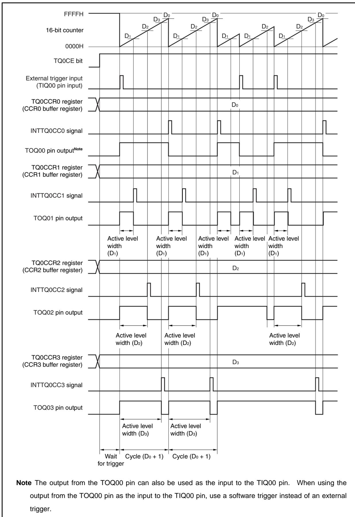
**Note** The output from the TOQ00 pin can also be used as the input to the TIQ00 pin. When using the output from the TOQ00 pin as the input to the TIQ00 pin, use a software trigger instead of an external trigger.
