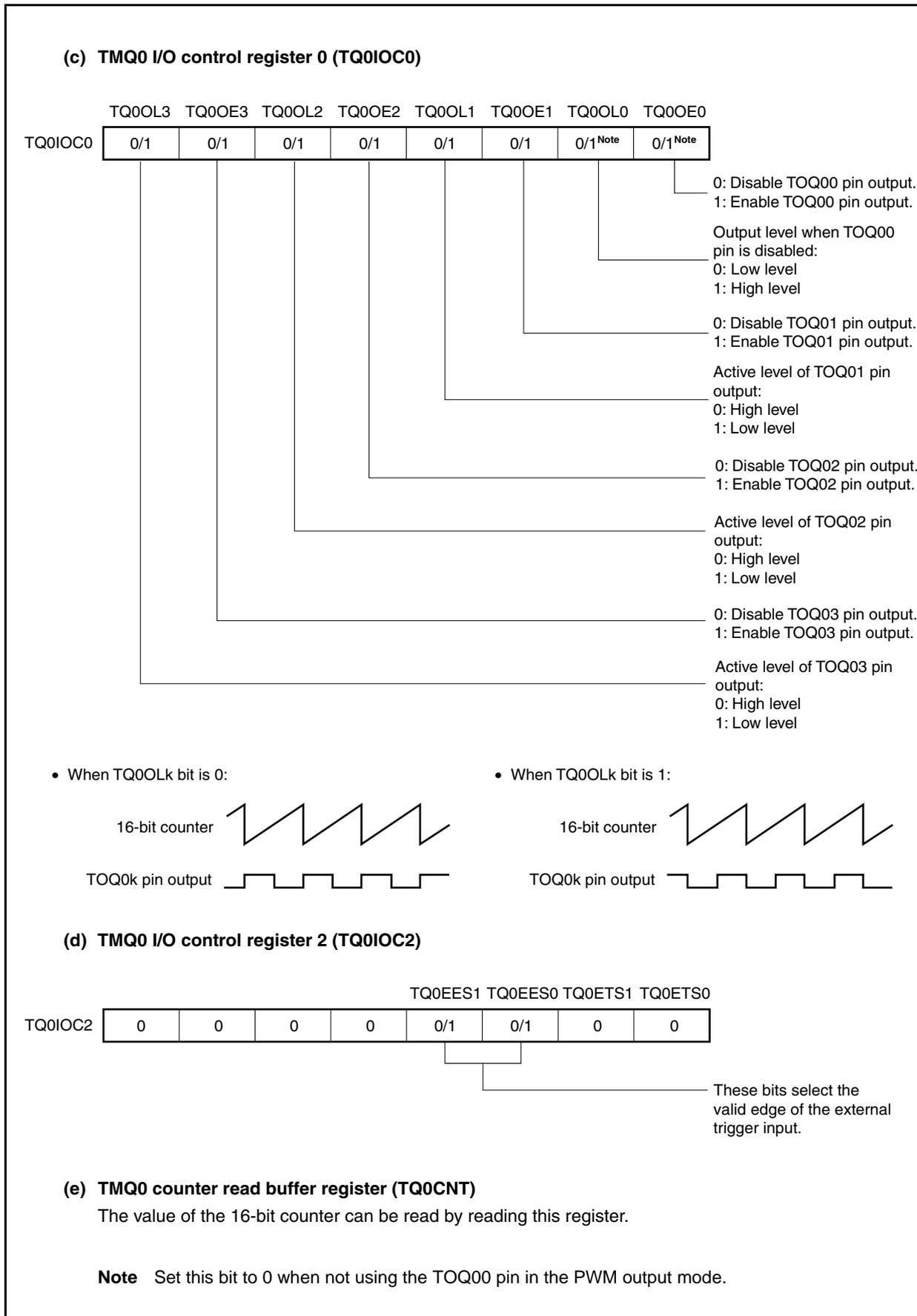
Figure 8-46. Register Settings in PWM Output Mode (3/3)
