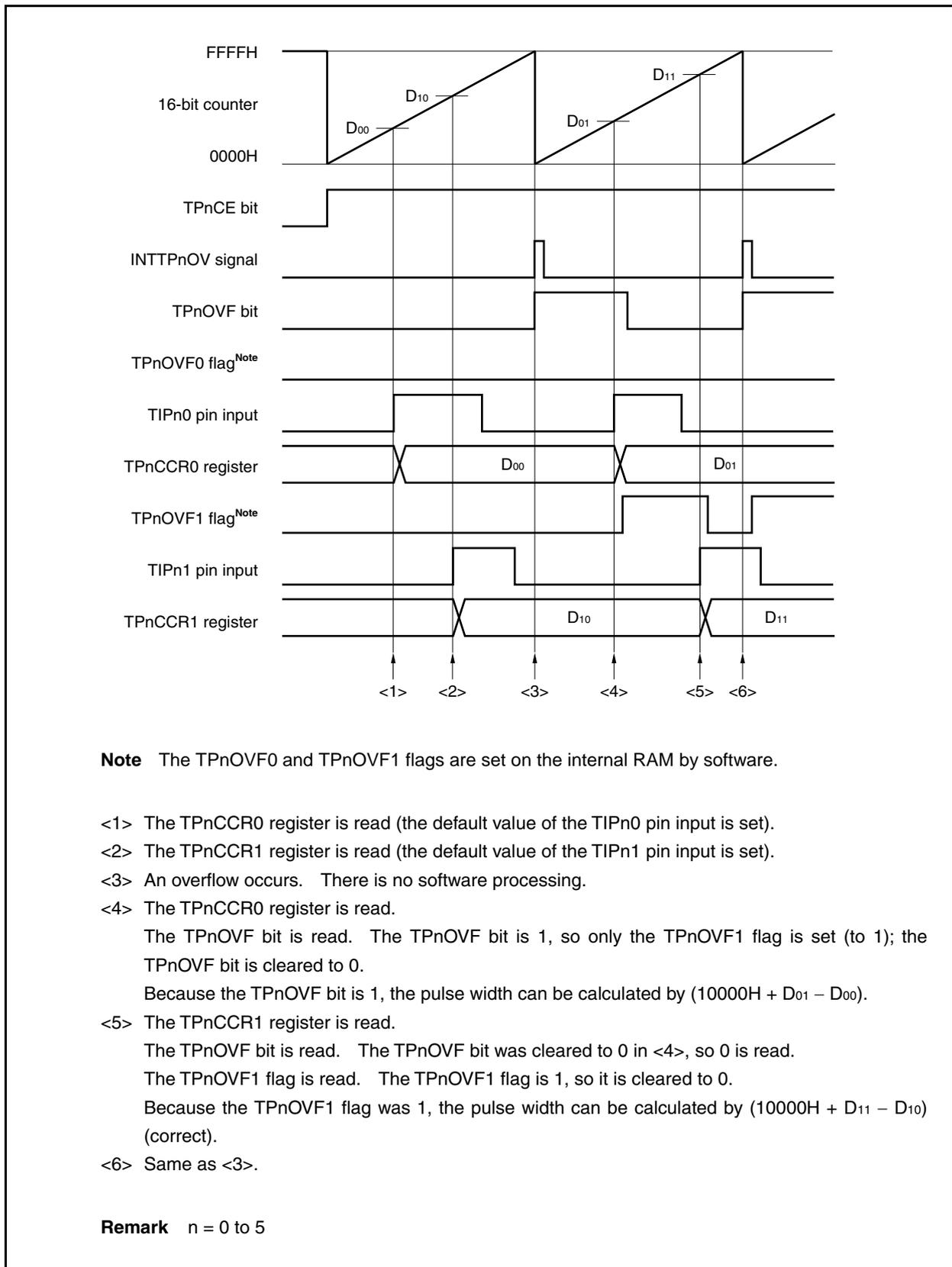
**(d) Processing of overflow if capture trigger interval is long**
