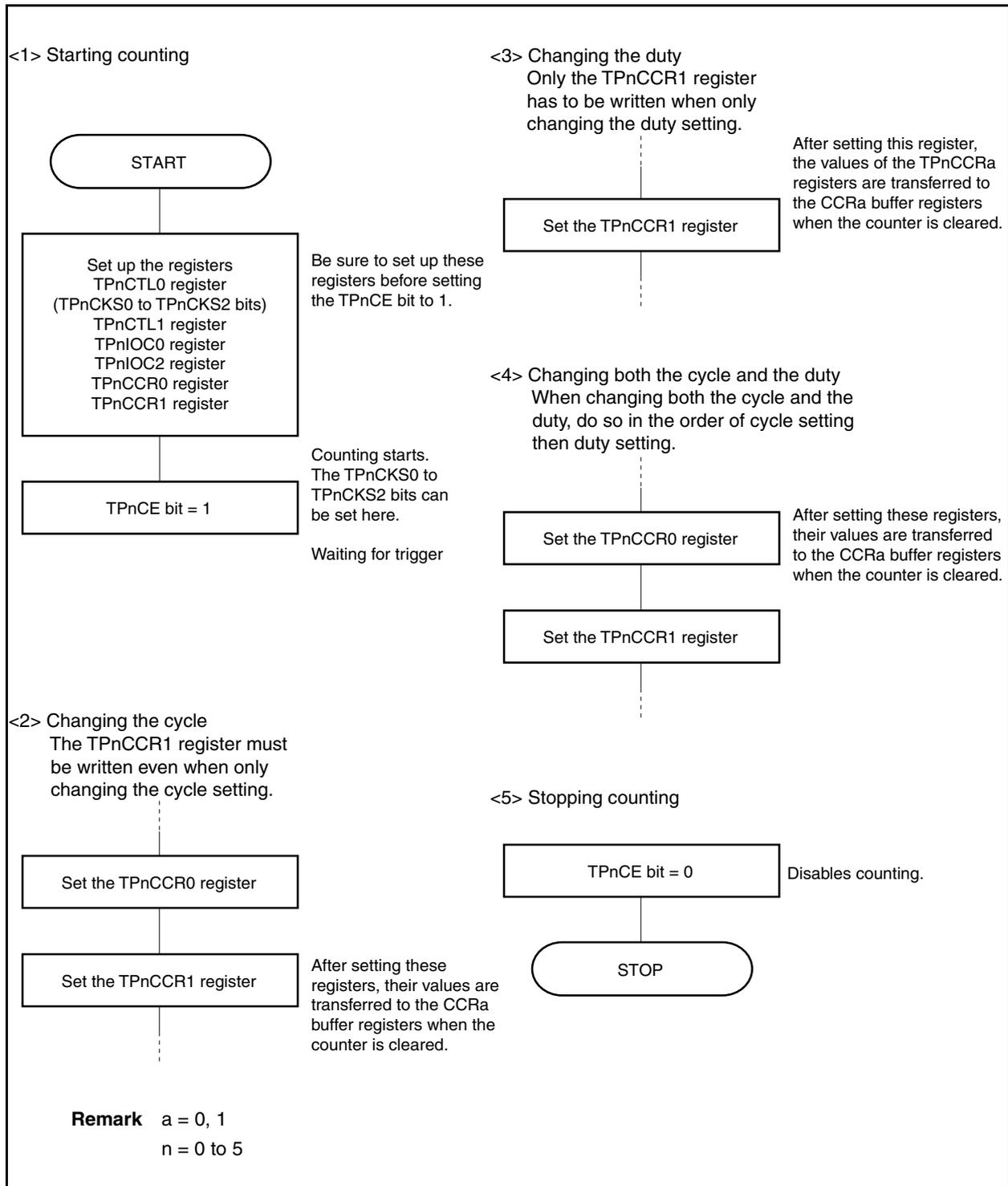
**(2) Using external trigger pulse output mode**
