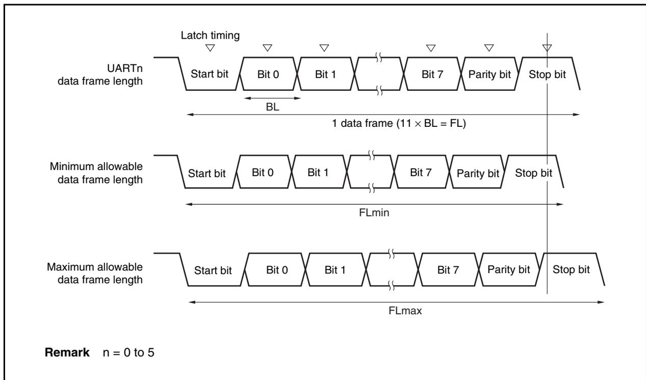
As shown in Figure 16-18, the receive data latch timing is determined by the counter set using the UAnCTL2 register following start bit detection. The transmit data can be received normally if up to the last data (stop bit) can be received in time for this latch timing.
