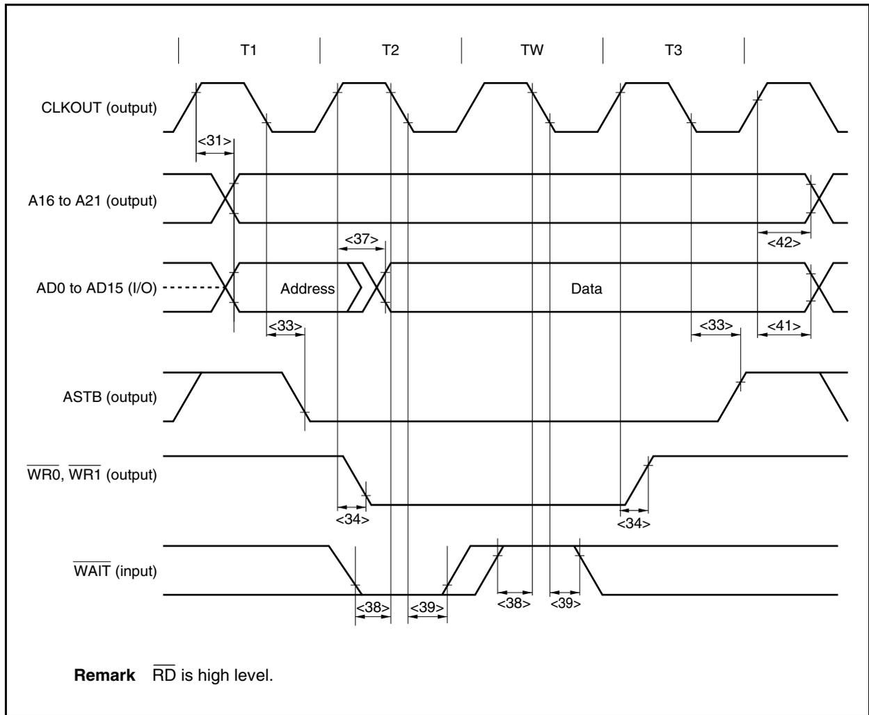
**(2) Bus hold****(a) Asynchronous to CLKOUT**
