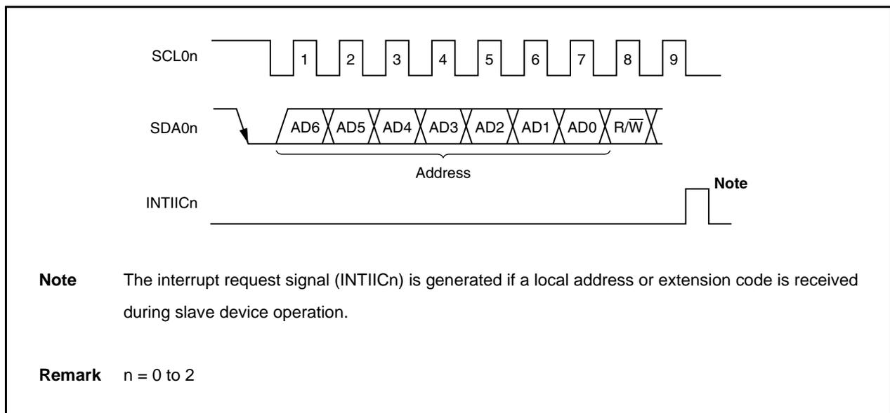
The slave address and the eighth bit, which specifies the transfer direction as described in **19.6.3 Transfer direction specification** below, are written together to IIC shift register n (IICn) and then output. Received addresses are written to the IICn register (n = 0 to 2).
