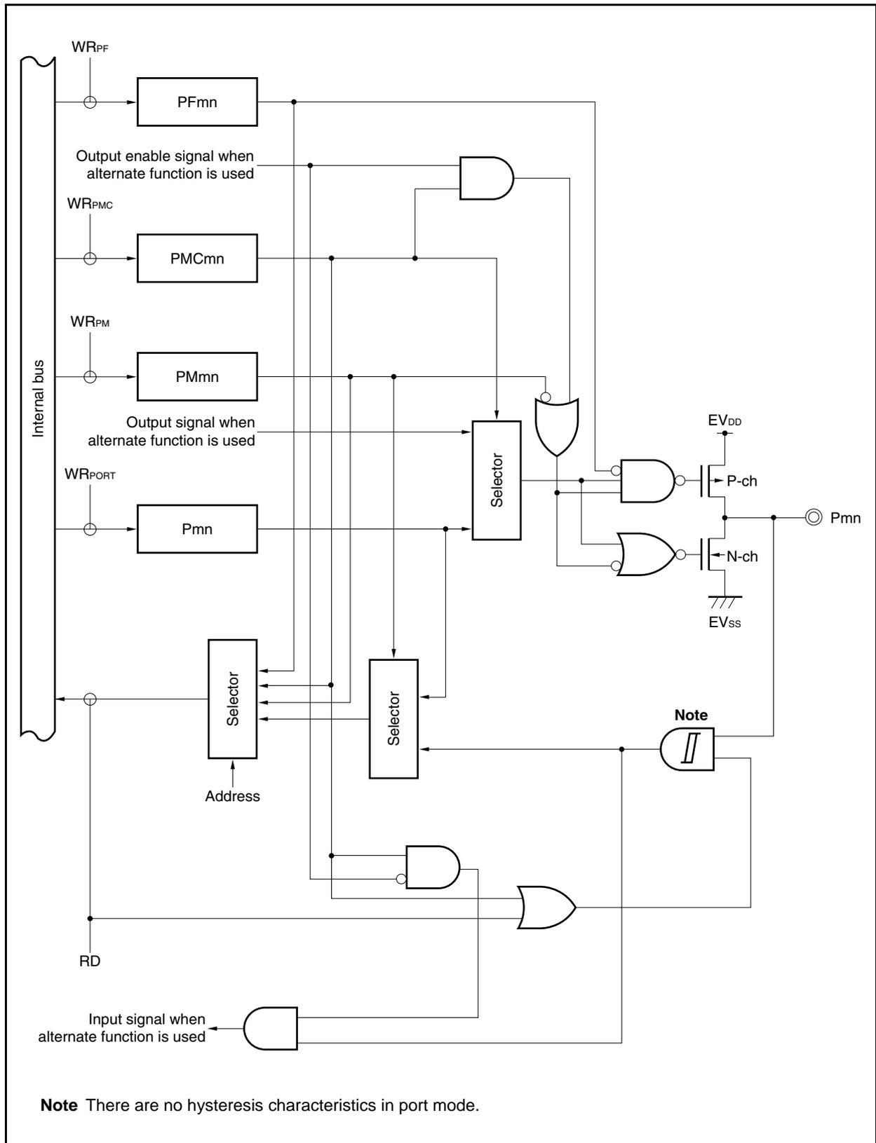
Figure 4-10. Block Diagram of Type G-1
