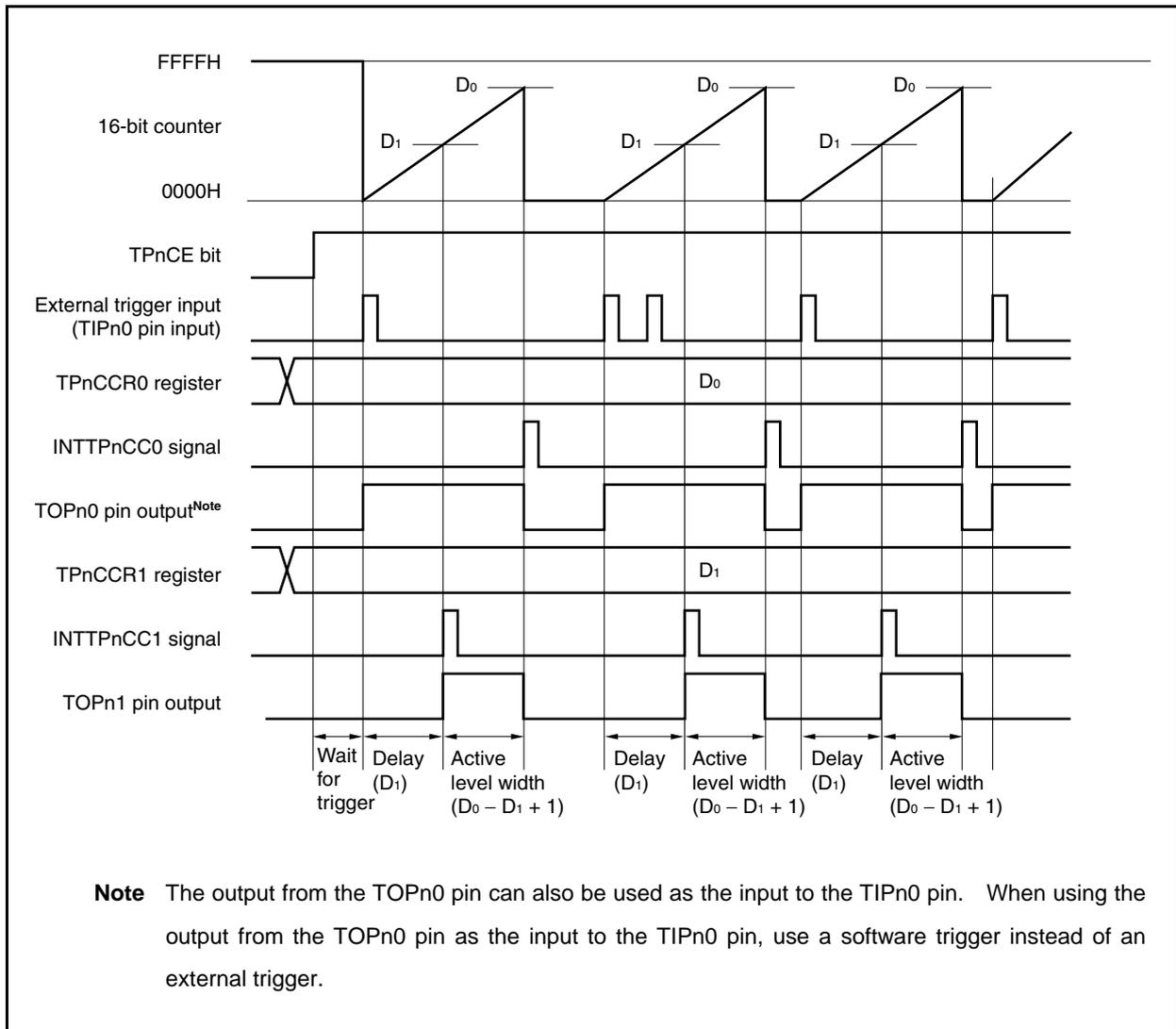
When the TPnCE bit is set to 1, TMPn waits for a trigger. When the trigger is generated, the 16-bit counter is cleared from FFFFH to 0000H, starts incrementing, and outputs a one-shot pulse from the TOPn1 pin. After the one-shot pulse is output, the 16-bit counter is set to 0000H, stops incrementing, and waits for a trigger. If a trigger is generated again while the one-shot pulse is being output, it is ignored.
