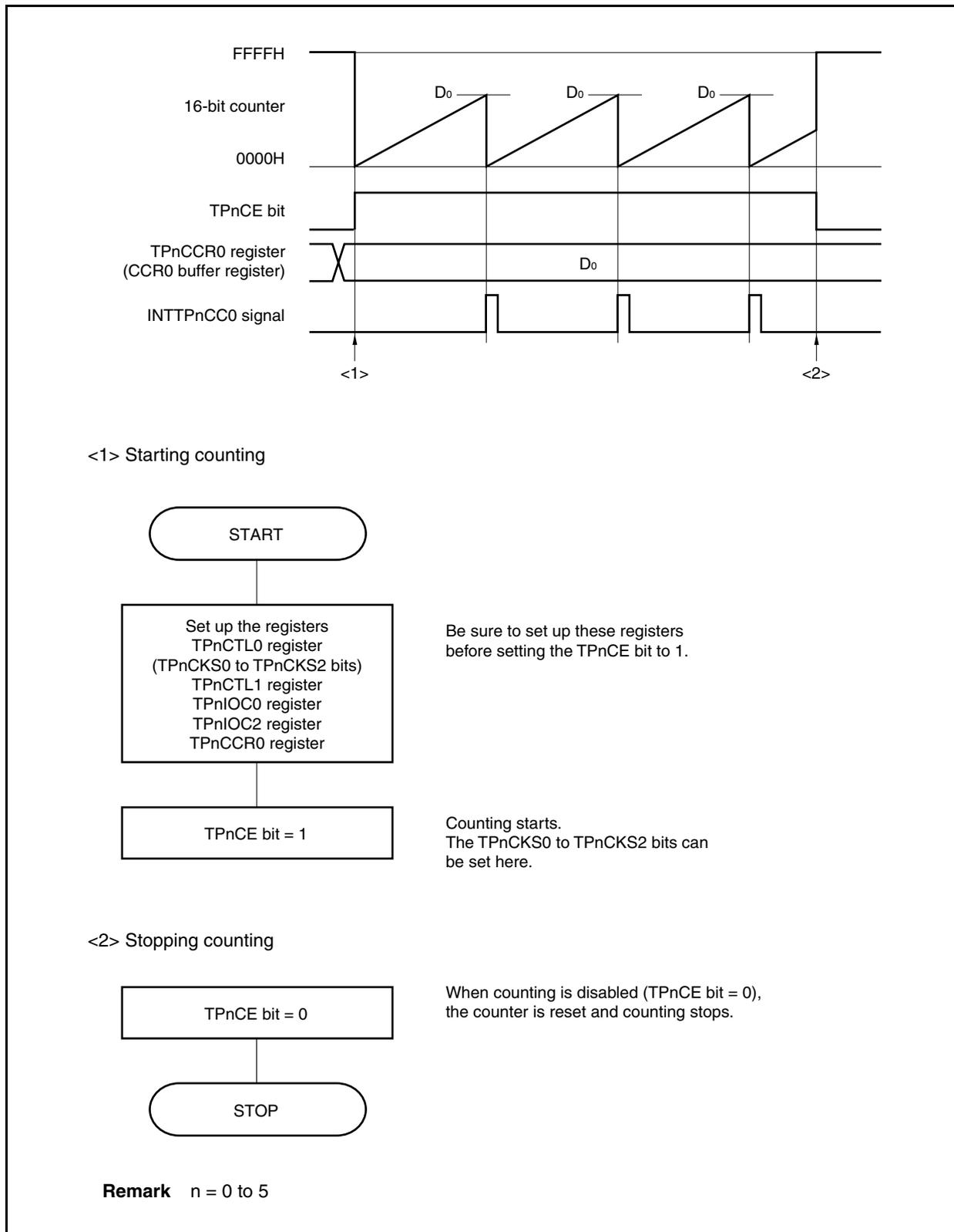
**(2) Using external event count mode****(a) Operation when TPnCCR0 register is set to FFFFH**
