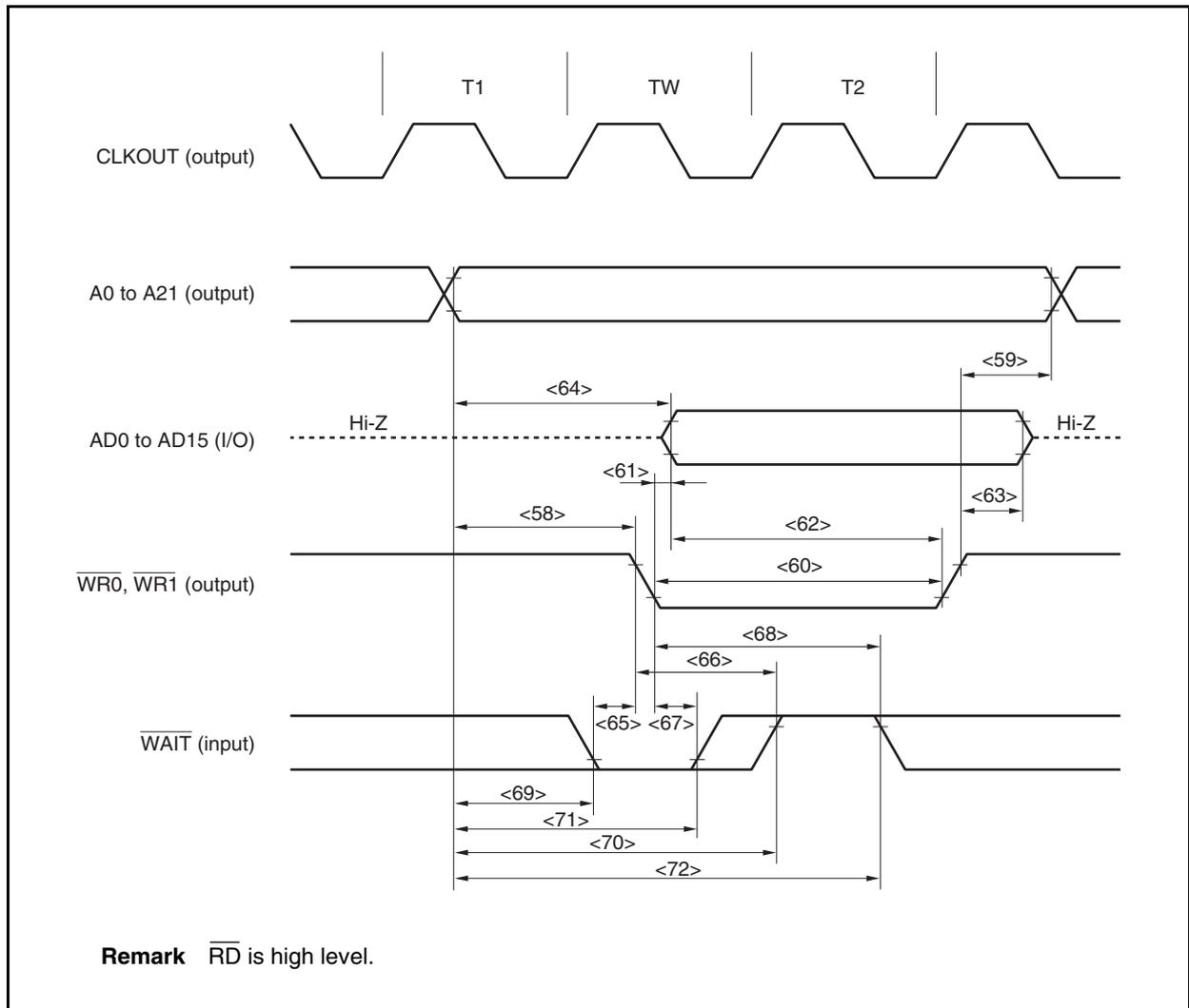
**(c) Read cycle (Synchronous with CLKOUT): In separate bus mode**
