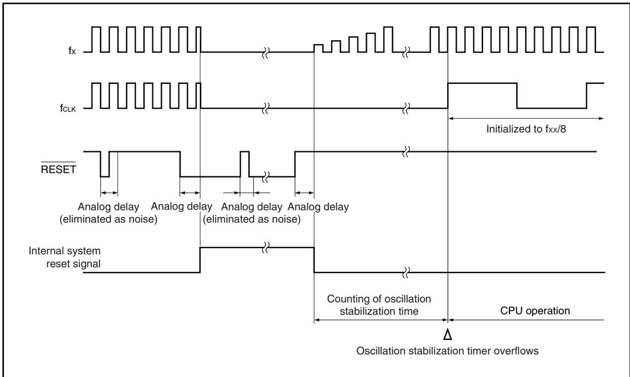
Figure 24-3. Timing of Power-on Reset Operation
