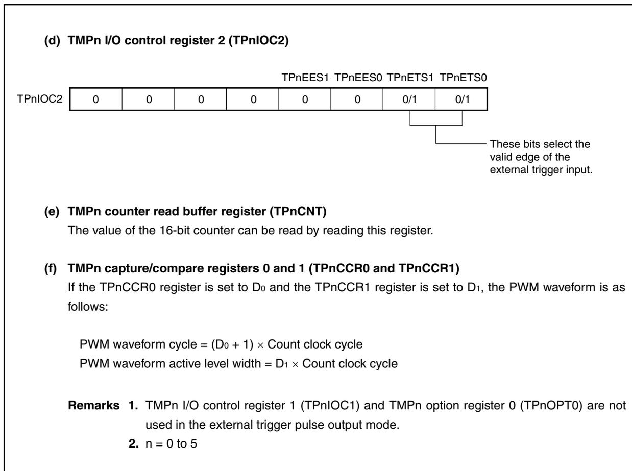
(1) Operations in external trigger pulse output mode
