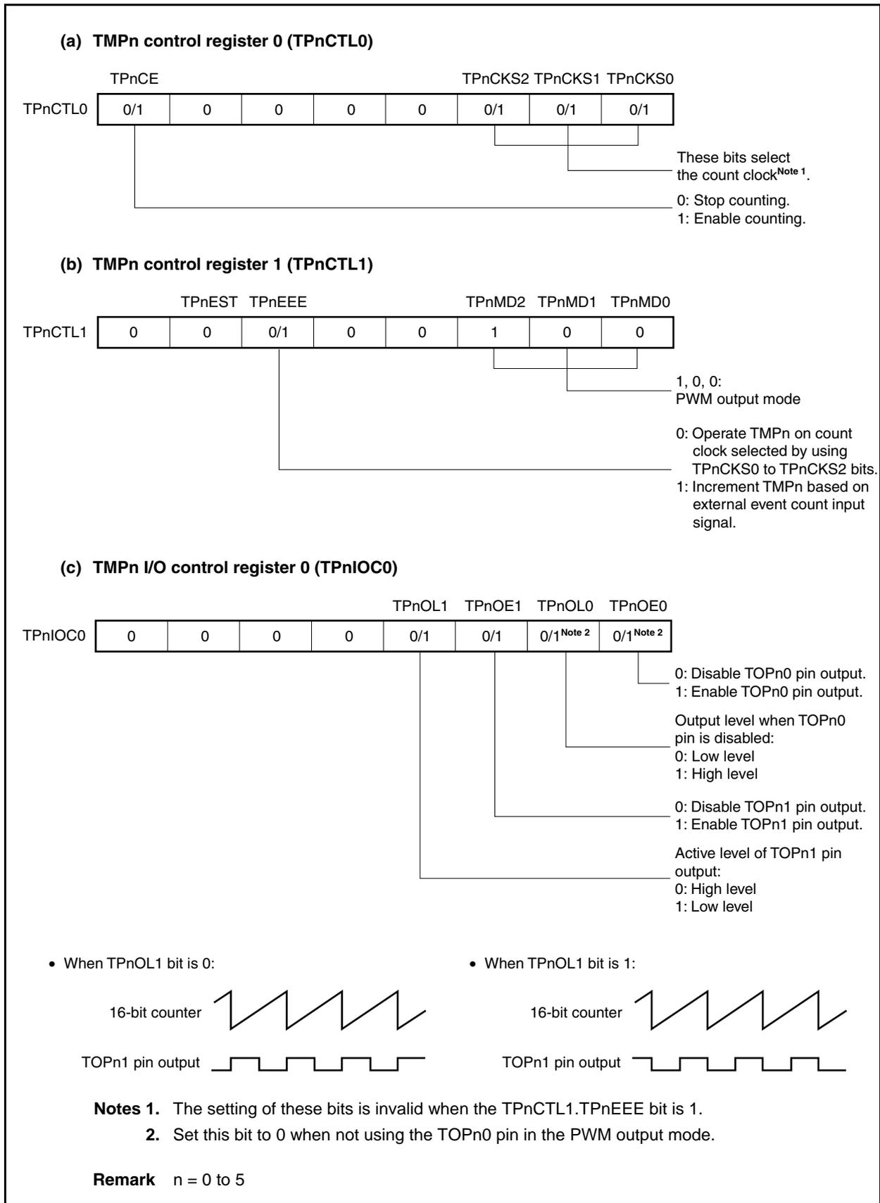
Figure 7-46. Register Settings in PWM Output Mode (2/2)
