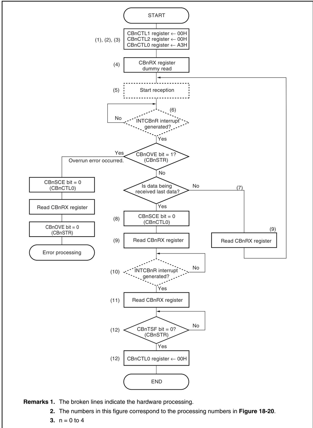
Figure 18-20. Continuous Transfer Mode Operation Timing (Master Mode, Reception Mode)
