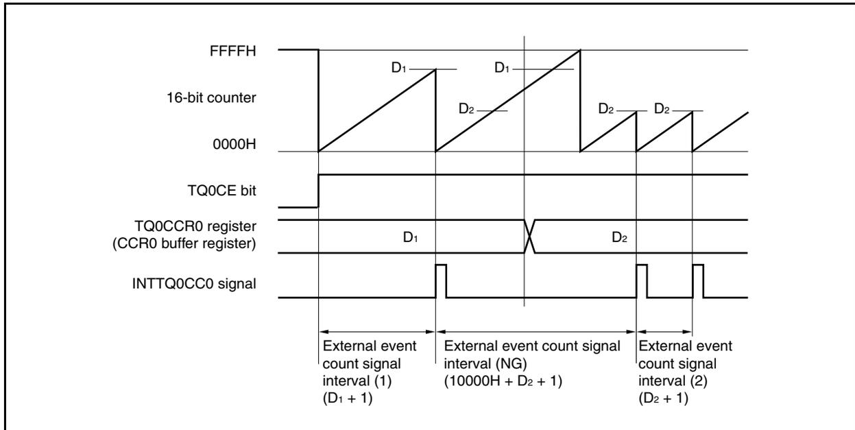
If the value of the TQ0CCR0 register is changed from  $D_1$  to  $D_2$  while the counter value is greater than  $D_2$  but less than  $D_1$ , the TQ0CCR0 register value is transferred to the CCR0 buffer register as soon as the register has been rewritten. Consequently, the value that is compared with the 16-bit counter value is  $D_2$ .
