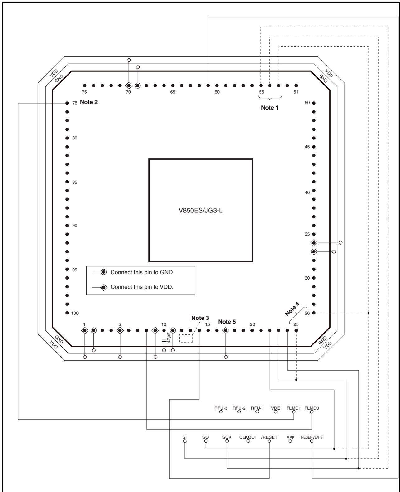
**Figure 30-6 Wiring Example of V850ES/JG3-L Flash Writing Adapter (FA-100GC-UEU-B)
