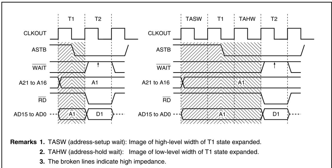
**Figure 5-11. Separate Bus Read Timing (Bus Size: 16 Bits, 16-bit Access)**
