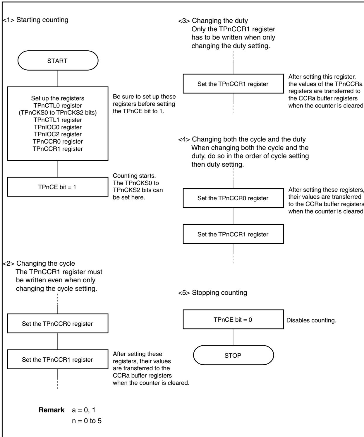
**(2) Using PWM output mode****(a) Changing the PWM waveform while the counter is incrementing**
