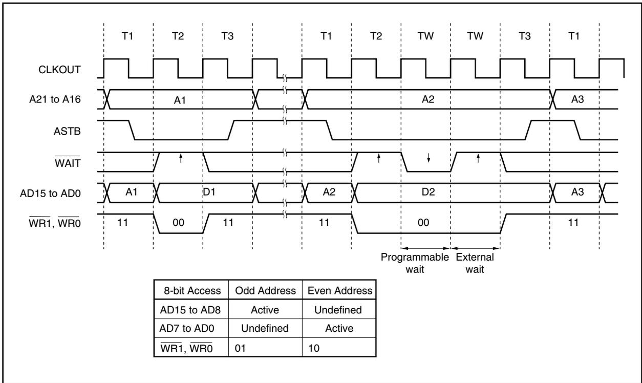
Figure 5-7. Multiplexed Bus Write Timing (Bus Size: 8 Bits)
