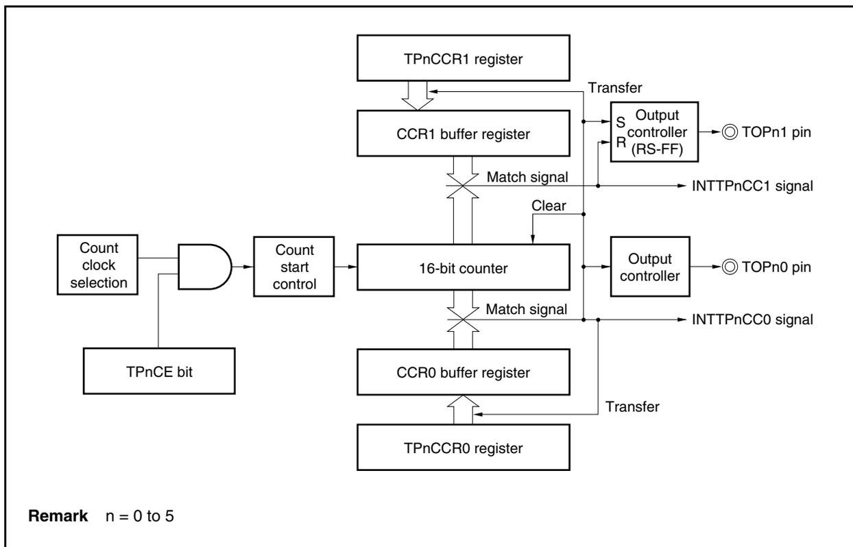
Figure 7-25. Basic Timing in PWM Output Mode
