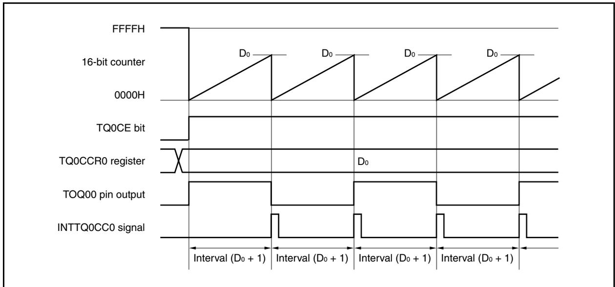
When the TQ0CE bit is set to 1, the value of the 16-bit counter is cleared from FFFFH to 0000H in synchronization with the count clock, and the counter starts counting. At this time, the output of the TOQ00 pin is inverted. Additionally, the set value of the TQ0CCR0 register is transferred to the CCR0 buffer register.
