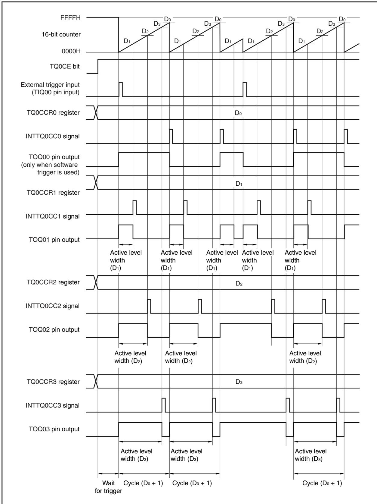
16-bit timer/event counter Q waits for a trigger when the TQ0CE bit is set to 1. When the trigger is generated, the 16-bit counter is cleared from FFFFH to 0000H, starts counting at the same time, and outputs a PWM waveform from the TOQ0k pin. If the trigger is generated again while the counter is operating, the counter is cleared to 0000H and restarted. (The output of the TOQ00 pin is inverted. The TOQ0k pin outputs a high-level regardless of the status (high/low) when a trigger is generated.)
