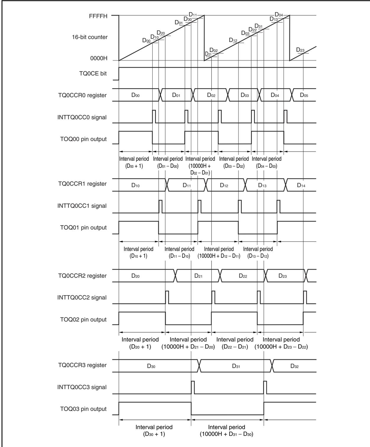
When performing an interval operation in the free-running timer mode, two intervals can be set with one channel.
