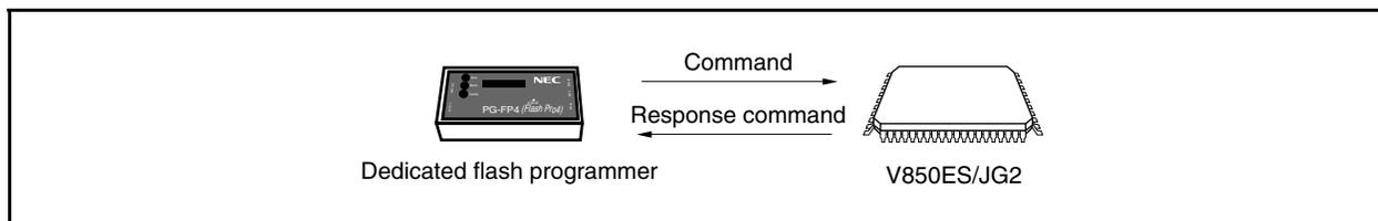
The following shows the commands for flash memory control in the V850ES/JG2. All of these commands are issued from the dedicated flash programmer, and the V850ES/JG2 performs the processing corresponding to the commands.
