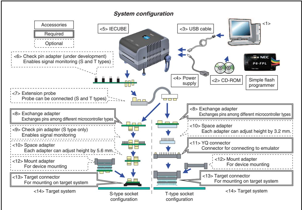
**Figure A-2. System Configuration (When Using QB-V850ESSX2) (2/2)**
