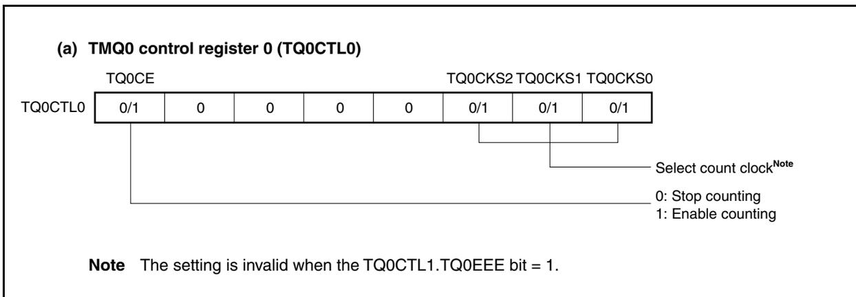
Figure 8-18. Setting of Registers in External Trigger Pulse Output Mode (2/3)
