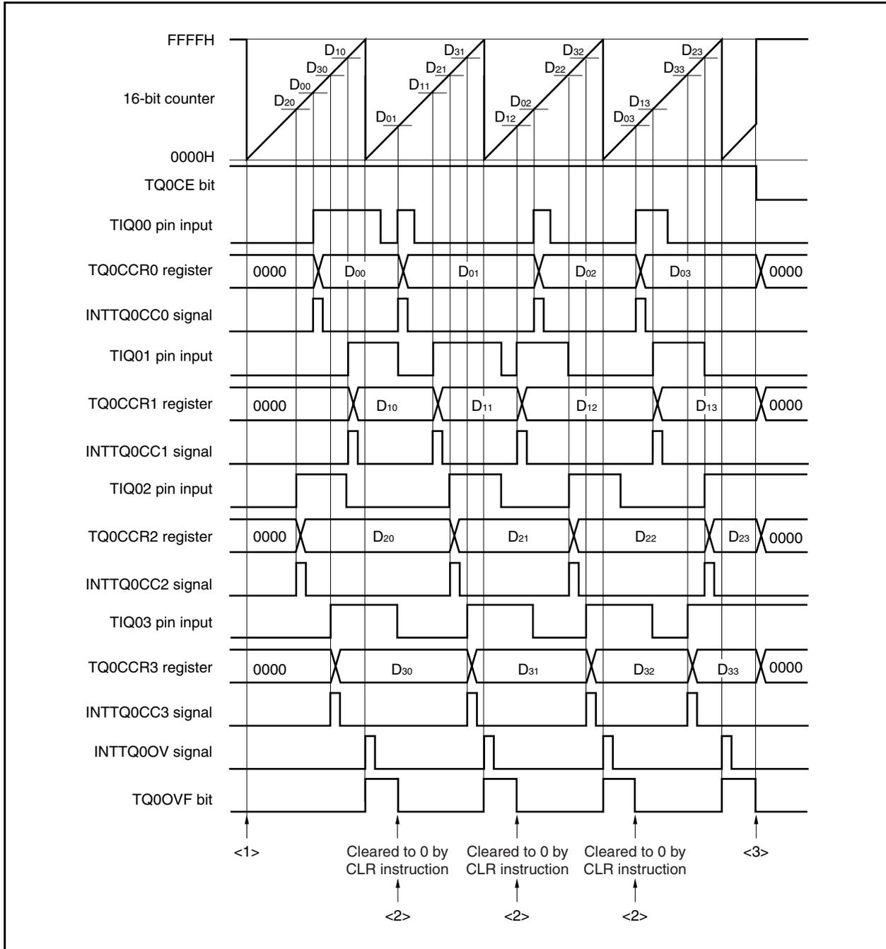
Figure 8-33. Software Processing Flow in Free-Running Timer Mode (Capture Function) (2/2)
