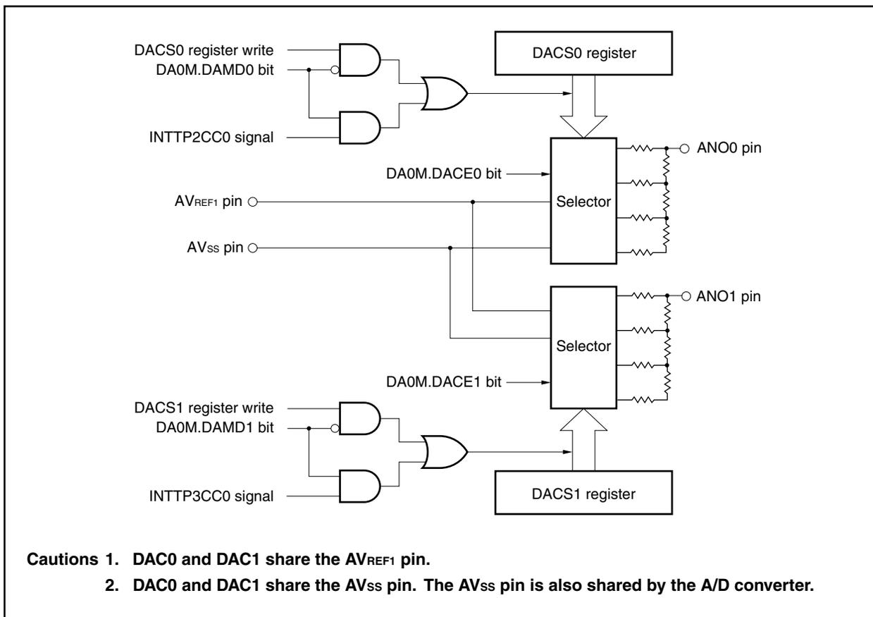
The D/A converter includes the following hardware.
