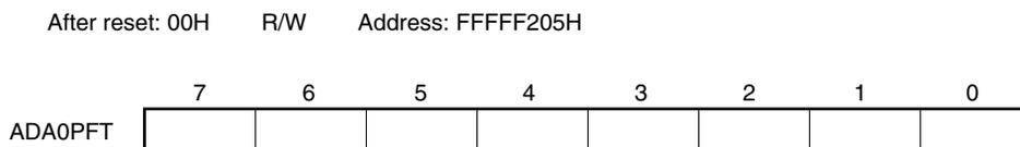
**Caution** In the following modes, write data to the ADA0PFT register while A/D conversion is stopped (ADA0M0.ADA0CE bit = 0), and then enable the A/D conversion operation (ADA0CE bit = 1).
