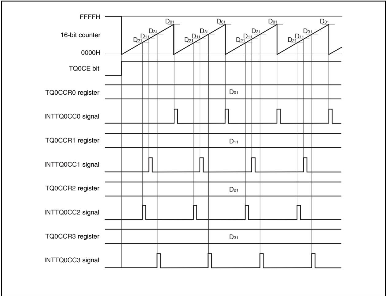
If the set value of the TQ0CCRk register is greater than the set value of the TQ0CCR0 register, the INTTQ0CCk signal is not generated because the count value of the 16-bit counter and the value of the TQ0CCRk register do not match.
