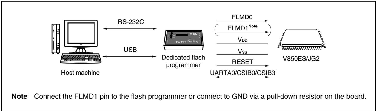
A host machine is required for controlling the dedicated flash programmer.
