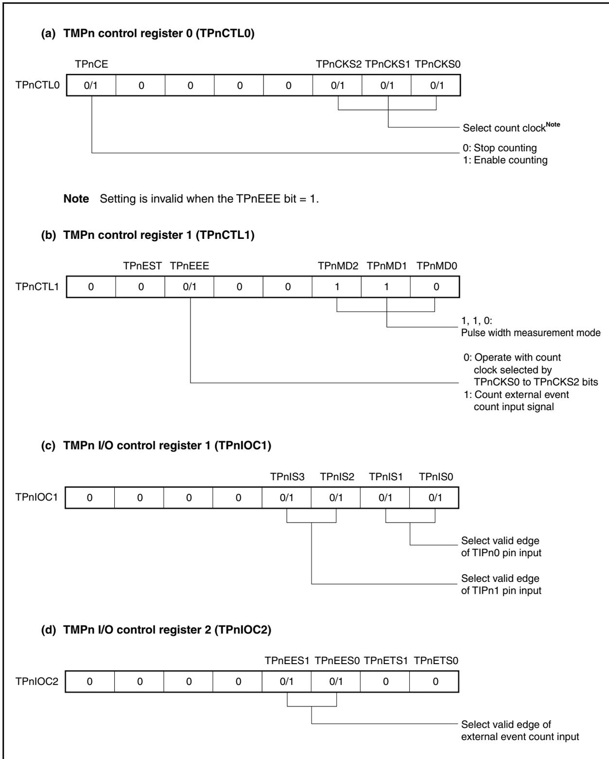
Figure 7-36. Register Setting in Pulse Width Measurement Mode (2/2)
