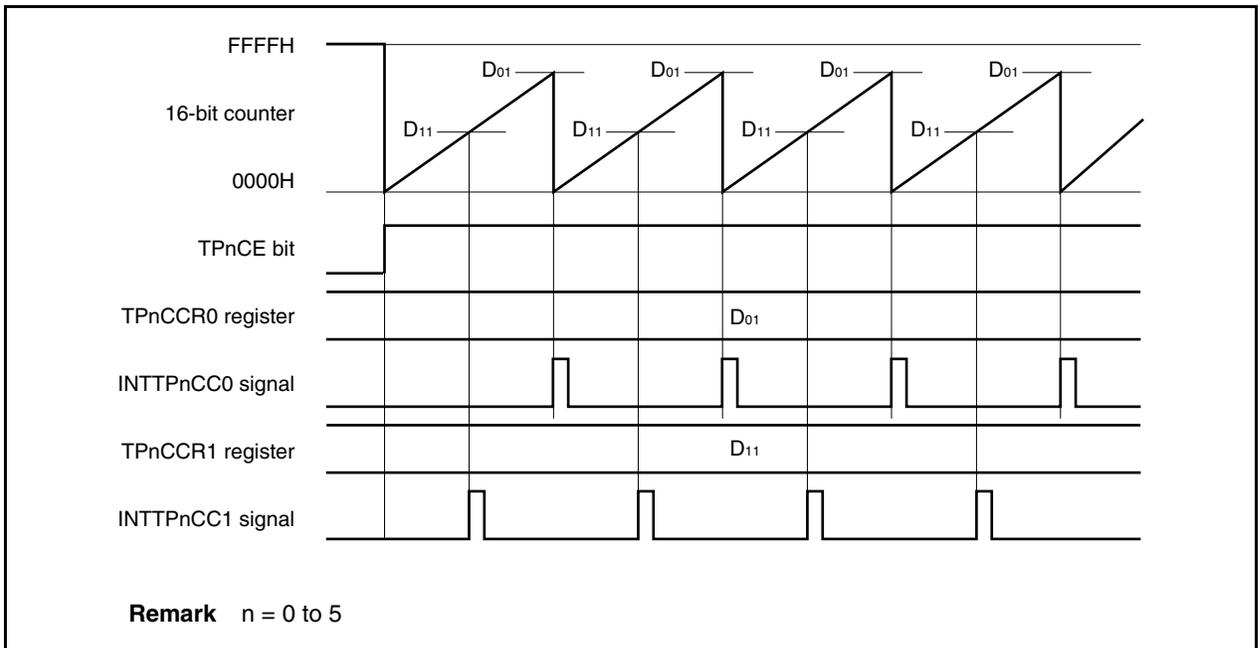
If the set value of the TPnCCR1 register is greater than the set value of the TPnCCR0 register, the INTTPnCC1 signal is not generated because the count value of the 16-bit counter and the value of the TPnCCR1 register do not match.
