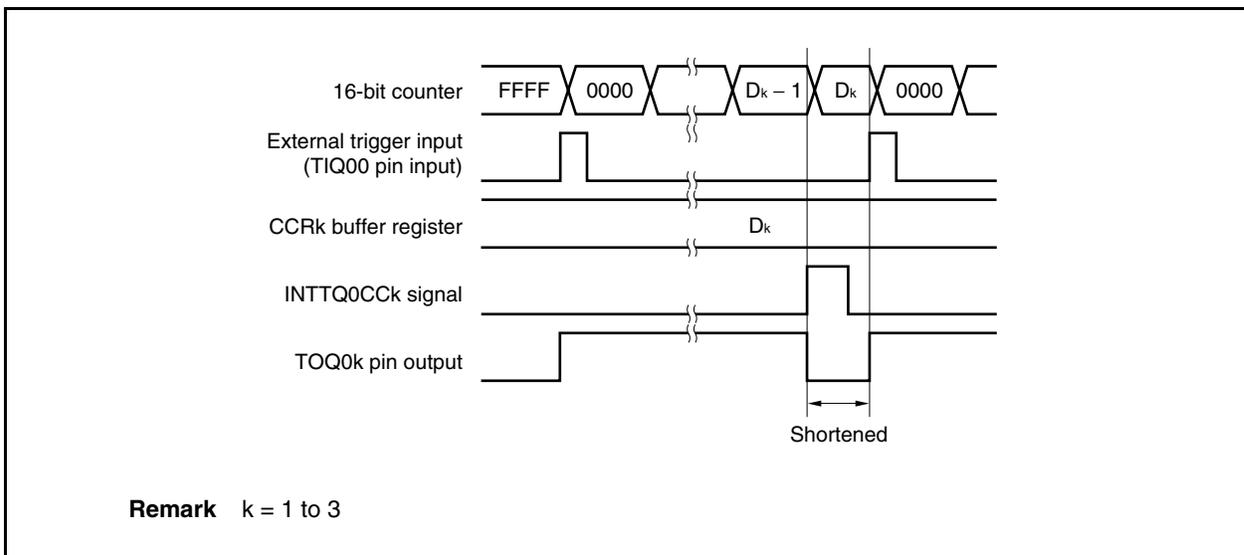
If the trigger is detected immediately before the INTTQ0CCk signal is generated, the INTTQ0CCk signal is not generated, and the 16-bit counter is cleared to 0000H and continues counting. The output signal of the TOQ0k pin remains active. Consequently, the active period of the PWM waveform is extended.
