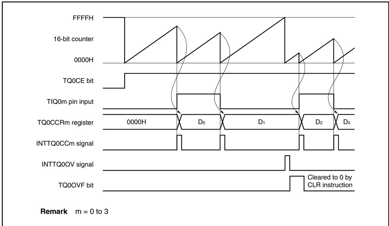
When the TQ0CE bit is set to 1, the 16-bit counter starts counting. When the valid edge input to the TIQ0m pin is later detected, the count value of the 16-bit counter is stored in the TQ0CCRm register, the 16-bit counter is cleared to 0000H, and a capture interrupt request signal (INTTQ0CCm) is generated.
