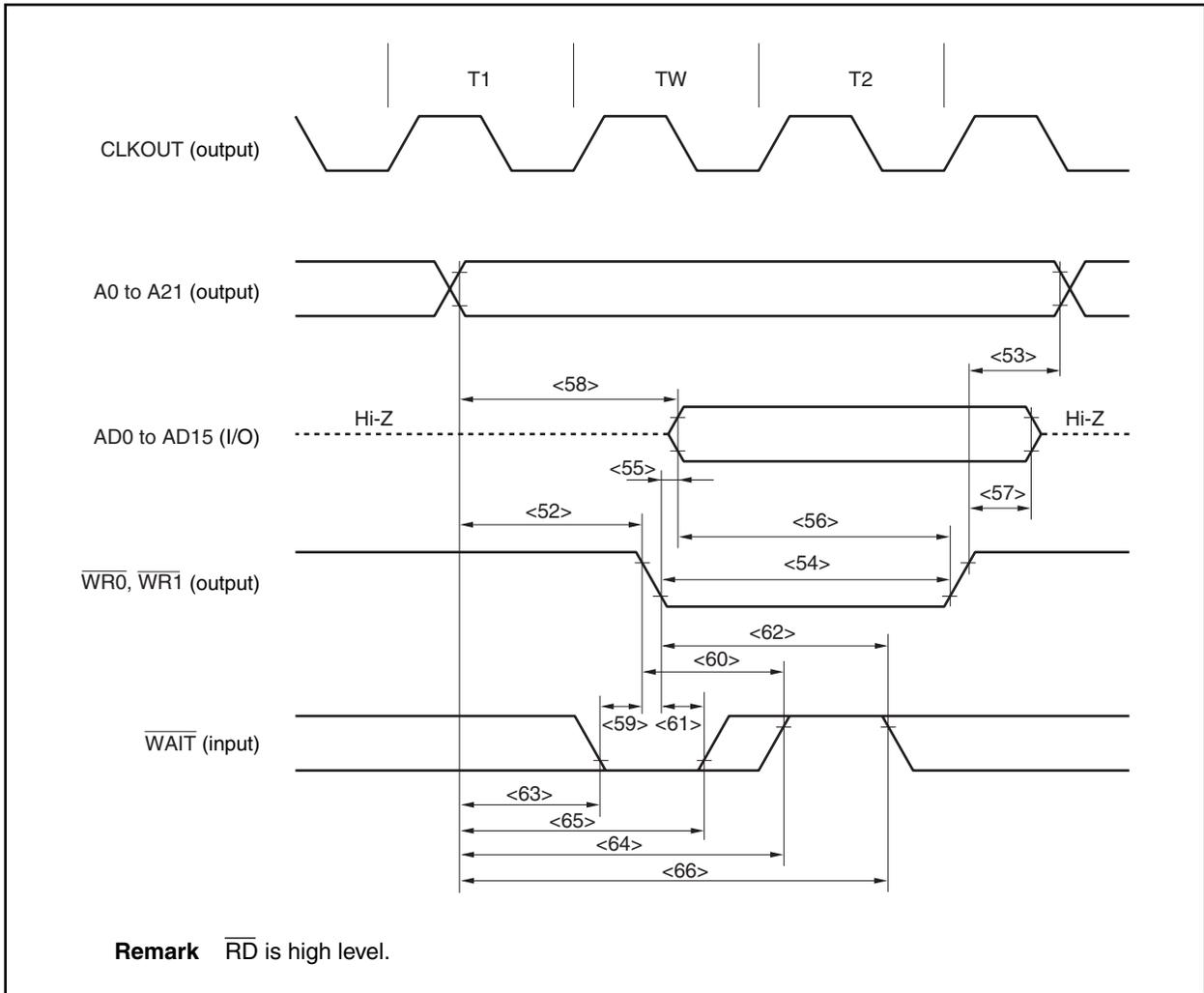
(c) Read cycle (CLKOUT synchronous): In separate bus mode
