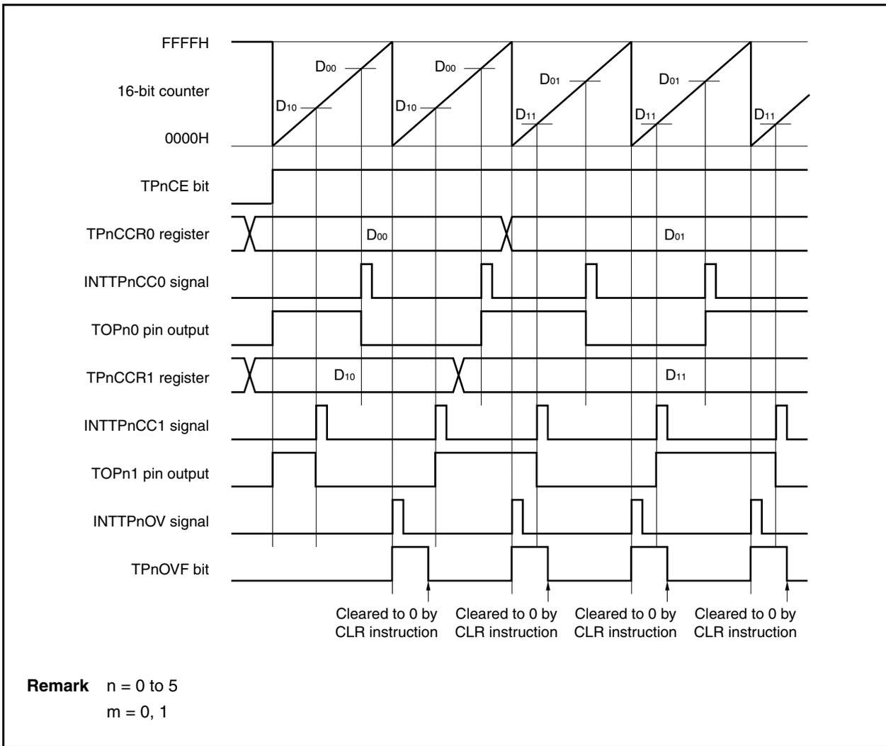
When the TPnCE bit is set to 1, the 16-bit counter starts counting. When the valid edge input to the TIPnm pin is detected, the count value of the 16-bit counter is stored in the TPnCCRm register, and a capture interrupt request signal (INTTPnCCm) is generated.
