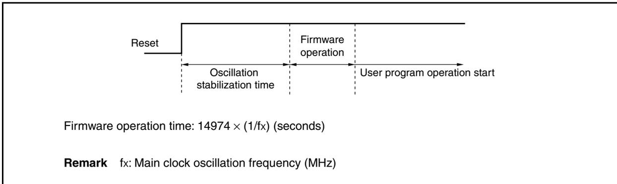
Since the firmware uses a part of the internal RAM, the contents of the following RAM areas are not retained after power-on reset.
