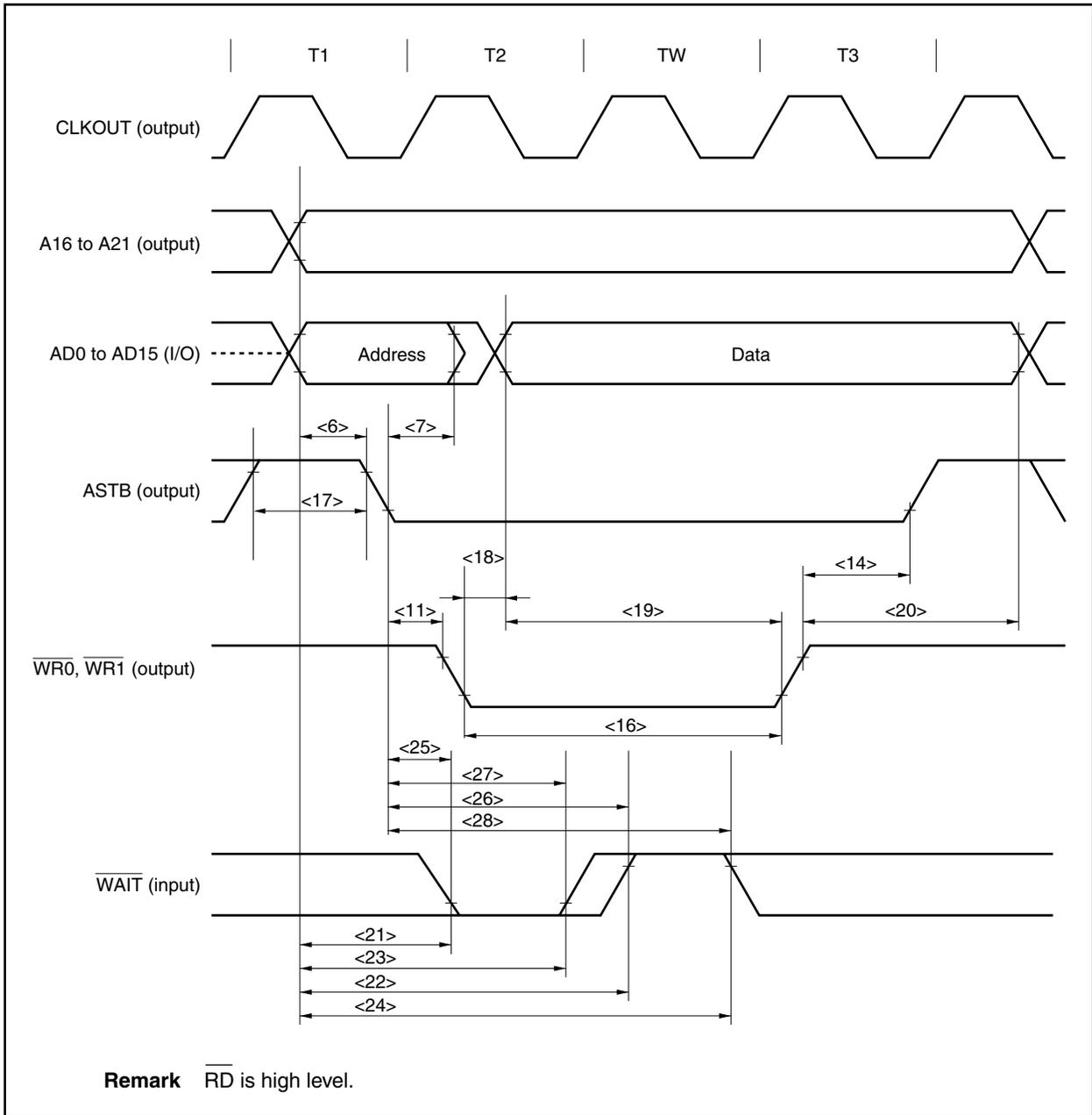
**(b) Read/write cycle (CLKOUT synchronous): In multiplexed bus mode**
