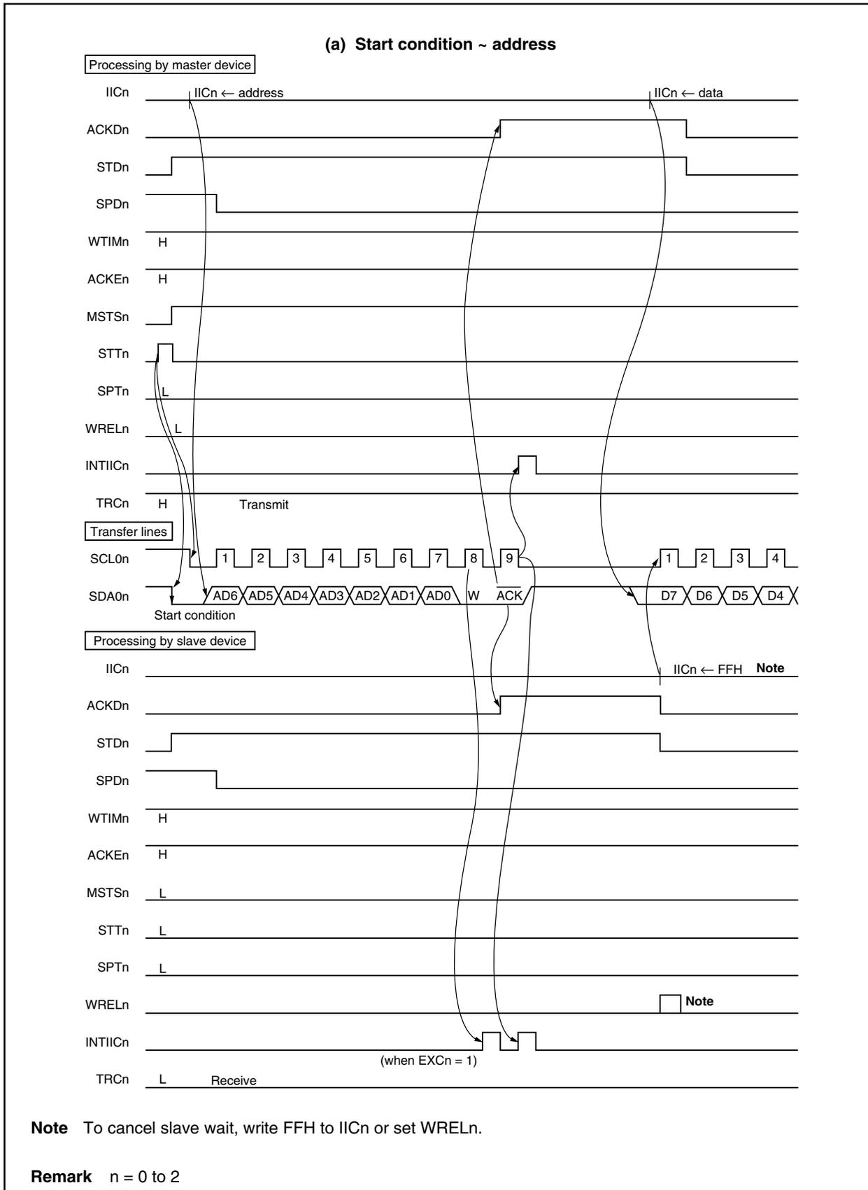
**Figure 17-23. Example of Master to Slave Communication
