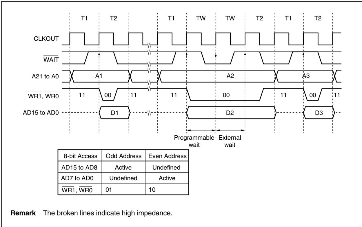
Figure 5-12. Separate Bus Write Timing (Bus Size: 8 Bits)
