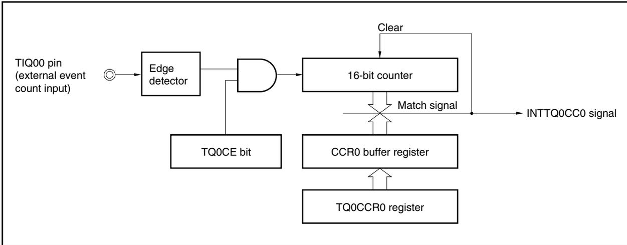
**Figure 8-10. Basic Timing in External Event Count Mode**
