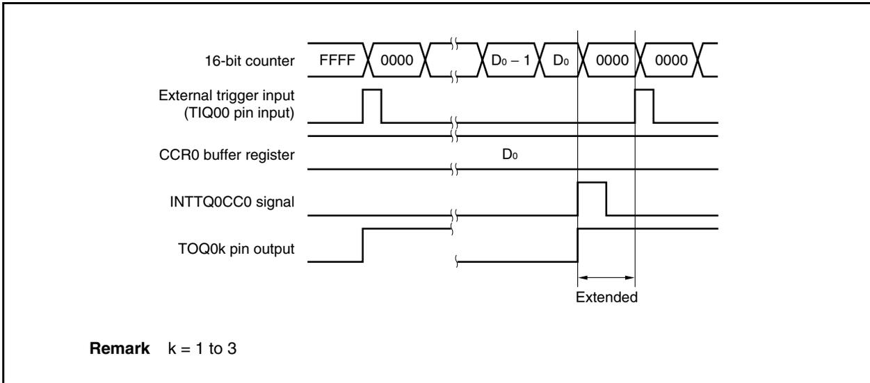
If the trigger is detected immediately before the INTTQ0CC0 signal is generated, the INTTQ0CC0 signal is not generated. The 16-bit counter is cleared to 0000H, the TOQ0k pin is asserted, and the counter continues counting. Consequently, the inactive period of the PWM waveform is shortened.
