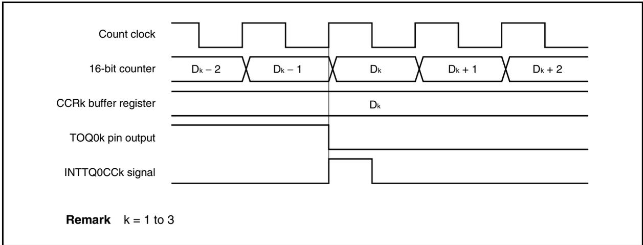
Usually, the INTTQ0CCk signal is generated in synchronization with the next count up after the count value of the 16-bit counter matches the value of the CCRk buffer register.
