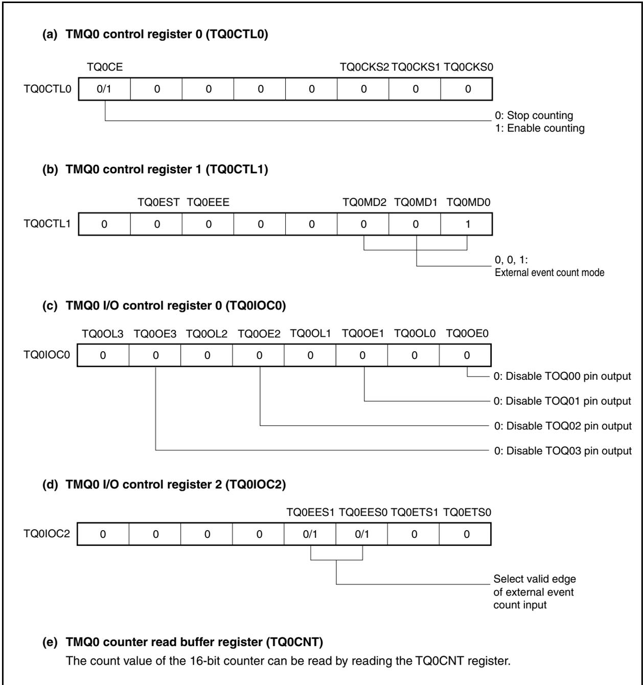
Figure 8-11. Register Setting for Operation in External Event Count Mode (2/2)
