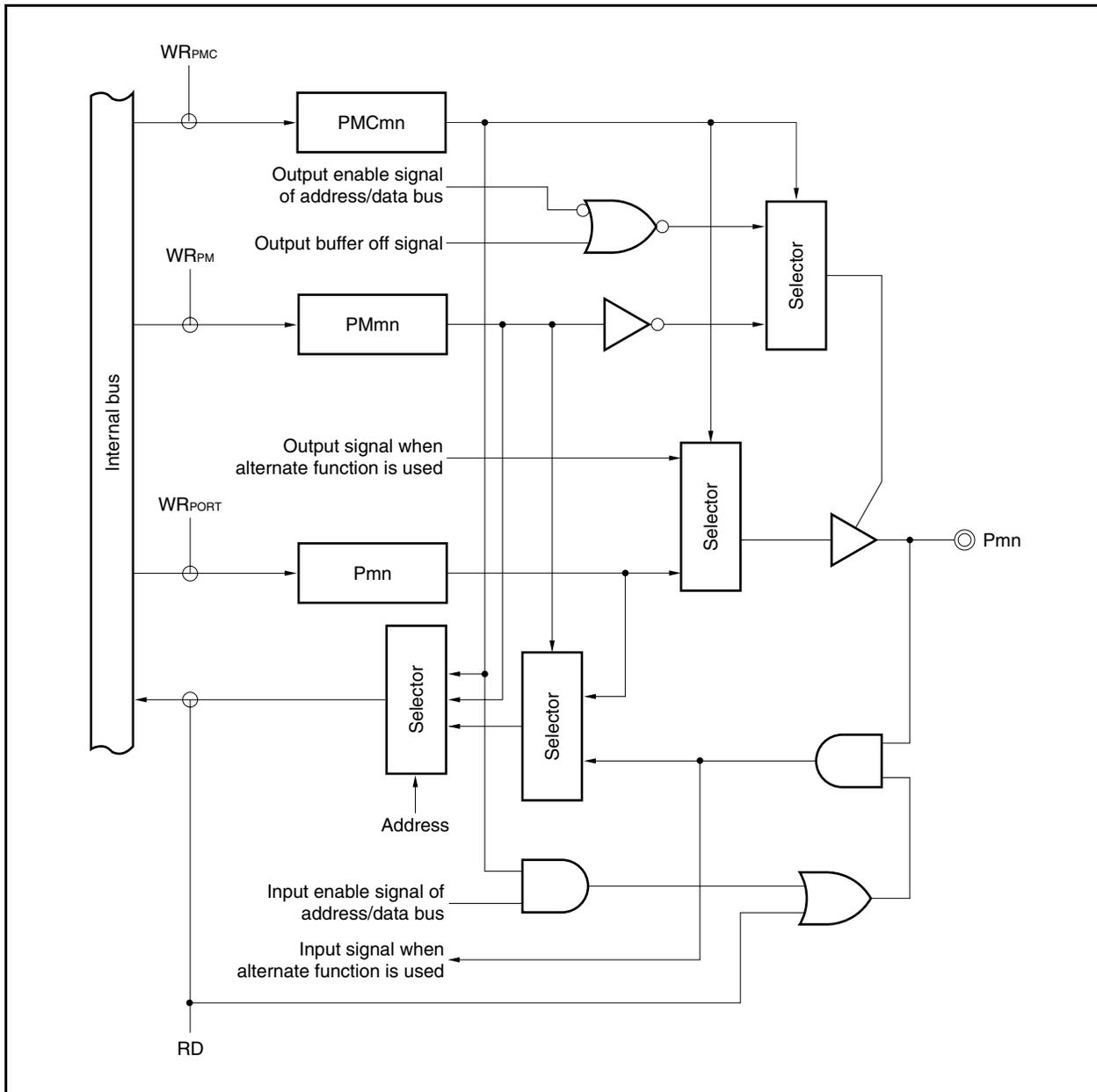
Figure 4-9. Block Diagram of Type E-3
