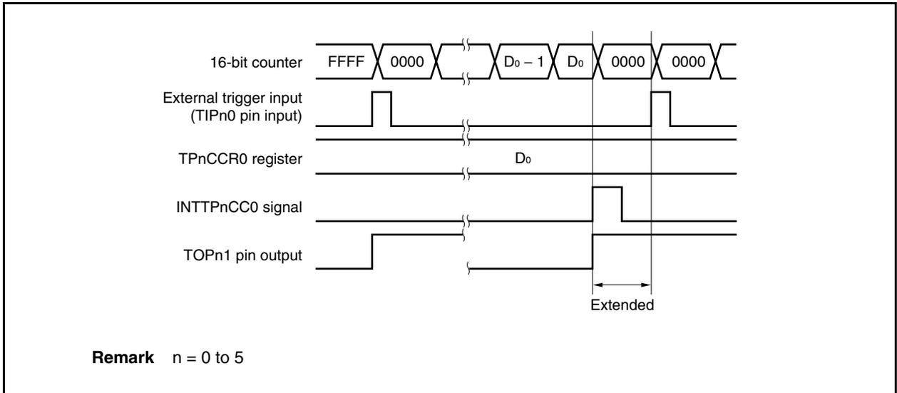
If the trigger is detected immediately before the INTTPnCC0 signal is generated, the INTTPnCC0 signal is not generated. The 16-bit counter is cleared to 0000H, the TOPn1 pin is asserted, and the counter continues counting. Consequently, the inactive period of the PWM waveform is shortened.
