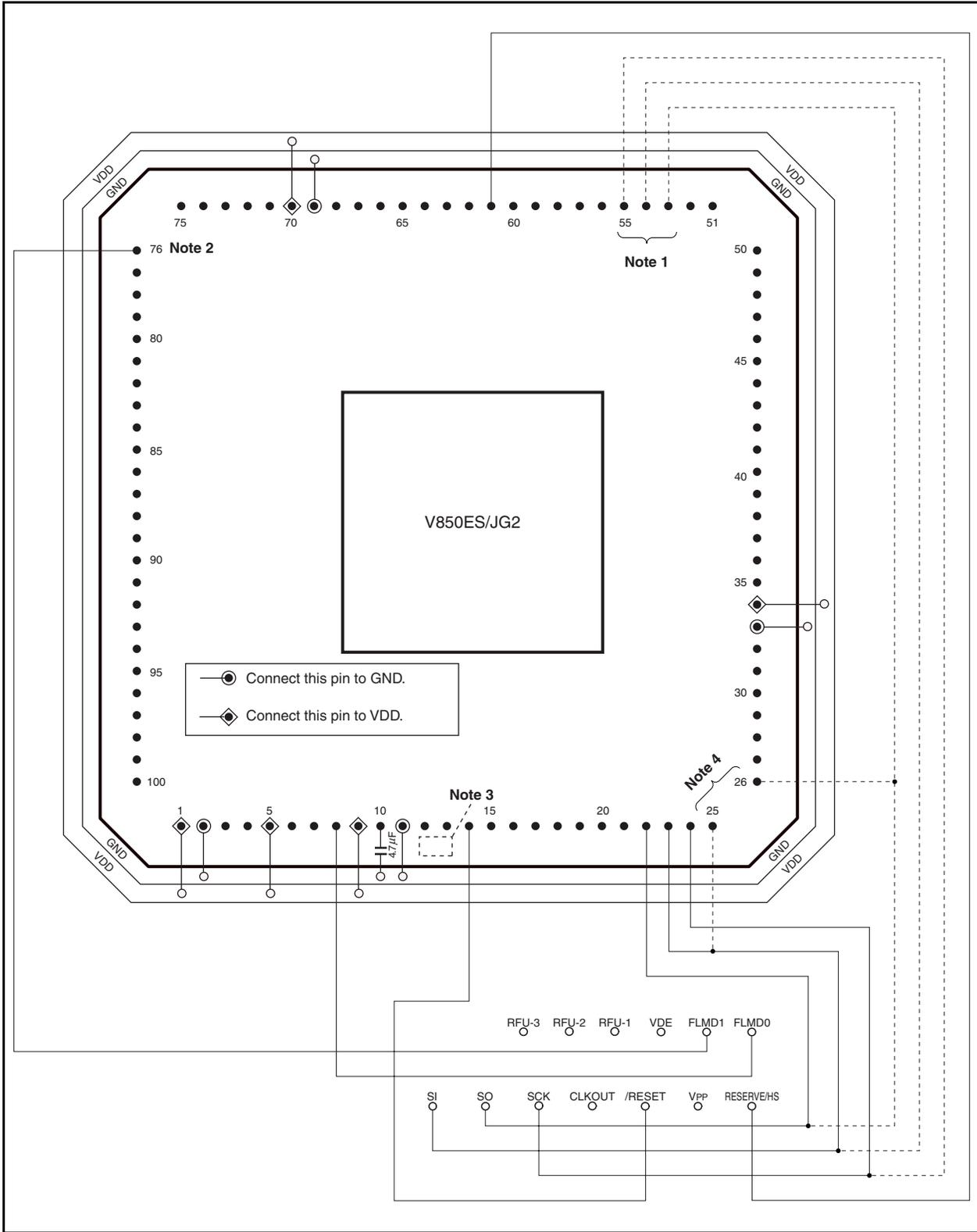
**Figure 26-7. Wiring Example of V850ES/JG2 Flash Writing Adapter (FA-100GC-8EU-A)
