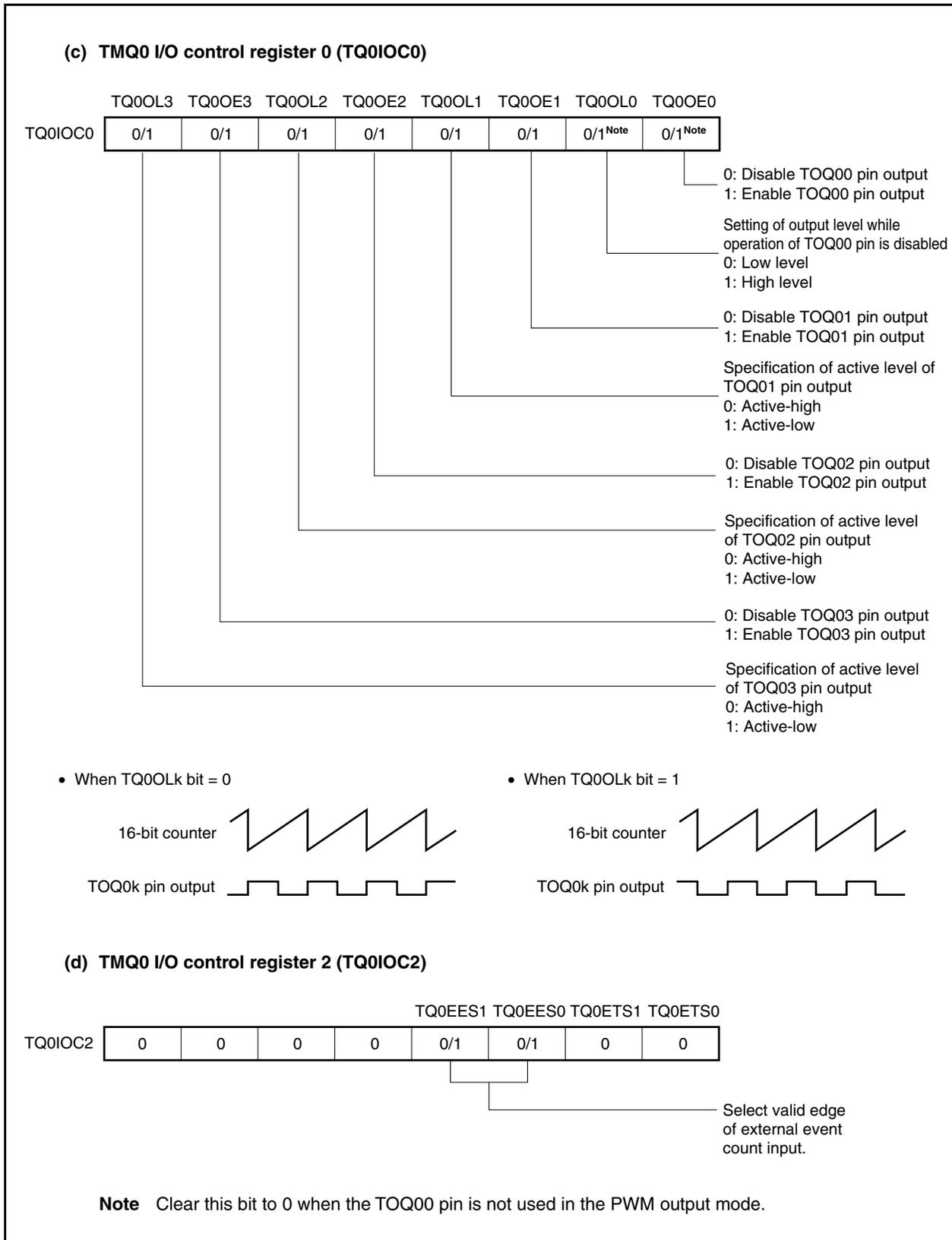
Figure 8-26. Register Setting in PWM Output Mode (3/3)
