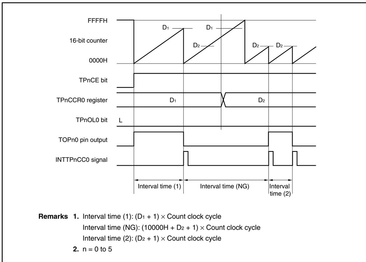
If the value of the TPnCCR0 register is changed from  $D_1$  to  $D_2$  while the count value is greater than  $D_2$  but less than  $D_1$ , the count value is transferred to the CCR0 buffer register as soon as the TPnCCR0 register has been rewritten. Consequently, the value of the 16-bit counter that is compared is  $D_2$ .
