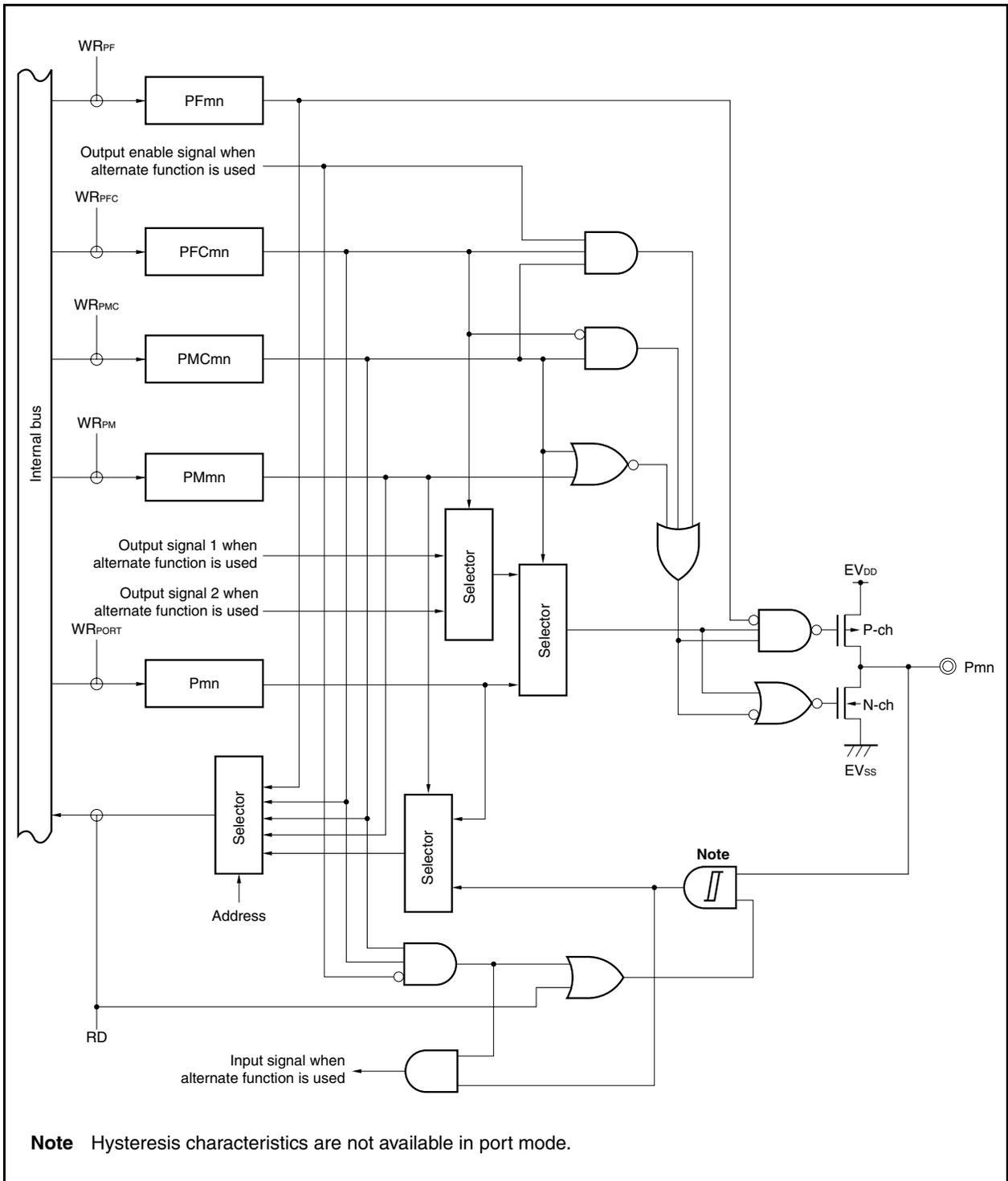
Figure 4-14. Block Diagram of Type G-6
