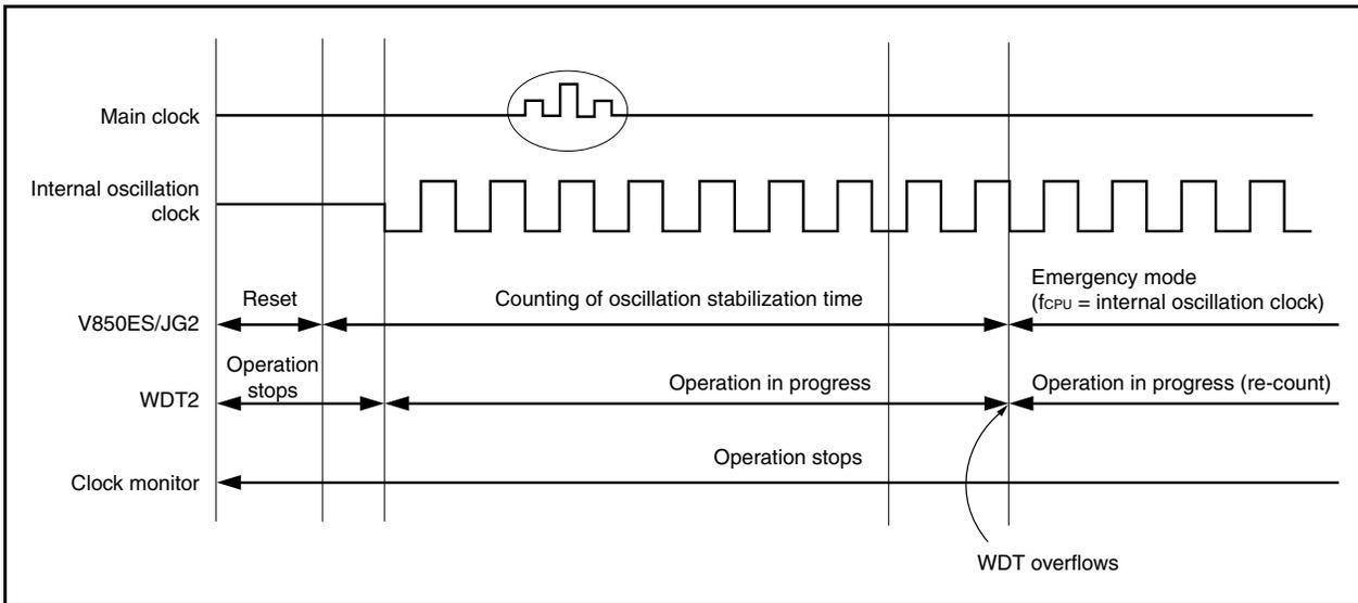
The CPU operation clock states can be checked with the CPU operation clock status register (CCLS).
