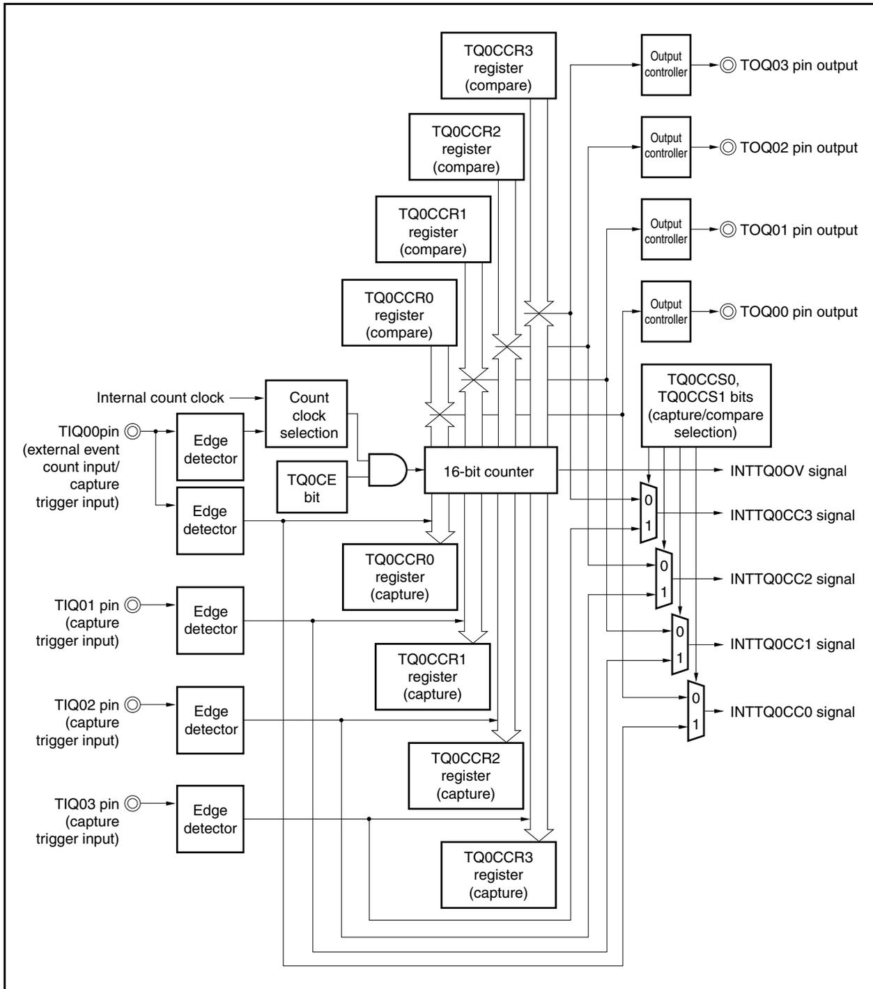
When the TQ0CE bit is set to 1, 16-bit timer/event counter Q starts counting, and the output signals of the TOQ00 to TOQ03 pins are inverted. When the count value of the 16-bit counter later matches the set value of the TQ0CCRm register, a compare match interrupt request signal (INTTQ0CCm) is generated, and the output signal of the TOQ0m pin is inverted.
