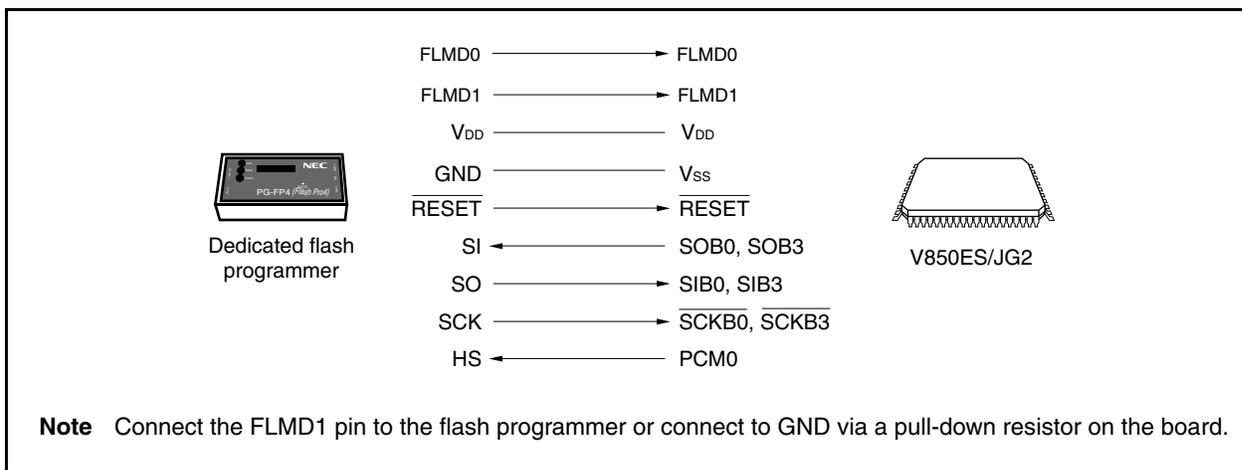
The dedicated flash programmer outputs the transfer clock, and the V850ES/JG2 operates as a slave.
