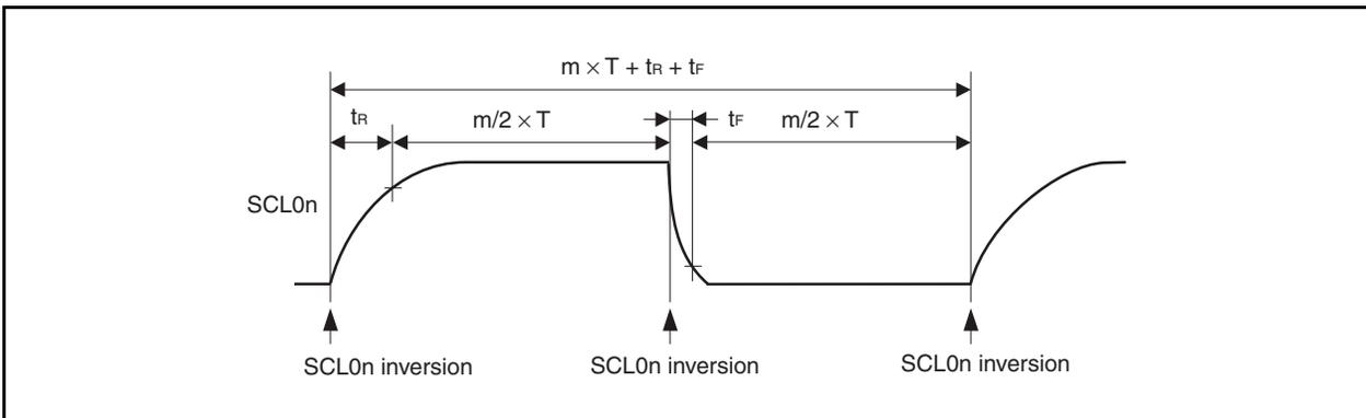
The clock to be selected can be set by the combination of the SMCn, CLn1, and CLn0 bits of the IICCLn register, the CLXn bit of the IICXn register, and the OCKSTHm, OCKSm1, and OCKSm0 bits of the OCKSm register (n = 0 to 2, m = 0, 1).
