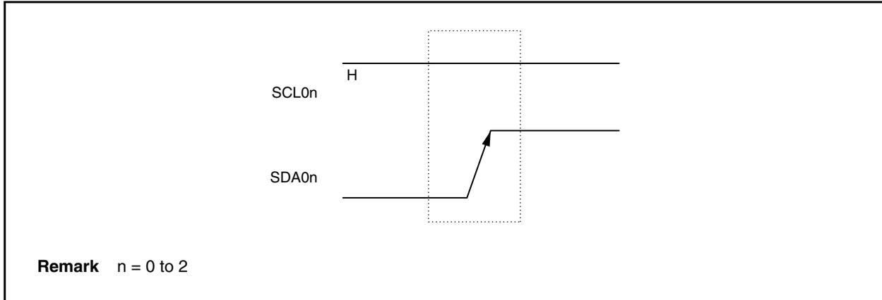
A stop condition is generated when the IICn.SPTn bit is set to 1. When the stop condition is detected, the IICn.SPn bit is set to 1 and the interrupt request signal (INTIICn) is generated when the IICn.SPIEn bit is set to 1 (n = 0 to 2).
