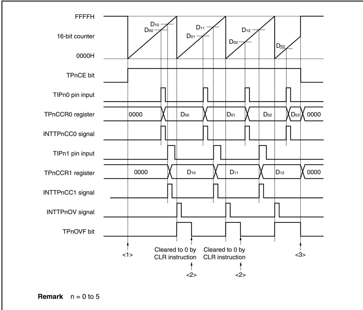
Figure 7-33. Software Processing Flow in Free-Running Timer Mode (Capture Function) (2/2)
