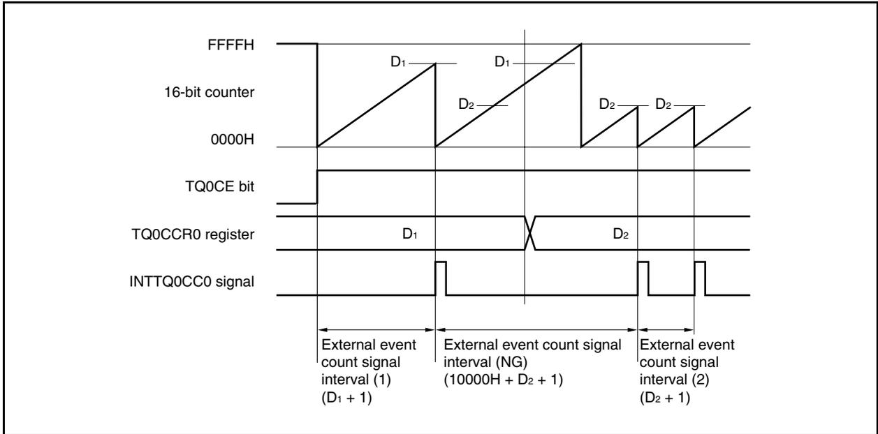
If the value of the TQ0CCR0 register is changed from D<sub>1</sub> to D<sub>2</sub> while the count value is greater than D<sub>2</sub> but less than D<sub>1</sub>, the count value is transferred to the CCR0 buffer register as soon as the TQ0CCR0 register has been rewritten. Consequently, the value that is compared with the 16-bit counter is D<sub>2</sub>.
