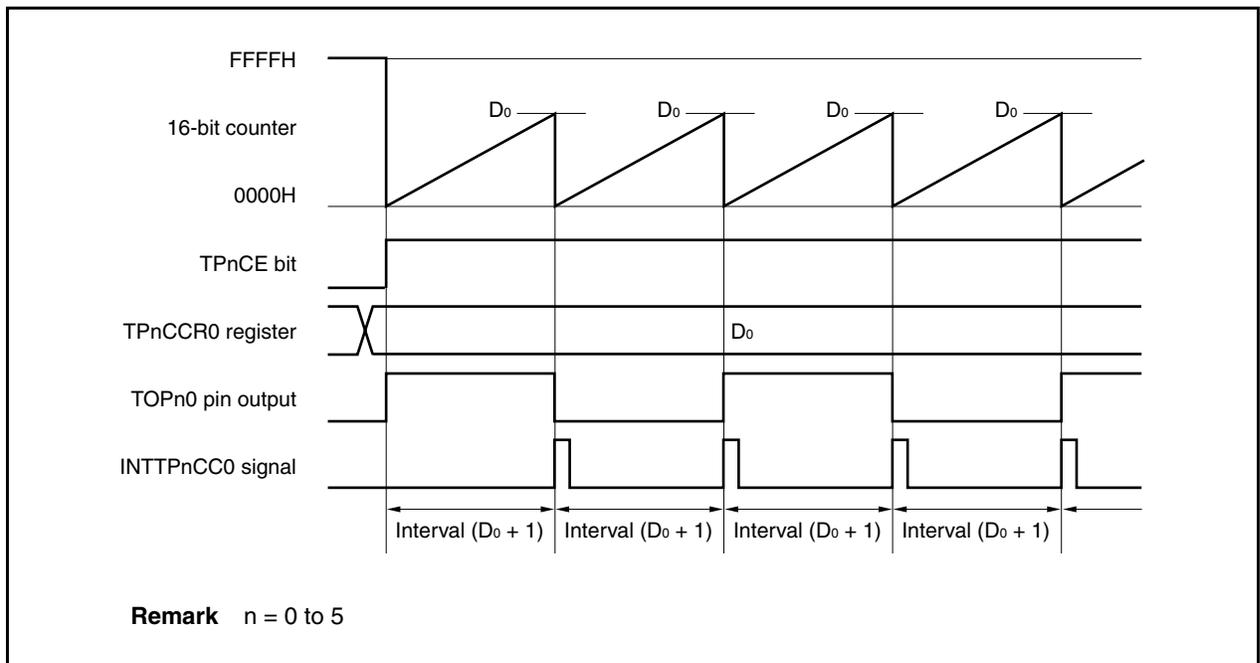
When the TPnCE bit is set to 1, the value of the 16-bit counter is cleared from FFFFH to 0000H in synchronization with the count clock, and the counter starts counting. At this time, the output of the TOPn0 pin is inverted. Additionally, the set value of the TPnCCR0 register is transferred to the CCR0 buffer register.
