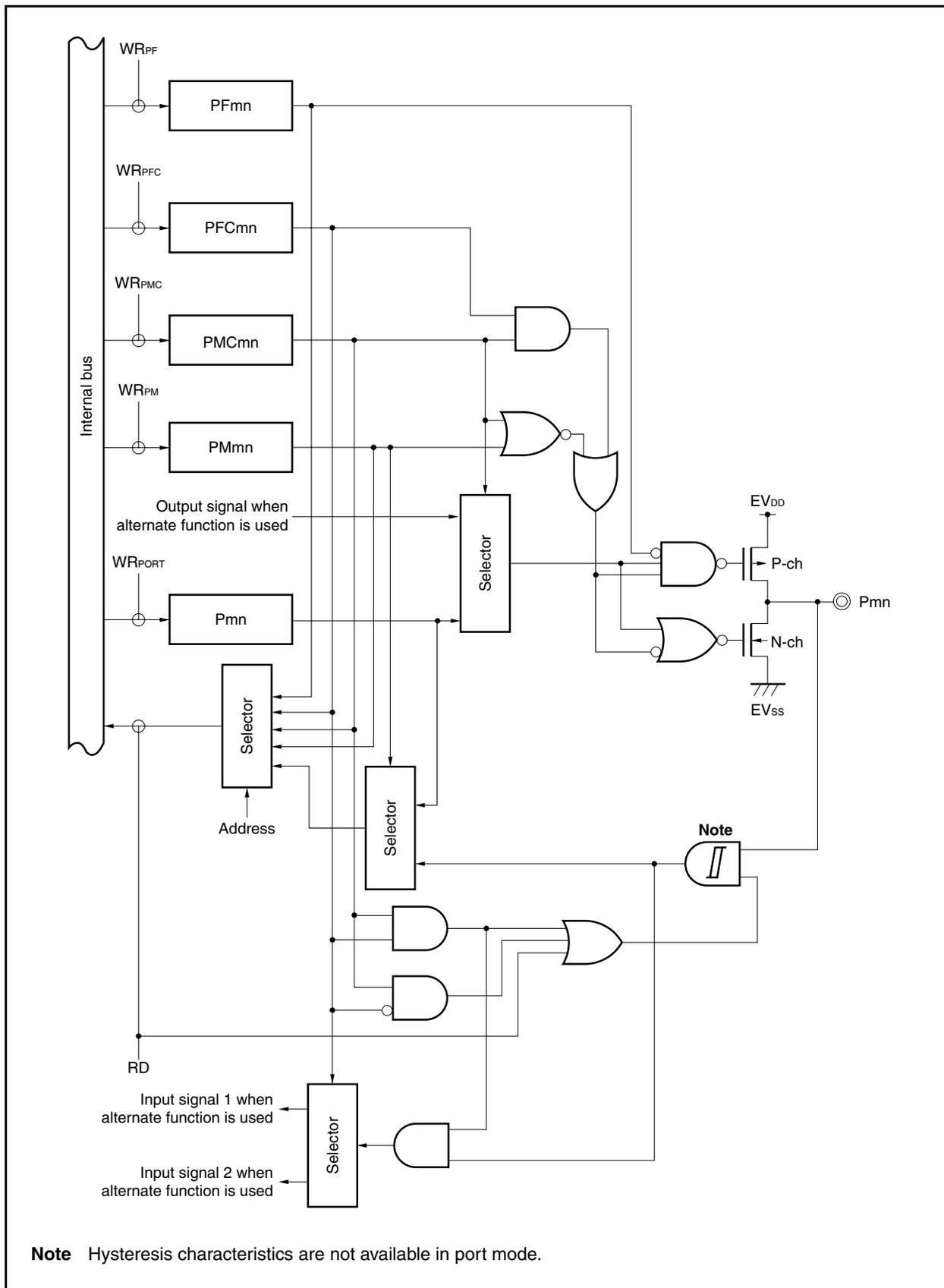
Figure 4-15. Block Diagram of Type G-12
