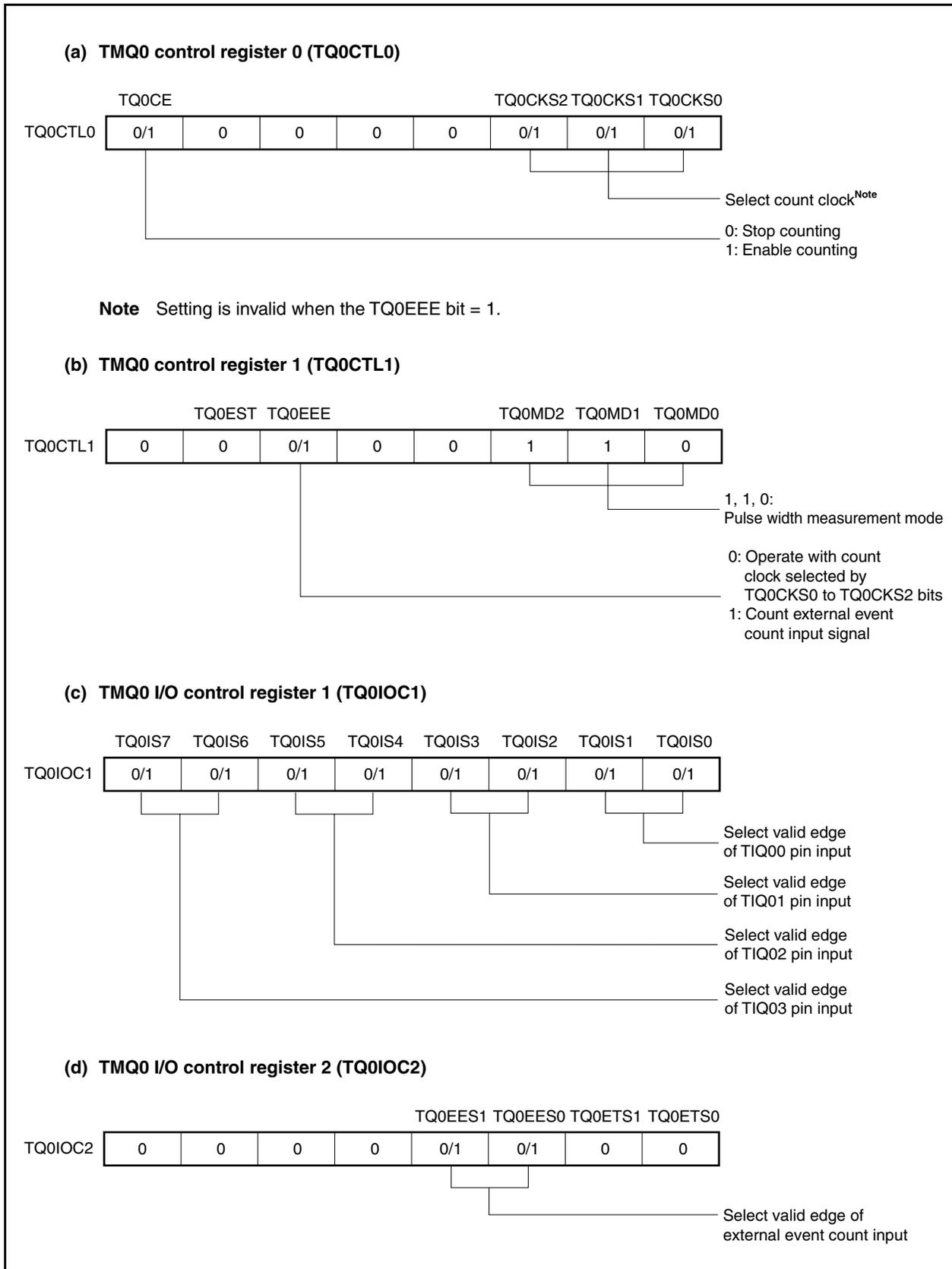
Figure 8-36. Register Setting in Pulse Width Measurement Mode (2/2)
