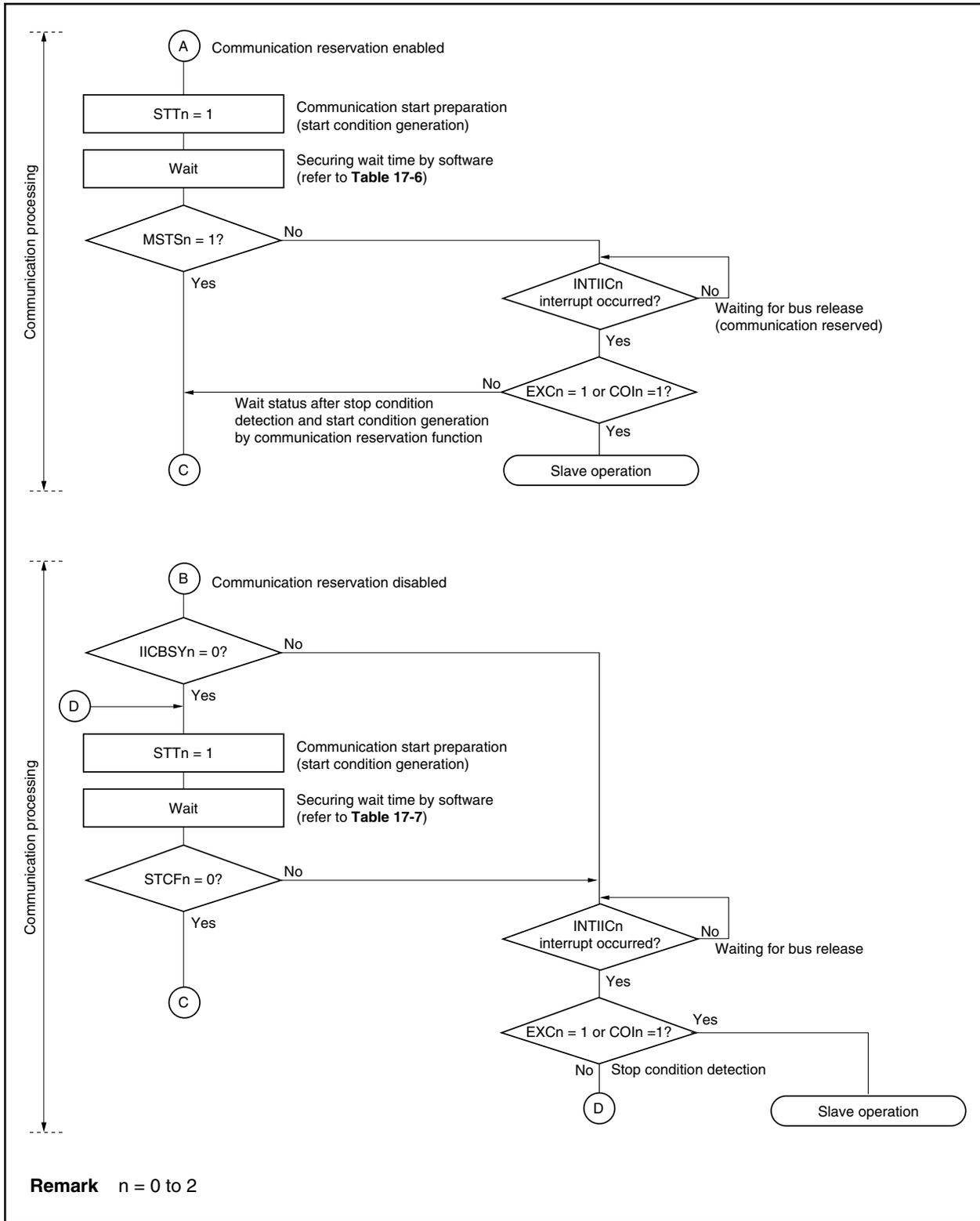
Figure 17-19. Master Operation in Multimaster System (3/3)
