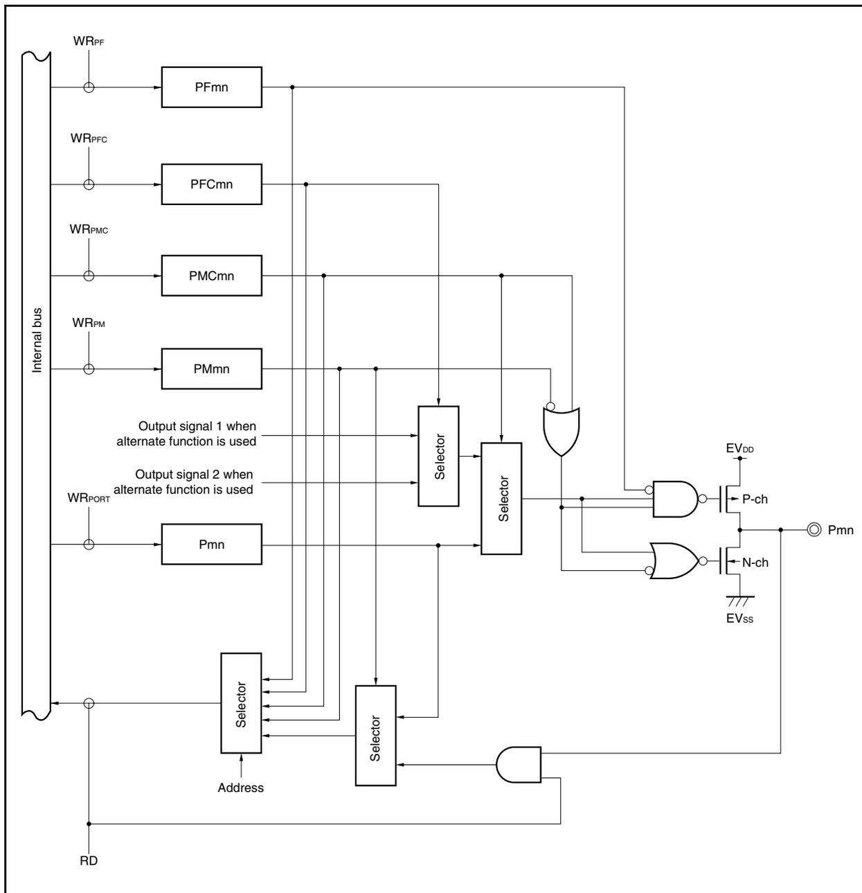
Figure 4-13. Block Diagram of Type G-5
