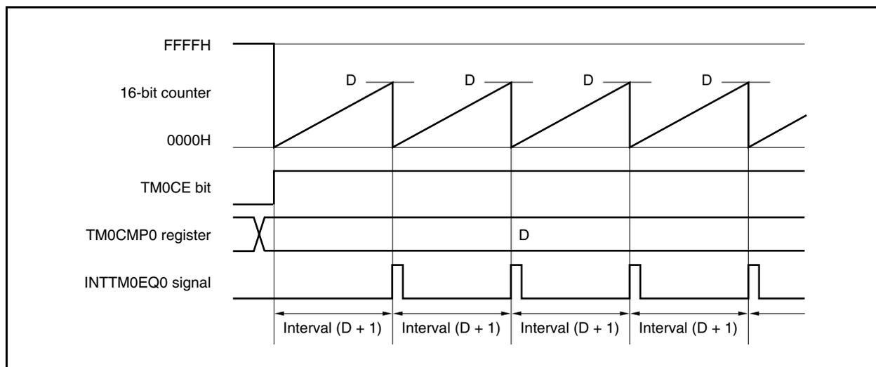
When the TM0CE bit is set to 1, the value of the 16-bit counter is cleared from FFFFH to 0000H in synchronization with the count clock, and the counter starts counting.
