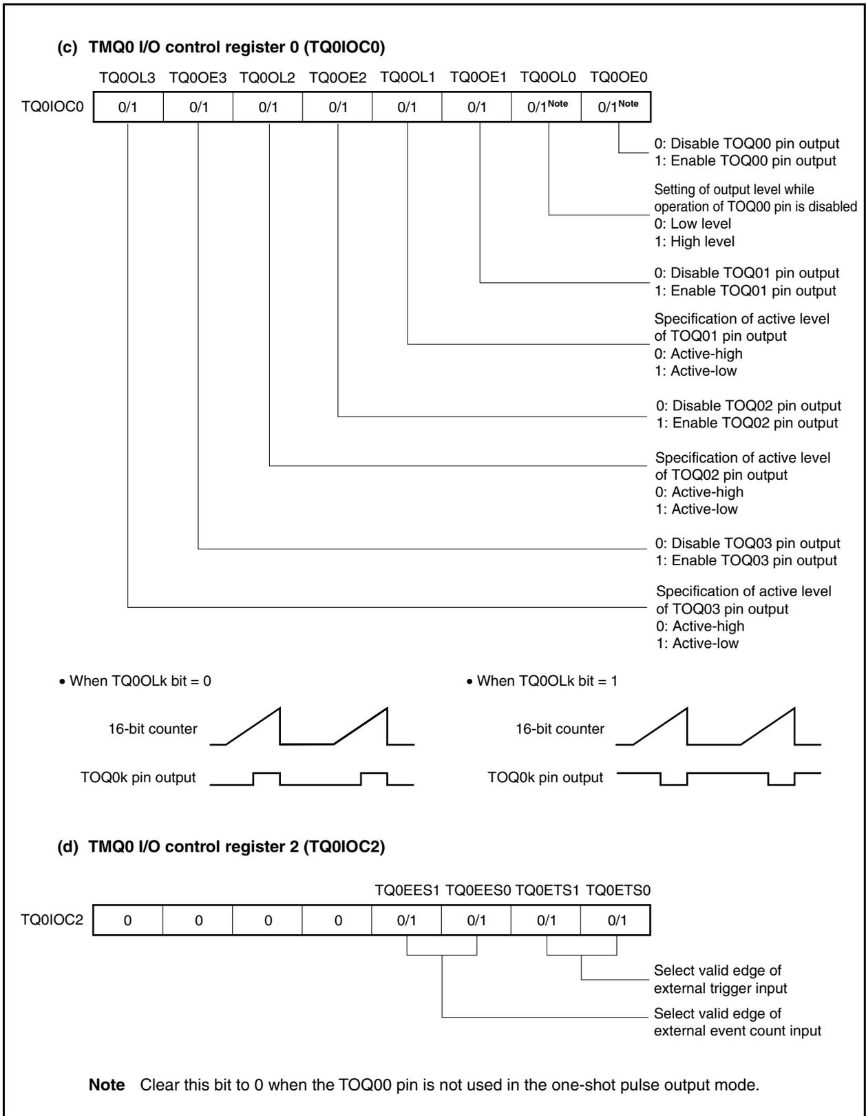
Figure 8-22. Register Setting in One-Shot Pulse Output Mode (3/3)
