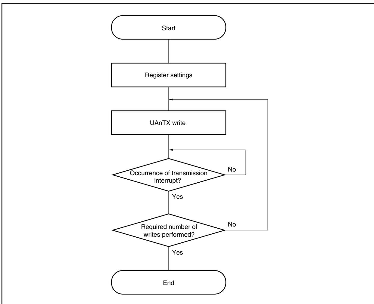
Figure 15-12. Continuous Transmission Operation Timing
