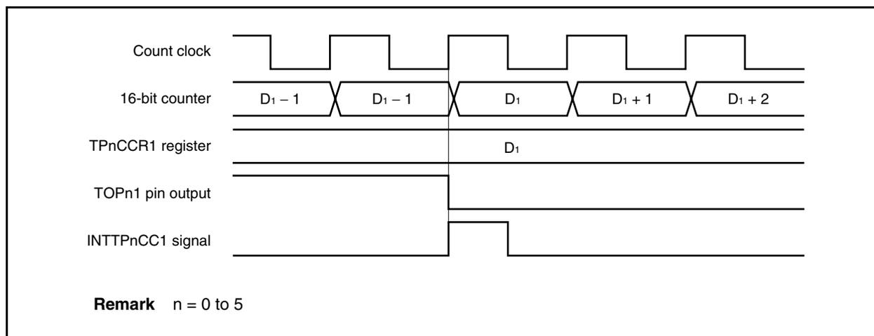
Usually, the INTTPnCC1 signal is generated in synchronization with the next count up, after the count value of the 16-bit counter matches the value of the TPnCCR1 register.
