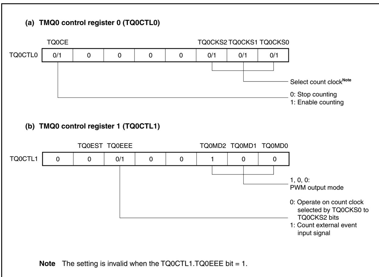
Figure 8-26. Setting of Registers in PWM Output Mode (2/3)
