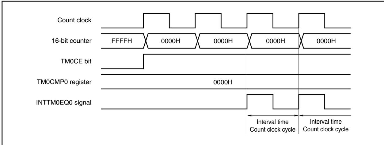
(b) Operation if TM0CMP0 register is set to N
