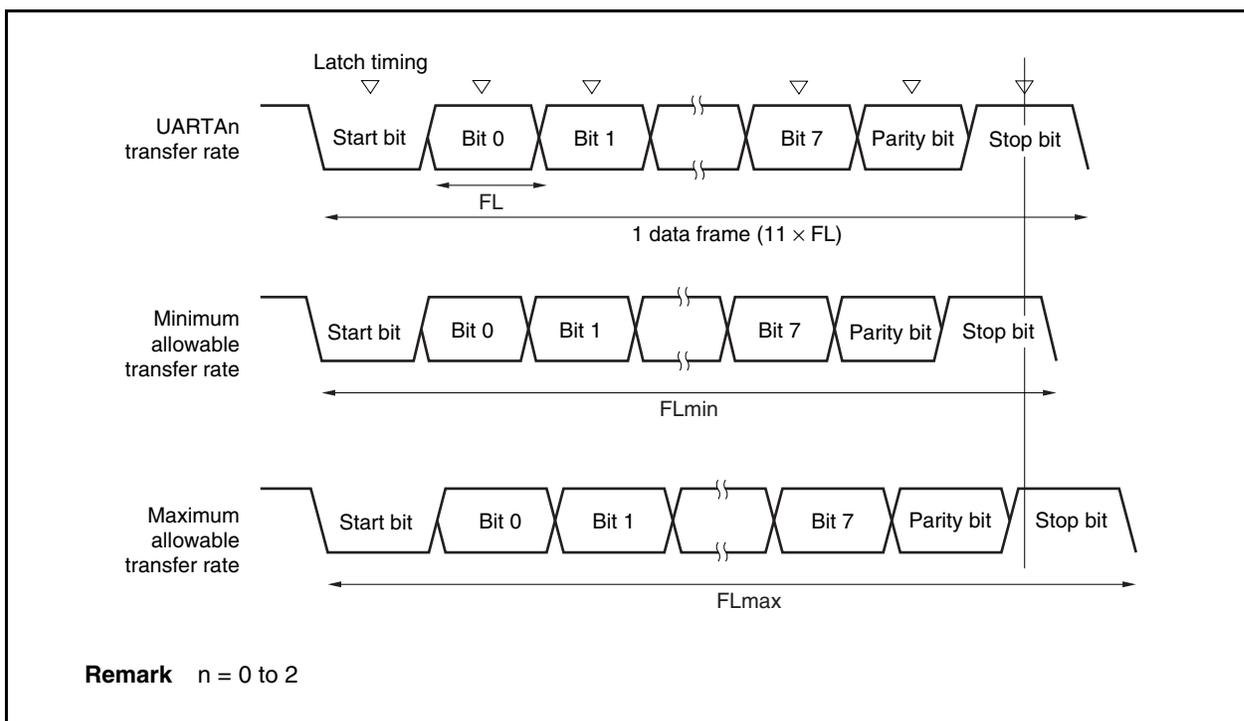
As shown in Figure 15-17, the receive data latch timing is determined by the counter set using the UAnCTL2 register following start bit detection. The transmit data can be normally received if up to the last data (stop bit) can be received in time for this latch timing.
