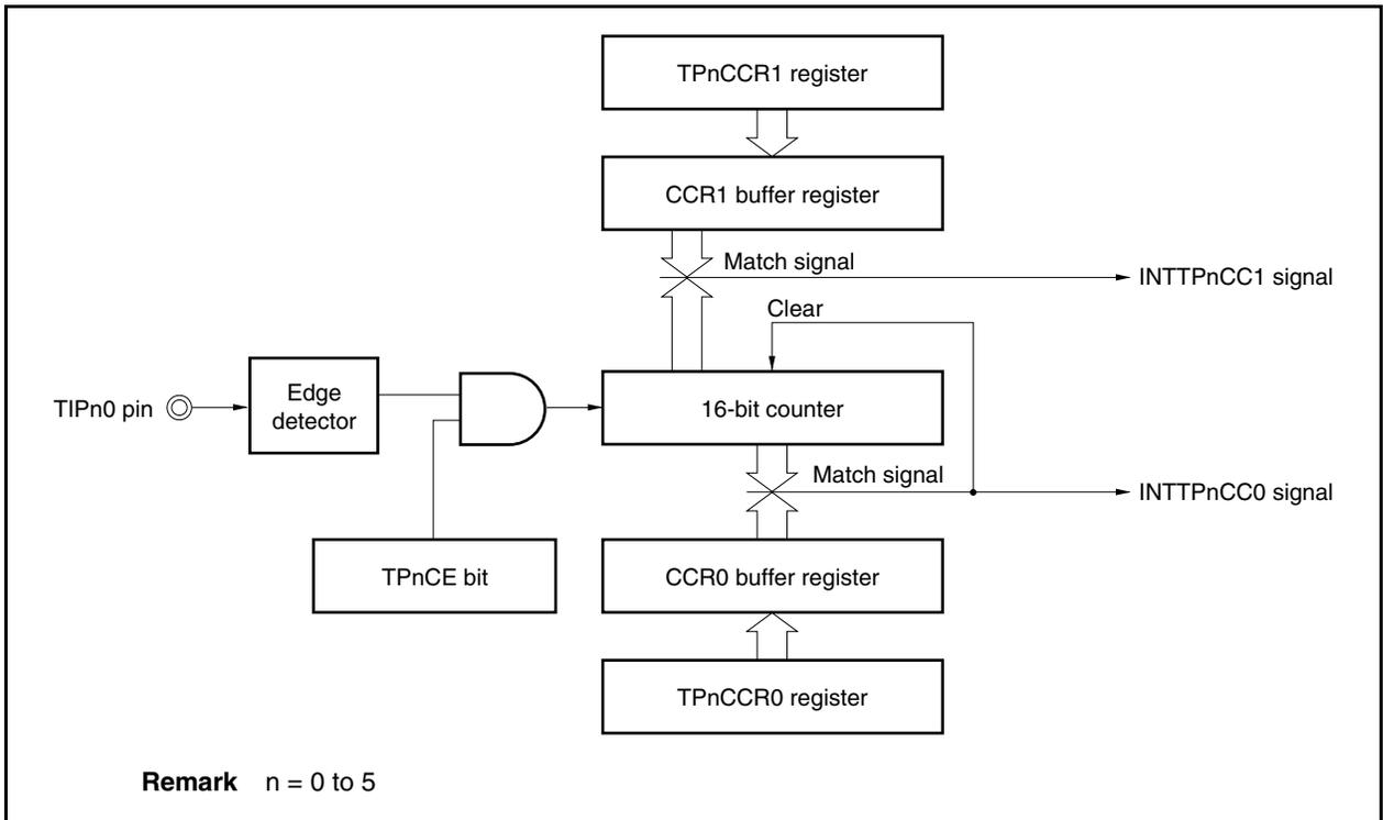
If the set value of the TPnCCR1 register is smaller than the set value of the TPnCCR0 register, the INTTPnCC1 signal is generated once per cycle.
