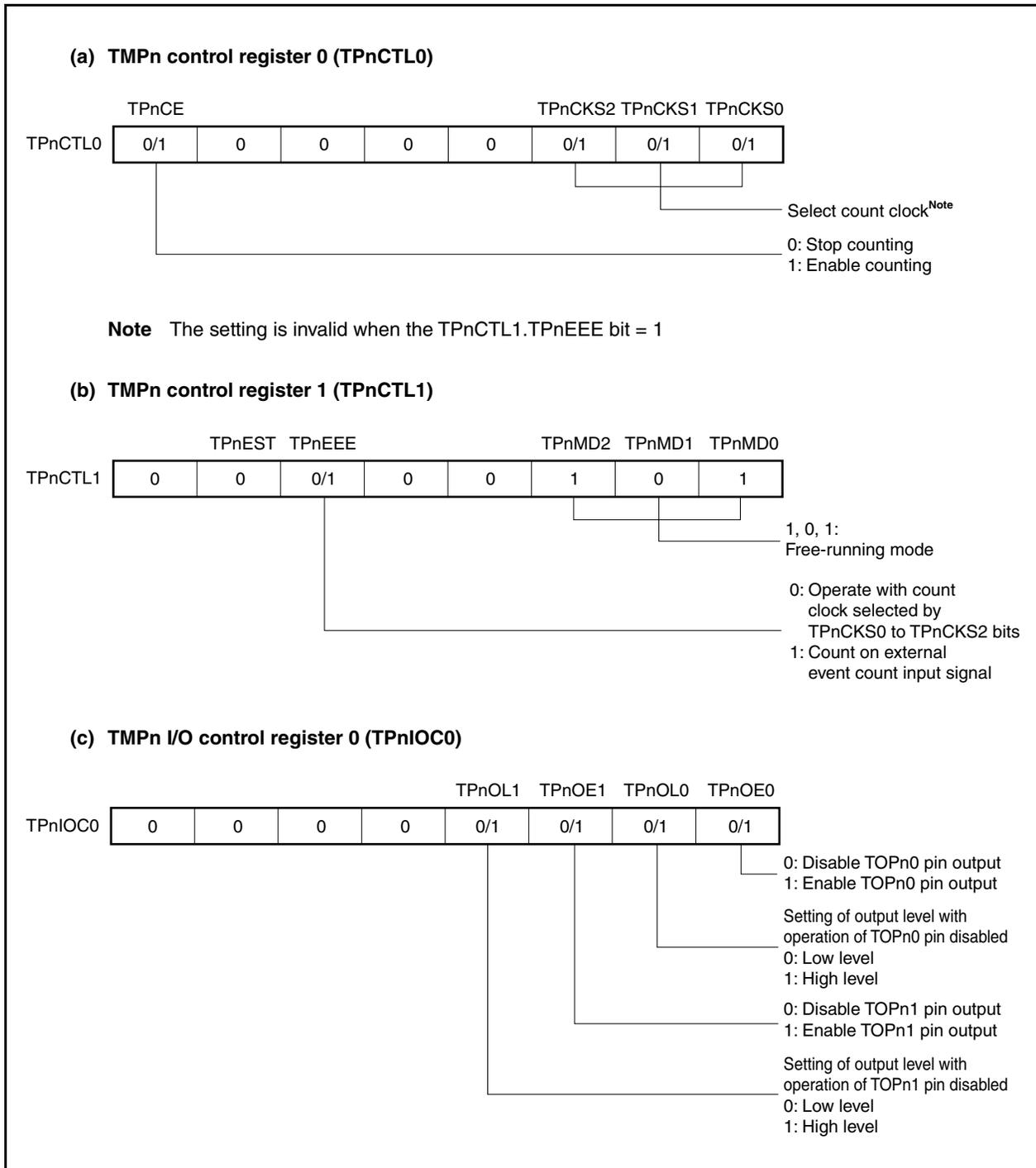
Figure 7-31. Register Setting in Free-Running Timer Mode (2/2)
