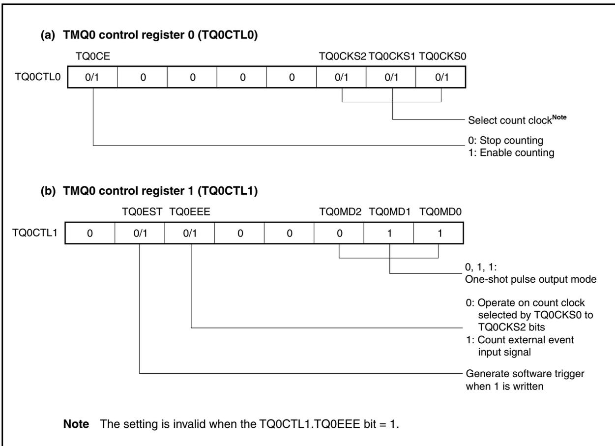
Figure 8-22. Register Setting in One-Shot Pulse Output Mode (2/3)
