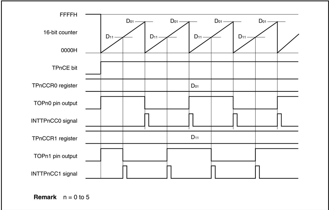
If the set value of the TPnCCR1 register is greater than the set value of the TPnCCR0 register, the count value of the 16-bit counter does not match the value of the TPnCCR1 register. Consequently, the INTTPnCC1 signal is not generated, nor is the output of the TOPn1 pin changed.
