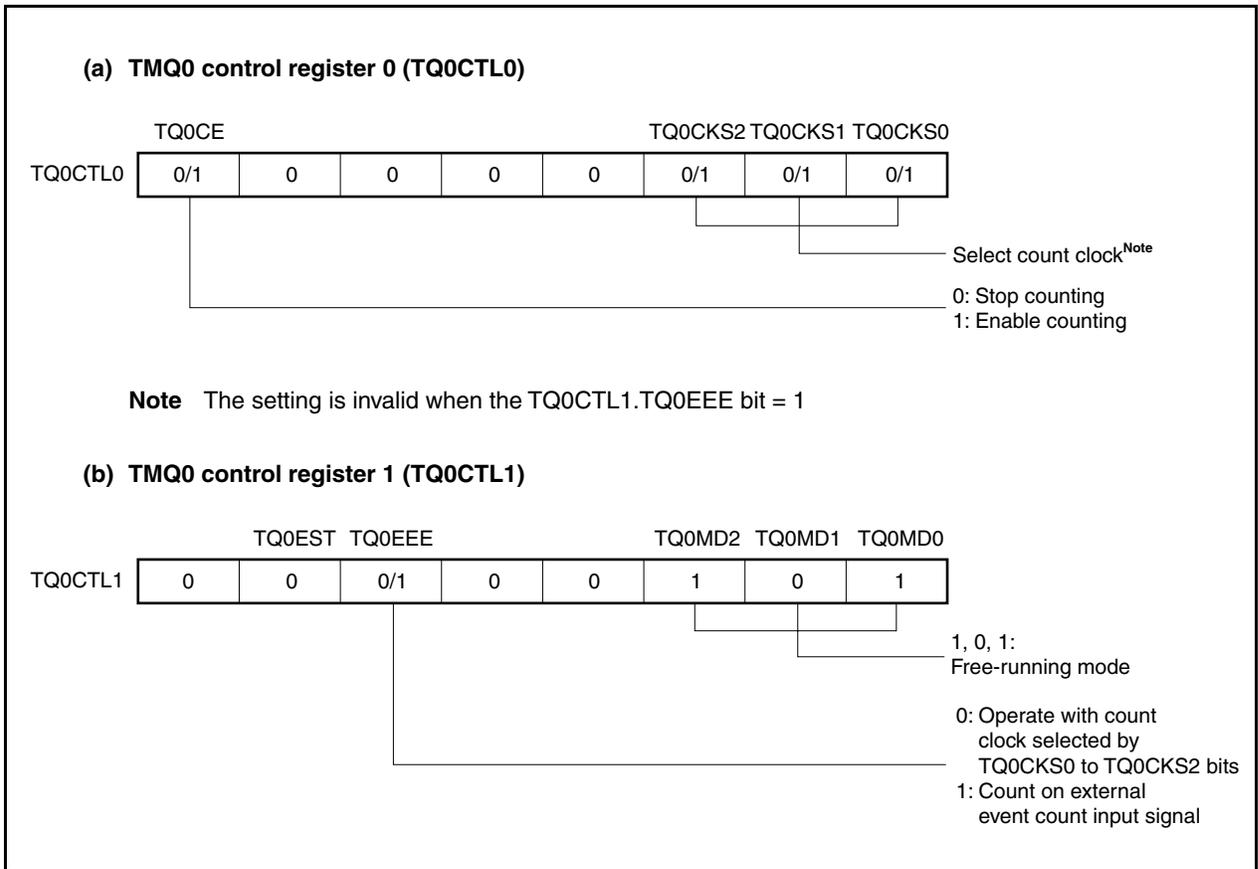
Figure 8-31. Register Setting in Free-Running Timer Mode (2/3)
