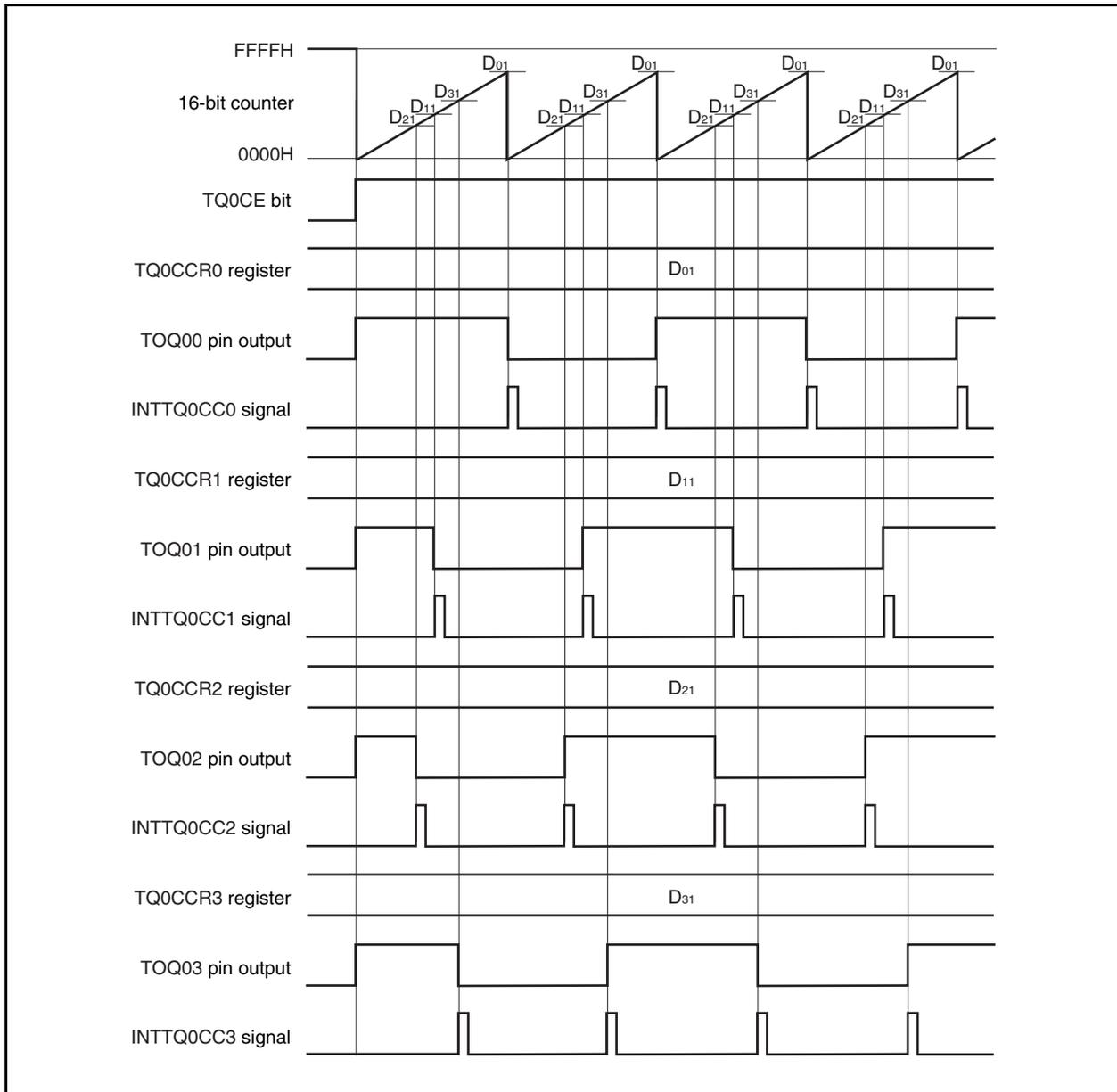
If the set value of the TQ0CCRk register is greater than the set value of the TQ0CCR0 register, the count value of the 16-bit counter does not match the value of the TQ0CCRk register. Consequently, the INTTQ0CCk signal is not generated, nor is the output of the TOQ0k pin changed.
