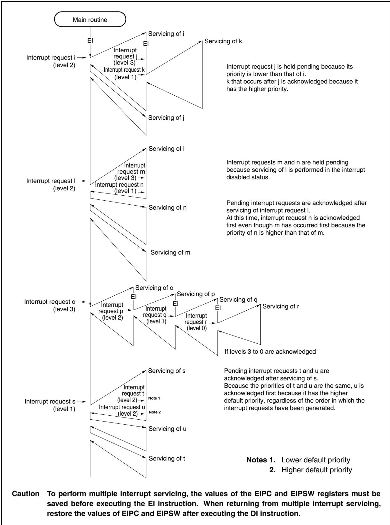
Figure 19-8. Example of Servicing Interrupt Request Signals Simultaneously Generated
