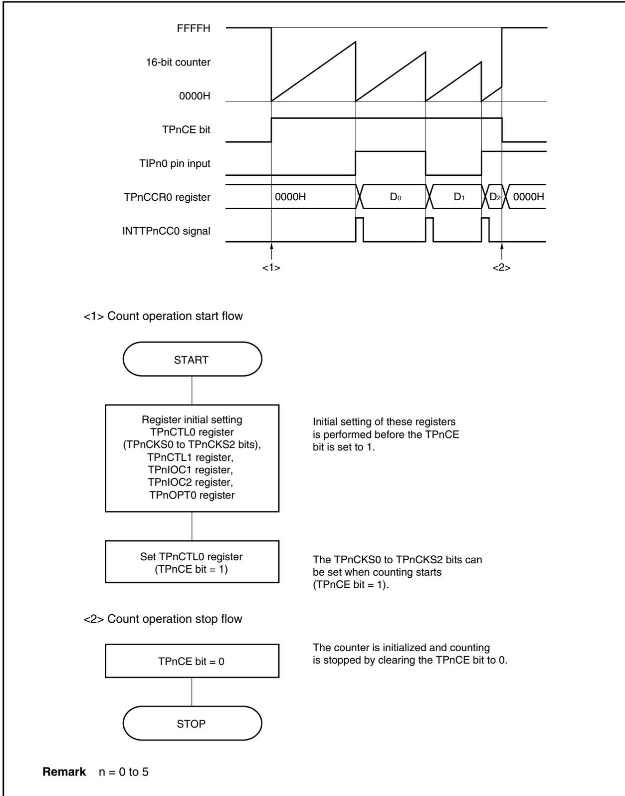
(2) Operation timing in pulse width measurement mode
