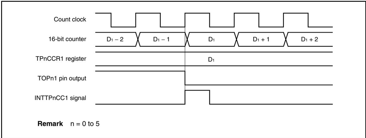
Usually, the INTTPnCC1 signal is generated when the 16-bit counter counts up next time after its count value matches the value of the TPnCCR1 register.
