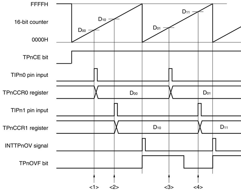
The following problem may occur when two pulse widths are measured in the free-running timer mode.
