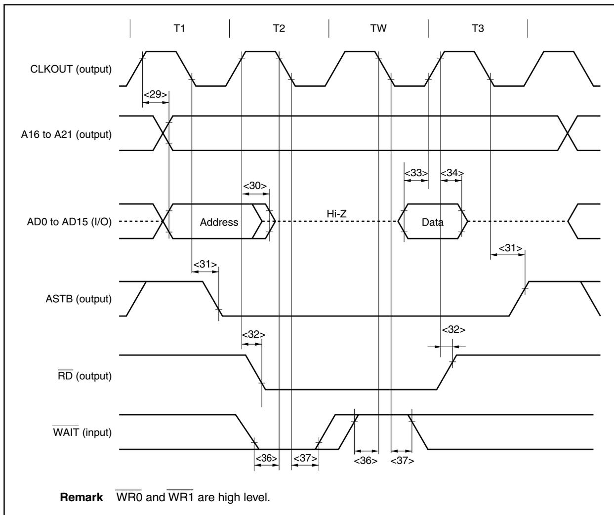
**Write Cycle (CLKOUT Synchronous): In Multiplexed Bus Mode**
