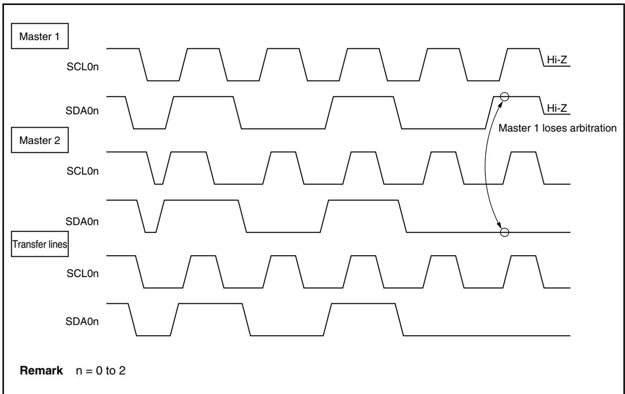
**Table 17-5. Status During Arbitration and Interrupt Request Signal Generation Timing**
