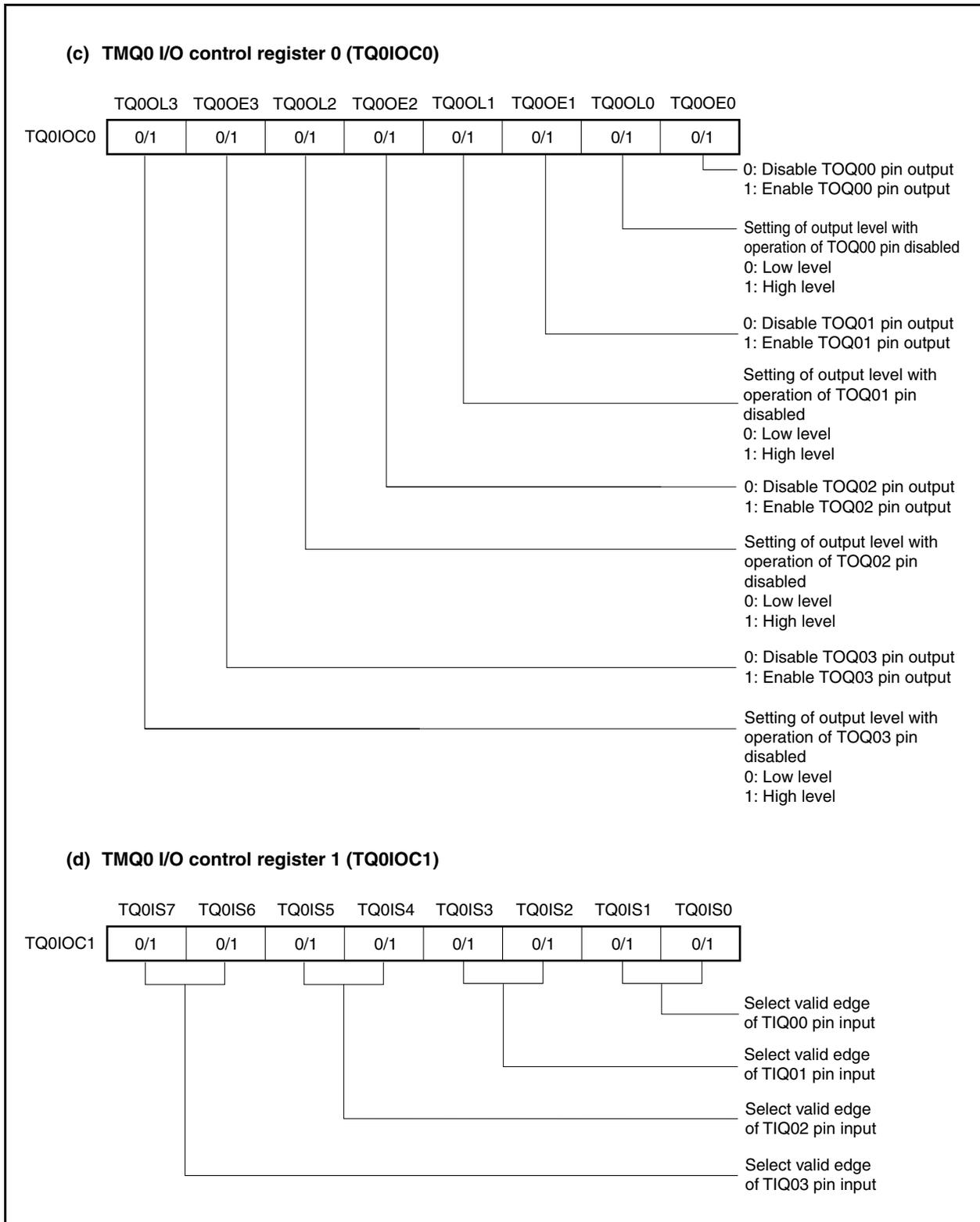
Figure 8-31. Register Setting in Free-Running Timer Mode (3/3)
