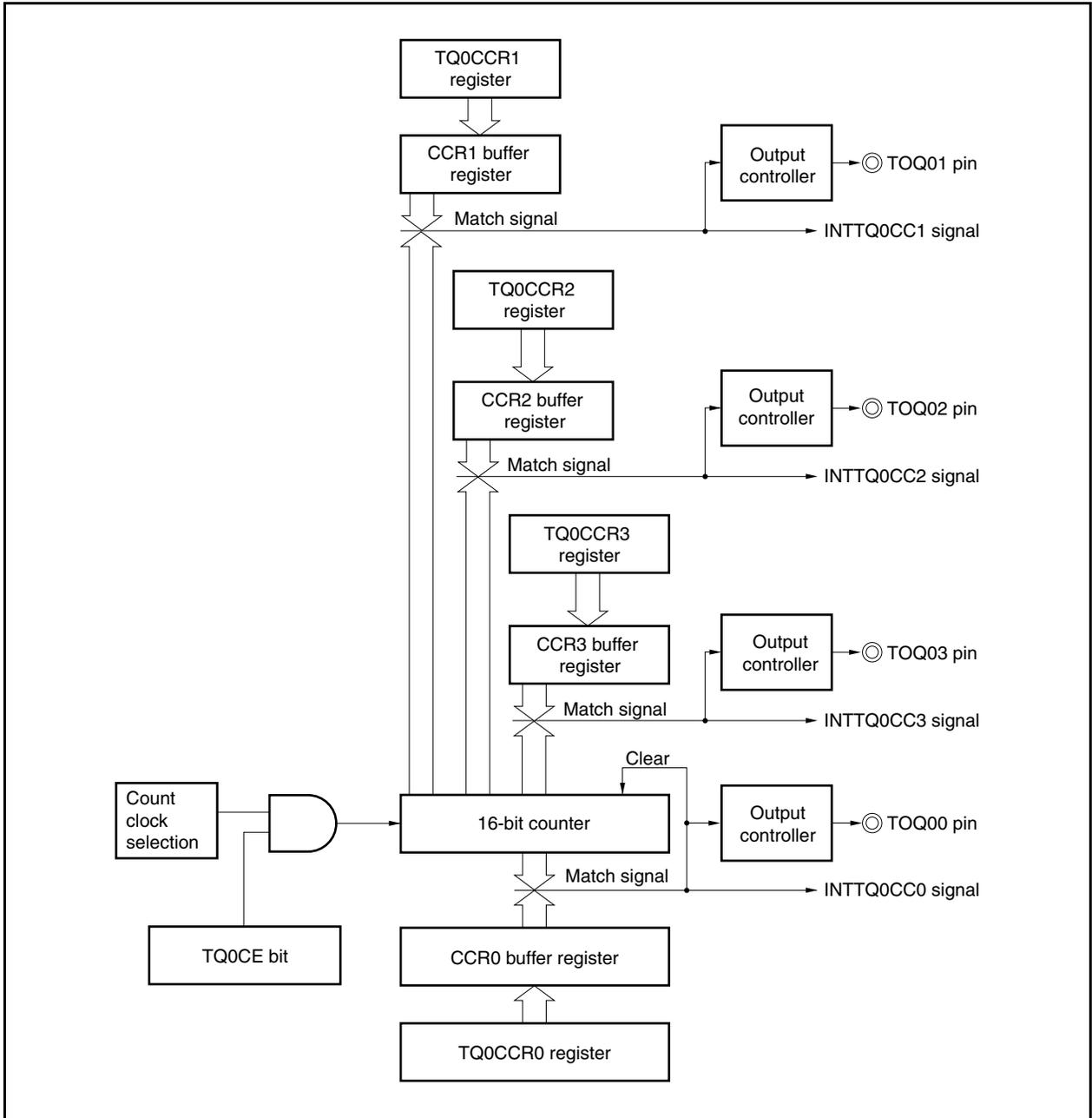
If the set value of the TQ0CCRk register is less than the set value of the TQ0CCR0 register, the INTTQ0CCk signal is generated once per cycle. At the same time, the output of the TOPQ0k pin is inverted.
