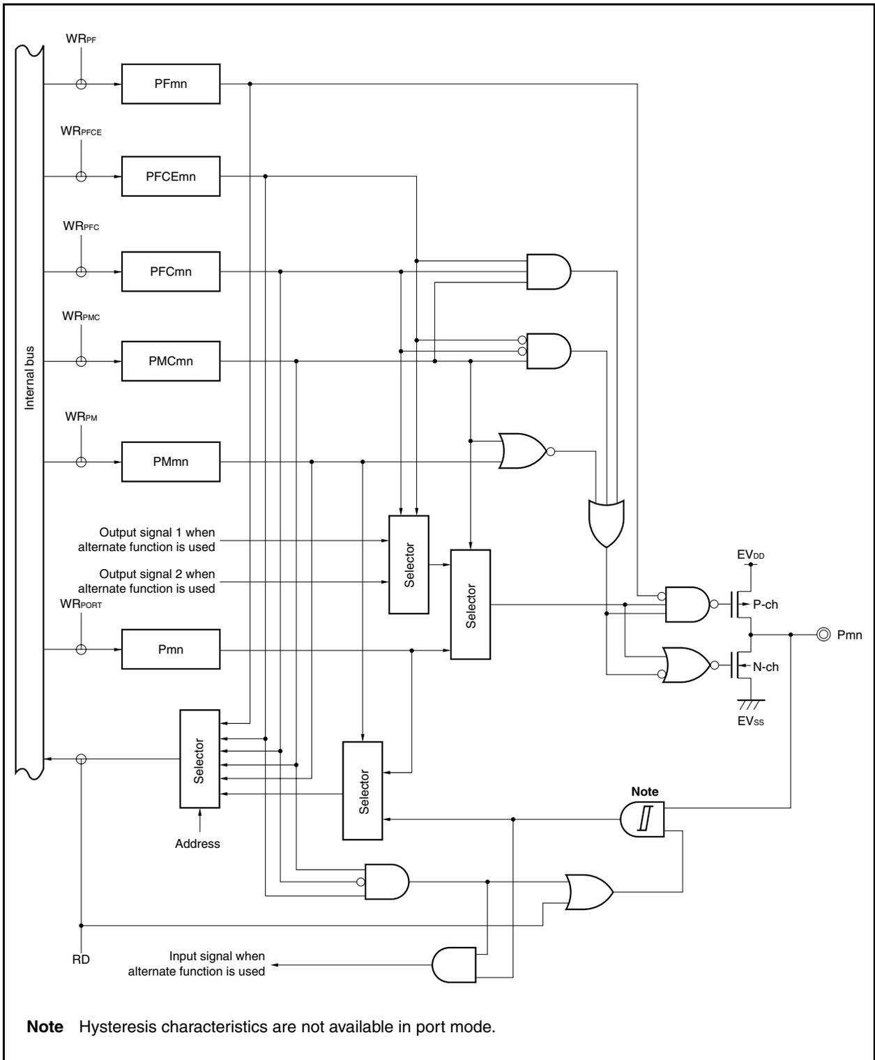
Figure 4-30. Block Diagram of Type U-14
