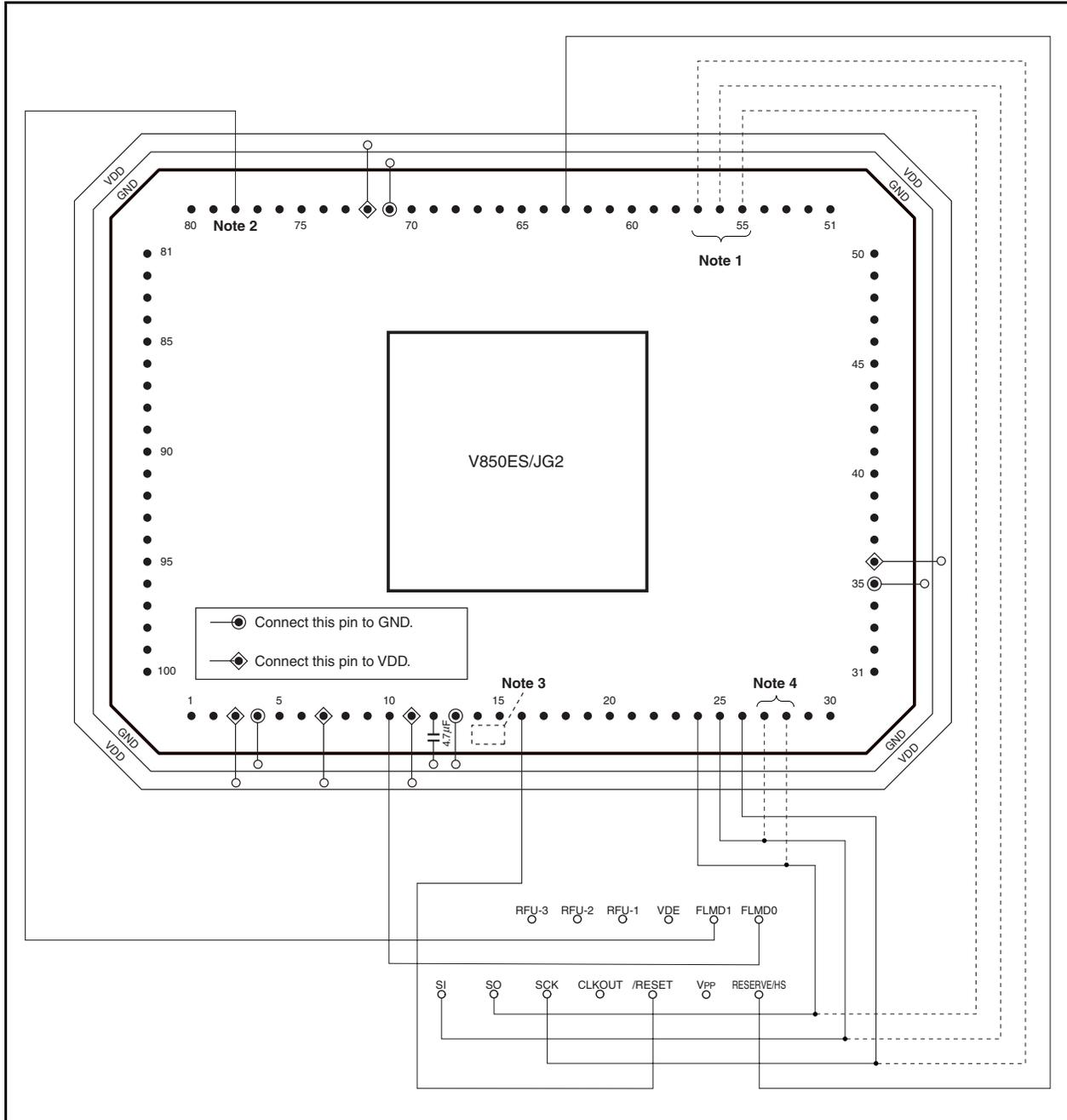
**Figure 26-6. Wiring Example of V850ES/JG2 Flash Writing Adapter (FA-100GF-3BA-A)
