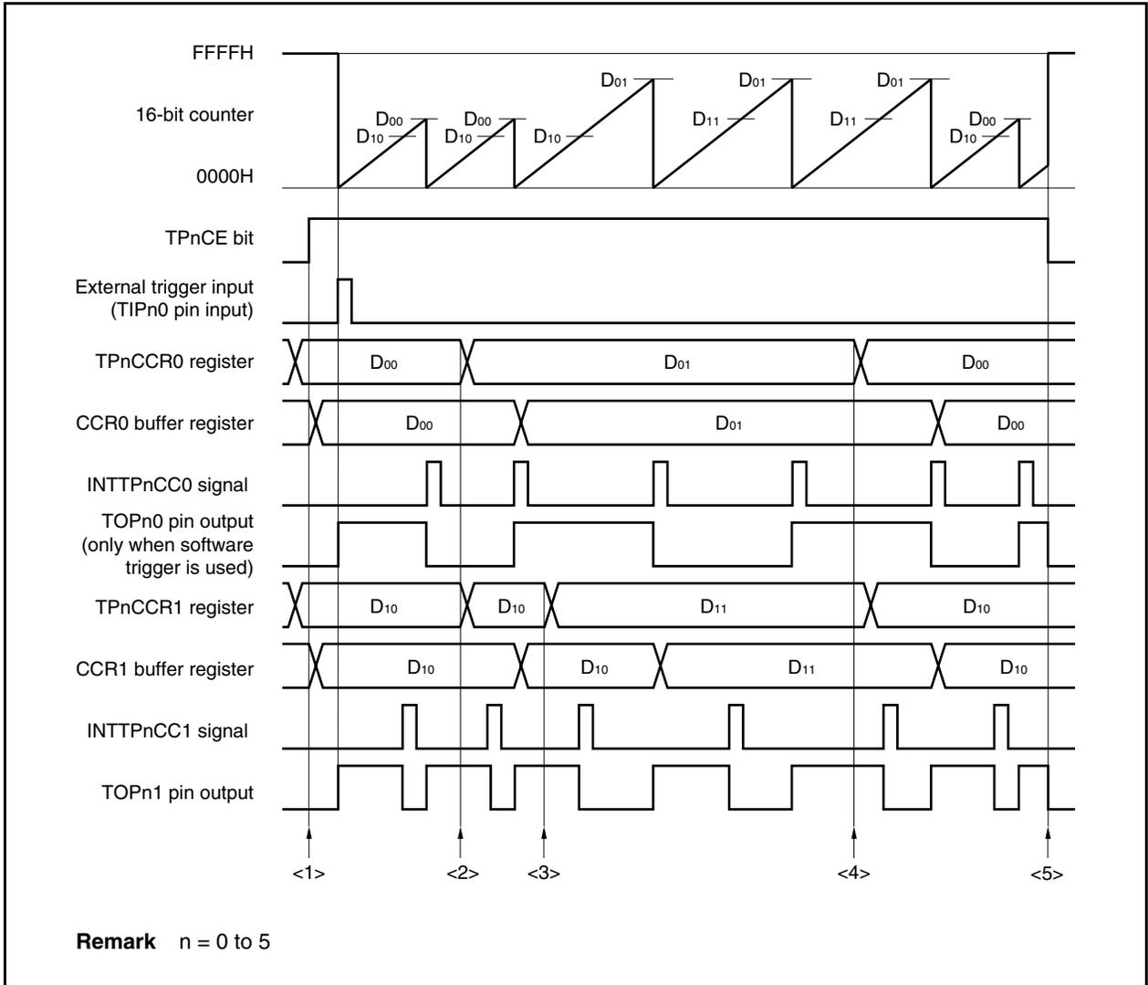
Figure 7-19. Software Processing Flow in External Trigger Pulse Output Mode (2/2)
