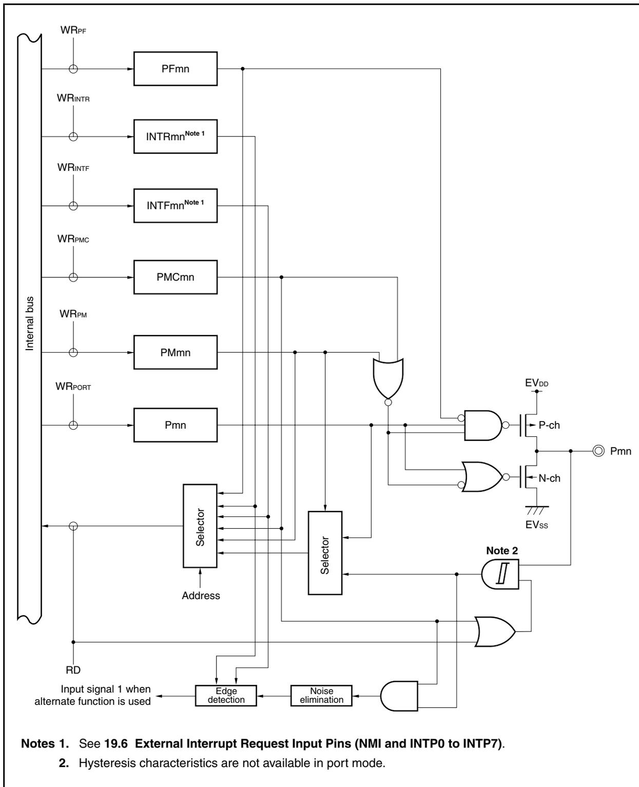
Figure 4-17. Block Diagram of Type N-1
