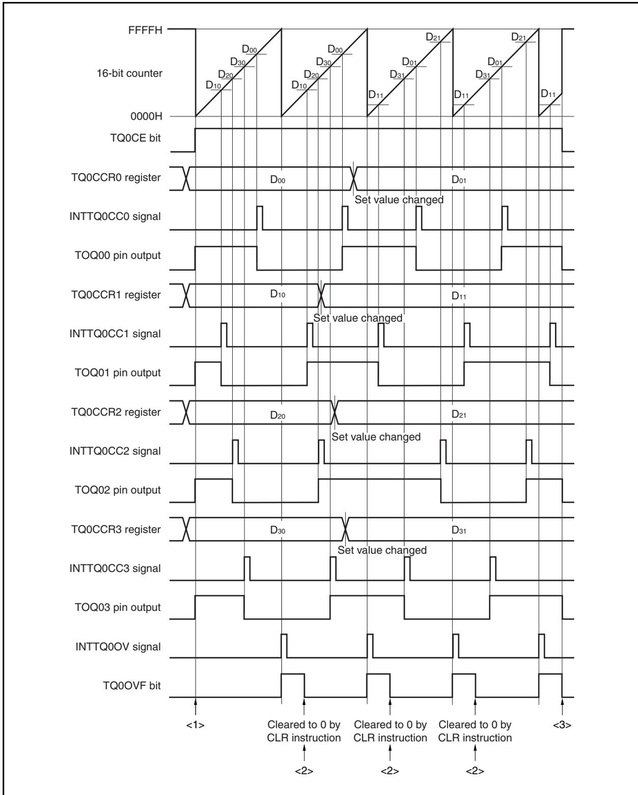
Figure 8-32. Software Processing Flow in Free-Running Timer Mode (Compare Function) (2/2)
