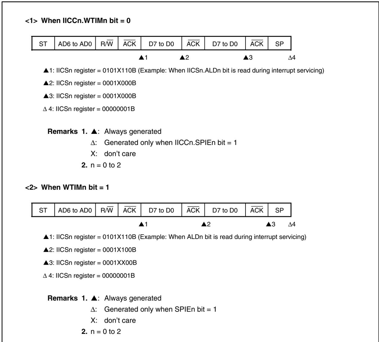
(2) When arbitration loss occurs during transmission of extension code
