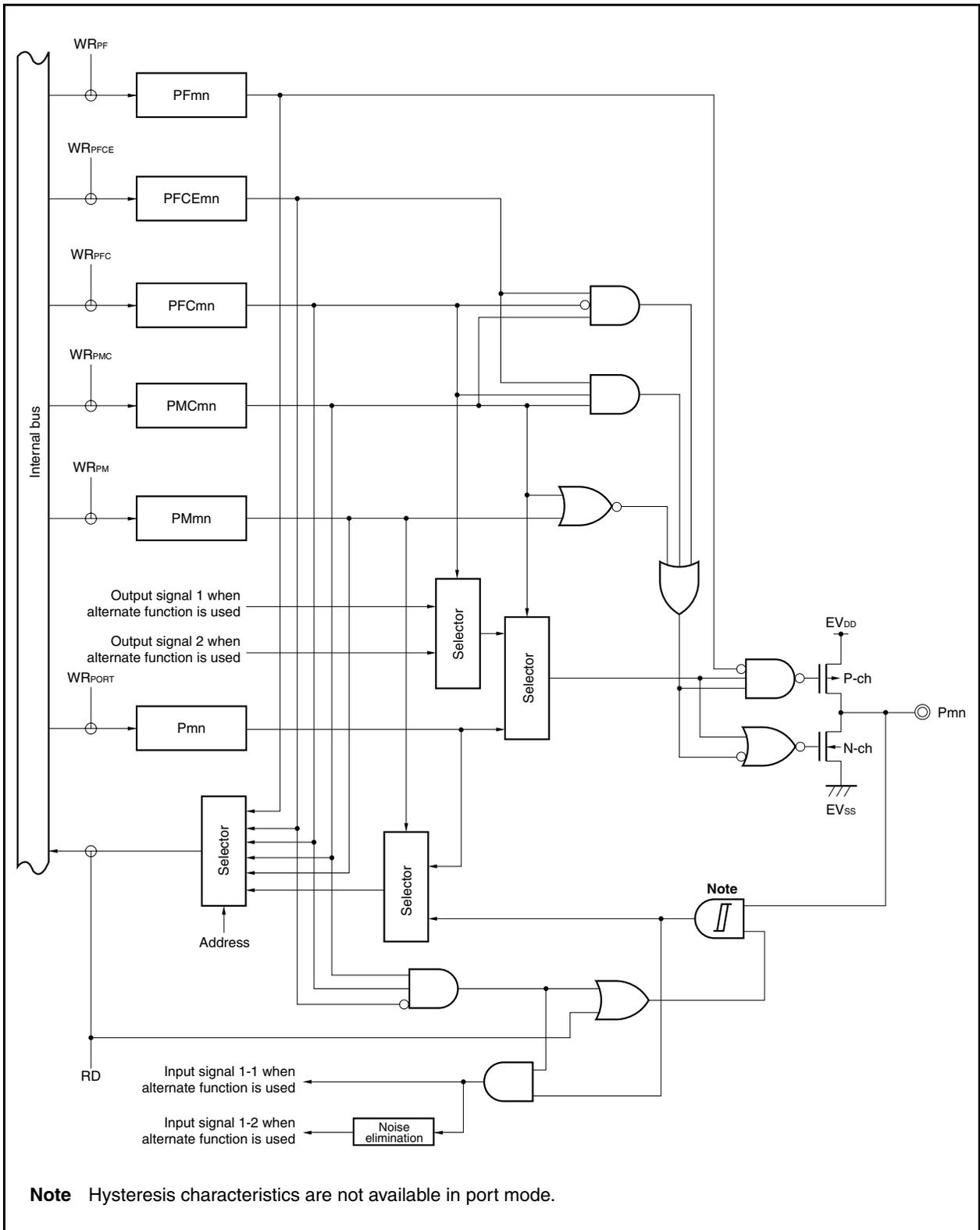
Figure 4-22. Block Diagram of Type U-6
