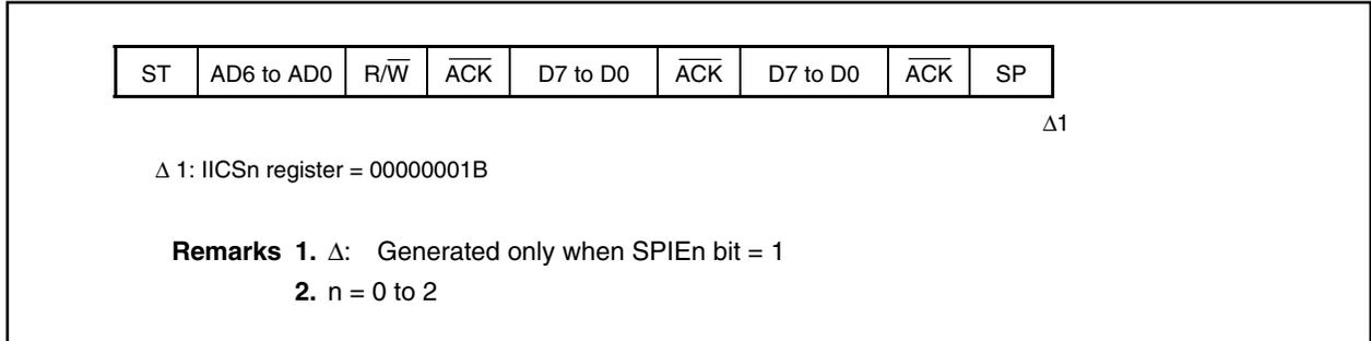
17.7.5 Arbitration loss operation (operation as slave after arbitration loss)
