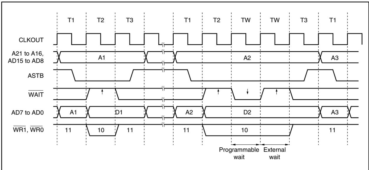
Figure 5-8. Multiplexed Bus Hold Timing (Bus Size: 16 Bits, 16-Bit Access)
