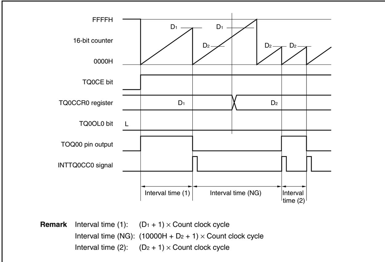
If the value of the TQ0CCR0 register is changed from  $D_1$  to  $D_2$  while the count value is greater than  $D_2$  but less than  $D_1$ , the count value is transferred to the CCR0 buffer register as soon as the TQ0CCR0 register has been rewritten. Consequently, the value of the 16-bit counter that is compared is  $D_2$ .
