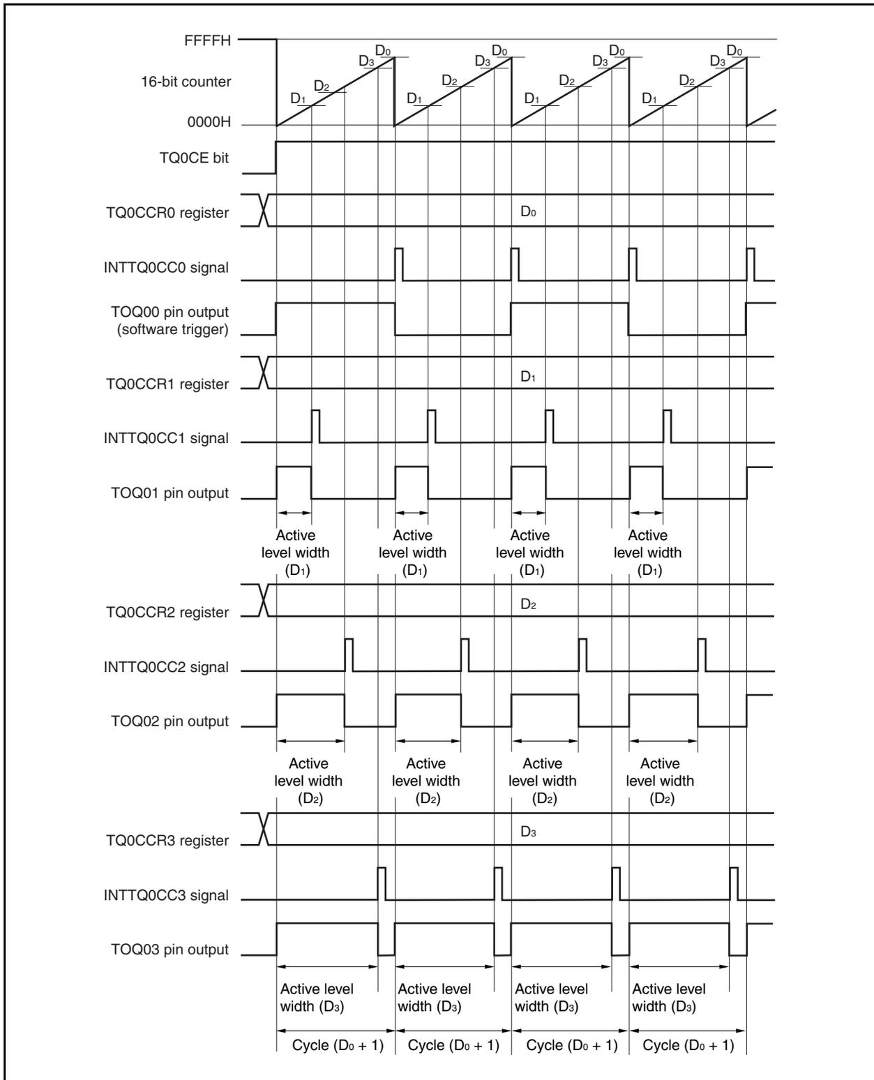
When the TQ0CE bit is set to 1, the 16-bit counter is cleared from FFFFH to 0000H, starts counting, and outputs PWM waveform from the TOQ0k pin.
