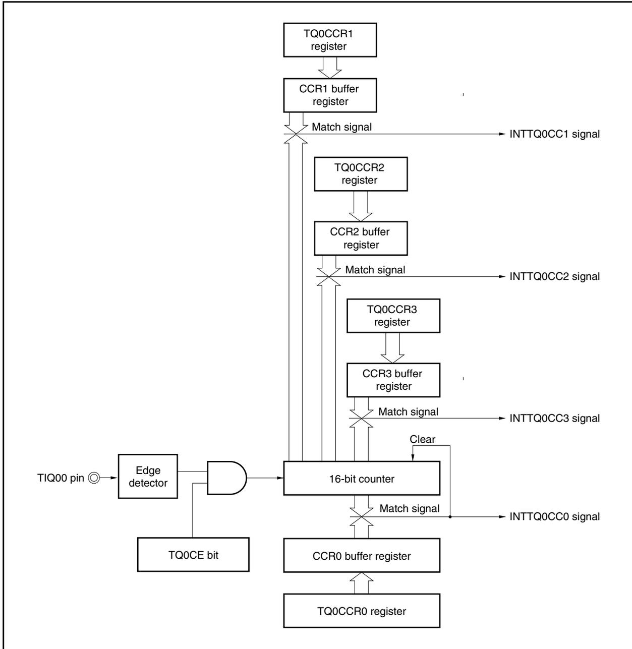
If the set value of the TQ0CCRk register is smaller than the set value of the TQ0CCR0 register, the INTTQ0CCk signal is generated once per cycle.
