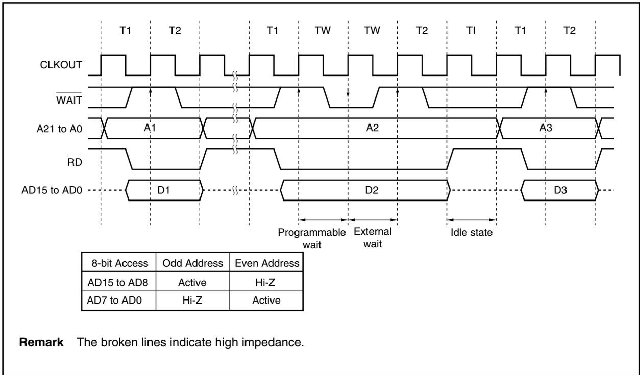
Figure 5-10. Separate Bus Read Timing (Bus Size: 8 Bits)
