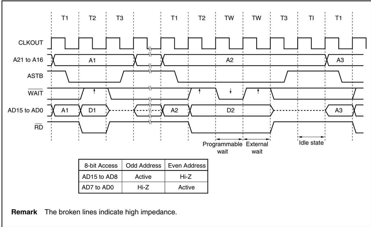
Figure 5-5. Multiplexed Bus Read Timing (Bus Size: 8 Bits)
