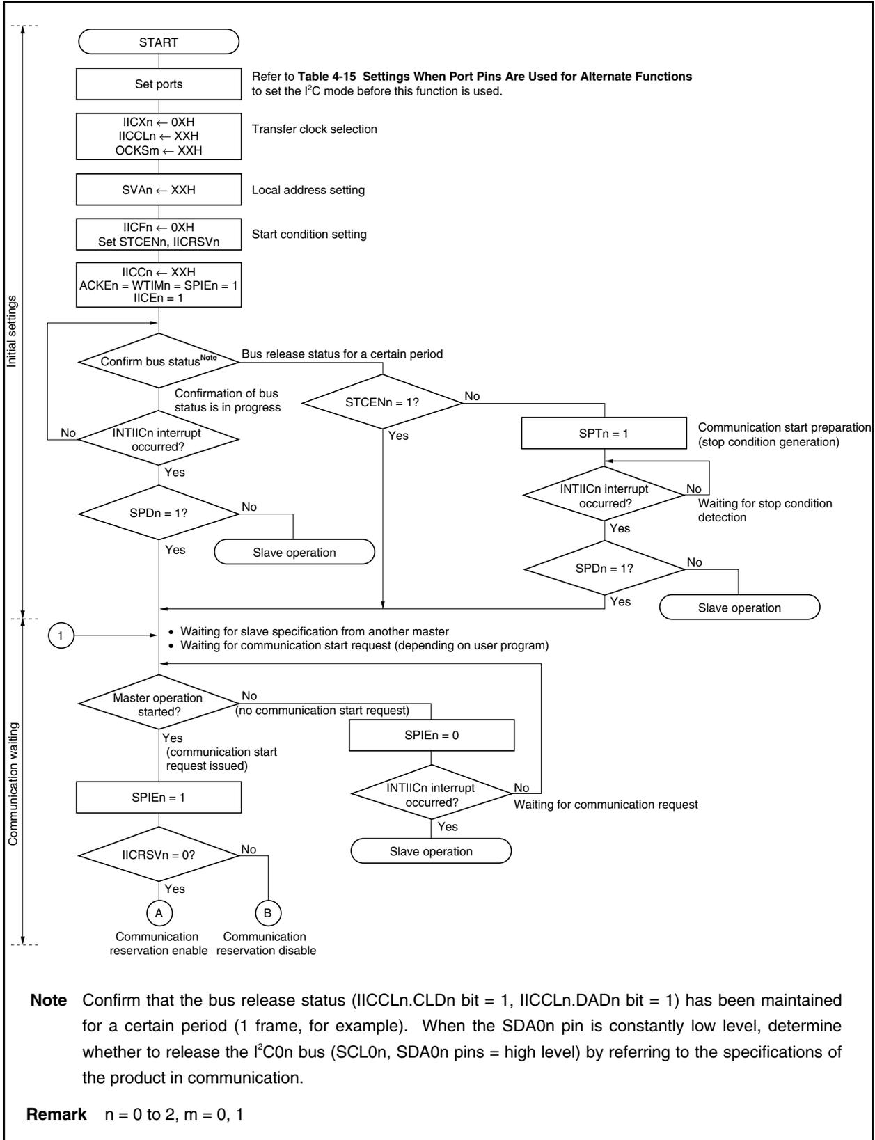
Figure 17-19. Master Operation in Multimaster System (2/3)
