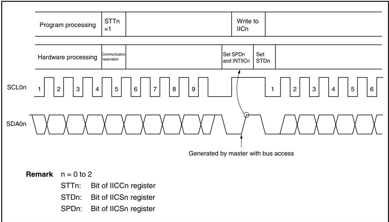
Communication reservations are accepted via the following timing. After the IICSn.STDn bit is set to 1, a communication reservation can be made by setting the IICCn.STTn bit to 1 before a stop condition is detected (n = 0 to 2).
