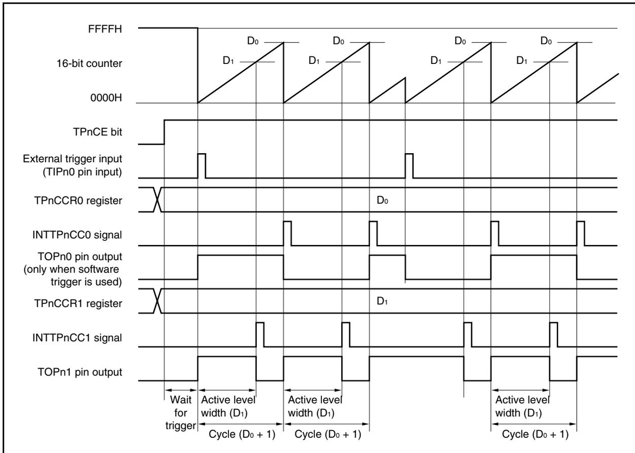
16-bit timer/event counter P waits for a trigger when the TPnCE bit is set to 1. When the trigger is generated, the 16-bit counter is cleared from FFFFH to 0000H, starts counting at the same time, and outputs a PWM waveform from the TOPn1 pin. If the trigger is generated again while the counter is operating, the counter is cleared to 0000H and restarted. (The output of the TOPn0 pin is inverted. The TOPn1 pin outputs a high-level regardless of the status (high/low) when a trigger occurs.)
