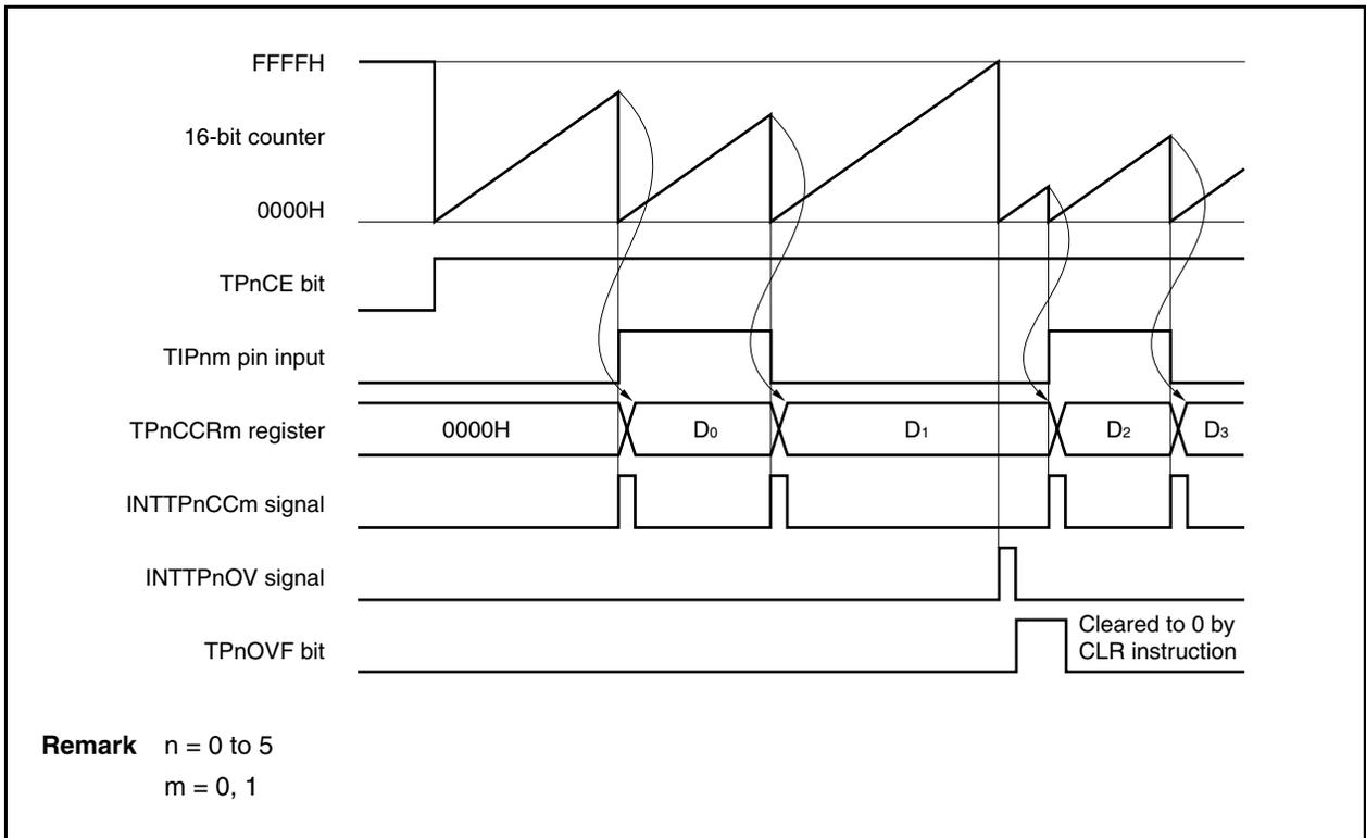
When the TPnCE bit is set to 1, the 16-bit counter starts counting. When the valid edge input to the TIPnm pin is later detected, the count value of the 16-bit counter is stored in the TPnCCRm register, the 16-bit counter is cleared to 0000H, and a capture interrupt request signal (INTTPnCCm) is generated.
