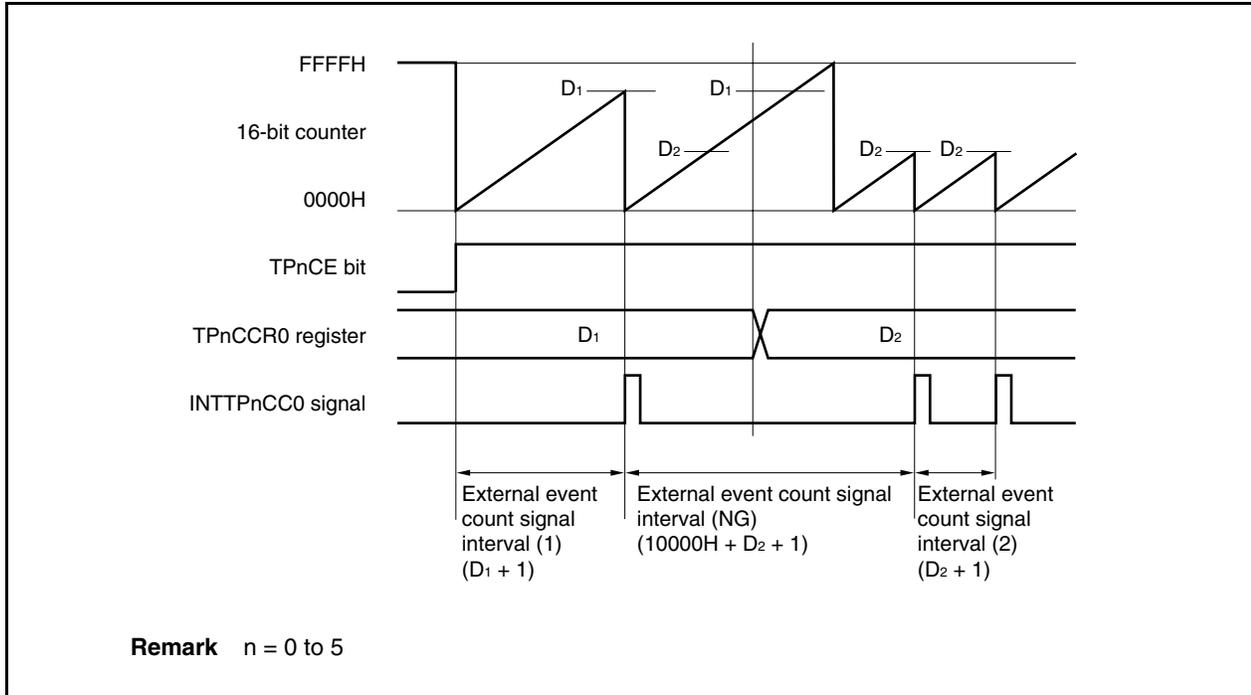
If the value of the TPnCCR0 register is changed from  $D_1$  to  $D_2$  while the count value is greater than  $D_2$  but less than  $D_1$ , the count value is transferred to the CCR0 buffer register as soon as the TPnCCR0 register has been rewritten. Consequently, the value that is compared with the 16-bit counter is  $D_2$ .
