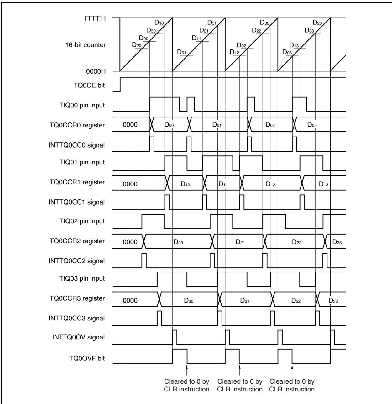
Figure 8-31. Register Setting in Free-Running Timer Mode (1/3)
