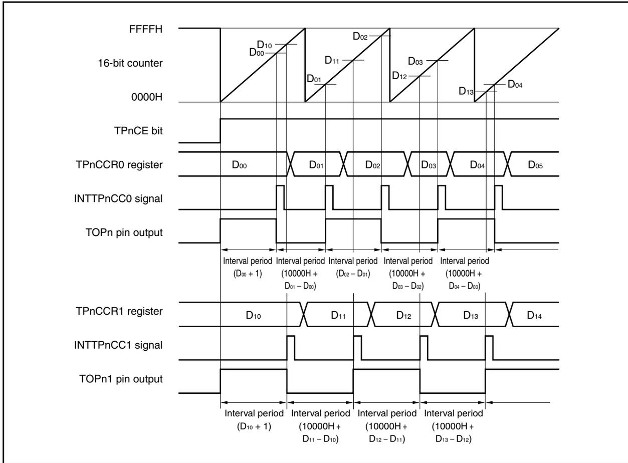
When performing an interval operation in the free-running timer mode, two intervals can be set with one channel.
