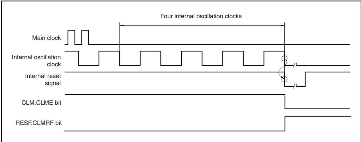
**(2) Clock monitor status after  $\overline{\text{RESET}}$  input**
