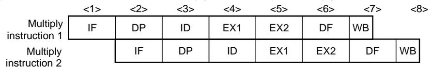
[Description] The pipeline has seven stages: the IF, DP, ID, EX, AT, DF, and WB stages. The EX stage requires two clocks, and EX1 and EX2 operate independently. Accordingly, even if the multiply instruction (or the multiply-accumulate instruction) is repeated, the number of execution clocks becomes one.
