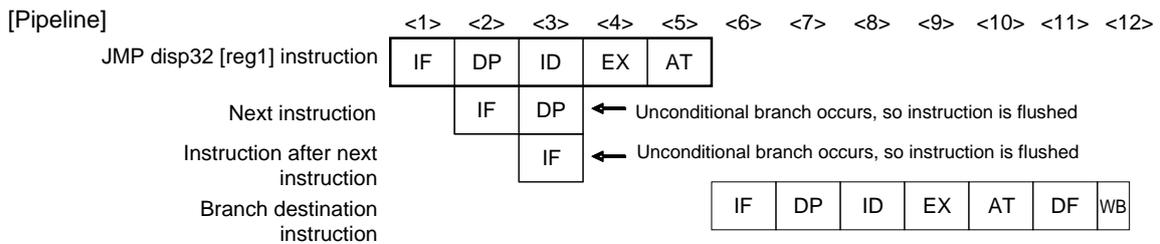
[Description] This figure shows an operation where a JMP is executed by the instruction execution pipeline right (Rpipe) and all instructions are executed by instruction execution pipeline left (Lpipe). This instruction can be executed in parallel with other instructions.
