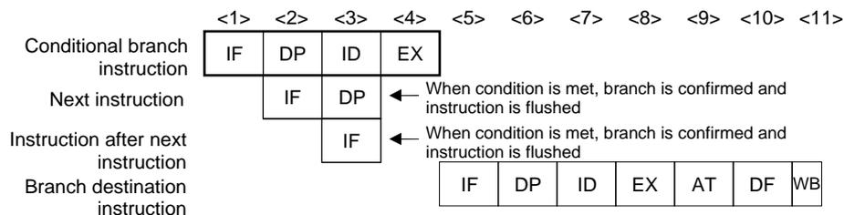
[Description] This figure shows an operation where a Bcond instruction is executed by the instruction execution pipeline right (Rpipe). Branch instructions can be executed in parallel with another instruction.
