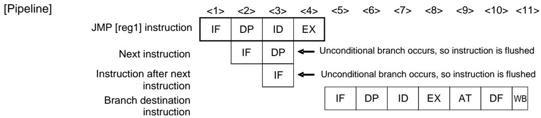
[Description] This figure shows an operation where a JMP is executed by the instruction execution pipeline right (Rpipe), and all instructions are executed by instruction execution pipeline left (Lpipe). This instruction can be executed in parallel with other instructions.
