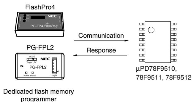
Communication commands are listed in the table below. All these communication commands are issued from the flash memory programmer and the  $\mu$ PD78F9510, 78F9511, 78F9512 perform processing corresponding to the respective communication commands.
