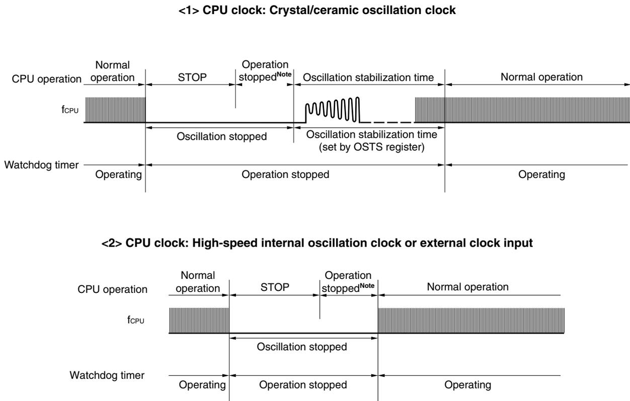
**Note** The operation stop time is 17  $\mu$ s (MIN.), 34  $\mu$ s (TYP.), and 67  $\mu$ s (MAX.).
