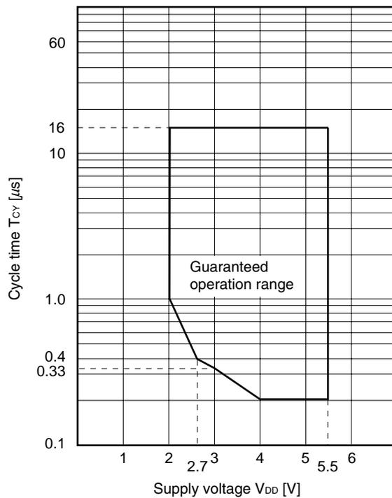
**T<sub>CY</sub> vs. V<sub>DD</sub> (High-speed internal oscillator Clock)**
