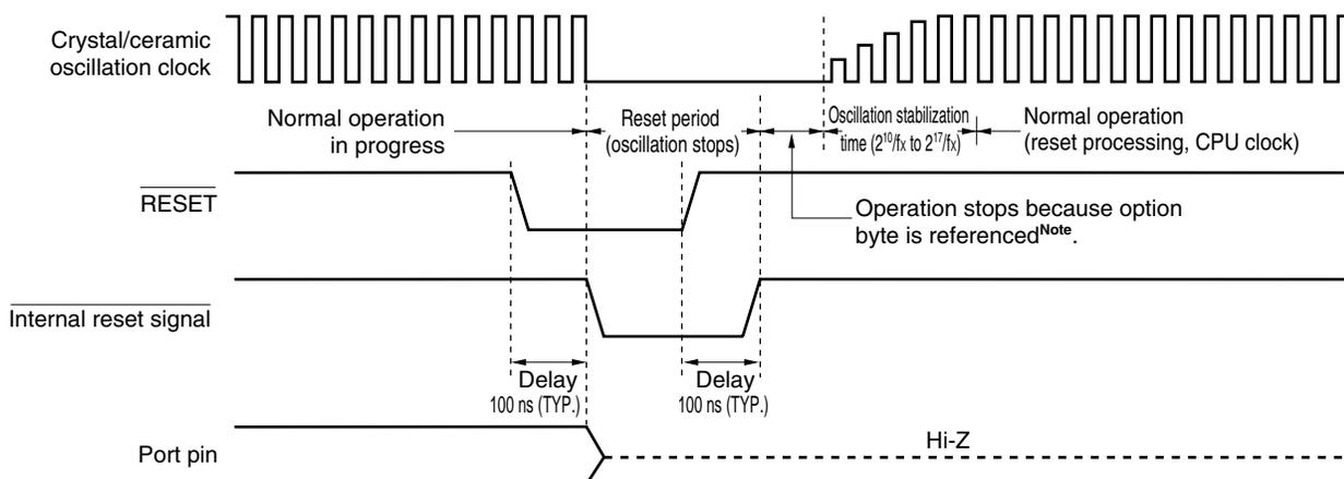
**Note** The operation stop time is 276  $\mu\text{s}$  (MIN.), 544  $\mu\text{s}$  (TYP.), and 1.074 ms (MAX.).
