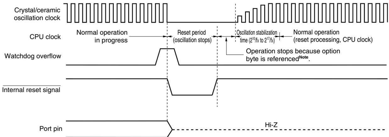
**Note** The operation stop time is 276  $\mu$ s (MIN.), 544  $\mu$ s (TYP.), and 1.074 ms (MAX.).
