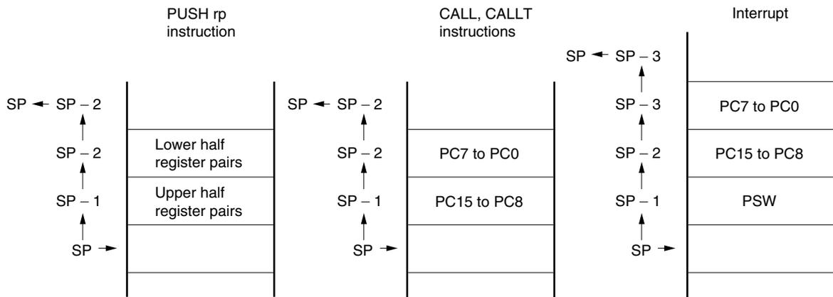
Figure 3-11. Data to Be Restored from Stack Memory
