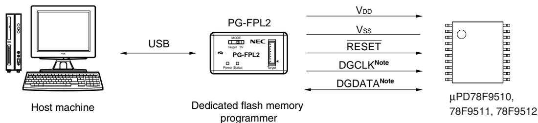
**Note** DGCLK is a clock for communication, while DGDATA is a transmit/receive signal for communication data.
