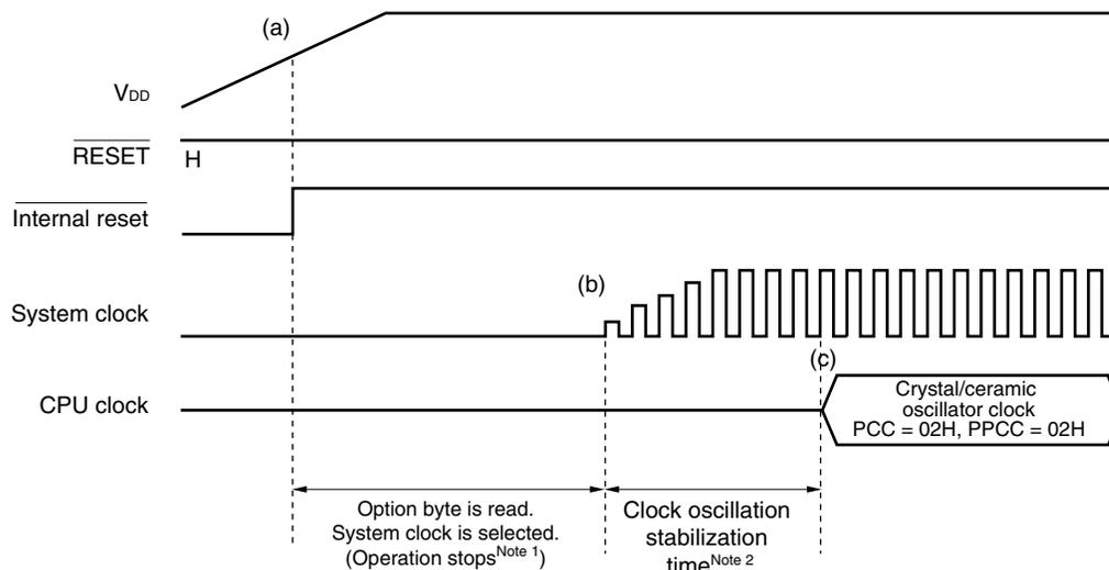
**Notes** 1. Operation stop time is 276  $\mu$ s (MIN.), 544  $\mu$ s (TYP.), and 1.074 ms (MAX.).
