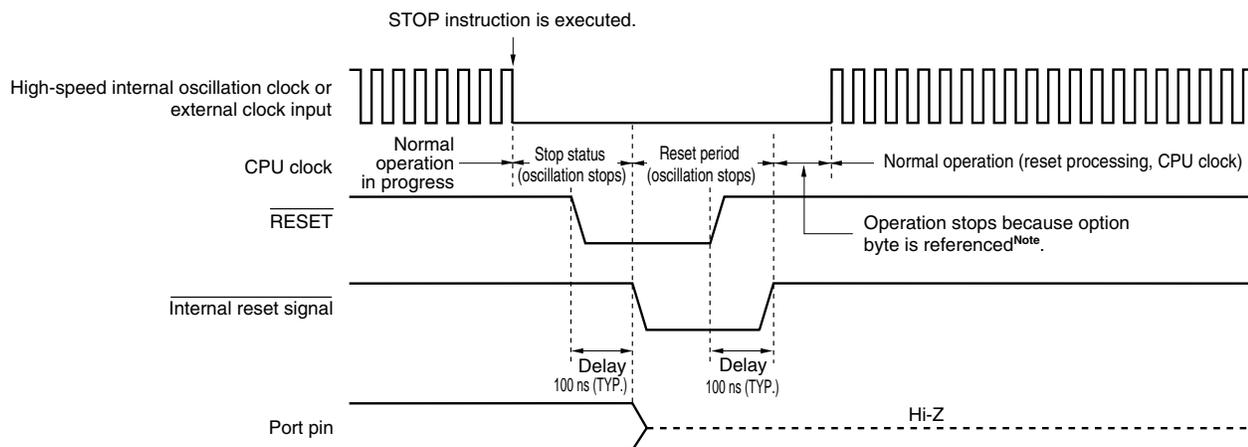
**Note** The operation stop time is 277  $\mu$ s (MIN.), 544  $\mu$ s (TYP.), and 1.075 ms (MAX.).
