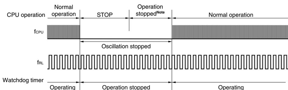
**Note** The operation stop time is 17 μs (MIN.), 34 μs (TYP.), and 67 μs (MAX.).
