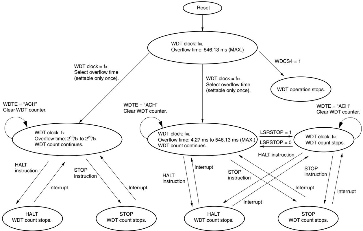
**8.4.3 Watchdog timer operation in STOP mode (when “low-speed internal oscillator can be stopped by software” is selected by option byte)**
