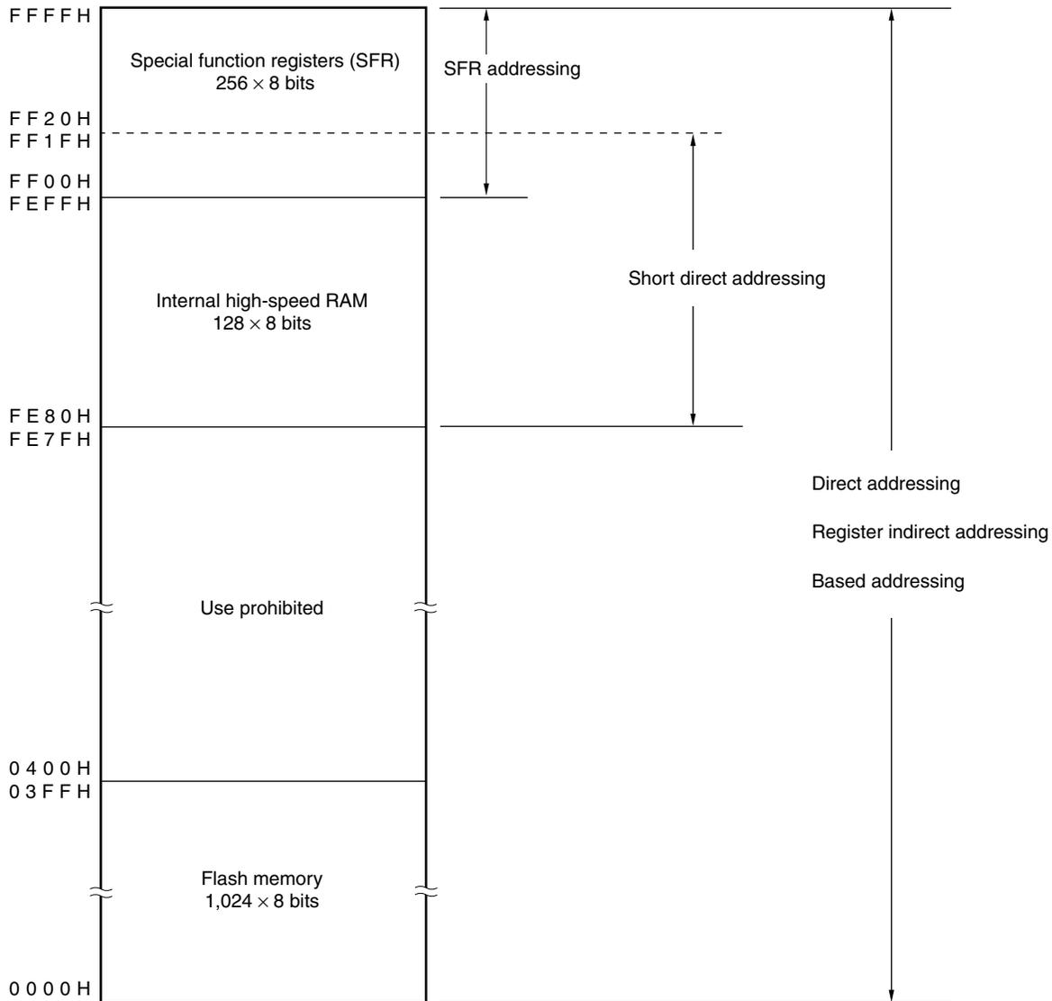
Figure 3-5. Data Memory Addressing ( $\mu$ PD78F9511)
