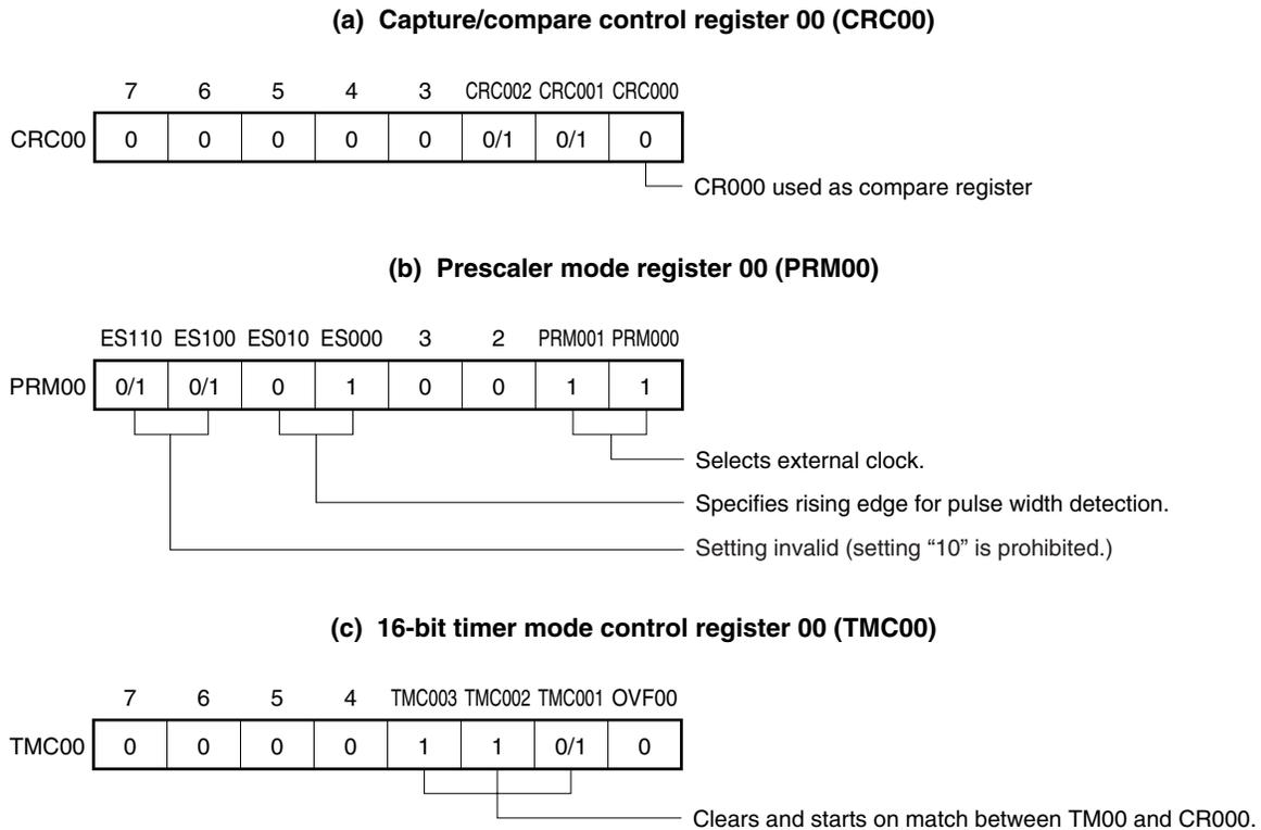
**Remark** 0/1: Setting 0 or 1 allows another function to be used simultaneously with the external event counter. See the description of the respective control registers for details.
