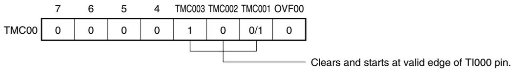
**Note** If the valid edge of TI000 is specified to be both the rising and falling edges, 16-bit timer capture/compare register 000 (CR000) cannot perform the capture operation.
