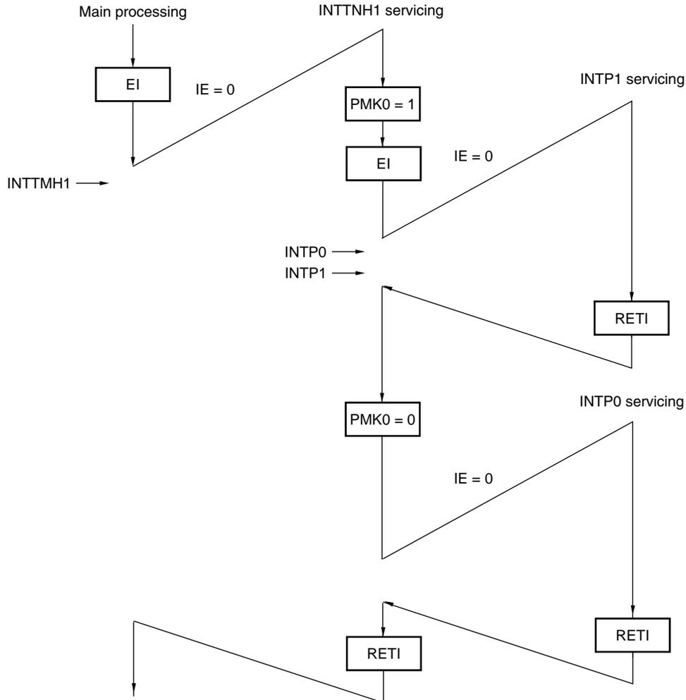
In the interrupt INTTMH1 servicing, servicing is performed such that the INTP1 interrupt is given priority, since the INTPO interrupt was first masked.
