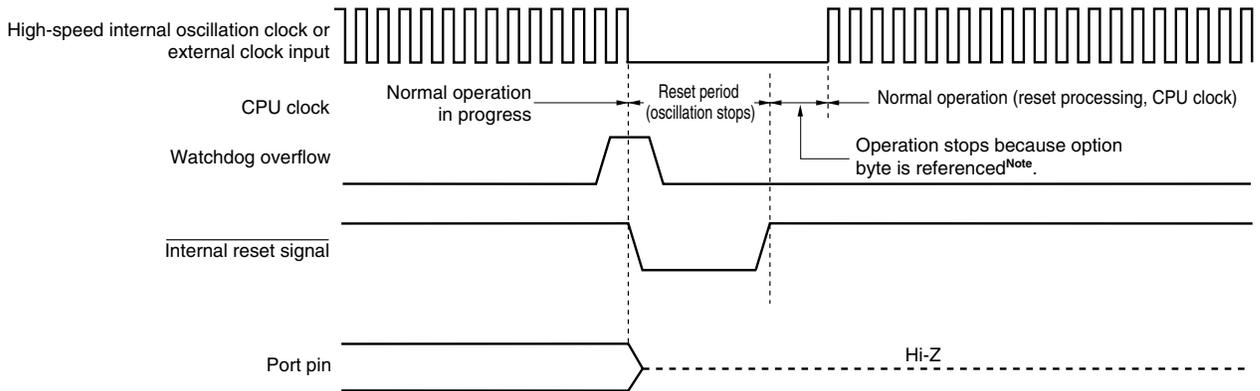
**Note** The operation stop time is 277  $\mu$ s (MIN.), 544  $\mu$ s (TYP.), and 1.075 ms (MAX.).
