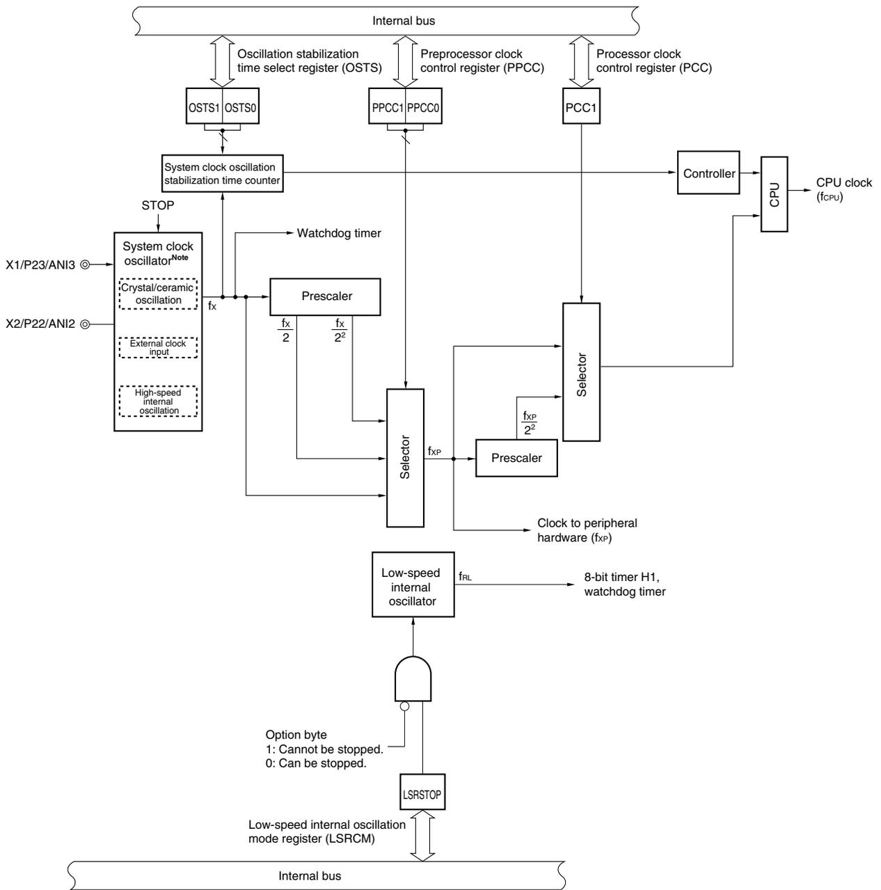
**Note** Select the high-speed internal oscillator, crystal/ceramic oscillator, or external clock input circuit as the system clock source by using the option byte.
