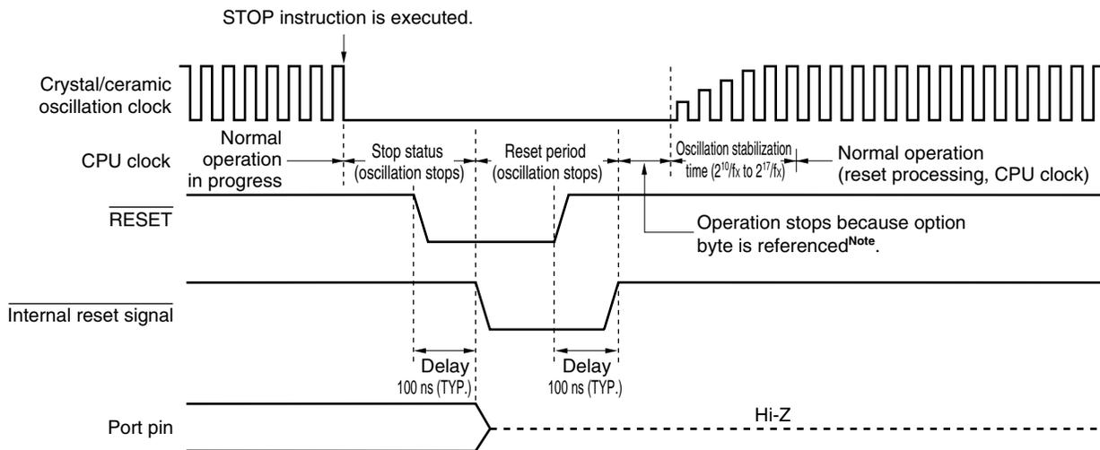
**Note** The operation stop time is 276  $\mu$ s (MIN.), 544  $\mu$ s (TYP.), and 1.074 ms (MAX.).
