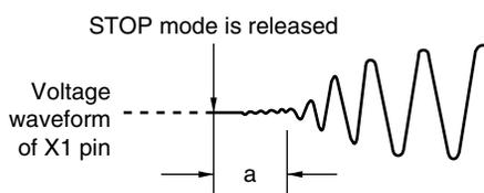
**3. The oscillation stabilization time that elapses on power application or after release of reset is selected by the option byte. For details, refer to CHAPTER 14 OPTION BYTE.**
