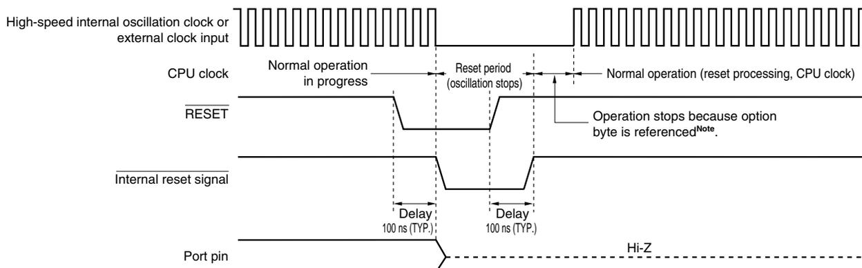
**Note** The operation stop time is 277  $\mu\text{s}$  (MIN.), 544  $\mu\text{s}$  (TYP.), and 1.075 ms (MAX.).
