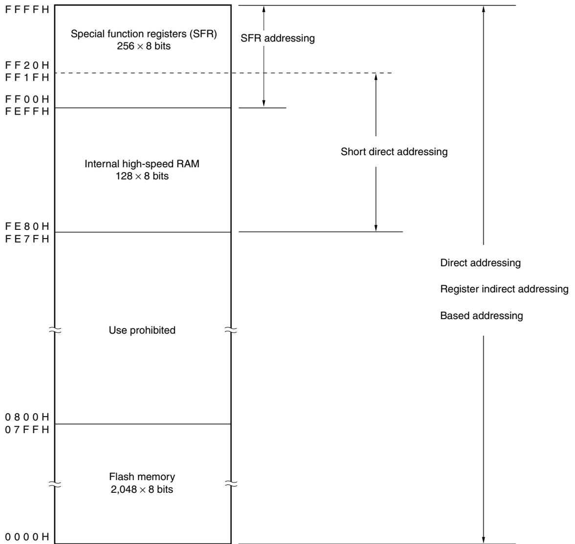
Figure 3-6. Data Memory Addressing ( $\mu$ PD78F9512)
