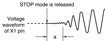
**3.** The oscillation stabilization time that elapses on power application or after release of reset is selected by the option byte. For details, refer to **CHAPTER 14 OPTION BYTE**.
