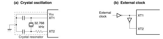
Caution When using the main system or subsystem clock oscillator, wire as follows in the area enclosed by the broken lines in Figures 7-5 and 7-6 to avoid an adverse effect from wiring capacitance.
