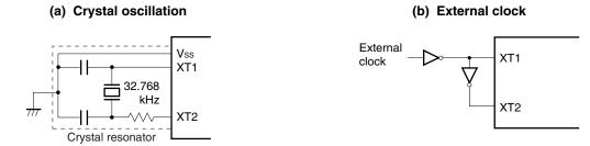
Caution When using the main system or subsystem clock oscillator, wire as follows in the area enclosed by the broken lines in Figures 8-5 and 8-6 to avoid an adverse effect from wiring capacitance.
