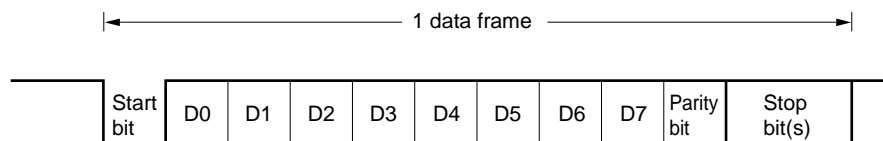
Figure 18-5. Asynchronous Serial Interface Transmit/Receive Data Format
