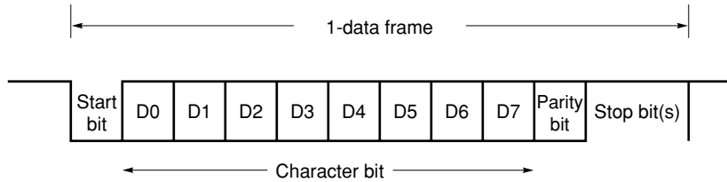
Figure 17-7. Asynchronous Serial Interface Transmit/Receive Data Format
