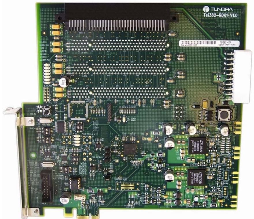
The evaluation board uses the Tsi382A to bridge between x1 PCIe on the card edge to four 32-bit PCI slots on the board.
