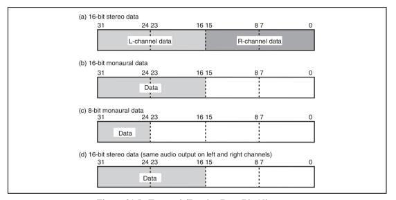
Figure 21.5 Transmit/Receive Data Bit Alignment
