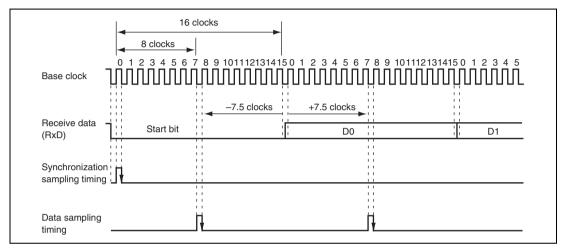
Figure 22.19 Receive Data Sampling Timing in Asynchronous Mode
