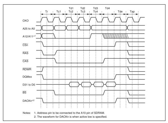
Figure 11.14 Burst Read Basic Timing (Auto-Precharge)
