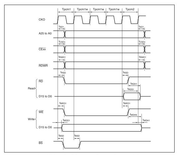
Figure 33.35 PCMCIA Memory Card Interface Bus Timing
