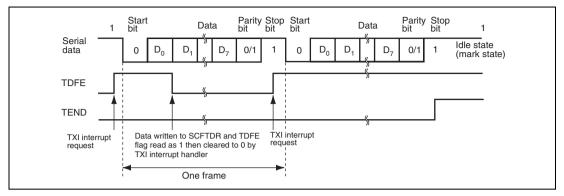
Figure 22.5 Example of Transmit Operation (8-Bit Data, Parity, 1 Stop Bit)
