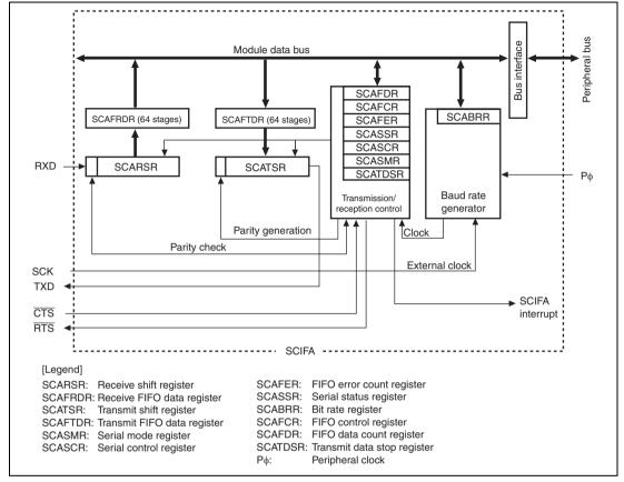
Figure 23.1 Block Diagram of SCIFA
