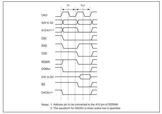
Figure 11.22 Single Write Timing (No Auto-Precharge)
