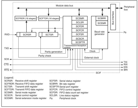
Figure 22.1 Block Diagram of SCIF
