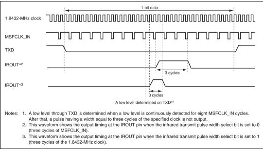
Figure 24.5 Timing for Encoding Infrared Transmit (Light-Emit) Pulse Data
