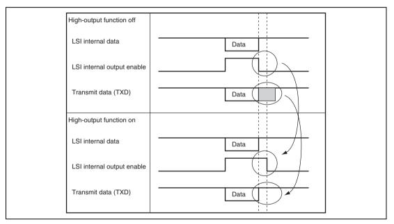
Figure 25.10 High-Output Function Timechart
