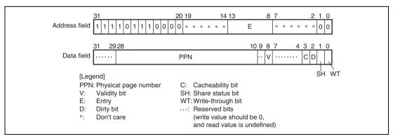
Figure 7.24 Memory-Mapped UTLB Data Array 1 (TLB Extended Mode)
