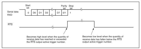
Figure 22.10 Example of Operation Using Modem Control (RTS)
