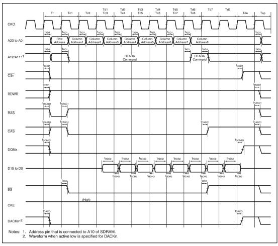
Figure 33.18 Burst Read Bus Cycle of SDRAM (Single Read × 8) (Auto Precharge Mode, CAS Latency 2, TRCD = 1 Cycle, TRP = 2 Cycles)
