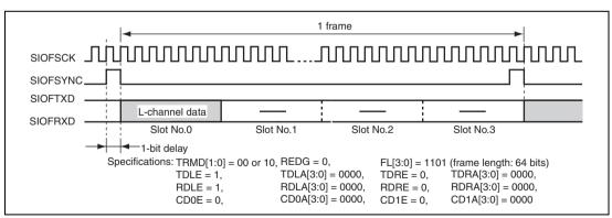
Figure 21.15 Transmit and Receive Timing (16-Bit Monaural Data)
