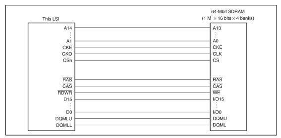
Figure 11.13 Example of 16-Bit Data-Width SDRAM Connection
