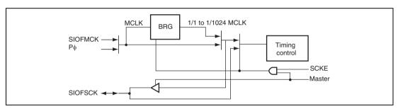
Figure 21.2 Serial Clock Supply
