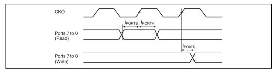
Figure 33.40 I/O Port Timing
