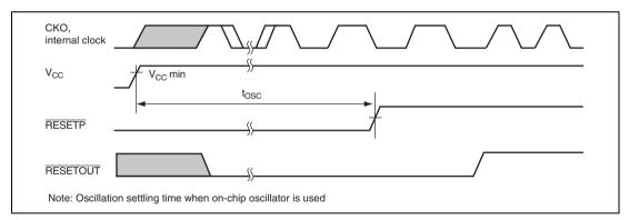
Figure 33.3 Power-On Oscillation Settling Time
