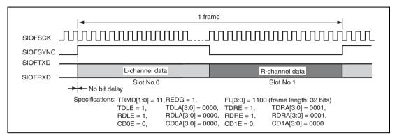
Figure 21.16 Transmit and Receive Timing (16-Bit Stereo Data (1))
