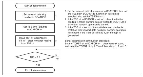
Figure 23.6 Transmit Data Stop Function Flowchart
