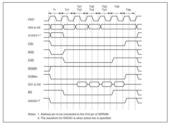
Figure 11.19 Burst Read Timing (No Auto-Precharge)
