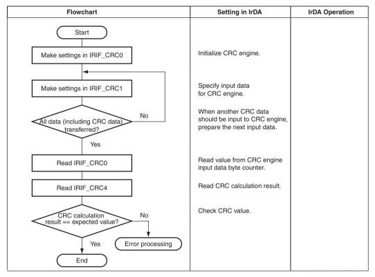
Figure 24.12 IrDA Reception (CRC Calculation) Flow
