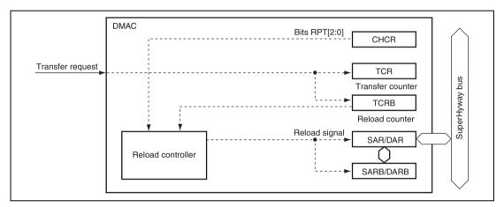
Figure 12.11 Reload Mode Transfer
