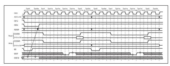
Figure 11.41 Timing for Dynamic Bus Sizing of PCMCIA I/O Card Interface (TED[3:0] = B'0010, TEH[3:0] = B'0001, Software Waits = 3)
