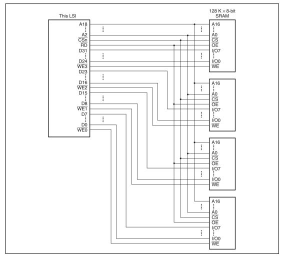
Figure 11.6 Example of 32-Bit Data-Width SRAM Connection
