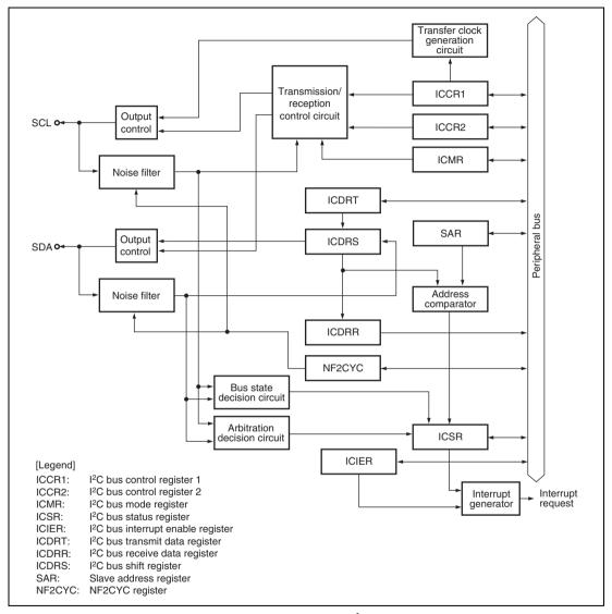
Figure 20.1 Block Diagram of I<sup>2</sup>C Bus Interface
