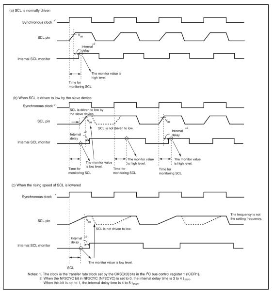
Figure 20.18 Bit Synchronous Circuit Timing
