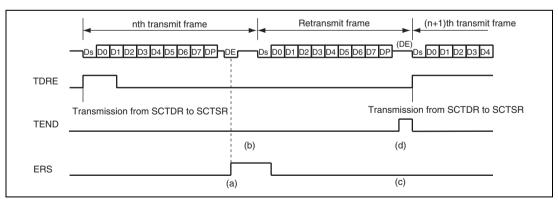
Figure 25.9 Retransmit Standby Mode (Clock Stopped) when Smart Card Interface is in Transmit Mode
