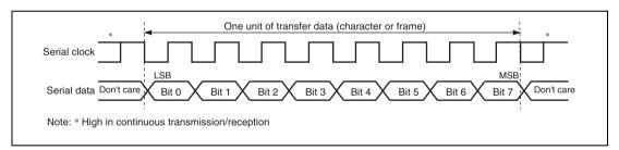
Figure 23.12 Data Format in Synchronous Communication
