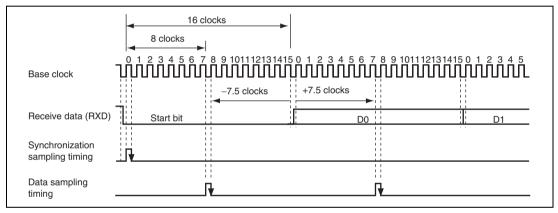
Figure 23.22 Receive Data Sampling Timing in Asynchronous Mode
