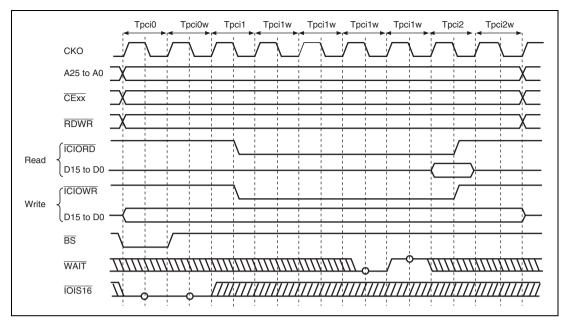
Figure 11.40 Wait Timing for PCMCIA I/O Card Interface (TED[3:0] = B'0010, TEH[3:0] = B'0001, Software Wait = 1, Hardware Wait = 1)
