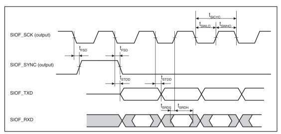
Figure 33.48 SIOF Transmission/Reception Timing (Master Mode 1, Rise Sampling)
