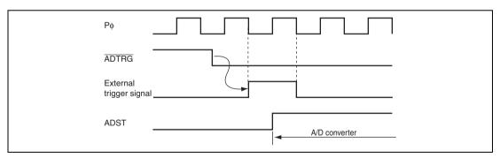
Figure 26.6 External Trigger Input Timing
