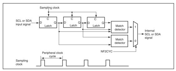
Figure 20.13 Block Diagram of Noise Filter
