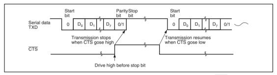
Figure 22.6 Example of Operation Using Modem Control (CTS)
