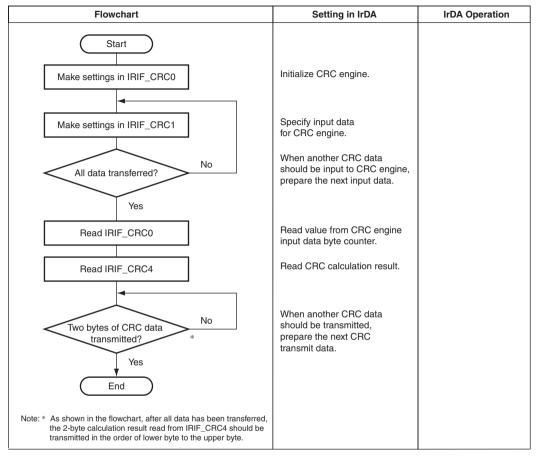
Figure 24.10 IrDA Transmission (CRC Calculation) Flow
