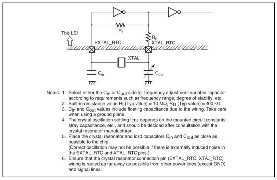
Figure 17.6 Example of Crystal Oscillator Circuit Connection
