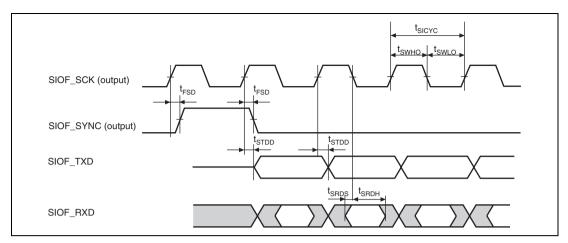
Figure 33.47 SIOF Transmission/Reception Timing (Master Mode 1, Fall Sampling)
