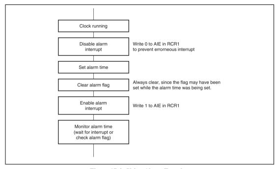
**Figure 17.4 Using Alarm Function**
