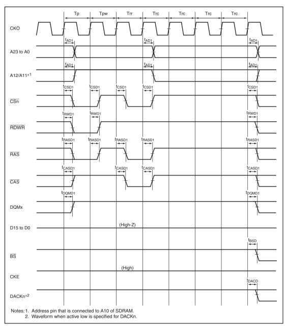
Figure 33.30 Auto Refresh Timing of SDRAM (TRP = 2 Cycles)
