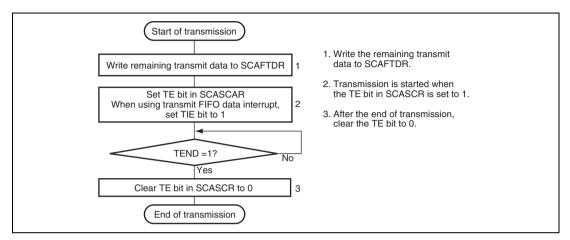
Figure 23.16 Sample Serial Transmission Flowchart (1) (First Transmission after Initialization)
