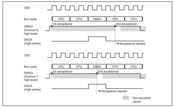
Figure 12.13 Example of DREQ Input Detection in Cycle Steal Mode Level Detection
