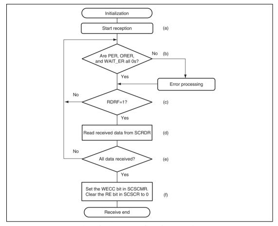
Figure 25.6 Example of Receive Processing
