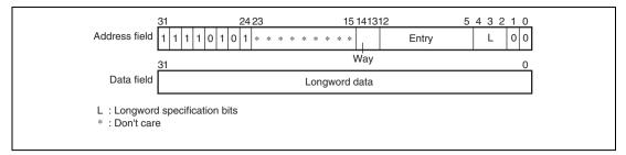
Figure 8.8 Memory-Mapped OC Data Array
