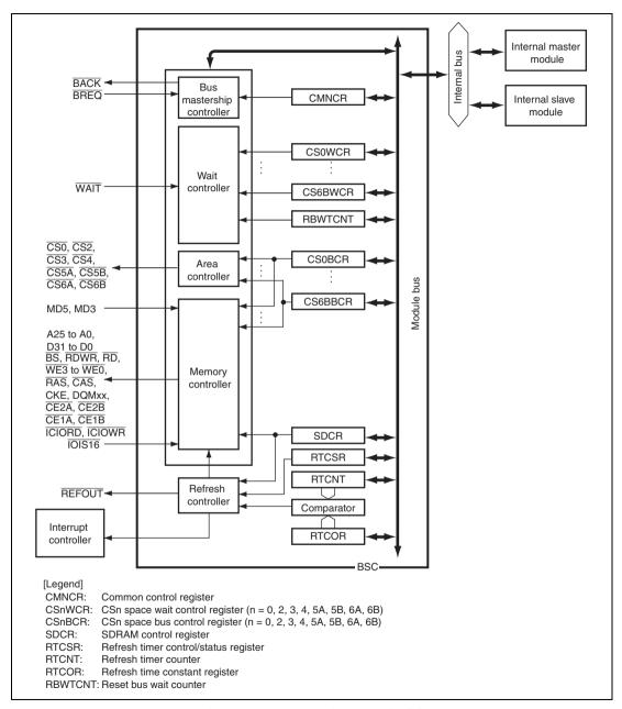
Figure 11.1 Block Diagram of BSC
