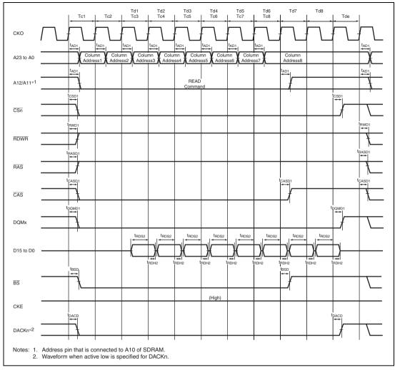
Figure 33.25 Burst Read Bus Cycle of SDRAM (Single Read × 8)
