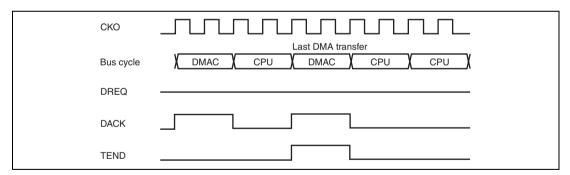
Figure 12.16 DMA Transfer End Signal Timing (Level Detection in Cycle Steal Mode)
