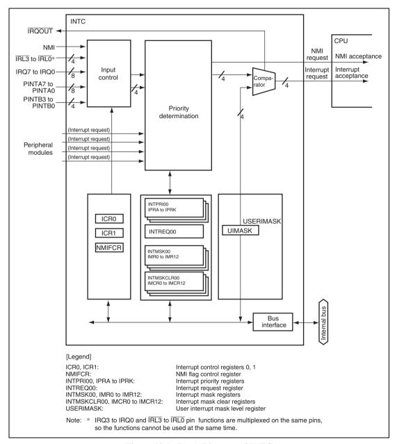
Figure 10.1 Block Diagram of INTC
