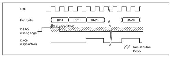
Figure 12.14 Example of DREQ Input Detection in Burst Mode Edge Detection
