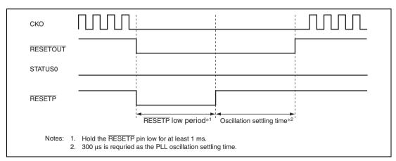
Figure 14.2 State of Output Pins at Power-On Reset
