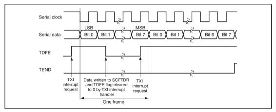
Figure 22.14 Example of SCIF Transmit Operation
