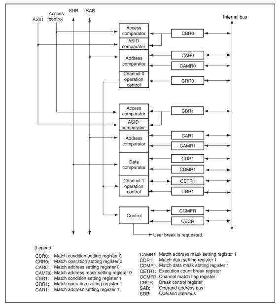
Figure 30.1 Block Diagram of UBC
