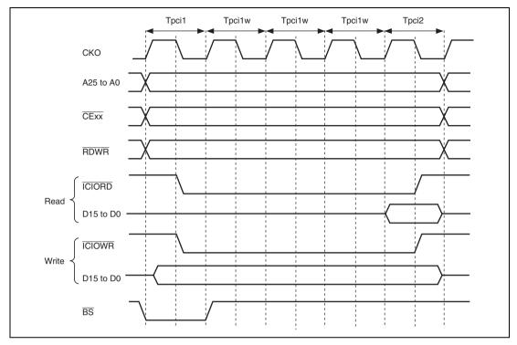
Figure 11.39 Basic Timing for PCMCIA I/O Card Interface
