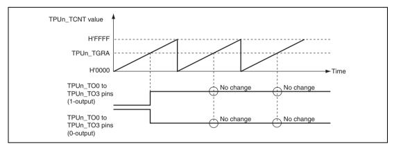
Figure 16.6 Example of 0-Output/1-Output Operation
