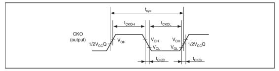
Figure 33.2 CKIO Clock Output Timing
