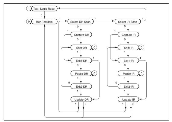
Figure 31.2 TAP Controller State Transitions
