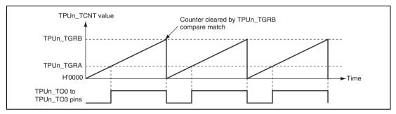
Figure 16.12 Example of PWM Mode Operation (1)
