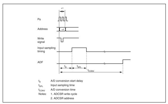
Figure 26.5 A/D Conversion Timing
