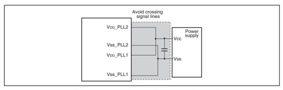
Figure 13.2 Points to Note in Use of the PLL Oscillator Circuit
