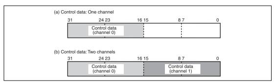
Figure 21.6 Control Data Bit Alignment
