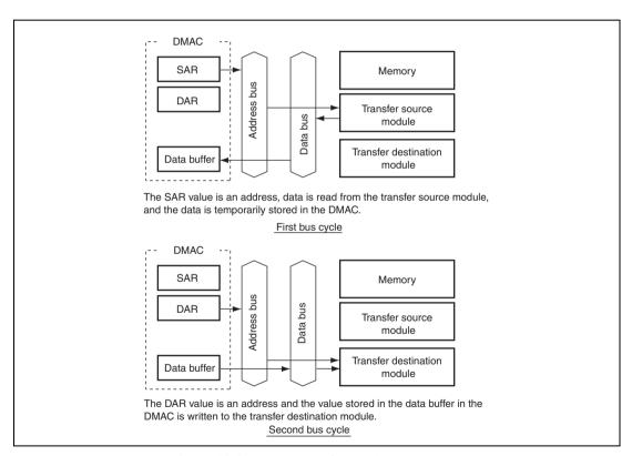
Figure 12.4 Data Flow of Dual Address Mode
