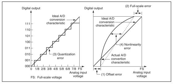
Figure 26.7 Definitions of A/D Conversion Accuracy
