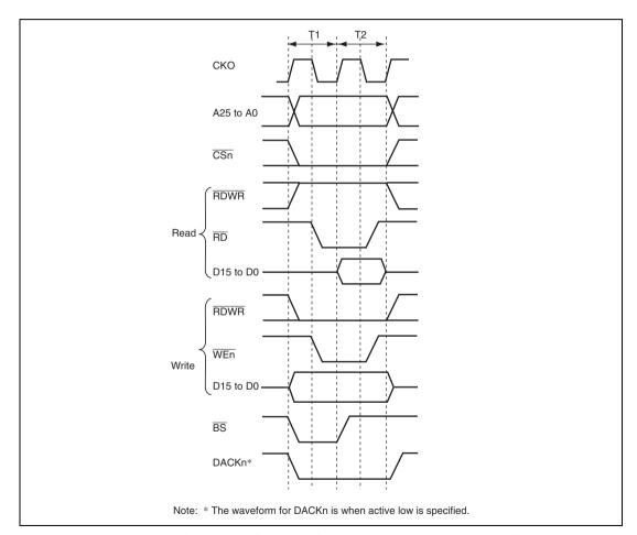
Figure 11.3 Normal Space Basic Access Timing (Access Wait 0)
