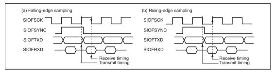
Figure 21.4 SIOF Transmit/Receive Timing
