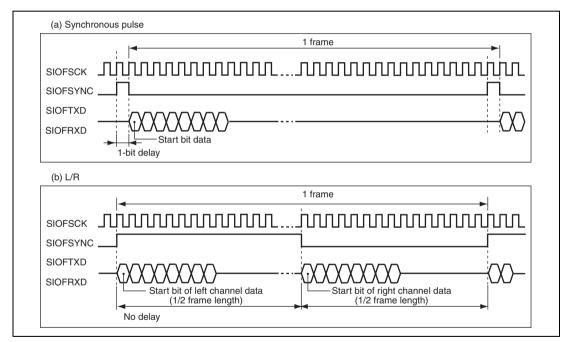
Figure 21.3 Serial Data Synchronization Timing
