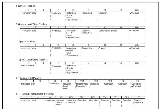
Figure 4.1 Basic Pipelines
