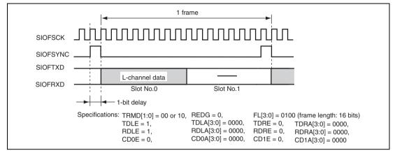
Figure 21.14 Transmit and Receive Timing (8-Bit Monaural Data (2))
