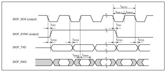
Figure 33.50 SIOF Transmission/Reception Timing (Master Mode 2, Rise Sampling)
