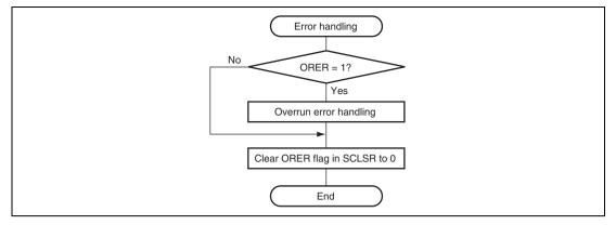
Figure 22.16 Sample Flowchart for Receiving Serial Data (2)
