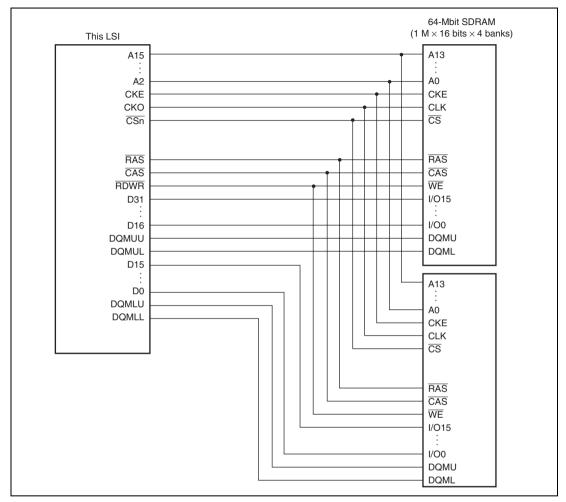
Figure 11.12 Example of 32-Bit Data-Width SDRAM Connection
