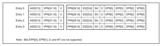
Figure 7.13 ITLB Configuration (TLB Extended Mode)
