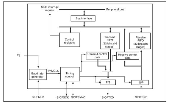
Figure 21.1 Block Diagram of SIOF
