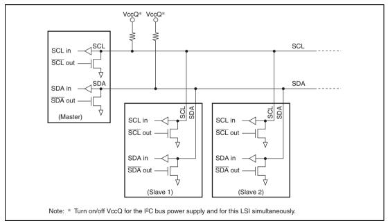
Figure 20.2 External Circuit Connections of I/O Pins
