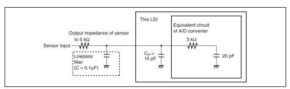
Figure 26.8 Analog Input Circuit Example
