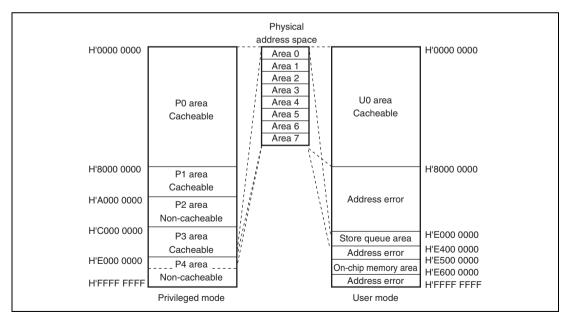
Figure 7.2 Virtual Address Space (AT in MMUCR= 0)
