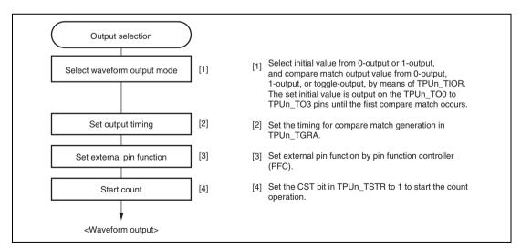
Figure 16.5 Example of Setting Procedure for Waveform Output by Compare Match
