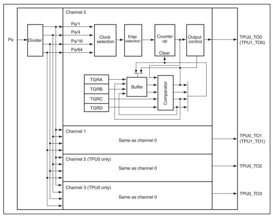
Figure 16.1 TPU0 and TPU1 Block Diagram
