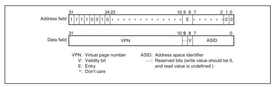
Figure 7.18 Memory-Mapped ITLB Address Array
