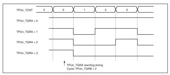
Figure 16.13 Example of PWM Mode Operation (2)
