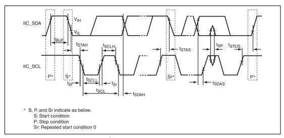
Figure 33.45 I<sup>2</sup>C Bus Interface Input/Output Timing
