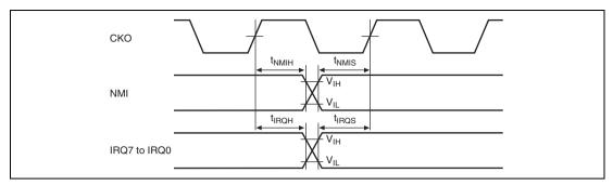
Figure 33.5 Interrupt Signal Input Timing
