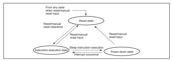
Figure 2.8 Processing State Transitions
