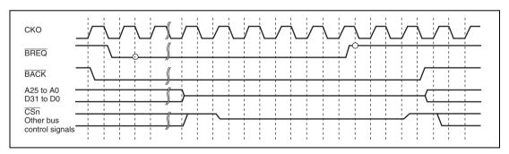
Figure 11.42 Bus Arbitration Timing
