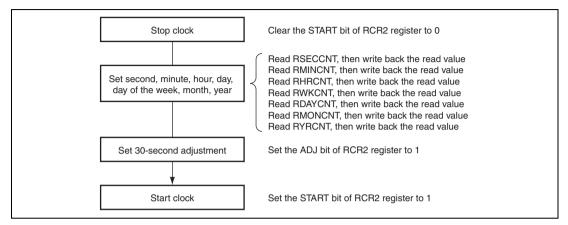
Figure 17.7 Usage of 30-Second Adjustment
