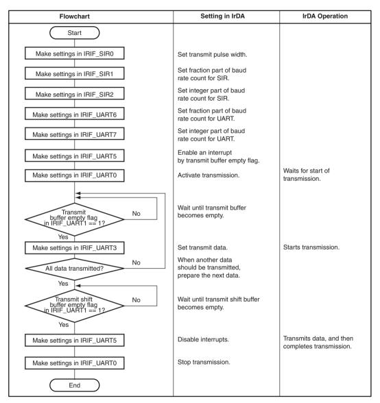
Figure 24.9 IrDA Transmission Flow
