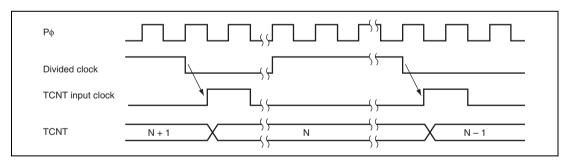
Figure 18.4 Count Timing when Internal Clock is Operating
