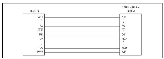
Figure 11.8 Example of 8-Bit Data-Width SRAM Connection
