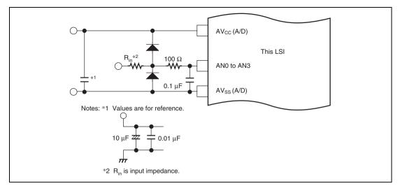
Figure 26.9 Example of Analog Input Protection Circuit
