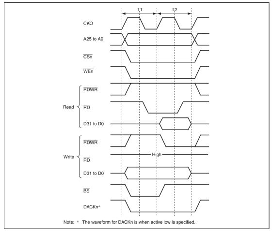
Figure 11.31 Basic Access Timing for Byte-Selection SRAM (BAS = 1)
