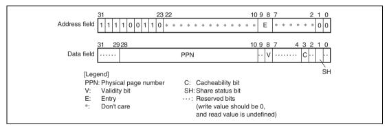
Figure 7.20 Memory-Mapped ITLB Data Array 1 (TLB Extended Mode)
