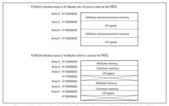
Figure 11.38 Example of PCMCIA Space Assignment (CS5BWCR.SA[1:0] = B'10, CS6BWCR.SA[1:0] = B'10)
