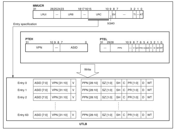
Figure 7.16 Operation of LDTLB Instruction (TLB Compatible Mode)
