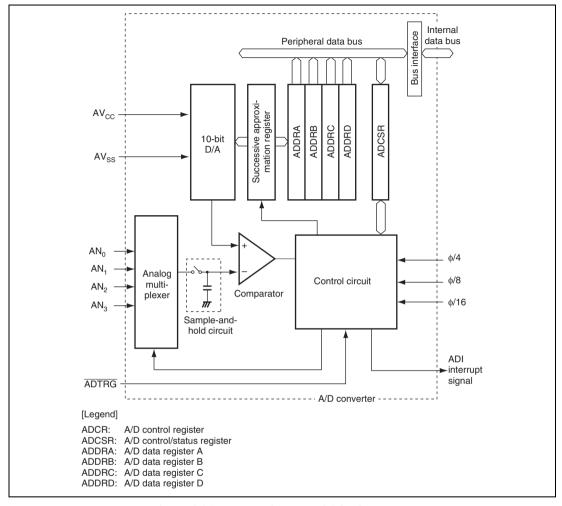
Figure 26.1 Block Diagram of A/D Converter
