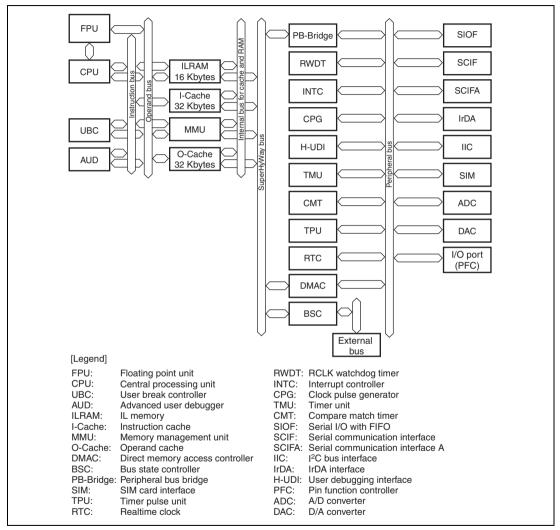
Figure 1.1 Block Diagram of This LSI
