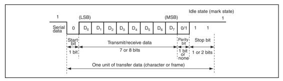
Figure 22.2 Example of Data Format in Asynchronous Communication (8-Bit Data with Parity and Two Stop Bits)
