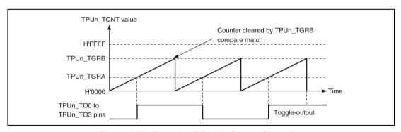
Figure 16.7 Example of Toggle Output Operation
