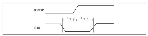
Figure 33.56 TRST Input Timing (Reset Hold)
