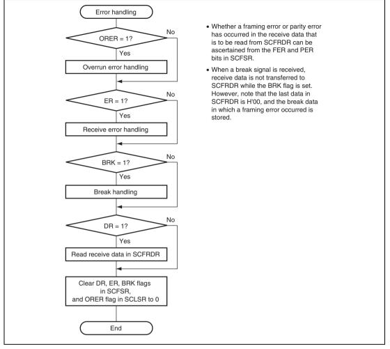
Figure 22.8 Sample Flowchart for Receiving Serial Data (cont)
