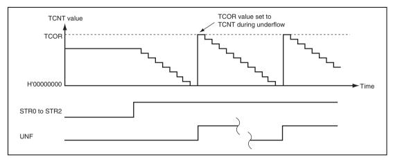
Figure 18.3 Auto-Reload Count Operation
