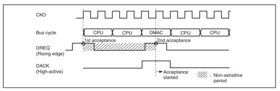
Figure 12.12 Example of DREQ Input Detection in Cycle Steal Mode Edge Detection
