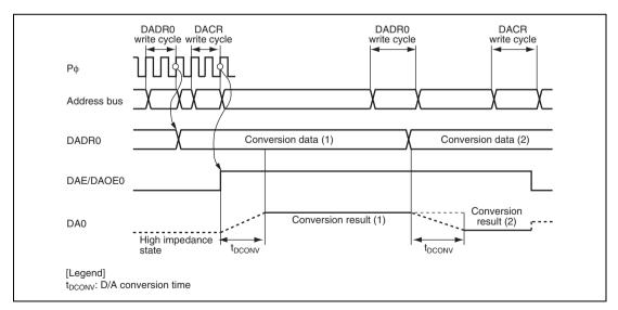
Figure 27.2 D/A Converter Operation Example
