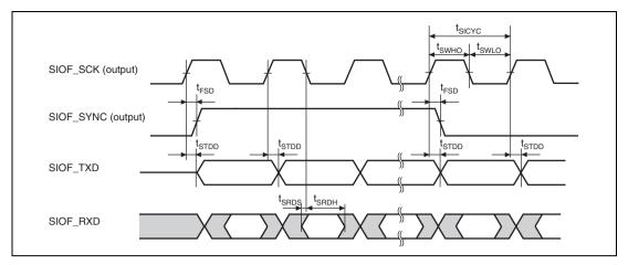
Figure 33.49 SIOF Transmission/Reception Timing (Master Mode 2, Fall Sampling)
