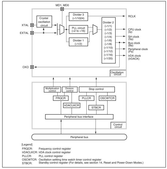
Figure 13.1 Block Diagram of CPG
