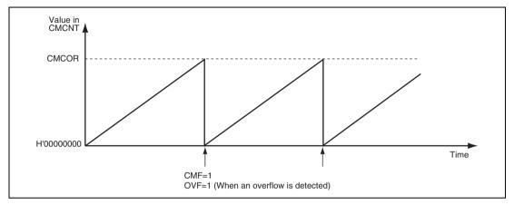
Figure 19.3 Counter Operation (Free-Running Operation)
