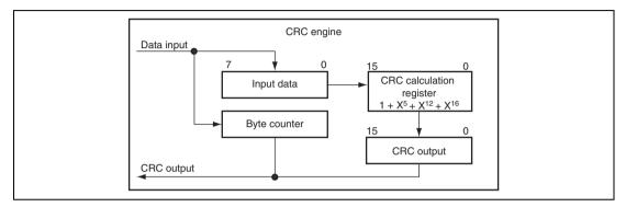
Figure 24.7 CRC Engine Configuration
