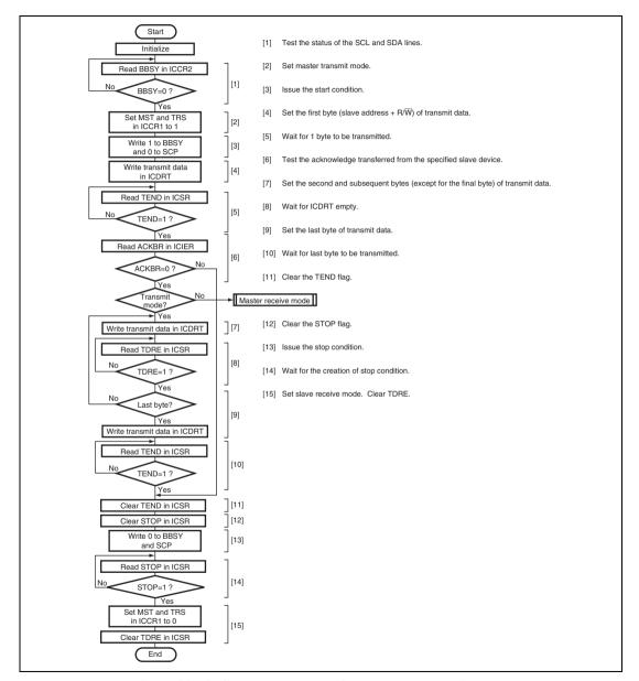
Figure 20.14 Sample Flowchart for Master Transmit Mode
