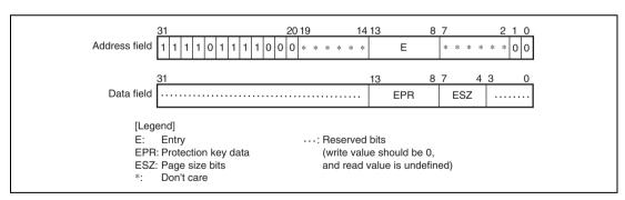
Figure 7.25 Memory-Mapped UTLB Data Array 2 (TLB Extended Mode)
