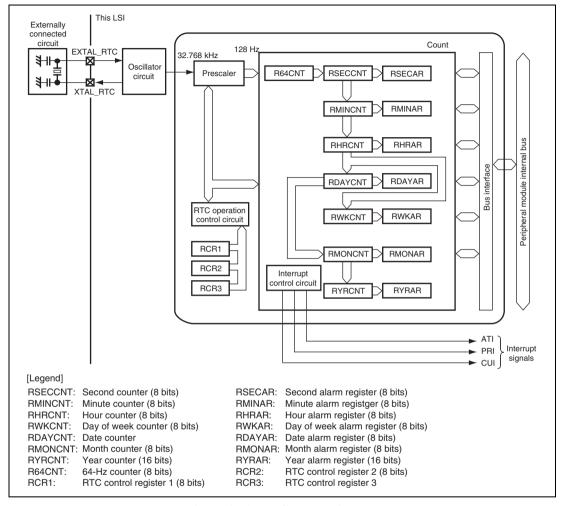
Figure 17.1 RTC Block Diagram
