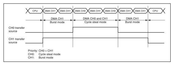
Figure 12.9 Bus State when Multiple Channels are Operating
