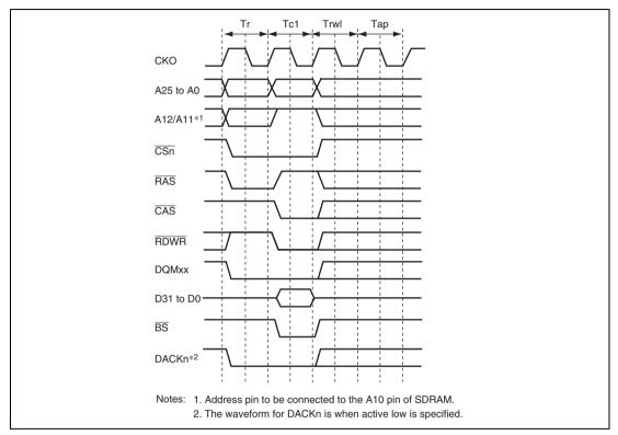
Figure 11.18 Basic Timing for Single Write (Auto-Precharge)
