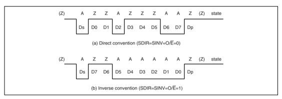
Figure 25.3 Examples of Start Character Waveforms
