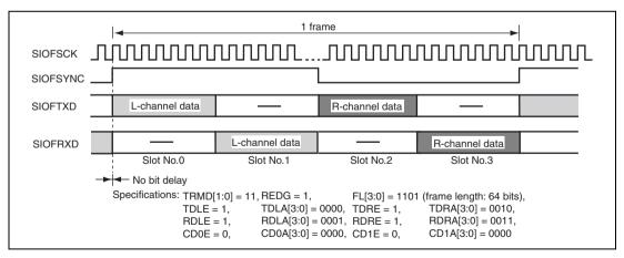
Figure 21.17 Transmit and Receive Timing (16-Bit Stereo Data (2))
