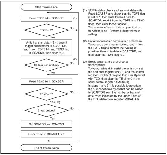
Figure 23.3 Sample Serial Transmission Flowchart
