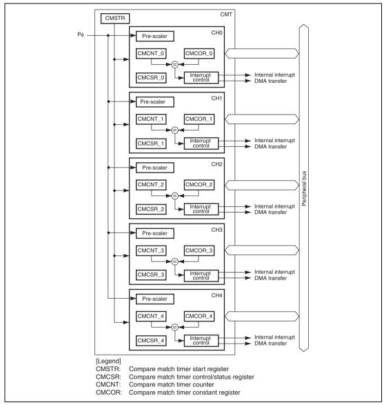
Figure 19.1 Block Diagram of CMT
