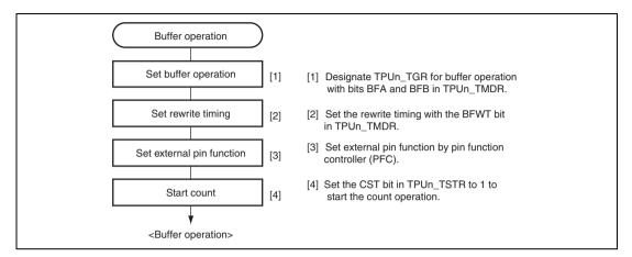
Figure 16.9 Example of Buffer Operation Setting Procedure
