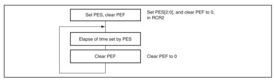
Figure 17.5 Using Periodic Interrupt Function
