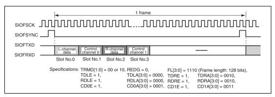
Figure 21.7 Control Data Interface (Slot Position)
