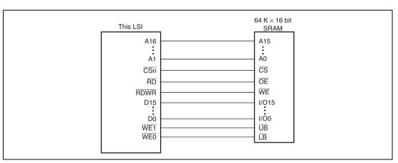
Figure 11.34 Example of Connection with 16-Bit Data-Width Byte-Selection SRAM
