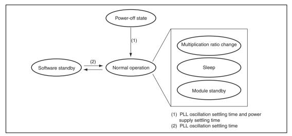
Figure 14.1 Mode Transition Diagram
