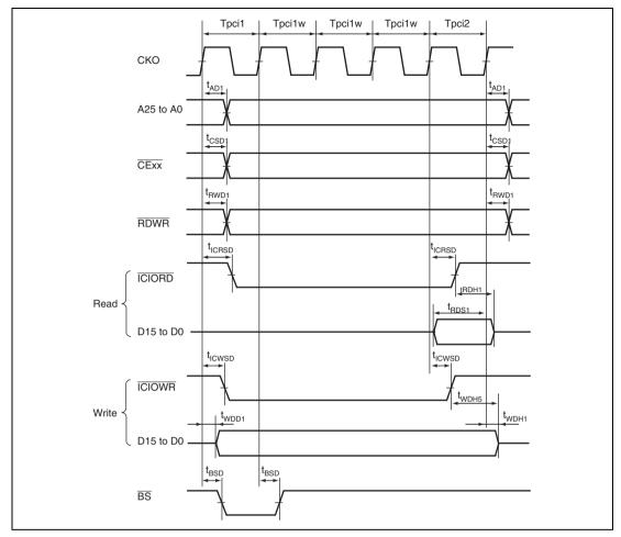
Figure 33.37 PCMCIA I/O Card Interface Bus Timing
