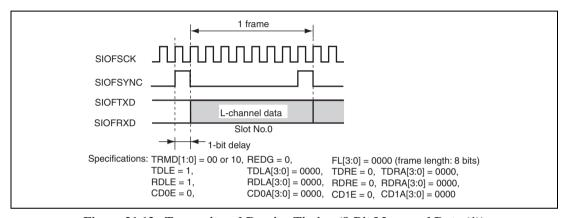
Figure 21.13 Transmit and Receive Timing (8-Bit Monaural Data (1))
