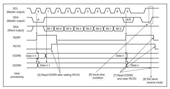
Figure 20.8 Master Receive Mode Operation Timing (2)
