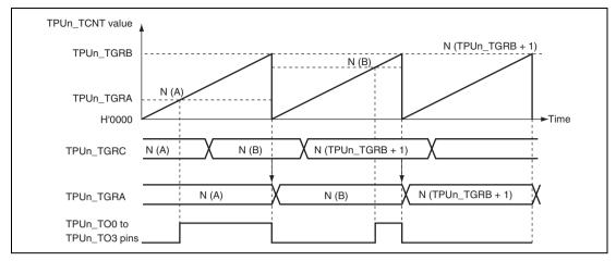
Figure 16.10 Example of Buffer Operation
