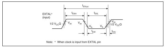
Figure 33.1 EXTAL Clock Input Timing
