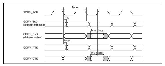
Figure 33.53 SCI Input/Output Timing in Clock Synchronous Mode
