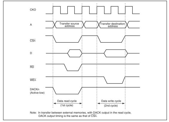
Figure 12.5 Example of DMA Transfer Timing in Dual Mode (Source: Ordinary Memory, Destination: Ordinary Memory)
