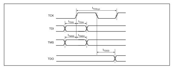
Figure 33.57 H-UDI Data Transfer Timing
