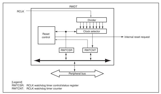
Figure 15.1 Block Diagram of RWDT
