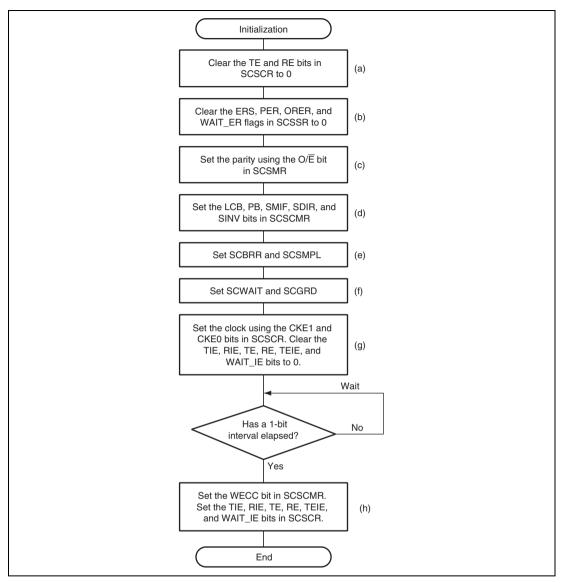
Figure 25.4 Example of Initialization Flow
