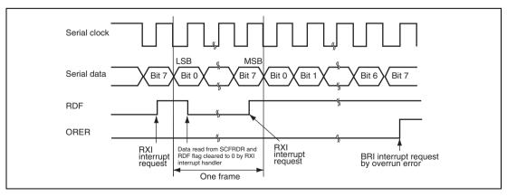
Figure 22.17 Example of SCIF Receive Operation
