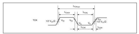
Figure 33.55 TCK Input Timing
