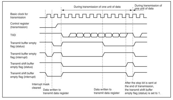
Figure 24.3 Data Transmission Timing
