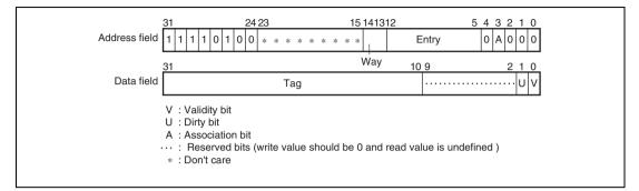
Figure 8.7 Memory-Mapped OC Address Array
