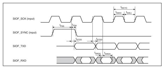
Figure 33.51 SIOF Transmission/Reception Timing (Slave Mode 1, Slave Mode 2)
