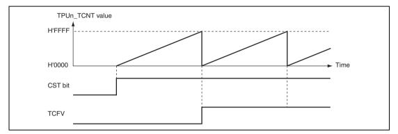
Figure 16.3 Free-Running Counter Operation
