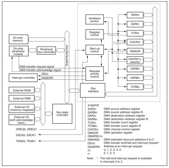
Figure 12.1 Block Diagram of DMAC
