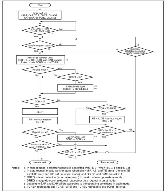
Figure 12.10 DMA Transfer Flowchart
