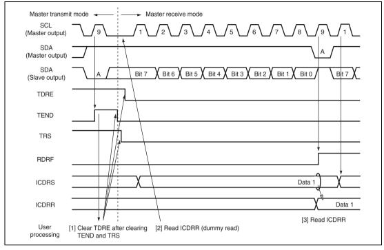
Figure 20.7 Master Receive Mode Operation Timing (1)
