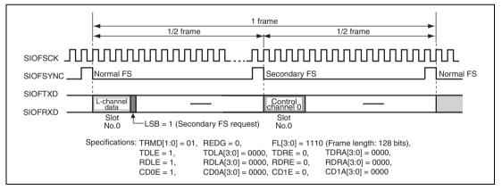
Figure 21.8 Control Data Interface (Secondary FS)
