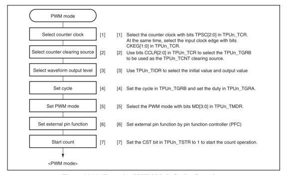
Figure 16.11 Example of PWM Mode Setting Procedure
