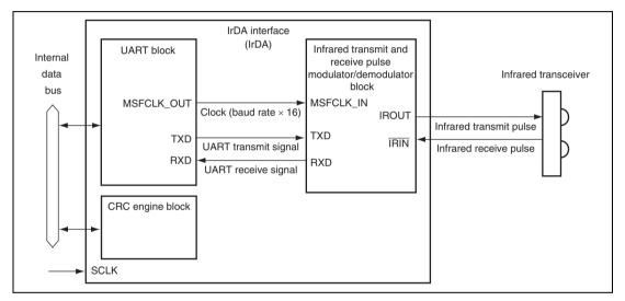
Figure 24.1 Block Diagram of IrDA
