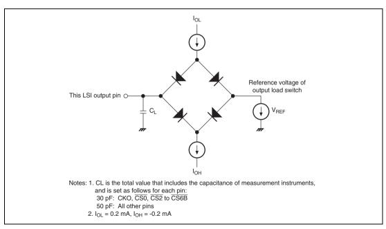
Figure 33.59 Output Load Circuit
