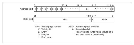
Figure 7.22 Memory-Mapped UTLB Address Array
