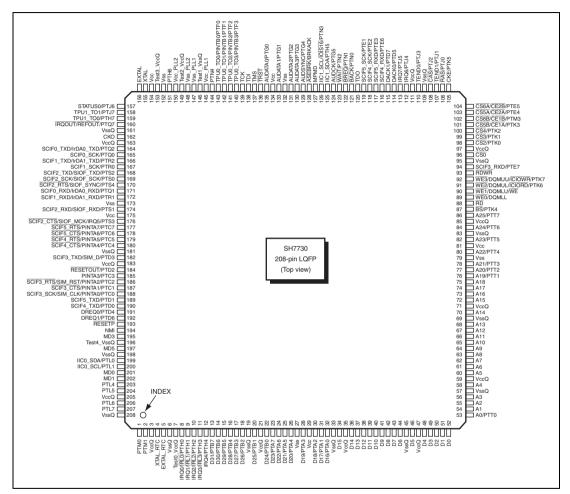
Figure 1.2 Pin Assignments (208-Pin LQFP)
