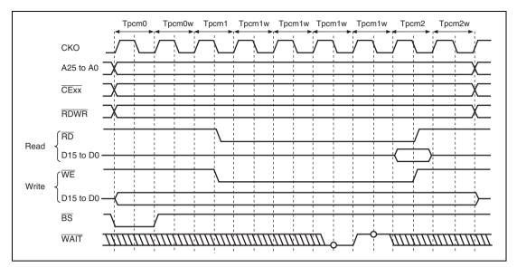
Figure 11.37 Wait Timing for PCMCIA Memory Card Interface (TED[3:0] = B'0010, TEH[3:0] = B'0001, Software Wait = 1, Hardware Wait = 1)
