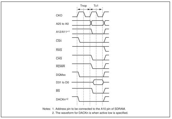
Figure 11.23 Single Write Timing (Bank Active, Same Row Address)
