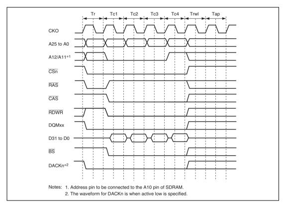
Figure 11.17 Basic Timing for Burst Write (Auto-Precharge)
