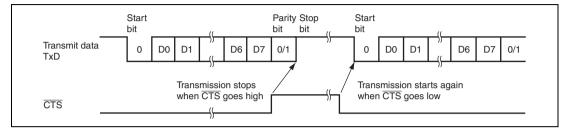
Figure 23.10 Example of CTS Control Operation
