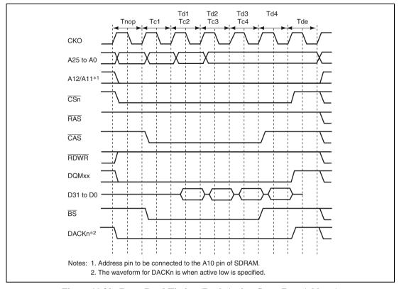
Figure 11.20 Burst Read Timing (Bank Active, Same Row Address)
