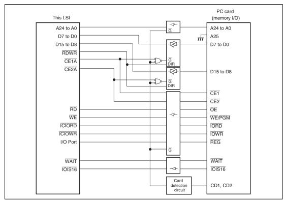
Figure 11.35 Example of PCMCIA Interface Connection
