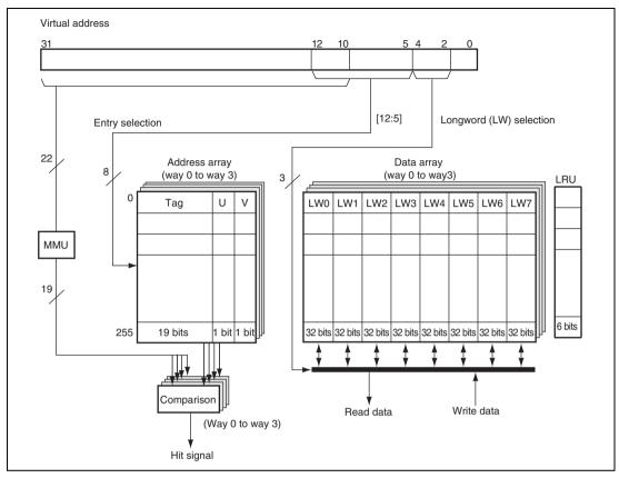
Figure 8.1 Configuration of Operand Cache
