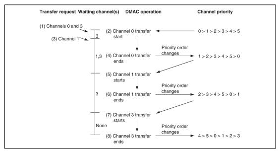
Figure 12.3 Changes in Channel Priority in Round-Robin Mode
