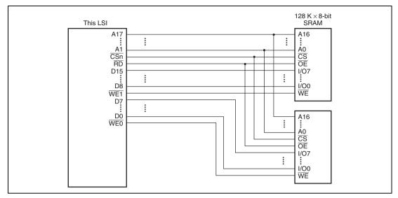
Figure 11.7 Example of 16-Bit Data-Width SRAM Connection
