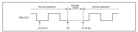
Figure 25.11 Procedure for Stopping Clock and Restarting
