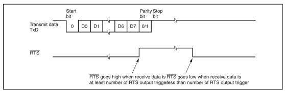
Figure 23.11 Example of RTS Control Operation
