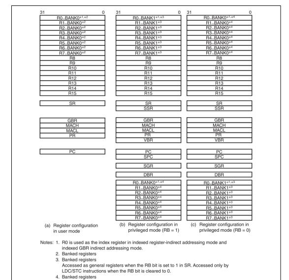
Figure 2.2 CPU Register Configuration in Each Processing Mode
