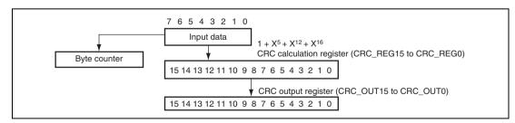
Figure 24.8 CRC Engine Operation
