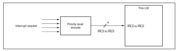
Figure 10.2 Example of IRL Interrupt Connection
