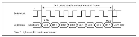
Figure 22.11 Data Format in Clock Synchronous Communication
