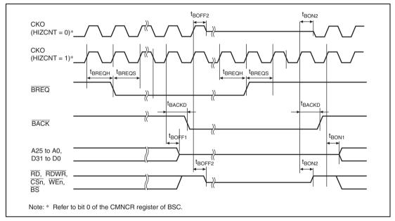
Figure 33.6 Bus Release Timing
