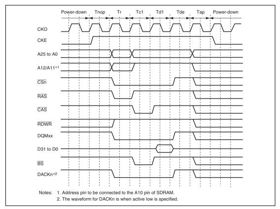
Figure 11.27 Access Timing in Power-Down Mode
