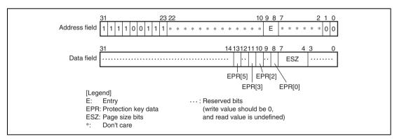
Figure 7.21 Memory-Mapped ITLB Data Array 2 (TLB Extended Mode)
