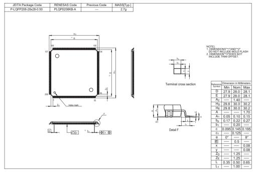
Figure D.1 Package Dimensions
