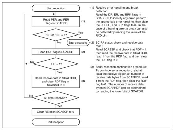
Figure 23.7 Sample Serial Reception Flowchart (1)
