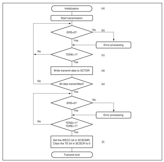
Figure 25.5 Example of Transmit Processing
