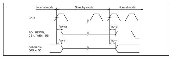
Figure 33.7 Pin Drive Timing at Standby
