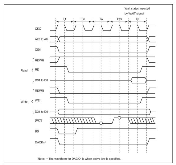
Figure 11.10 Wait State Timing for Normal Space Access (Wait State Insertion using WAIT Signal)
