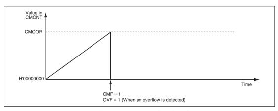
Figure 19.2 Counter Operation (One-Shot Operation)
