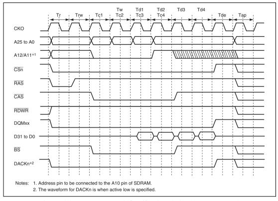
Figure 11.15 Burst Read Wait Specification Timing (Auto-Precharge)
