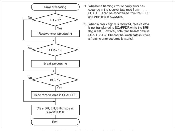
Figure 23.8 Sample Serial Reception Flowchart (2)
