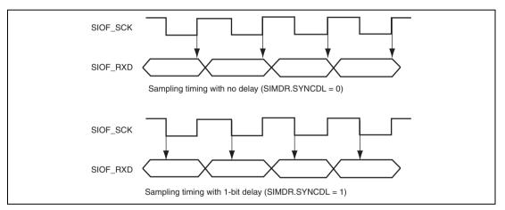
Figure 21.21 Timing of Sampling for Data Reception in Slave Mode
