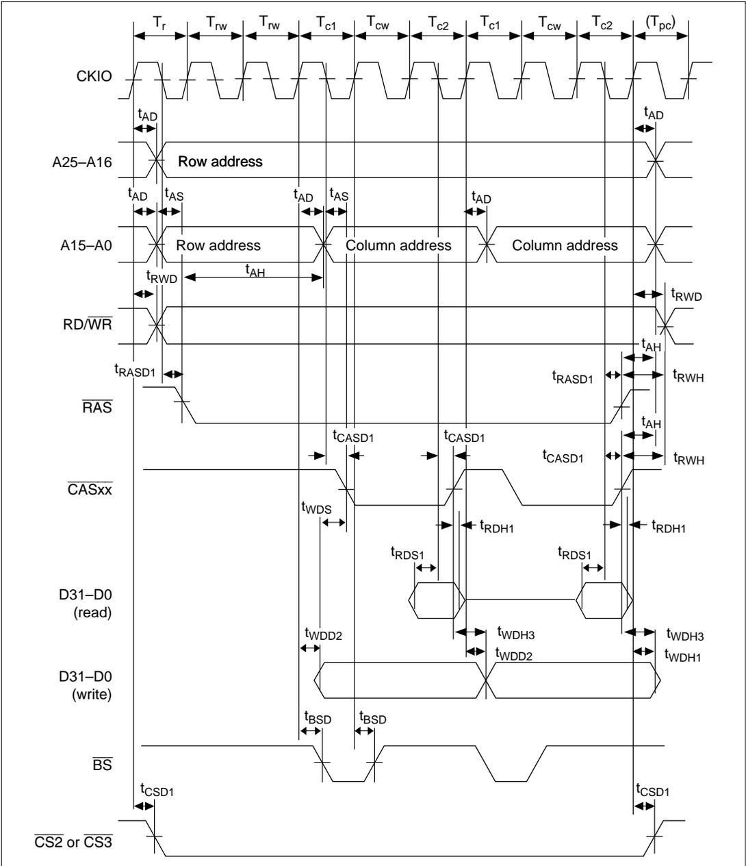
Figure 16.26 DRAM Burst Bus Cycle (RCD = 2, AnW = 2, TPC = 0)
