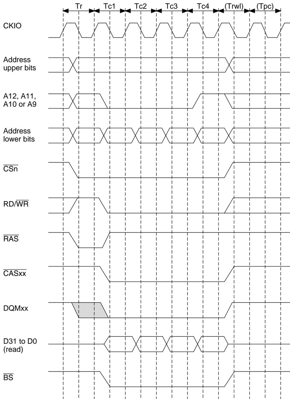
**Figure 10.27 Basic Timing for Synchronous DRAM Burst Write**
