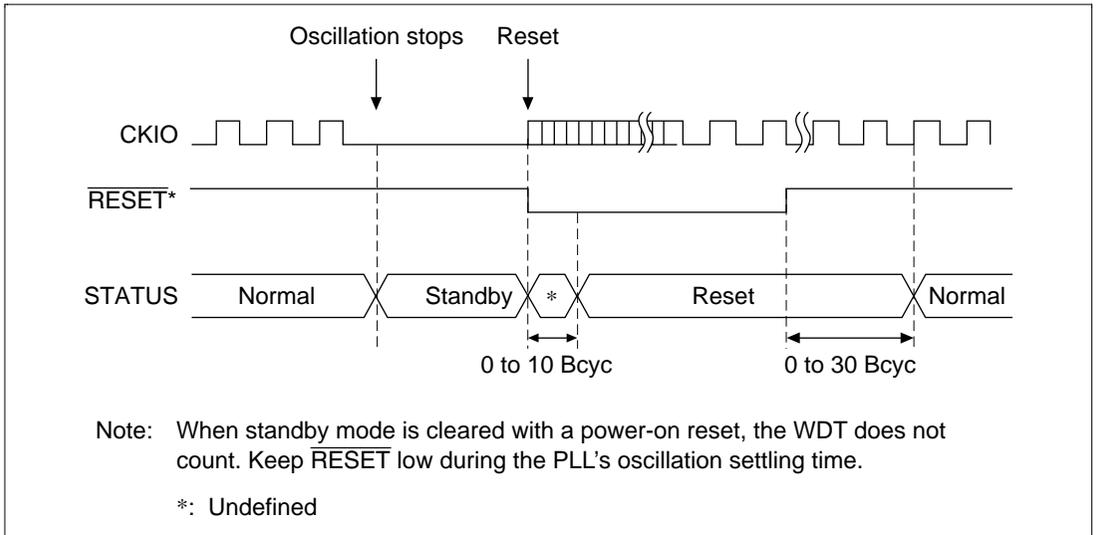
Figure 8.5 Standby to Power-On Reset STATUS Output
