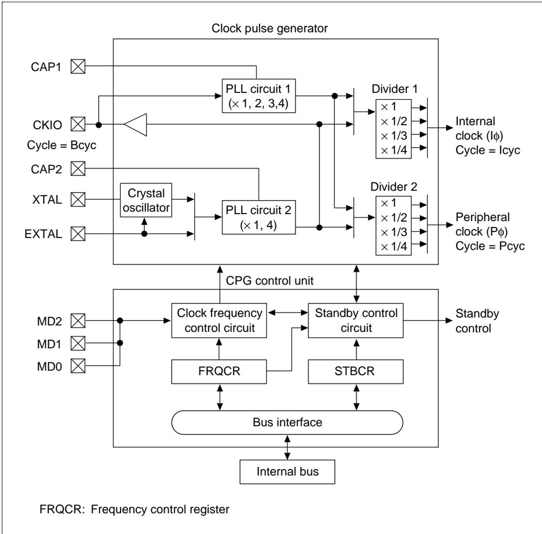
**Figure 9.2 Block Diagram of Clock Pulse Generator(SH7708R)**
