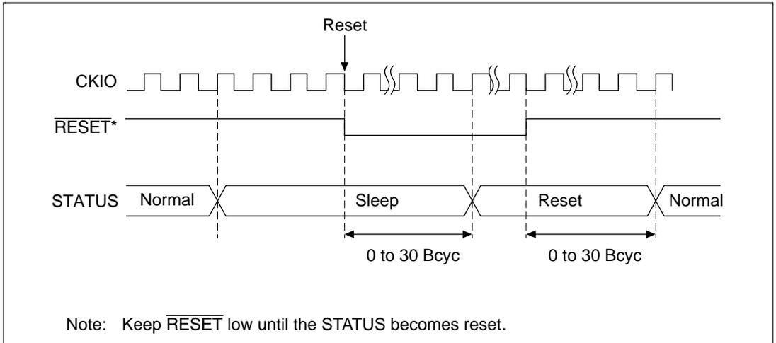
**Figure 8.9 Sleep to Manual Reset STATUS Output**
