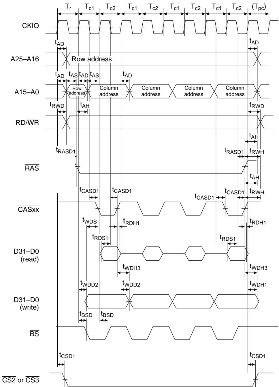
Figure 17.25 DRAM Burst Bus Cycle (RCD = 0, AnW = 1, TPC = 0)
