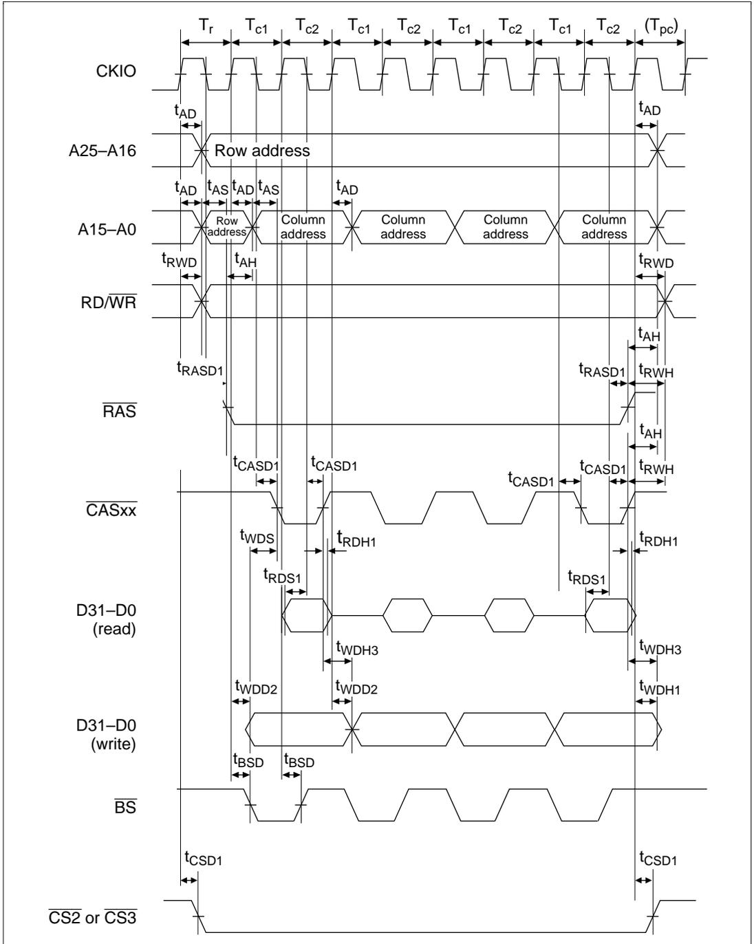
Figure 16.25 DRAM Burst Bus Cycle (RCD = 0, AnW = 1, TPC = 0)
