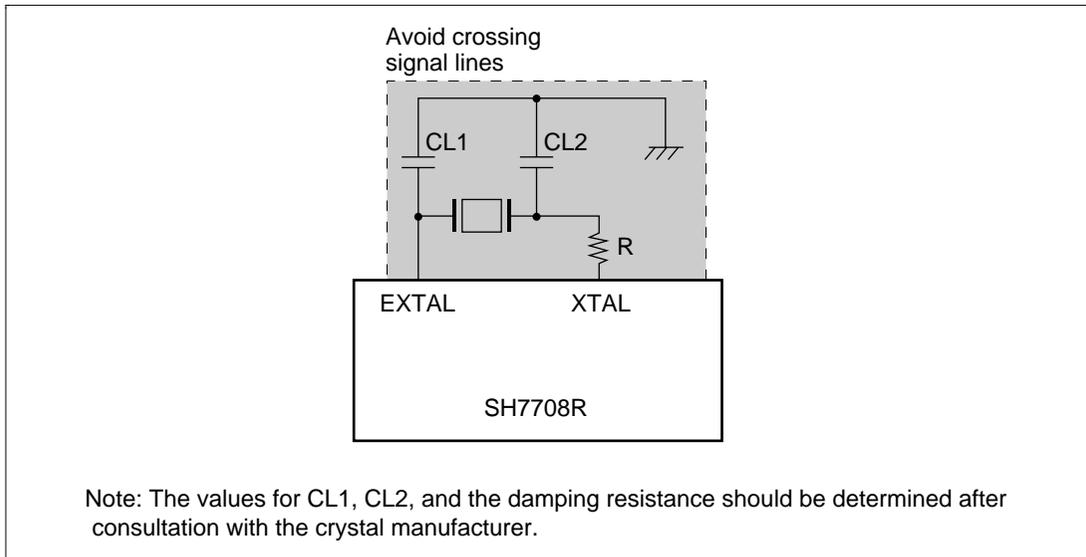
**Figure 9.8 Points for Attention when Using Crystal Resonator**
