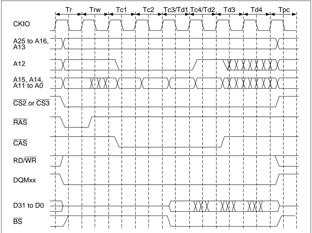
**Figure 10.25 Synchronous DRAM Burst Read Wait Specification Timing**
