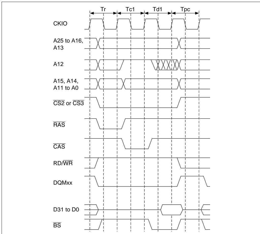
**Figure 10.26 Basic Timing for Synchronous DRAM Single Read**
