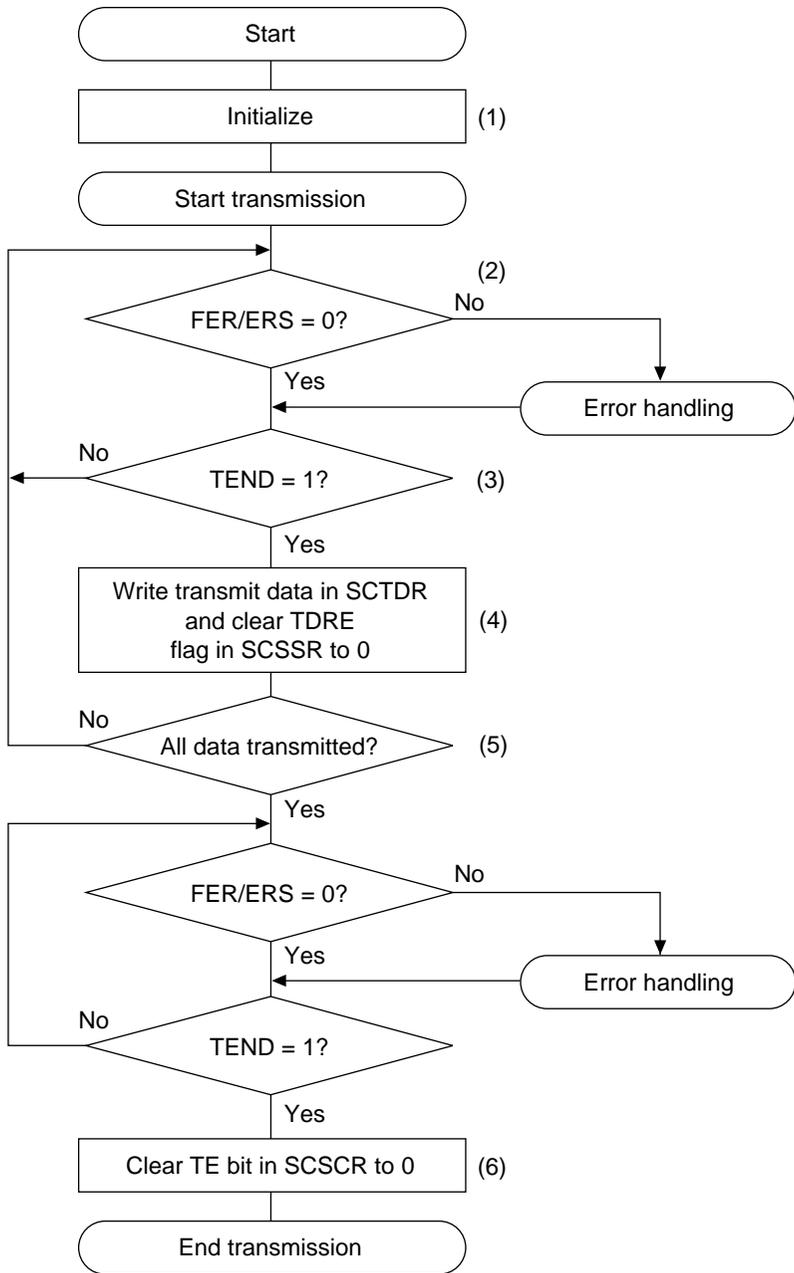
Figure 14.6 Transmission Flowchart
