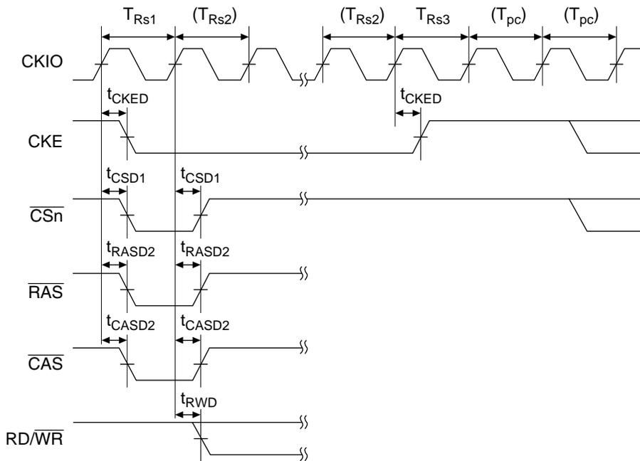
**Figure 17.43 Synchronous DRAM Self-Refresh Cycle ( $TPC = 0$ )**
