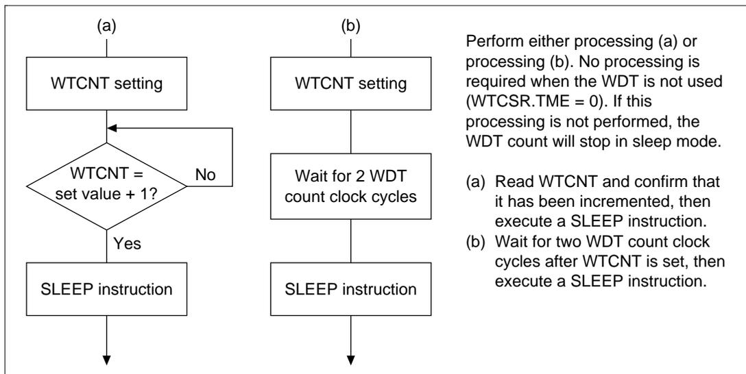
**Figure 9.6 To Operate the WDT in Sleep Mode**
