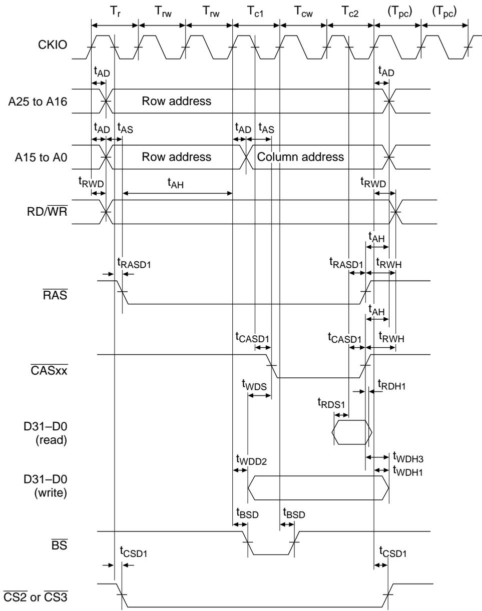
Figure 17.24 DRAM Bus Cycle (RCD = 2, AnW = 2, TPC = 1)
