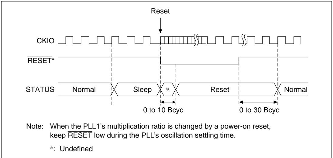
**Figure 8.8 Sleep to Power-On Reset STATUS Output**
