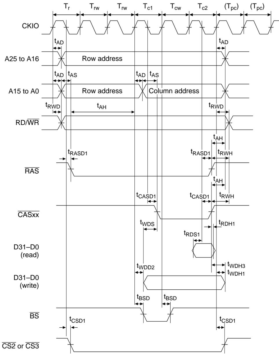
Figure 16.24 DRAM Bus Cycle (RCD = 2, AnW = 2, TPC = 1)
