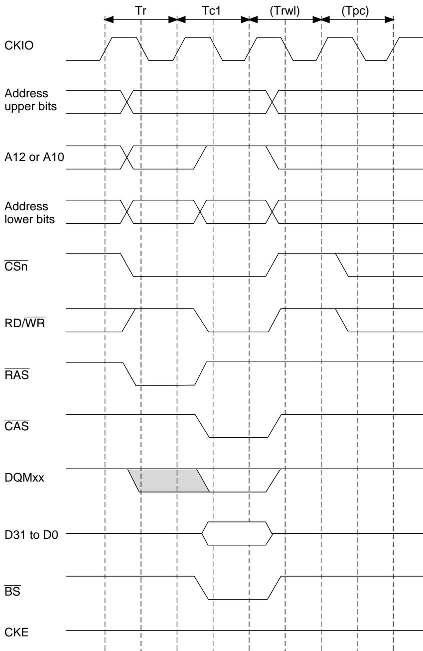
Figure 10.28 Basic Timing for Synchronous DRAM Single Write
