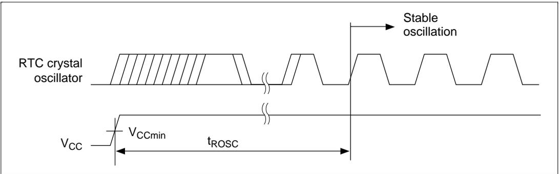
**Figure 16.61 RTC Crystal Oscillator Power-On Oscillation Settling Time**
