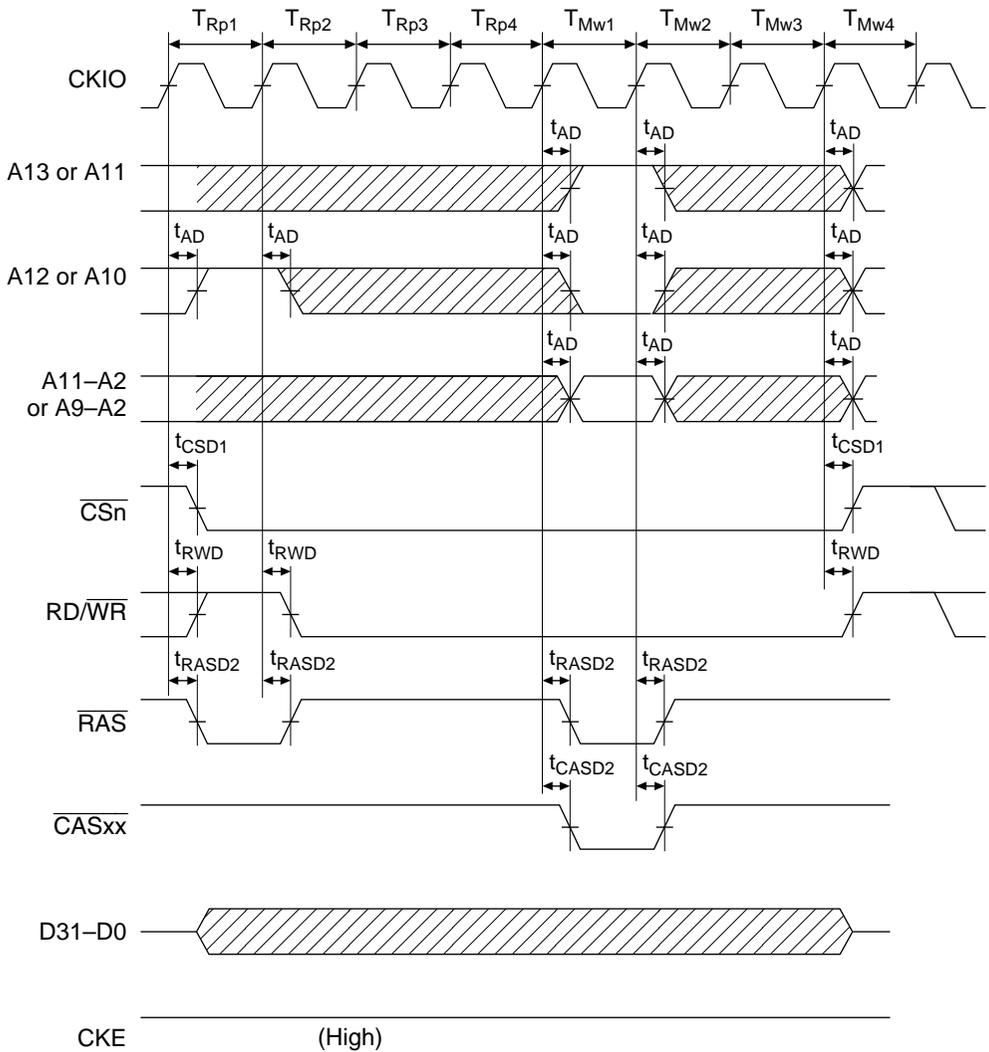
**Figure 17.44 Synchronous DRAM Mode Register Write Cycle**
