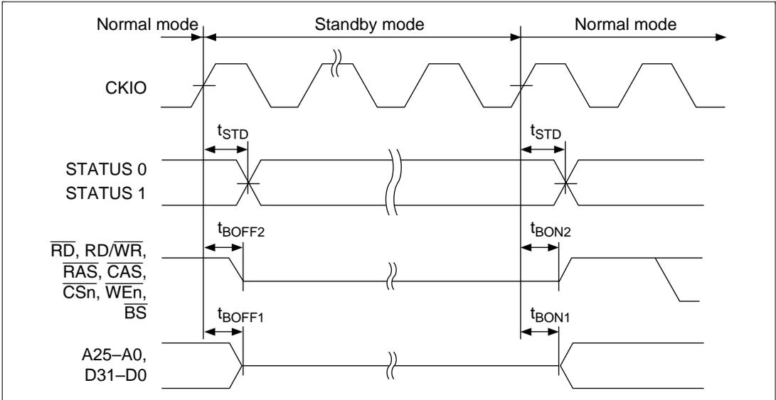
**Figure 17.16 Pin Drive Timing for Standby Mode**
