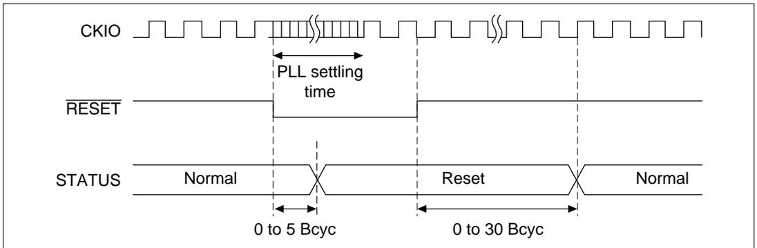
Figure 8.1 Power-On Reset (Clock Mode 0, 1, 2, and 7) STATUS Output
