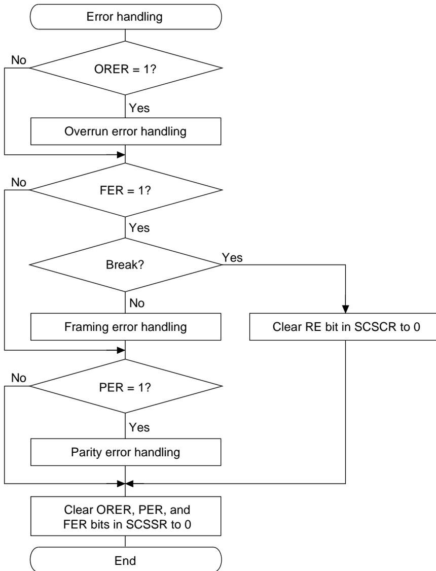
**Figure 13.7 Sample Flowchart for Receiving Serial Data (cont)**
