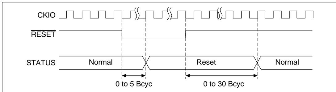
**Figure 8.2 Power-On Reset (Clock Mode 3 and 4) STATUS Output**
