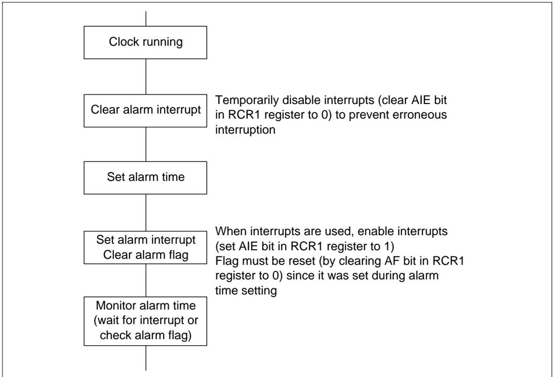
**Figure 12.4 Using the Alarm Function**
