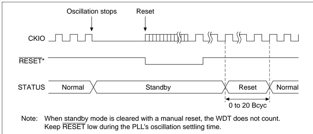
**Figure 8.6 Standby to Manual Reset STATUS Output**
