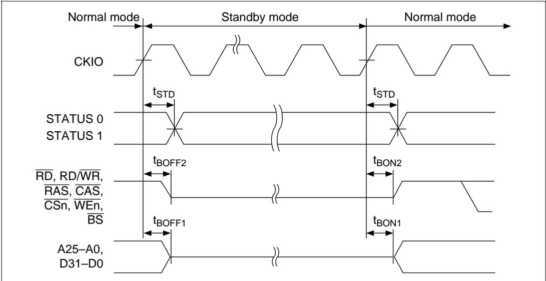
**Figure 16.16 Pin Drive Timing for Standby Mode**
