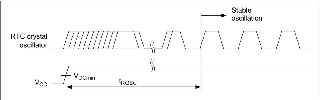
**Figure 17.61 RTC Crystal Oscillator Power-On Oscillation Settling Time**
