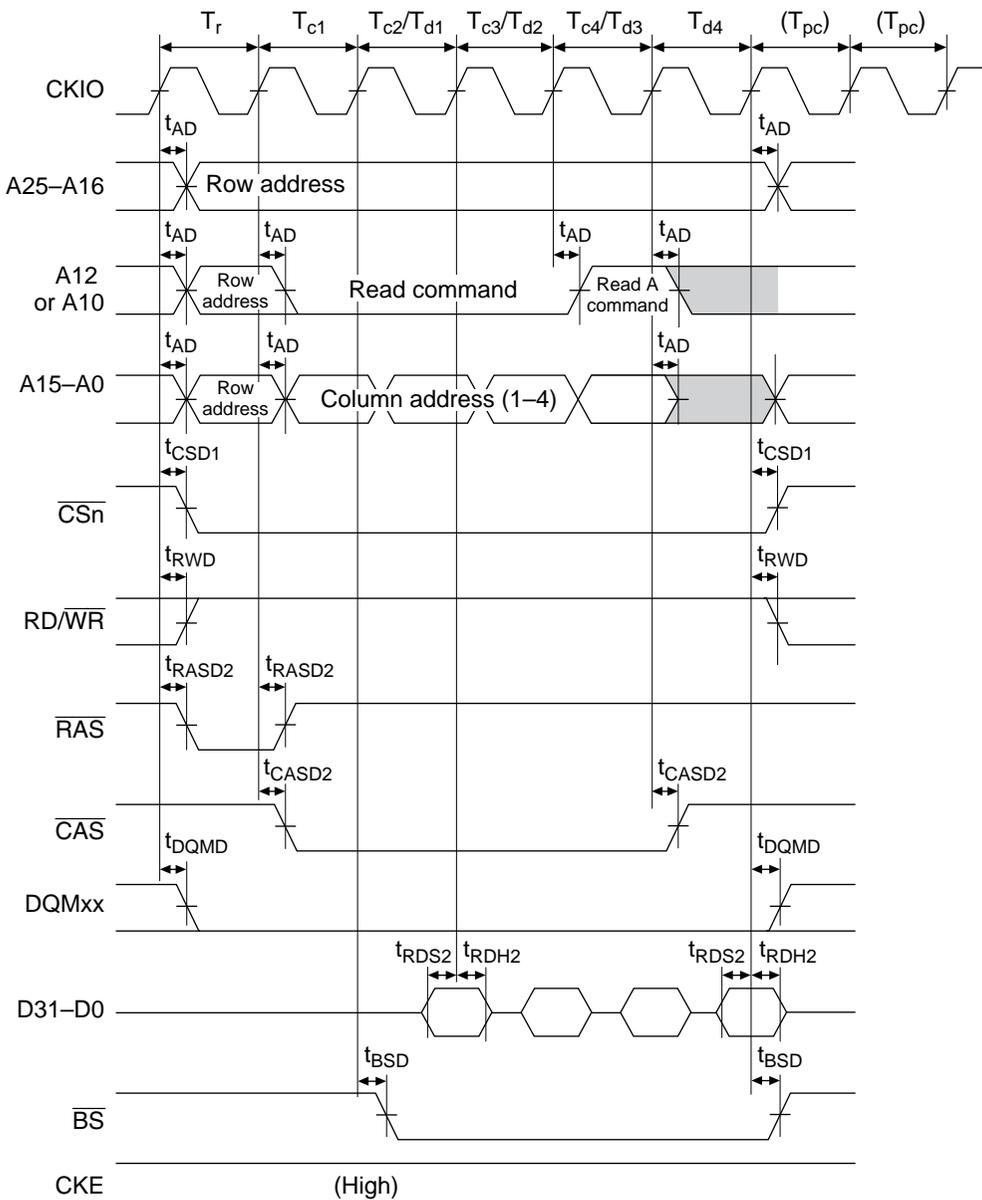
**Figure 16.36 Synchronous DRAM Read Bus Cycle (Burst Read (Single Read × 4), RCD = 0, CAS Latency = 1, TPC = 1)**
