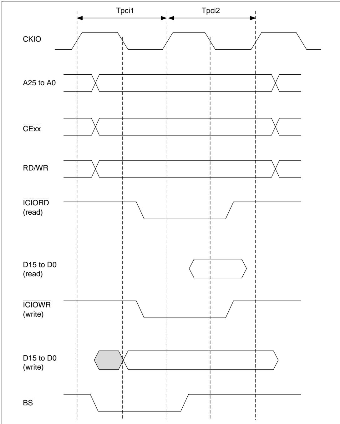
**Figure 10.47 Basic Timing for PCMCIA I/O Card Interface**
