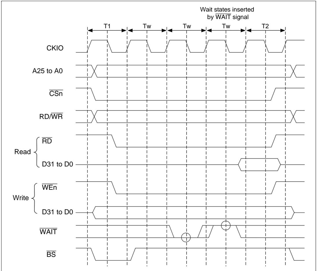
**Figure 10.12 Basic Interface Wait State Timing**
