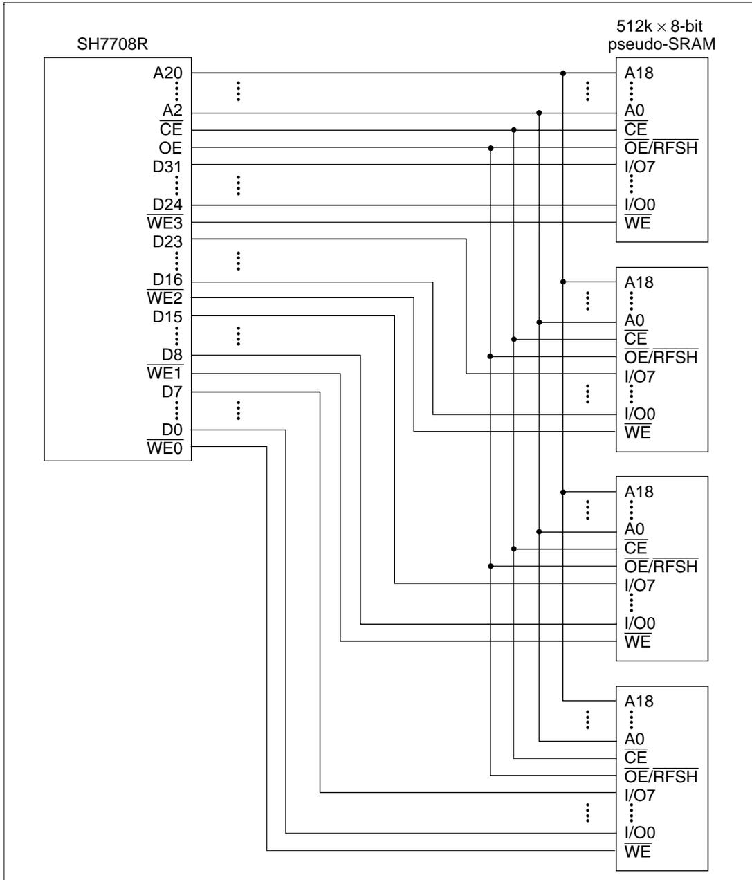
**Figure 10.33 Example of Pseudo-SRAM Connection (4M-Bit Devices)**
