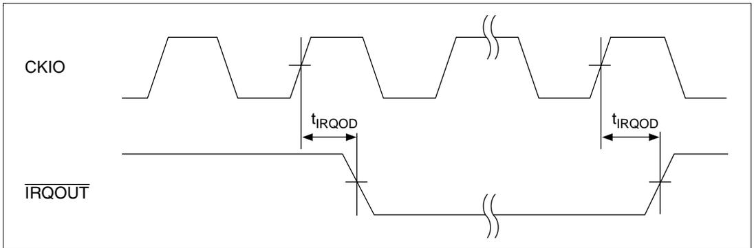
**Figure 17.14  $\overline{IRQOUT}$  Timing**
