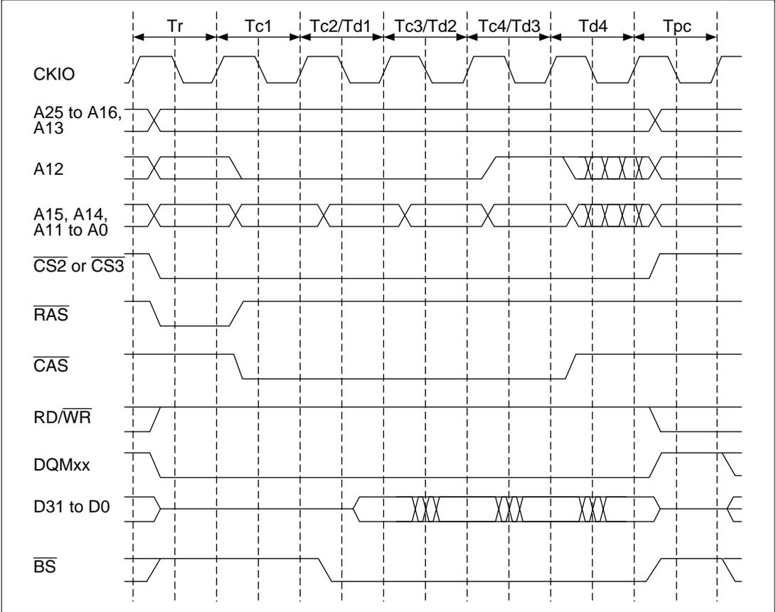
**Figure 10.24 Basic Timing for Synchronous DRAM Burst Read**
