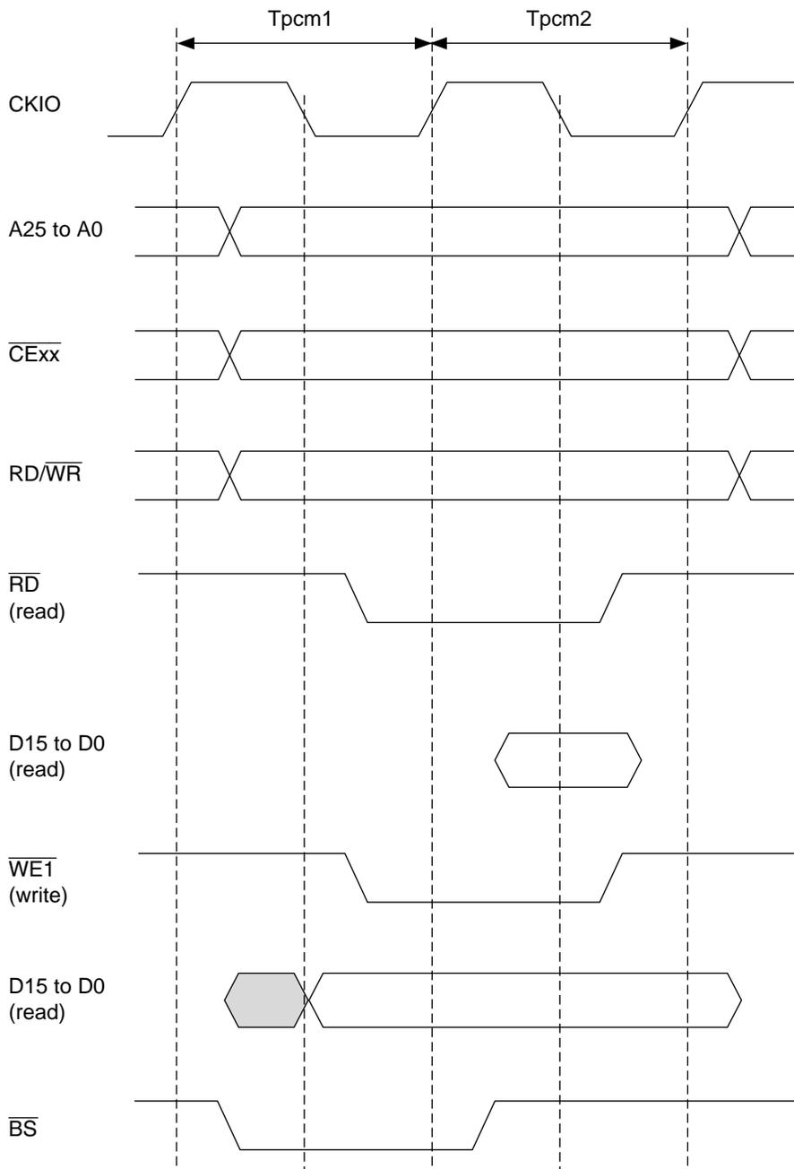
**Figure 10.42 Basic Timing for PCMCIA Memory Card Interface**
