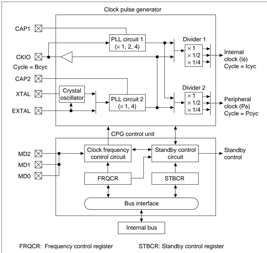
Figure 9.1 Block Diagram of Clock Pulse Generator(SH7708, SH7708S)
