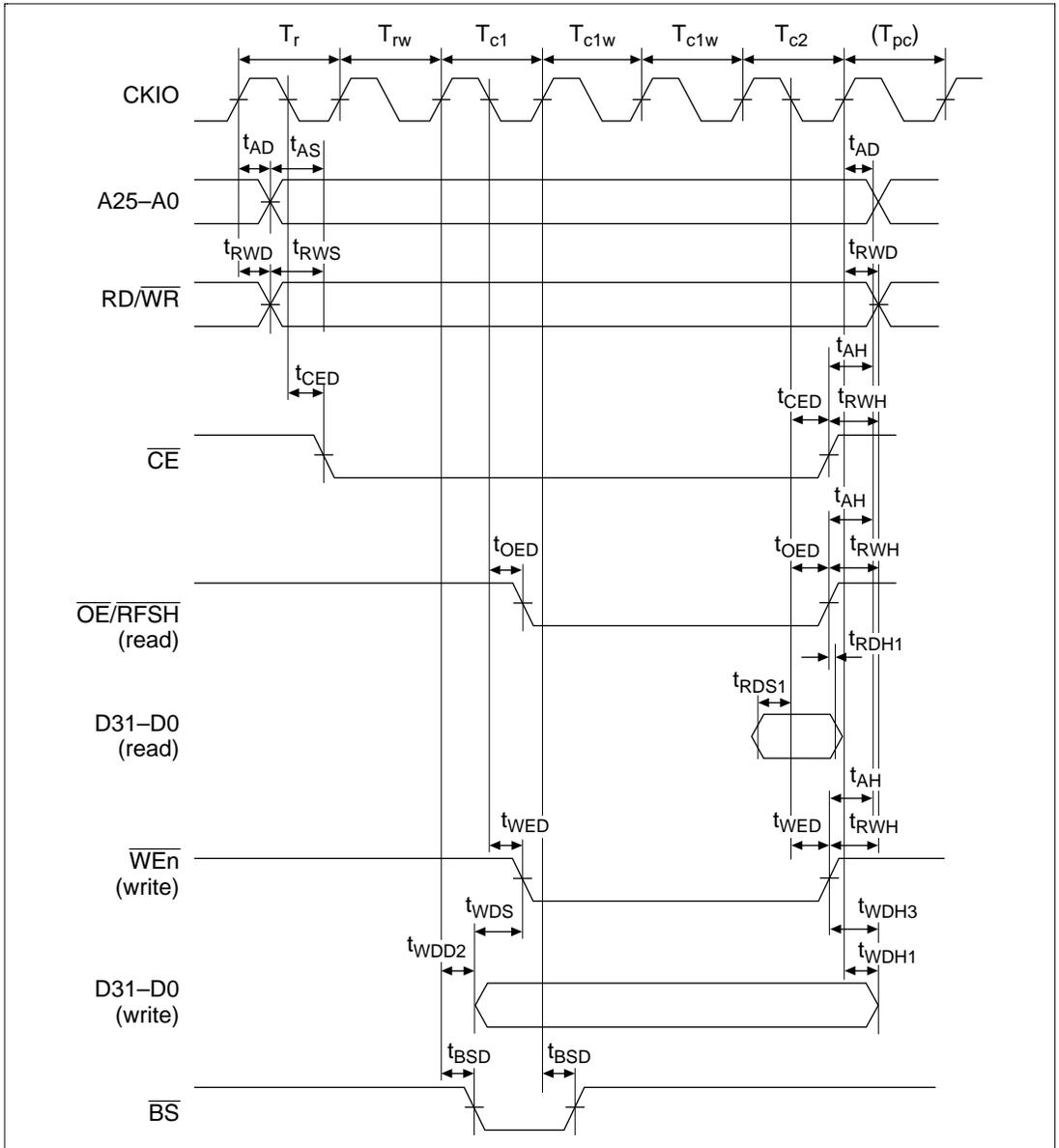
Figure 17.46 Pseudo-SRAM Read Cycle (RCD = 1, A3W = 3, TPC = 0)
