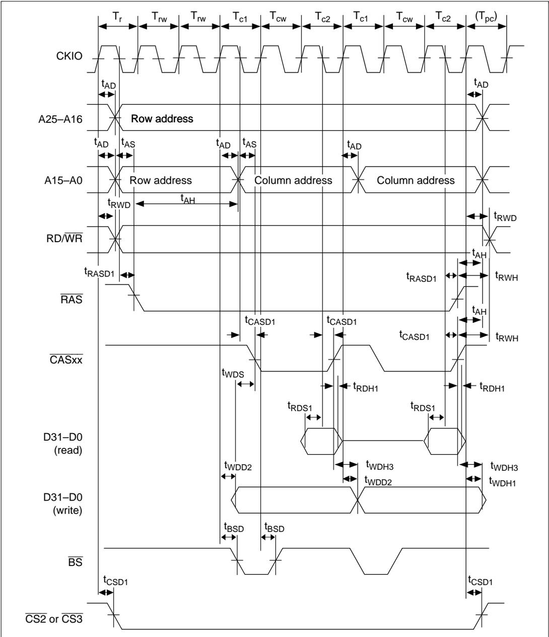
Figure 17.26 DRAM Burst Bus Cycle (RCD = 2, AnW = 2, TPC = 0)
