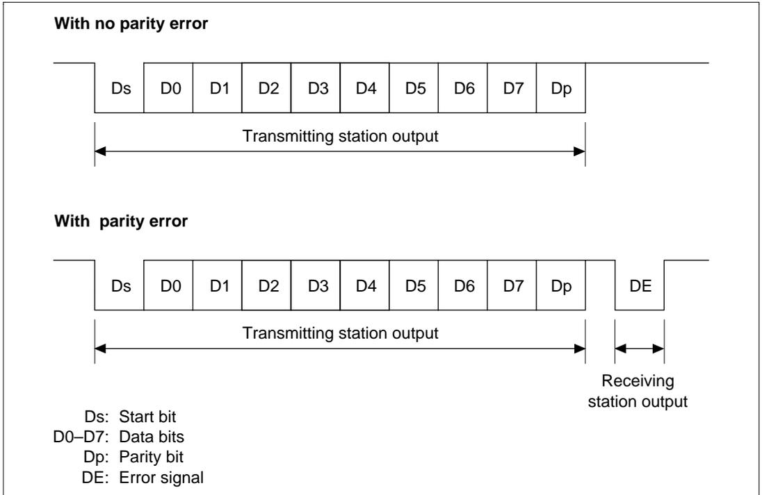
**Figure 14.3 Data Format for Smart Card Interface**
