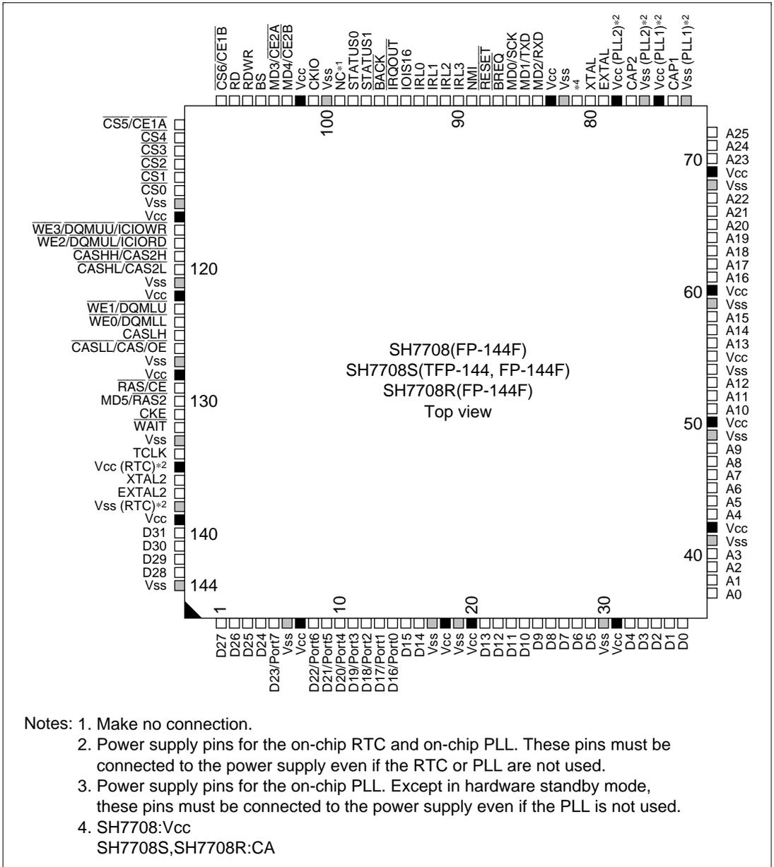
Figure 1.2 Pin Arrangement
