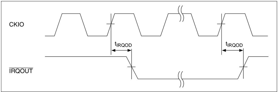
**Figure 16.14  $\overline{IRQOUT}$  Timing**
