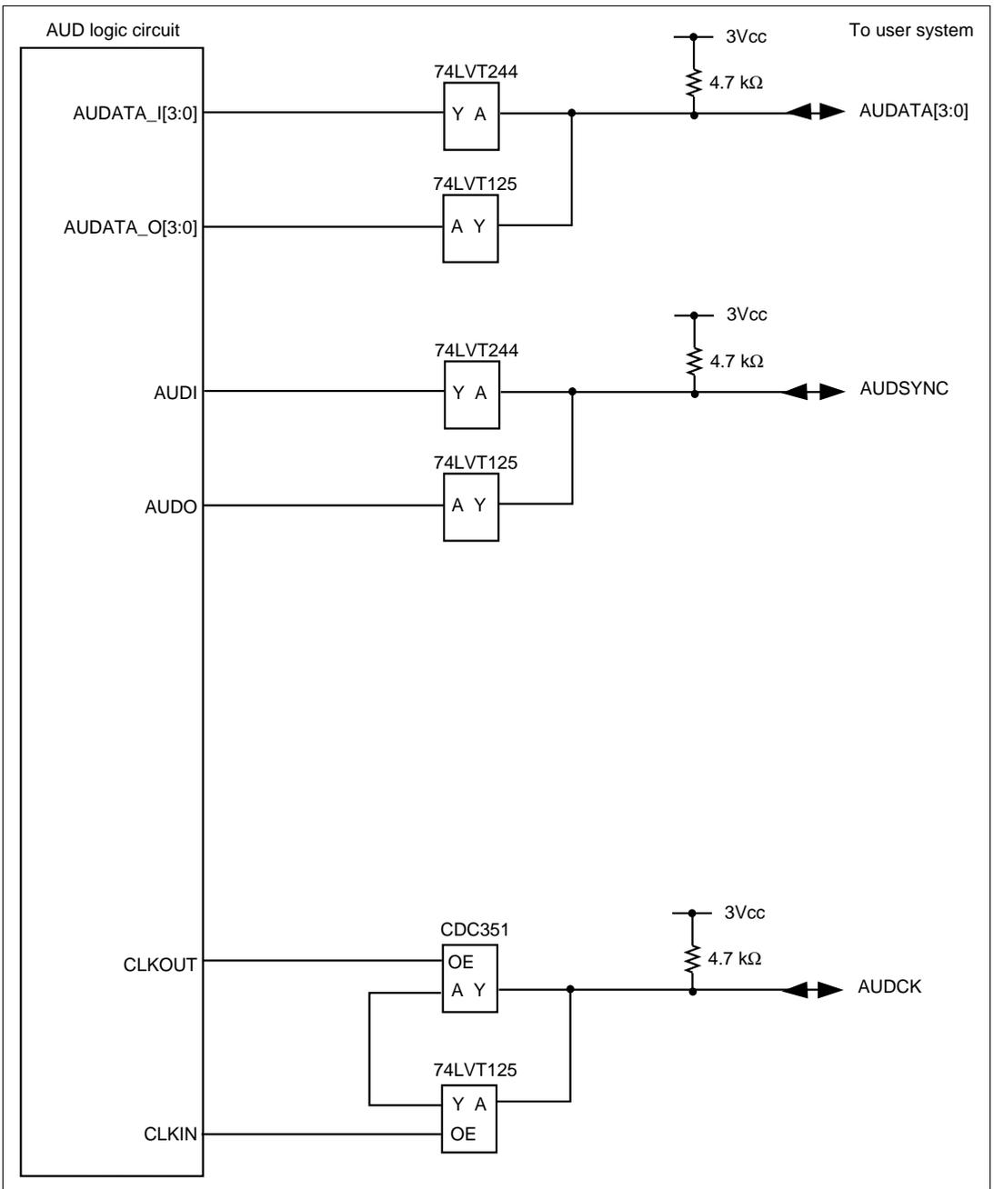
**Figure 6.9** User System Interface Circuit of the AUD Pin in the Emulator (HS7660KCI02H) (Model Name: HS0005KCI04H)
