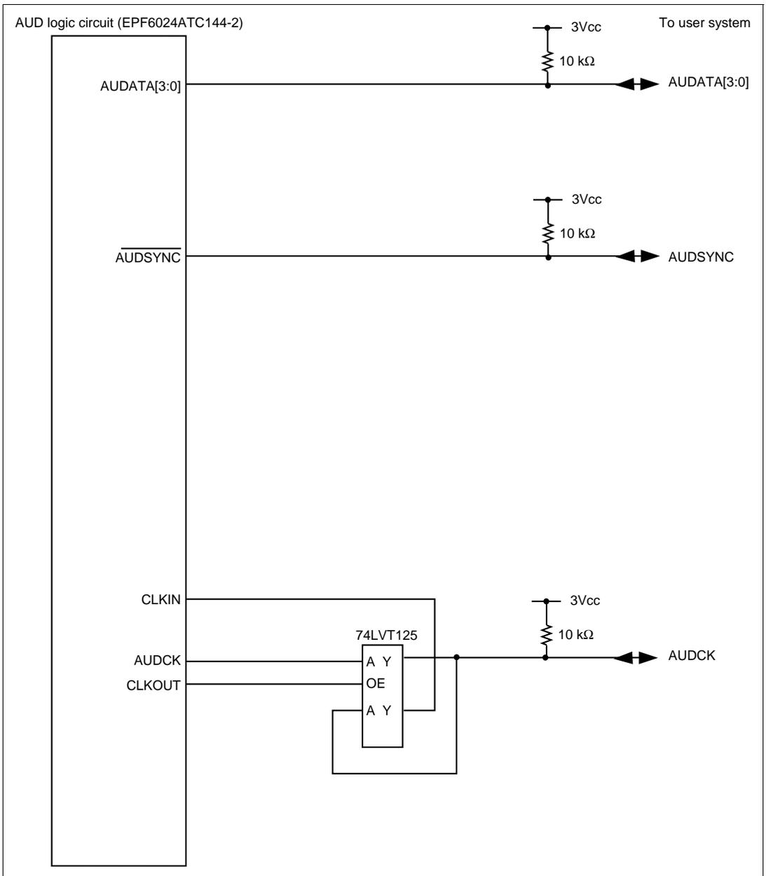
**Figure 6.6 User System Interface Circuit of the AUD Pin in the Emulator (HS7660KCM02H) (Model Name: HS0005KCM04H)**
