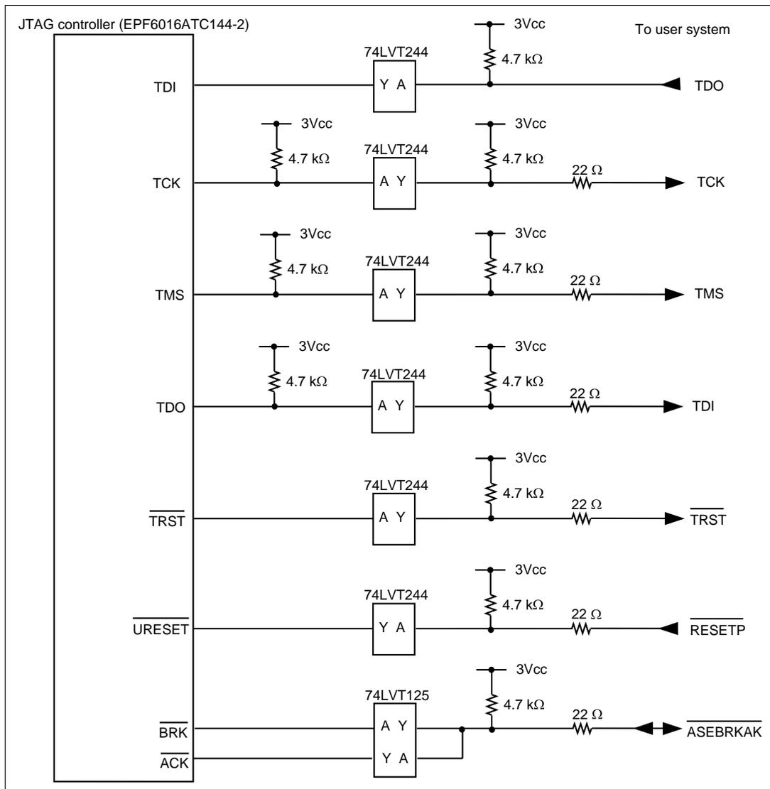
**Figure 6.4 User System Interface Circuit in the Emulator (HS7660KCM01H)
