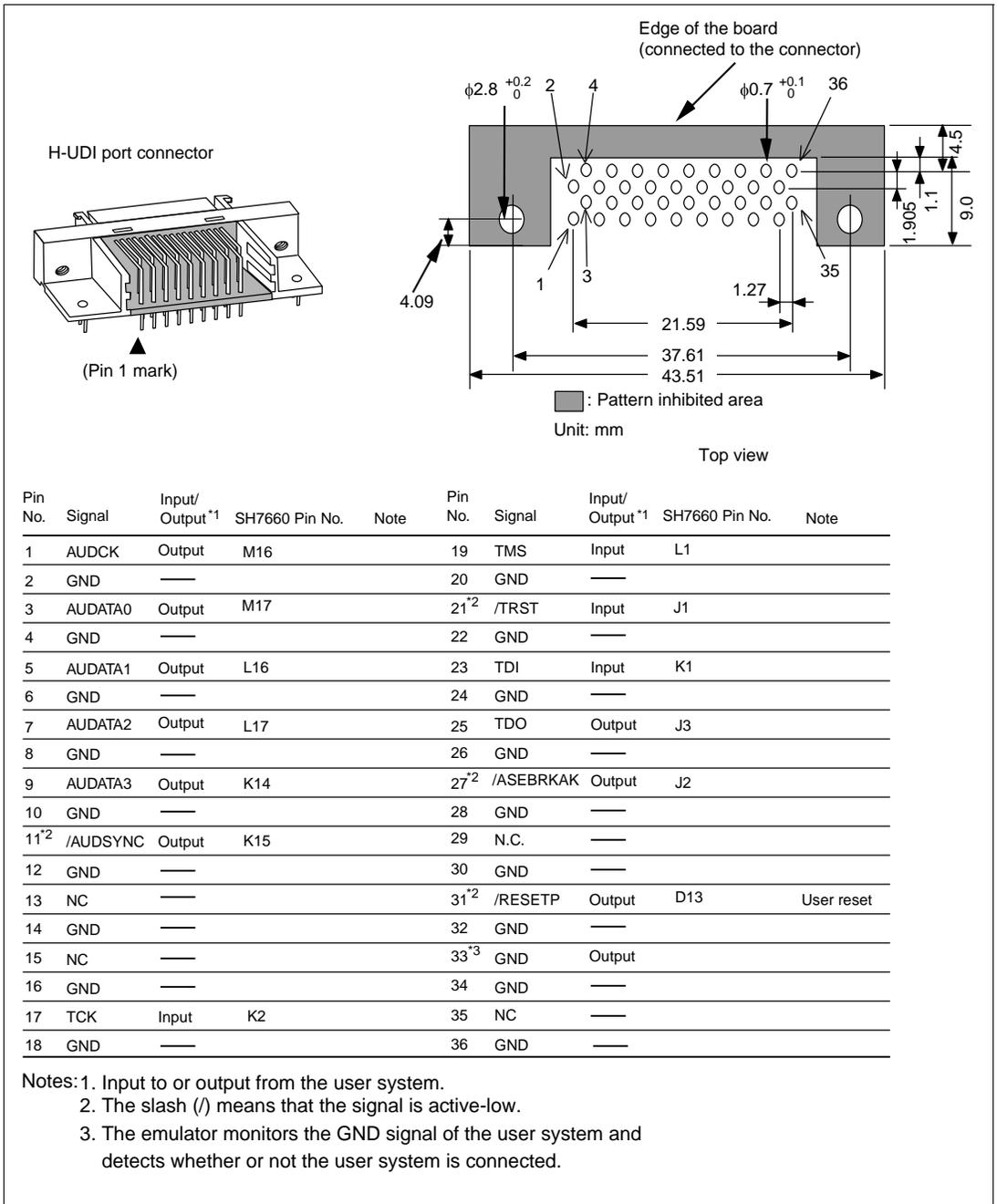
Figure 6.3 Pin Arrangement of the H-UDI Port Connector (36 Pins)
