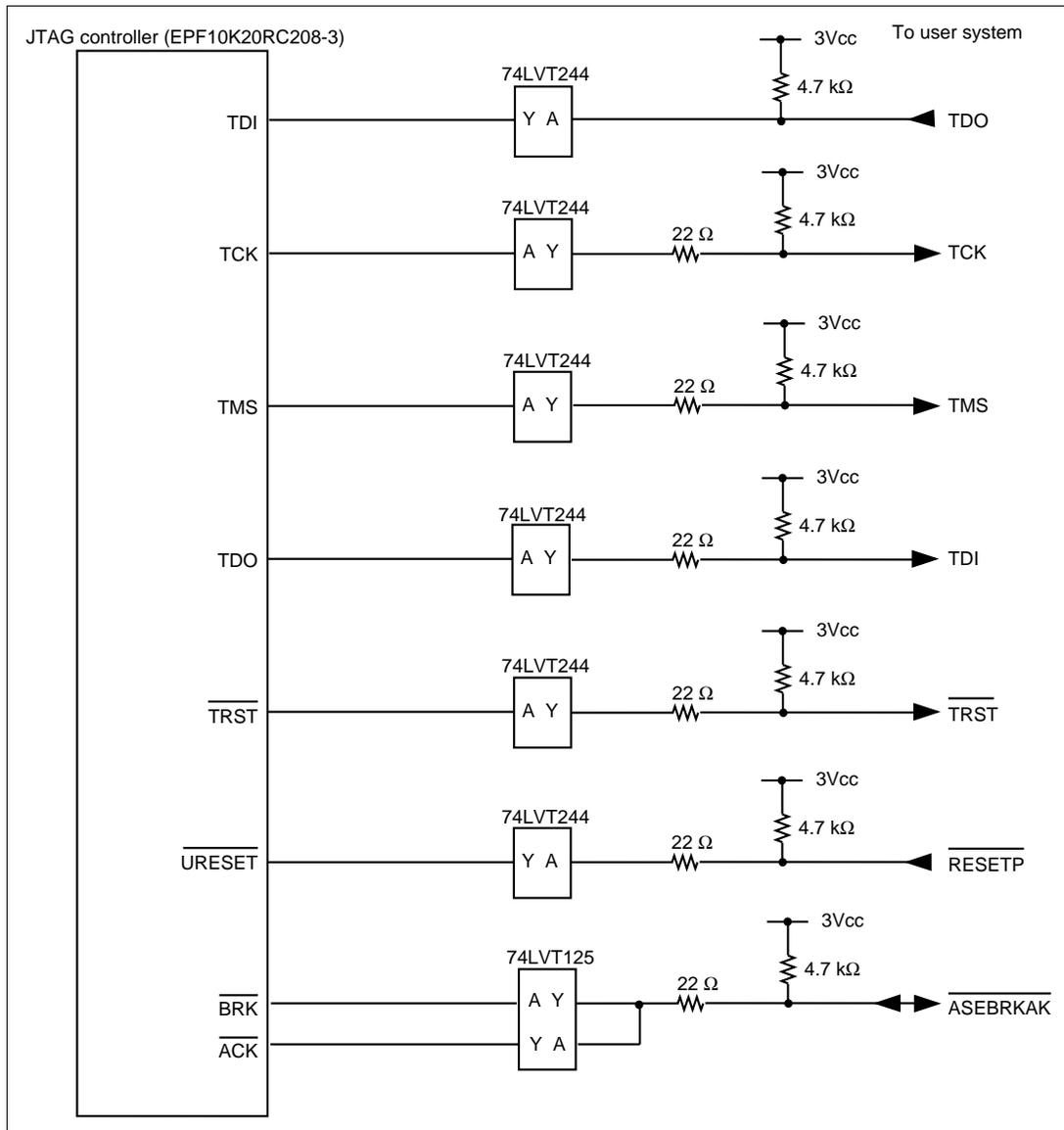
**Figure 6.7 User System Interface Circuit in the Emulator (HS7660KCI01H)
