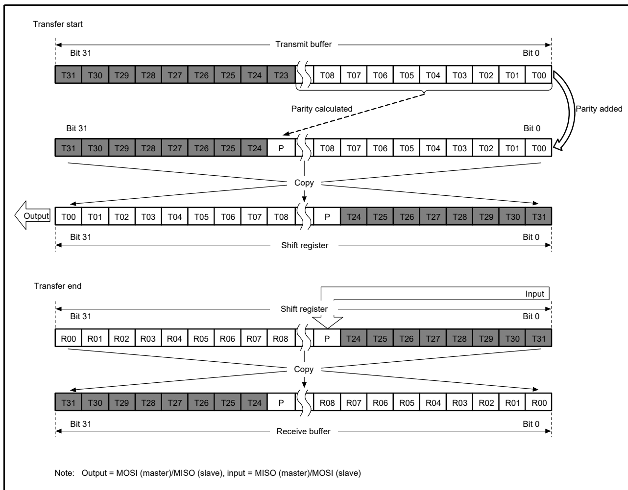
Figure 36.21 LSB-first transfer with 24-bit data and parity enabled
