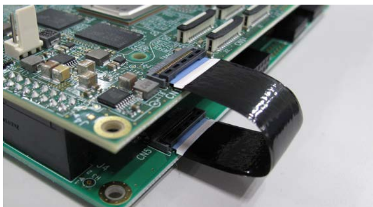
Figure 2.1-2 Connect FFC to RZ/V2H Secure Evaluation Board
