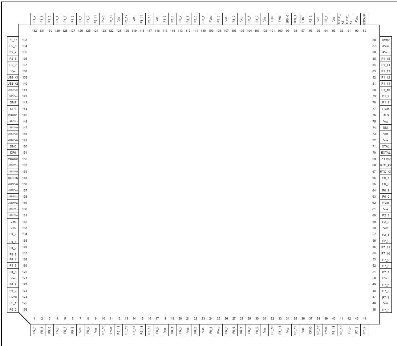
Figure 1.2 Pin Assignment of the 176-pin QFP (Top View)
