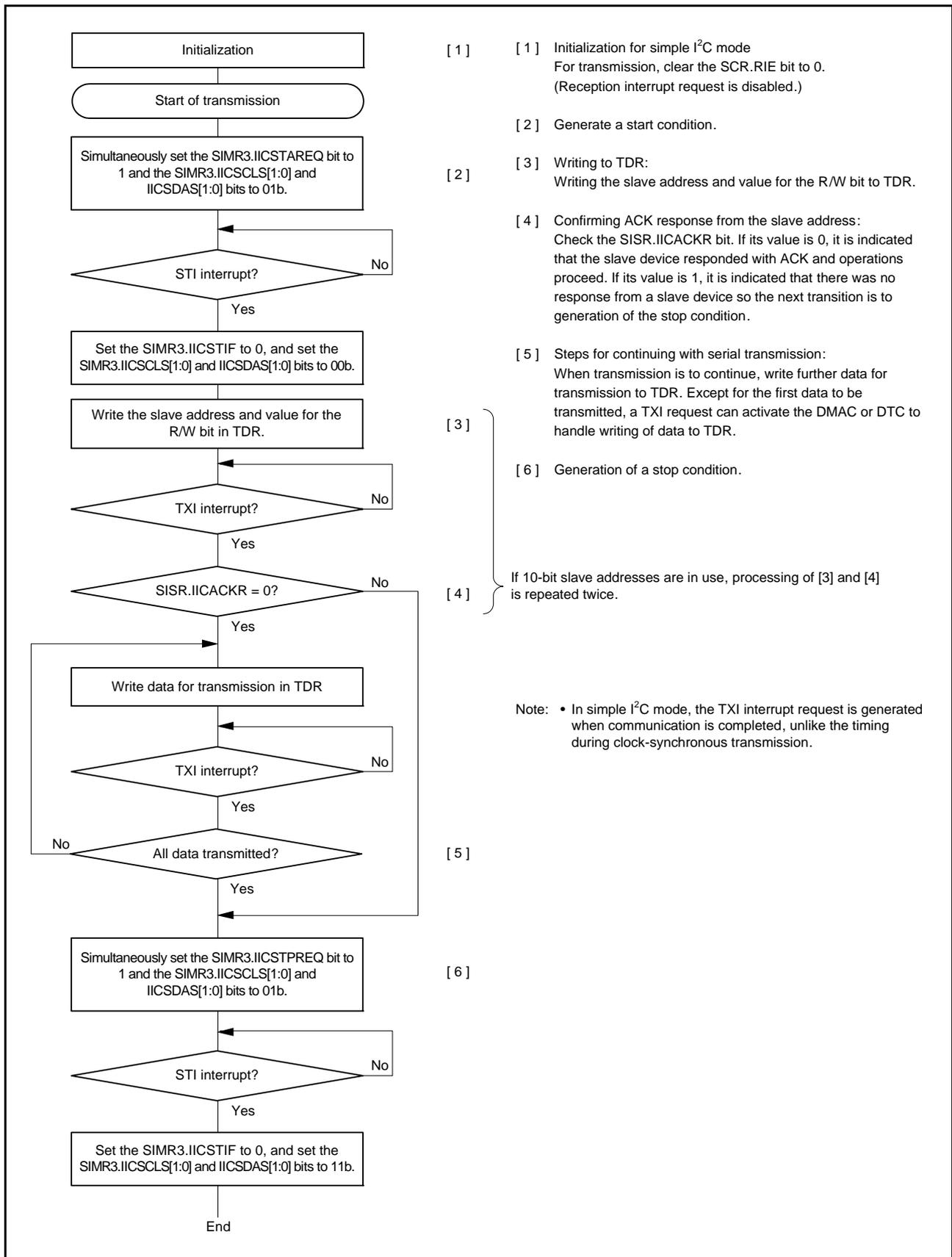
**Figure 27.48 Example of the Procedure for Master Transmission Operations in Simple I<sup>2</sup>C Mode (with Transmission Interrupts and Reception Interrupts in Use)**
