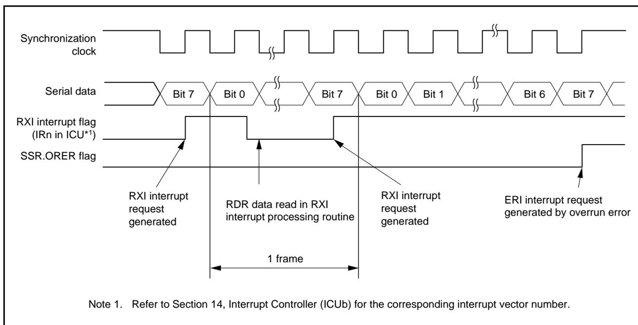
**Figure 27.24 Example of Operation for Serial Reception in Clock Synchronous Mode (1) (when RTS Function is not Used)**
