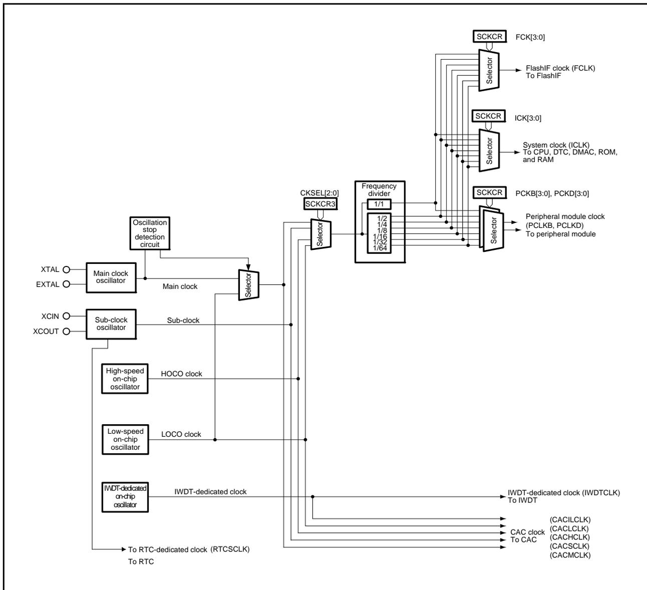
Figure 9.1 Block Diagram of Clock Generation Circuit
