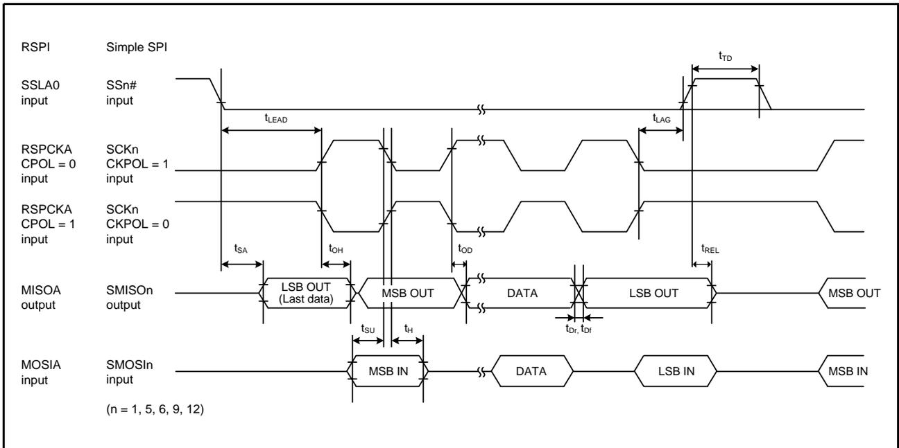
Figure 38.47 RSPI Timing (Slave, CPHA = 1) and Simple SPI Timing (Slave, CKPH = 0)
