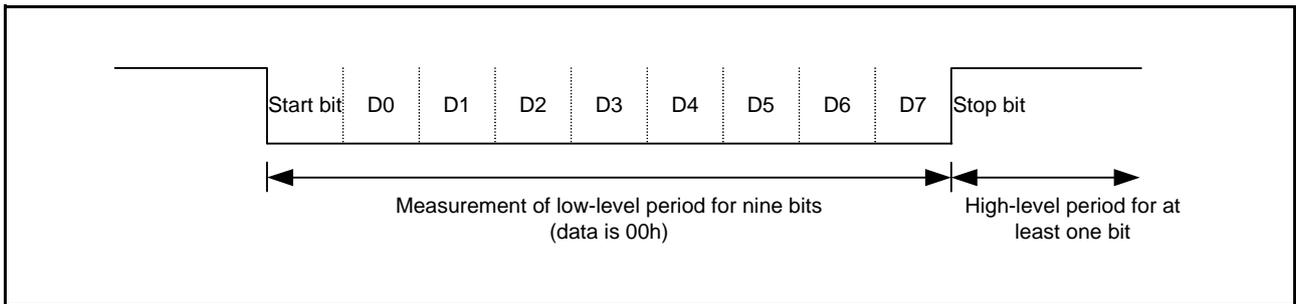
Figure 36.23 Transfer Format Used by SCI in Automatic Adjustment of Bit Rate
