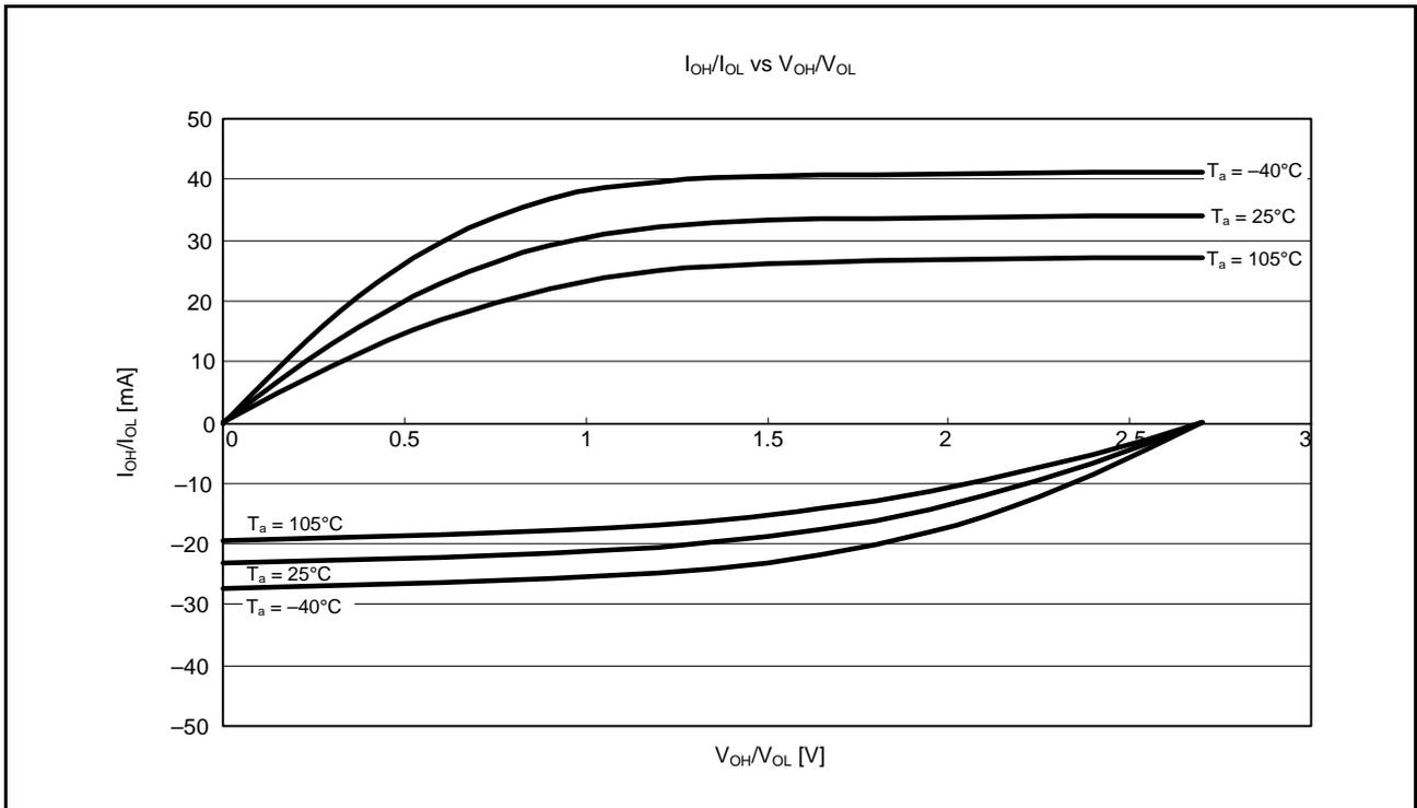
Figure 38.14  $V_{OH}/V_{OL}$  and  $I_{OH}/I_{OL}$  Temperature Characteristics at  $V_{CC} = 2.7$  V when High-Drive Output is Selected (Reference Data)
