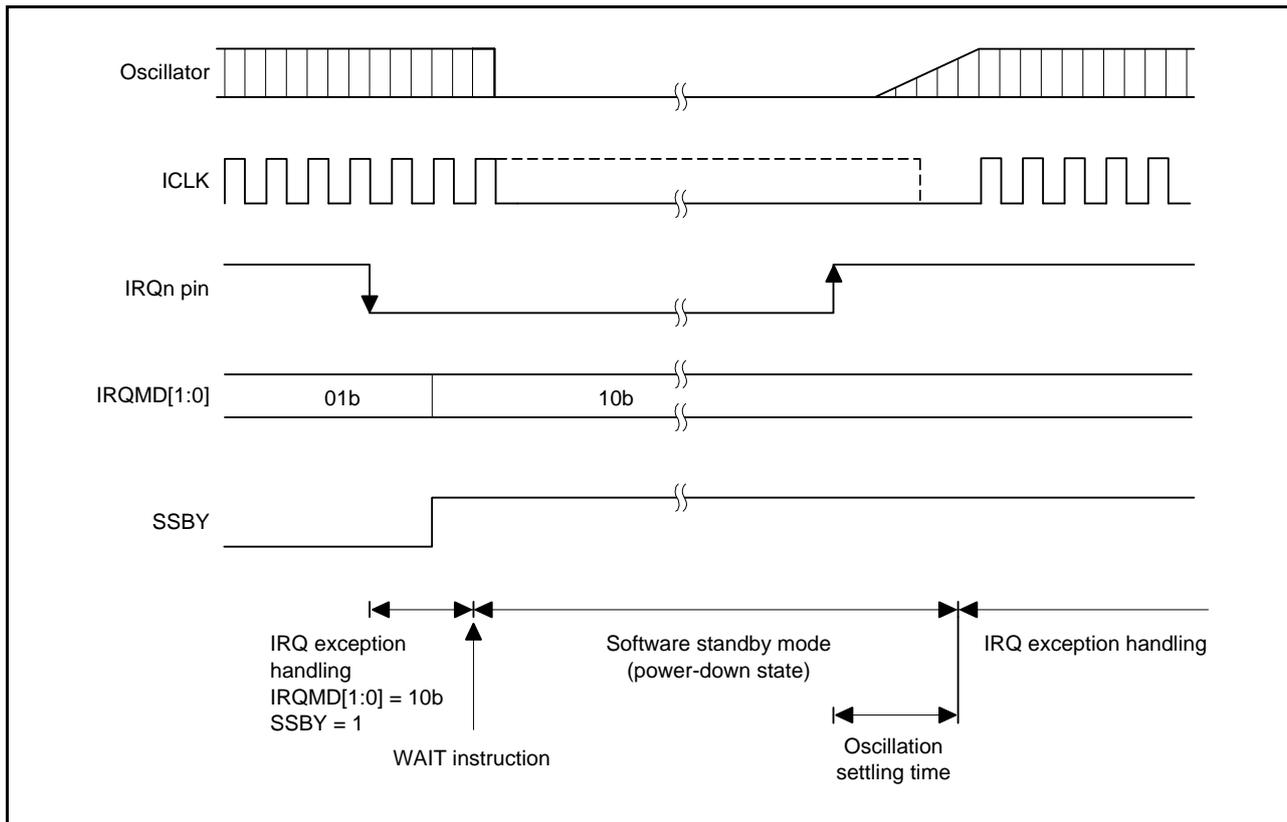
Figure 11.5 Example of Software Standby Mode Application
