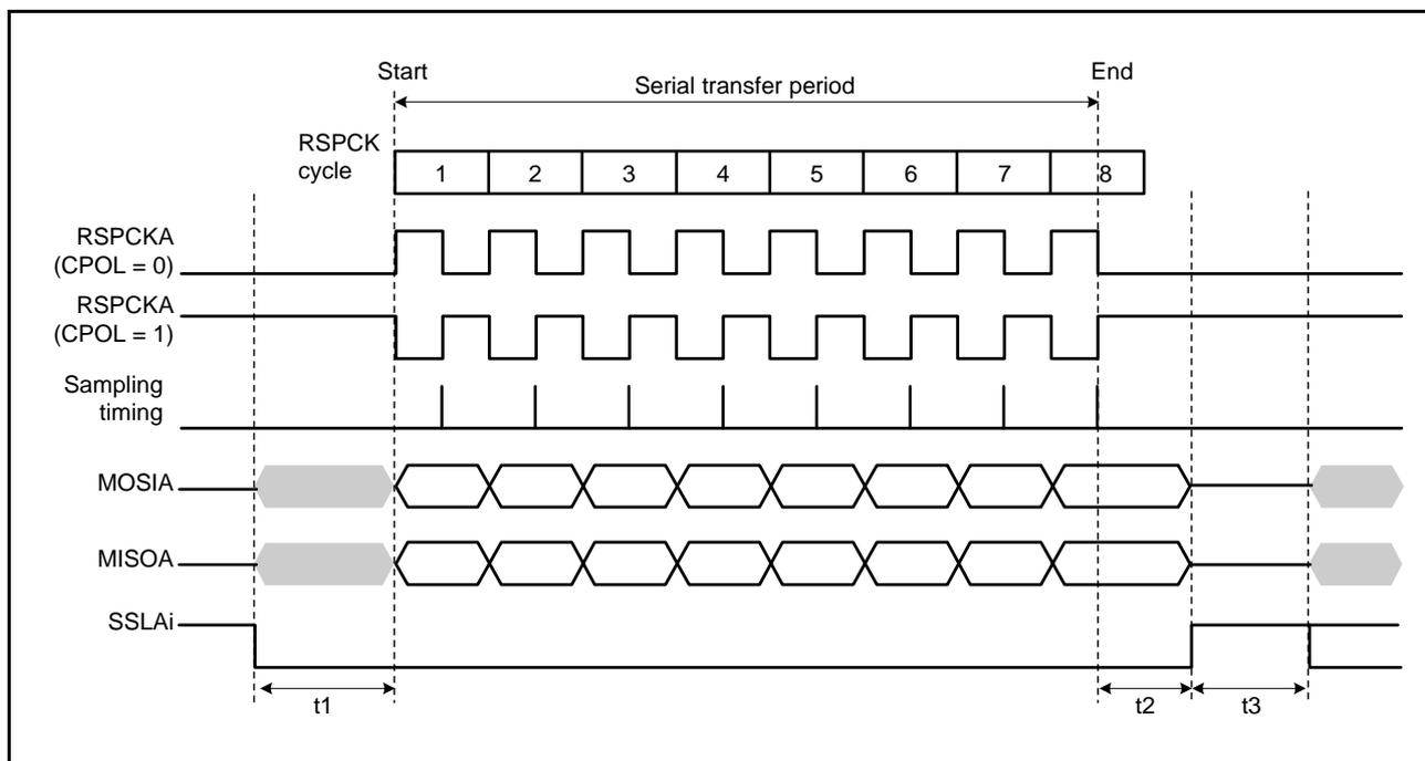
Figure 30.24 RSPI Transfer Format (CPHA = 1)
