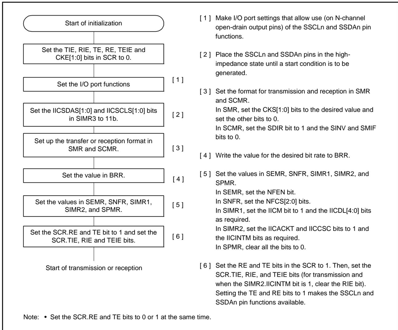
Figure 27.45 Example of the Flow of SCI Initialization (for Simple I<sup>2</sup>C Mode)
