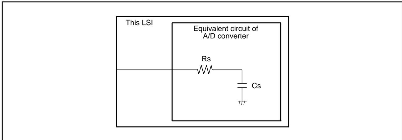
Figure 32.17 Internal Equivalent Circuit of Analog Input Pin
