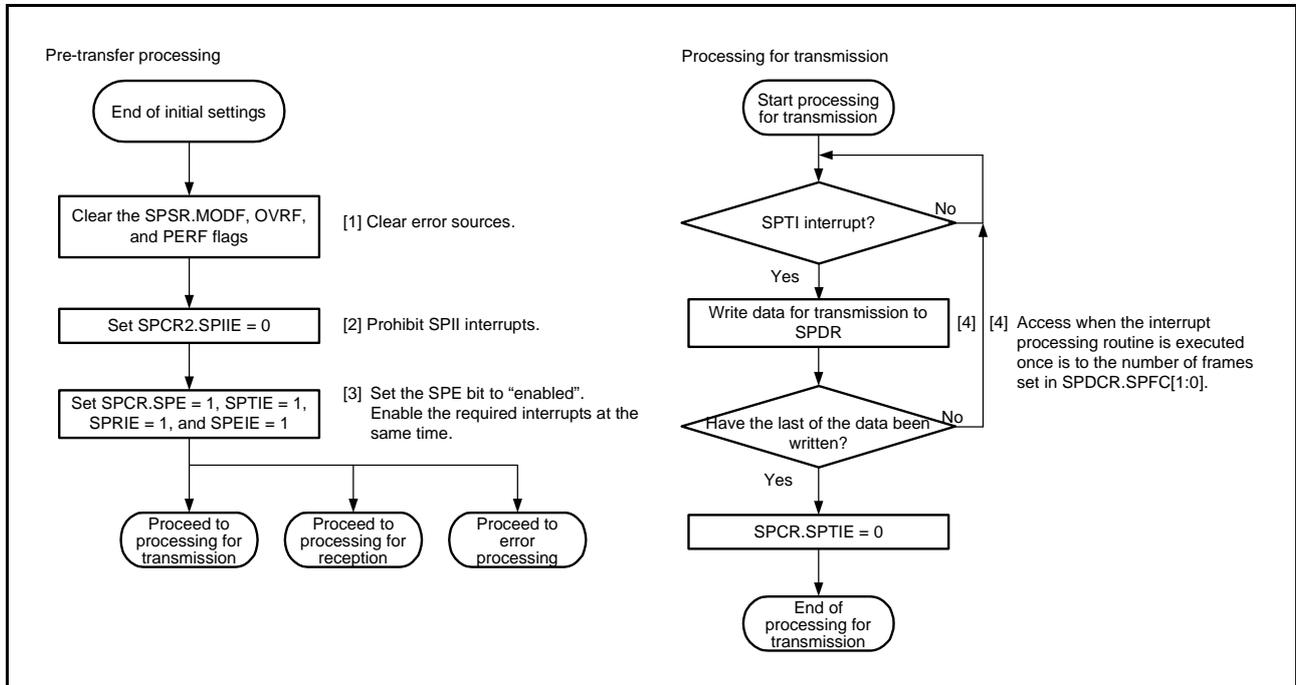
Figure 30.39 Flowchart in Slave Mode (Transmission)
