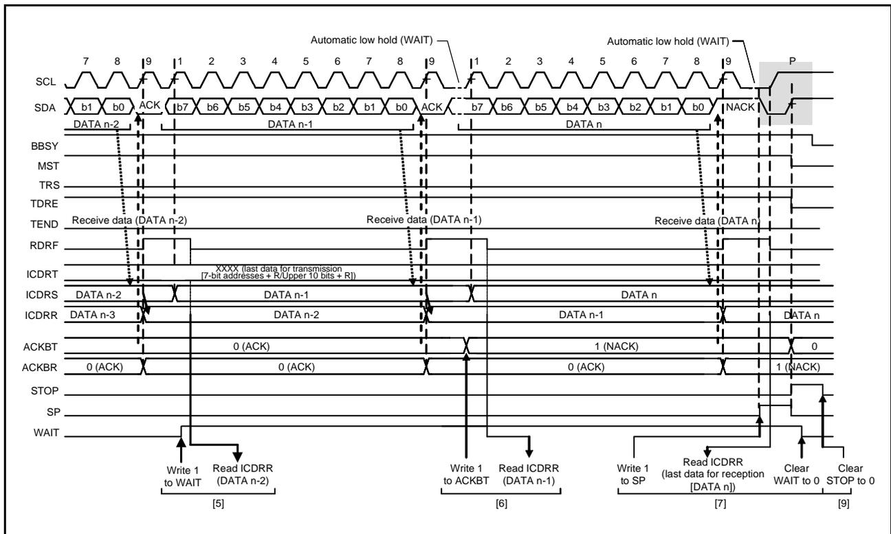
Figure 29.14 Master Receive Operation Timing (3) (when RDRFS = 0)
