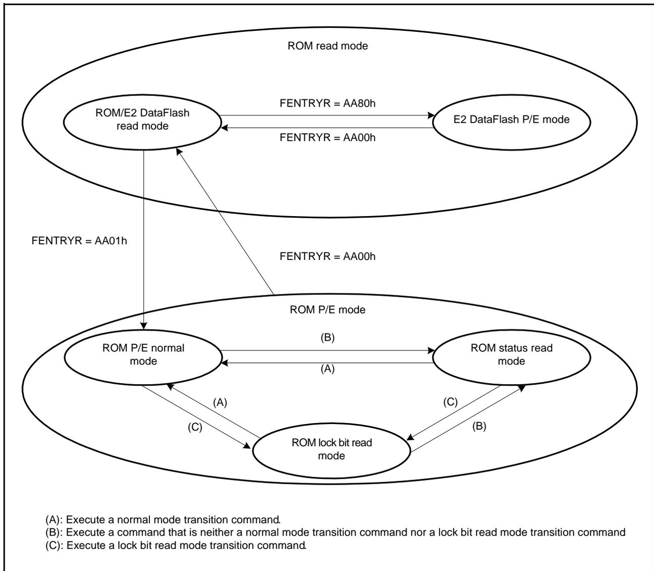
Figure 36.4 Mode Transitions of the FCU (Associated with the ROM)
