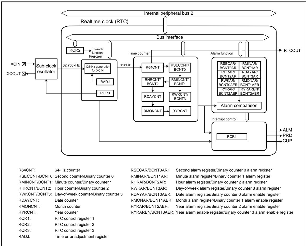
Figure 25.1 Block Diagram of RTC
