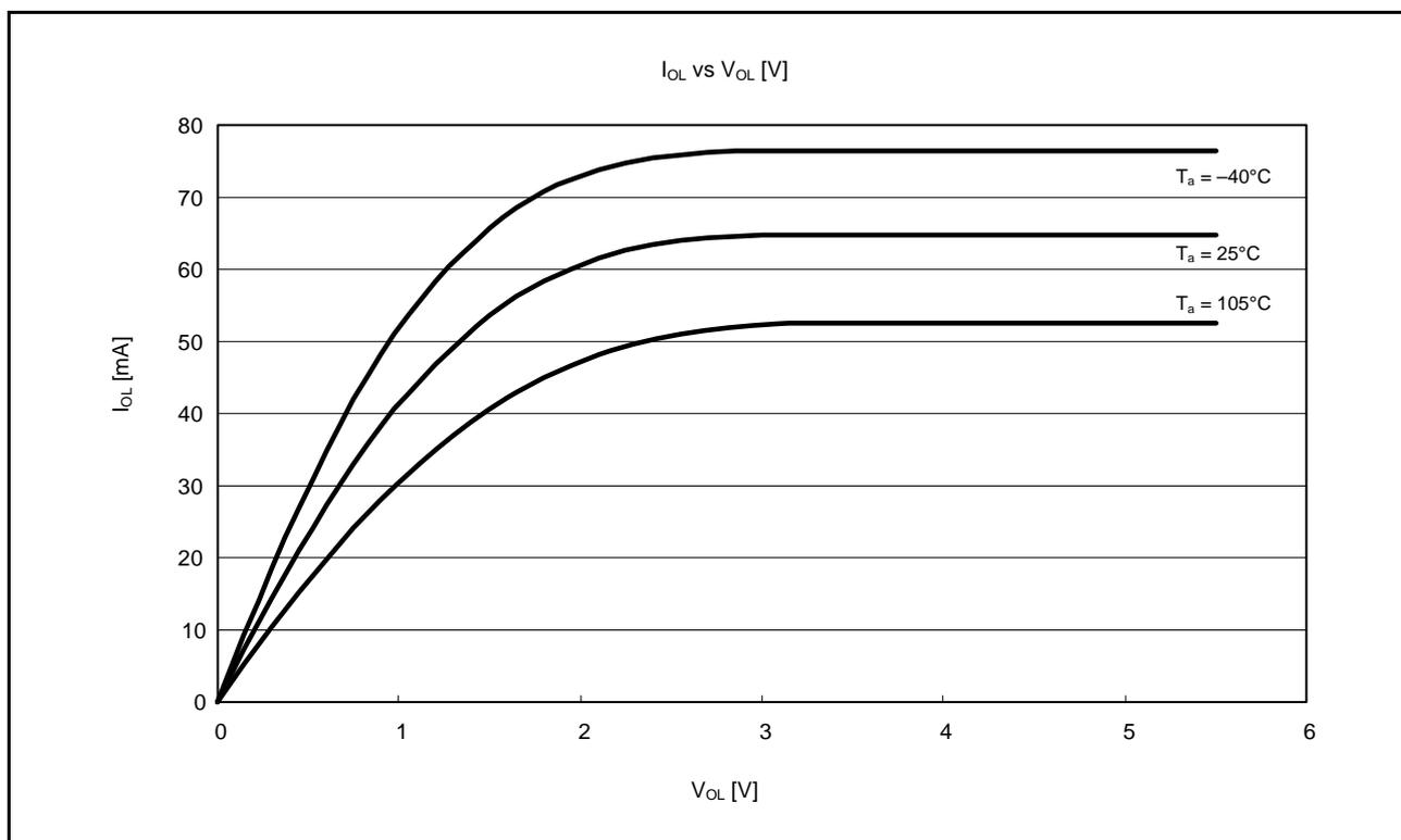
Figure 38.20  $V_{OL}$  and  $I_{OL}$  Temperature Characteristics of RIIC Output Pin at  $V_{CC} = 5.5$  V (Reference Data)
