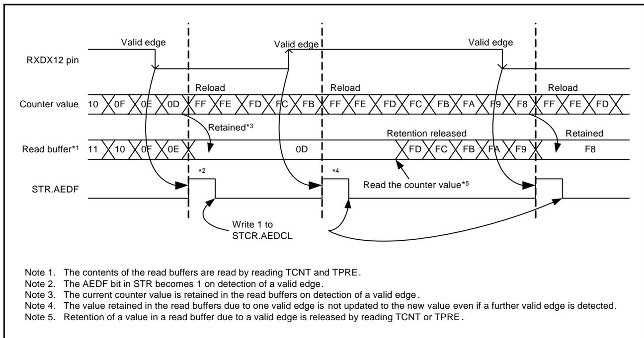
Figure 27.64 Example of Operations for Bit-Rate Measurement
