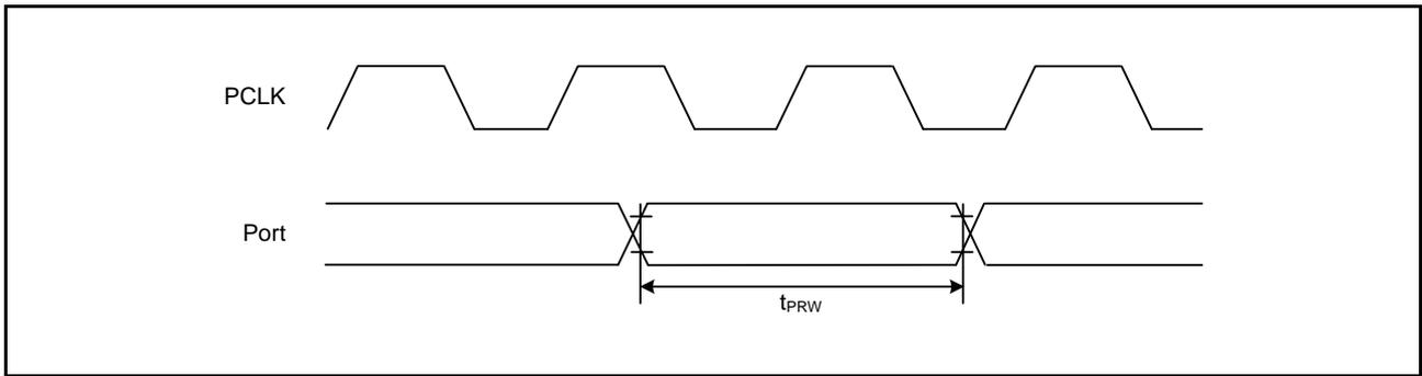
Figure 38.33 I/O Port Input Timing
