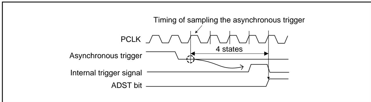
Figure 32.16 Asynchronous Trigger Input Timing
