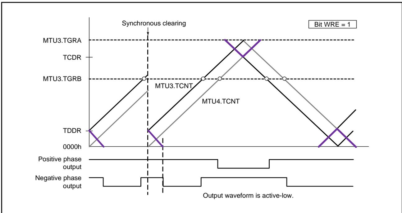
**Figure 21.58** Example of Synchronous Clearing in Dead Time during Up-Counting (Timing (3) in Figure 21.56; Bit WRE of TWCR is 1 in the MTU)
