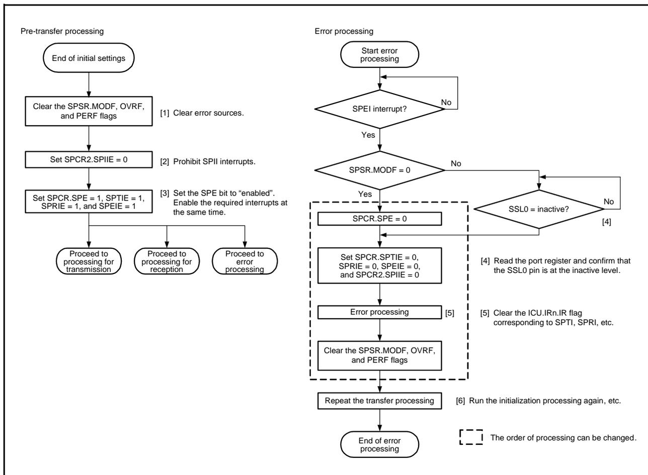
Figure 30.37 Flowchart for Master Mode (Error Processing)
