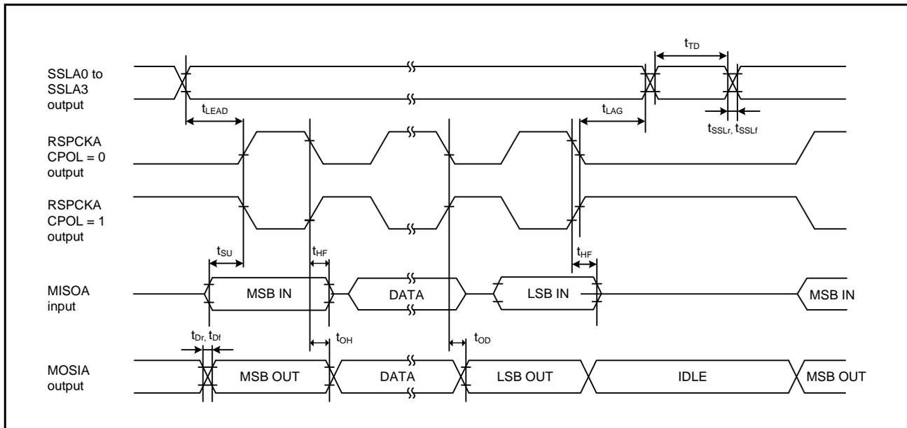
**Figure 38.43 RSPI Timing (Master, CPHA = 0) (Bit Rate: PCLKB Set to Divided by 2)**
