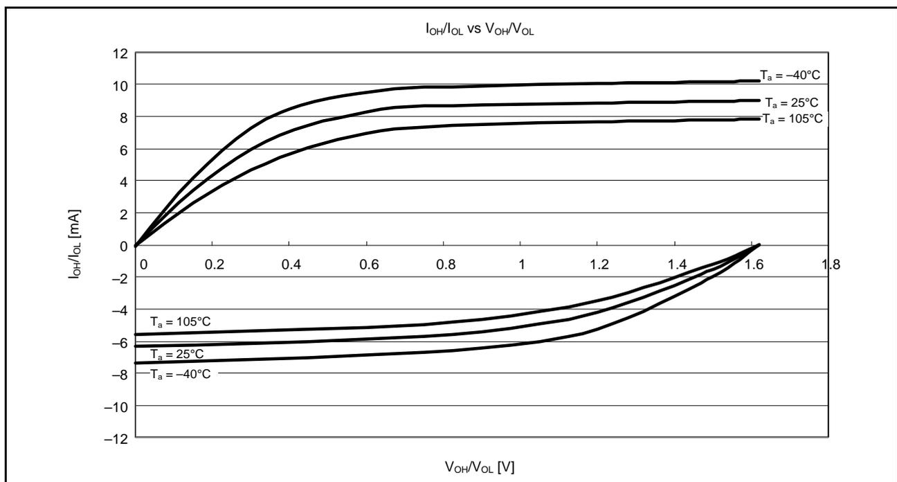
Figure 38.13  $V_{OH}/V_{OL}$  and  $I_{OH}/I_{OL}$  Temperature Characteristics at  $V_{CC} = 1.62$  V when High-Drive Output is Selected (Reference Data)
