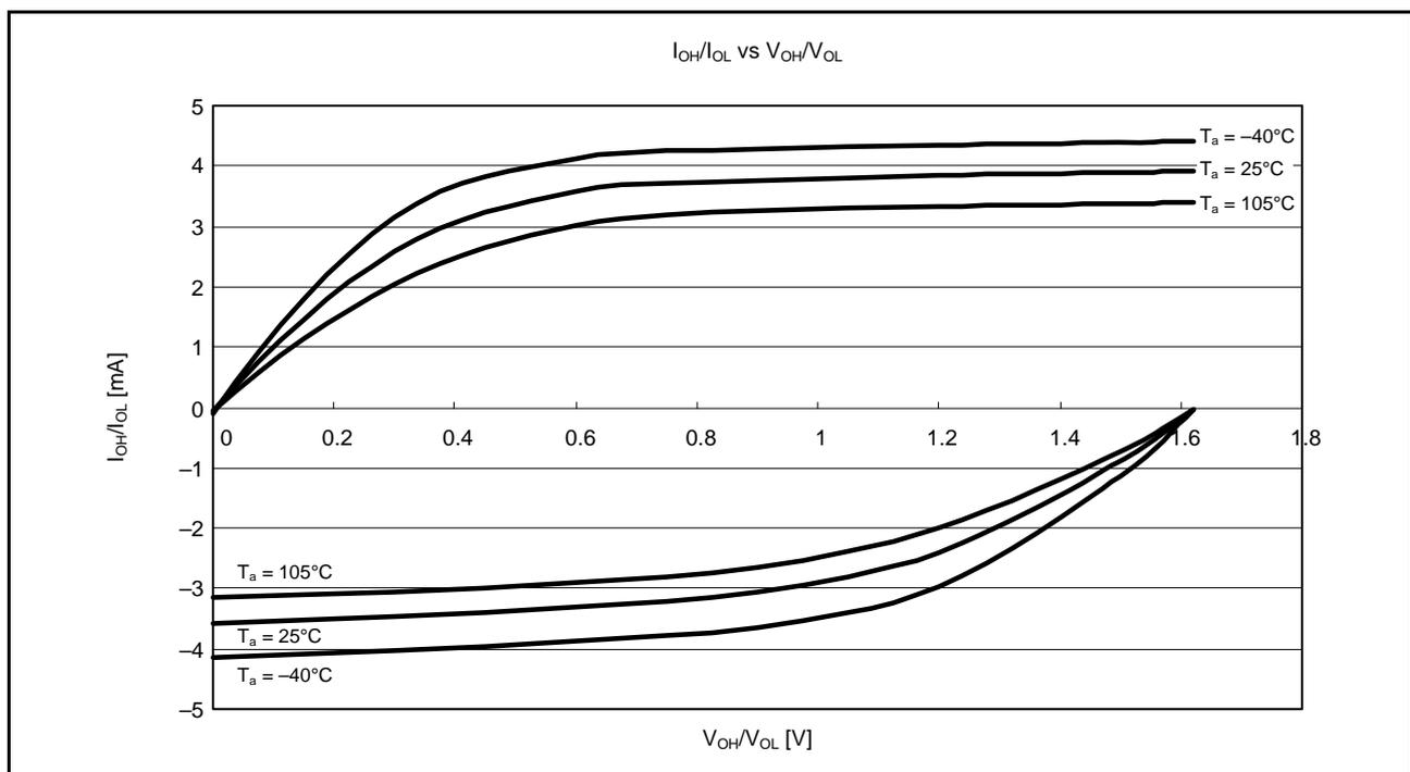
Figure 38.8 V<sub>OH/V<sub>OL</sub></sub> and I<sub>OH/I<sub>OL</sub></sub> Temperature Characteristics at VCC = 1.62 V when Normal Output is Selected (Reference Data)
