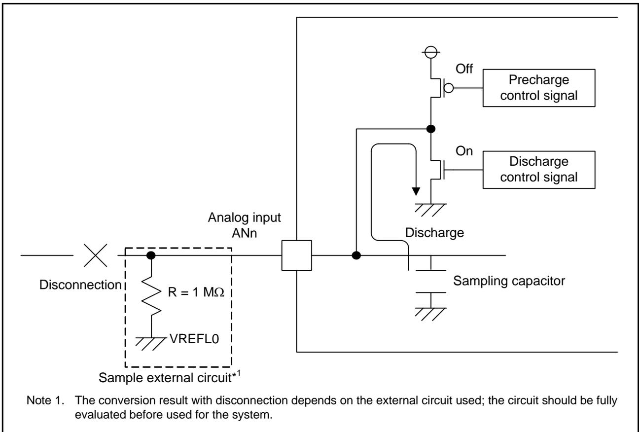
Figure 32.15 VREFL0 Disconnection Detection Example (Discharge Selected)
