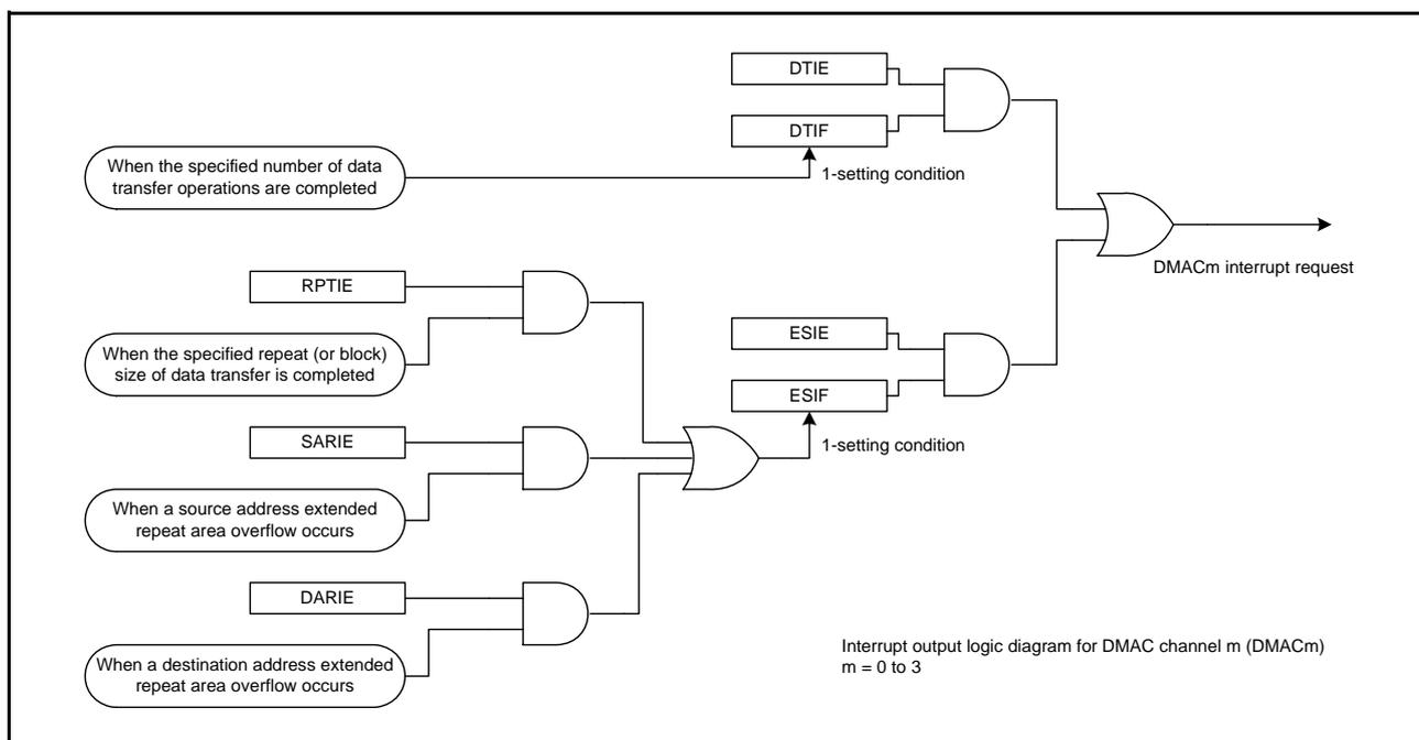
**Figure 16.13 Schematic Logic Diagram of Interrupt Outputs**
