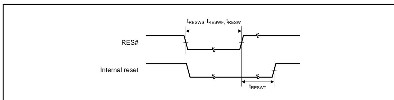
**Figure 38.29 Reset Input Timing**
