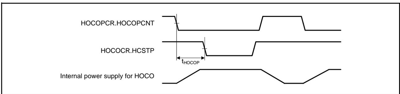
**Figure 38.26 HOCO Power Control Timing**
