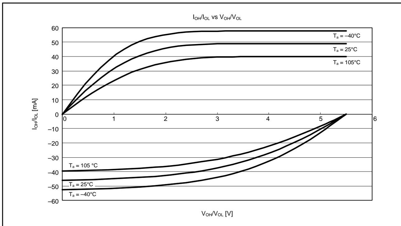
Figure 38.11  $V_{OH}/V_{OL}$  and  $I_{OH}/I_{OL}$  Temperature Characteristics at  $V_{CC} = 5.5\text{ V}$  when Normal Output is Selected (Reference Data)
