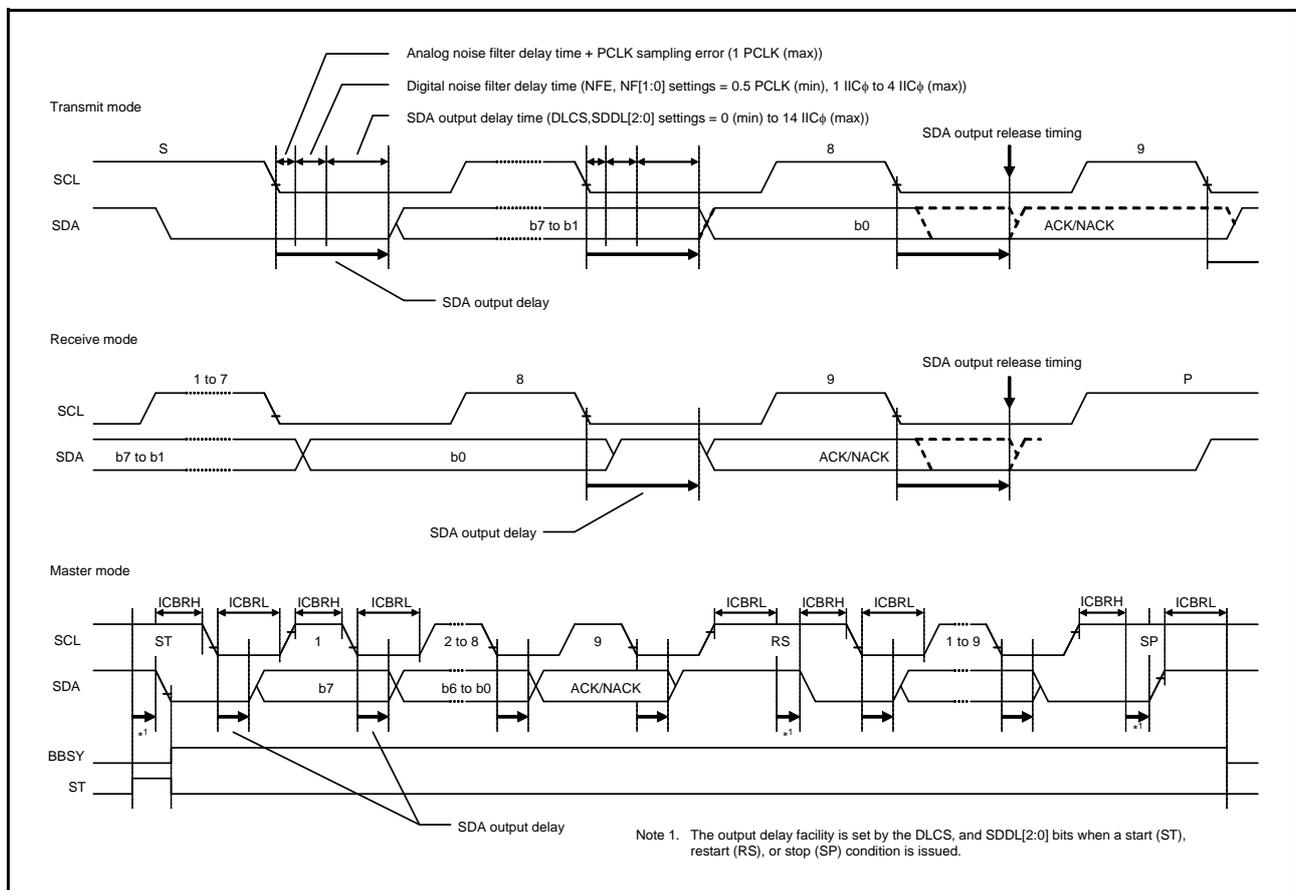
Figure 29.22 SDA Output Delay Facility
