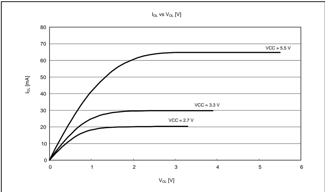
Figure 38.17 V<sub>OL</sub> and I<sub>OL</sub> Voltage Characteristics of RIIC Output Pin at T<sub>a</sub> = 25°C (Reference Data)
