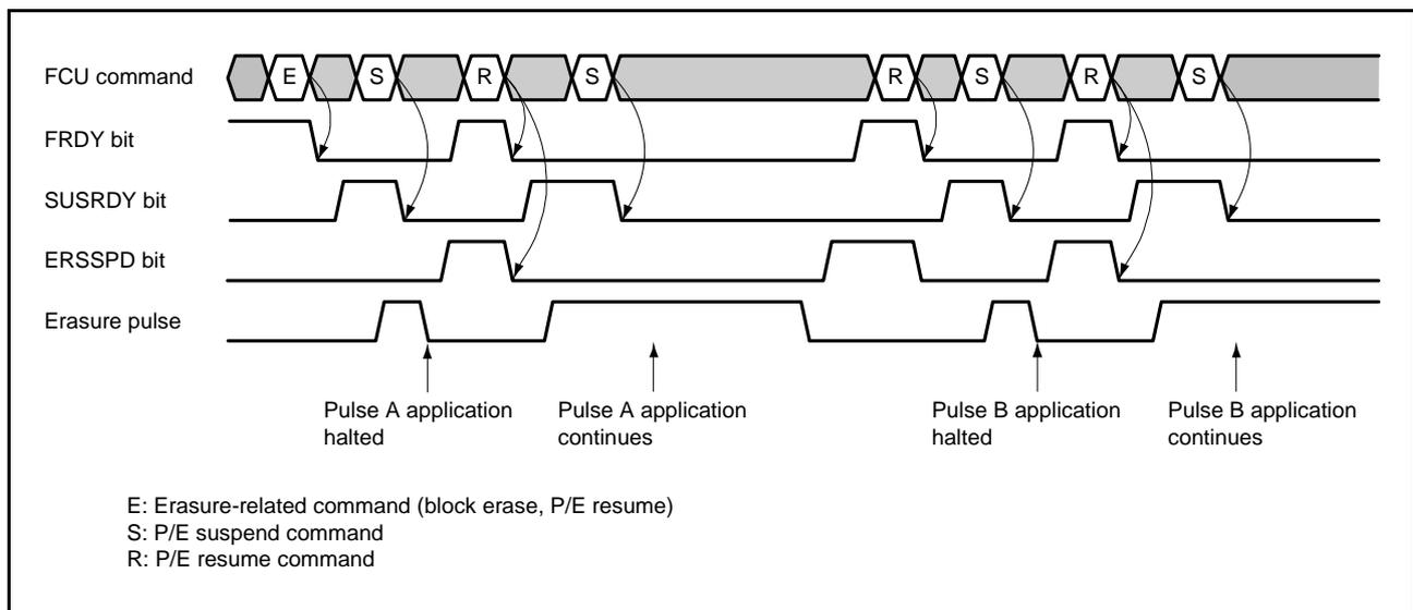
Figure 36.19 Suspension during Erasure (Suspension Priority Mode)
