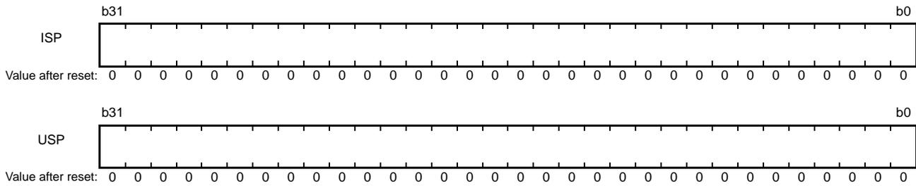
The stack pointer (SP) can be either of two types, the interrupt stack pointer (ISP) or the user stack pointer (USP). Whether the stack pointer operates as the ISP or USP depends on the value of the stack pointer select bit (U) in the processor status word (PSW).
