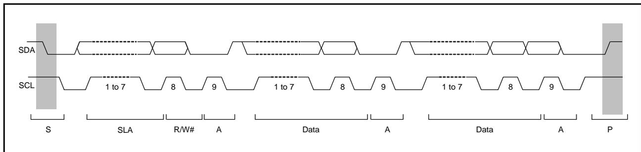
Figure 29.4 I<sup>2</sup>C Bus Timing (SLA = 7 Bits)
