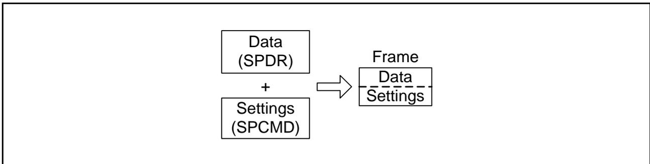
Figure 30.43 Concept of a Frame
