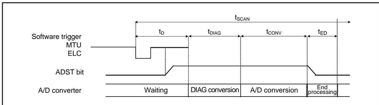
**Figure 32.11 Scan Conversion Timing (Activated by Software, or Triggers from the MTU or ELC)**
