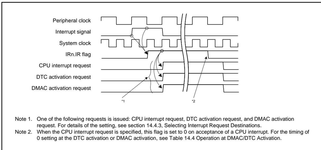
Figure 14.2 IR<sub>n</sub>.IR Flag Operation for Edge Detection Interrupts
