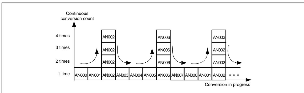
Figure 32.2 Scan Conversion Sequence with ADADC.ADC[1:0] = 11b, ADS[2] = 1, and ADS[6] = 1
