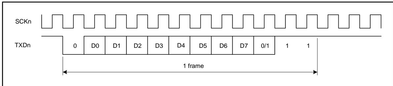
**Figure 27.7** Phase Relationship between Output Clock and Transmit Data
