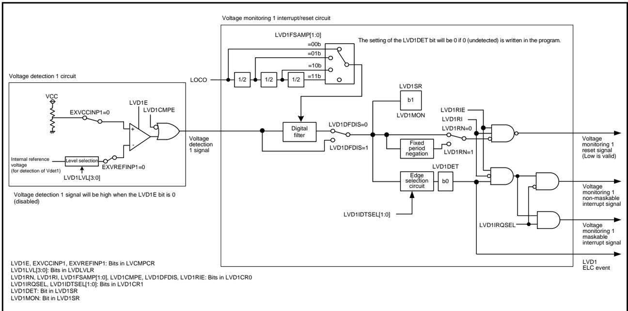
Figure 8.2 Block Diagram of Voltage Monitoring 1 Interrupt/Reset Circuit
