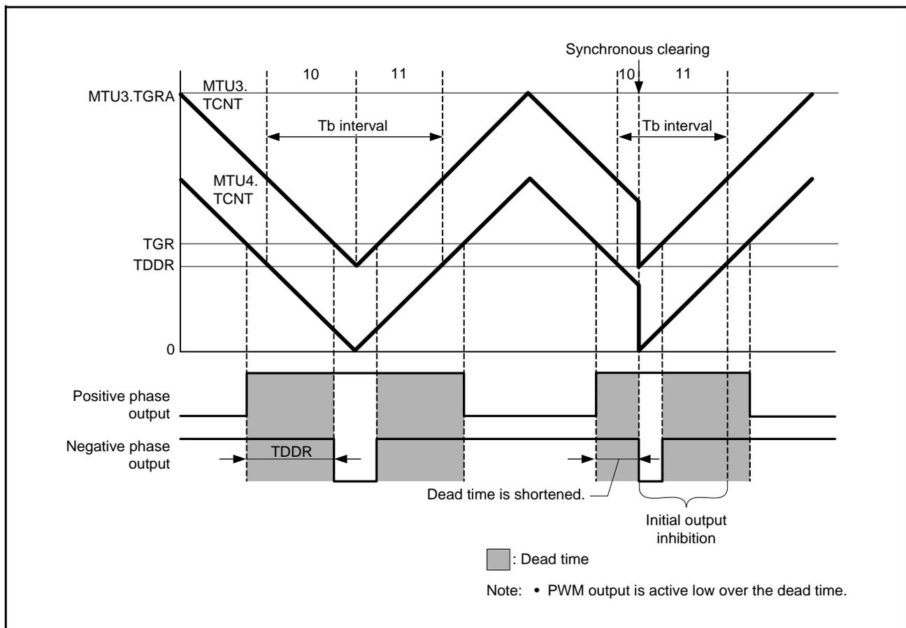
Figure 21.122 Example of Synchronous Clearing (when Condition 1 Applies)
