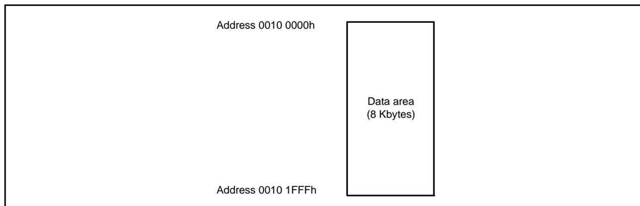
Figure 37.2 Configuration of the Data Area for the E2 DataFlash Memory
