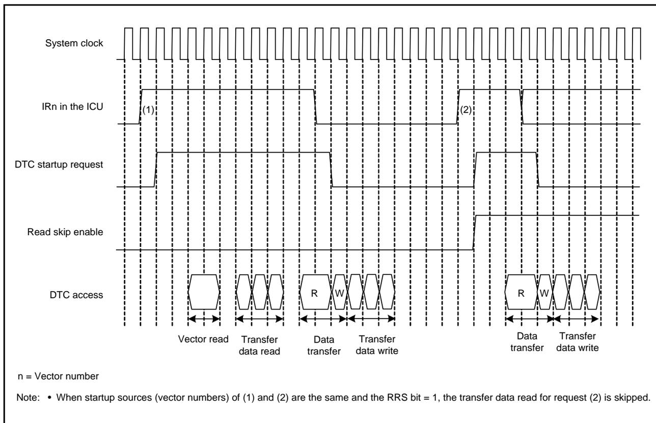
**Figure 17.13 Example of Operation when Transfer Information Skip is Executed (Vector, Transfer Information, and Transfer Destination Data on the RAM, and Transfer Source Data on the Peripheral Module)**
