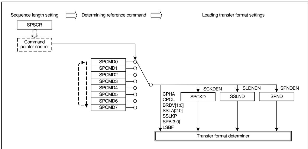
Figure 30.30 Procedure for Determining the Form of Serial Transfer in Master Mode
