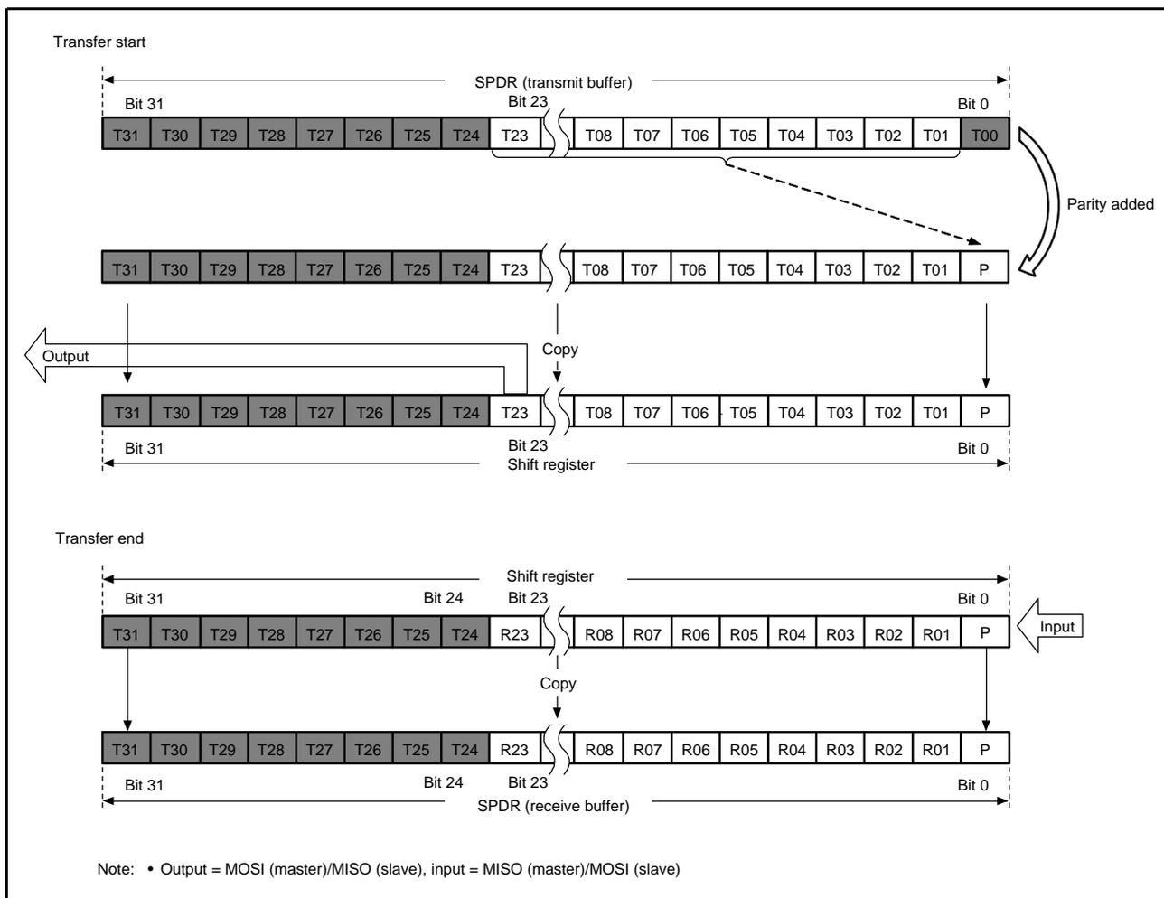
Figure 30.20 MSB-First Transfer (24-Bit Data, Parity Enabled)
