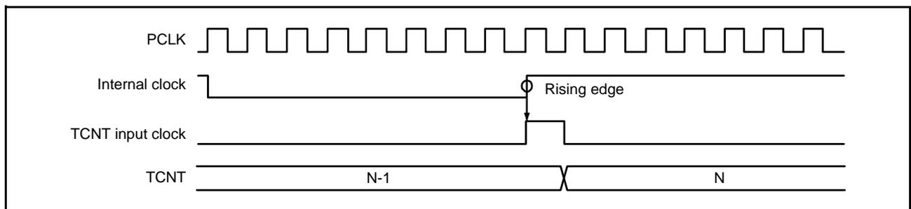
**Figure 21.85** Count Timing in Internal Clock Operation (MTU5)
