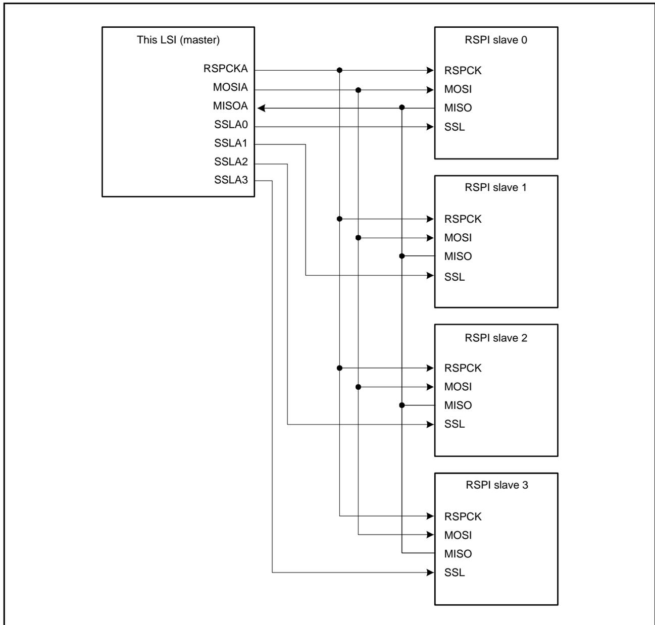
Figure 30.8 Single-Master/Multi-Slave Configuration Example (This LSI = Master)
