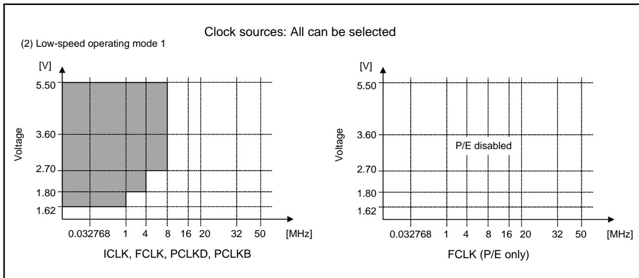
Figure 11.3 Relationship between the Operating Voltages and Operating Frequencies in Low-Speed Operating Mode 1
