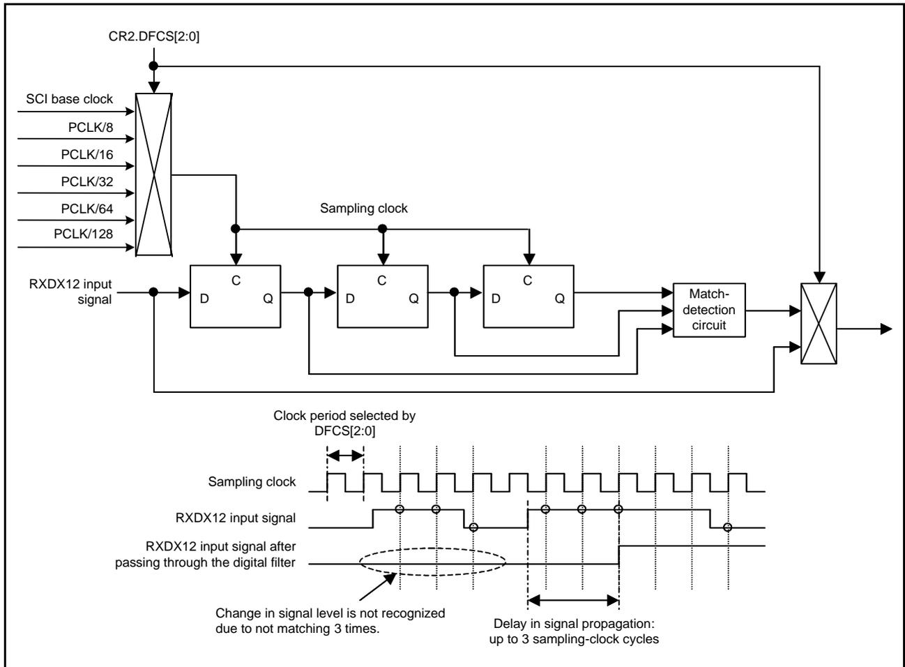
Figure 27.63 Example of Operations with the Digital Filter
