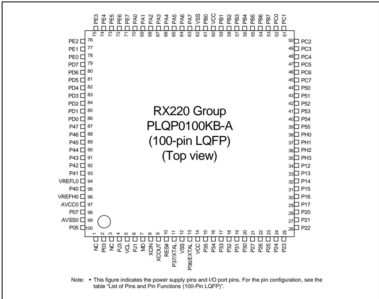
**Figure 1.3 Pin Assignments of the 100-Pin LQFP**
