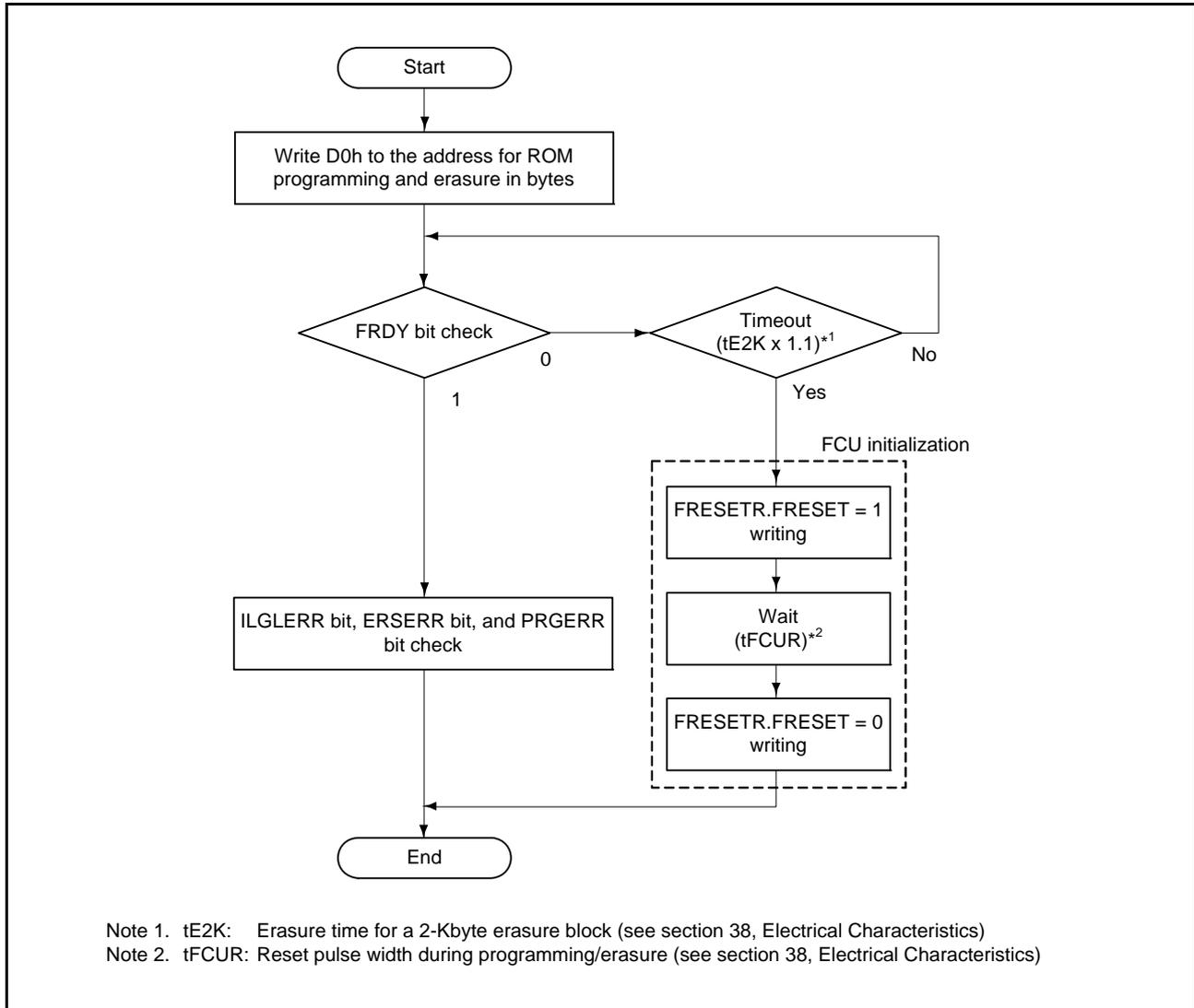
Figure 36.18 Procedure for Resuming Programming or Erasure
