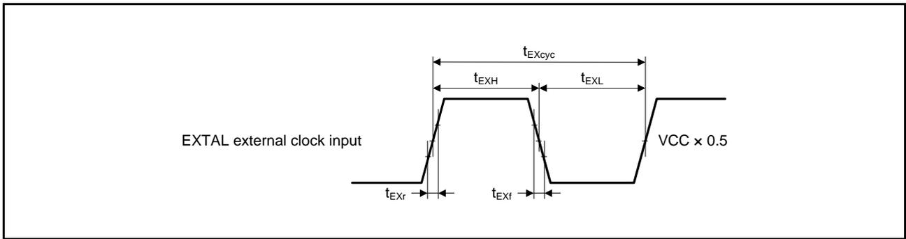
Figure 38.21 EXTAL External Clock Input Timing
