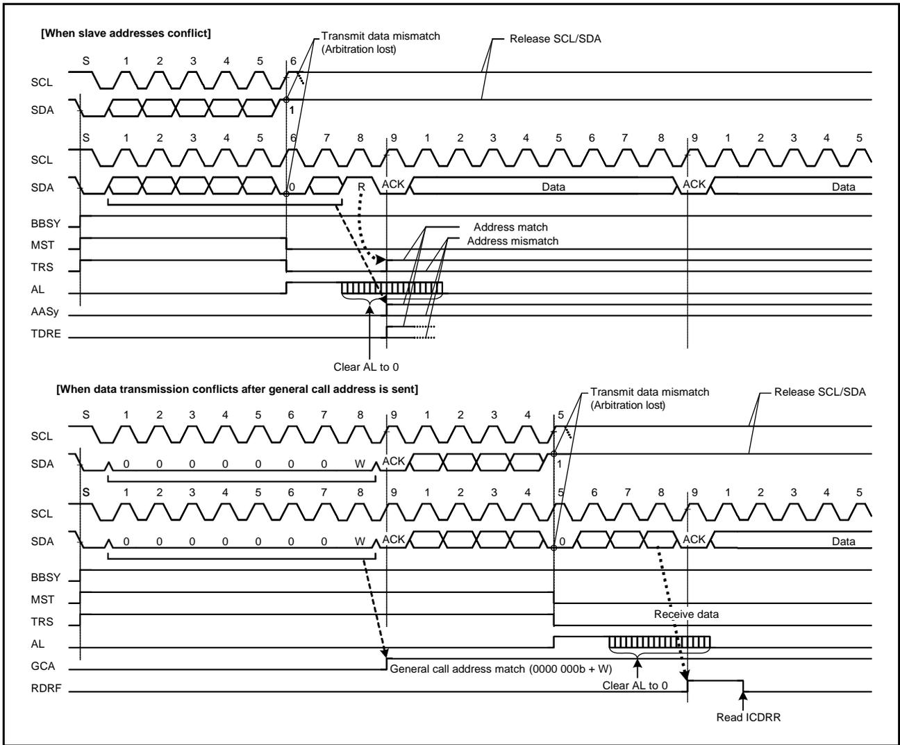
Figure 29.33 Examples of Master Arbitration-Lost Detection (MALE = 1)
