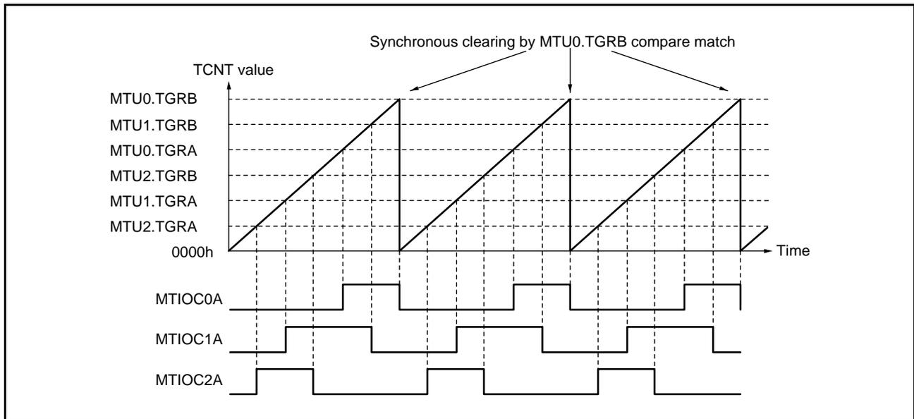
Figure 21.13 Example of Synchronous Operation
