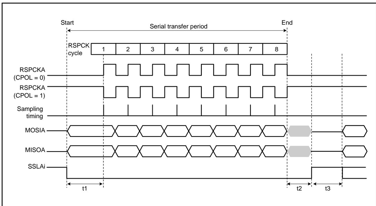
Figure 30.23 RSPI Transfer Format (CPHA = 0)
