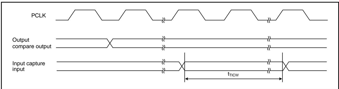
Figure 38.34 MTU Input/Output Timing
