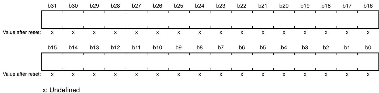
DAR is used to set the transfer destination start address.
