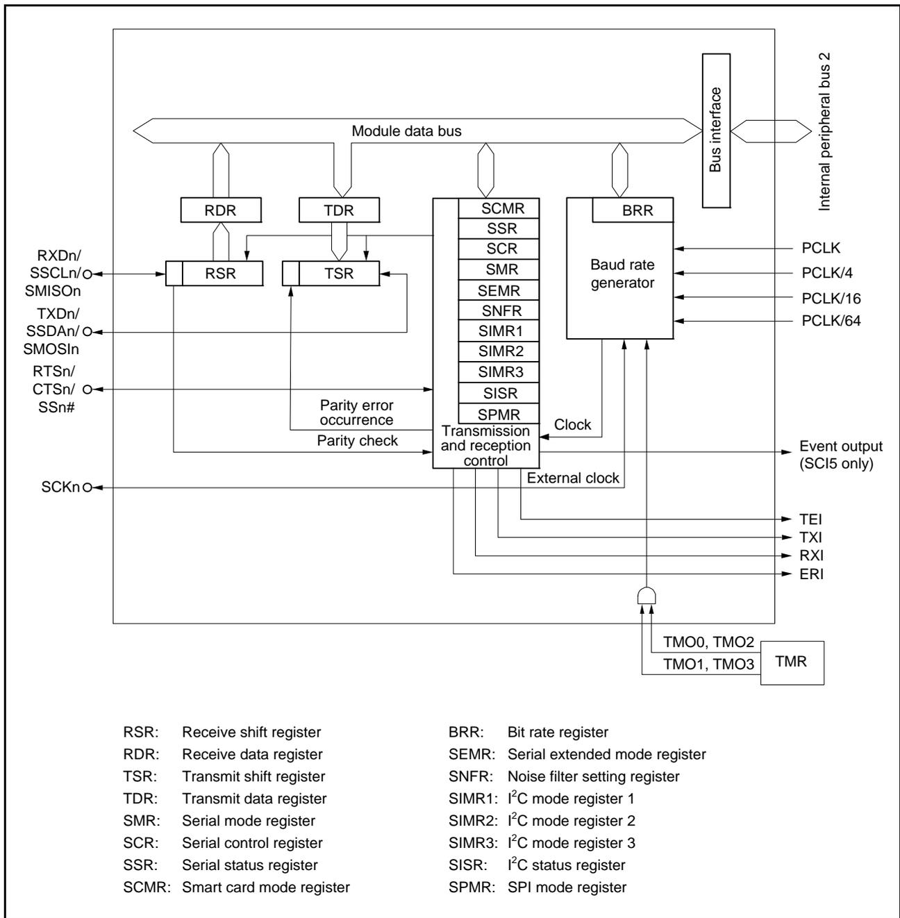
Figure 27.2 Block Diagram of SCI5 and SCI6
