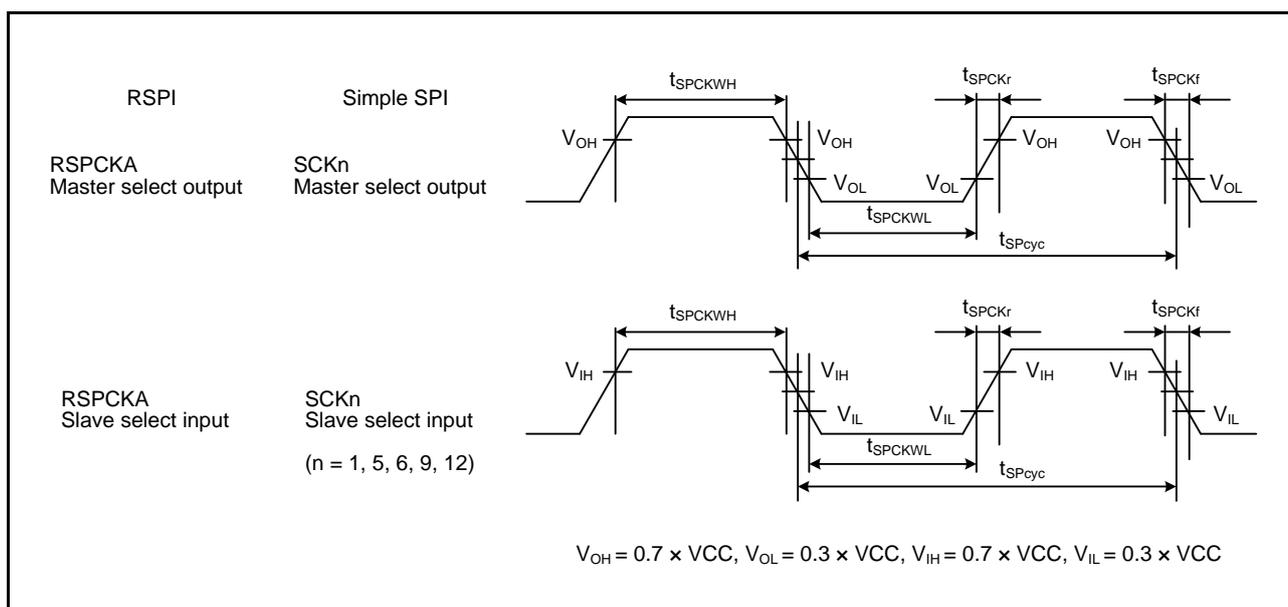
Figure 38.41 RSPCKA Clock Timing and Simple SPI Clock Timing
