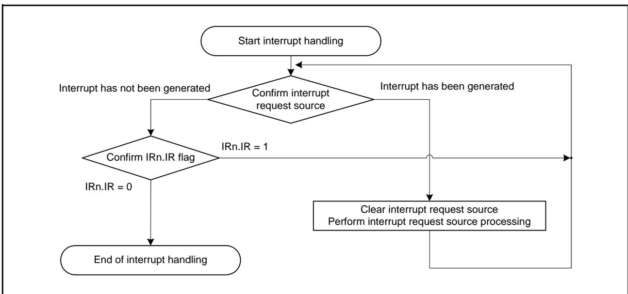
Figure 14.7 Procedure for Handling Level Detection Interrupts
