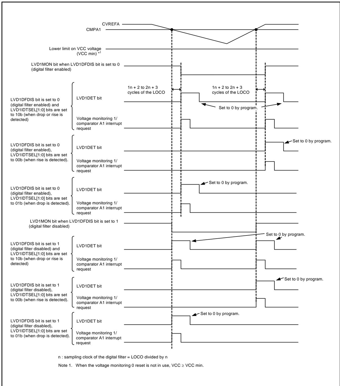
Figure 33.2 Operating Example of Comparator A1
