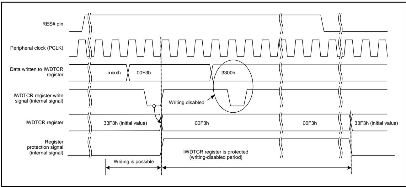
**Figure 26.5 Control Waveforms Produced in Response to Writing to the IWDTCR**
