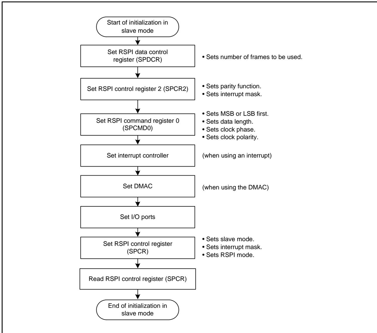
Figure 30.46 Example of Initialization Flowchart in Slave Mode (Clock Synchronous Operation)
