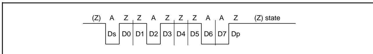
Figure 27.30 Direct Convention (SDIR in SCMR = 0, SINV in SCMR =0, PM in SMR = 0)
