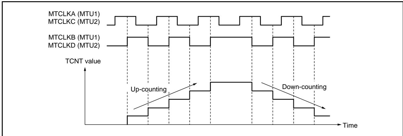
Figure 21.33 Example of Operation in Phase Counting Mode 4
