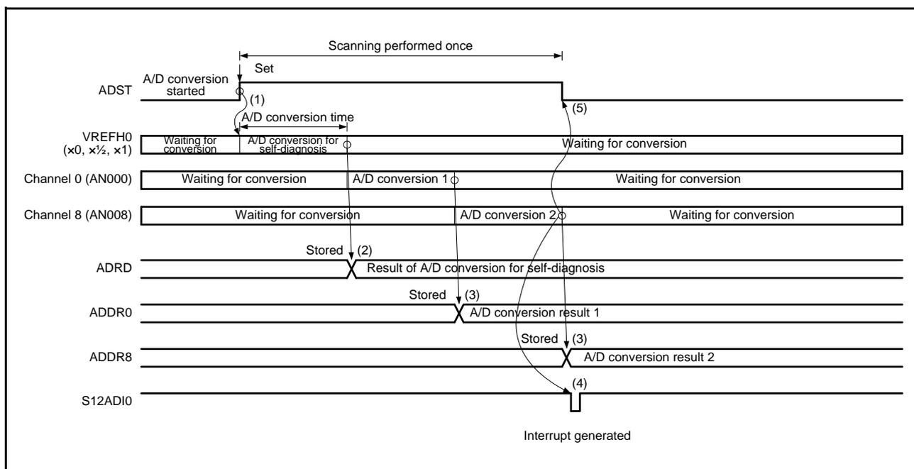
Figure 32.4 Example of Operation in Single Scan Mode (Basic Operation + Self-Diagnosis)
