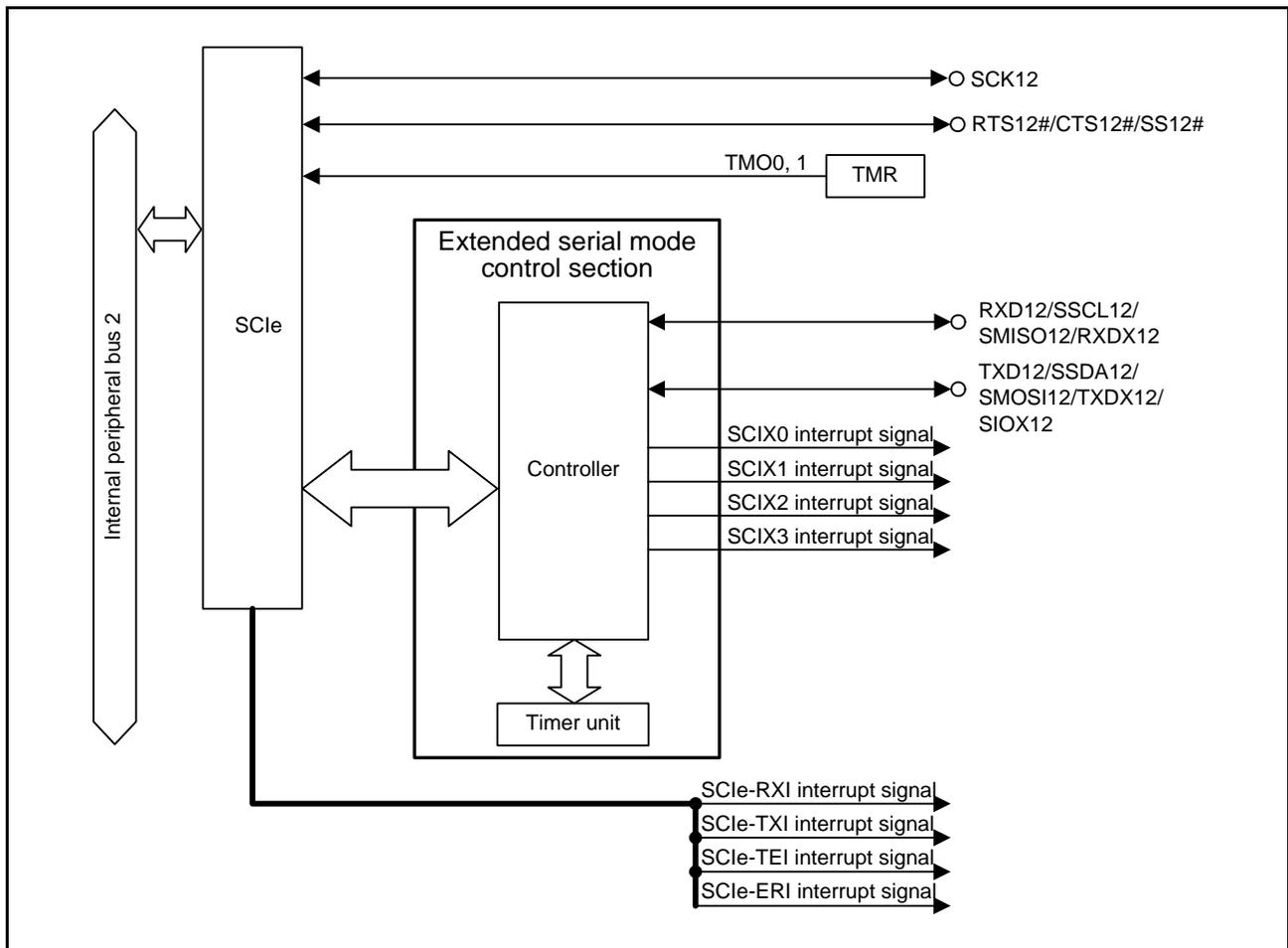
Figure 27.3 Block Diagram of SCI2 (SCIf)
