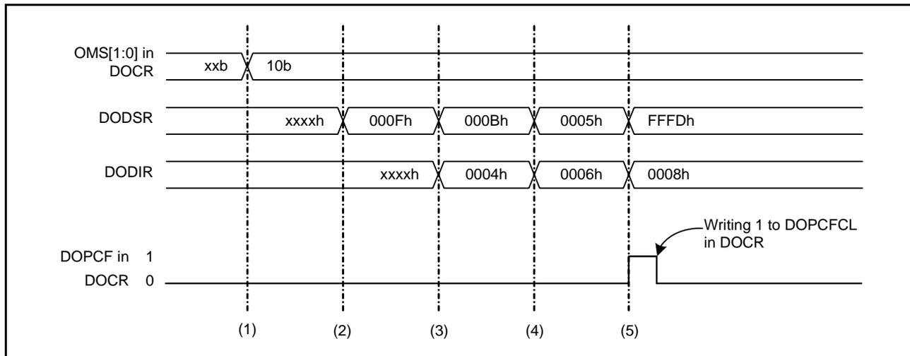
Figure 34.4 Example of Operation in Data Subtraction Mode
