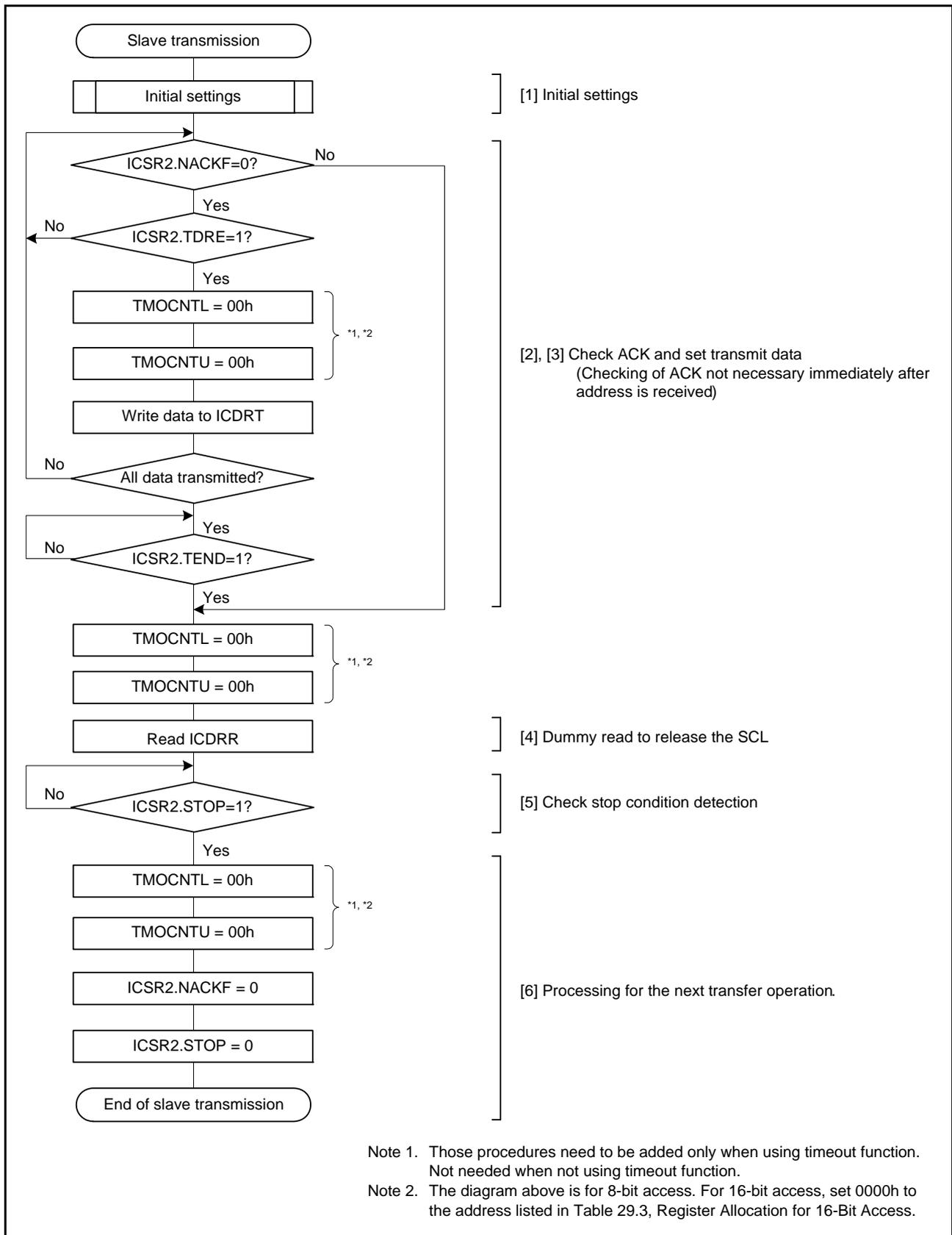
Figure 29.15 Example of Slave Transmission Flowchart
