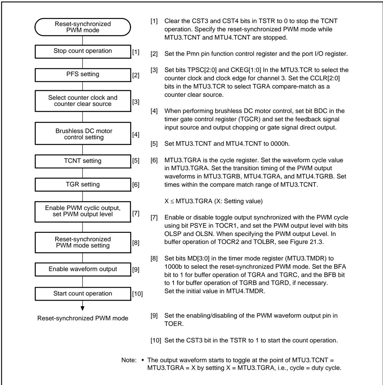
Figure 21.35 Procedure for Selecting Reset-Synchronized PWM Mode
