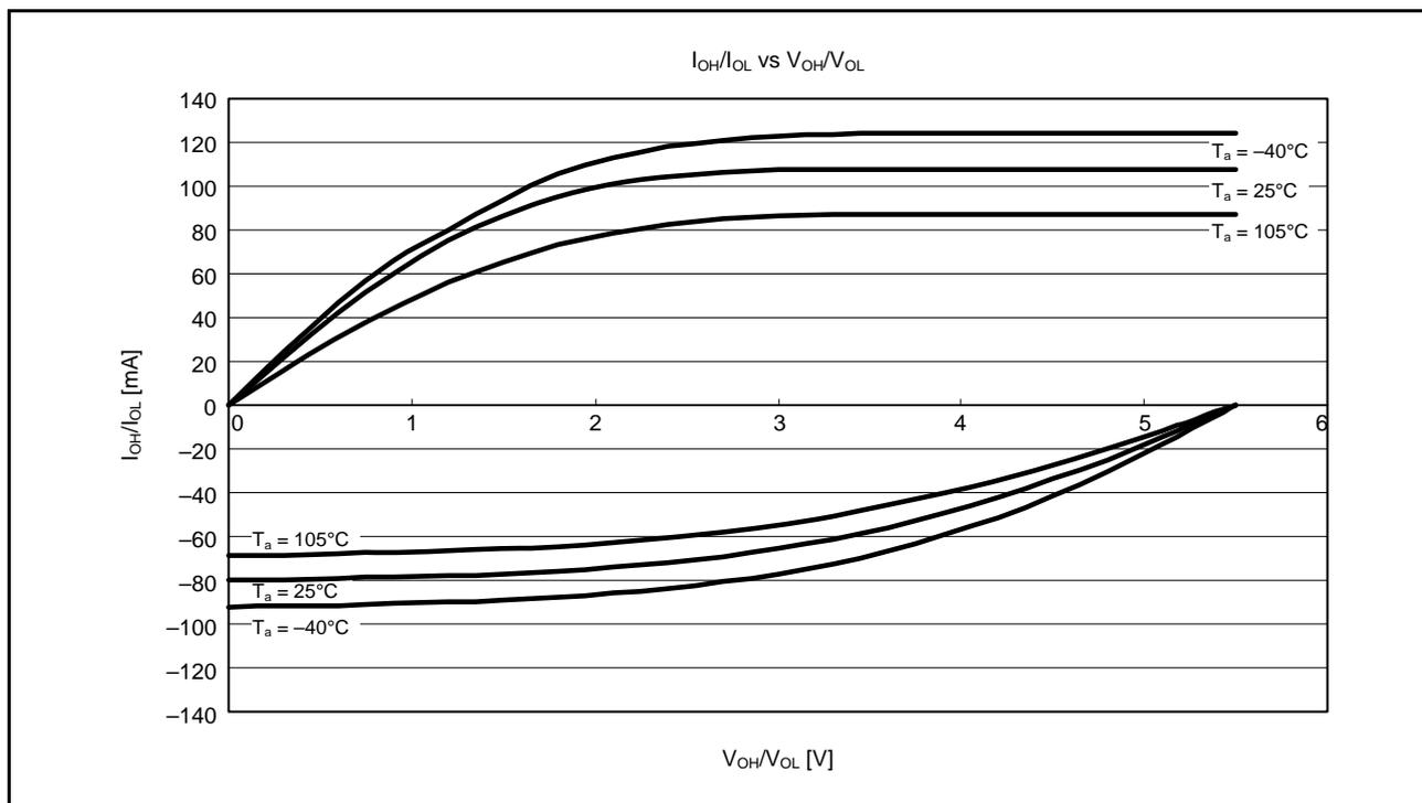
Figure 38.16 VOH/VOL and IOH/IOL Temperature Characteristics at VCC = 5.5 V when High-Drive Output is Selected (Reference Data)
