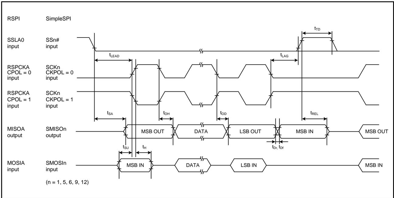
Figure 38.46 RSPI Timing (Slave, CPHA = 0) and Simple SPI Timing (Slave, CKPH = 1)
