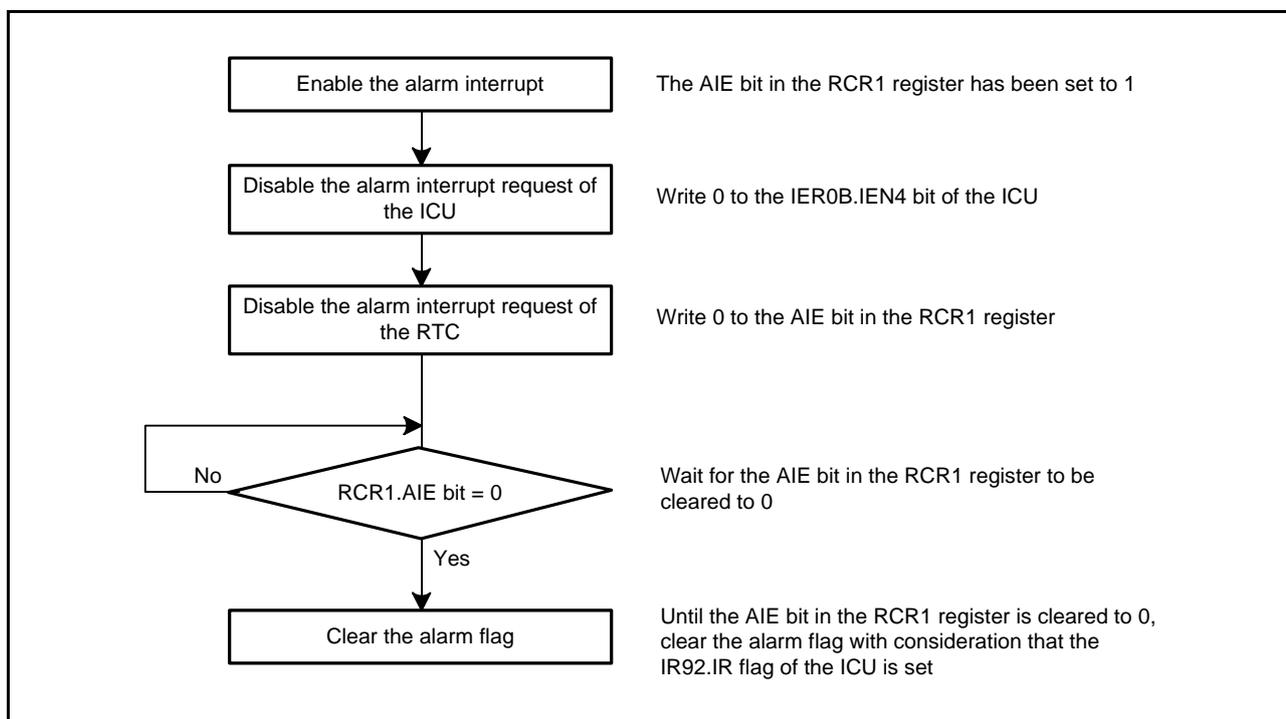
**Figure 25.8 Procedure for Disabling Alarm Interrupt Request**
