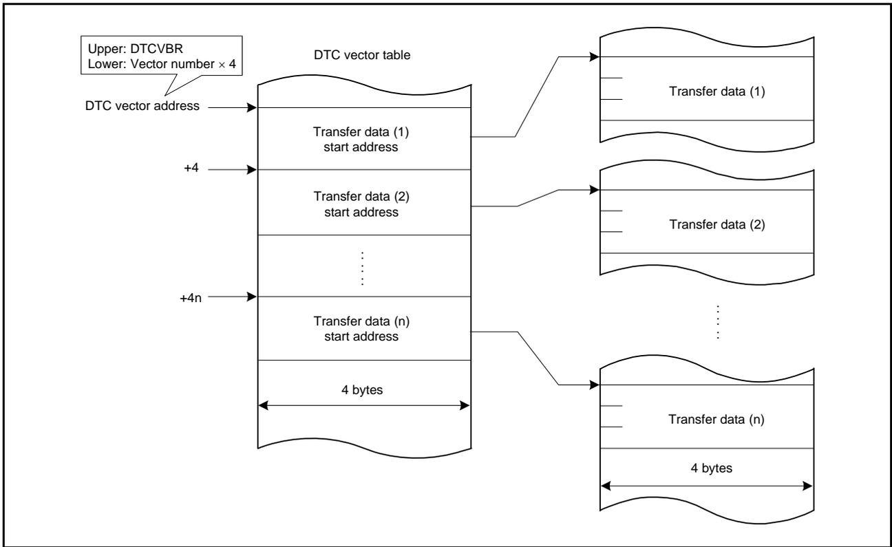
Figure 17.2 DTC Vector Table and Transfer Data
