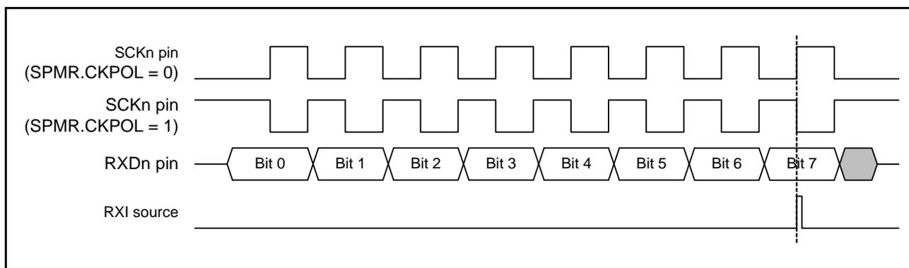
Figure 27.73 Timing of the RXI Interrupt in Simple SPI Mode (with Clock Delay)
