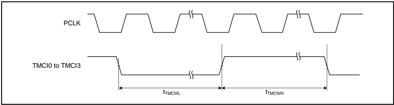
Figure 38.37 8-Bit Timer Clock Input Timing
