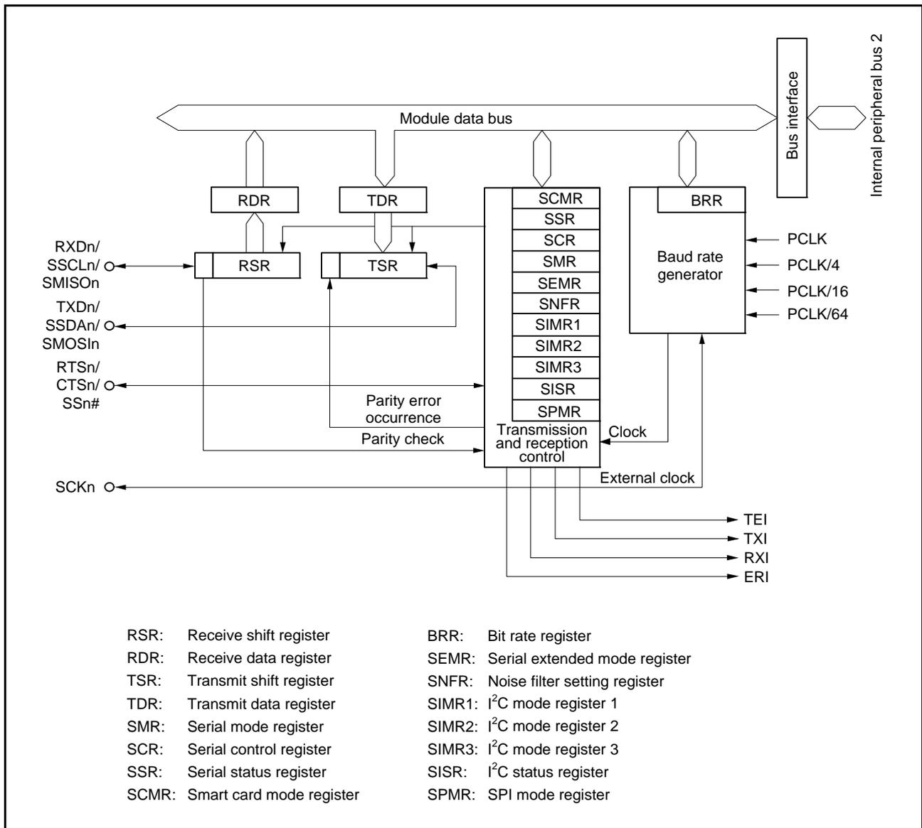
Figure 27.1 Block Diagram of SCI1 and 9
