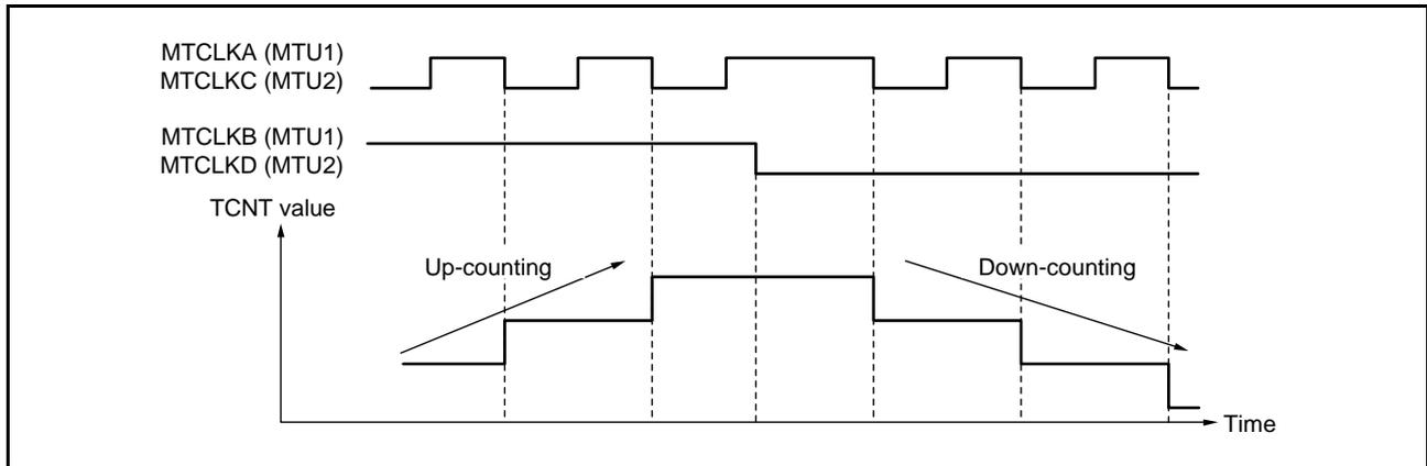
Figure 21.31 Example of Operation in Phase Counting Mode 2
