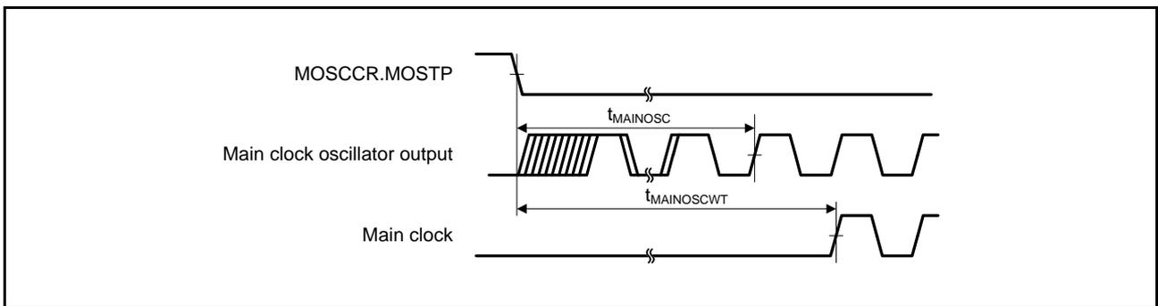
Figure 38.22 Main Clock Oscillation Start Timing
