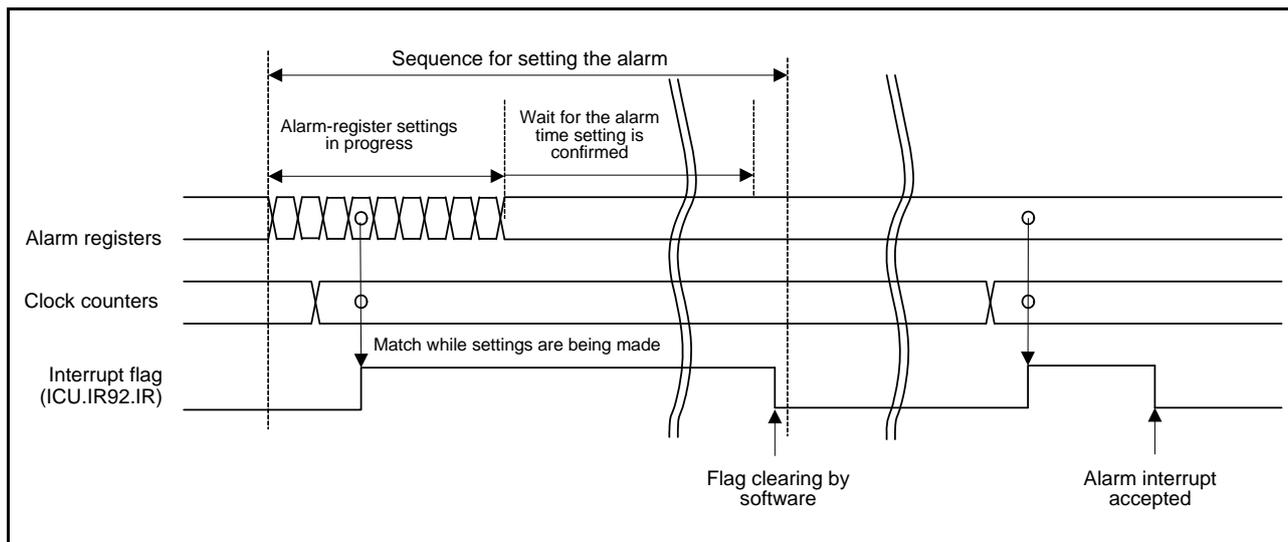
**Figure 25.9 Timing Chart for the Alarm Interrupt (ALM)**
