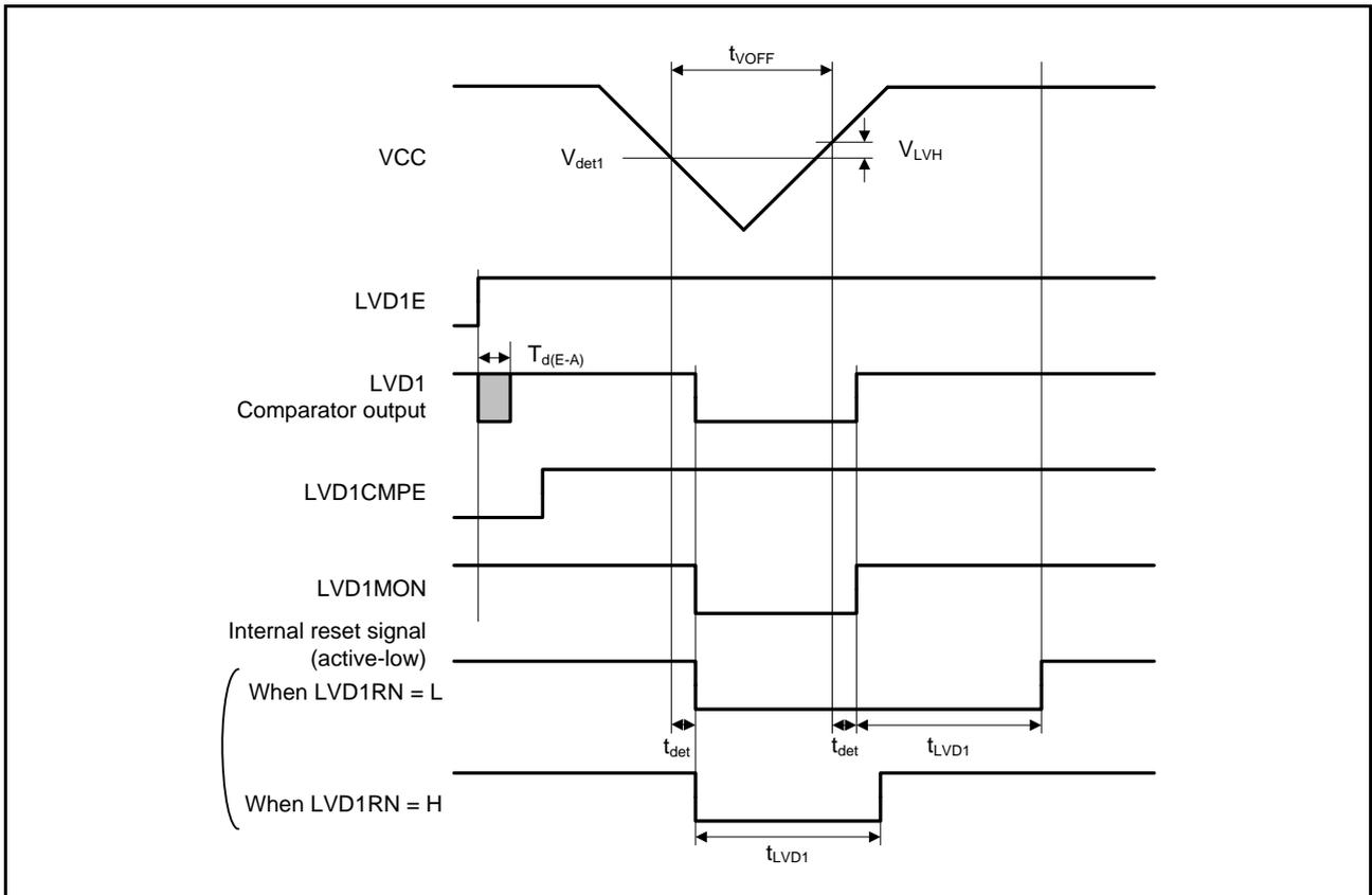
Figure 38.54 Voltage Detection Circuit Timing ( $V_{det1}$ )
