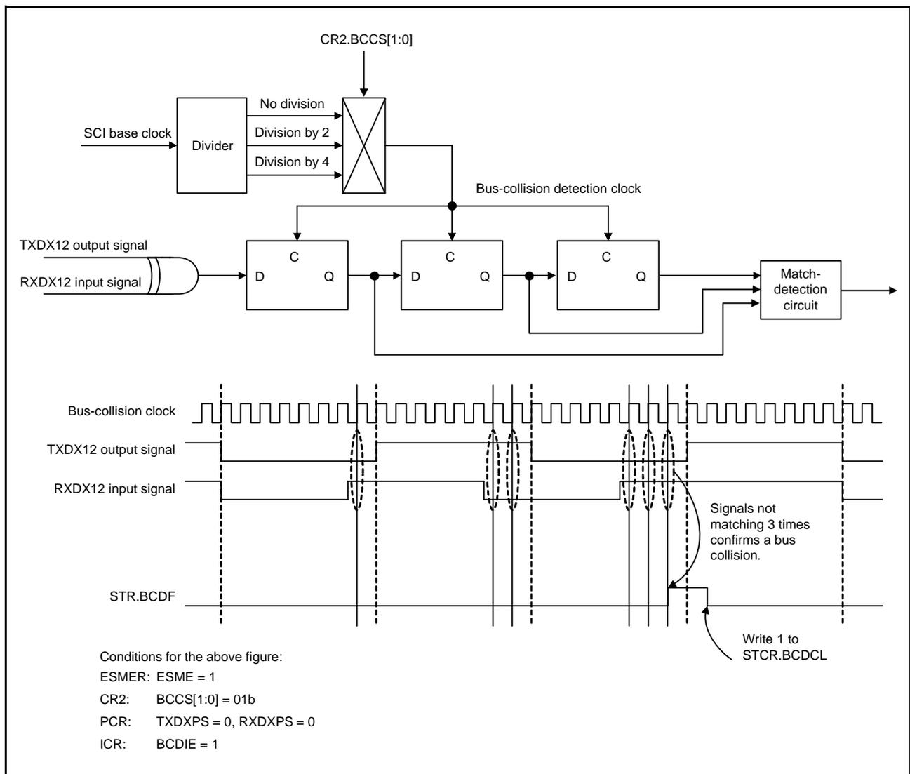
Figure 27.62 Example of Operations with Bus-Collision Detection
