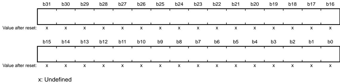
SAR is used to set the transfer source start address.
