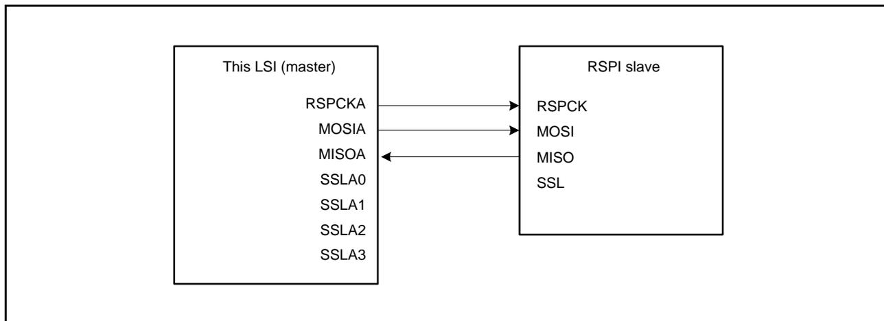
**Figure 30.11 Master (Clock Synchronous Operation)/Slave (Clock Synchronous Operation) Configuration Example (This LSI = Master)**
