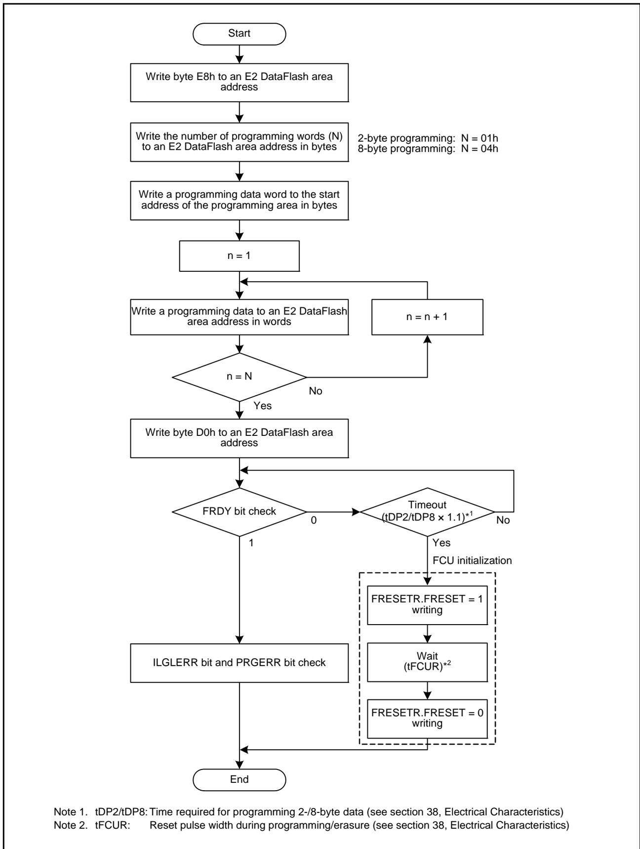
Figure 37.5 Procedure for E2 DataFlash Programming
