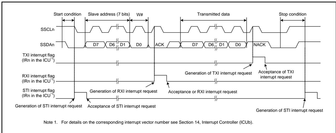
**Figure 27.47 Example 2 of Operations for Master Transmission in Simple I<sup>2</sup>C Bus Mode (with Seven-Bit Slave Addresses, ACK Interrupts, and NACK Interrupts in Use)**
