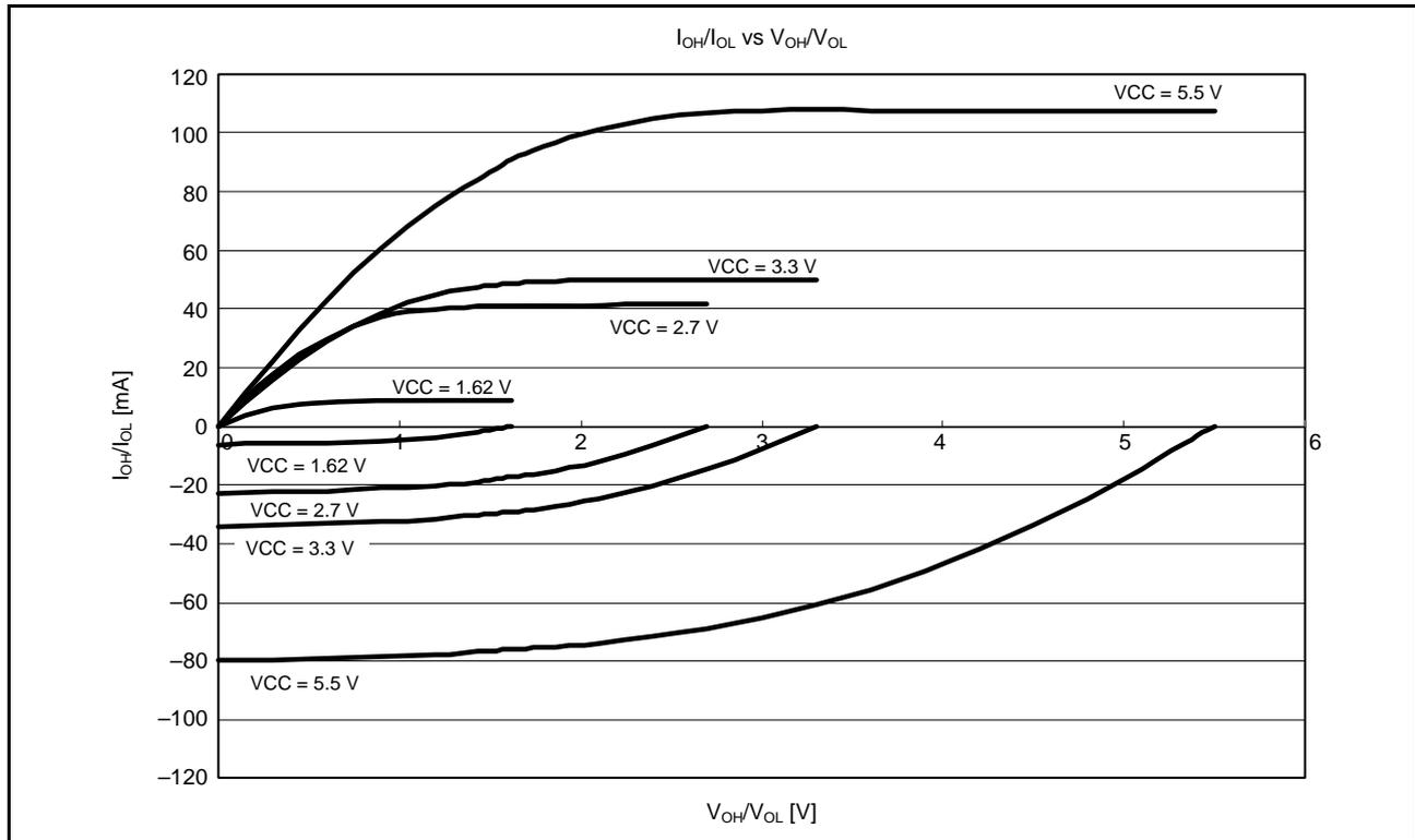
Figure 38.12  $V_{OH}/V_{OL}$  and  $I_{OH}/I_{OL}$  Voltage Characteristics at  $T_a = 25^\circ\text{C}$  when High-Drive Output is Selected (Reference Data)
