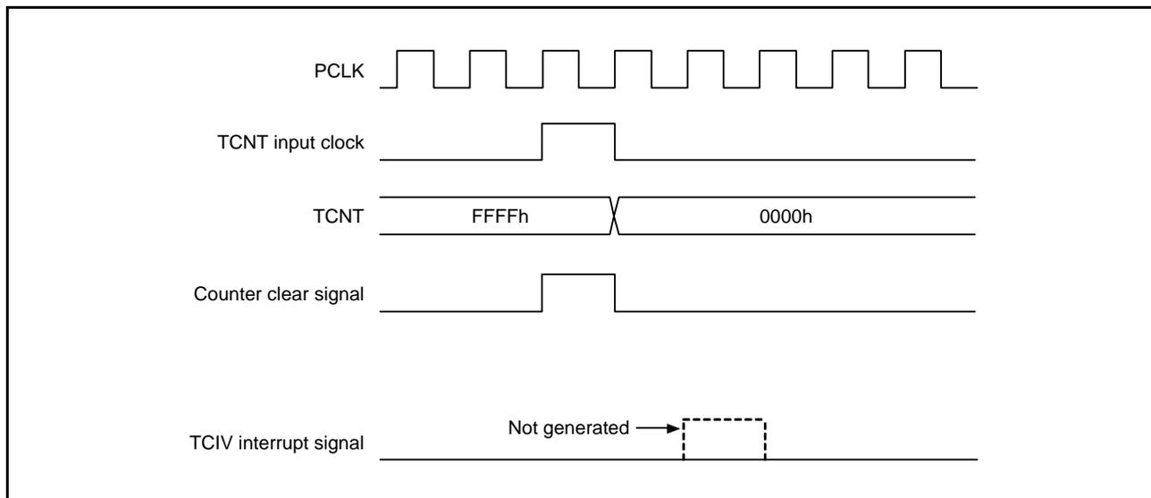
Figure 21.120 Contention between Overflow and Counter Clearing
