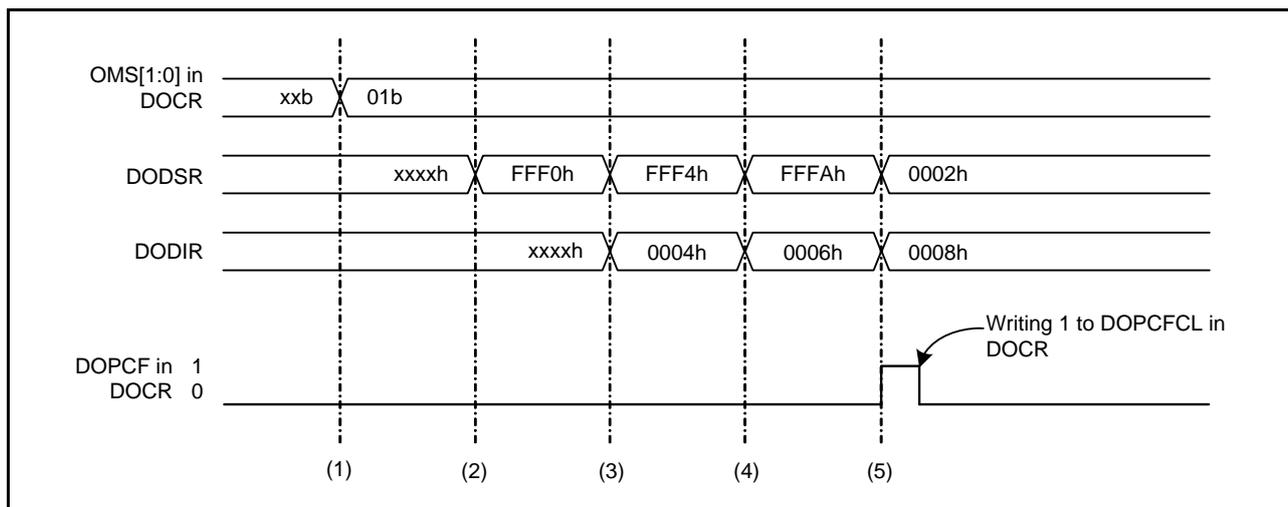
Figure 34.3 Example of Operation in Data Addition Mode
