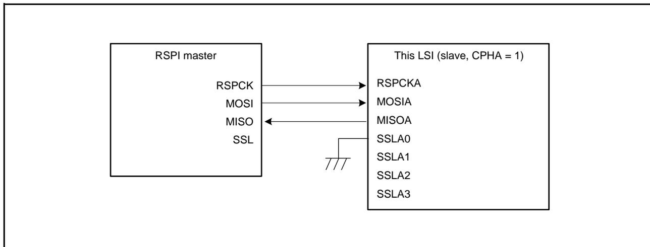
Figure 30.7 Single-Master/Single-Slave Configuration Example (This LSI = Slave, CPHA = 1)
