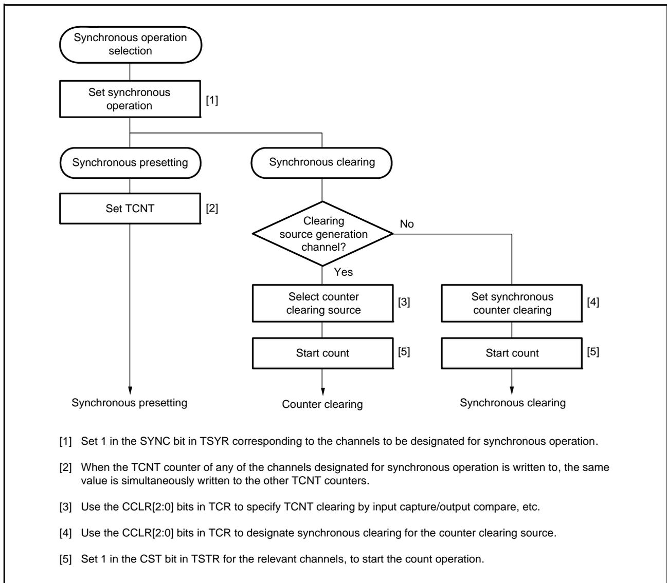
Figure 21.12 Example of Synchronous Operation Setting Procedure
