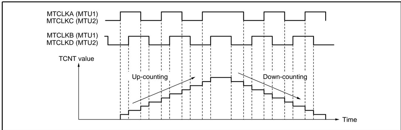
Figure 21.30 Example of Operation in Phase Counting Mode 1
