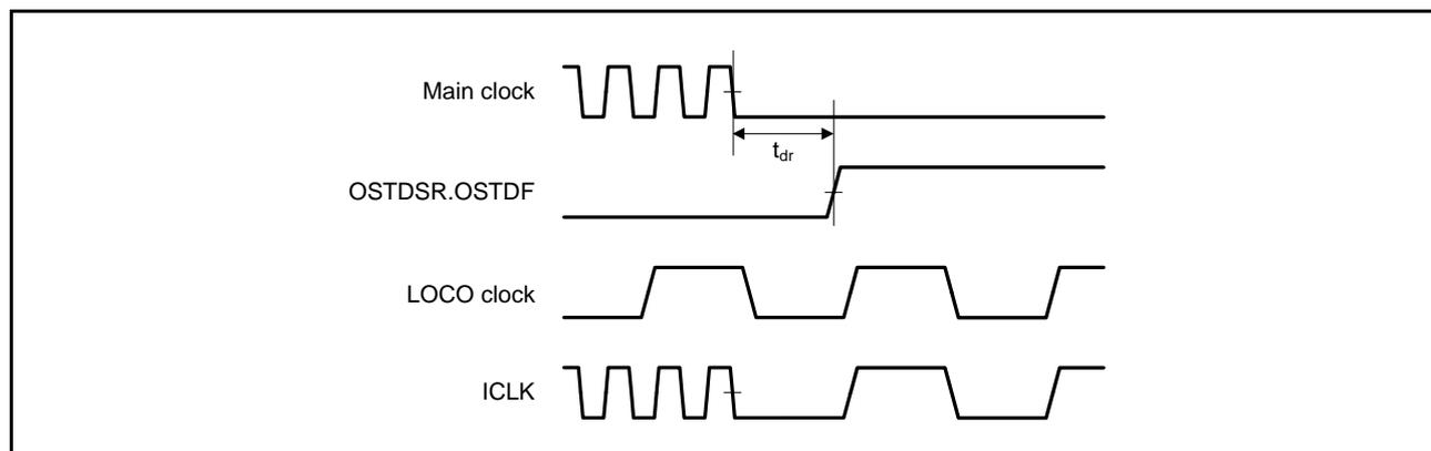
**Figure 38.56 Oscillation Stop Detection Timing**
