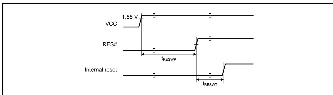
**Figure 38.28 Reset Input Timing at Power-On**
