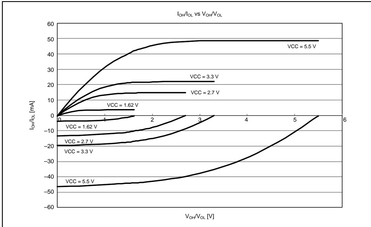
Figure 38.7 V<sub>OH/V<sub>OL</sub></sub> and I<sub>OH/I<sub>OL</sub></sub> Voltage Characteristics at T<sub>a</sub> = 25°C when Normal Output is Selected (Reference Data)
