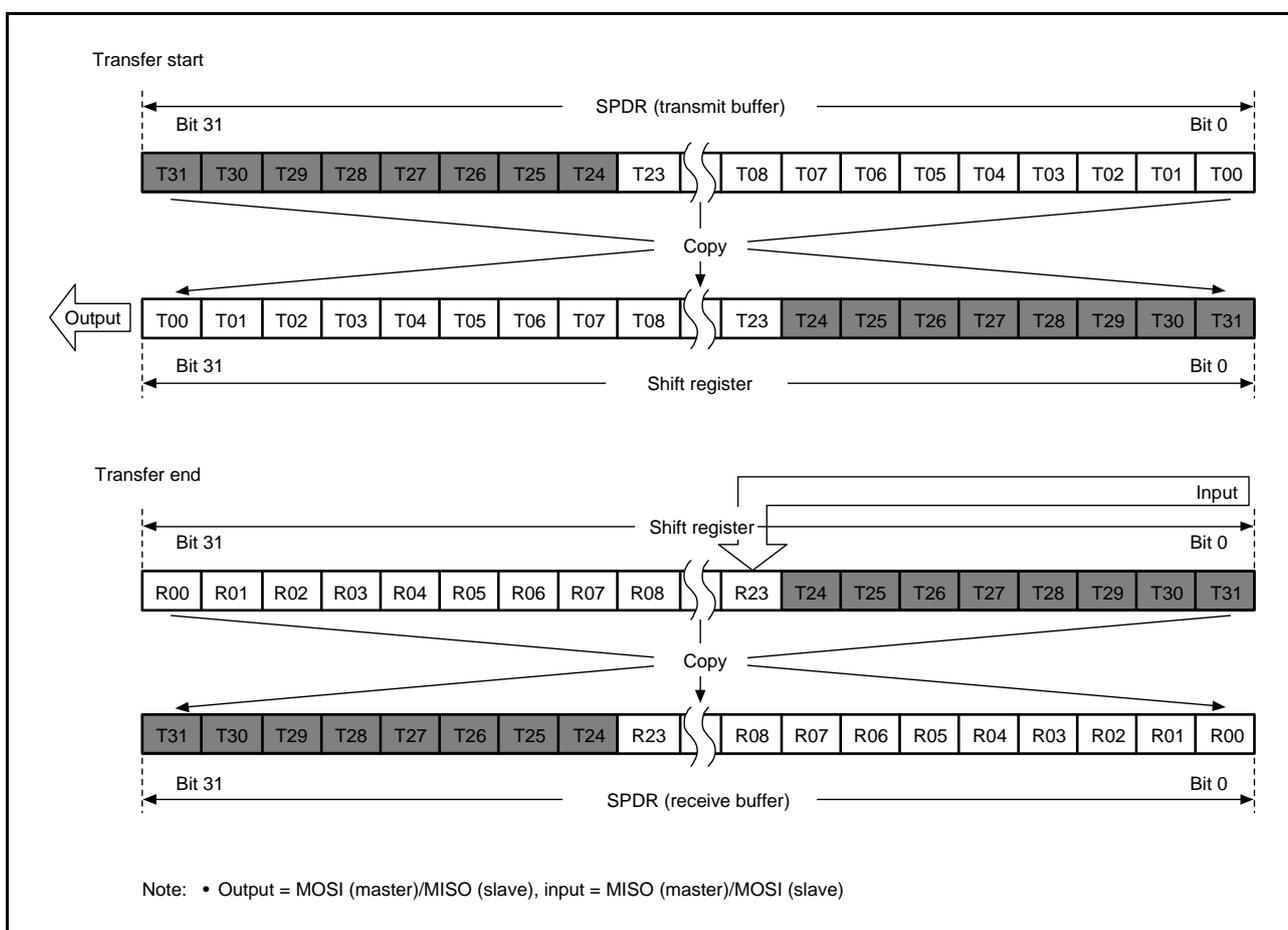
Figure 30.18 LSB-First Transfer (24-Bit Data, Parity Disabled)
