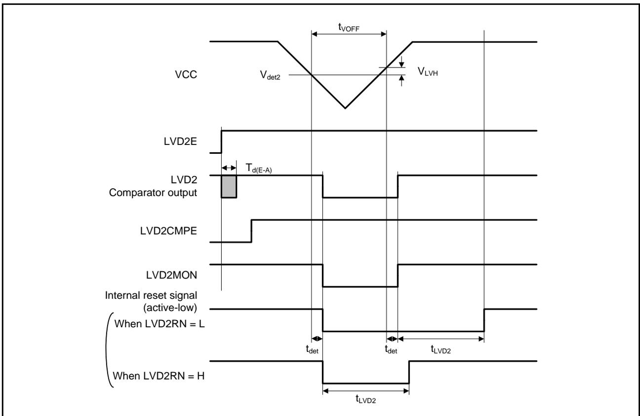
Figure 38.55 Voltage Detection Circuit Timing ( $V_{det2}$ )
