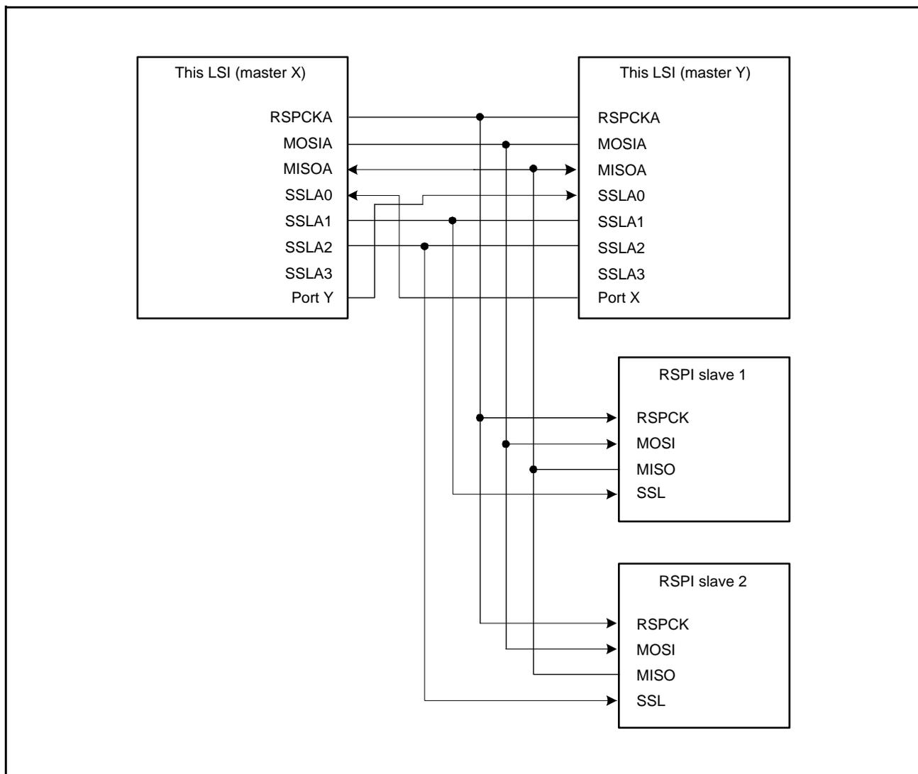
Figure 30.10 Multi-Master/Multi-Slave Configuration Example (This LSI = Master)
