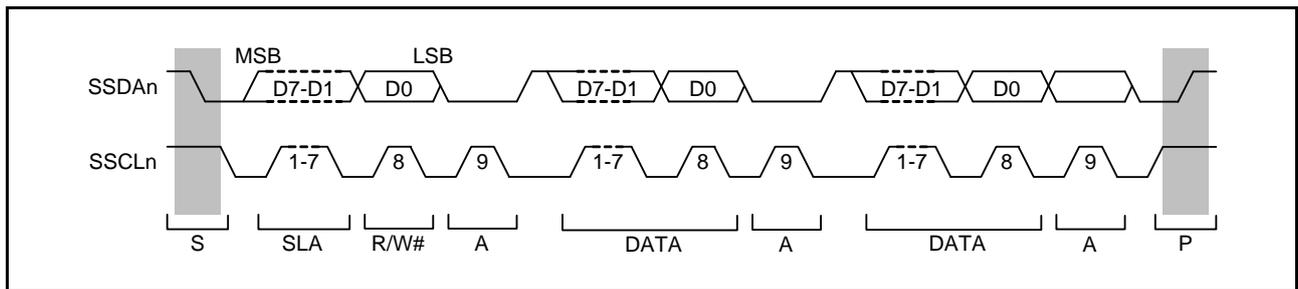
Figure 27.41 I<sup>2</sup>C Bus Timing (When SLA is 7 Bits)
