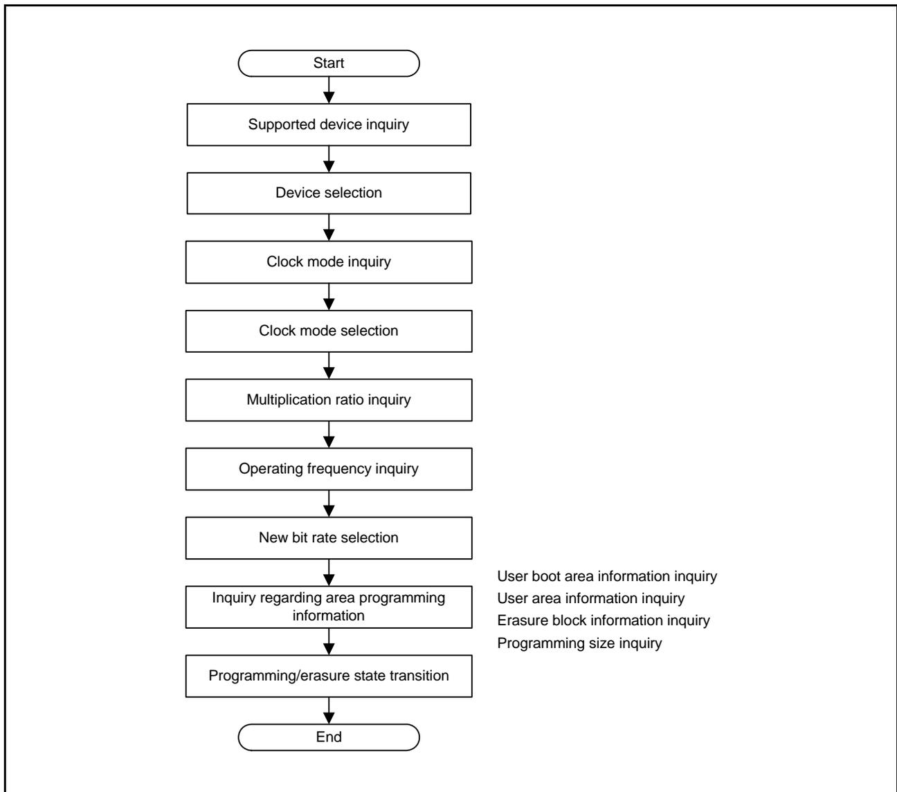
**Figure 36.26 Example of Procedure to Use Inquiry/Selection Commands for User Area/User Boot Area**
