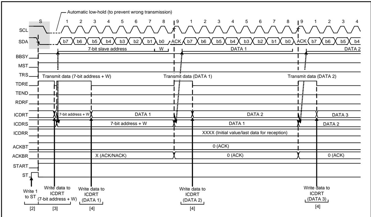
Figure 29.7 Master Transmit Operation Timing (1) (7-Bit Address Format)
