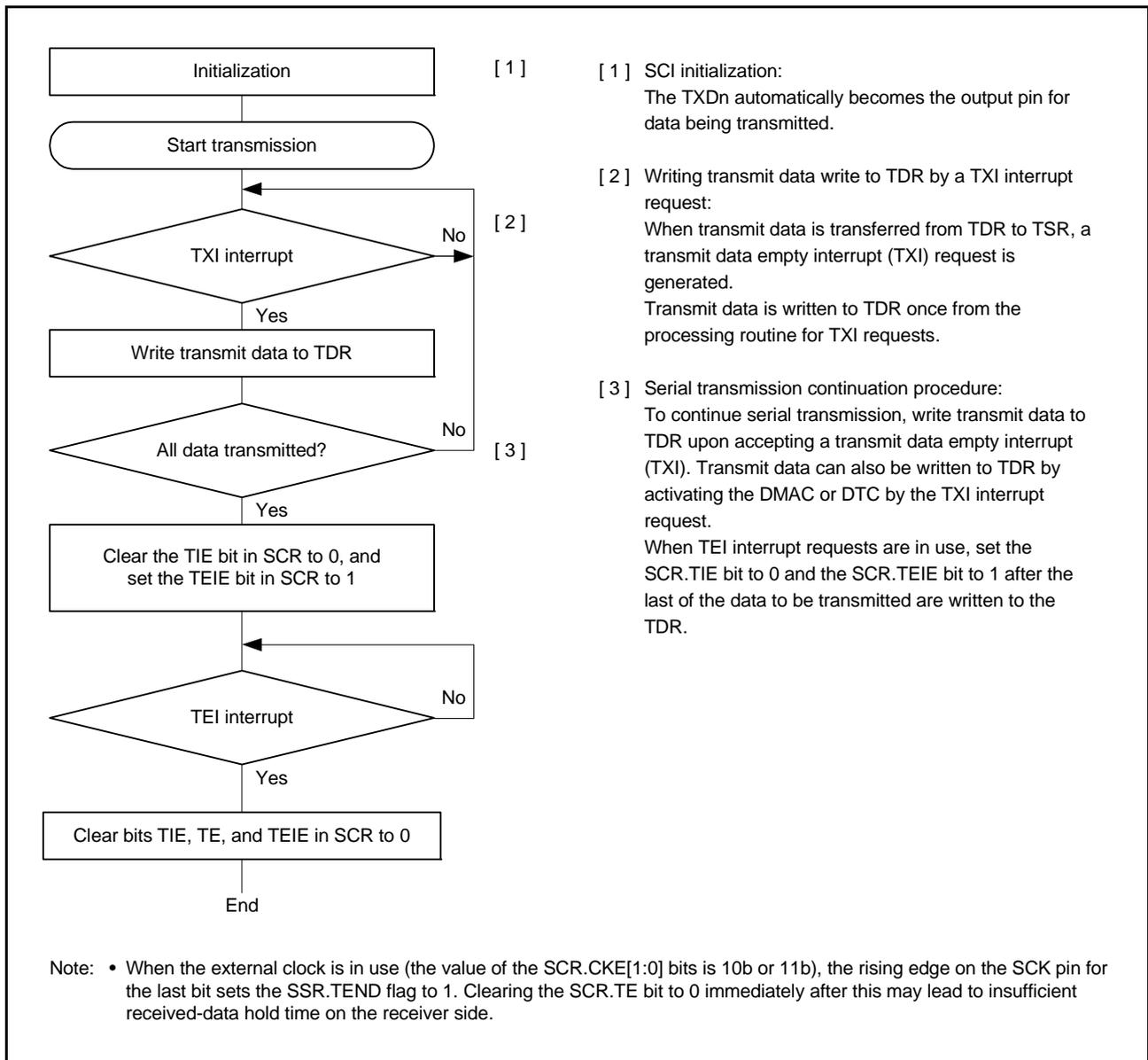
Figure 27.23 Example of Serial Transmission Flowchart (Clock Synchronous Mode)
