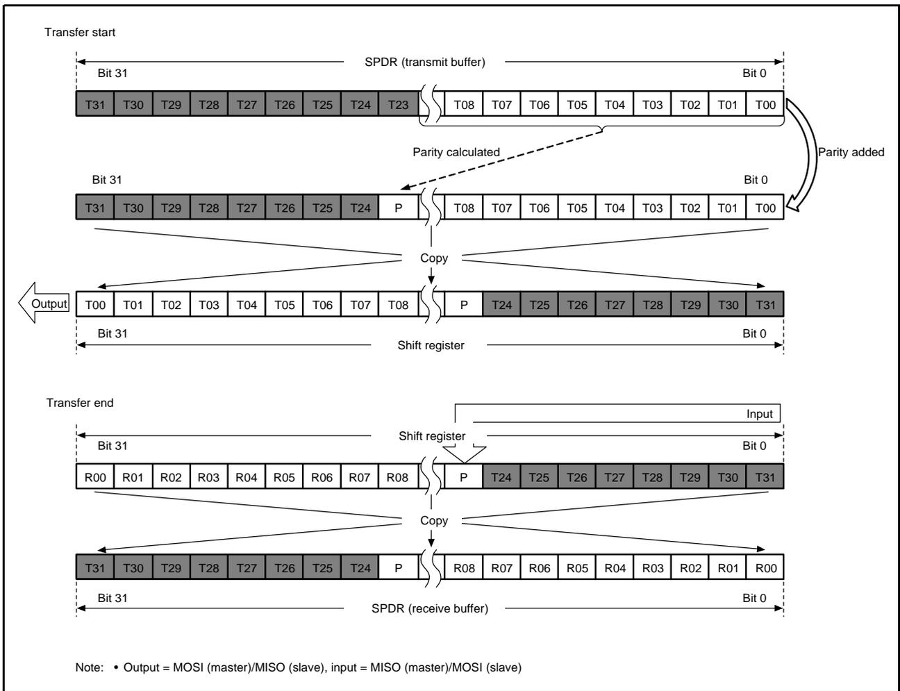
Figure 30.22 LSB-First Transfer (24-Bit Data, Parity Enabled)
