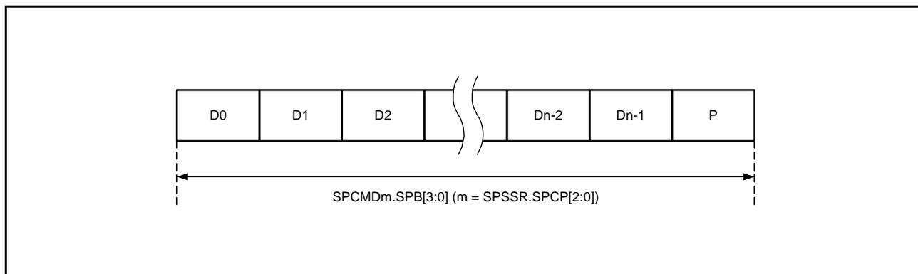
Figure 30.14 Outline of the Data Format (with Parity Enabled)
