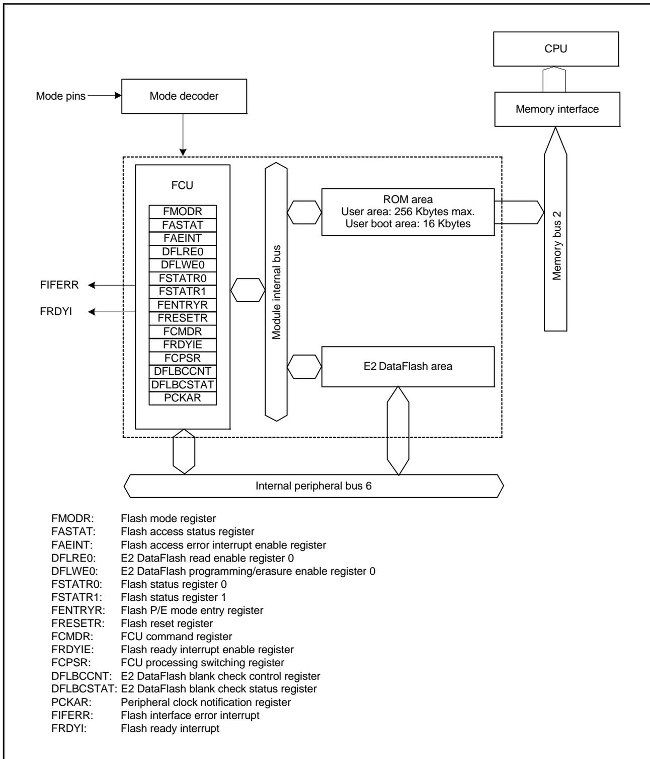
Figure 36.1 Block Diagram of ROM
