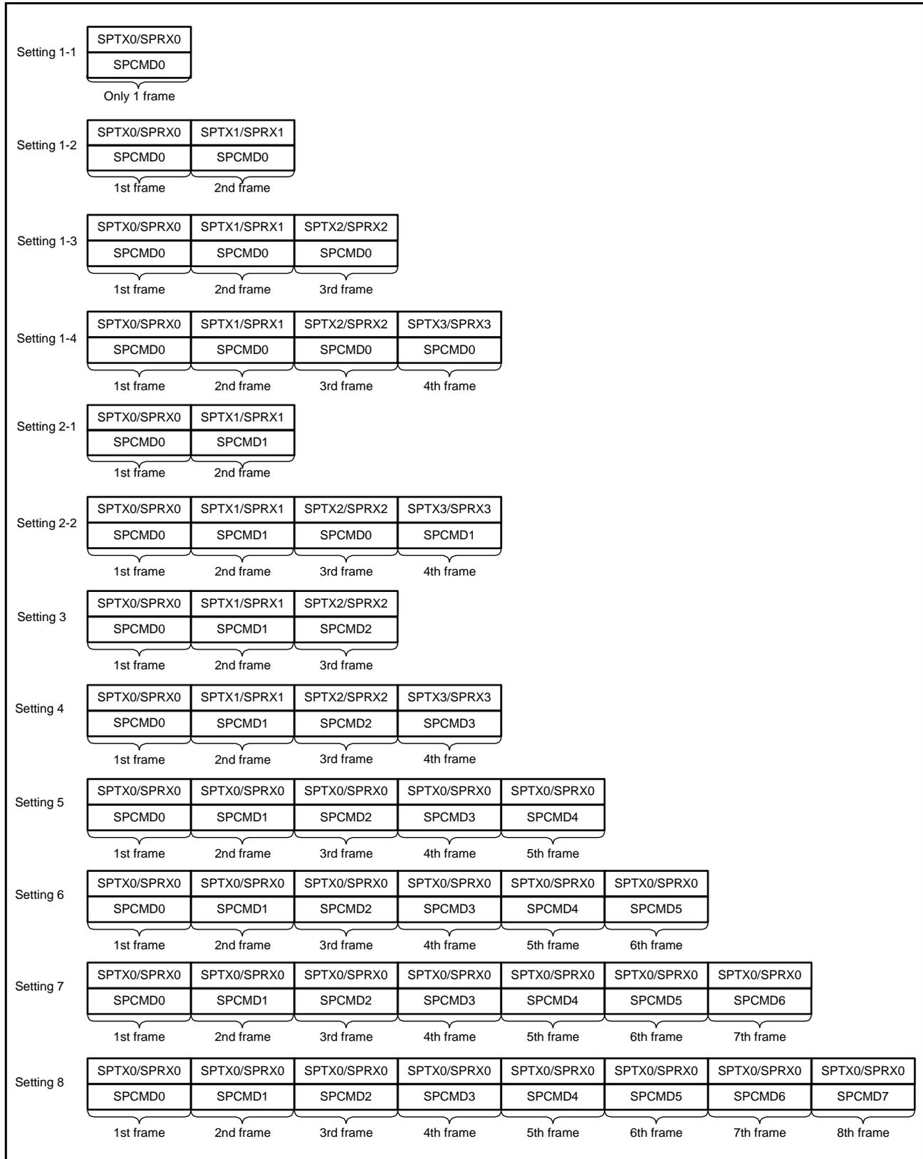
**Figure 30.32 Correspondence between the RSPI Command Register and Transmit/Receive Buffers in Sequence Operations**
