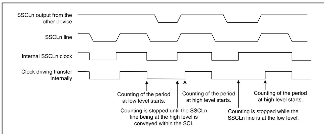
Figure 27.43 Example of Operations for Clock Synchronization
