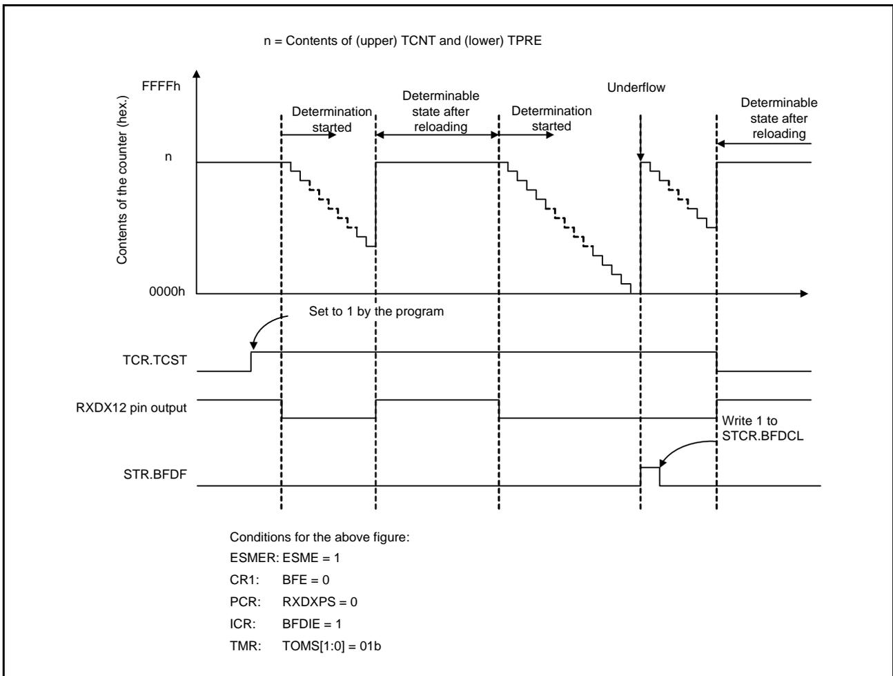
Figure 27.67 Example of Operations in Break Field Low Width Determination Mode
