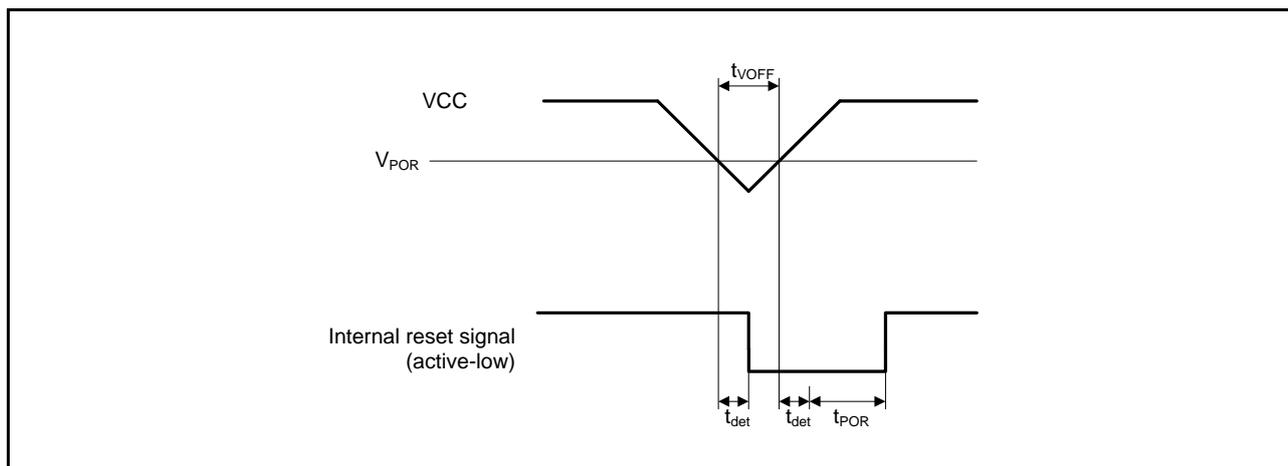
Figure 38.51 Voltage Detection Reset Timing
