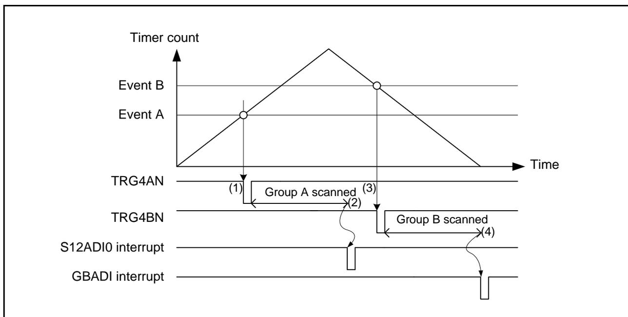
Figure 32.9 Example of Operation in Group Scan Mode (Basic Operation: MTU Triggers Used)
