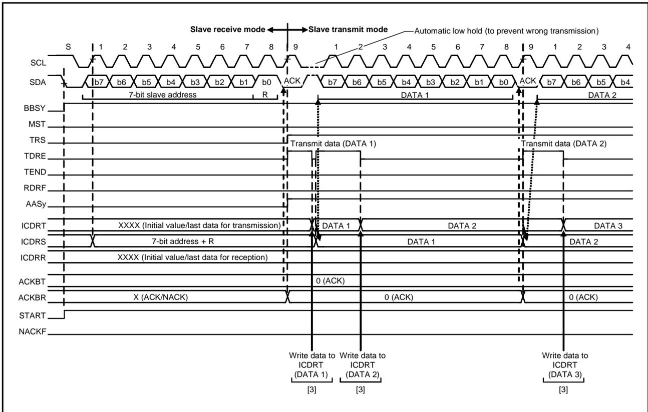
Figure 29.16 Slave Transmit Operation Timing (1) (7-Bit Address Format)
