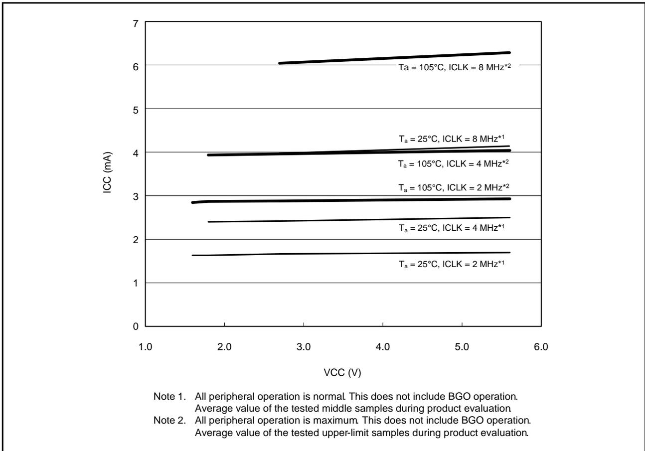
**Figure 38.2 Voltage Dependency in Low-Speed Operating Mode 1 (Reference Data)**
