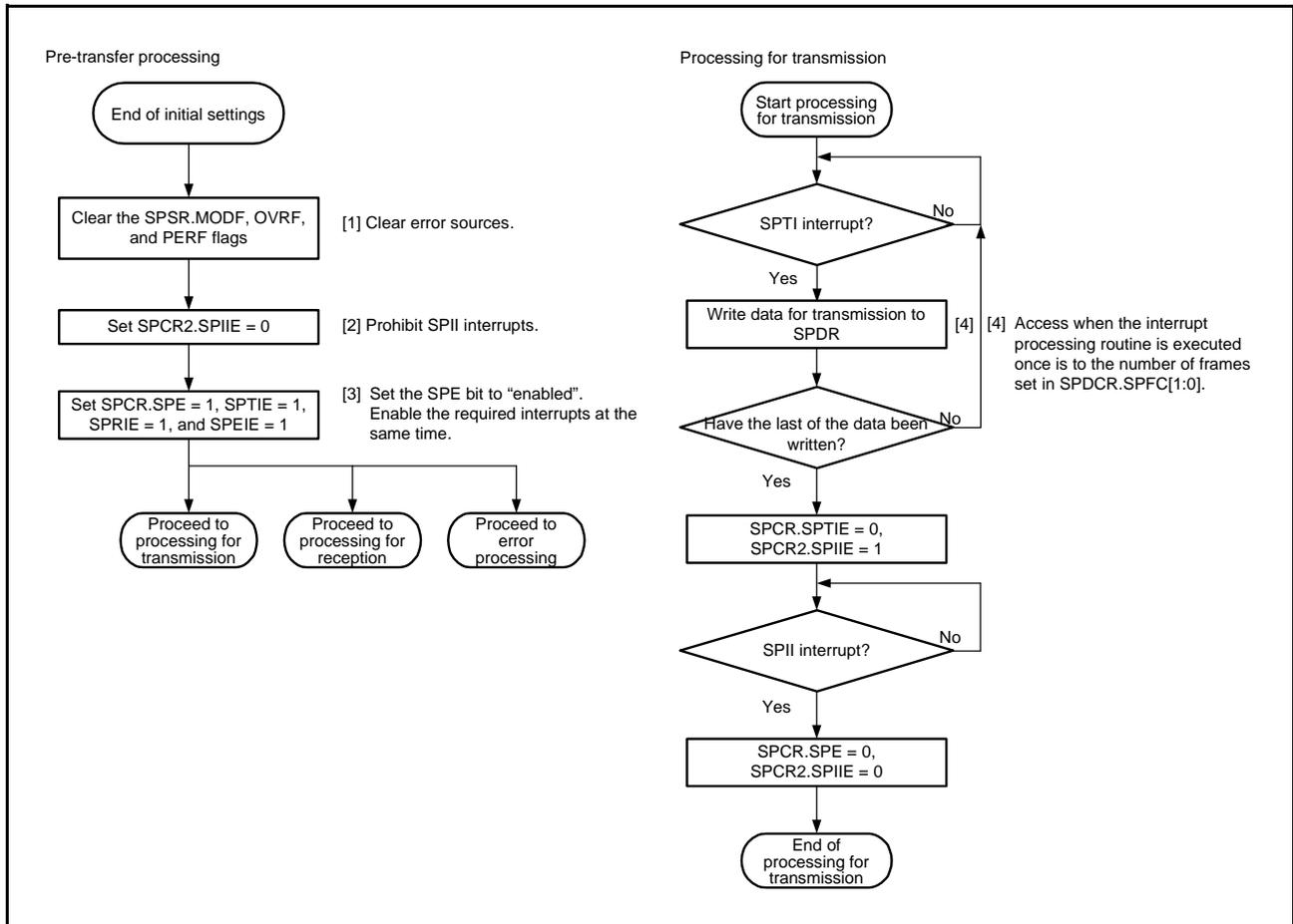
Figure 30.35 Flowchart in Master Mode (Transmission)
