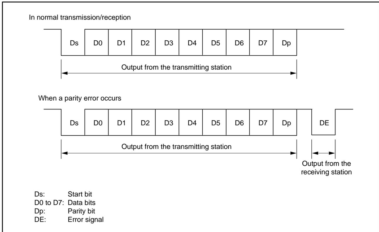
Figure 27.29 Data Formats in Smart Card Interface Mode
