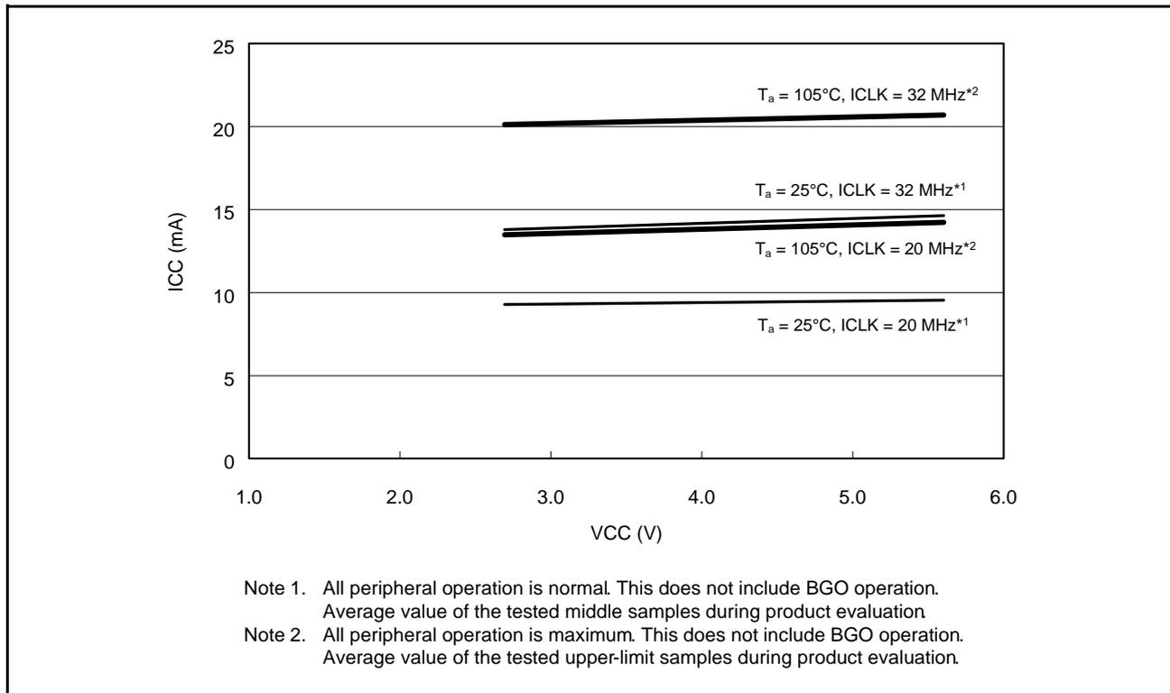
**Figure 38.1 Voltage Dependency in Medium-Speed Operating Modes 1A and 1B (Reference Data)**
