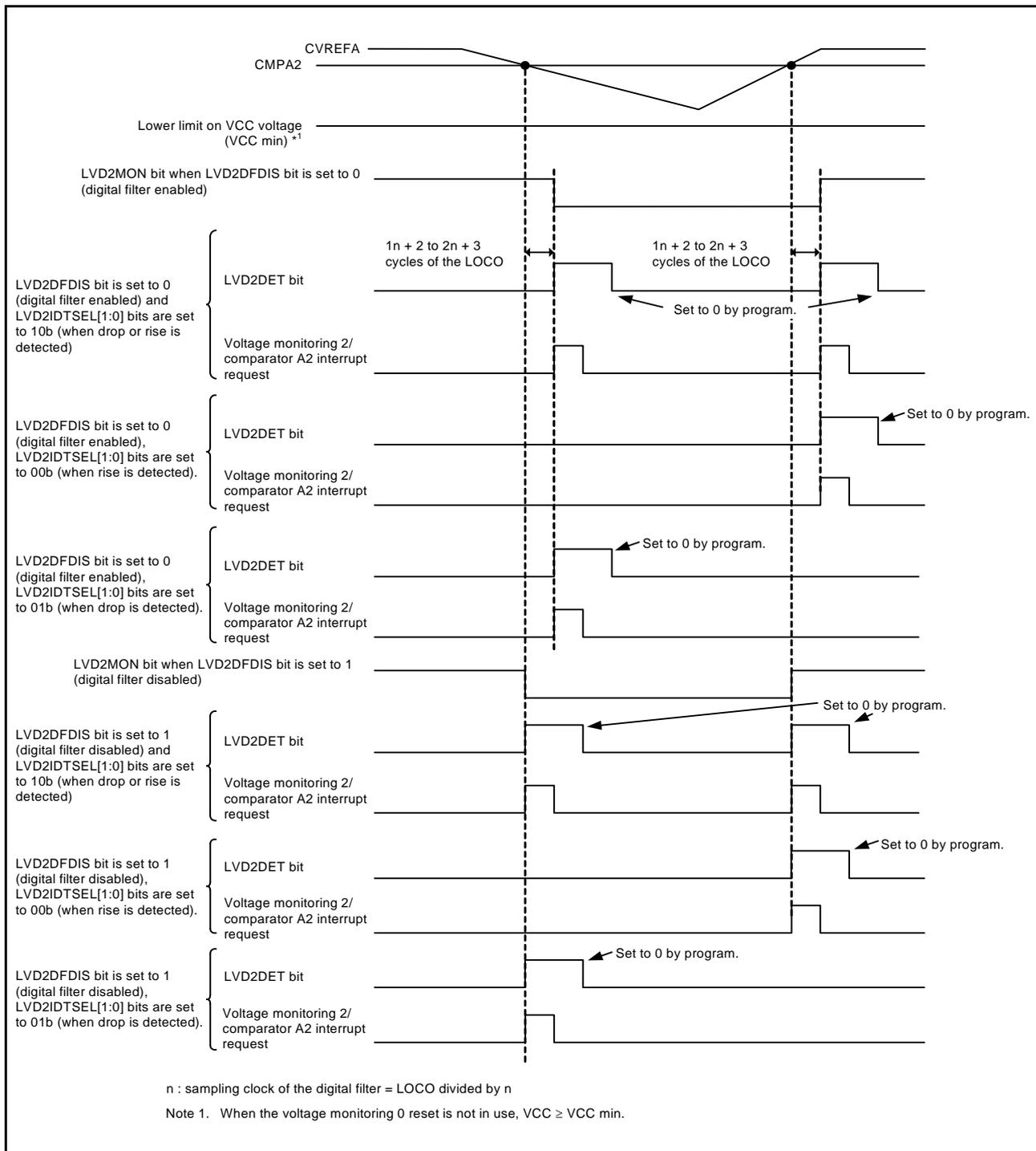
Figure 33.3 Operating Example of Comparator A2
