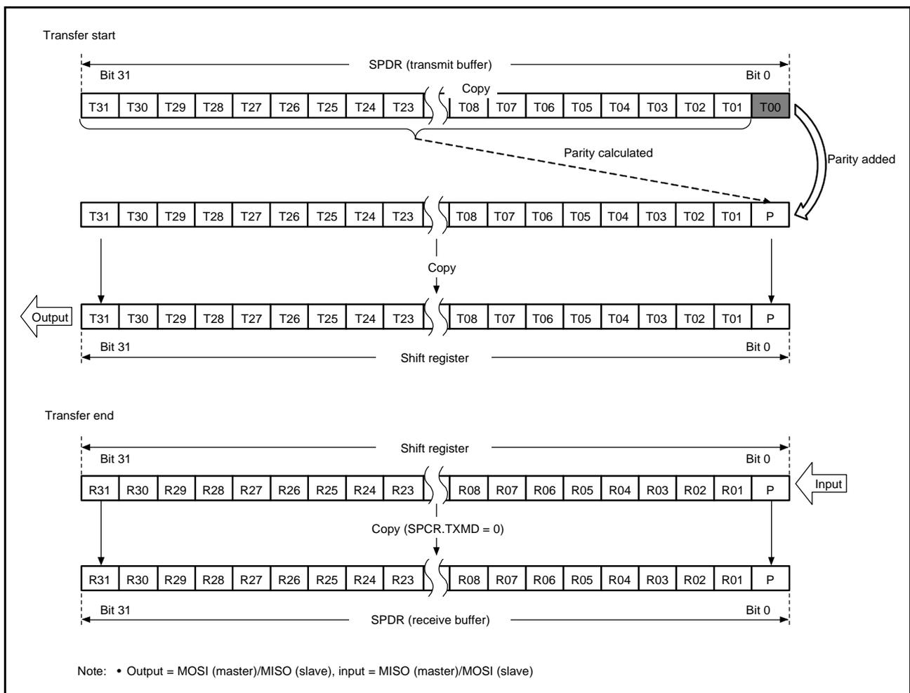
Figure 30.19 MSB-First Transfer (32-Bit Data, Parity Enabled)
