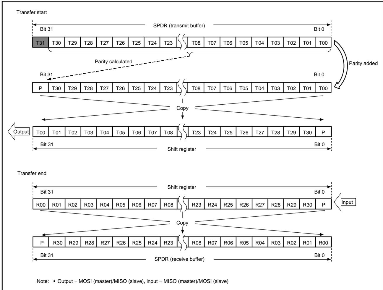
Figure 30.21 LSB-First Transfer (32-Bit Data, Parity Enabled)
