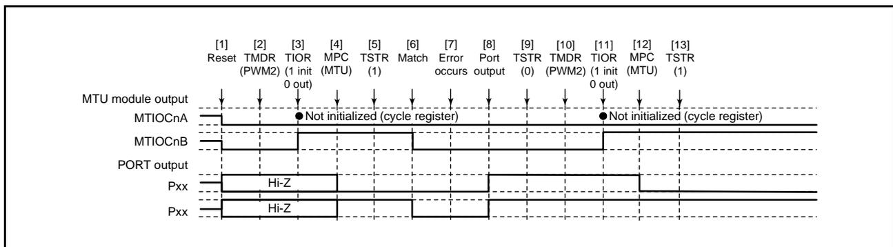
Figure 21.139 Error Occurrence in PWM Mode 2, Recovery in PWM Mode 2
