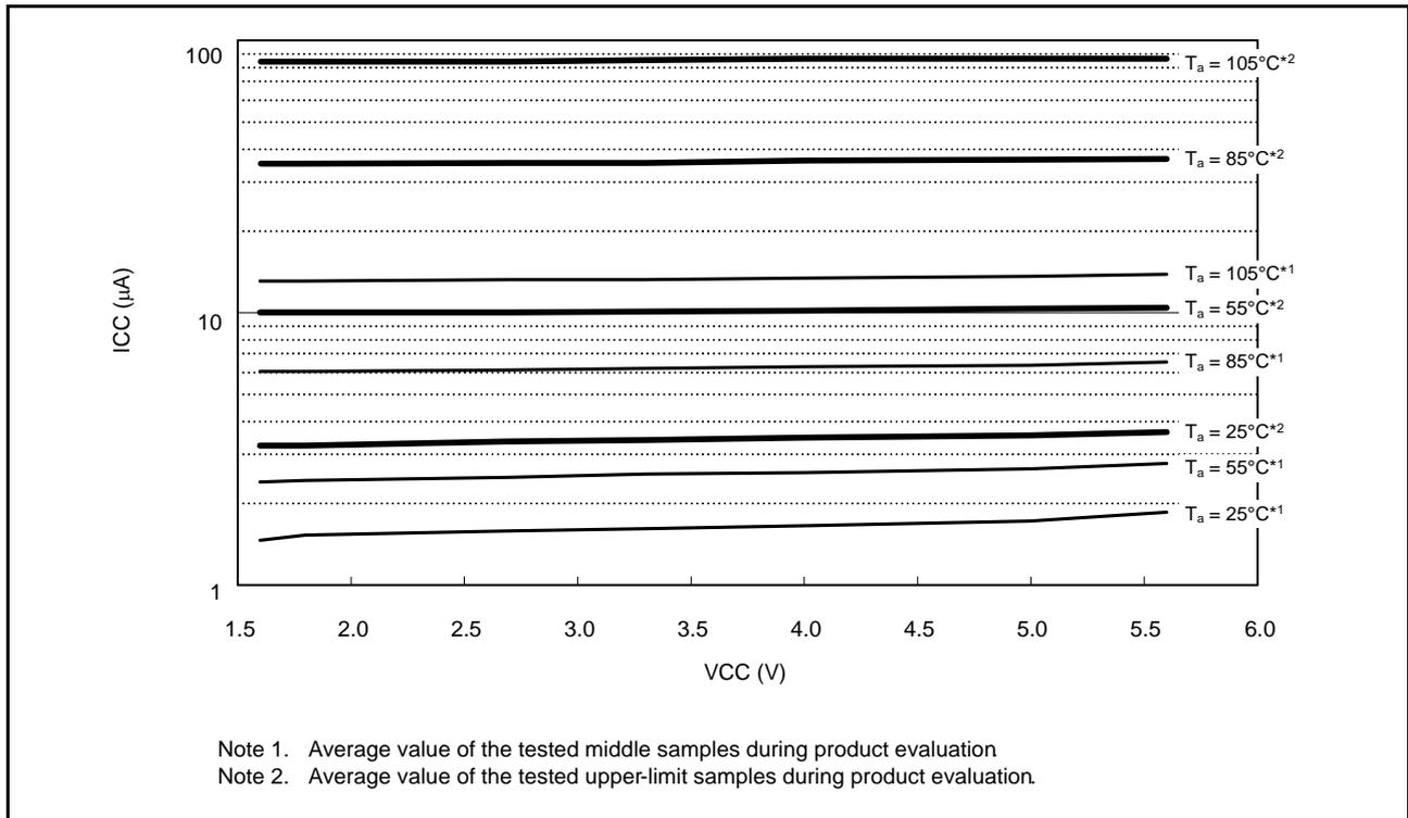
Figure 38.4 Voltage Dependency in Software Standby Mode (SOFTCUT Bit = 11xb) (Reference Data)
