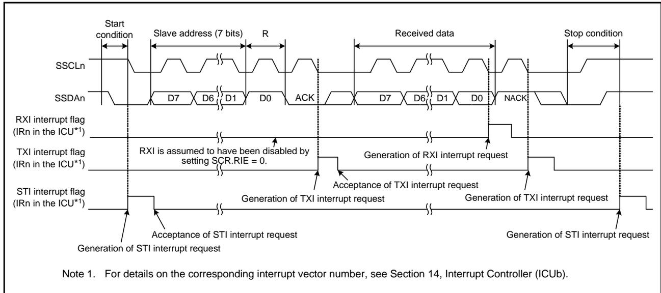
**Figure 27.49 Example of Operations for Master Reception in I<sup>2</sup>C Bus Mode (with Seven-Bit Slave Addresses, Transmission Interrupts, and Reception Interrupts in Use)**
