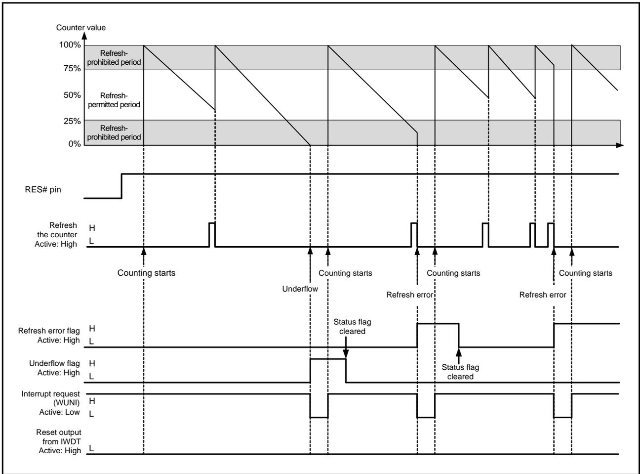
Figure 26.4 Operation Example in Auto-Start Mode
