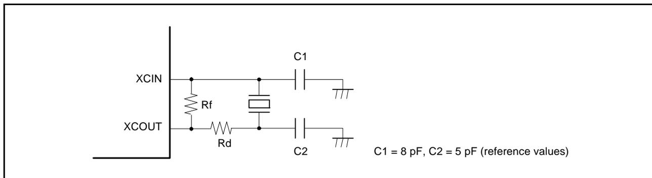
Figure 9.5 Connection Example of 32.768-kHz Crystal Resonator
