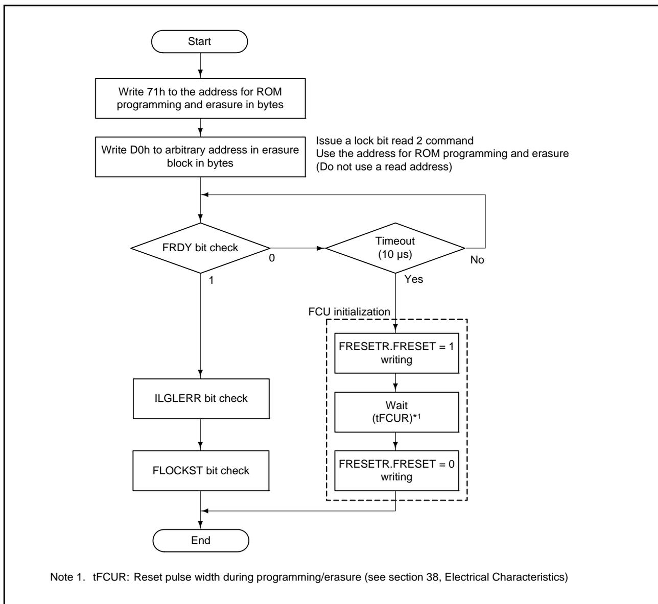
Figure 36.15 Procedure for Reading Lock Bit in Register Read Mode
