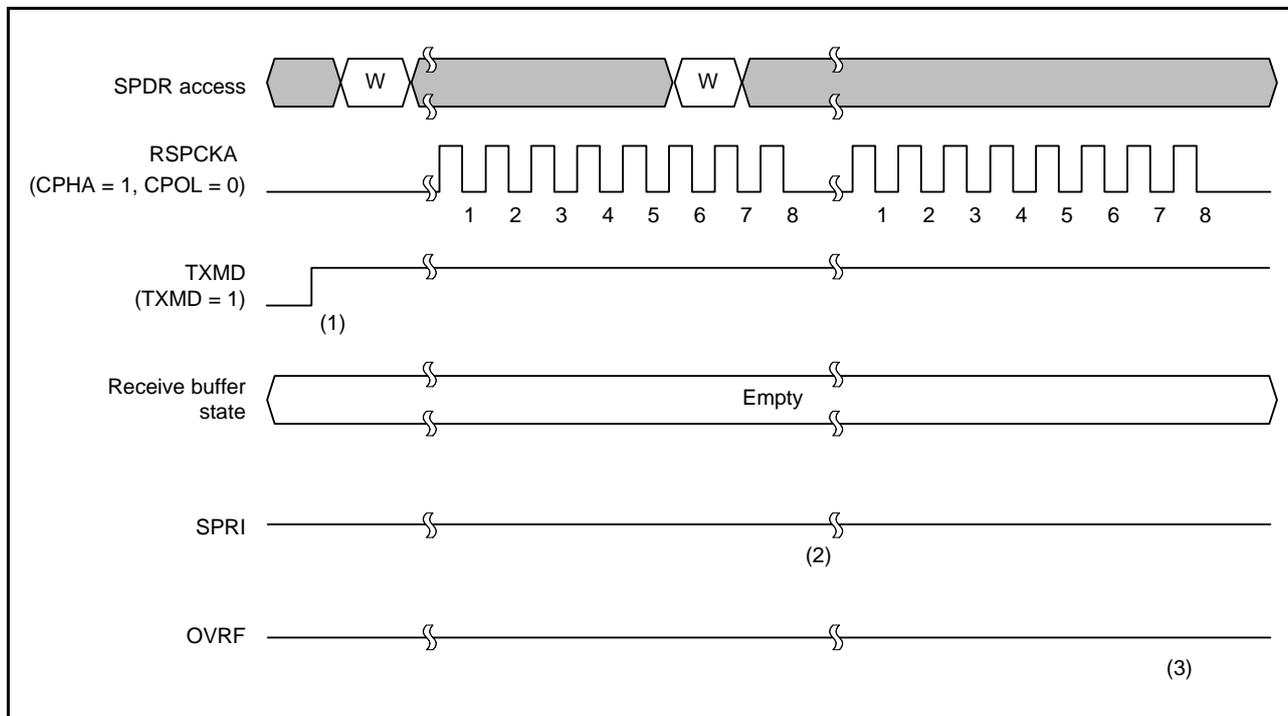
**Figure 30.26** Operation Example of SPCR.TXMD = 1
