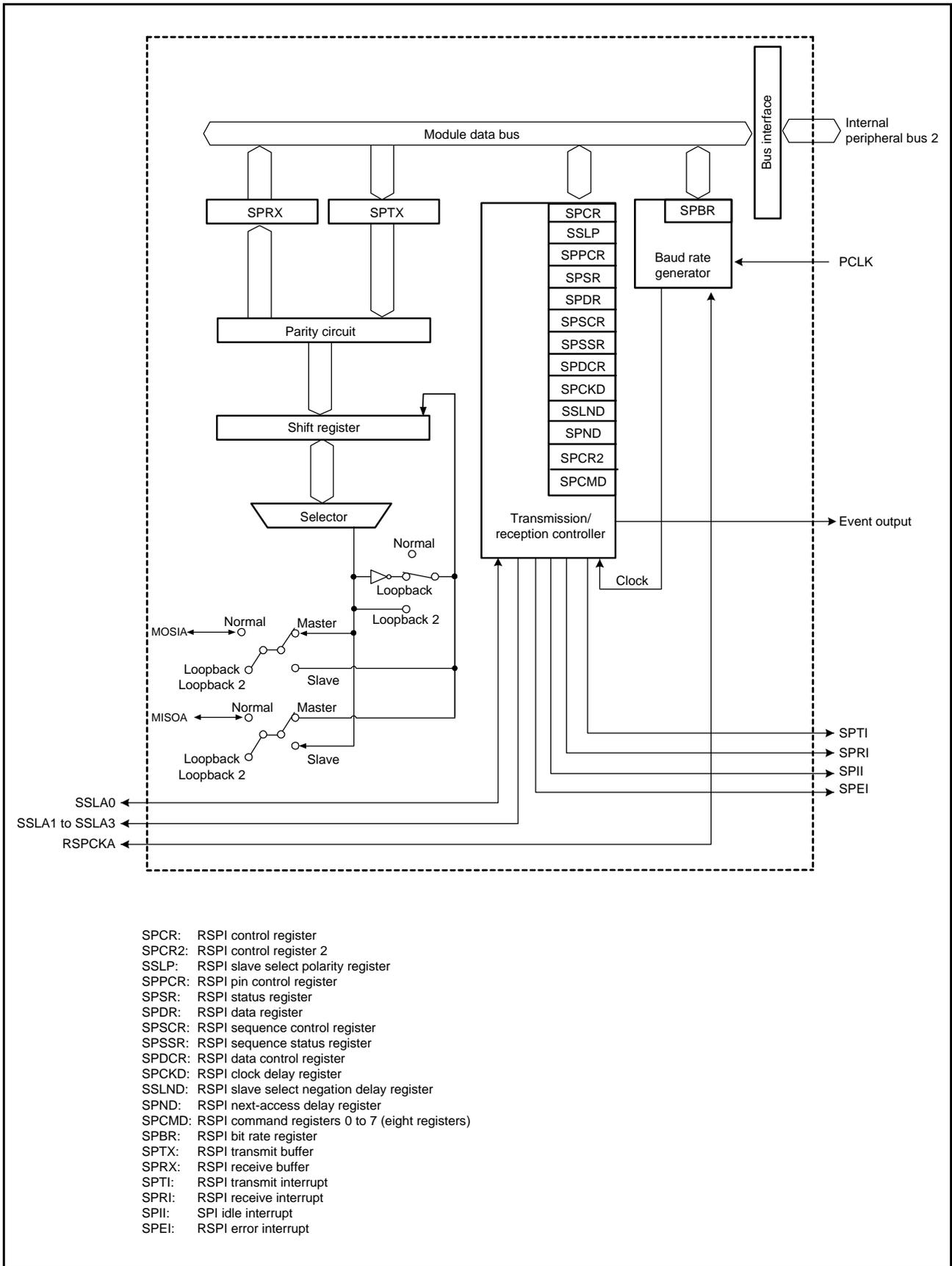
Figure 30.1 Block Diagram of RSPI
