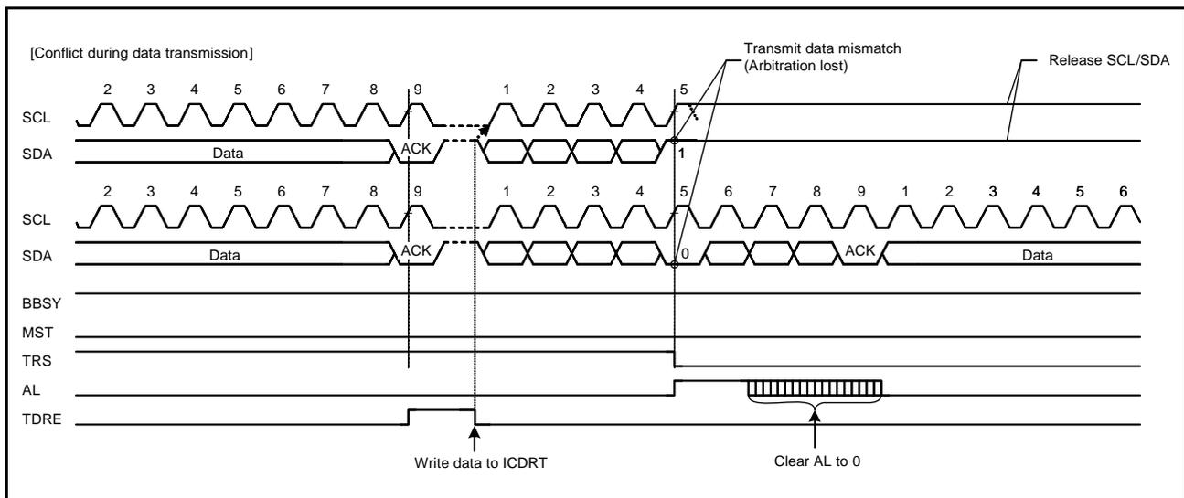
Figure 29.36 Example of Slave Arbitration-Lost Detection (SALE = 1)
