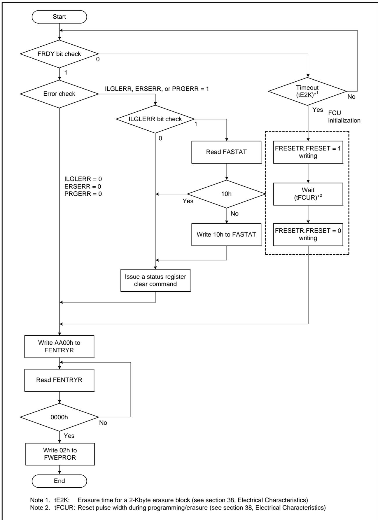
Figure 36.6 Procedure for Transition to ROM Read Mode
