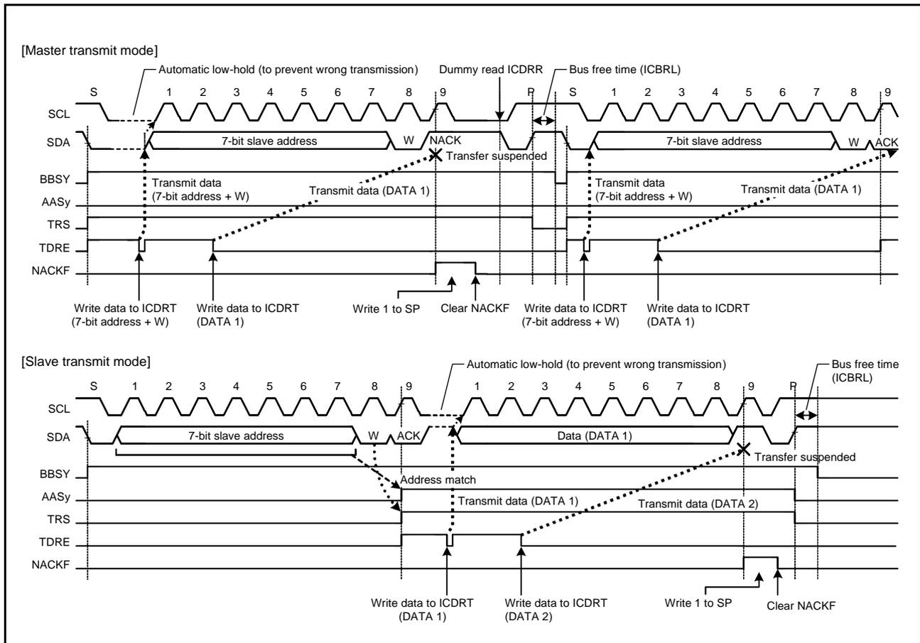
Figure 29.31 Suspension of Data Transfer when NACK is Received (NACKEN = 1)
