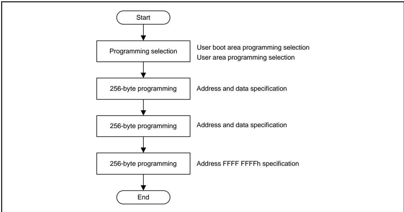
**Figure 36.28 Procedure for ROM Programming in Boot Mode**
