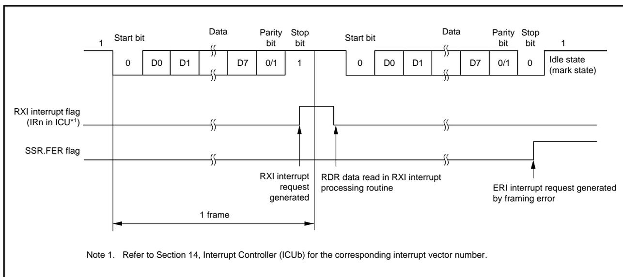
**Figure 27.11 Example of SCI Operation for Serial Reception in Asynchronous Mode (1)
