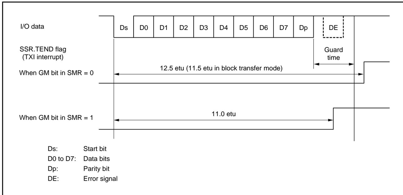
Figure 27.34 SSR.TEND Flag Generation Timing during Transmission
