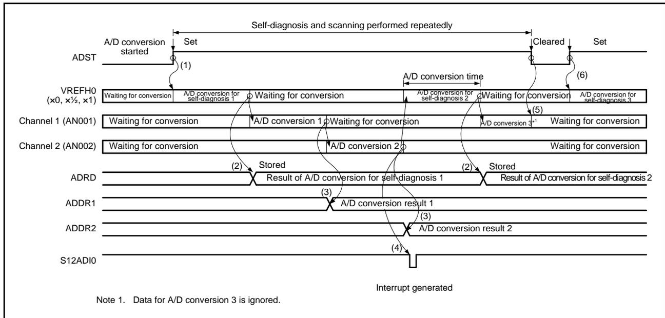
Figure 32.8 Example of Operation in Continuous Scan Mode (Basic Operation + Self-Diagnosis)
