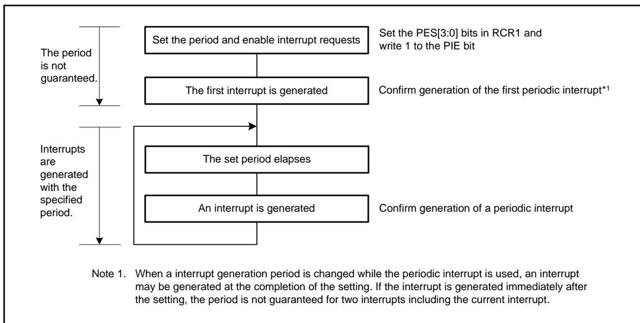
Figure 25.11 Using Periodic Interrupt Function
