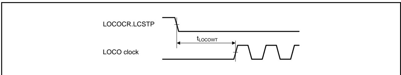
Figure 38.23 LOCO Clock Oscillation Start Timing
