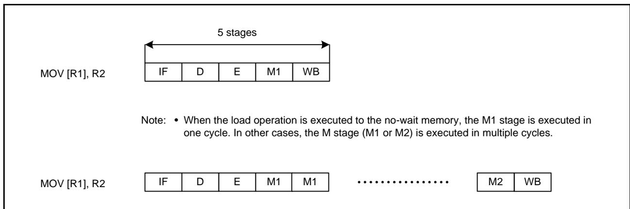
**Figure 2.8 Load Operation**
