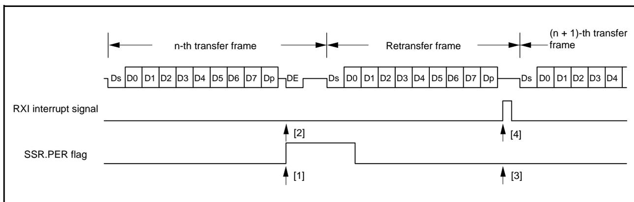
Figure 27.36 Data Retransfer Operation in SCI Reception Mode
