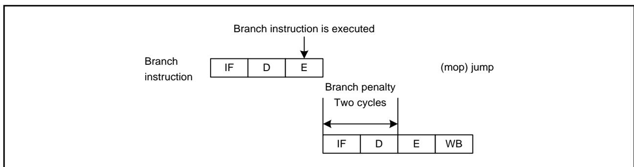
Figure 2.17 When a Branch Instruction is Executed (an Unconditional Branch Instruction is Executed or the Condition is Satisfied for a Conditional Branch Instruction)
