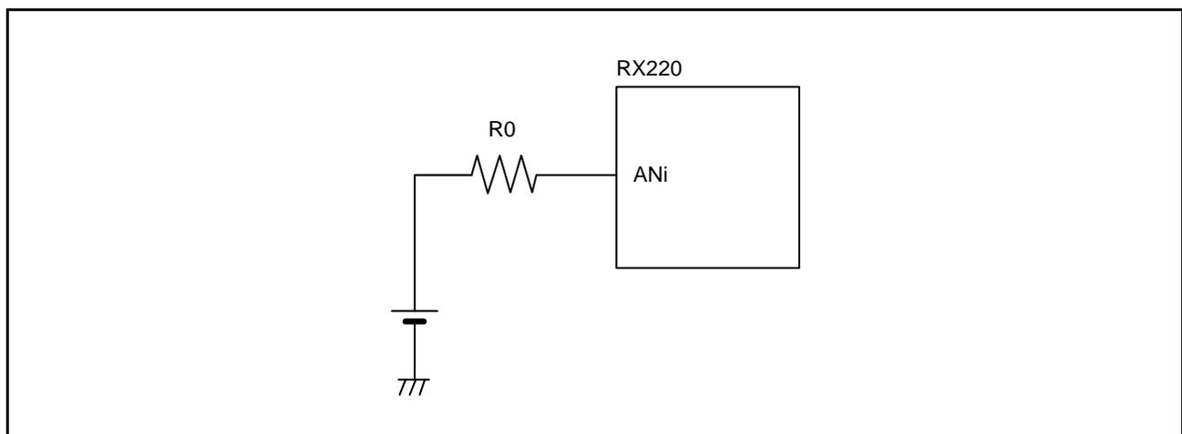
**Figure 38.49 Internal Equivalent Circuit of Analog Input Pin**
