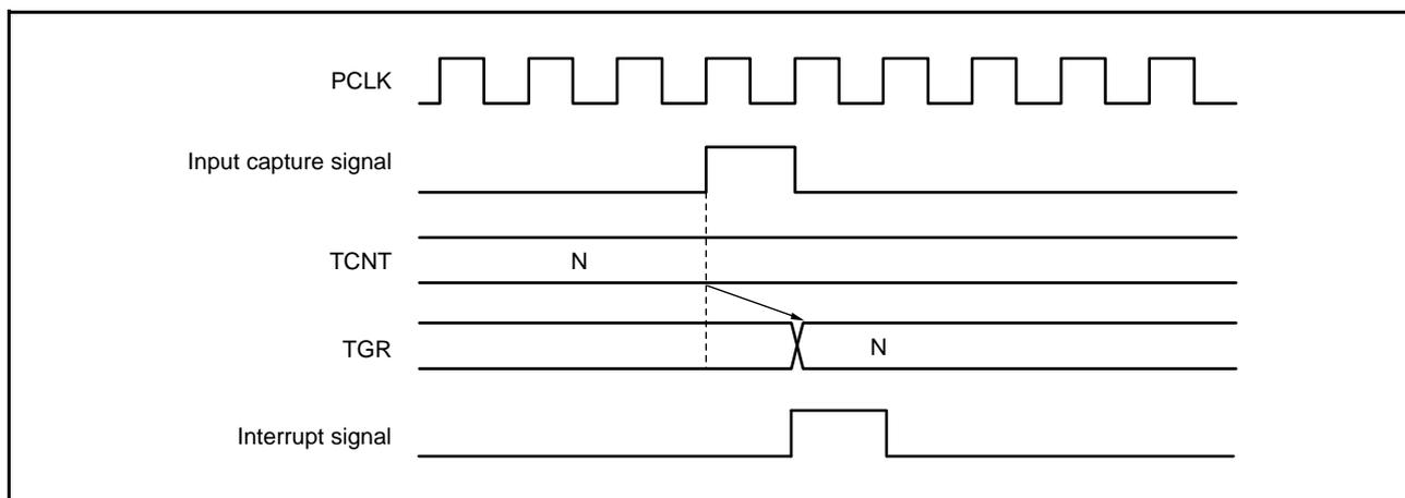
Figure 21.103 TGI Interrupt Timing (Input Capture) (MTU5)
