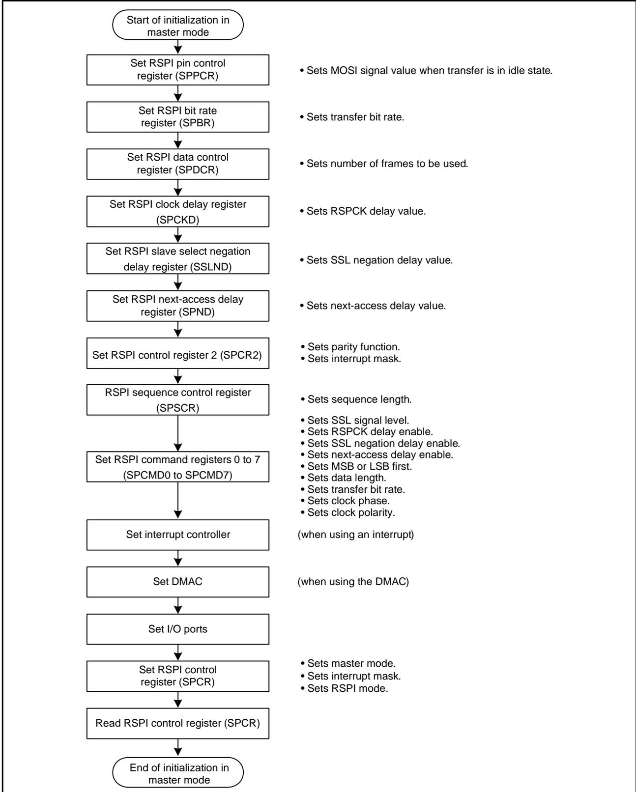
Figure 30.34 Example of Initialization Flowchart in Master Mode (SPI Operation)
