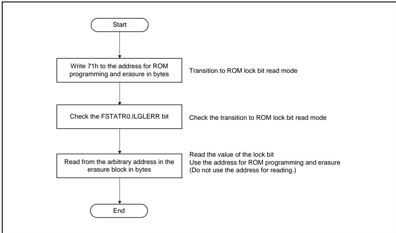
Figure 36.9 Procedure for Transition to ROM Lock-Bit Read Mode and Lock-Bit Reading
