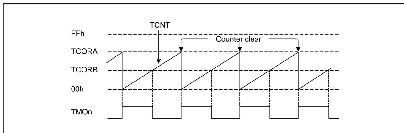
Figure 23.3 Example of Pulse Output (n = 0 to 3)
