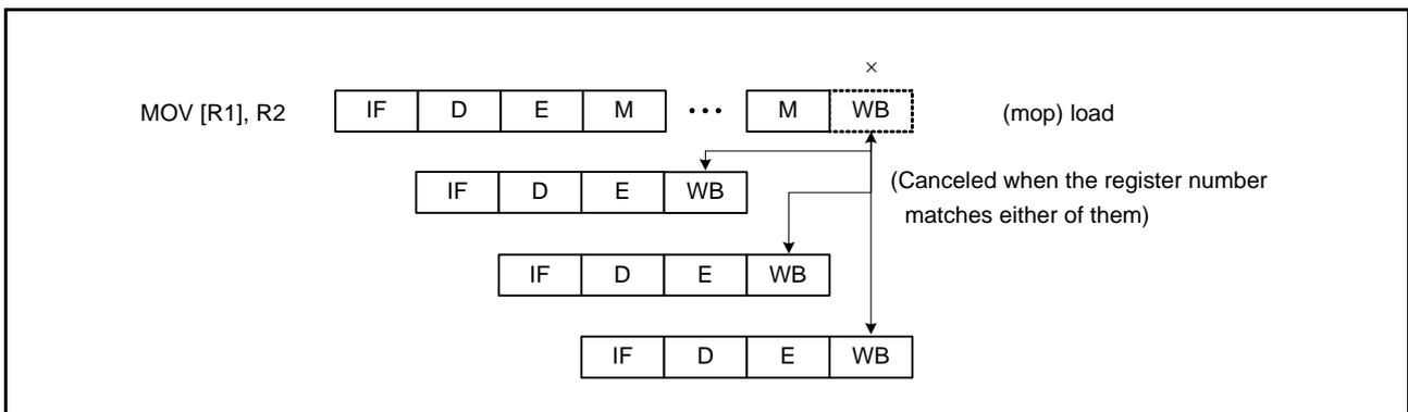
Figure 2.21 When Subsequent Instruction Writes to the Same Register before the End of Memory Load
