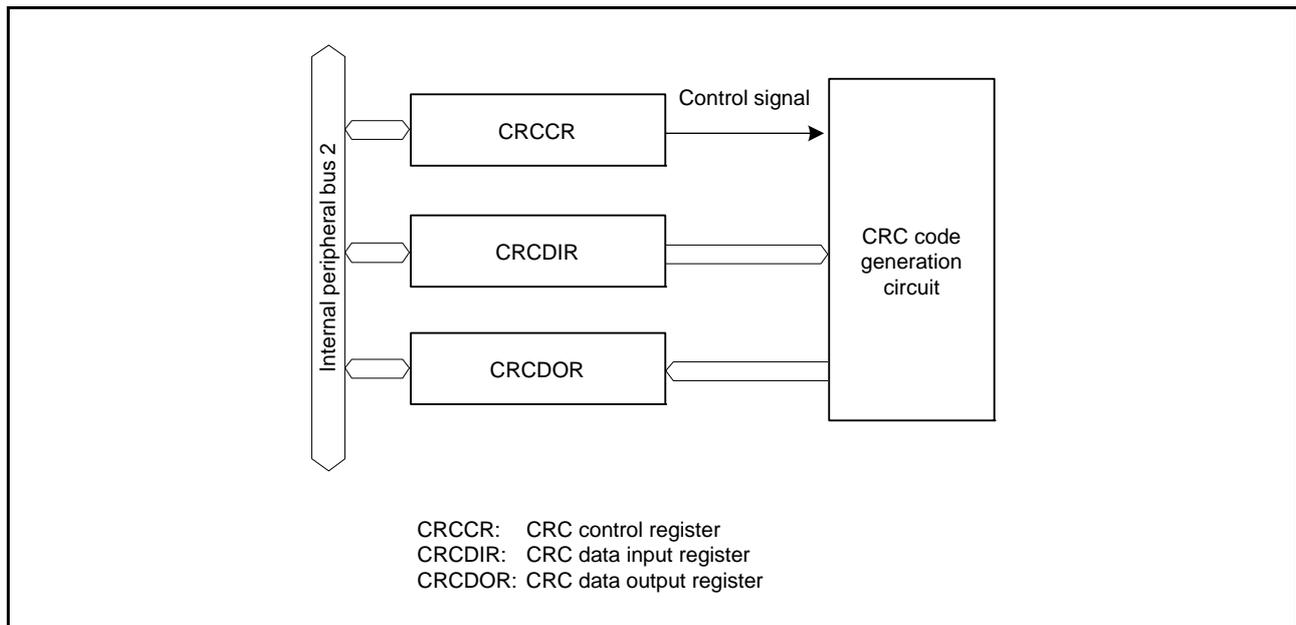
**Figure 31.1 Block Diagram of CRC Calculator**
