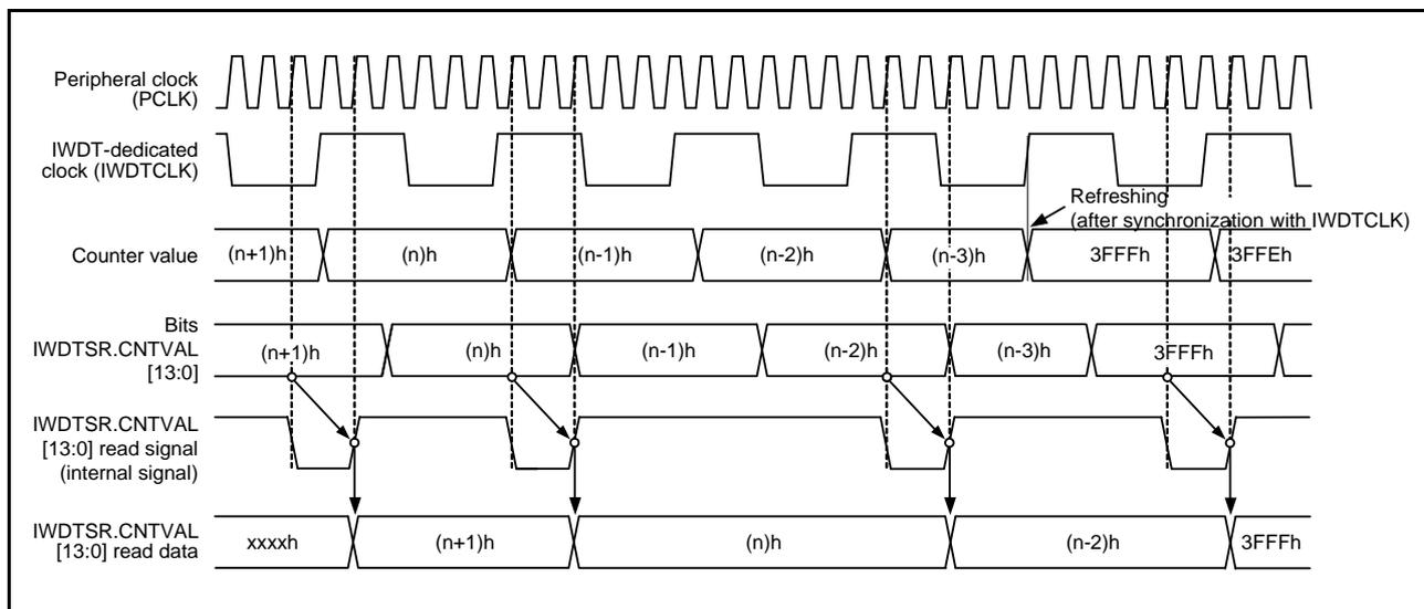
**Figure 26.7 Processing for Reading IWDT Down-Counter Value (IWDTCR.CKS[3:0] = 0000b, IWDTCR.TOPS[1:0] = 11b)**
