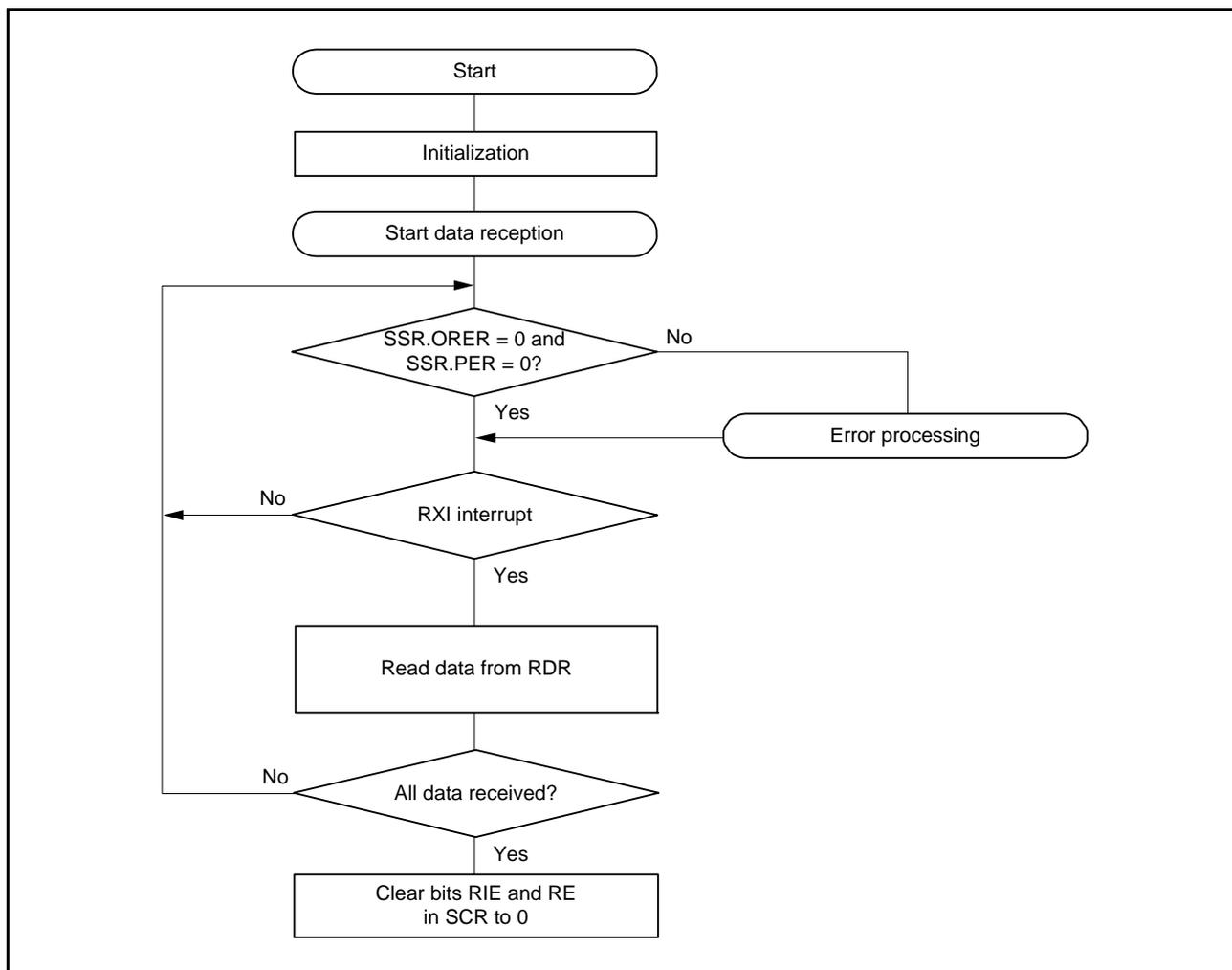
Figure 27.37 Sample Smart Card Interface Reception Flowchart
