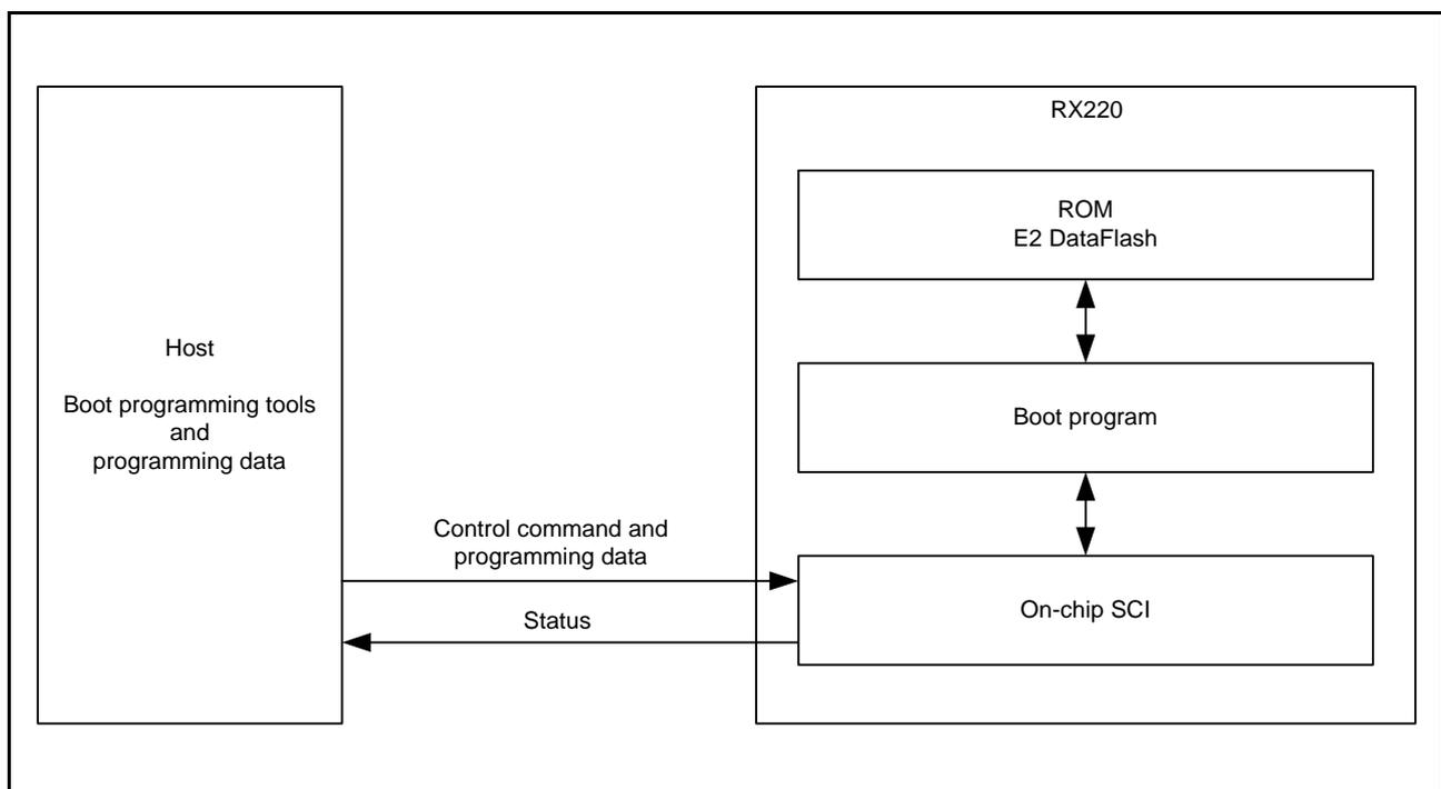
Figure 36.21 System Configuration for Operations in Boot Mode
