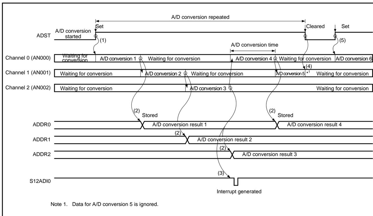
Figure 32.7 Example of Operation in Continuous Scan Mode (Basic Operation: AN000 to AN002 Selected)
