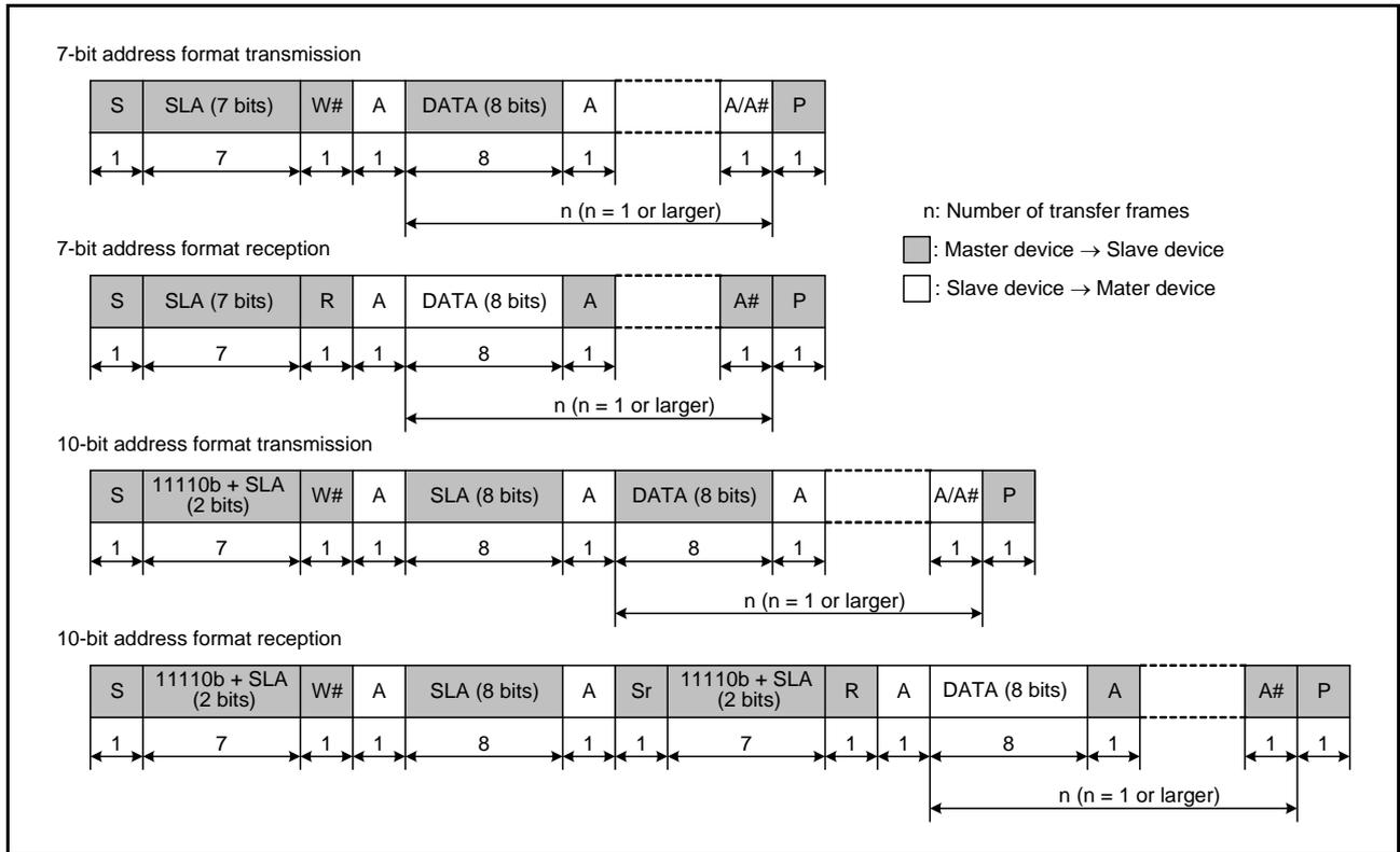
Figure 27.40 I<sup>2</sup>C Bus Master Format
