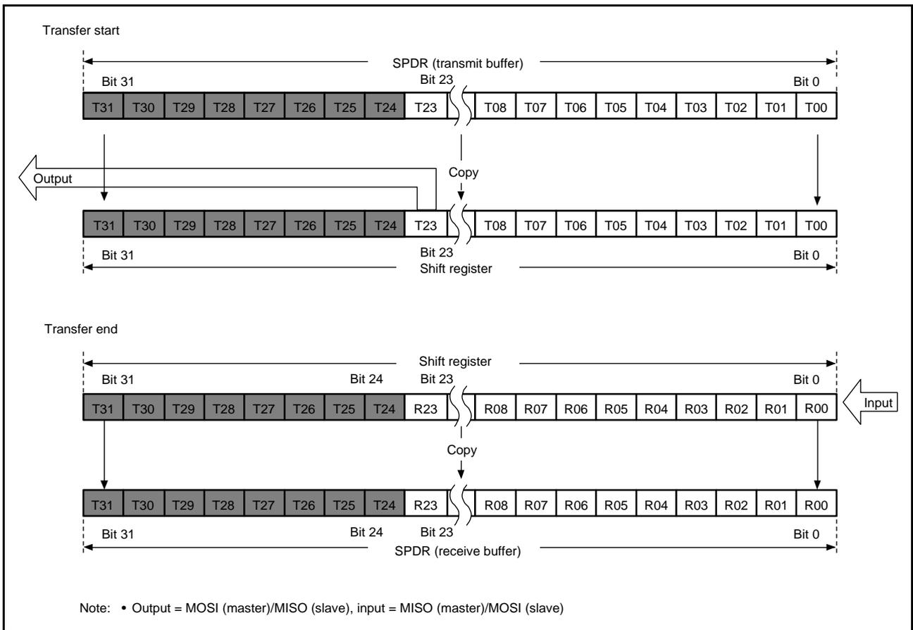
Figure 30.16 MSB-First Transfer (24-Bit Data, Parity Disabled)
