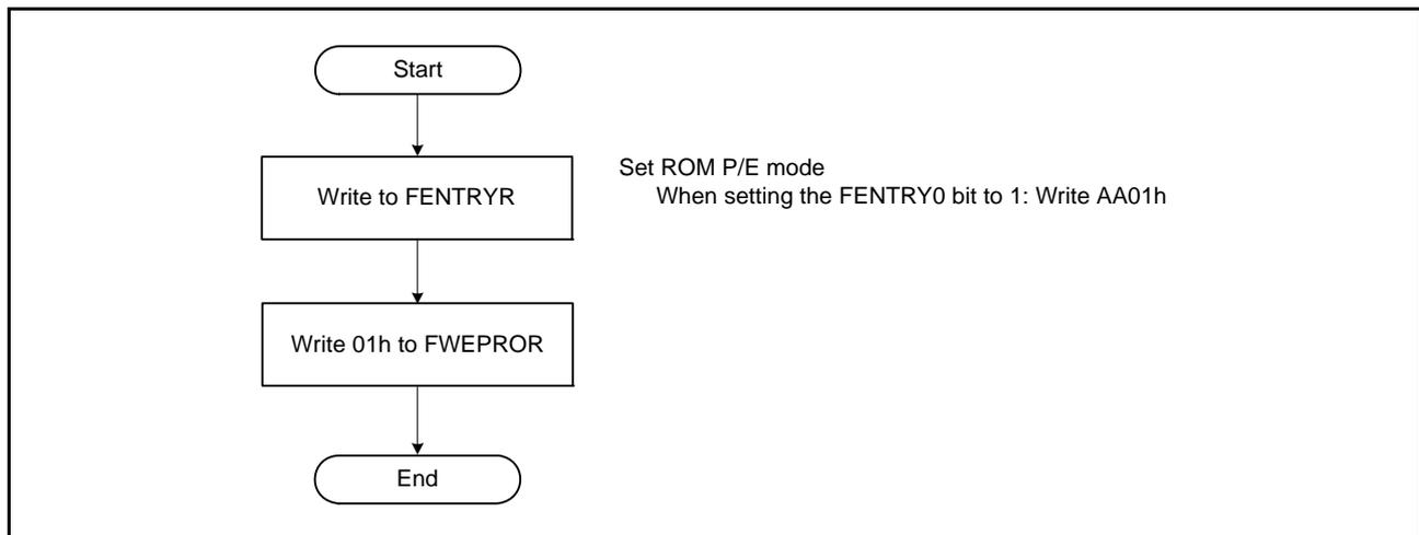
**Figure 36.5 Procedure for Transition to ROM P/E Mode**
