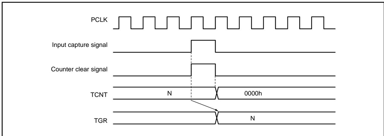
Figure 21.93 Counter Clear Timing (Input Capture) (MTU0 to MTU5)
