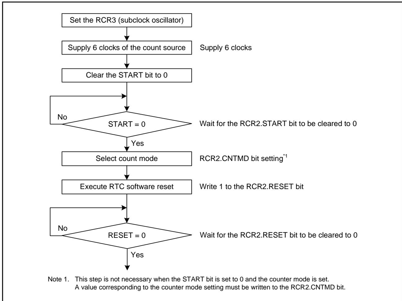
**Figure 25.3** Clock and the count mode Setting Procedure
