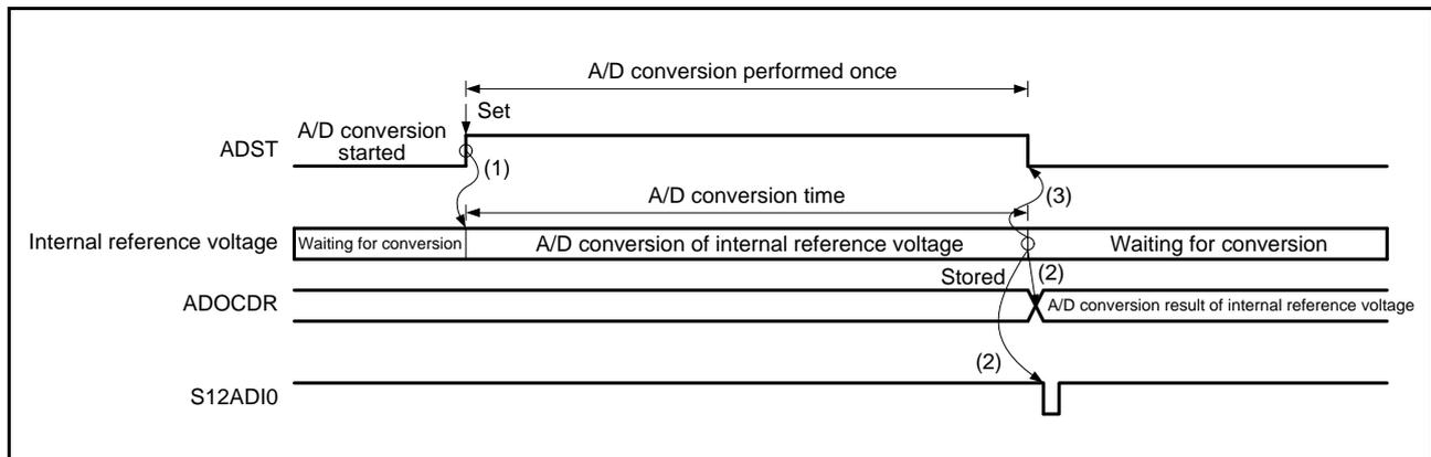
Figure 32.5 Example of Operation in Single Scan Mode (Internal Reference Voltage Selected)
