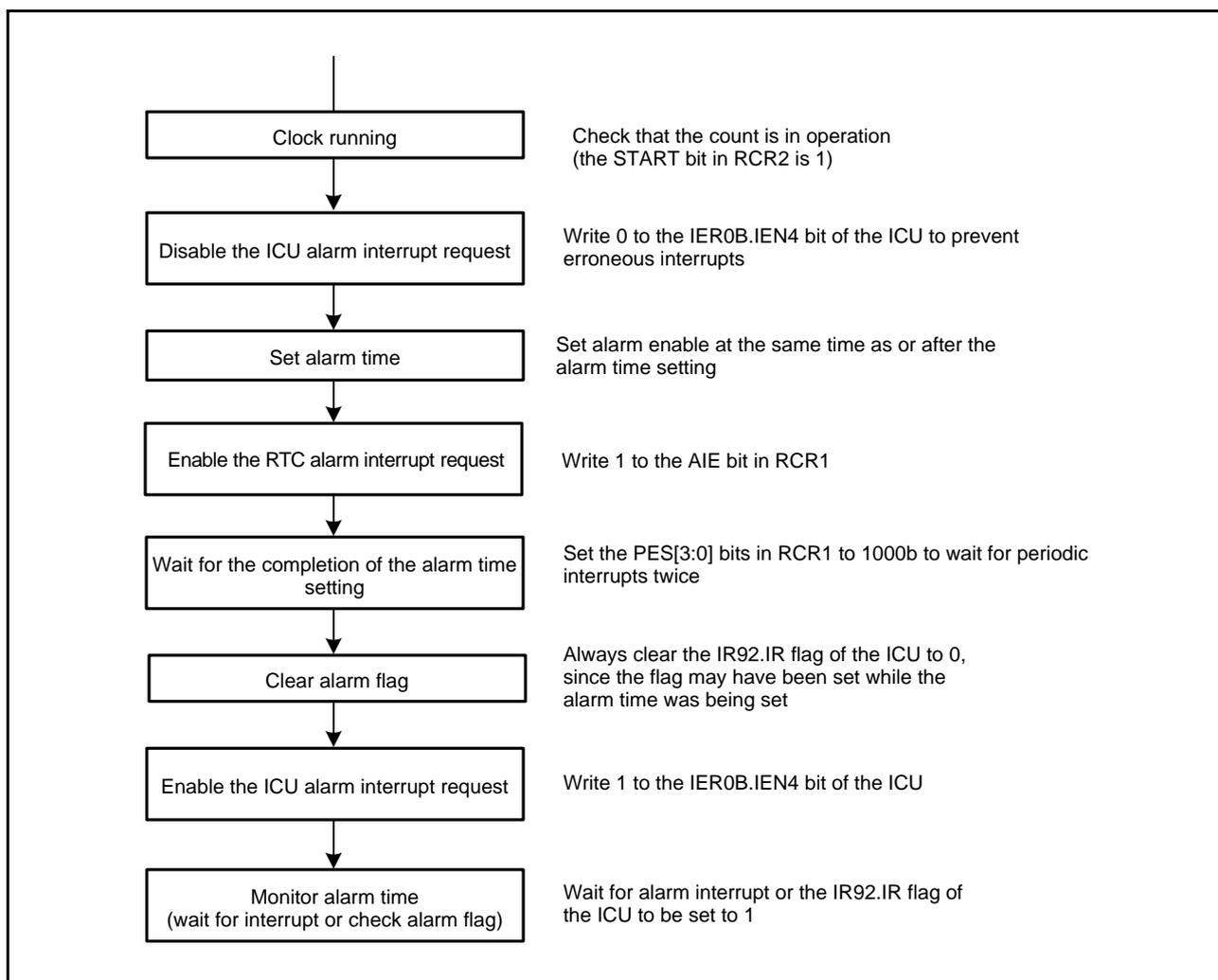
**Figure 25.7 Using Alarm Function**
