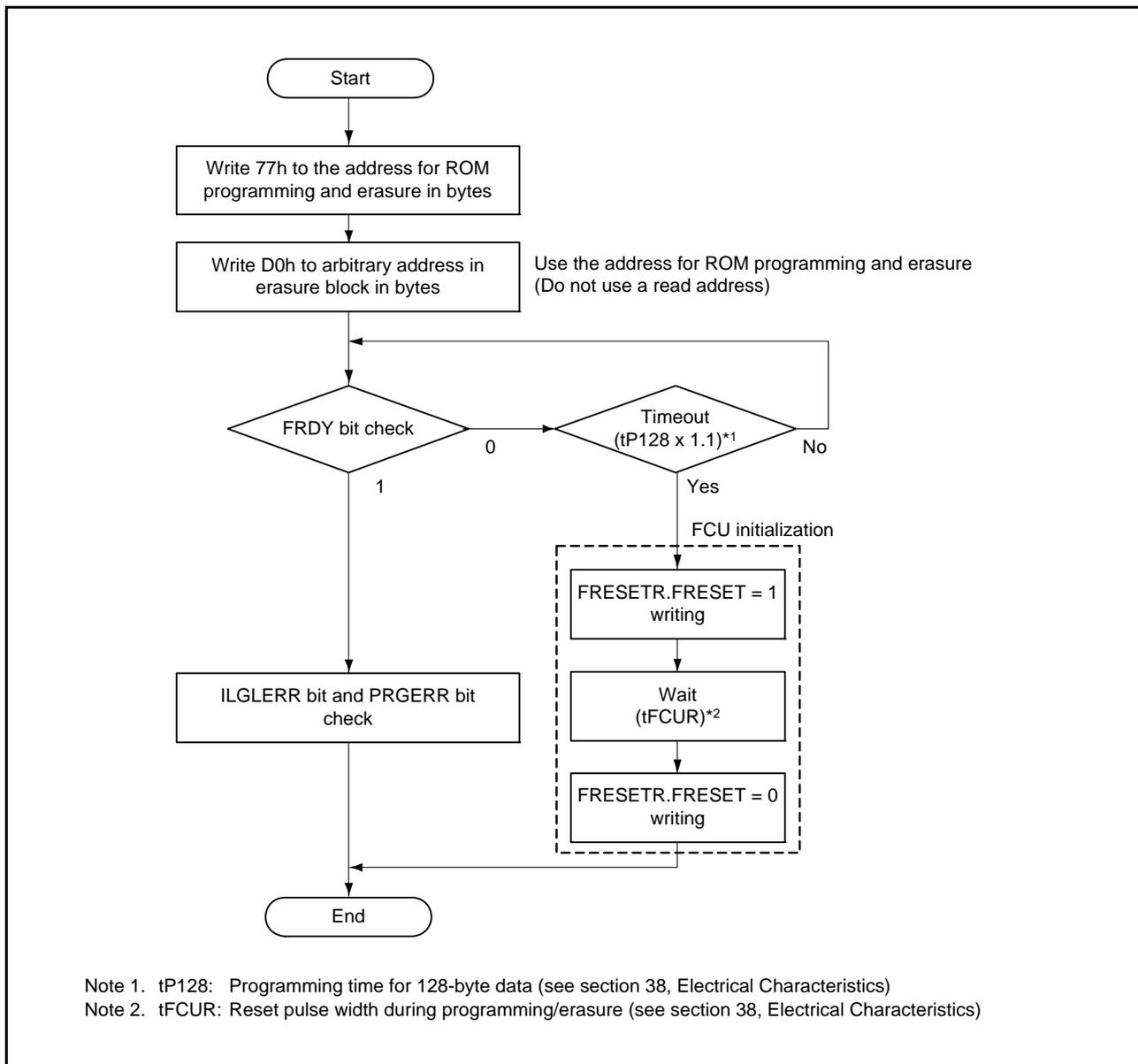
Figure 36.14 Procedure for Programming the Lock Bit
