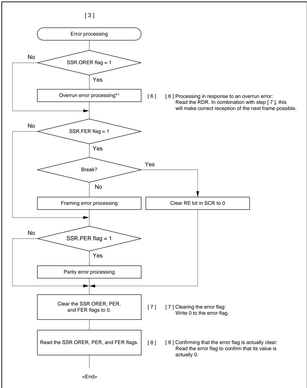
Figure 27.14 Example of Serial Reception Flowchart (2) (Asynchronous Mode)
