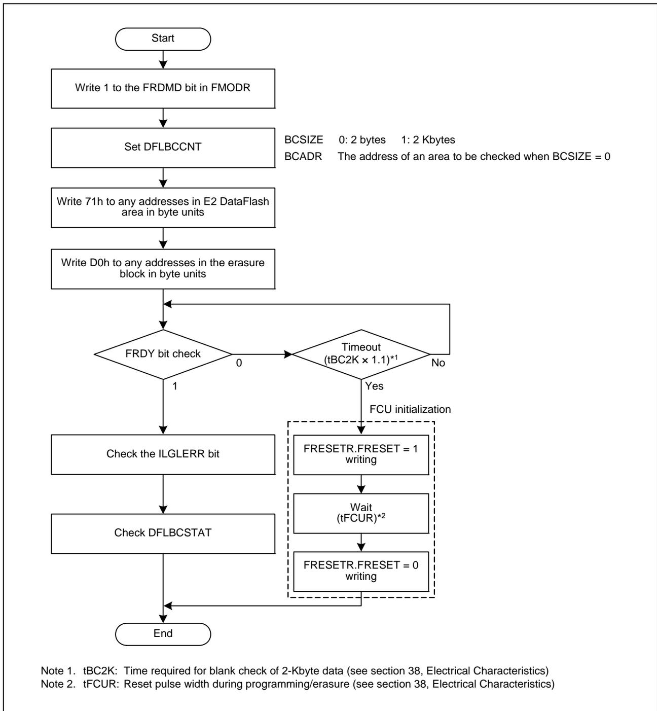
Figure 37.6 Procedure for Blank Checking of the E2 DataFlash
