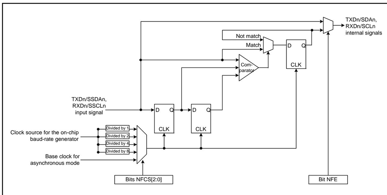
Figure 27.68 Block Diagram of Digital Noise Filter Circuit
