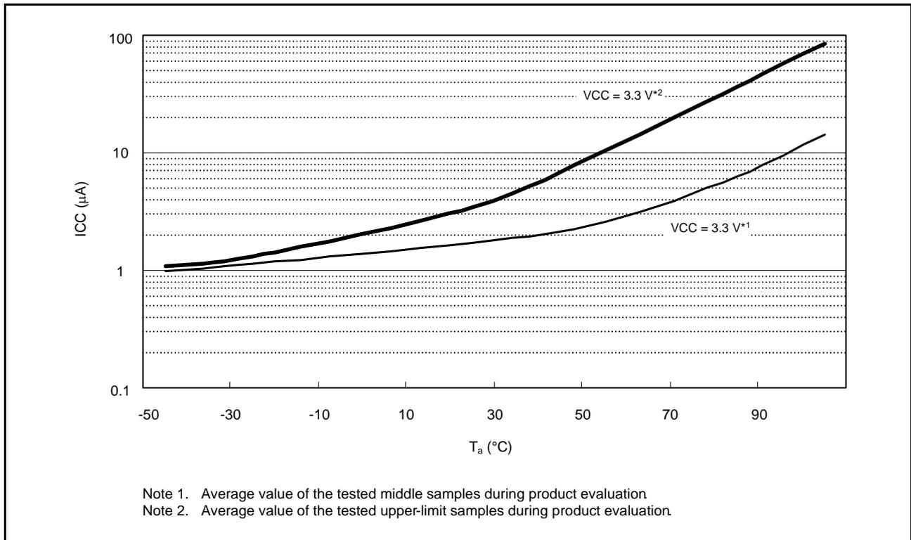
Figure 38.5 Temperature Dependency in Software Standby Mode (SOFTCUT Bit = 11xb) (Reference Data)
