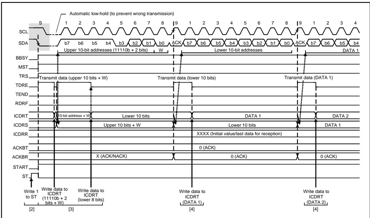
Figure 29.8 Master Transmit Operation Timing (2) (10-Bit Address Format)
