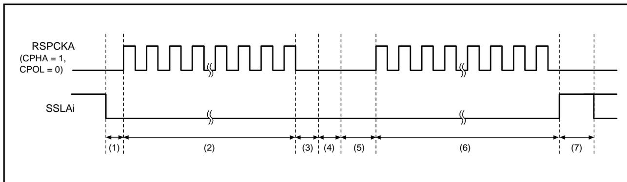
**Figure 30.33 Example of Burst Transfer Operation using SSLKP Bit**
