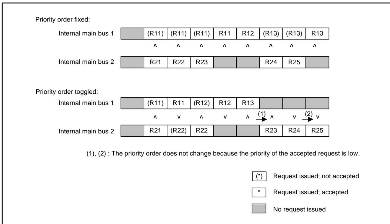
**Figure 15.2 Priority Order Between Internal Peripheral Bus Accesses**
