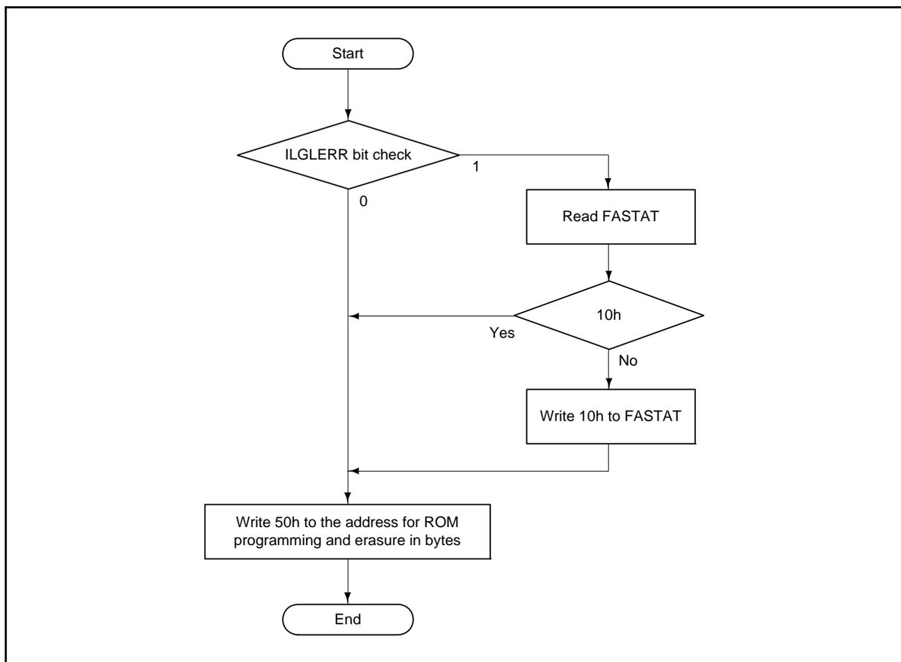
Figure 36.16 Procedure for Clearing FSTATR0
