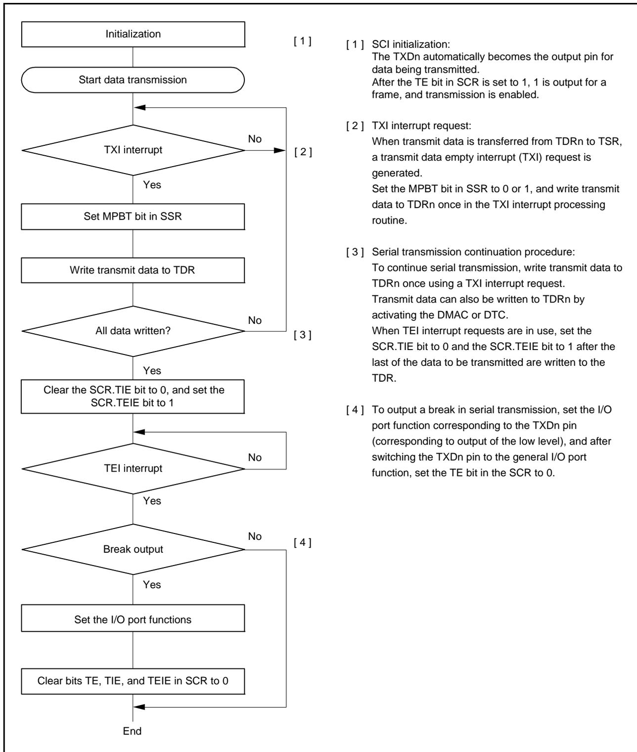
Figure 27.16 Example of Multi-Processor Serial Transmission Flowchart
