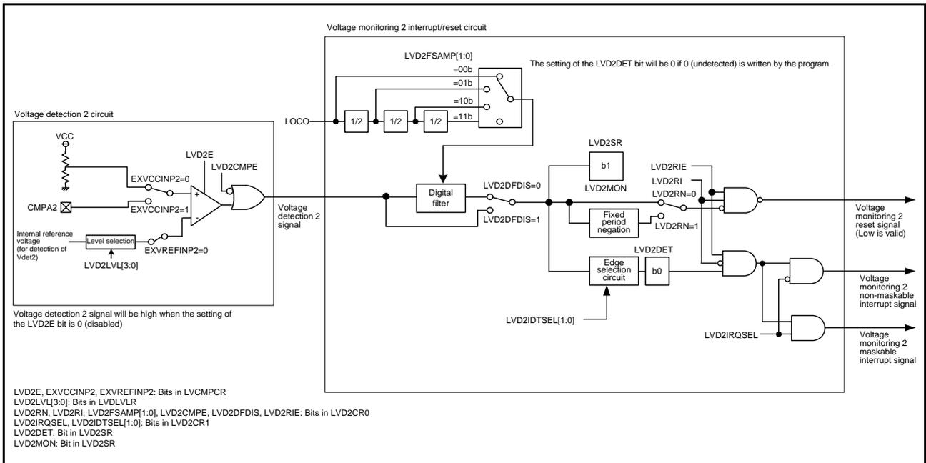
Figure 8.3 Block Diagram of Voltage Monitoring 2 Interrupt/Reset Circuit
