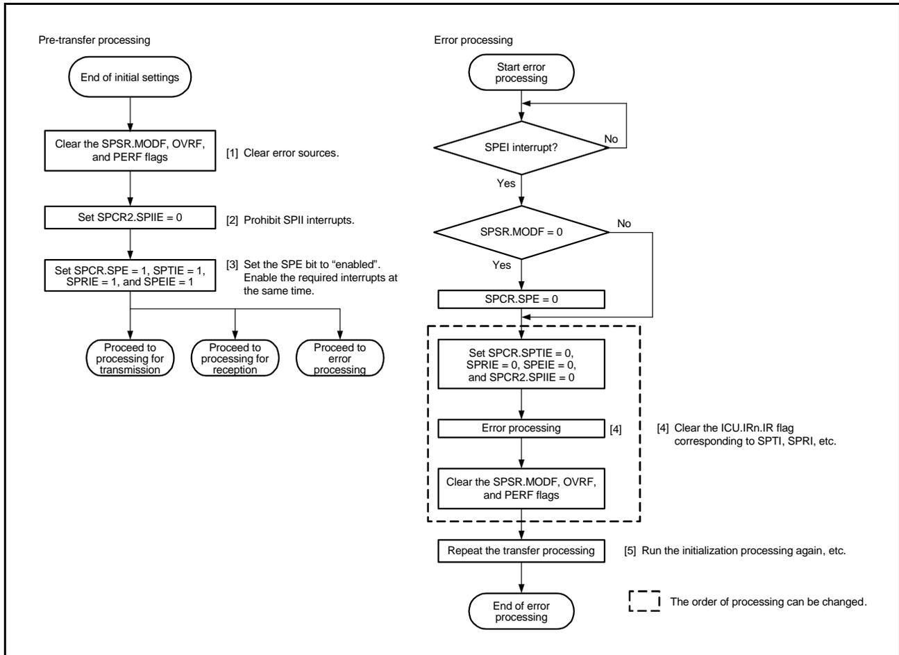
Figure 30.41 Flowchart for Slave Mode (Error Processing)
