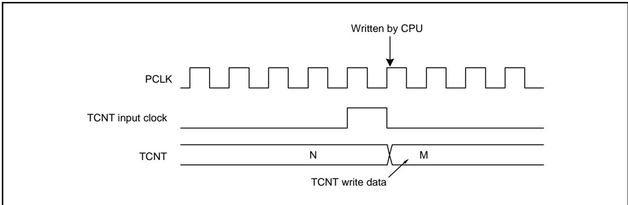
Figure 21.108 Contention between TCNT Write and Increment Operations
