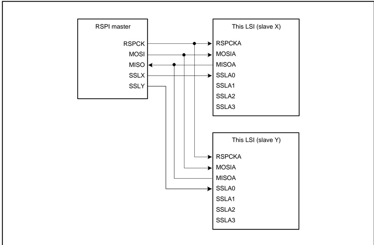
Figure 30.9 Single-Master/Multi-Slave Configuration Example (This LSI = Slave)
