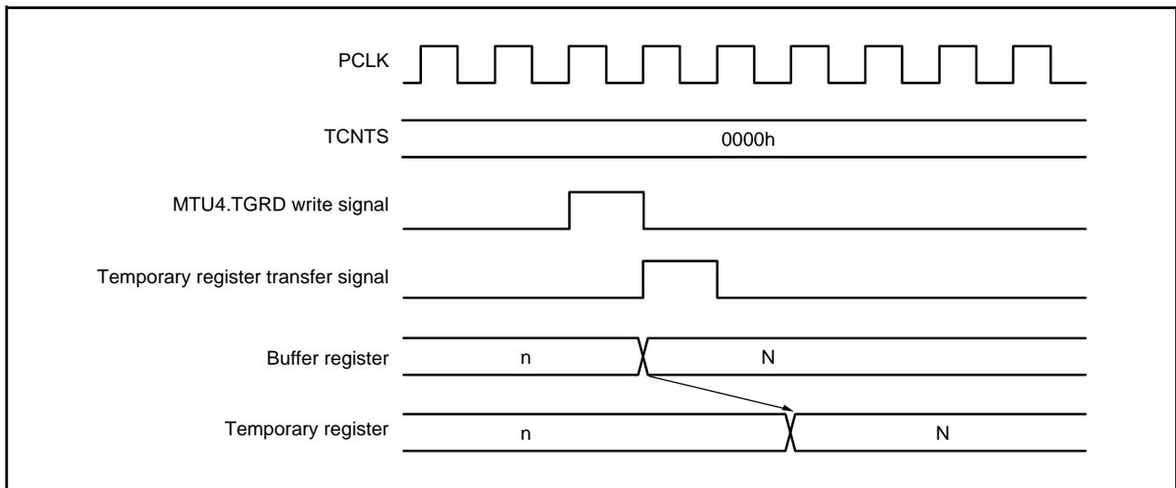
Figure 21.97 Transfer Timing from Buffer Register to Temporary Register (TCNTS Stop)
