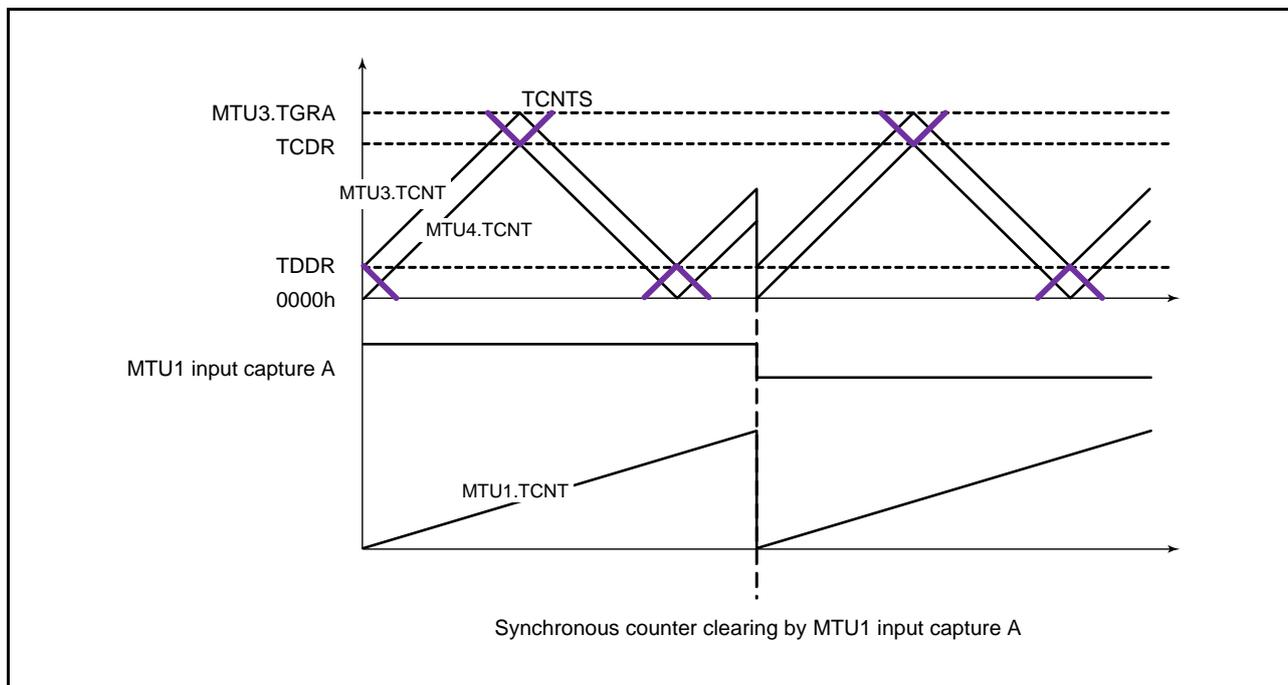
Figure 21.55 Counter Clearing Synchronized with Another Channel
