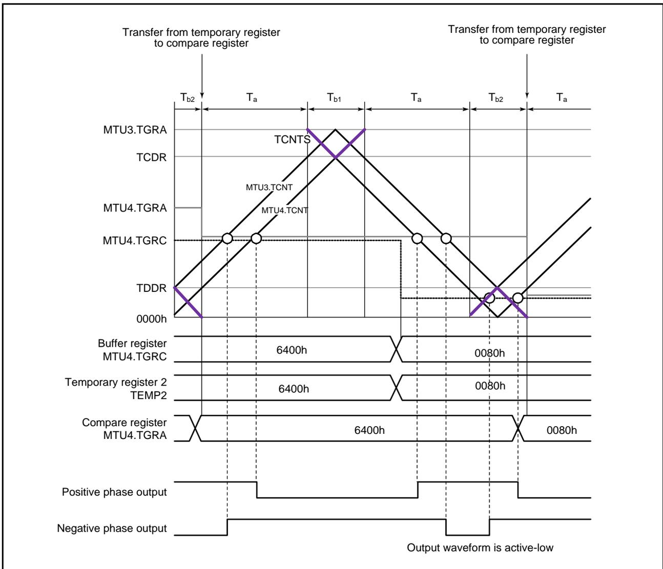
Figure 21.40 Example of Operation in Complementary PWM Mode
