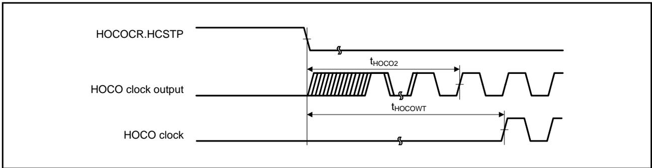
**Figure 38.25 HOCO Clock Oscillation Start Timing (Oscillation is Started by Setting the HOCO CR.HCSTP Bit)**
