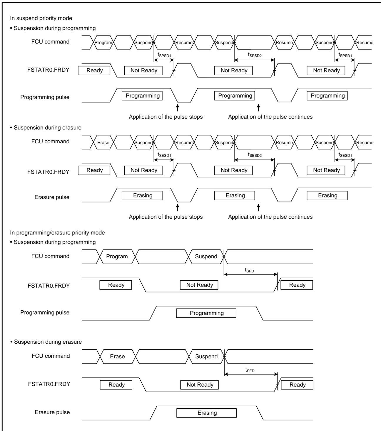
Figure 38.57 Flash Memory Program/Erase Suspend Timing
