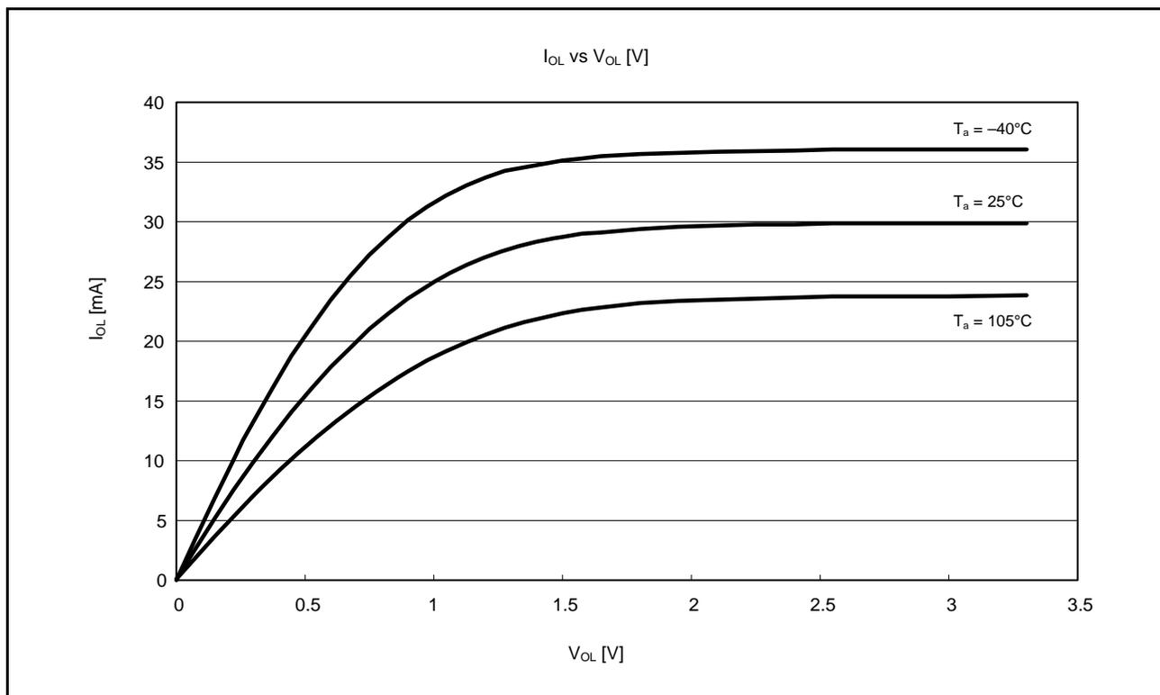
Figure 38.19  $V_{OL}$  and  $I_{OL}$  Temperature Characteristics of RIIC Output Pin at  $V_{CC} = 3.3$  V (Reference Data)
