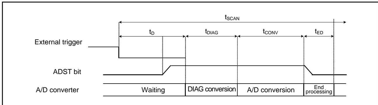
**Figure 32.12 Scan Conversion Timing (Activated by ADTRG0#)**
