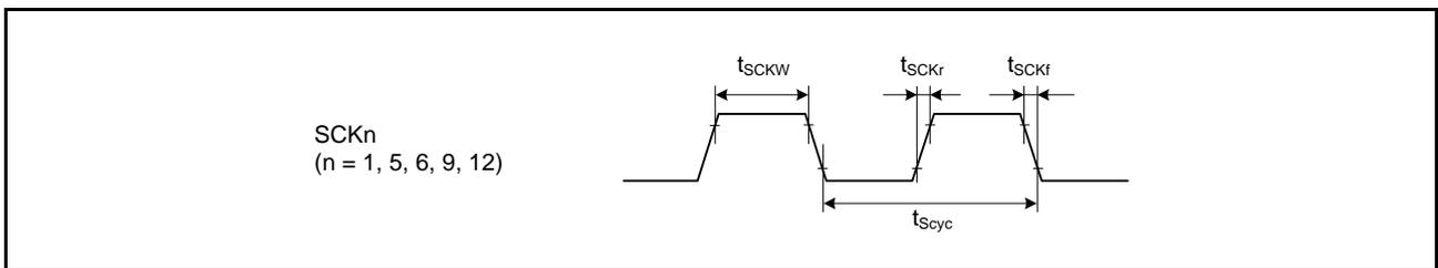
Figure 38.38 SCK Clock Input Timing
