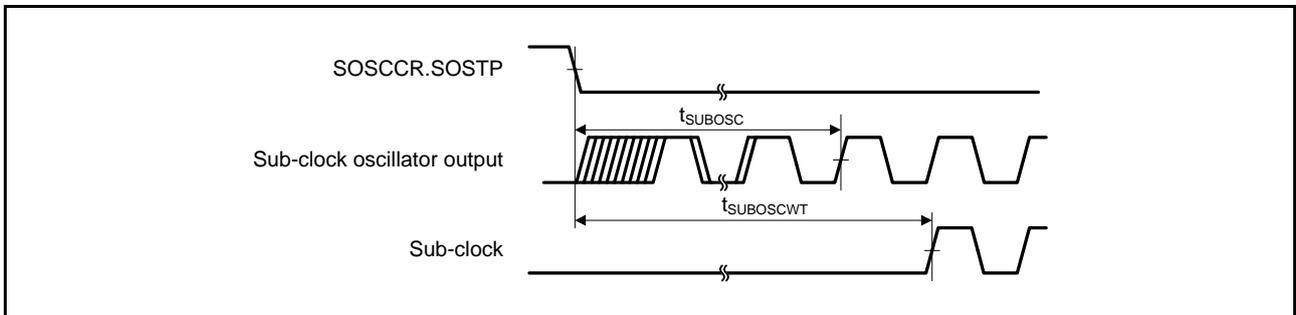
**Figure 38.27 Sub-clock Oscillation Start Timing**
