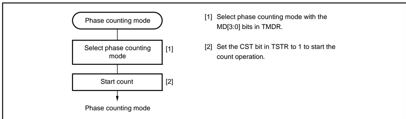
**Figure 21.29 Example of Phase Counting Mode Setting Procedure**
