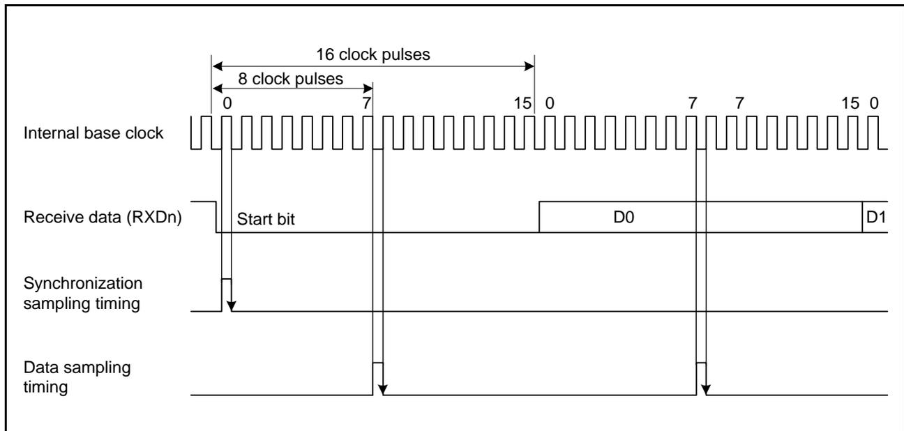
Figure 27.6 Receive Data Sampling Timing in Asynchronous Mode
