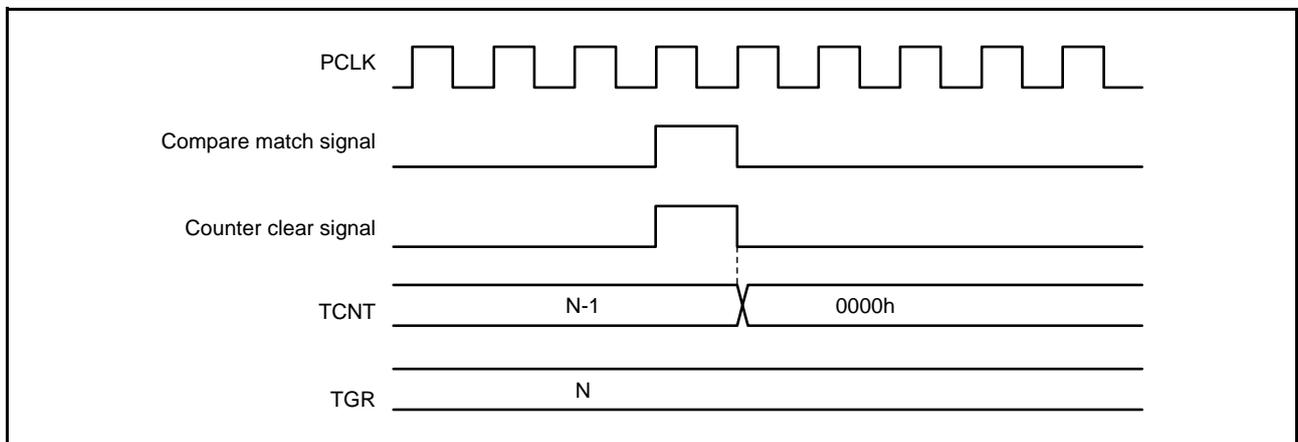
Figure 21.92 Counter Clear Timing (Compare Match) (MTU5)
