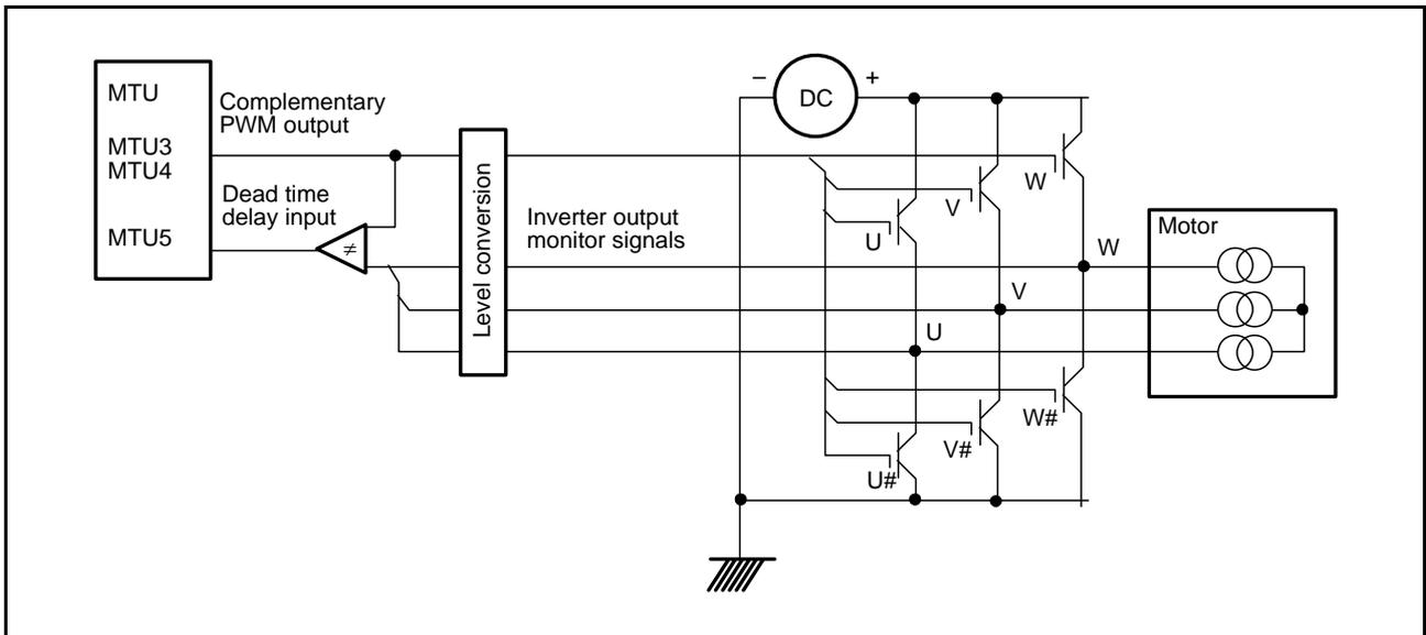
Figure 21.81 Example of Motor Control Circuit Configuration
