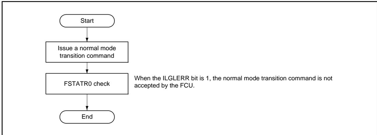
**Figure 36.7 Procedure for Transition to ROM P/E Normal Mode**
