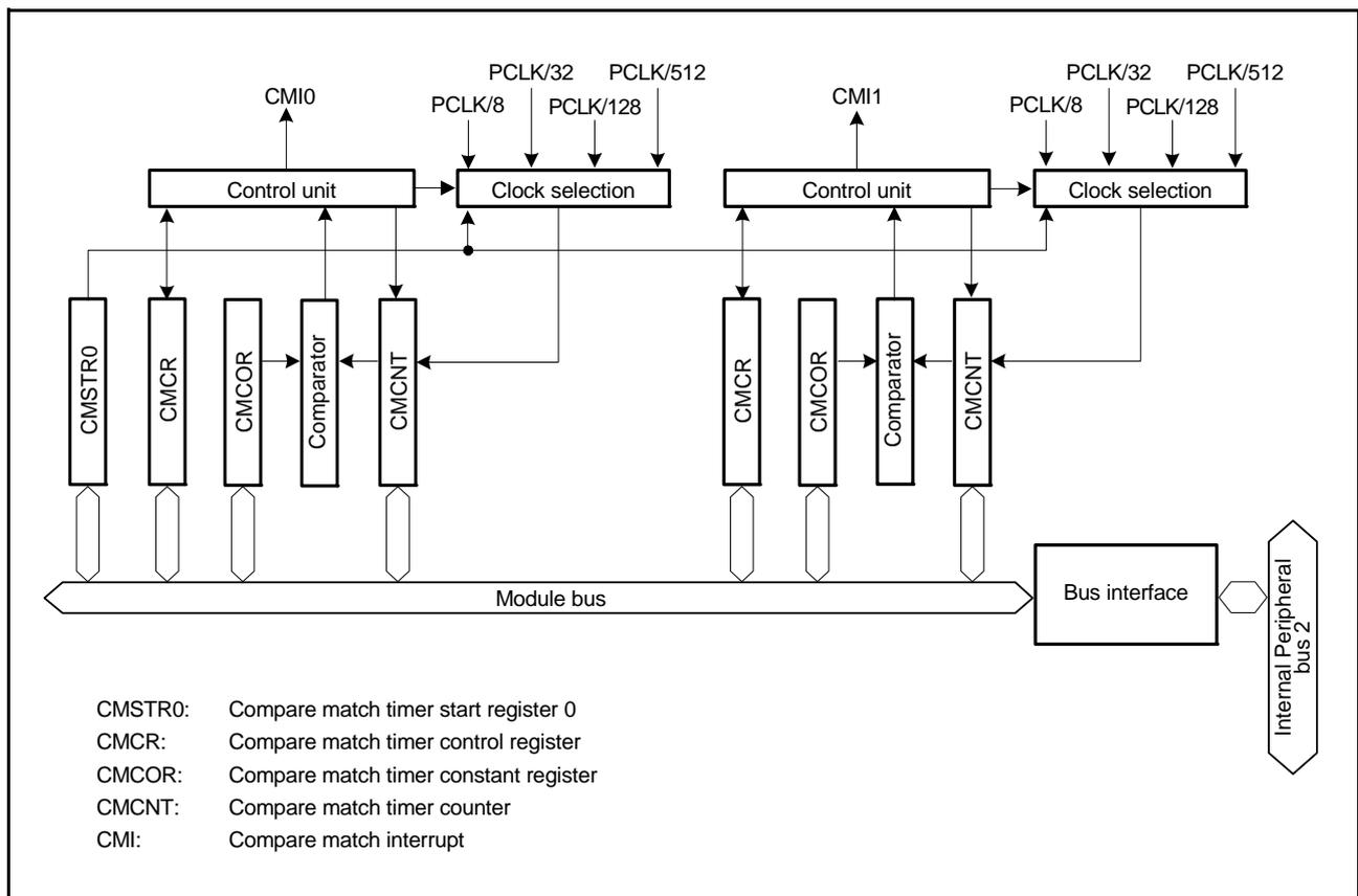
**Figure 24.1 Block Diagram of CMT (Unit 0)**
