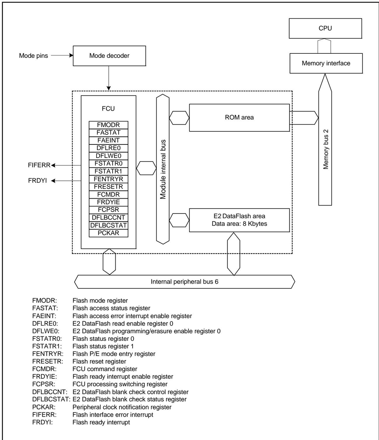
**Figure 37.1 Block Diagram of E2 DataFlash Memory**
