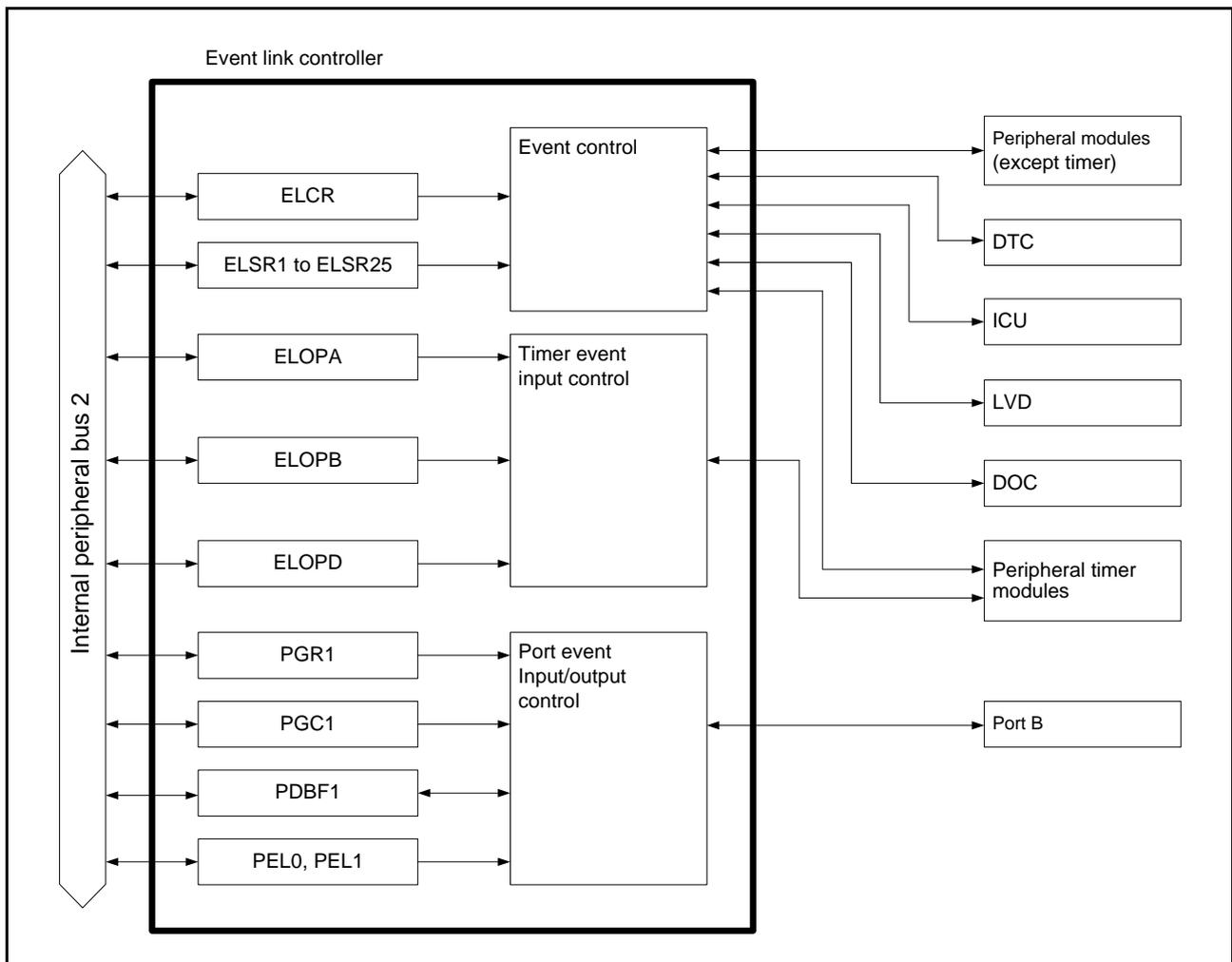
**Figure 18.1 Block Diagram of Event Link Controller**
