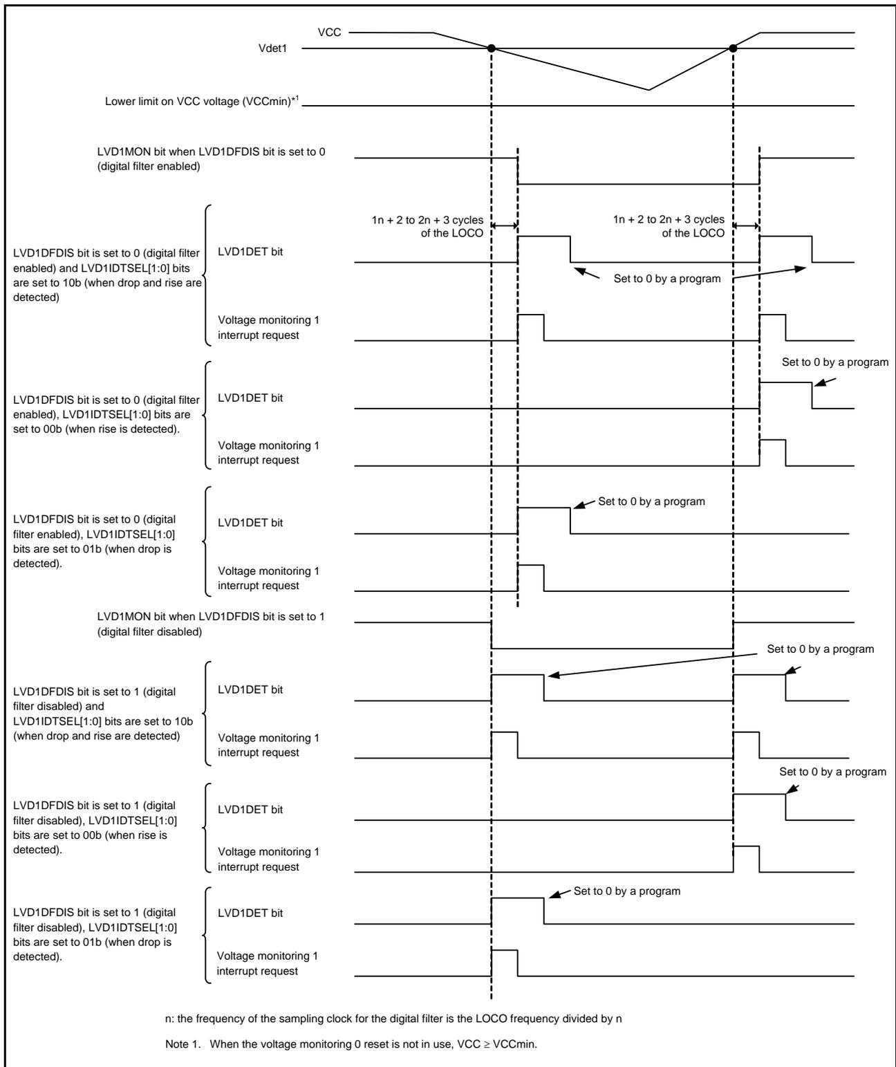
Figure 8.5 Example of Voltage Monitoring 1 Interrupt Operation
