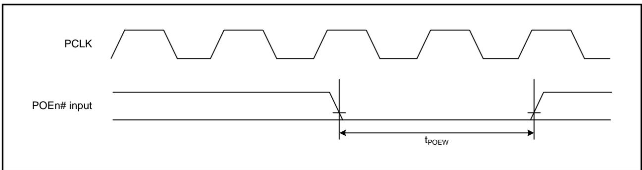
Figure 38.36 POE# Input Timing
