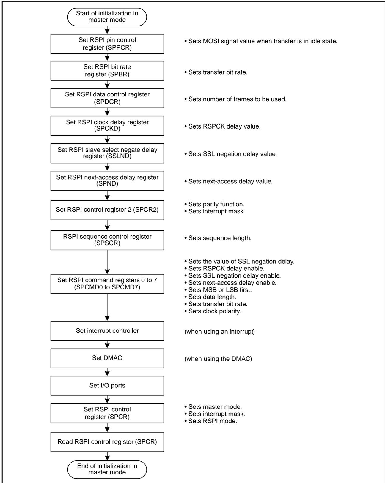
Figure 30.45 Example of Initialization Flowchart in Master Mode (Clock Synchronous Operation)
