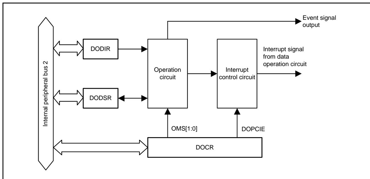
**Figure 34.1 Block Diagram of Data Operation Circuit**
