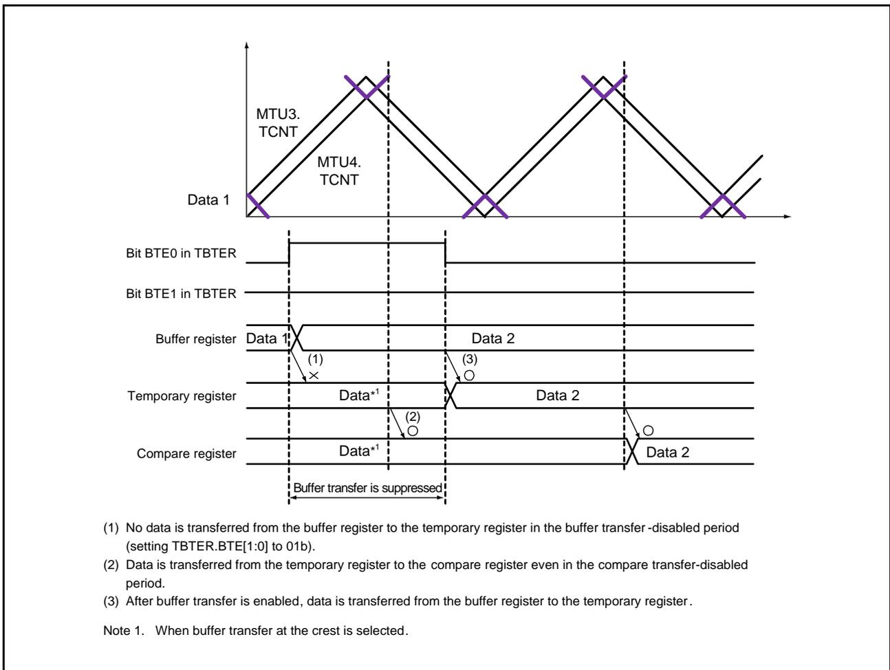
Figure 21.70 Example of Operation when Buffer Transfer is Disabled (BTE[1:0] = 01b)
