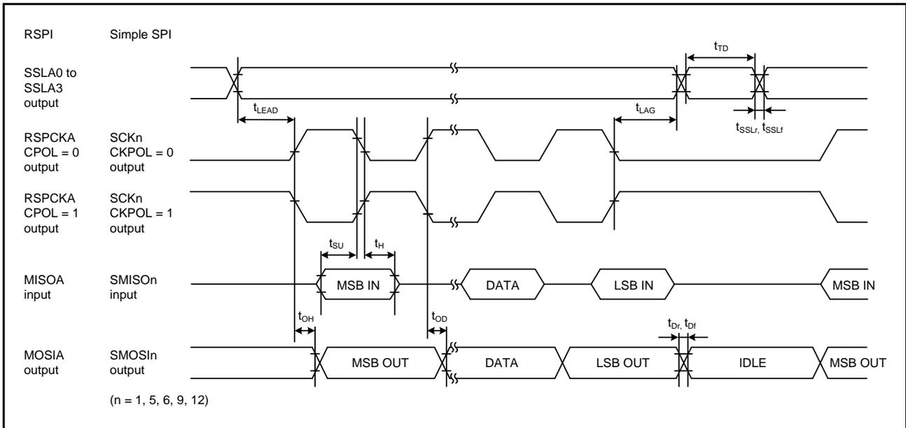
**Figure 38.44 RSPI Timing (Master, CPHA = 1) (Bit Rate: PCLKB Set to Division Ratio Other Than Divided by 2) and Simple SPI Timing (Master, CKPH = 0)**
