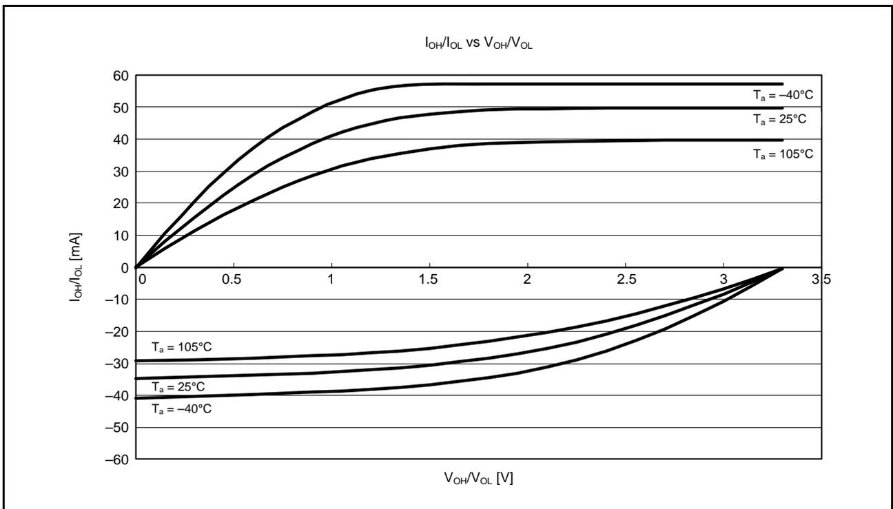
Figure 38.15  $V_{OH}/V_{OL}$  and  $I_{OH}/I_{OL}$  Temperature Characteristics at  $V_{CC} = 3.3$  V when High-Drive Output is Selected (Reference Data)
