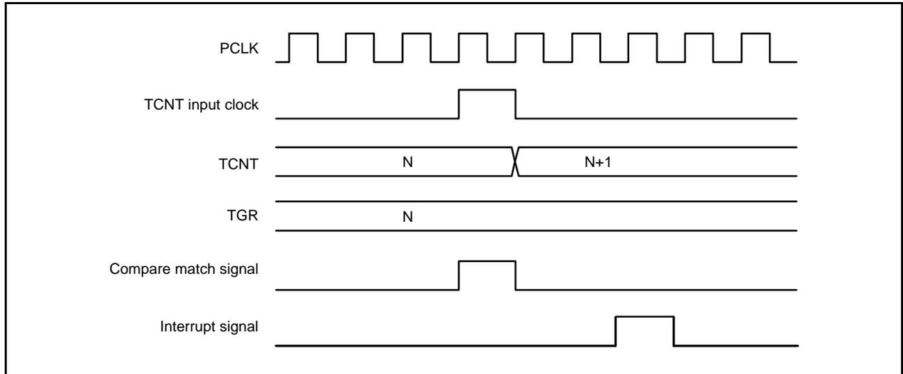
**Figure 21.100 TGI Interrupt Timing (Compare Match) (MTU0 to MTU4)**
