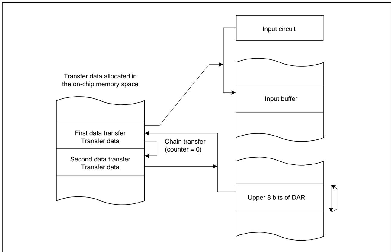
Figure 17.15 Chain Transfer when Counter = 0
