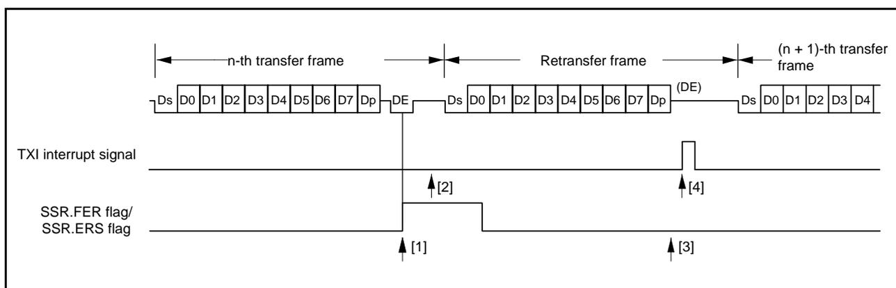
Figure 27.33 Data Retransfer Operation in SCI Transmission Mode
