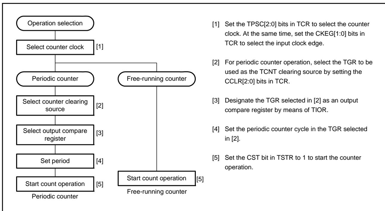
Figure 21.4 Example of Counter Operation Setting Procedure
