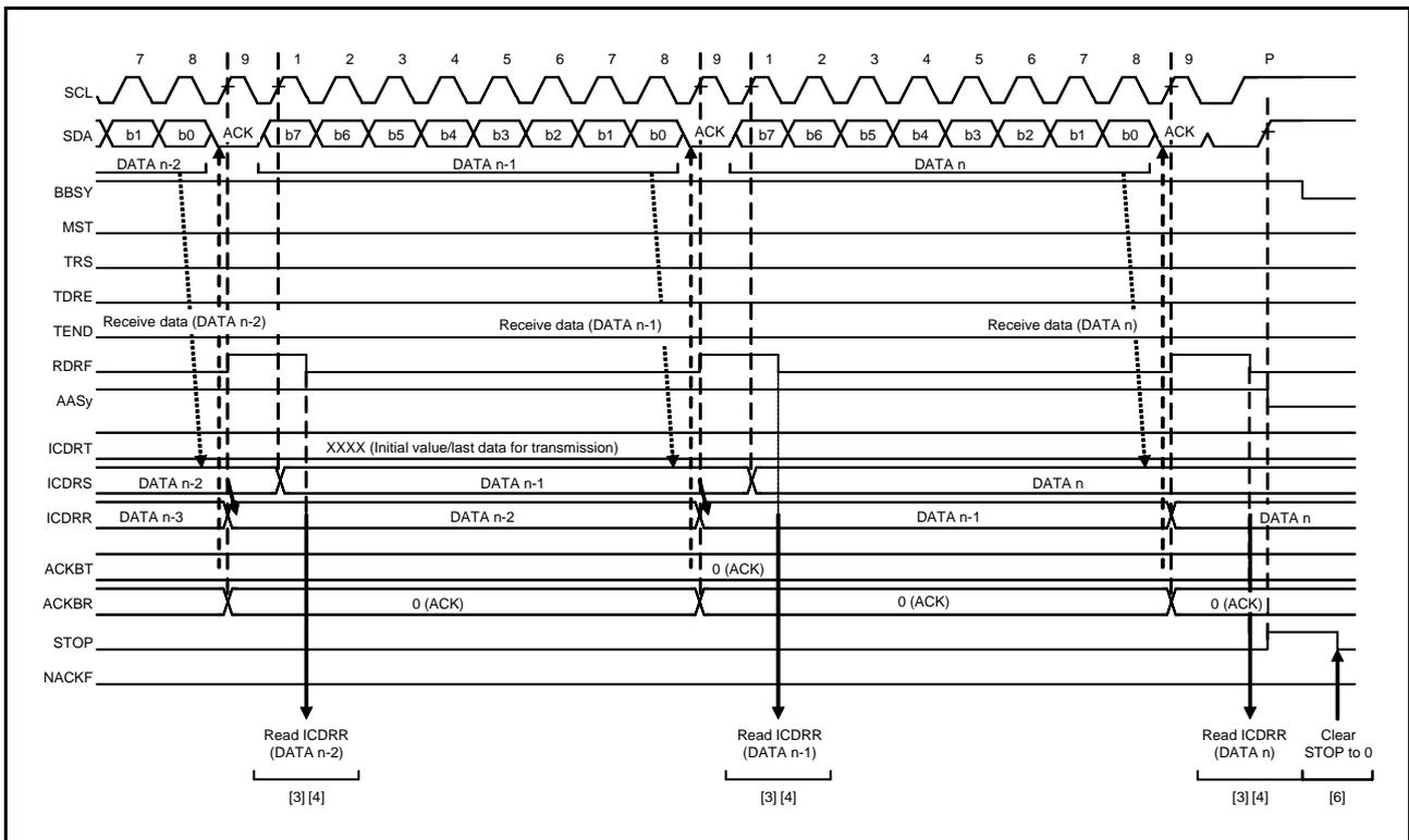
Figure 29.20 Slave Receive Operation Timing (2) (when RDRFS = 0)
