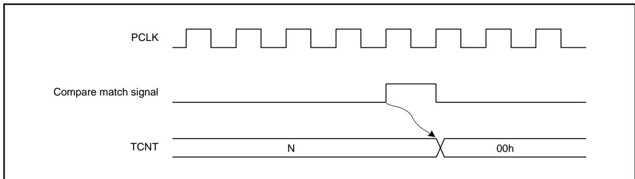
Figure 23.9 Timing of Counter Clear by Compare Match
