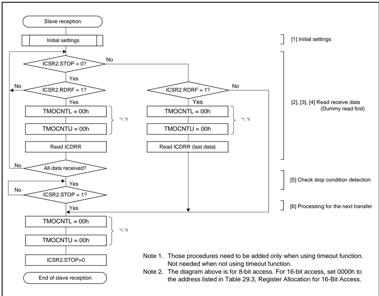
Figure 29.18 Example of Slave Reception Flowchart
