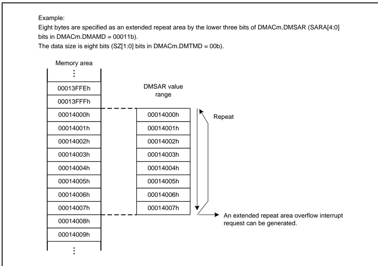
Figure 16.5 Example of Extended Repeat Area Operation
