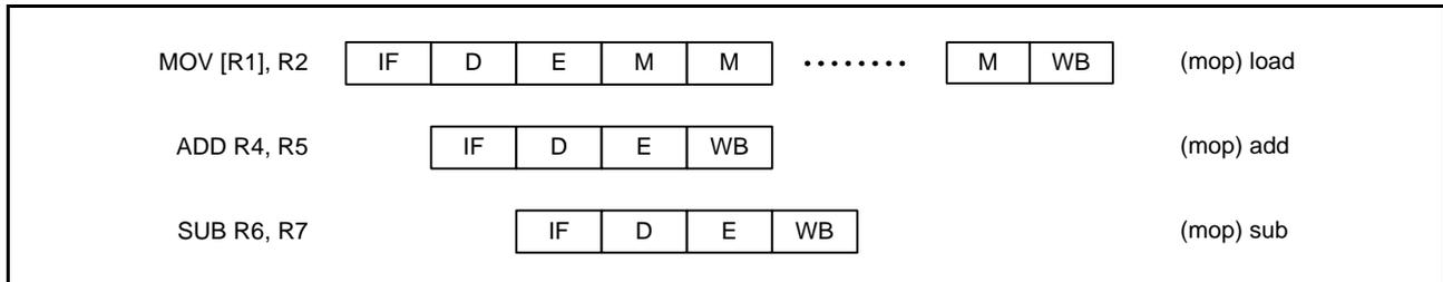
**Figure 2.22** When Load Data is not Used by the Subsequent Instruction
