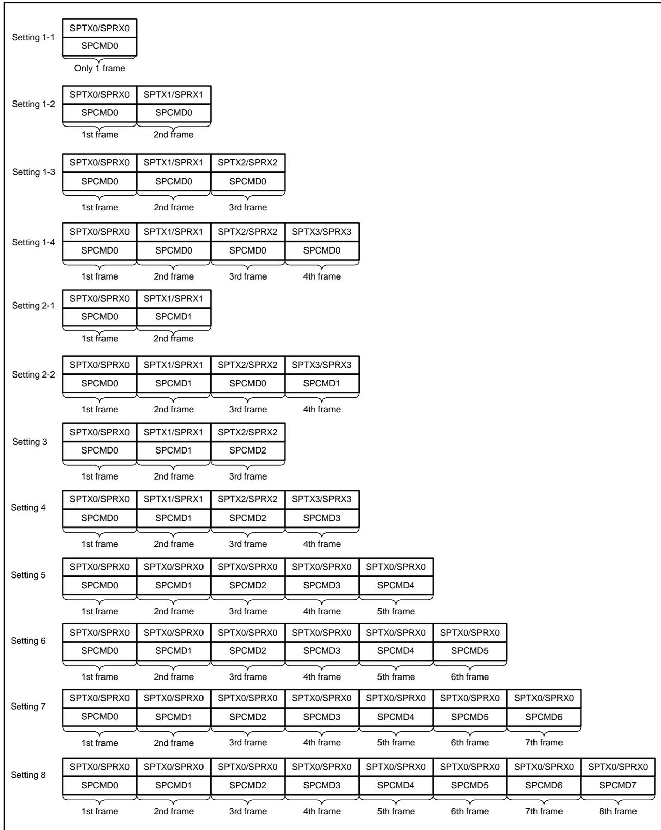
**Figure 30.44 Correspondence between the RSPI Command Register and Transmit/Receive Buffers in Sequence Operations**
