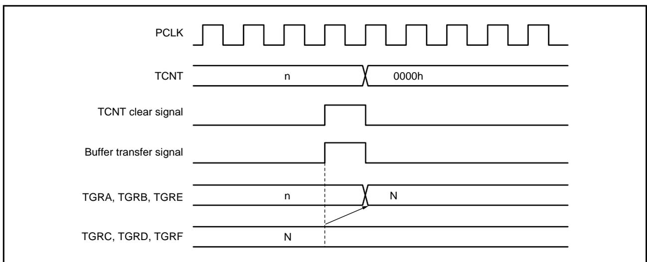
Figure 21.96 Buffer Operation Timing (when TCNT Cleared)
