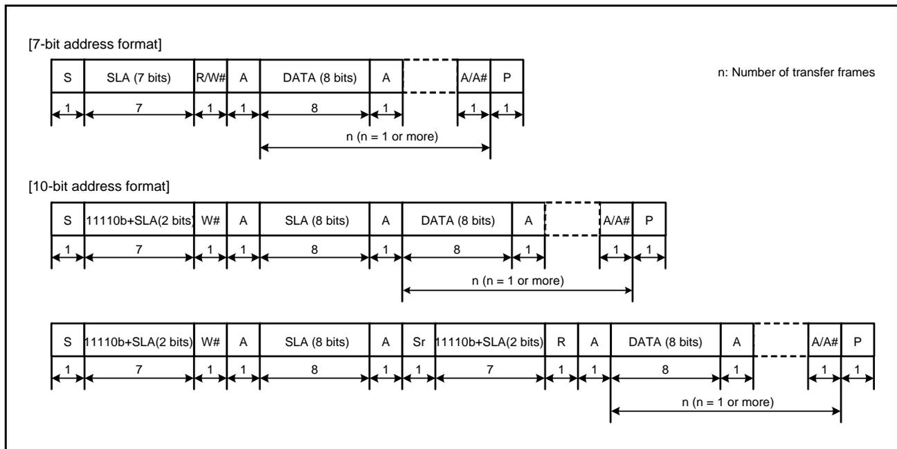
Figure 29.3 I<sup>2</sup>C Bus Format
