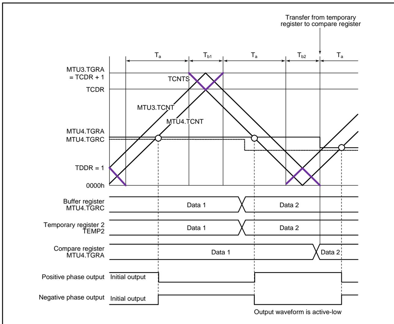
Figure 21.41 Example of Operation without Dead Time
