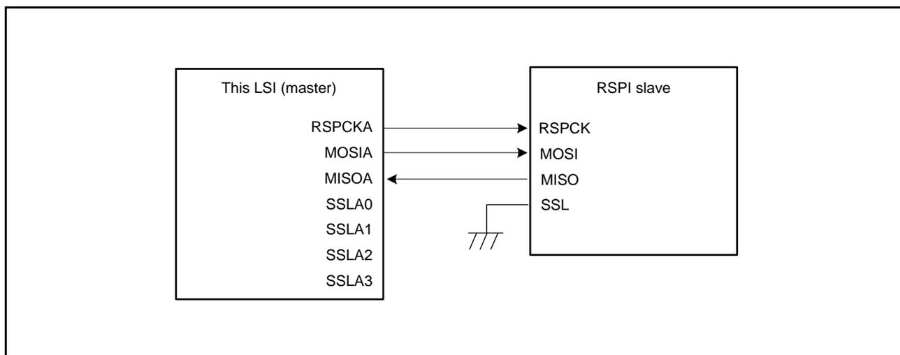
Figure 30.5 Single-Master/Single-Slave Configuration Example (This LSI = Master)
