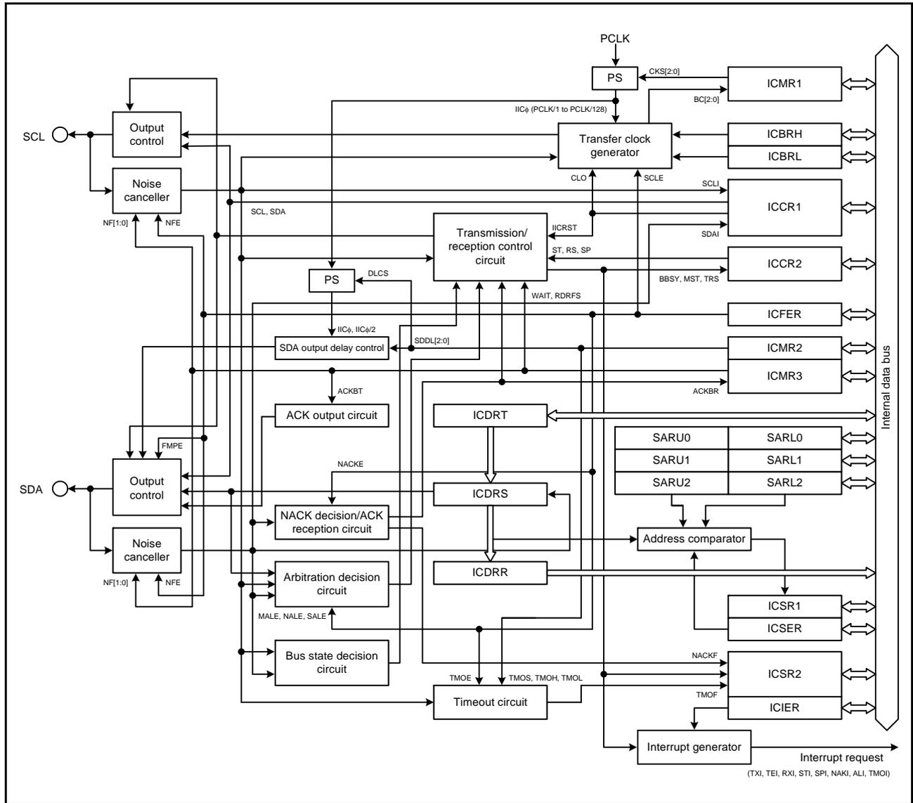
**Figure 29.1 Block Diagram of RIIC**
