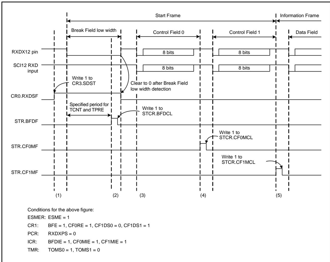
Figure 27.57 Example of Operations at the Time of Start-Frame Reception
