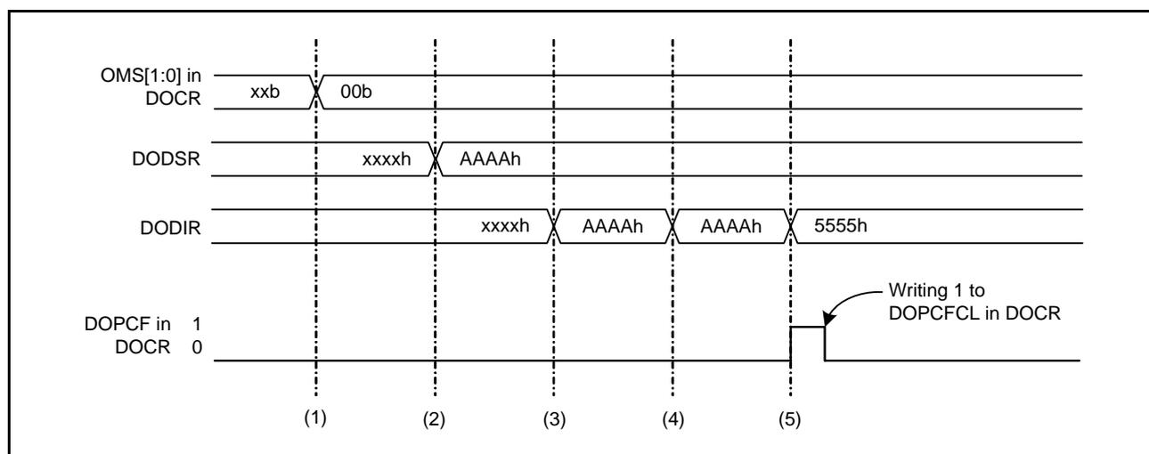
Figure 34.2 Example of Operation in Data Comparison Mode
