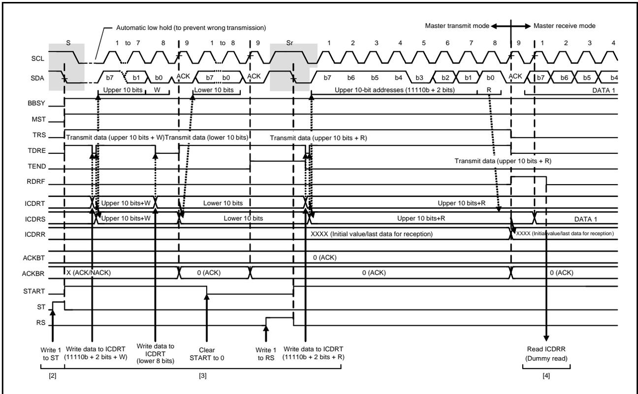
Figure 29.13 Master Receive Operation Timing (2) (10-Bit Address Format, when RDRFS = 0)
