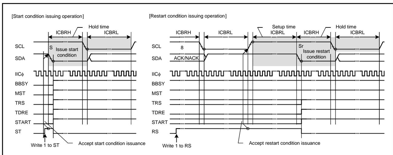
Figure 29.37 Start Condition/Restart Condition Issue Timing (ST and RS Bits)
