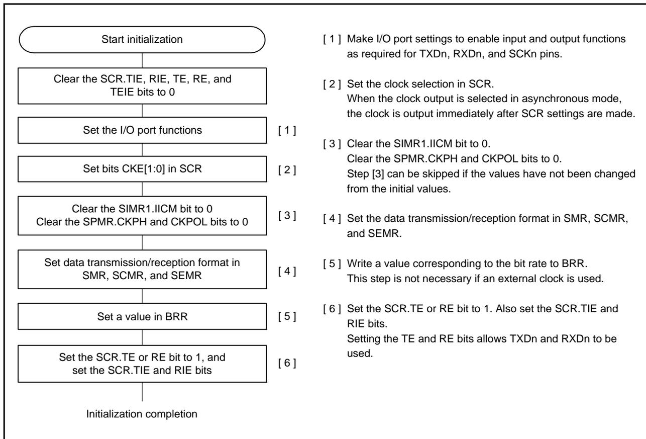
Figure 27.8 Sample SCI Initialization Flowchart (Asynchronous Mode)
