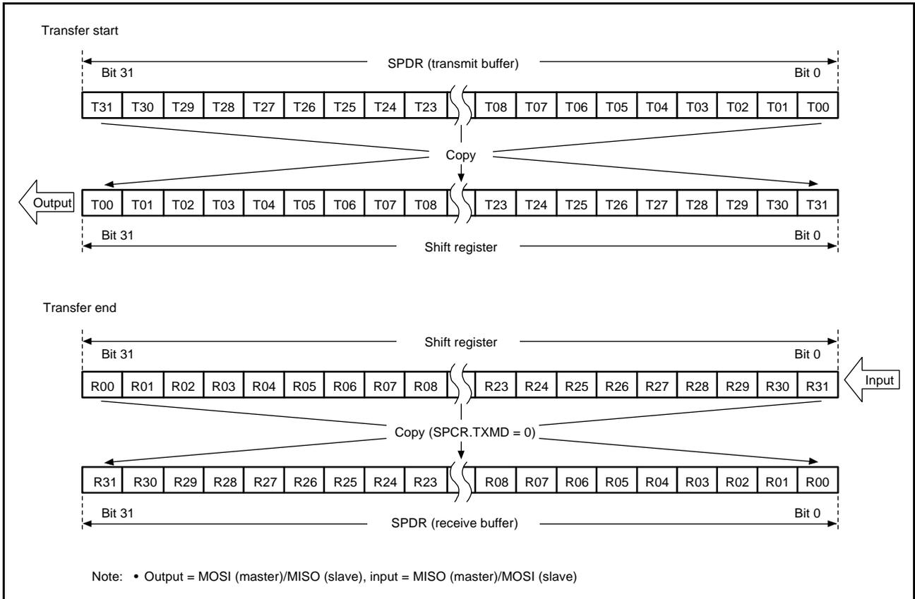
Figure 30.17 LSB-First Transfer (32-Bit Data, Parity Disabled)
