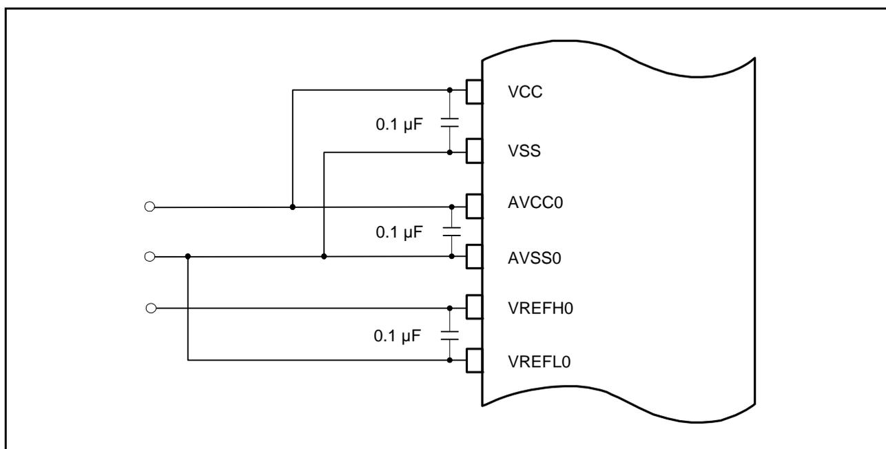
Figure 32.18 Power Supply Pin Connection Example
