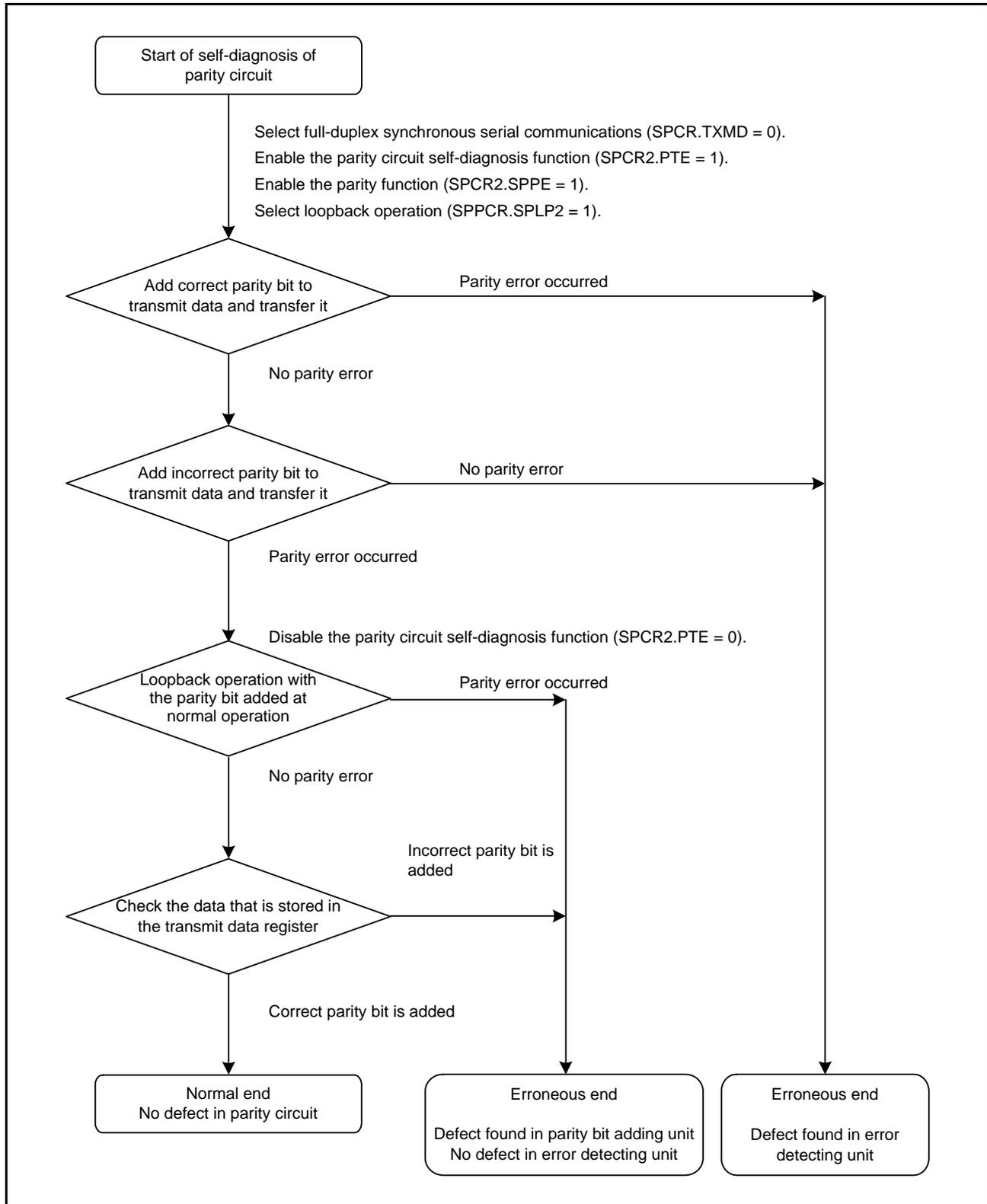
Figure 30.48 Flowchart for Self-Diagnosis of Parity Circuit
