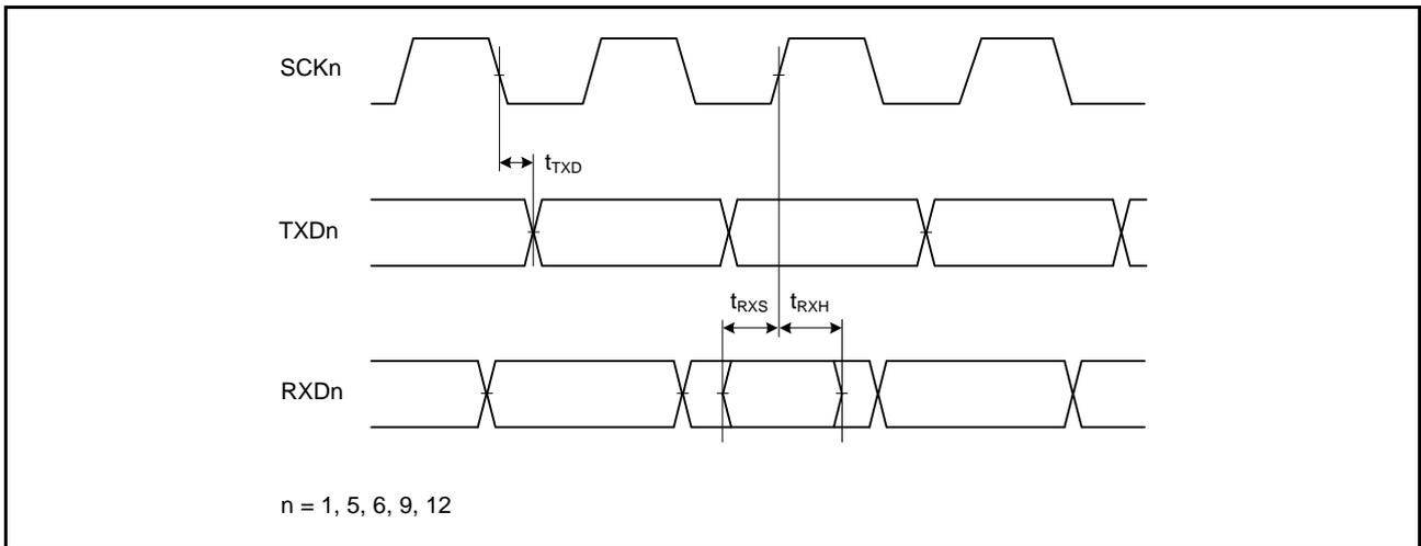
Figure 38.39 SCI Input/Output Timing: Clock Synchronous Mode
