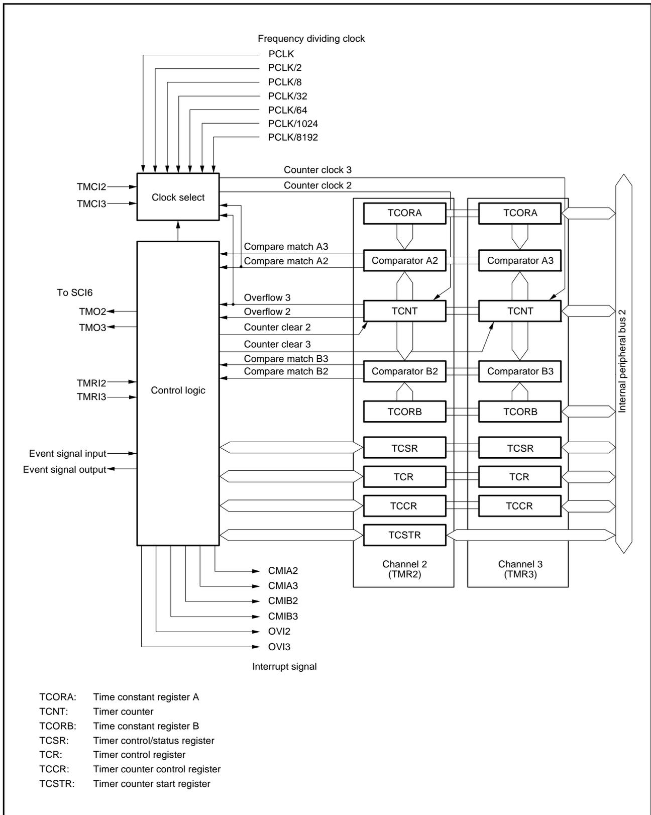
Figure 23.2 Block Diagram of TMR (Unit 1)
