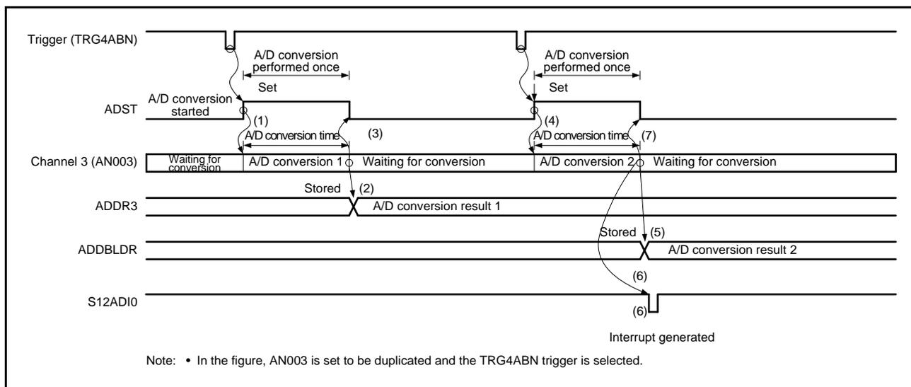
Figure 32.6 Example of Operation in Single Scan Mode (Double Trigger Mode Selected; AN003 Duplicated)
