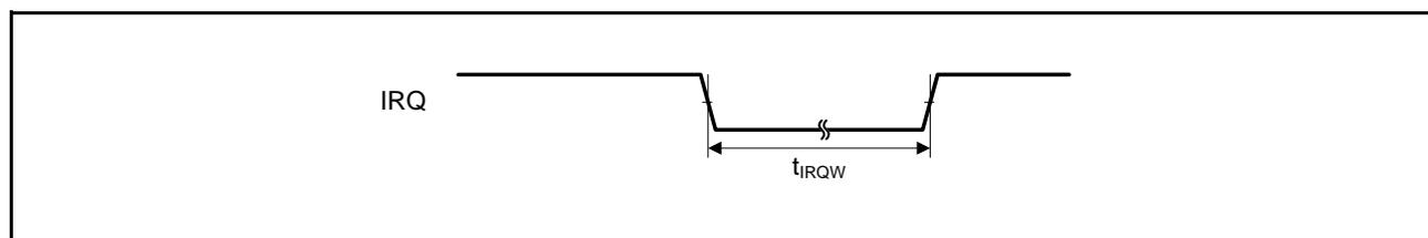
**Figure 38.32 IRQ Interrupt Input Timing**
