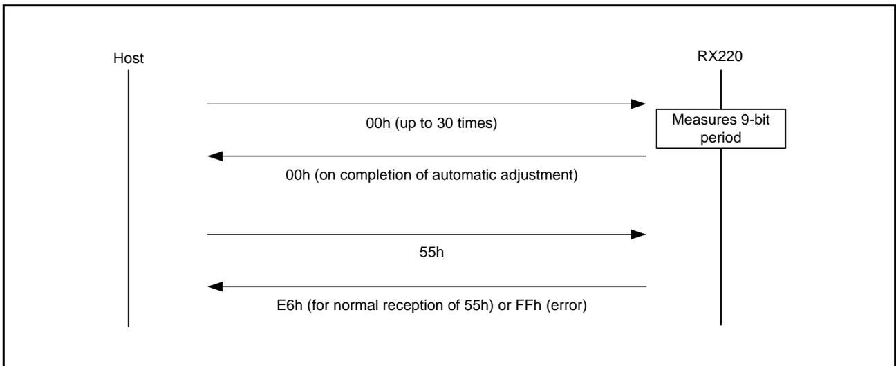
Figure 36.24 Sequence of Transfer between Host and RX220
