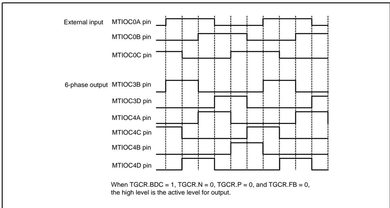
Figure 21.63 Example of Output Phase Switching by External Input (1)
