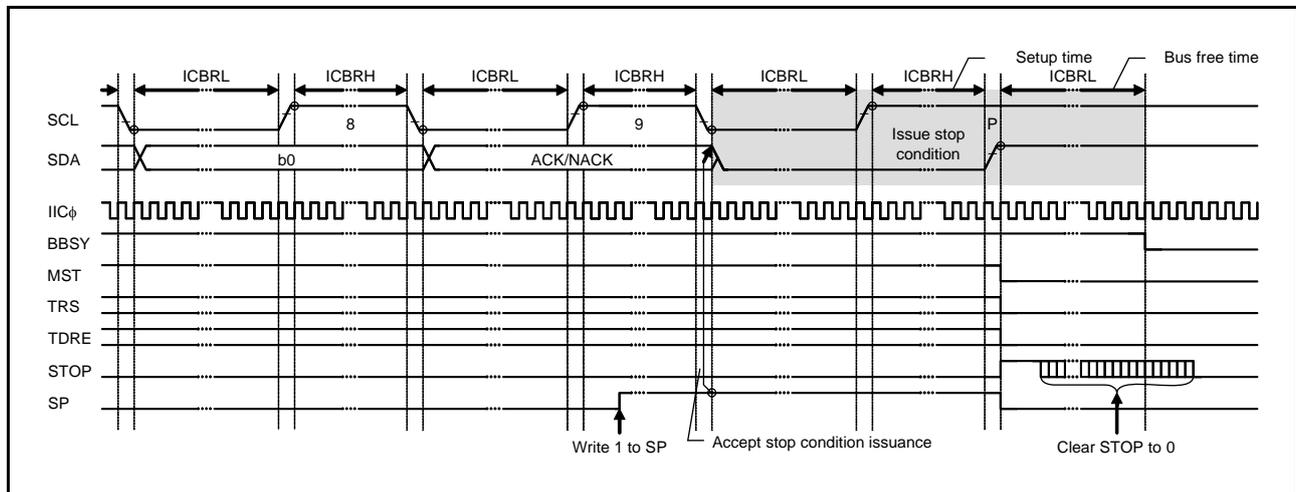
Figure 29.38 Stop Condition Issue Timing (SP Bit)
