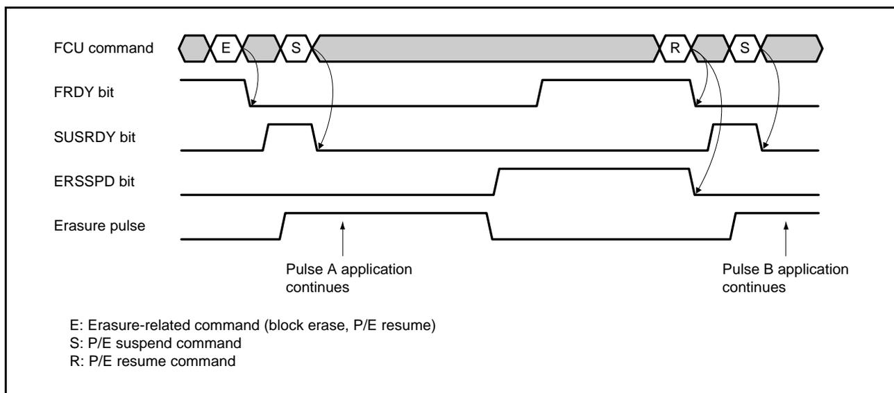
Figure 36.20 Suspension during Erasure (Programming/Erase Priority Mode)
