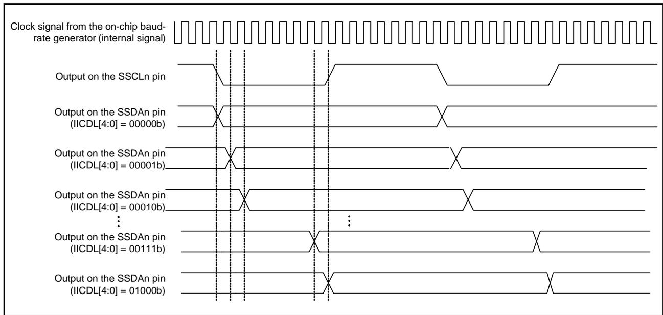
Figure 27.44 Timing of Delays in SSDA Output
