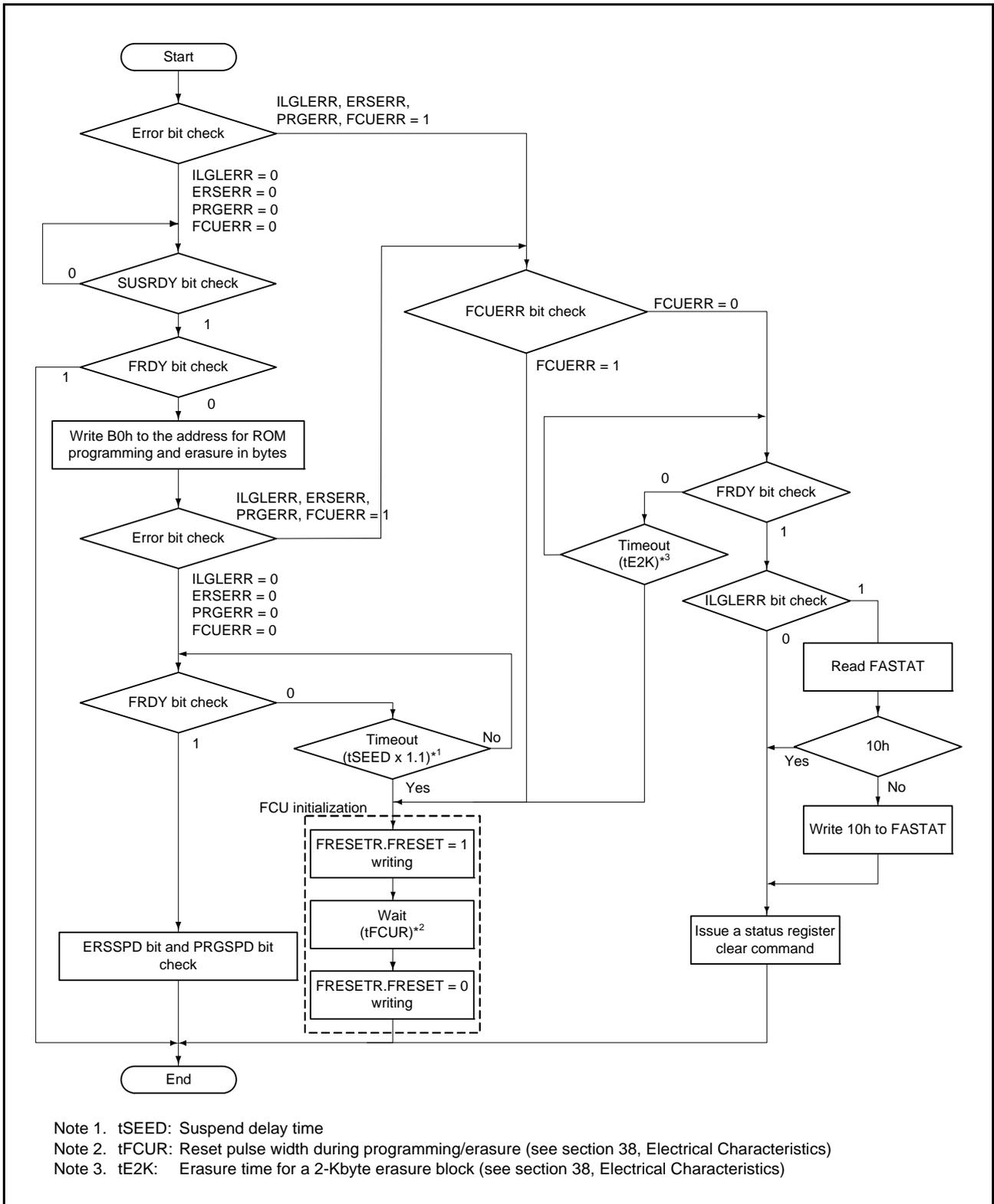
Figure 36.17 Procedure for Programming/Erasure Suspension
