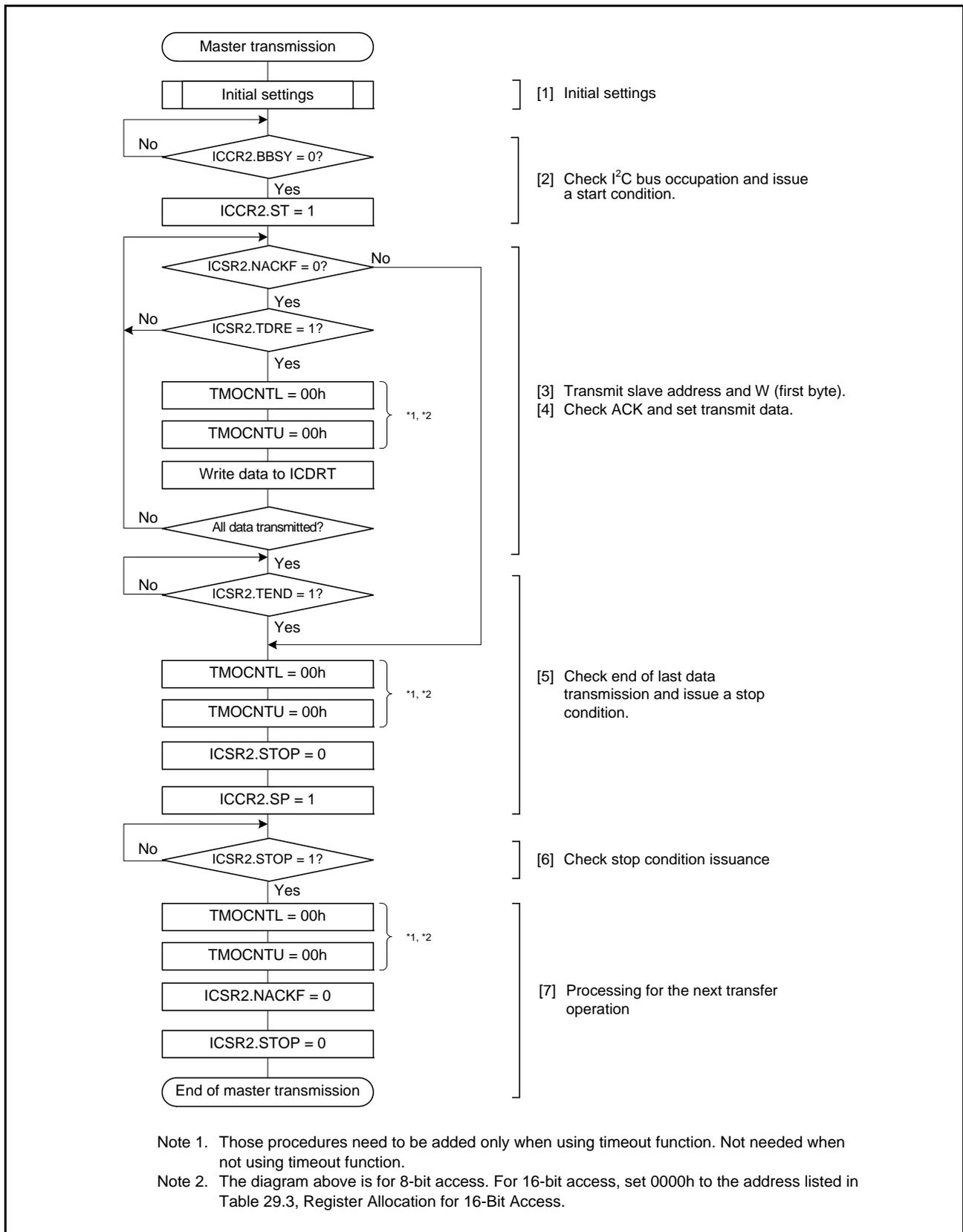
Figure 29.6 Example of Master Transmission Flowchart
