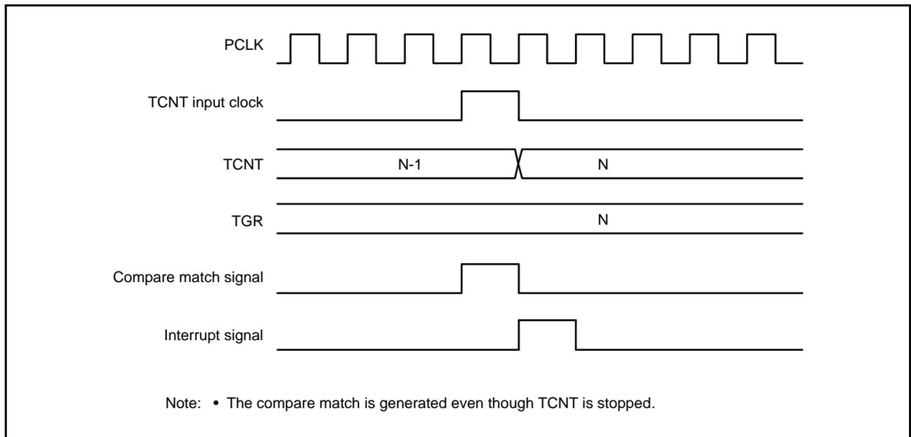
**Figure 21.101 TGI Interrupt Timing (Compare Match) (MTU5)**
