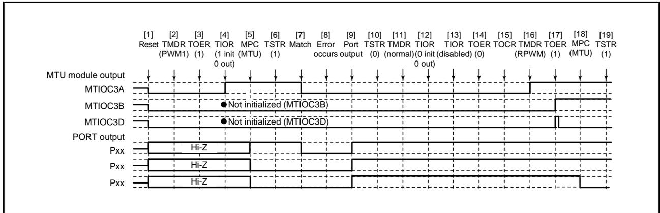
**Figure 21.136 Error Occurrence in PWM Mode 1, Recovery in Reset-Synchronized PWM Mode**
