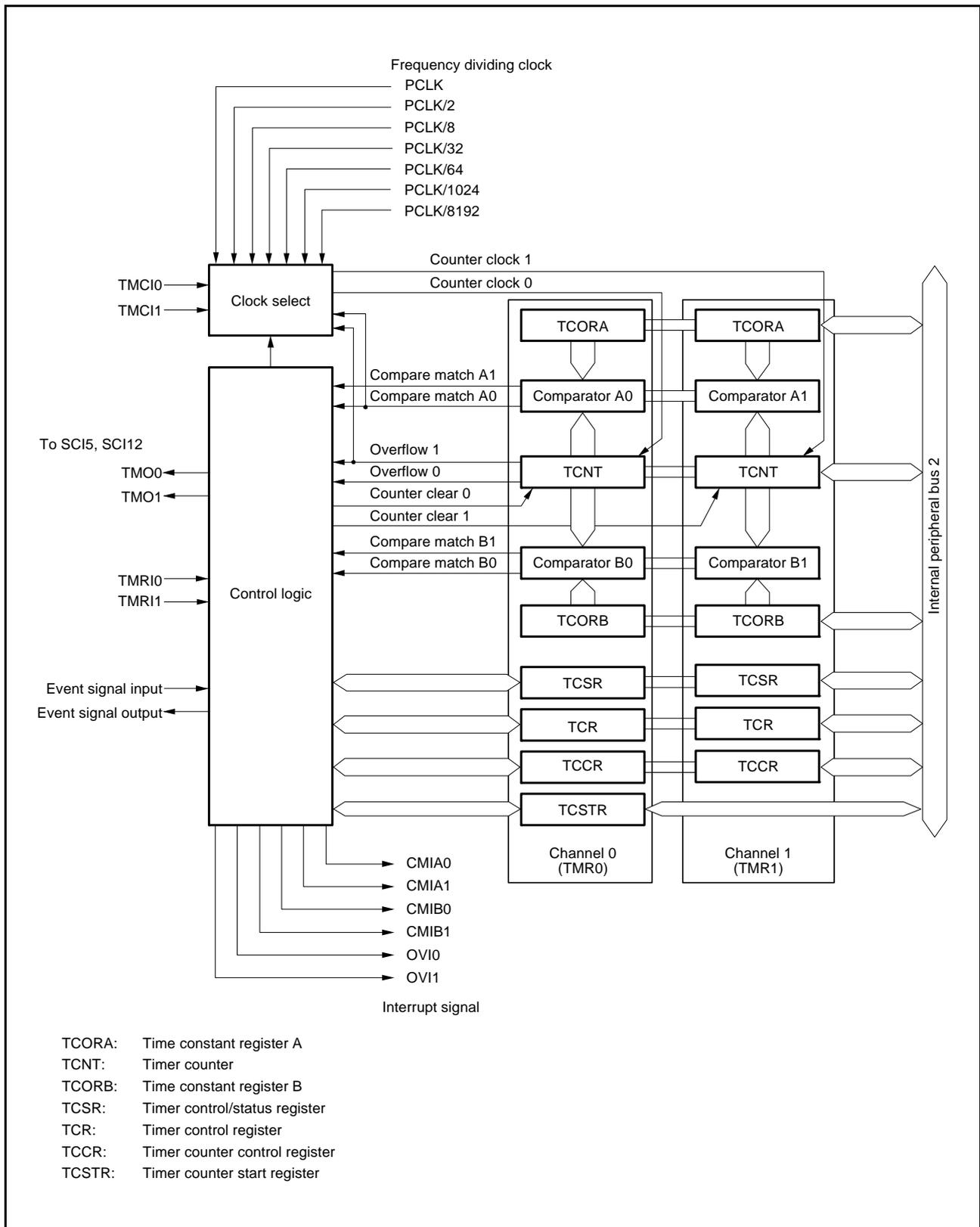
Figure 23.1 Block Diagram of TMR (Unit 0)
