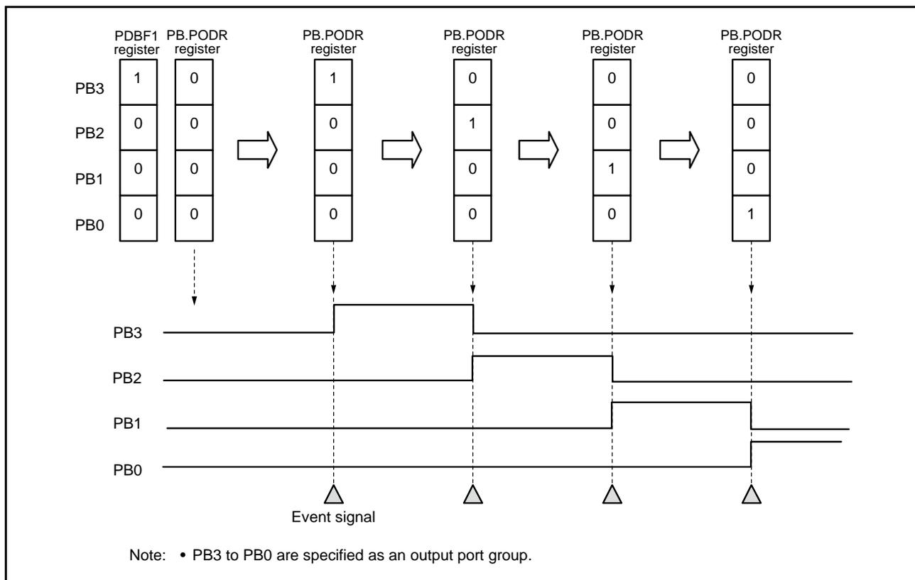
Figure 18.6 Bit-Rotating Operation of Output Port Groups
