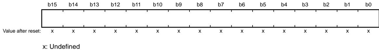
CRB is used to set the block transfer count for block transfer mode. The transfer count is 1, 65535, and 65536 when the set value is 0001h, FFFFh, and 0000h, respectively. The CRB value is decremented (-1) when the final data of a single block size is transferred. When normal transfer mode or repeat transfer mode is selected, this register is not used and the set value is ignored. CRB cannot be accessed directly from the CPU.
