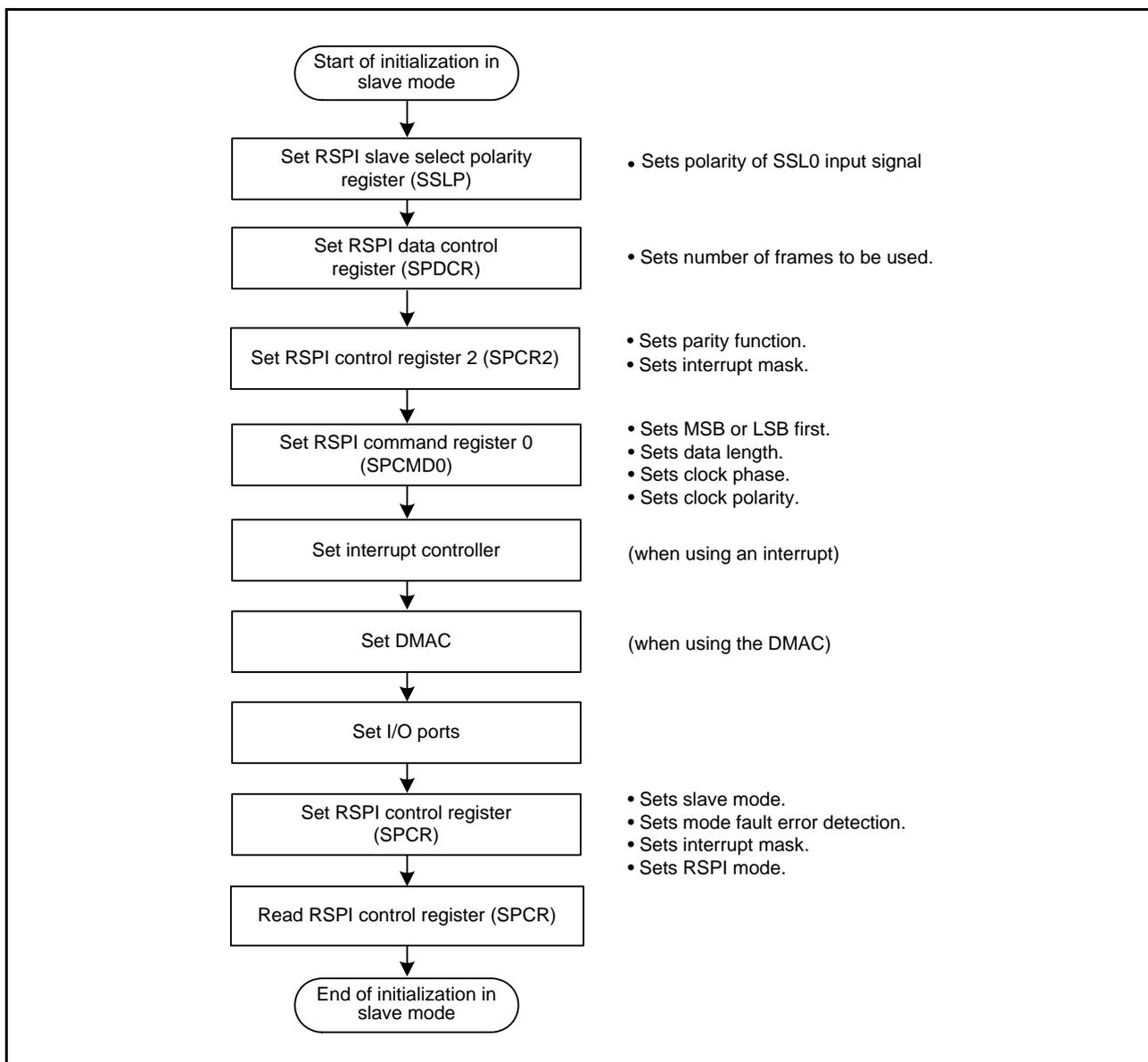
Figure 30.38 Example of Initialization Flowchart in Slave Mode (SPI Operation)
