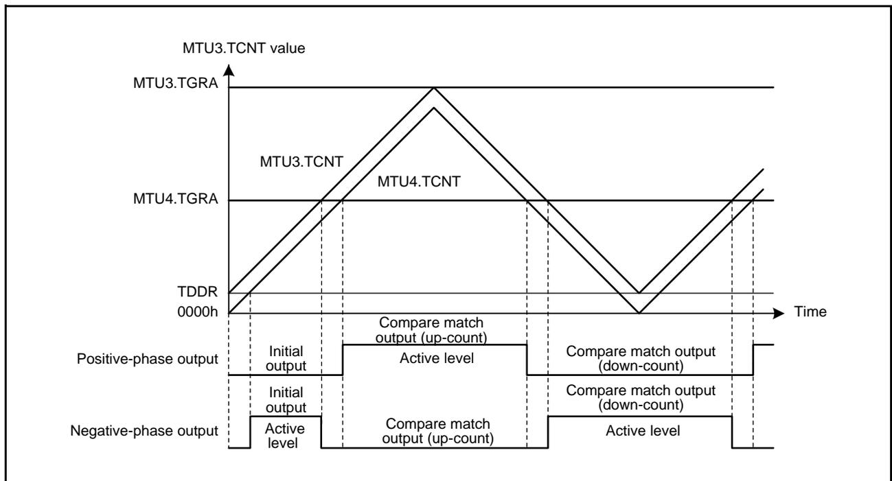
**Figure 21.2 Example of Output in Complementary PWM Mode**
