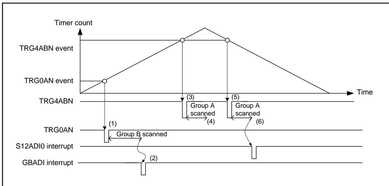
**Figure 32.10** Example of Operation in Group Scan Mode with Double Trigger Mode (Basic Operation: MTU Triggers Used)
