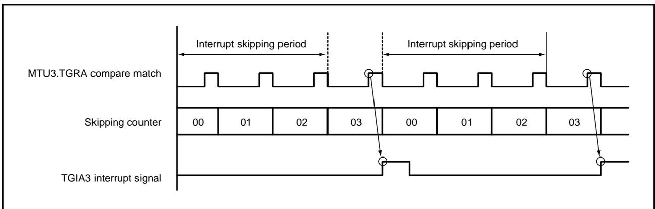
**Figure 21.69** Example of Interrupt Skipping Operation
