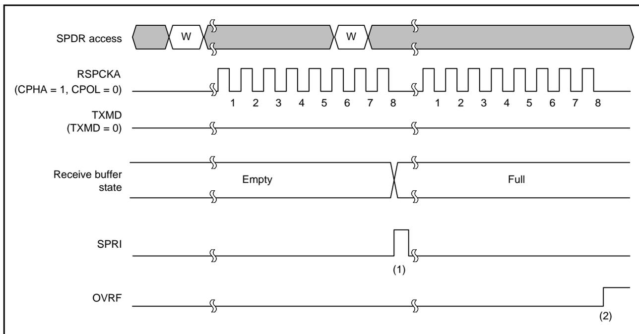
Figure 30.25 Operation Example of SPCR.TXMD = 0
