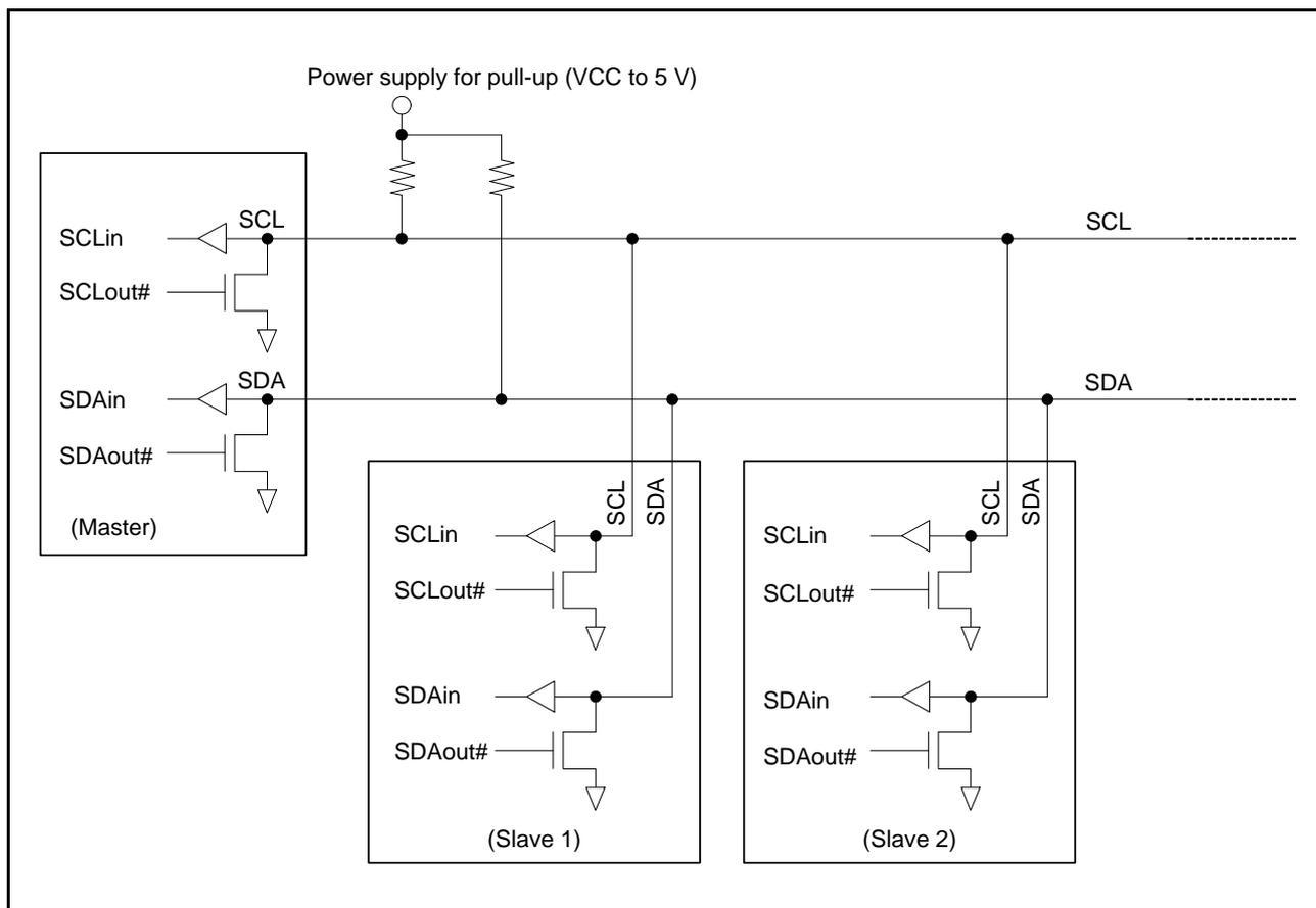
**Figure 29.2** Connections to the External Circuit by the I/O Pins (I<sup>2</sup>C Bus Configuration Example)
