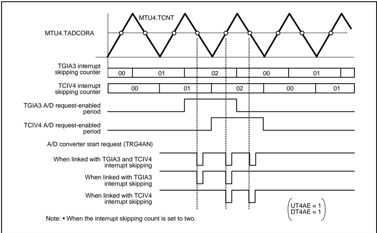
**Figure 21.75 Example of A/D Converter Start Request Signal (TRG4AN) Operation Linked with Interrupt Skipping (when the output of TRG4AN in counting up and down by TCNT is enabled)**
