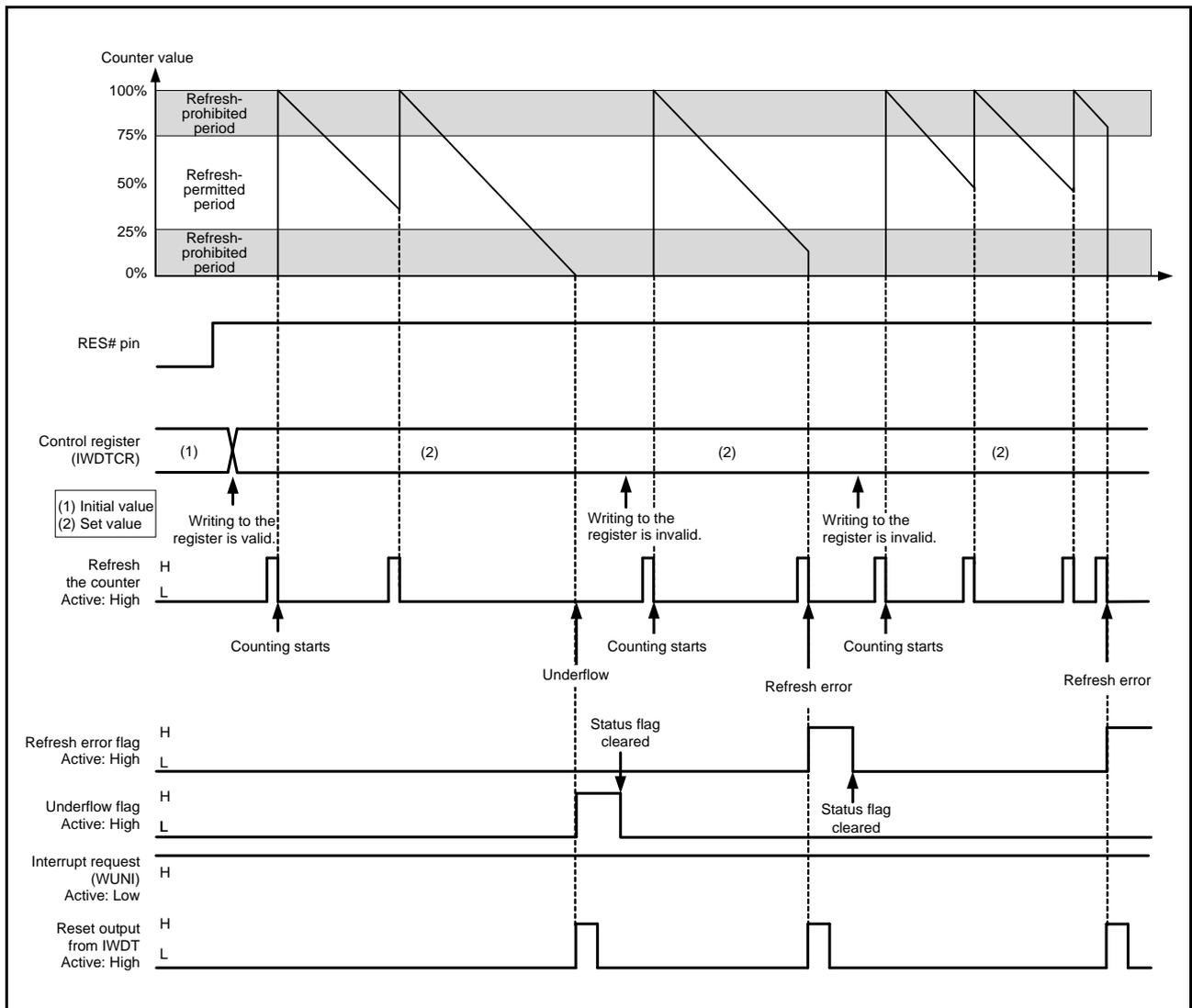
Figure 26.3 Operation Example in Register Start Mode
