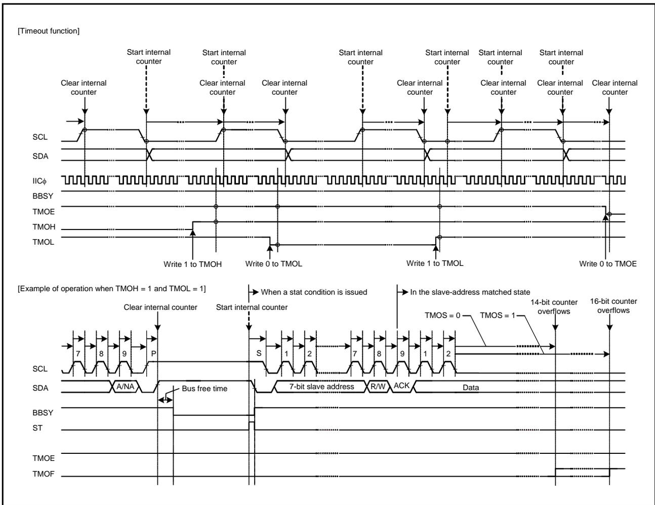
Figure 29.39 Timeout Function (TMOE, TMOS, TMOH, and TMOL Bits)
