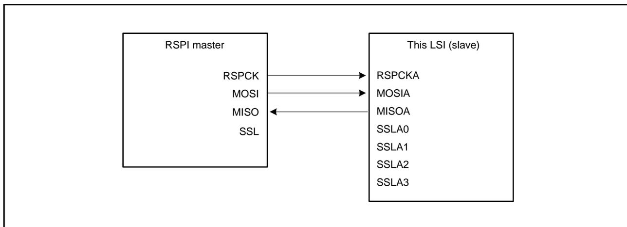
**Figure 30.12 Master (Clock Synchronous Operation)/Slave (Clock Synchronous Operation) Configuration Example (This LSI = Slave, CPHA = 1)**
