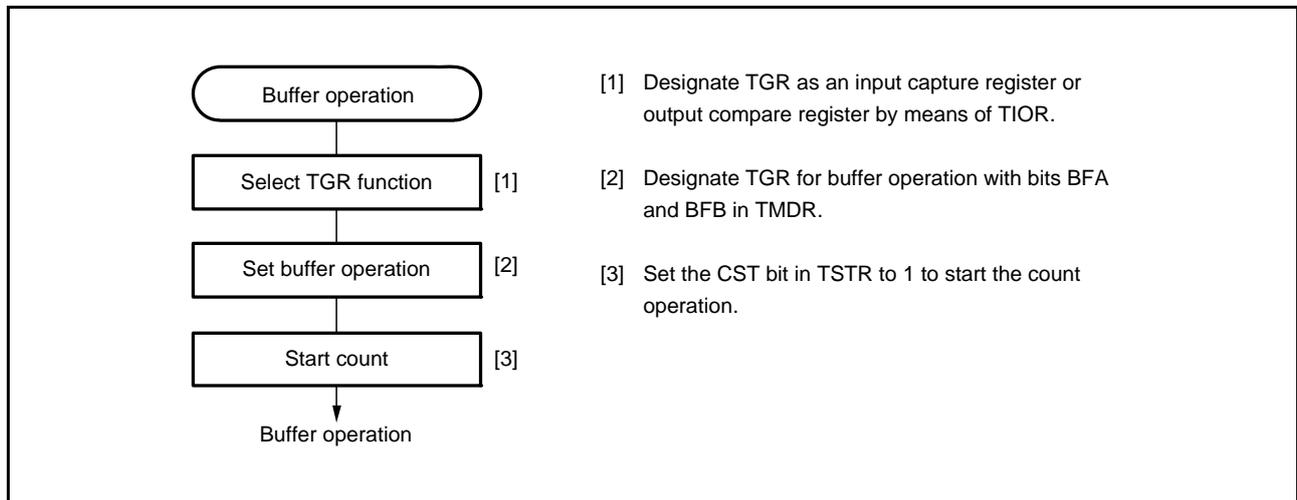
Figure 21.16 Example of Buffer Operation Setting Procedure
