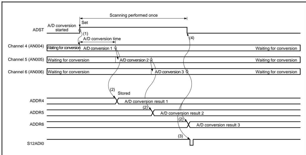
Figure 32.3 Example of Operation in Single Scan Mode (Basic Operation: AN004 to AN006 Selected)
