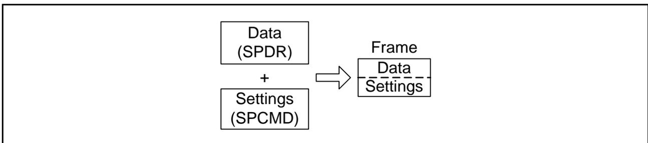
Figure 30.31 Concept of a Frame
