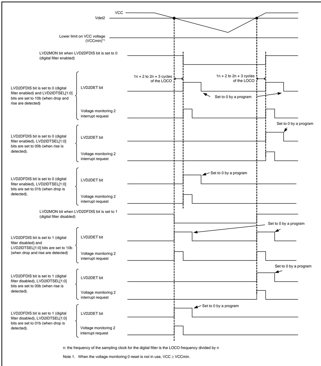
Figure 8.6 Example of Voltage Monitoring 2 Interrupt Operation
