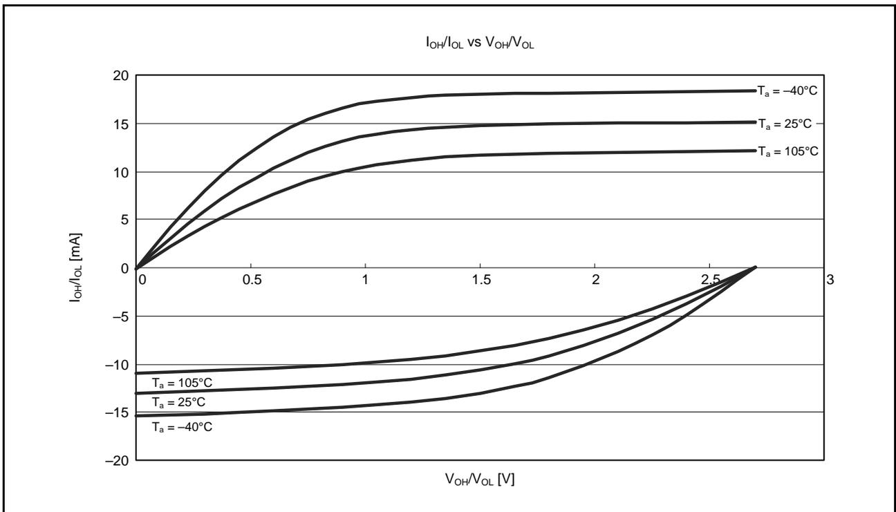
Figure 38.9  $V_{OH}/V_{OL}$  and  $I_{OH}/I_{OL}$  Temperature Characteristics at  $V_{CC} = 2.7\text{ V}$  when Normal Output is Selected (Reference Data)
