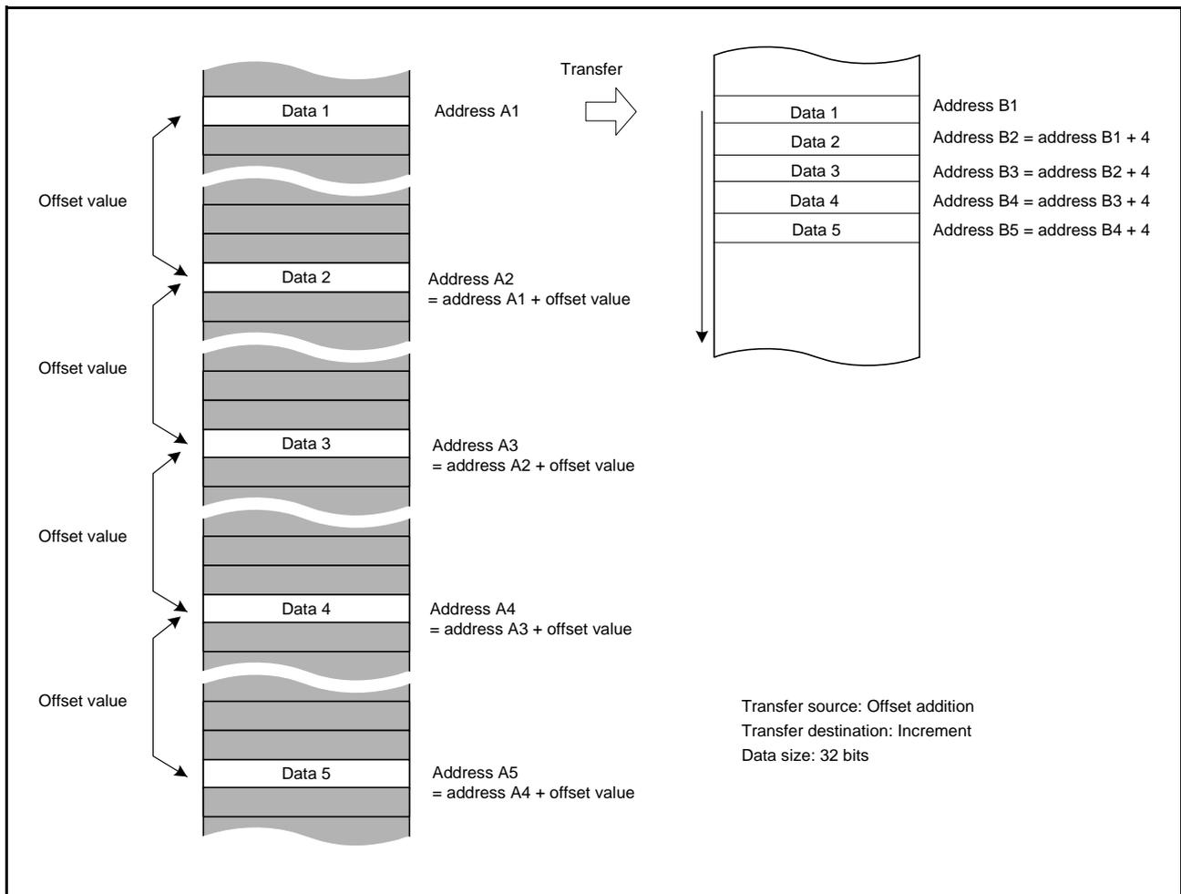
Figure 16.7 Example of Address Updating by Offset Addition
