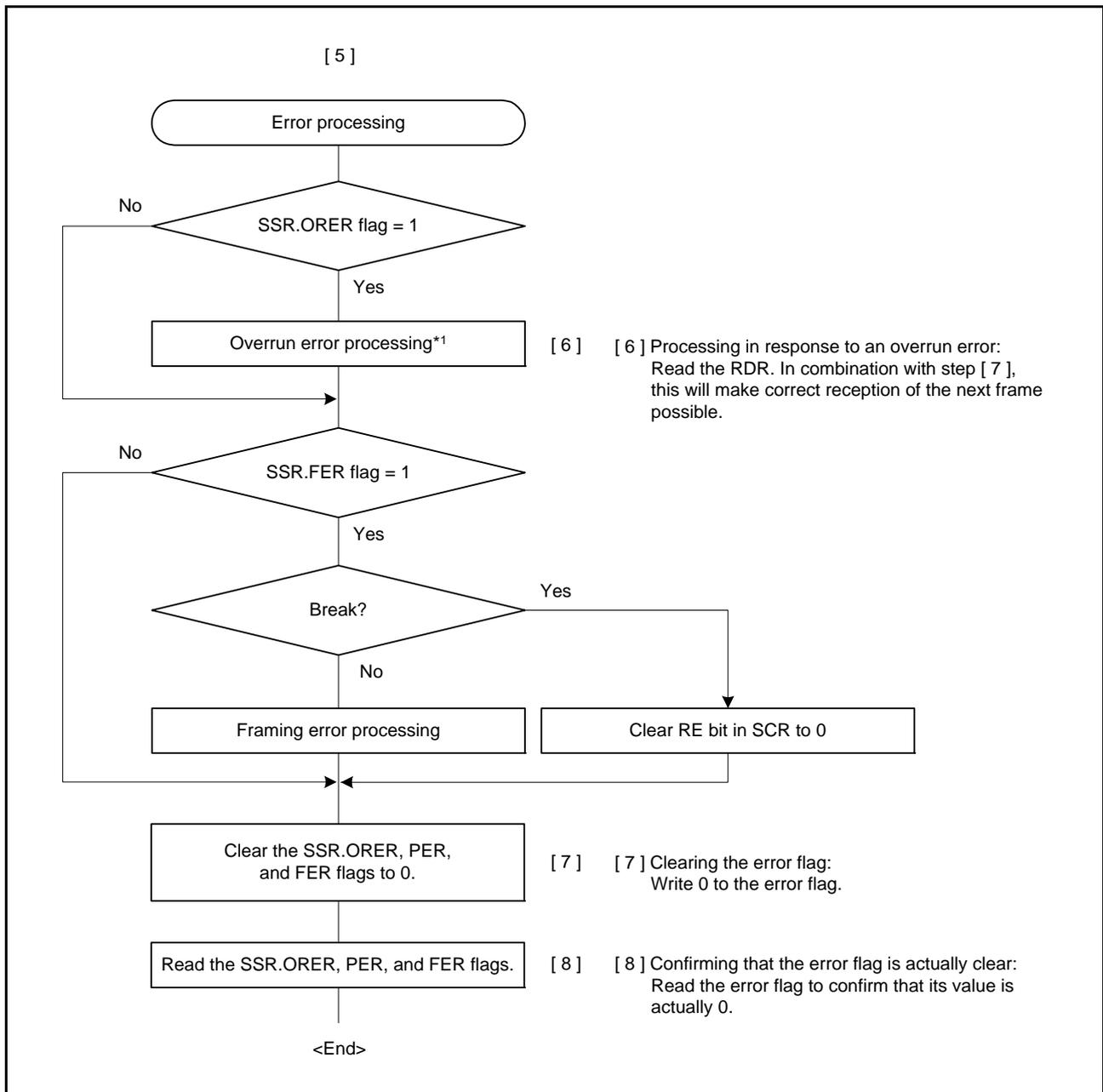
Figure 27.19 Example of Multi-Processor Serial Reception Flowchart (2)
