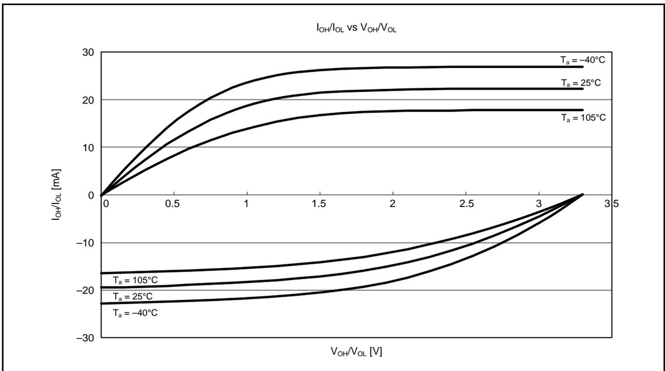
Figure 38.10  $V_{OH}/V_{OL}$  and  $I_{OH}/I_{OL}$  Temperature Characteristics at  $V_{CC} = 3.3\text{ V}$  when Normal Output is Selected (Reference Data)
