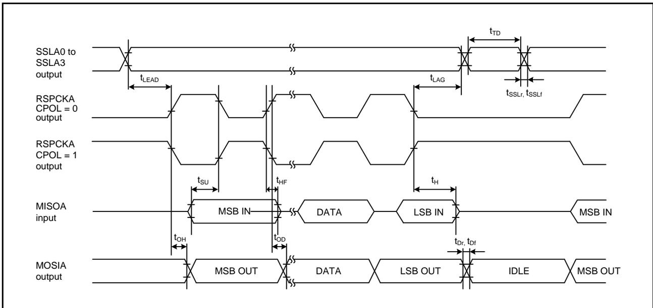
**Figure 38.45 RSPI Timing (Master, CPHA = 1) (Bit Rate: PCLKB Set to Divided by 2)**
