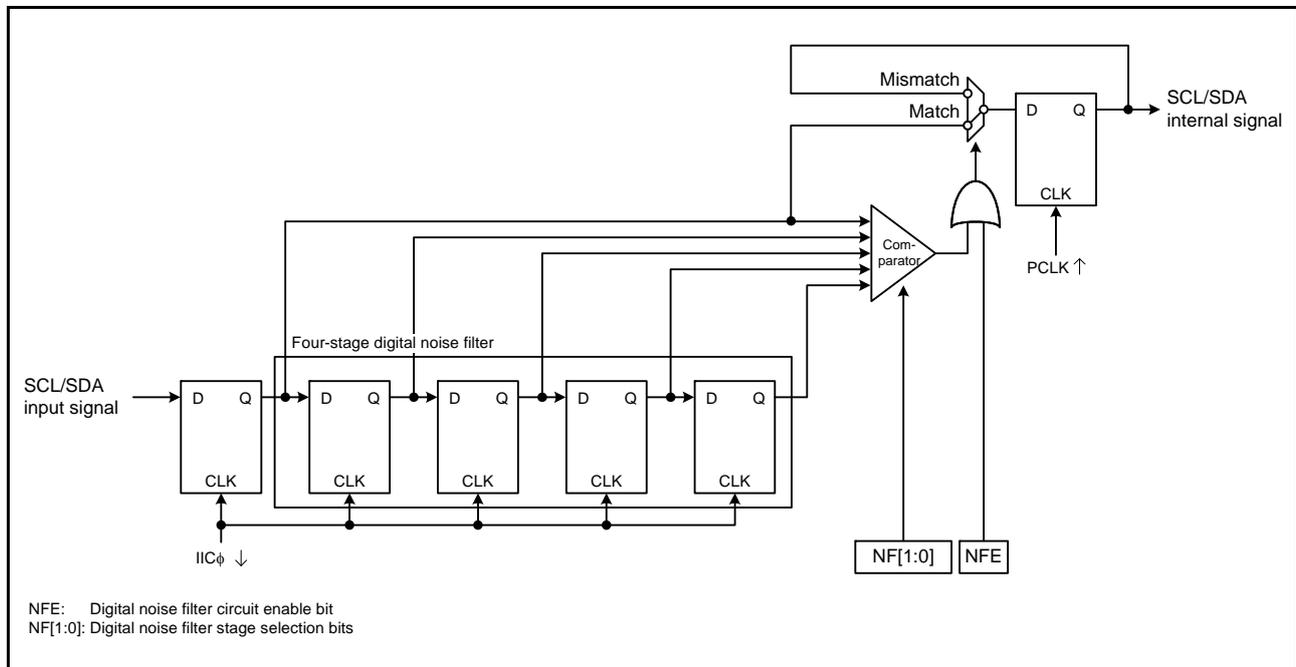
**Figure 29.23** Block Diagram of Digital Noise Filter Circuit
