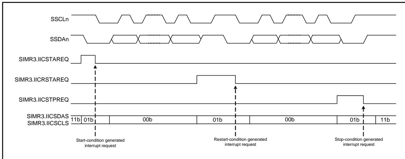
**Figure 27.42** Timing of Operations in the Generation of Start, Restart, and Stop Conditions
