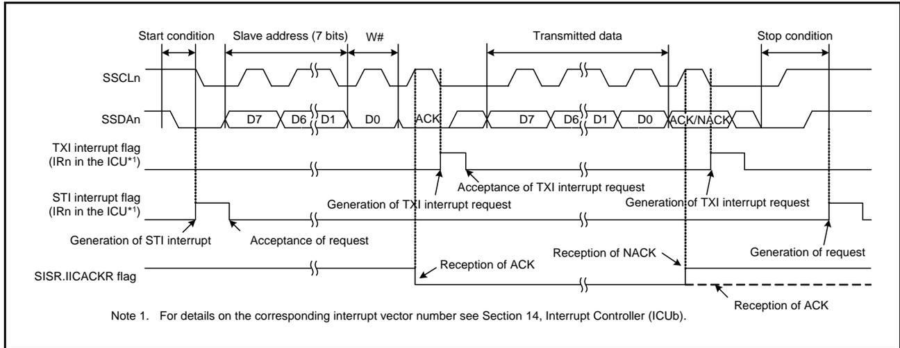
**Figure 27.46 Example of Operations for Master Transmission in I<sup>2</sup>C Bus Mode (with Seven-Bit Slave Addresses, Transmission Interrupts, and Reception Interrupts in Use)**
