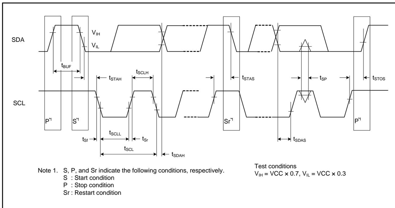
Figure 38.48 RIIC Bus Interface Input/Output Timing and Simple IIC Bus Interface Input/Output Timing
