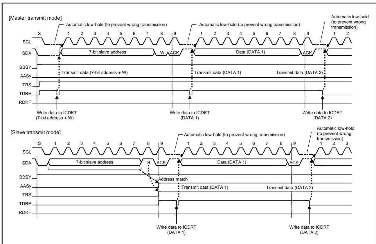
Figure 29.30 Automatic Low-Hold Operation in Transmit Mode
