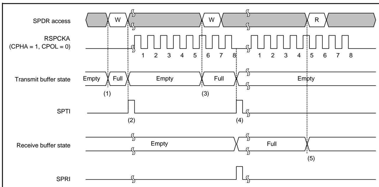
**Figure 30.27** Operation Example of SPTI and SPRI Interrupts
