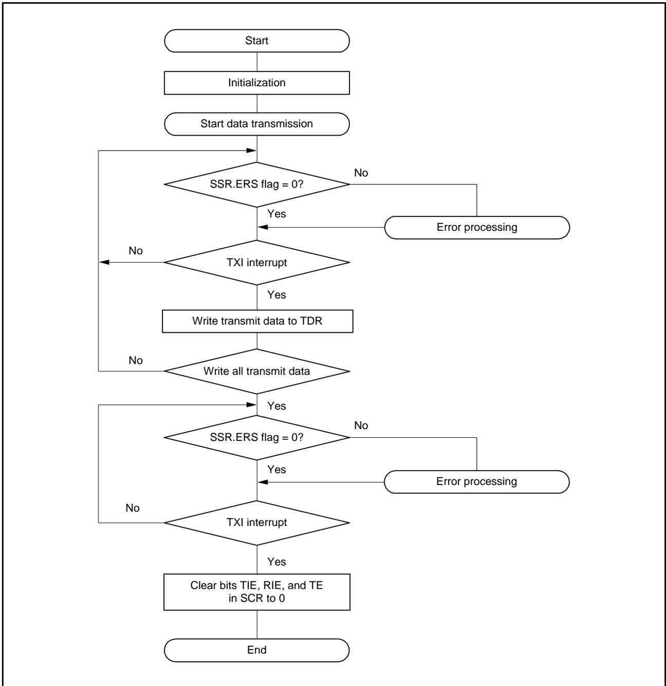
Figure 27.35 Sample Smart Card Interface Transmission Flowchart
