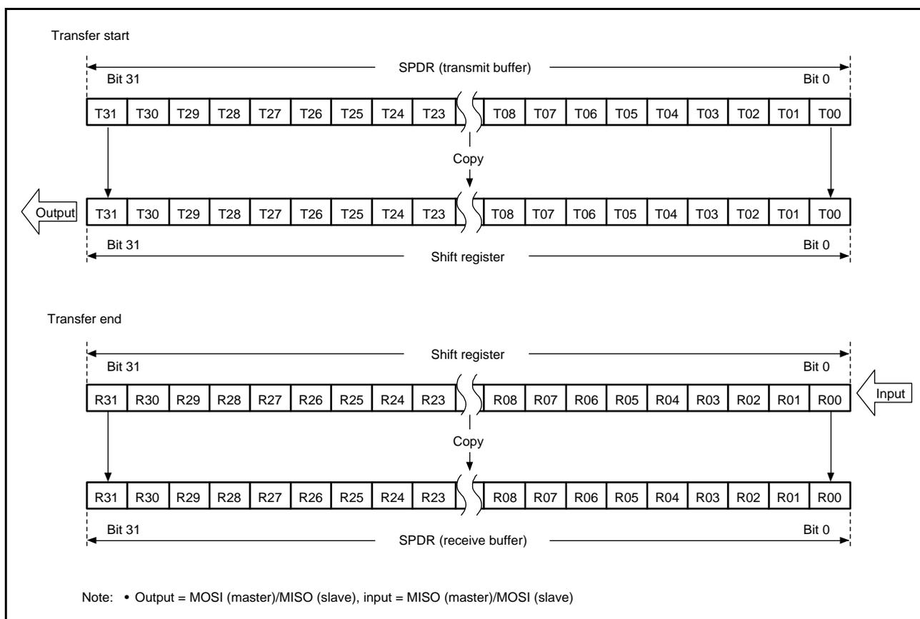
Figure 30.15 MSB-First Transfer (32-Bit Data, Parity Disabled)
