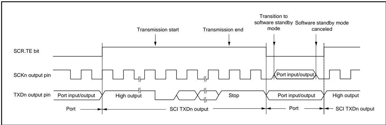
**Figure 27.70 Port Pin States during Transition to Software Standby Mode (Internal Clock, Asynchronous Transmission)**
