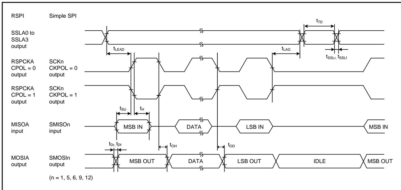
**Figure 38.42 RSPI Timing (Master, CPHA = 0) (Bit Rate: PCLKB Set to Division Ratio Other Than Divided by 2) and Simple SPI Timing (Master, CKPH = 1)**
