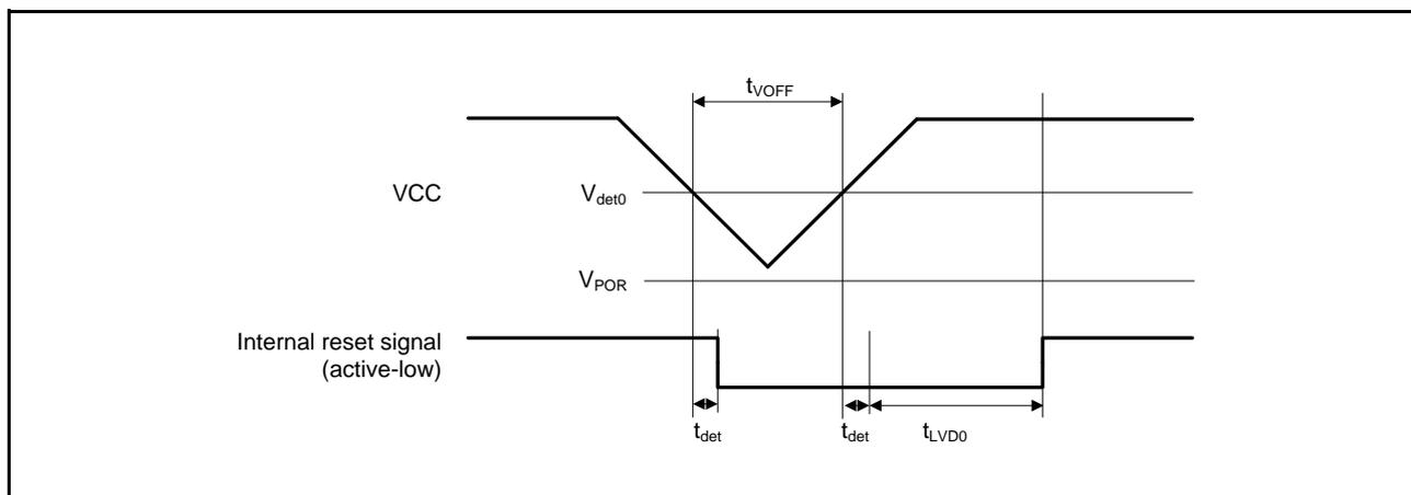
Figure 38.53 Voltage Detection Circuit Timing (V<sub>det0</sub>)
