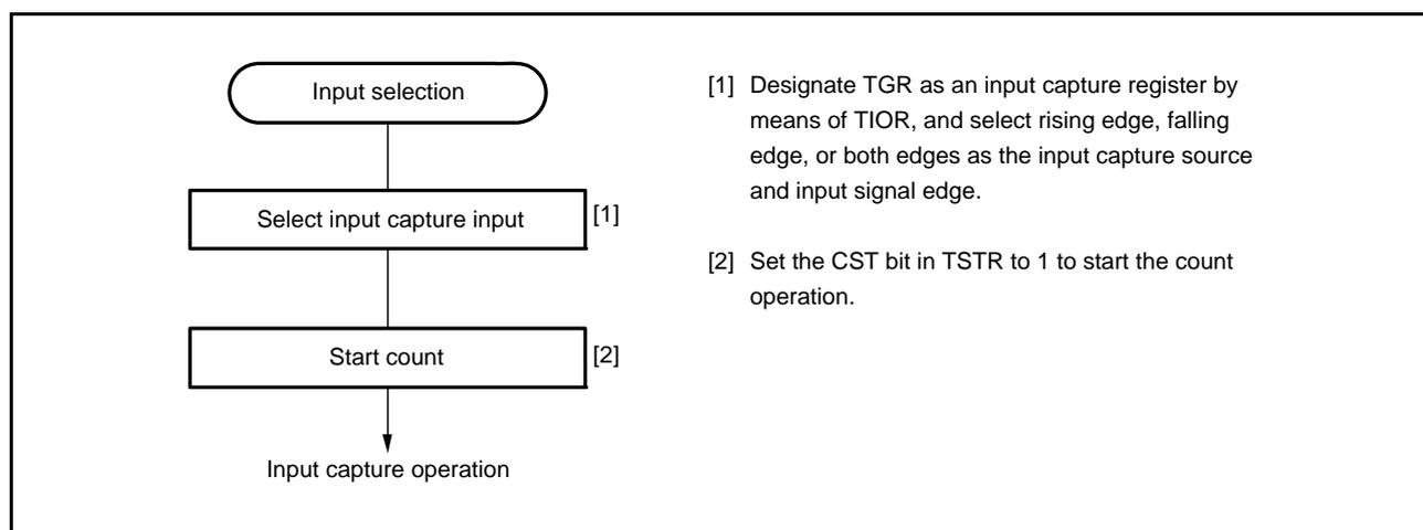
**Figure 21.10 Example of Input Capture Operation Setting Procedure**
