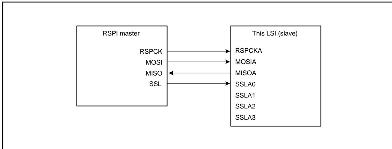
Figure 30.6 Single-Master/Single-Slave Configuration Example (This LSI = Slave, CPHA = 0)
