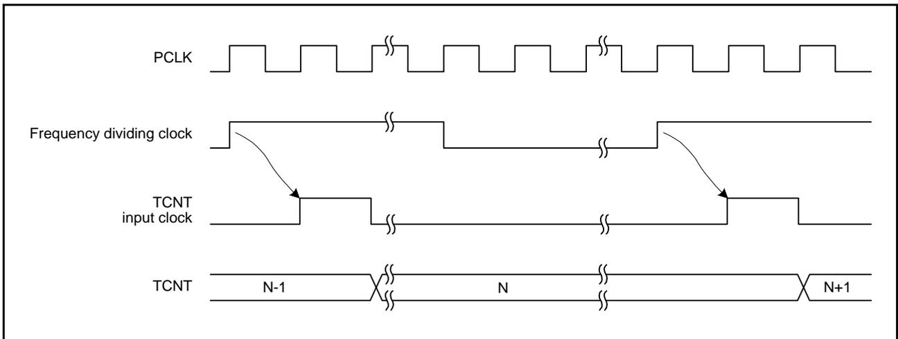
Figure 23.5 Count Timing for Frequency Dividing Clock Input
