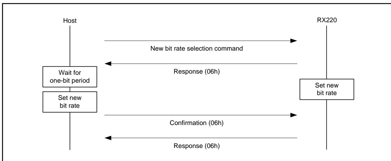
Figure 36.27 New Bit Rate Selection Sequence
