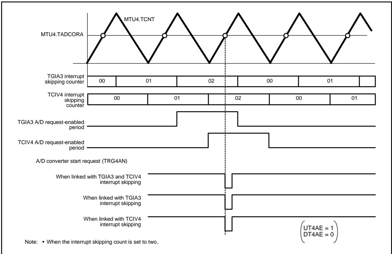
**Figure 21.76 Example of A/D Converter Start Request Signal (TRG4AN) Operation Linked with Interrupt Skipping (when the output of TRG4AN in counting up by TCNT is enabled)**
