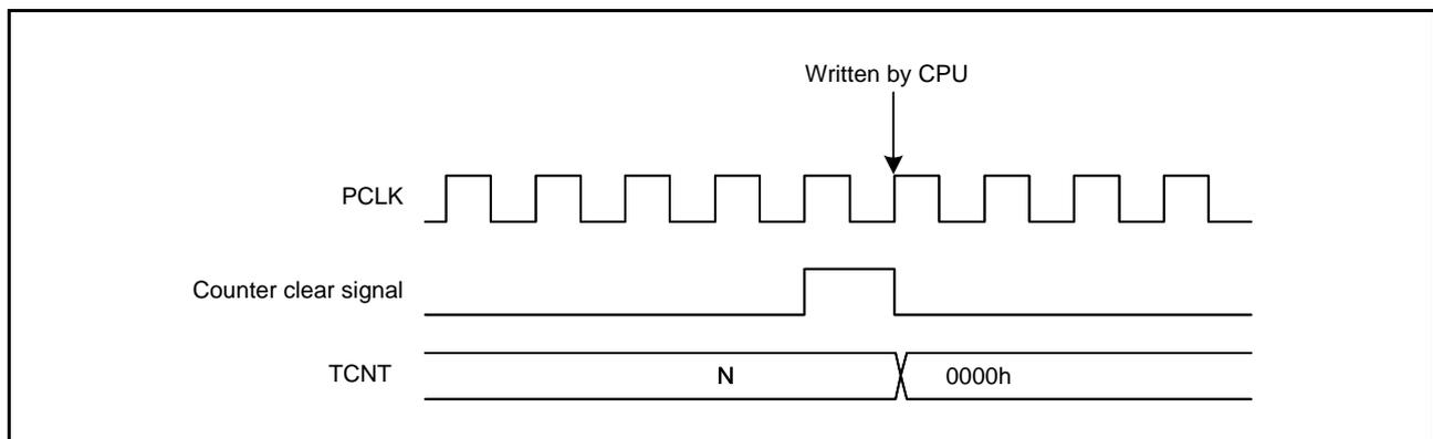
Figure 21.107 Contention between TCNT Write and Counter Clear Operations
