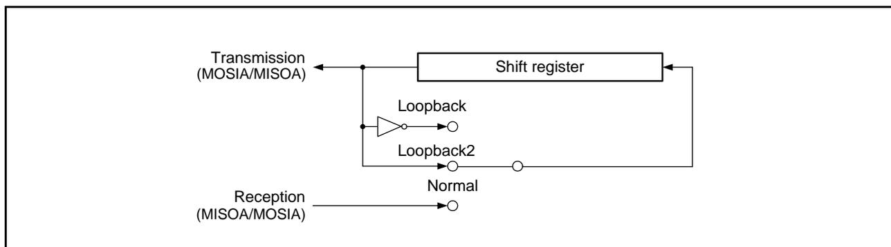
**Figure 30.47 Configuration of Shift Register I/O Paths in Loopback Mode (Master Mode)**
