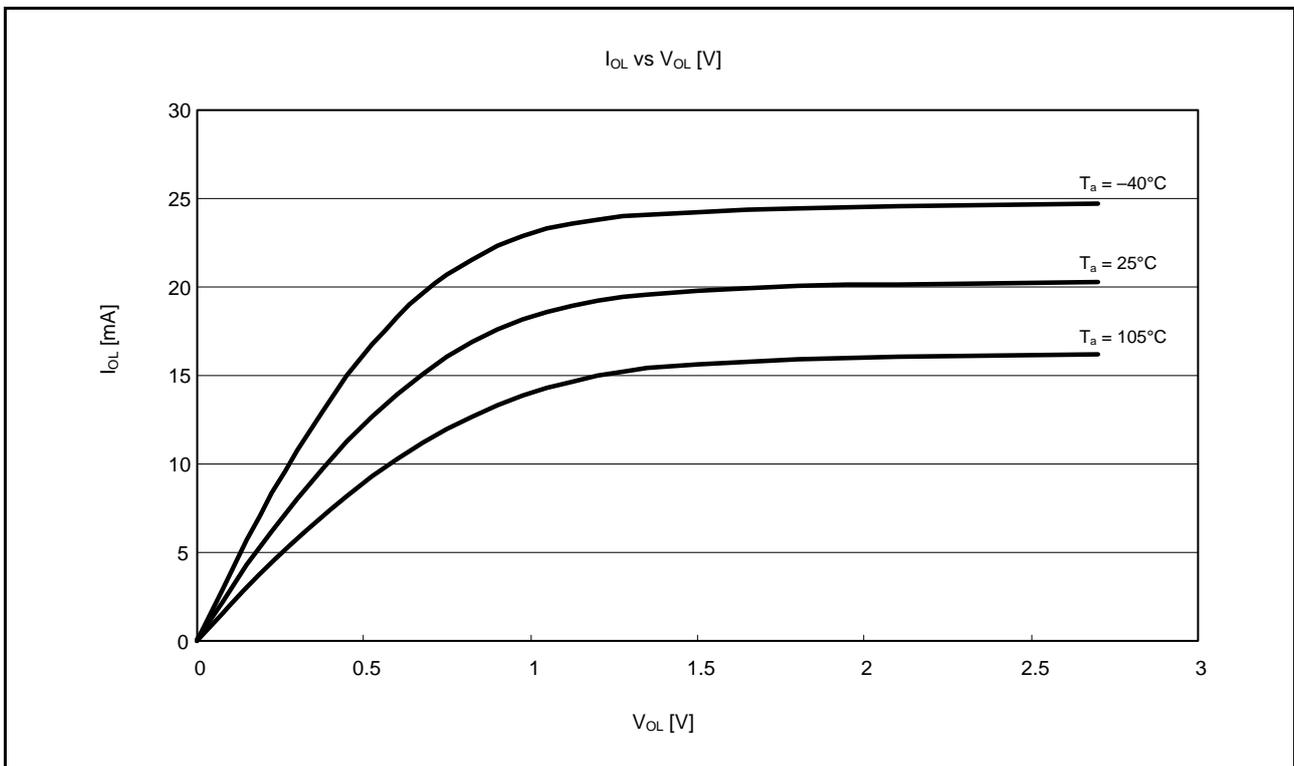
Figure 38.18 V<sub>OL</sub> and I<sub>OL</sub> Temperature Characteristics of RIIC Output Pin at VCC = 2.7 V (Reference Data)
