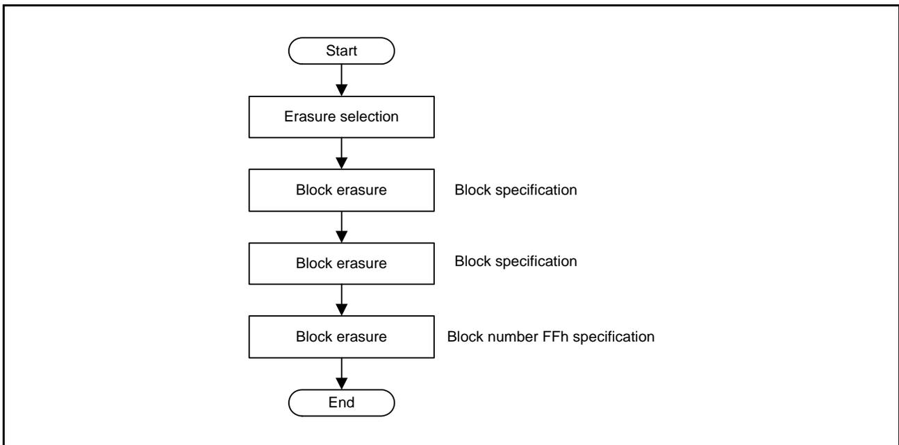
**Figure 36.29 Procedure for ROM Erasure in Boot Mode**
