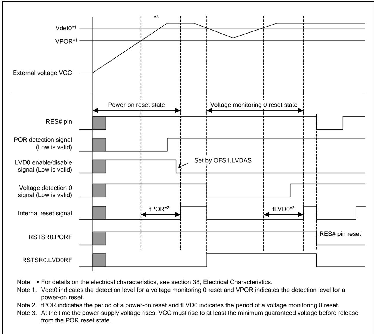
Figure 8.4 Example of Voltage Monitoring 0 Reset Operation
