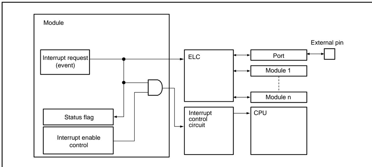
Figure 18.2 Relation between Interrupt Processing and ELC
