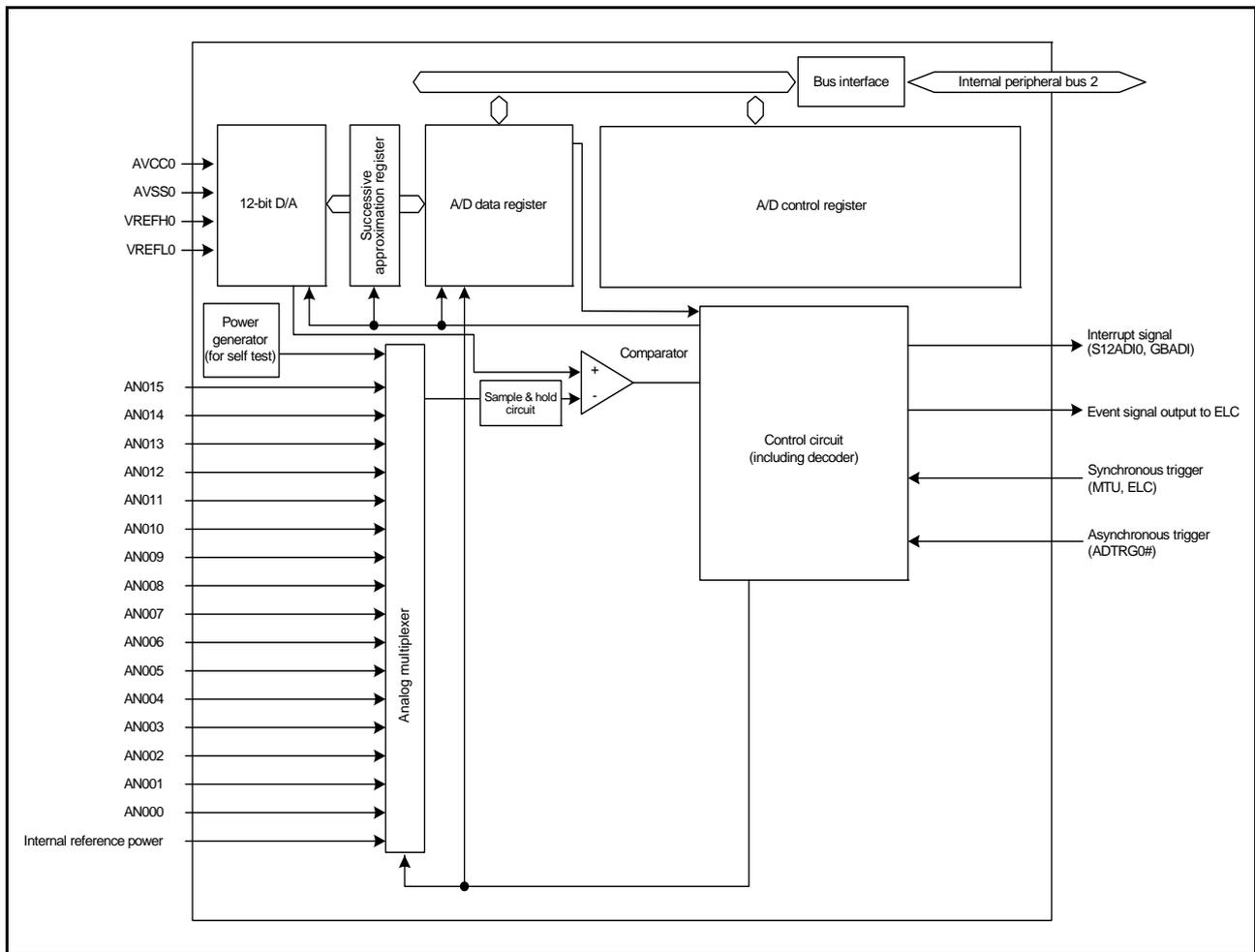
Figure 32.1 Block Diagram of 12-Bit A/D Converter
