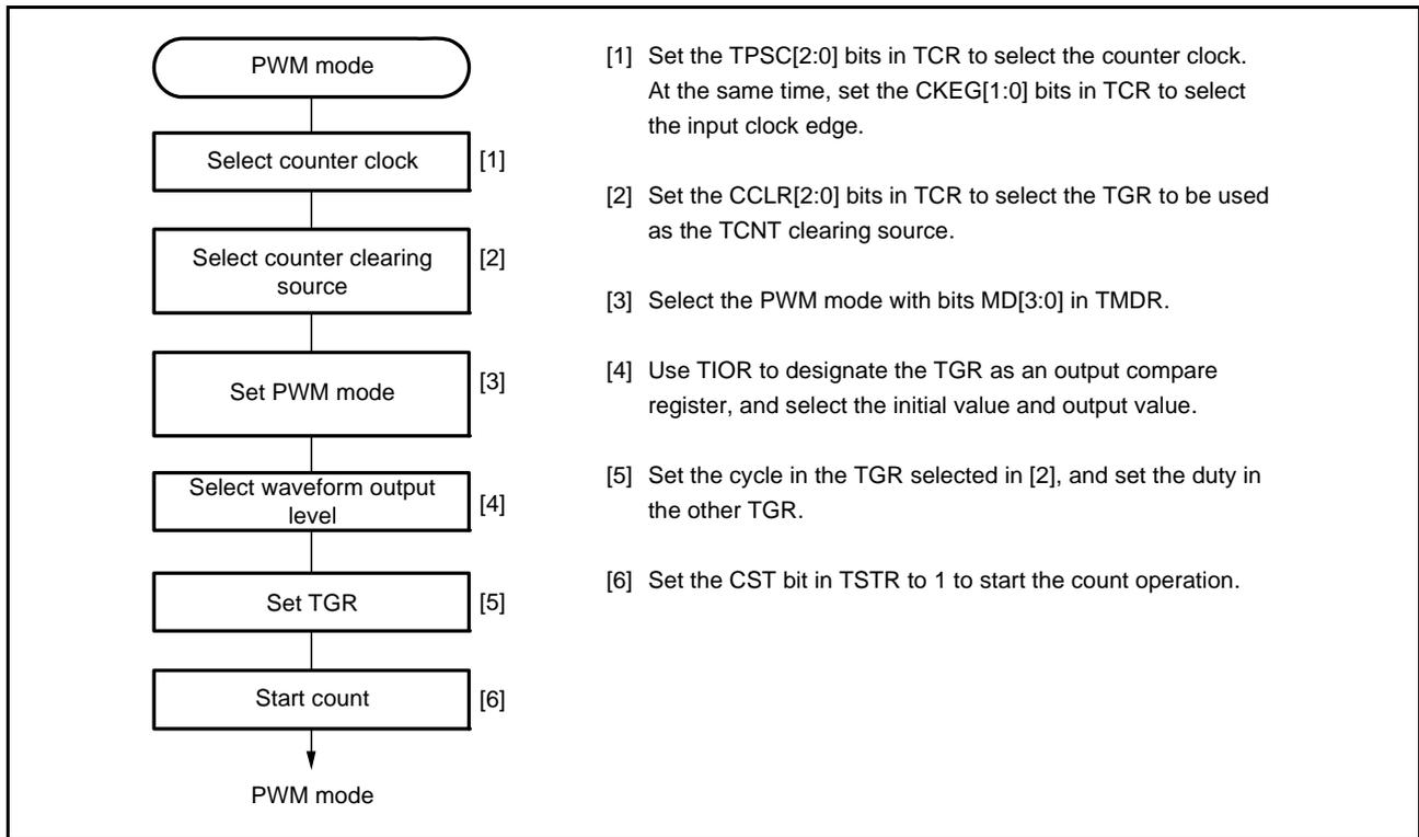
Figure 21.25 Example of PWM Mode Setting Procedure
