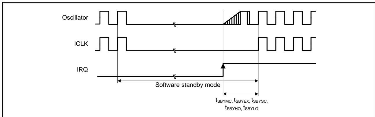
**Figure 38.30 Software Standby Mode Cancellation Timing**
