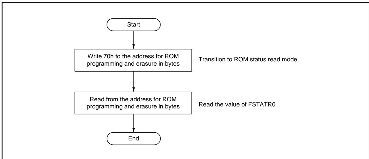
**Figure 36.8 Procedure for Transition to ROM Status Read Mode and the Status Checking**
