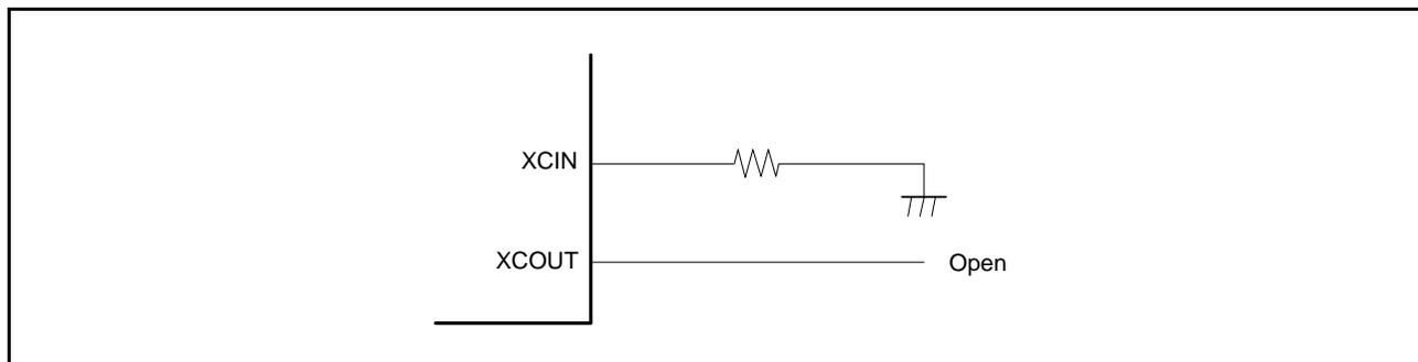
Figure 9.7 Pin Handling when Sub-Clock is not Used
