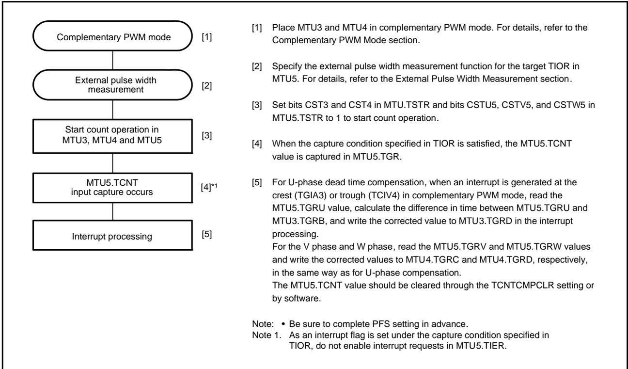
Figure 21.80 Example of Dead Time Compensation Setting Procedure
