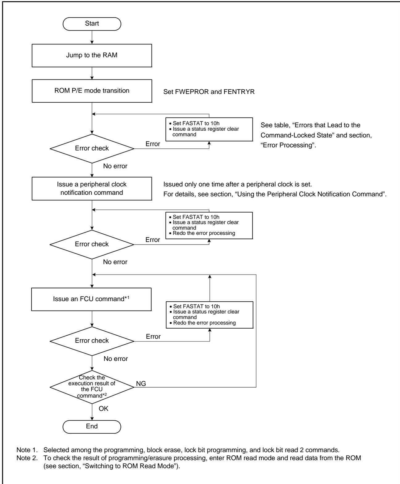
Figure 36.10 Simple Flowchart of the Procedure for Programming and Erasure
