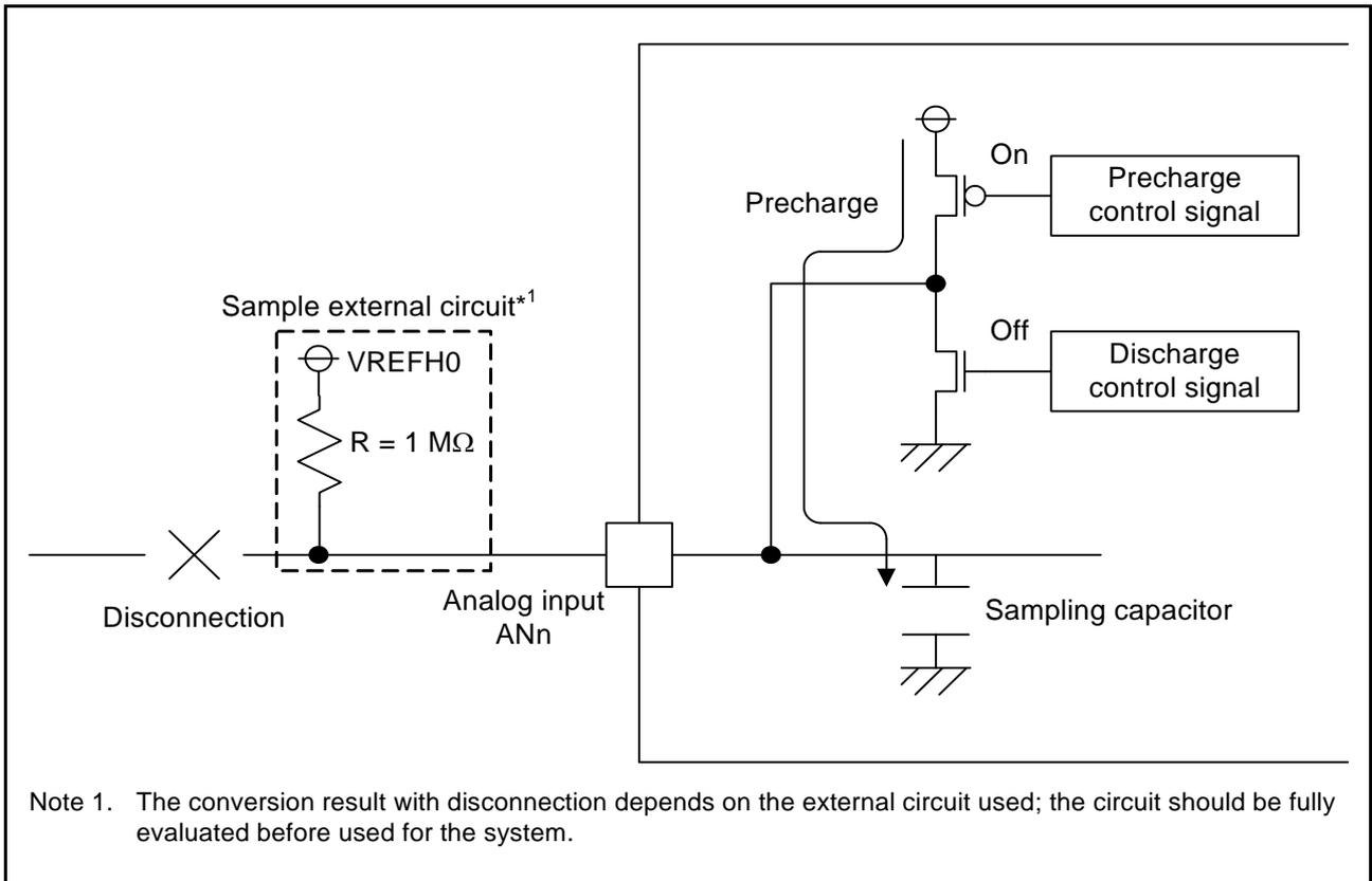
Figure 32.14 VREFH0 Disconnection Detection Example (Precharge Selected)
