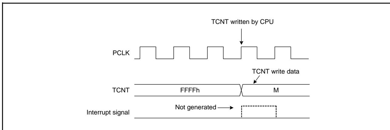
Figure 21.121 Contention between TCNT Write Operation and Overflow
