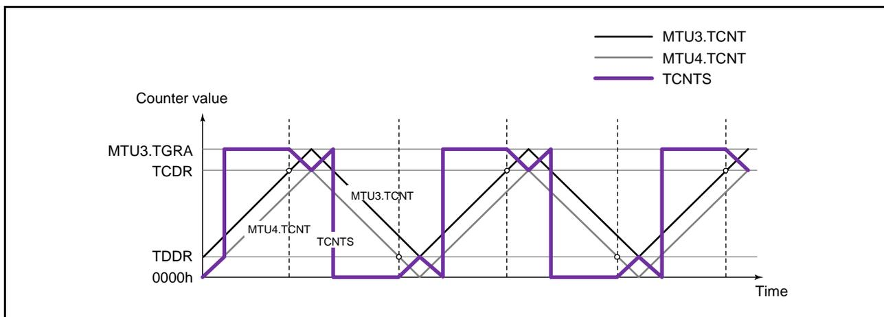
Figure 21.39 Counter Operation in Complementary PWM Mode
