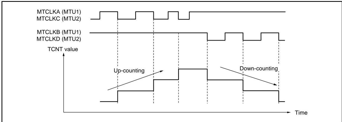
Figure 21.32 Example of Operation in Phase Counting Mode 3
