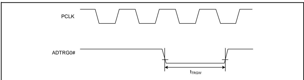
Figure 38.40 A/D Converter External Trigger Input Timing
