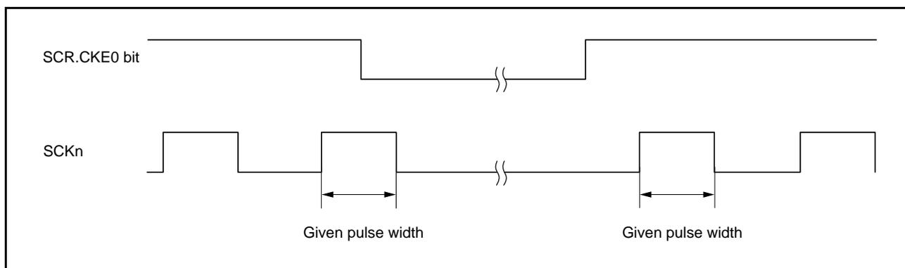
**Figure 27.38** Clock Output Fixing Timing
