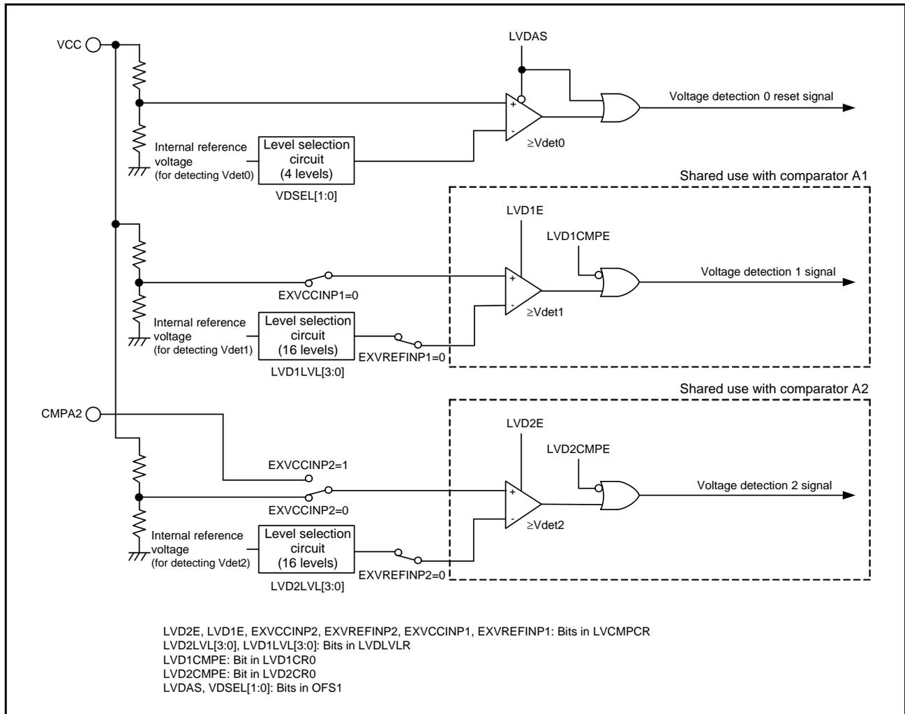
**Figure 8.1 Block Diagram of Voltage Detection Circuit**
