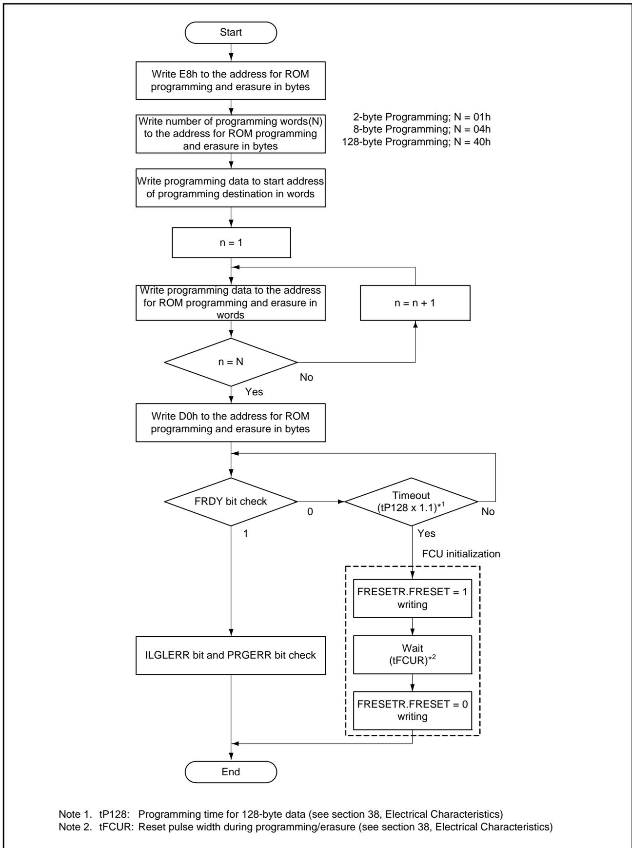
Figure 36.12 Procedure for ROM Programming
