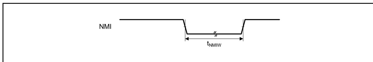
**Figure 38.31 NMI Interrupt Input Timing**
