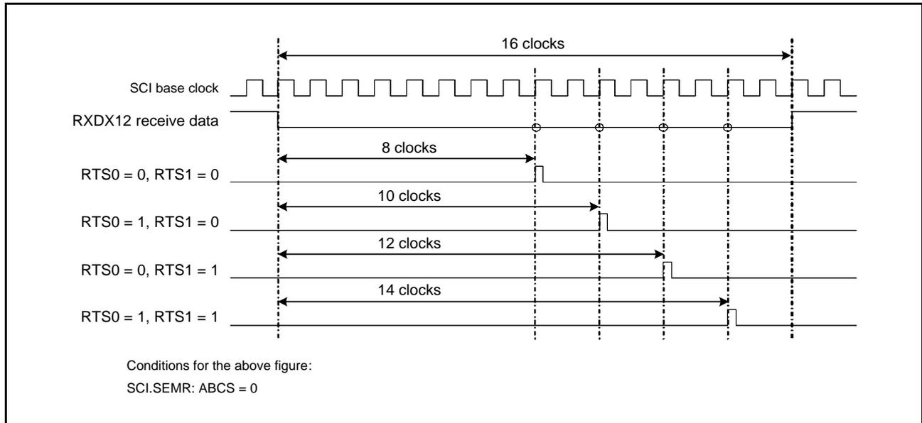
Figure 27.65 Timing for Sampling of Data Received through RXDX12
