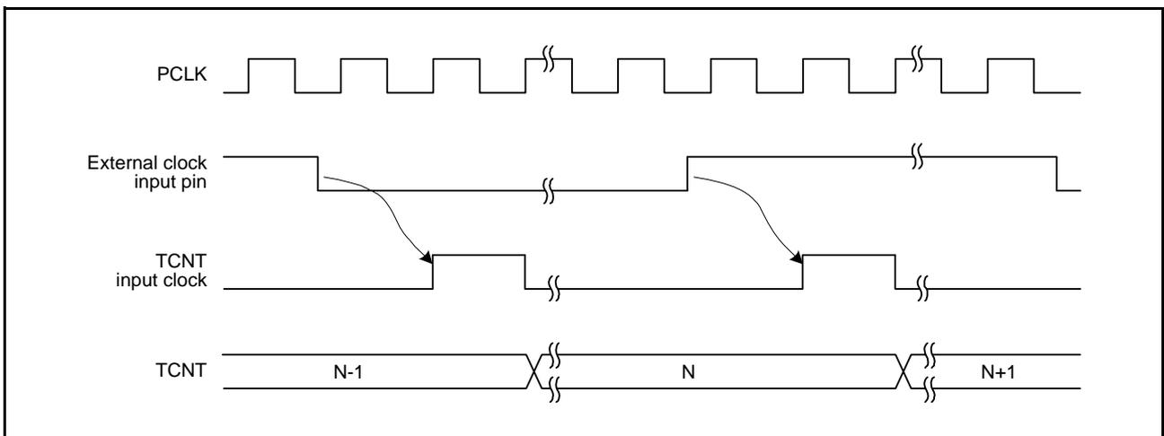
Figure 23.6 Count Timing for External Clock Input (at Both Edges)
