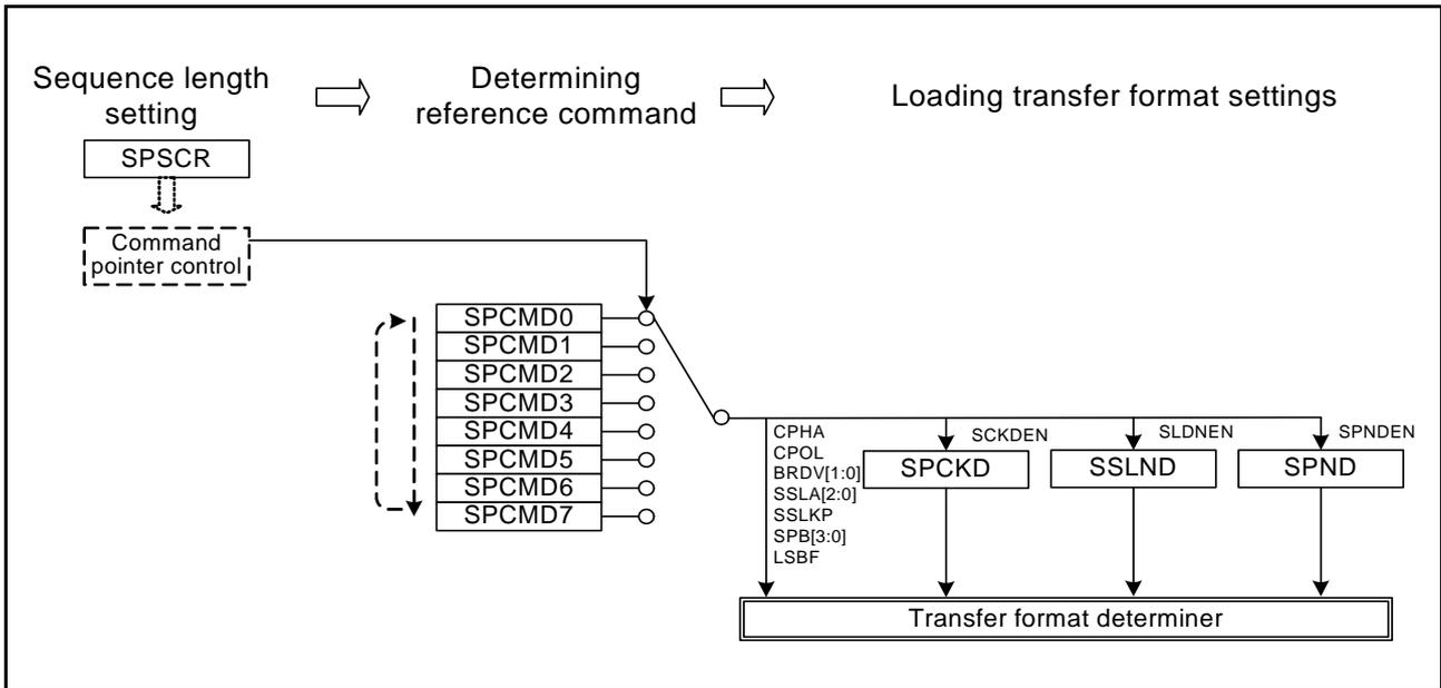
Figure 30.42 Procedure for Determining the Form of Serial Transmission in Master Mode
