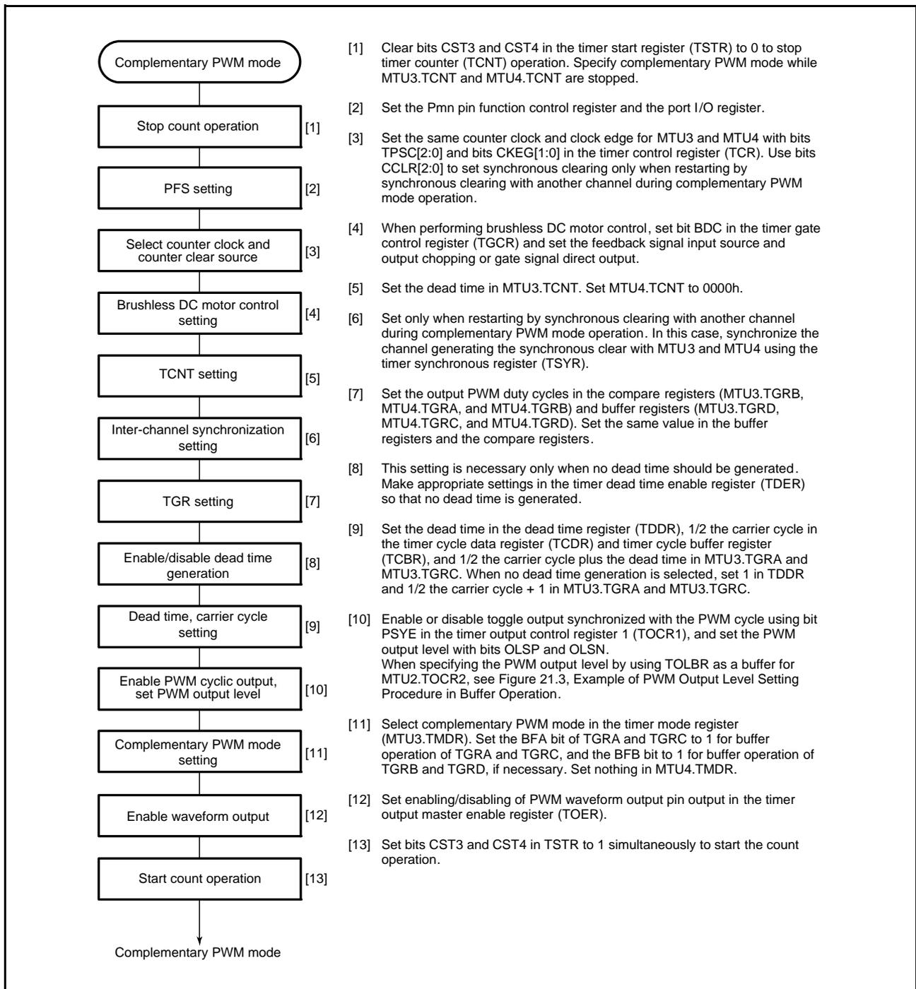
Figure 21.38 Example of Complementary PWM Mode Setting Procedure
