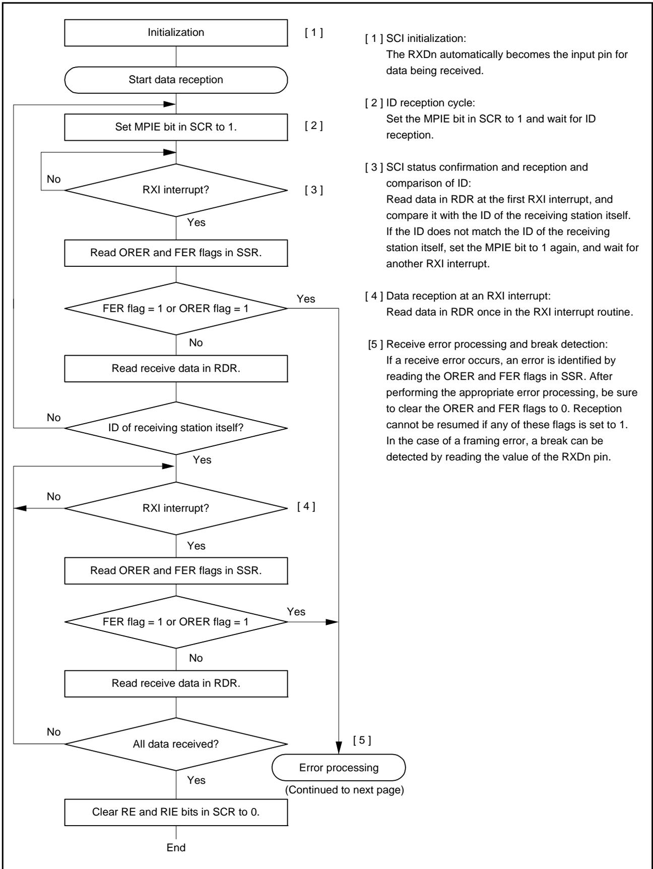
Figure 27.18 Example of Multi-Processor Serial Reception Flowchart (1)
