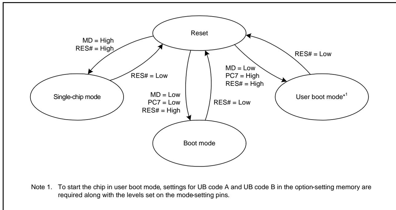
**Figure 3.1 Mode-Setting Pin Levels and Operating Modes**
