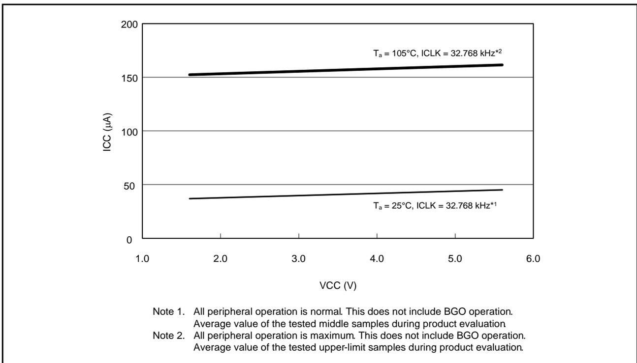
**Figure 38.3 Voltage Dependency in Low-Speed Operating Mode 2 (Reference Data)**
