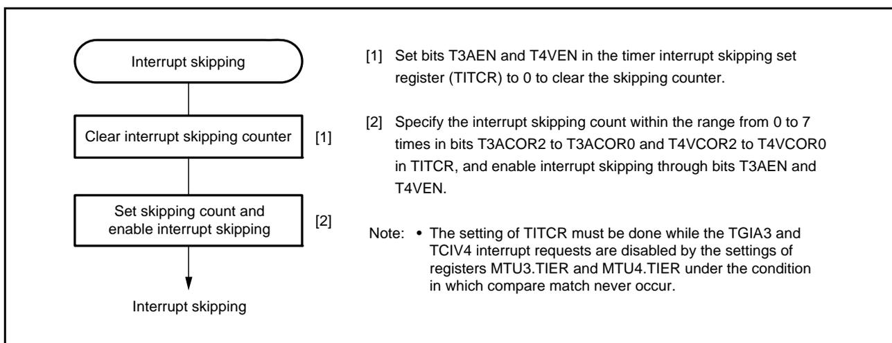
Figure 21.67 Example of Interrupt Skipping Operation Setting Procedure
