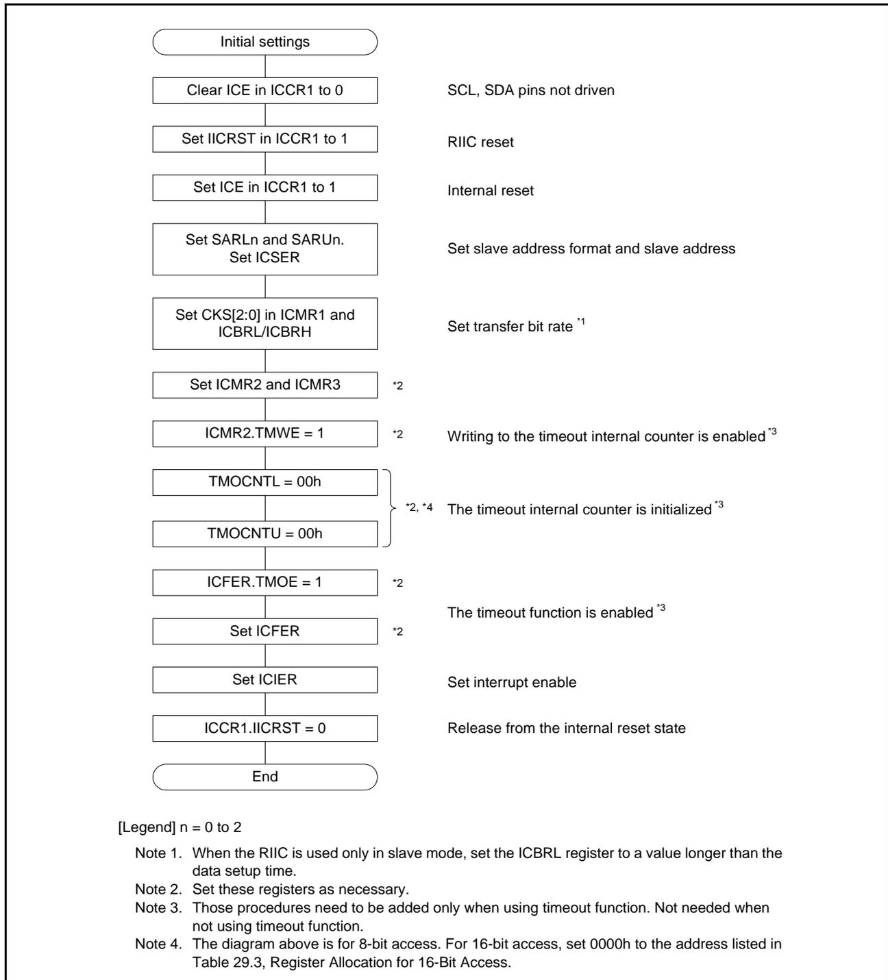
**Figure 29.5 Example of RIIC Initialization Flowchart**
