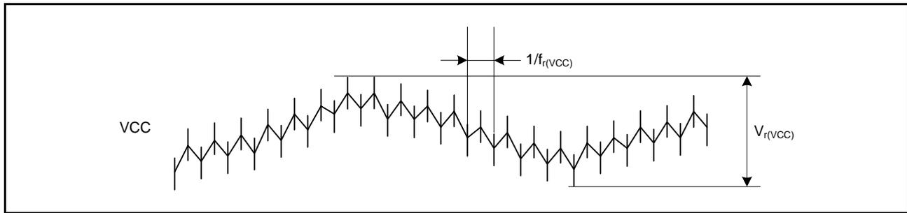
**Figure 38.6** Ripple Waveform
