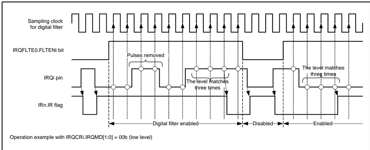
**Figure 14.8** Digital Filter Operation Example
