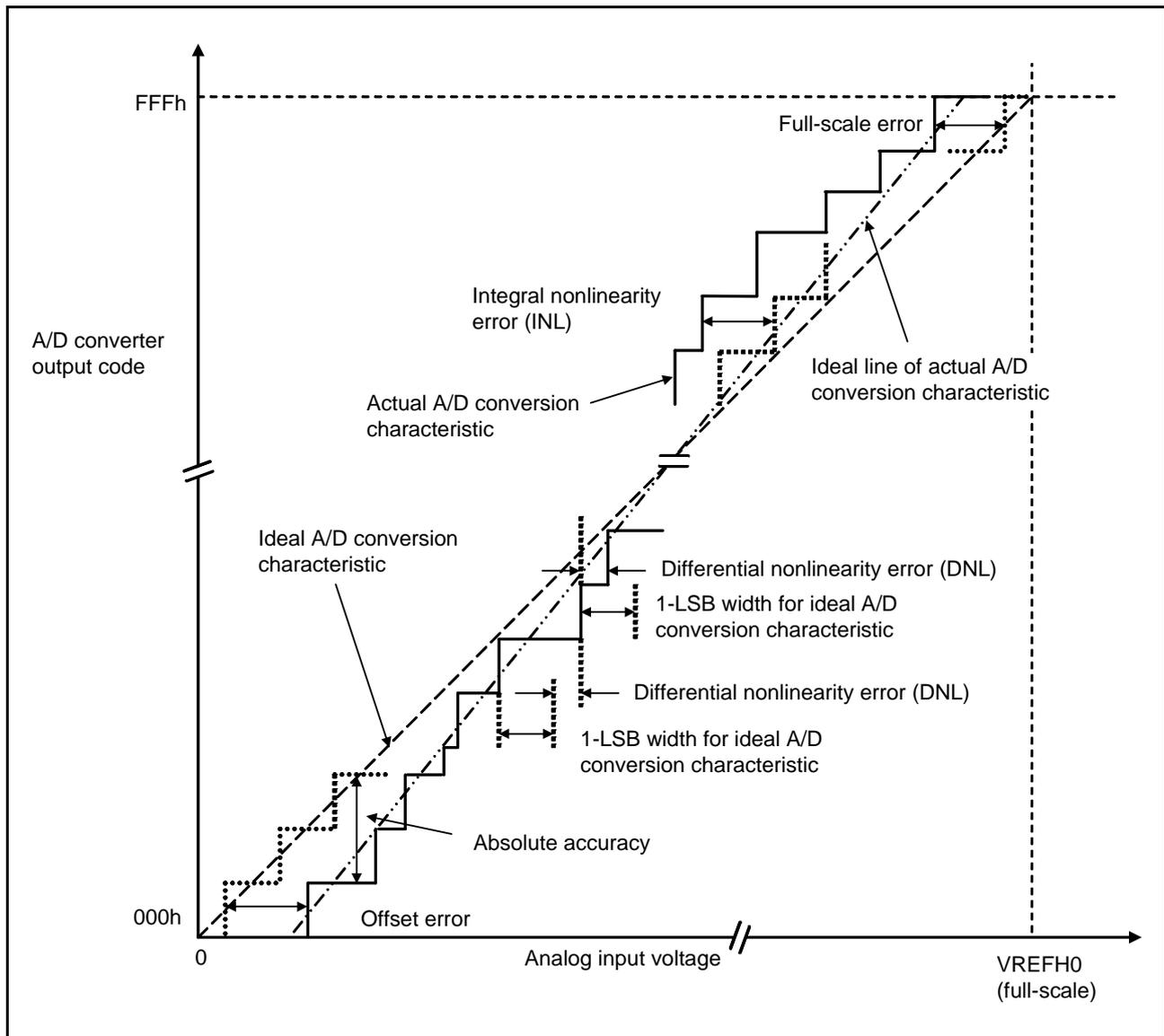
**Figure 38.50 Illustration of A/D Converter Characteristic Terms**
