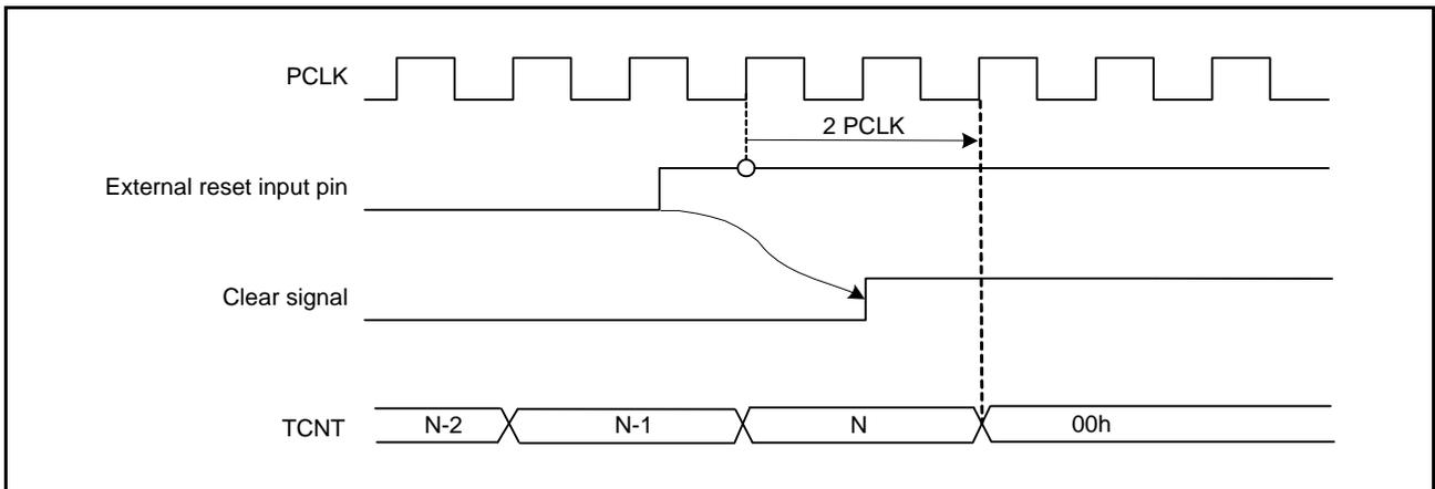
Figure 23.11 Timing of Clearance by External Reset (High Level)
