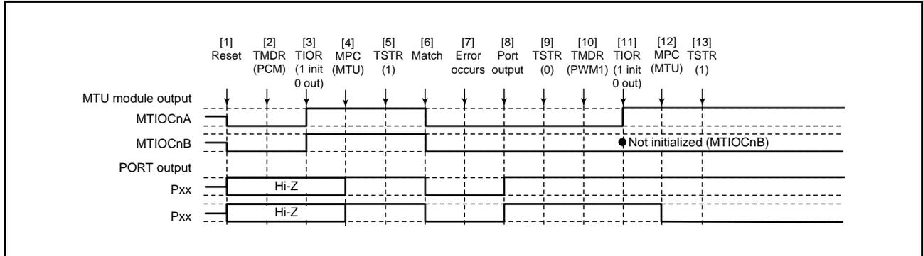
Figure 21.142 Error Occurrence in Phase Counting Mode, Recovery in PWM Mode 1
