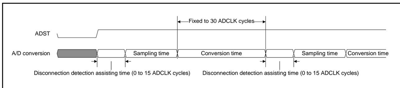
Figure 32.13 A/D Conversion with Disconnection Detection Assist Function Used
