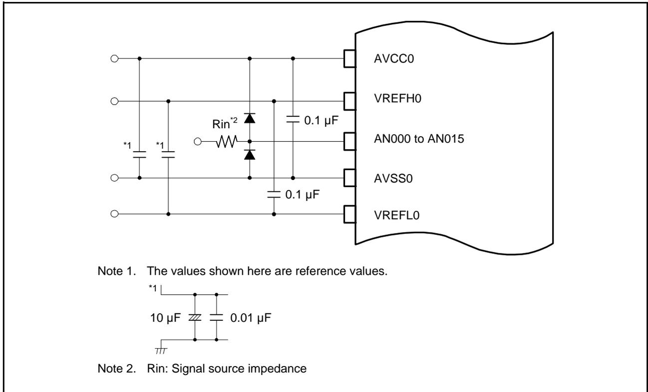
Figure 32.19 Sample Protection Circuit for Analog Inputs
