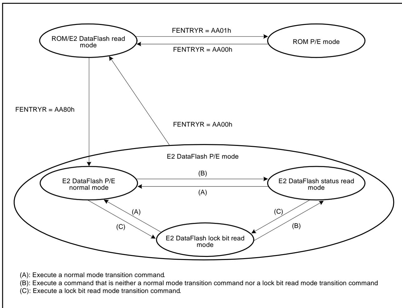
Figure 37.4 Mode Transitions of the FCU (Associated with the E2 DataFlash)
