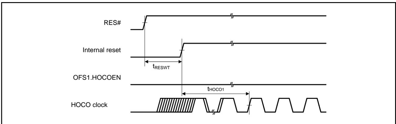
Figure 38.24 HOCO Clock Oscillation Start Timing (After Reset is Canceled by Setting the OFS1.HOCOEN Bit to 0)
