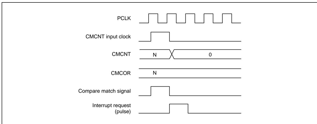
**Figure 24.4 Timing of a Compare Match Interrupt**
