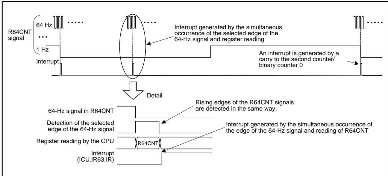
Figure 25.10 Carry Interrupt (CUP) Timing Chart
