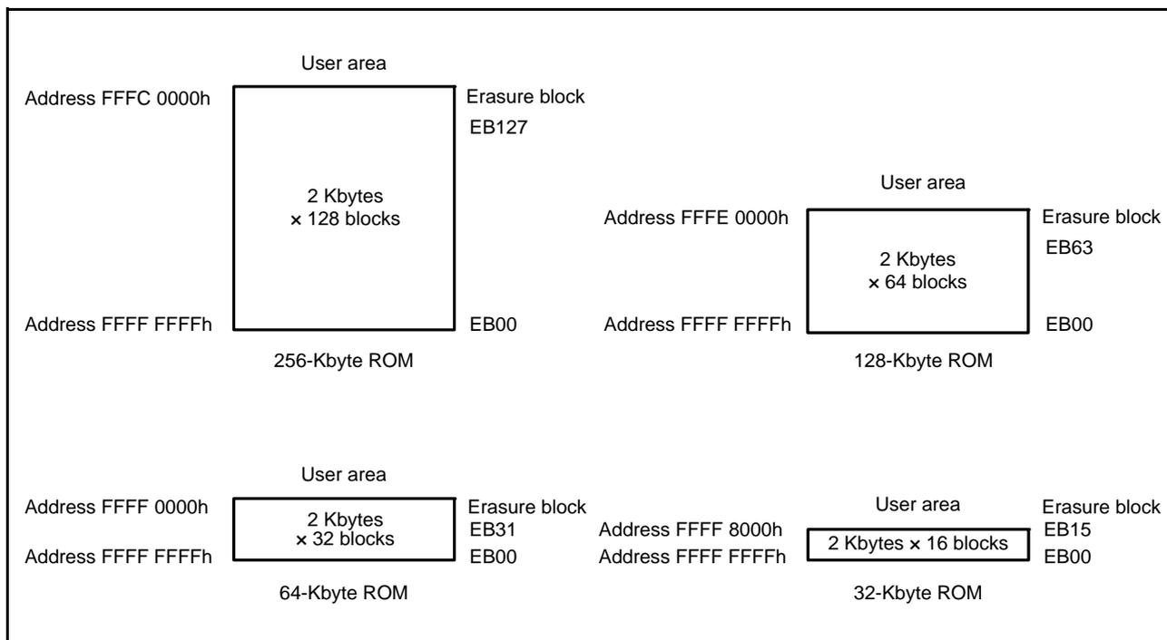
Figure 36.3 Configuration of Erasure Blocks for the User Area
