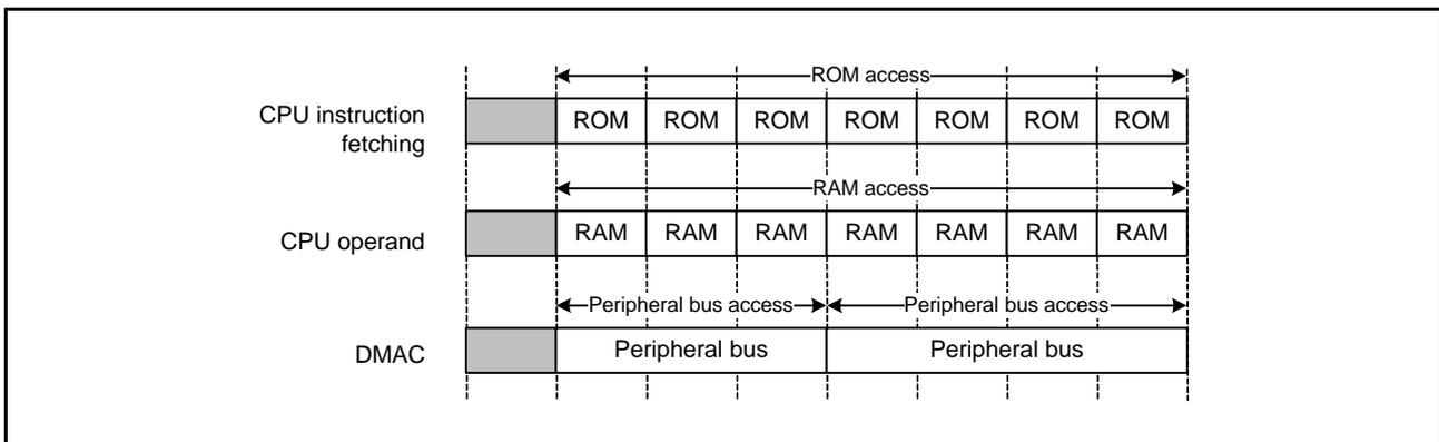
Figure 15.4 Example of Parallel Operations
