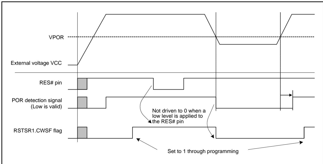
Figure 6.3 Example of Cold/Warm Start Determination Operation
