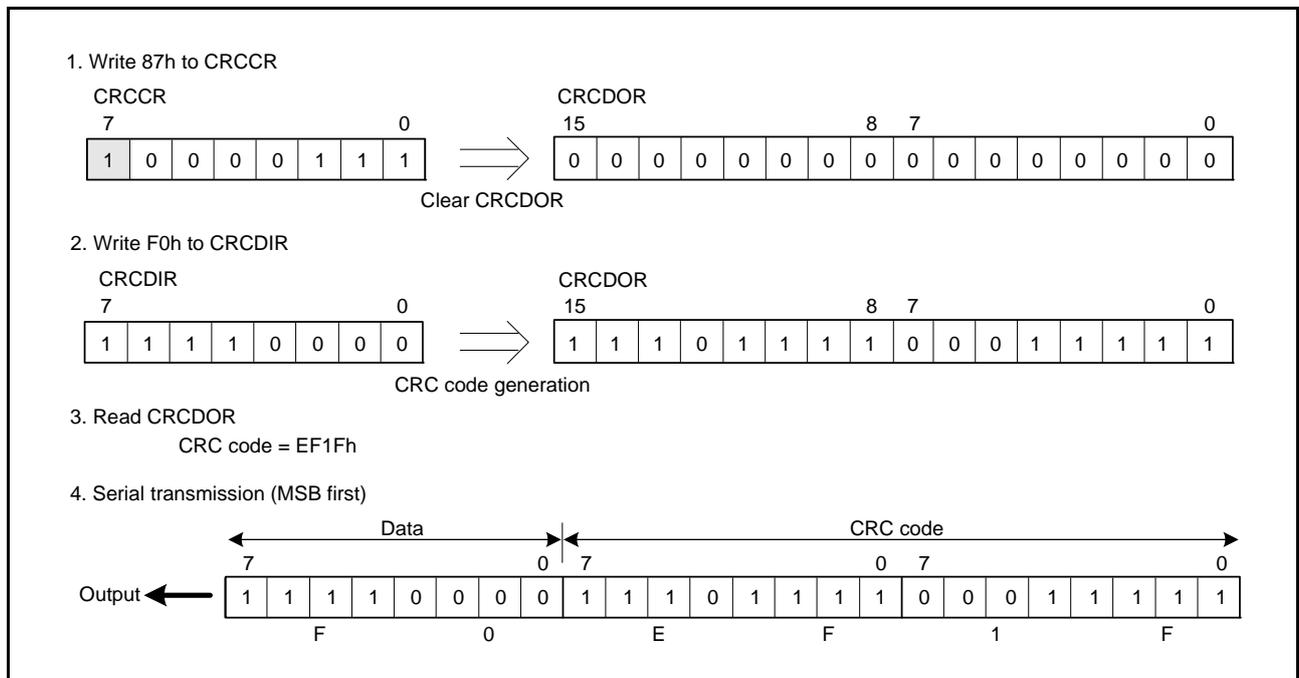
Figure 31.3 MSB-First Data Transmission
