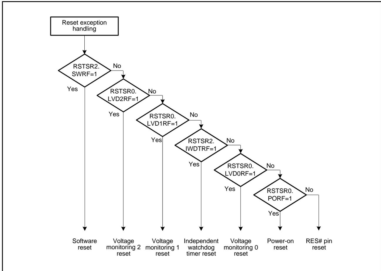
Figure 6.4 Example of Reset Generation Source Determination Flow
