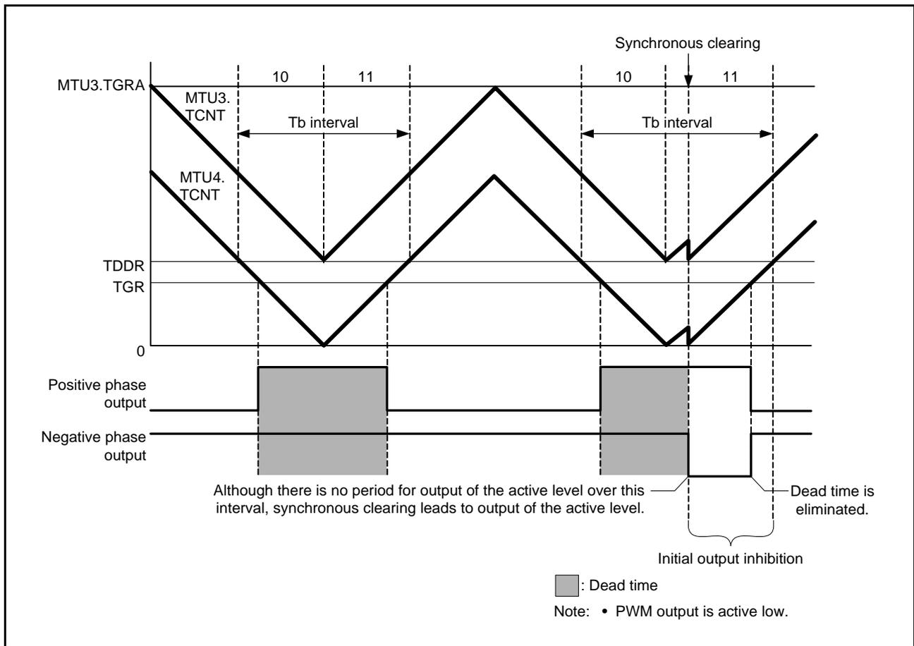
Figure 21.123 Example of Synchronous Clearing (when Condition 2 Applies)
