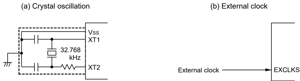
Figure 6-21. Example of External Circuit of XT1 Oscillator
