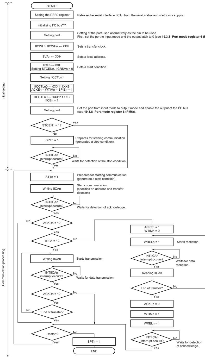
**Note** Release (SCLAn and SDAAn pins = high level) the I<sup>2</sup>C bus in conformance with the specifications of the product that is communicating. If EEPROM is outputting a low level to the SDAAn pin, for example, set the SCLAn pin in the output port mode, and output a clock pulse from the output port until the SDAAn pin is constantly at high level.
