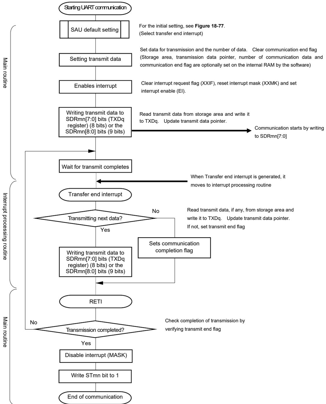
(4) Processing flow (in continuous transmission mode)
