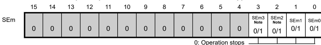
\* The SEm register is a read-only status register, whose operation is stopped by using the STm register. With a channel whose operation is stopped, the value of the CKOm bit of the SOm register can be set by software.
