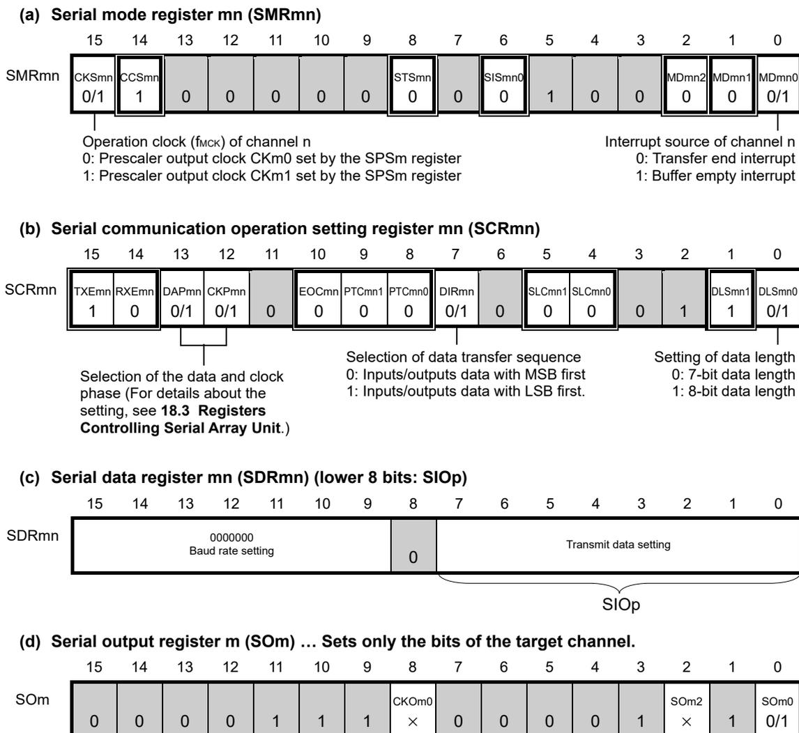
**Note** Only provided for the SCR00 register. This bit is fixed to 1 for the other registers.
