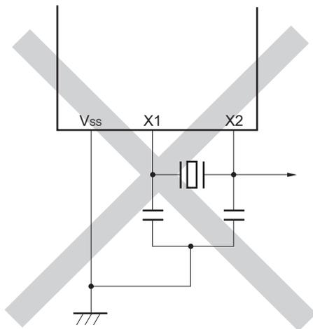
**Caution** When X2 and XT1 are wired in parallel, the crosstalk noise of X2 may increase with XT1, resulting in malfunctioning.
