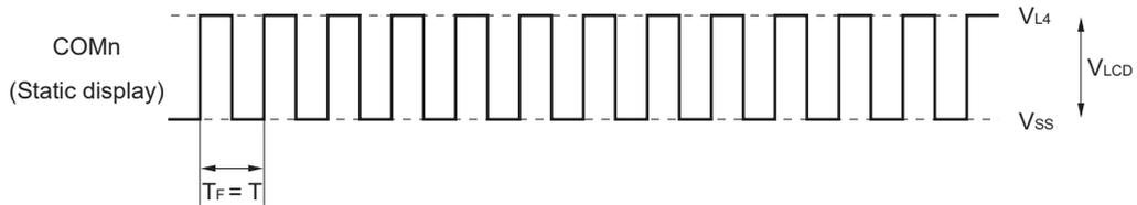
T: One LCD clock period       $T_F$ : Frame frequency
