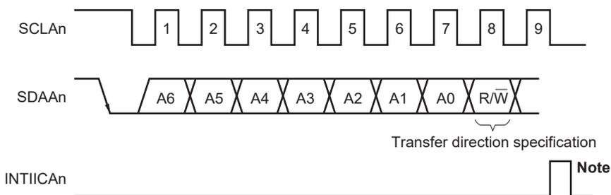
**Note** INTIICAn is not issued if data other than a local address or extension code is received during slave device operation.
