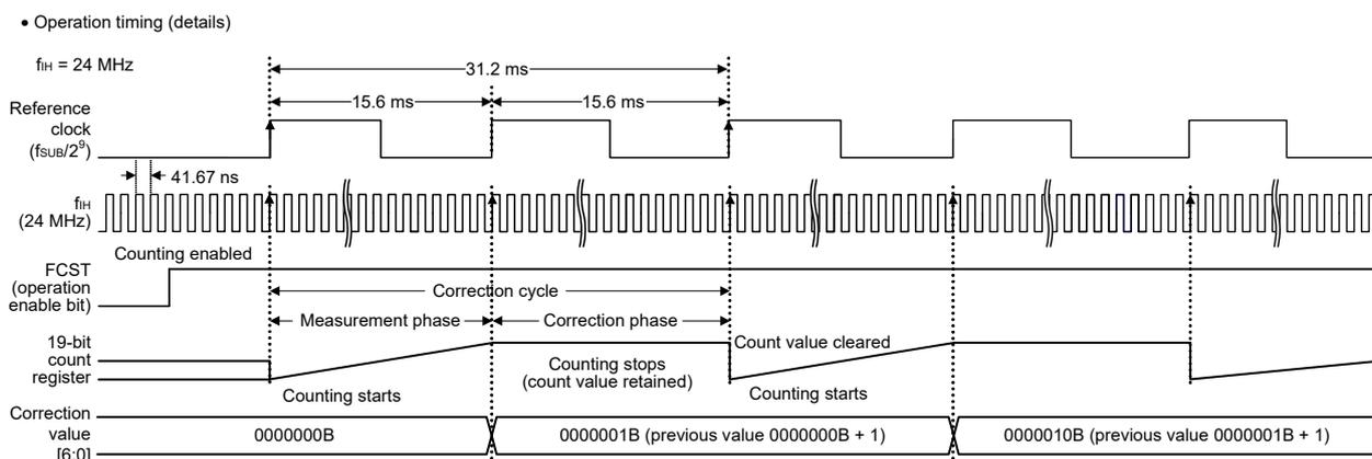
**Remark** Basic operation is the same in both continuous and intermittent operating modes. Only the difference between these modes is clearing the FCST bit is controlled by either software or hardware. In addition, the correction value is not cleared until a reset is applied to the system.
