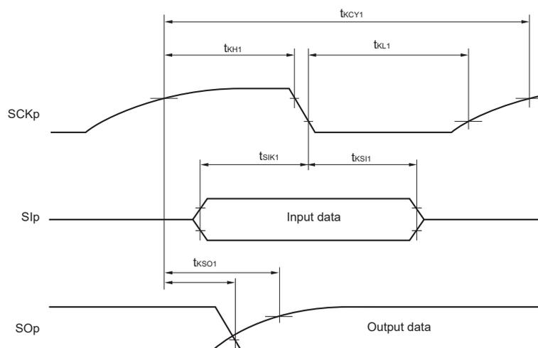
**Caution** Select the TTL input buffer for the Slp pin and the N-ch open drain output ( $V_{DD}$  tolerance) mode for the SOp pin and SCKp pin by using port input mode register g (PIMg) and port output mode register g (POMg). For  $V_{IH}$  and  $V_{IL}$ , see the DC characteristics with TTL input buffer selected.
