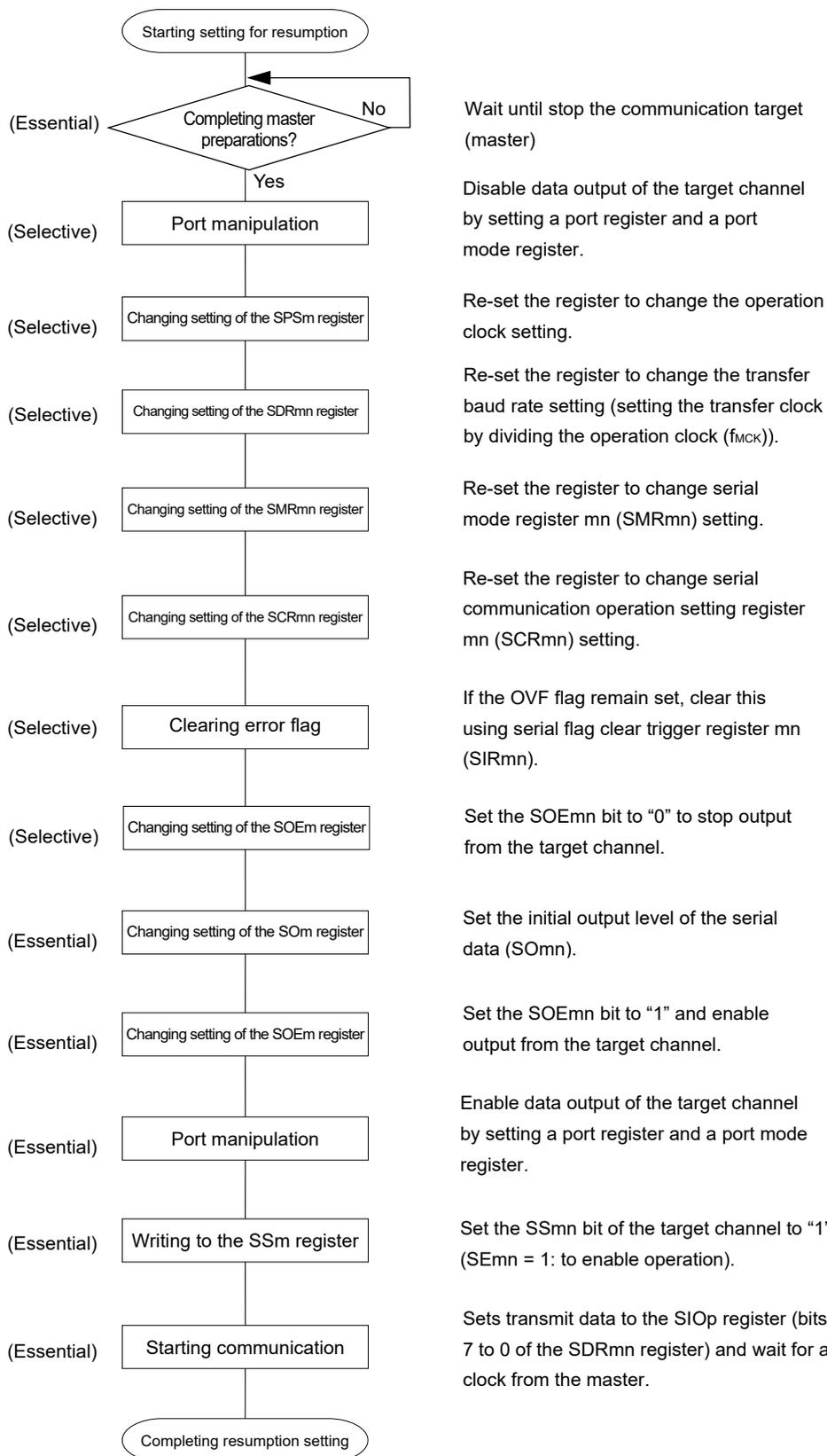
**Remark** If PER0 is rewritten while stopping the master transmission and the clock supply is stopped, wait until the transmission target (master) stops or transmission finishes, and then perform initialization instead of restarting the transmission.
