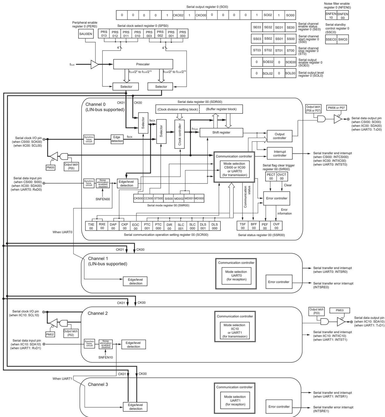
Figure 18-2 shows the block diagram of the serial array unit 1.
