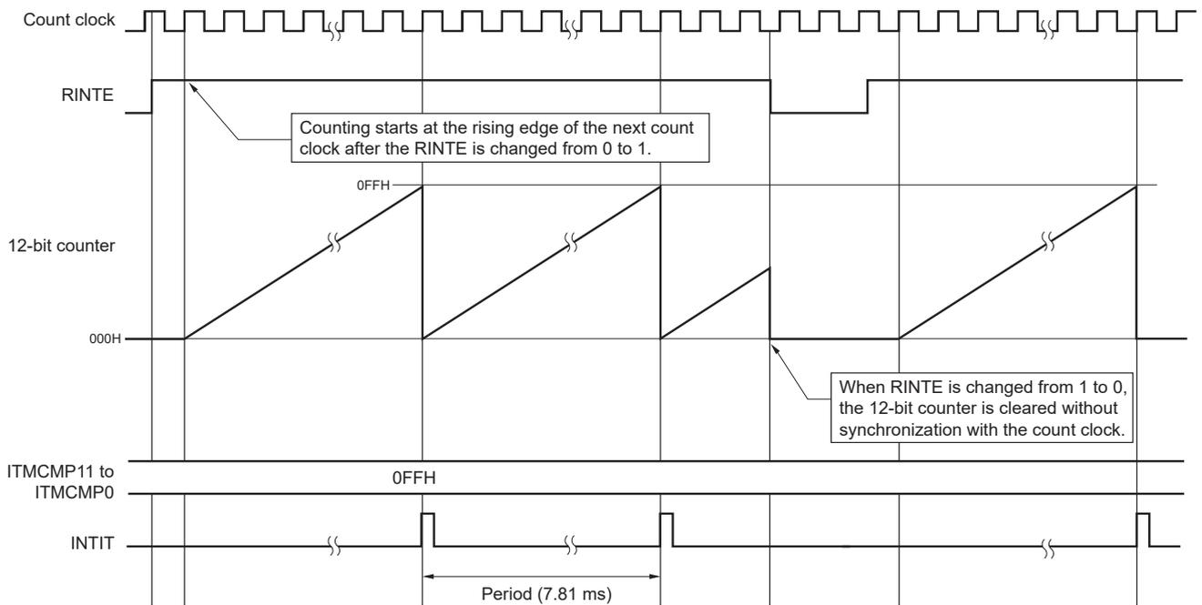
**10.4.2 Start of count operation and re-enter to HALT/STOP mode after returned from HALT/STOP mode**
