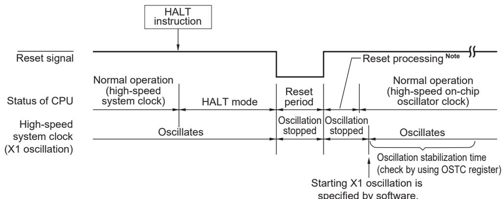
**(2) When high-speed on-chip oscillator clock is used as CPU clock**
