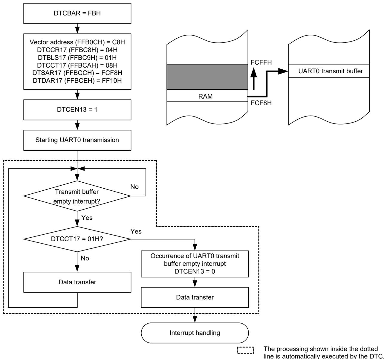
The value of the DTRLD17 register is not used because of normal mode, but initialize the register to 00H when parity error resets are enabled (RPERDIS = 0) using the RAM parity error detection function. Start the first UART0 transmission by software. The second and subsequent transmissions are automatically sent when the DTC is activated by a transmit buffer empty interrupt.
