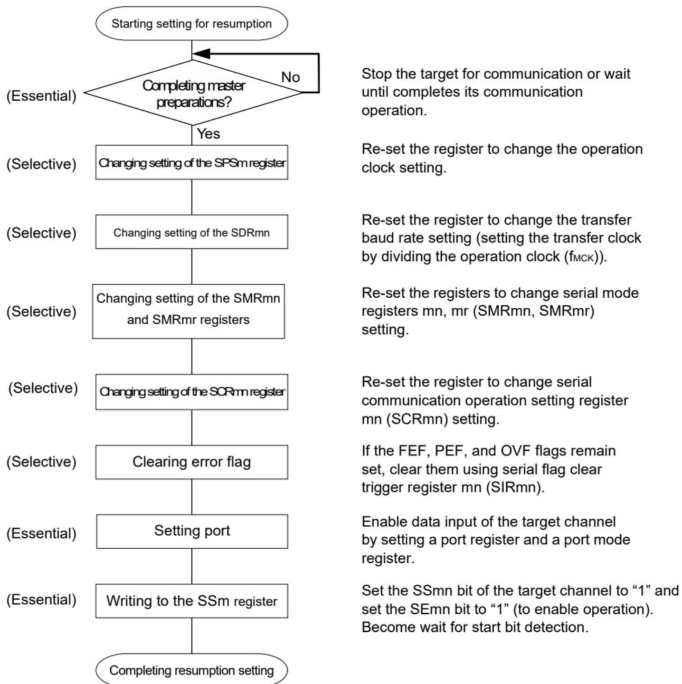
**Caution** After is set RXEmn bit to 1 of SCRmn register, set the SSmn = 1 from an interval of at least four clocks of fmck.
