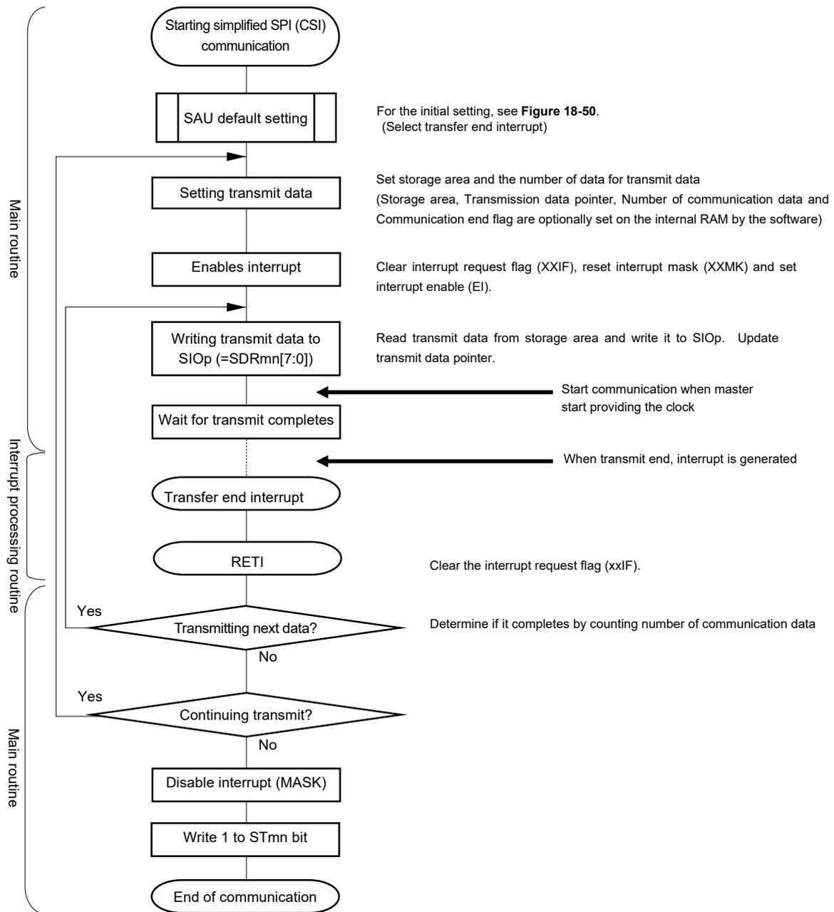
(4) Processing flow (in continuous transmission mode)
