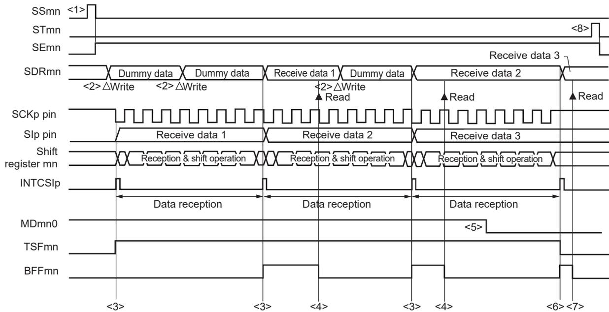
**Caution** The MDmn0 bit can be rewritten even during operation. However, rewrite it before receive of the last bit is started, so that it has been rewritten before the transfer end interrupt of the last receive data.
