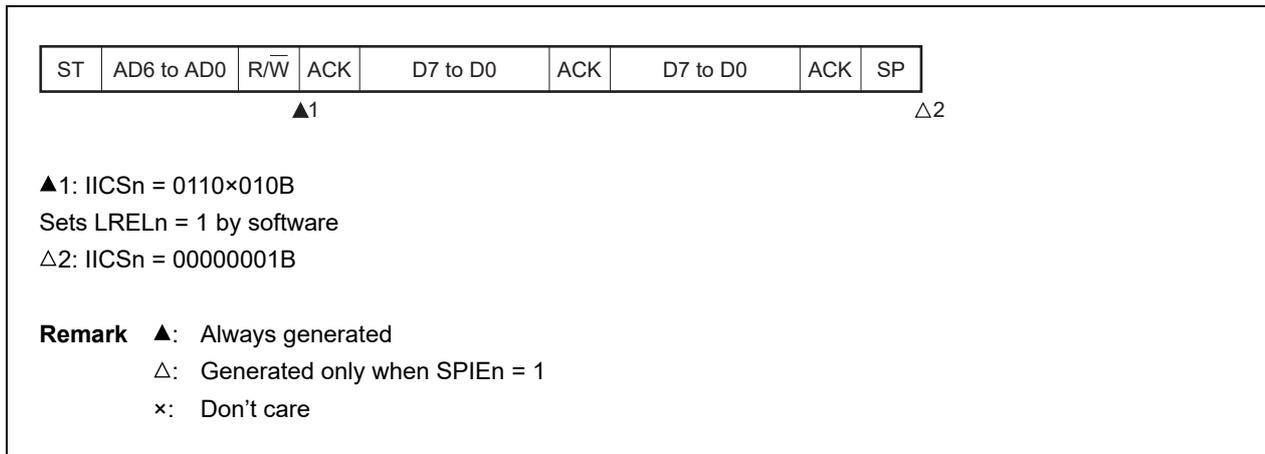
**(c) When arbitration loss occurs during transmission of data**
