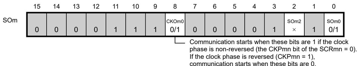
**Note** Only provided for the SCR00 register. This bit is fixed to 1 for the other registers.
