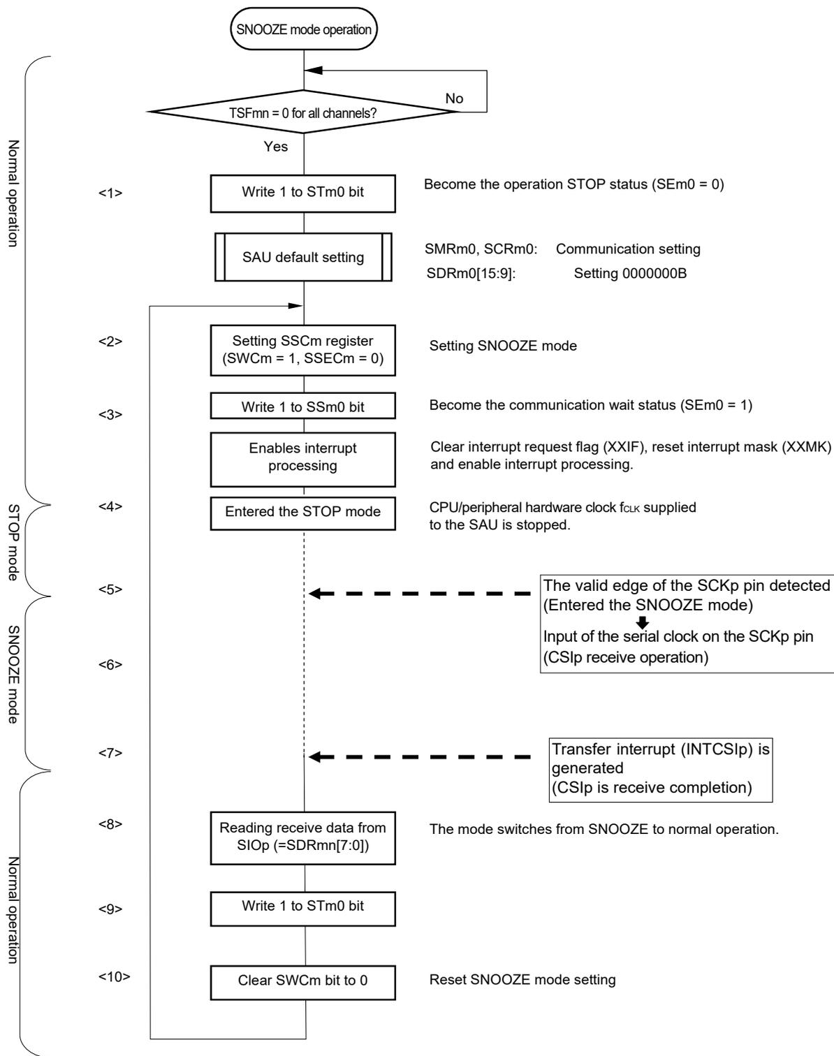
Remarks 1. <1> to <10> in the figure correspond to <1> to <10> in Figure 18-73 Timing Chart of SNOOZE Mode Operation (Continuous Startup).
