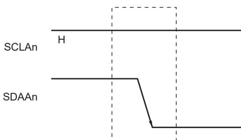
A start condition is output when bit 1 (STTn) of IICA control register n0 (IICCTLn0) is set (1) after a stop condition has been detected (SPDn: Bit 0 of the IICA status register n (IICSn) = 1). When a start condition is detected, bit 1 (STDn) of the IICSn register is set (1).
