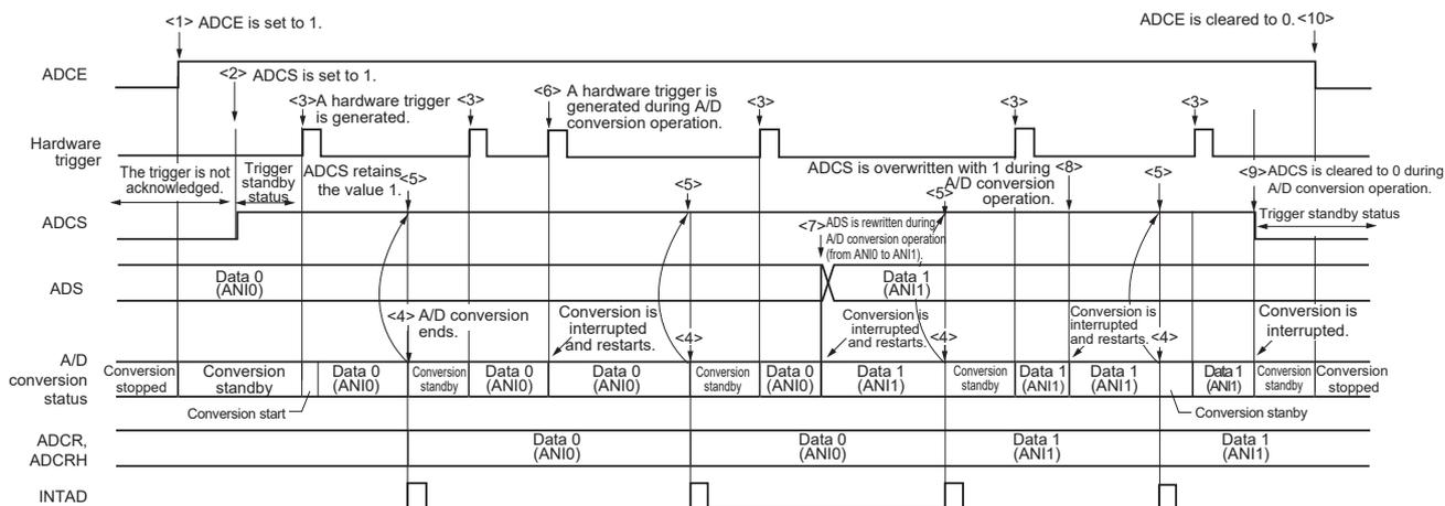
14.6.7 Hardware trigger no-wait mode (scan mode, sequential conversion mode)
