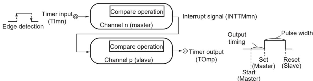
**(2) PWM (Pulse Width Modulation) output**
