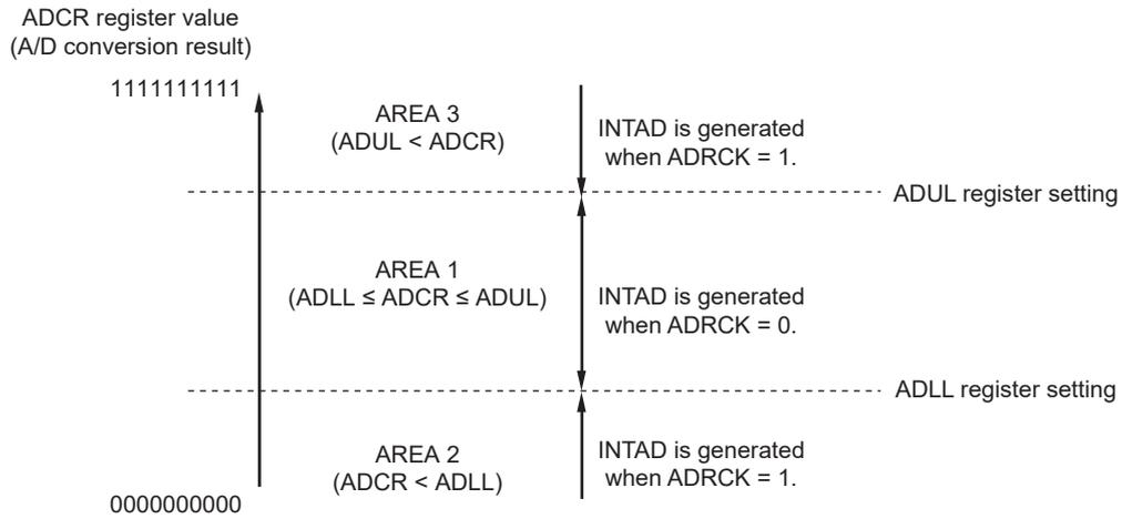
**Remark** If INTAD does not occur, the A/D conversion result is not stored in the ADCR or ADCRH register.
