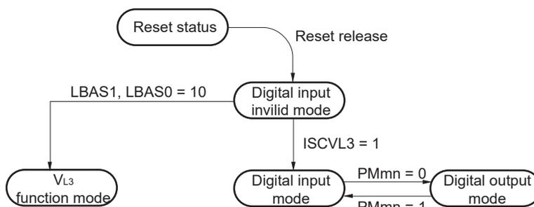
**Caution** Be sure to set the VL3 function mode before segment output starts (while SCOC bit of LCD mode register 1 (LCDM1) is 0).
