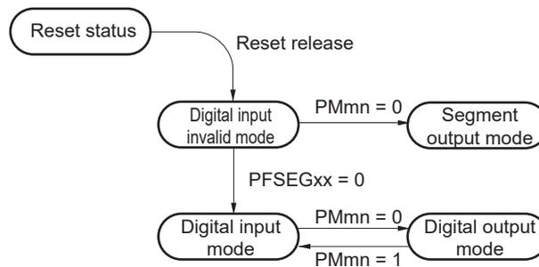
**Caution** Be sure to set the segment output mode before segment output starts (while SCOC of LCD mode register 1 (LCDM1) is 0).
