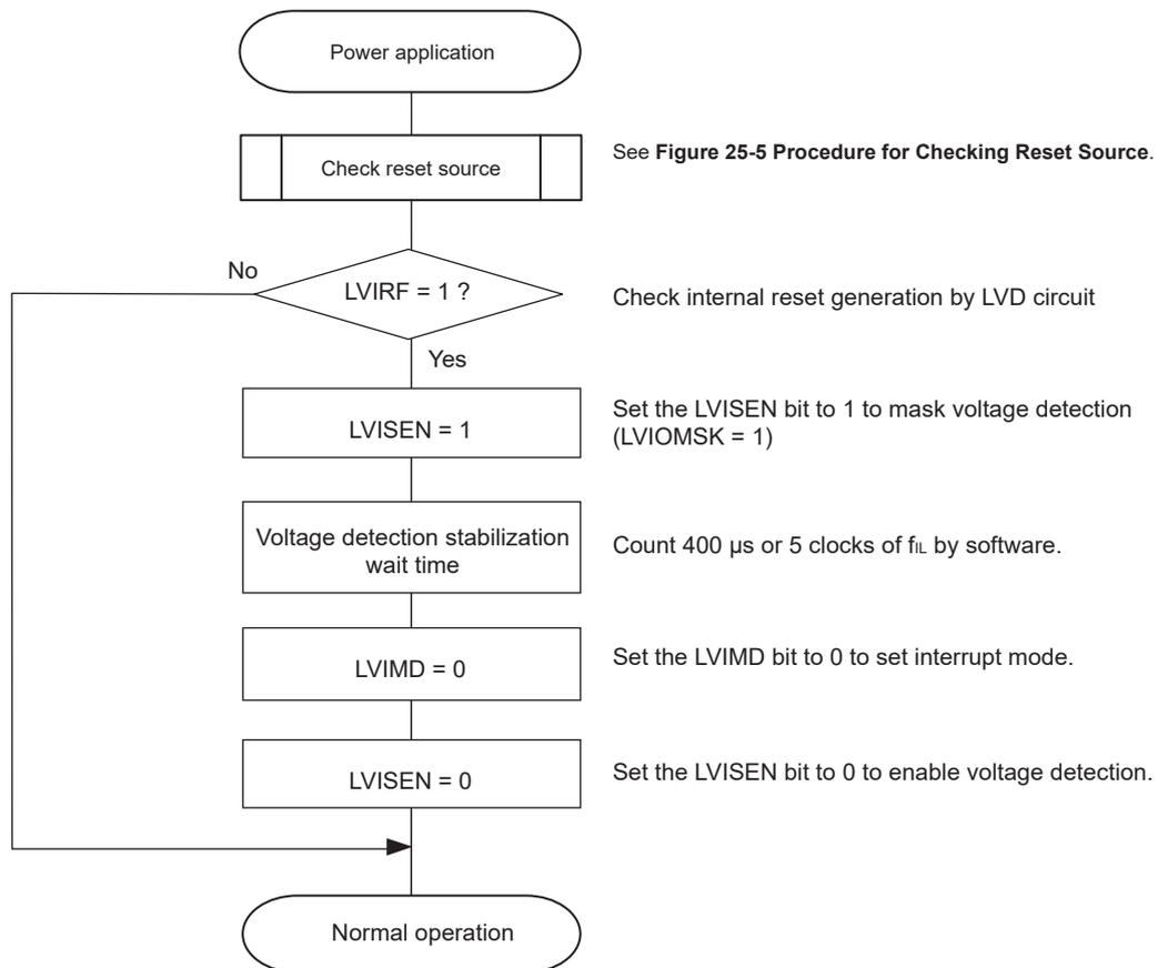
**Remark**  $f_{IL}$ : Low-speed on-chip oscillator clock frequency
