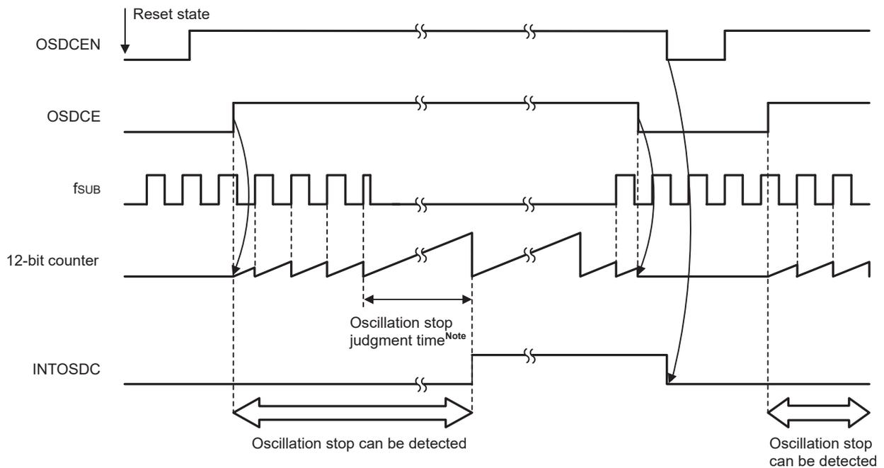
**Note** It is judged that oscillation has stopped when oscillation has been stopped for (A-2) to (A+1) clock cycles, where A refers to the time specified by these bits.
