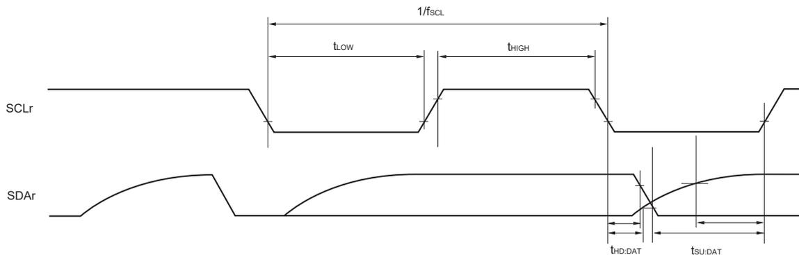
**Caution** Select the normal input buffer and the N-ch open drain output ( $V_{DD}$  tolerance) mode for the SDAr pin and the normal output mode for the SCLr pin by using port input mode register g (PIMg) and port output mode register g (POMg).
