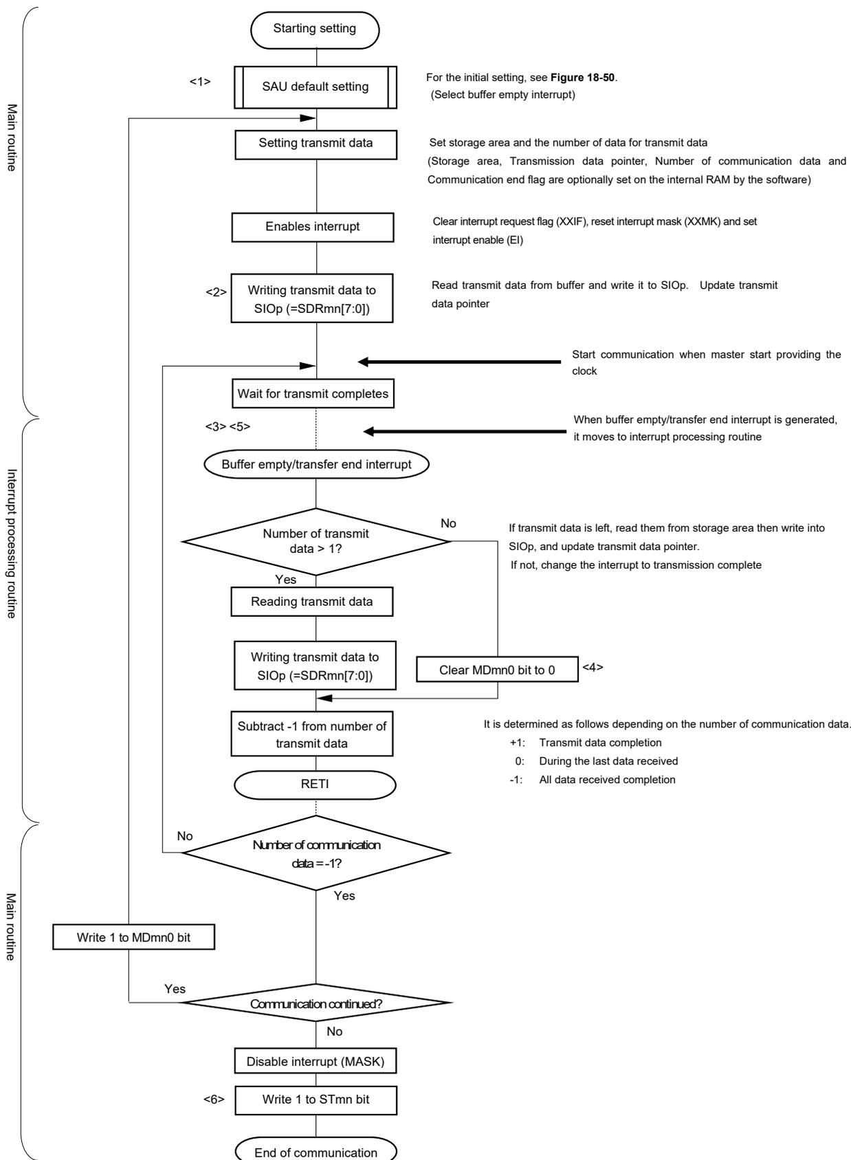
Remark <1> to <6> in the figure correspond to <1> to <6> in Figure 18-55 Timing Chart of Slave Transmission (in Continuous Transmission Mode).
