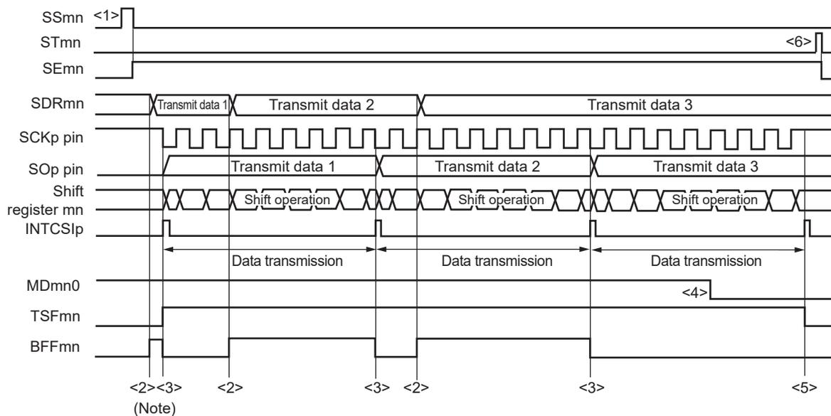
**Note** If transmit data is written to the SDRmn register while the BFFmn bit of serial status register mn (SSRmn) is 1 (valid data is stored in serial data register mn (SDRmn)), the transmit data is overwritten.
