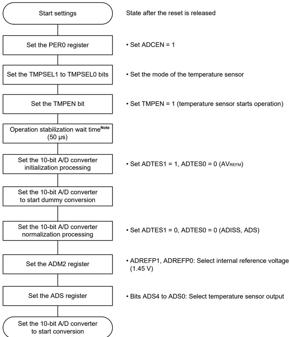
**Note** Operation stabilization wait time is required until the A/D converter starts conversion.
