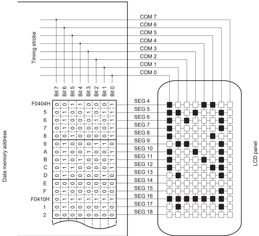
**Figure 21-43. Eight-Time-Slice LCD Drive Waveform Examples Between SEG4 and Each Common Signals (1/4 Bias Method) (1/2)**
