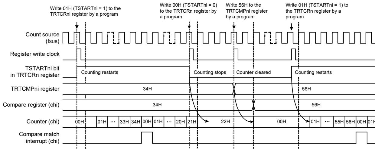
The TCSMDn bit in the TRTCRn register is set to 0 (8-bit counter operation).
