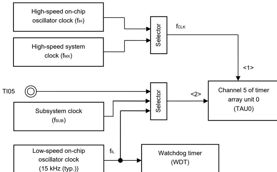
If input pulse interval measurement results in an abnormal value, it can be concluded that the clock frequency is abnormal.
