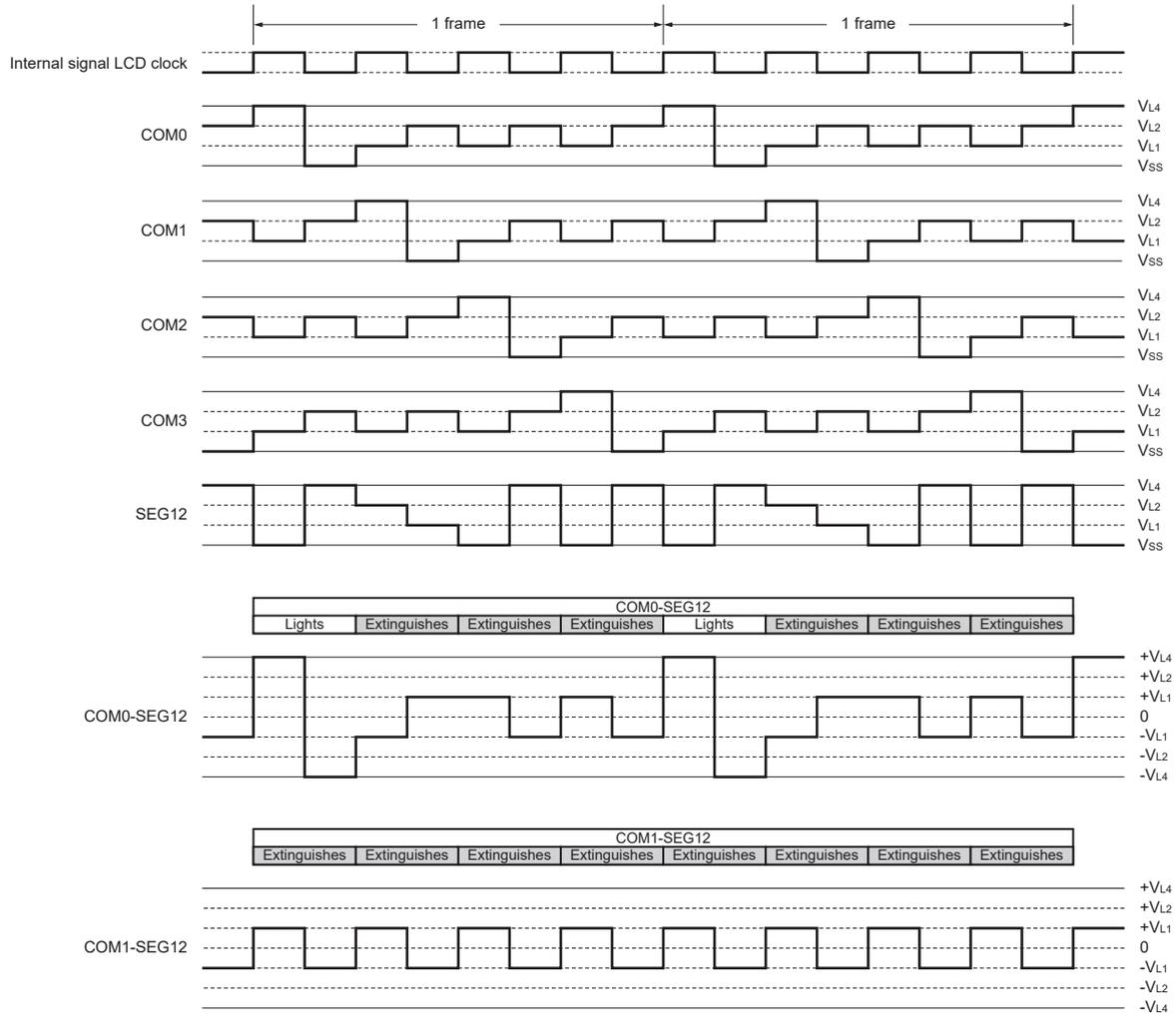
**Figure 21-37. Four-Time-Slice LCD Drive Waveform Examples Between SEG12 and Each Common Signals (1/3 Bias Method) (2/2)**
