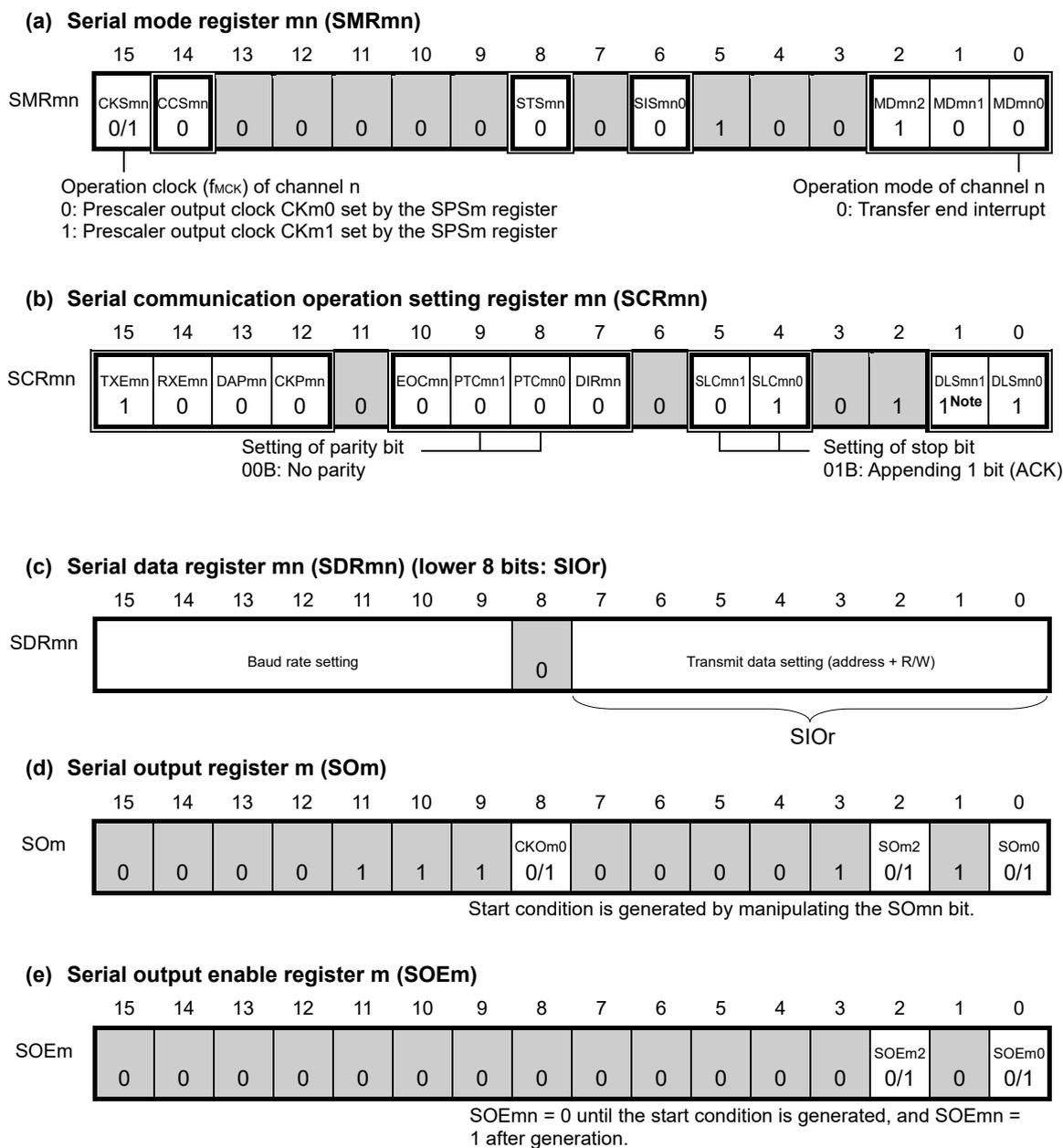
**Note** Only provided for the SCR00 register. This bit is fixed to 1 for the other registers.
