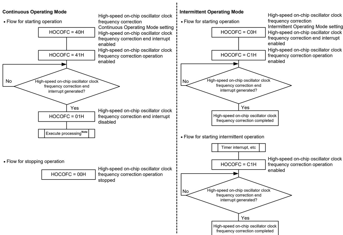
**Note** The high speed on-chip oscillator clock frequency correction is repeated until the high speed on-chip oscillator clock frequency correction function is stopped.
