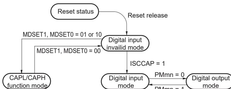
**Caution** Be sure to set the CAPL/CAPH function mode before segment output starts (while SCOC bit of LCD mode register 1 (LCDM1) is 0).
