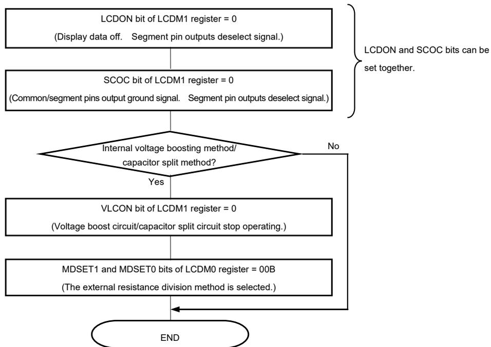
**Caution** Stopping the voltage boost/capacitor split circuits is prohibited while the display is on (SCOC and LCDON bits of LCDM1 register = 11B). Otherwise, the operation will not be guaranteed. Be sure to turn off display (SCOC and LCDON bits of LCDM1 register = 00B) before stopping the voltage boost/capacitor split circuits (VLCON bit of LCDM1 register = 0).
