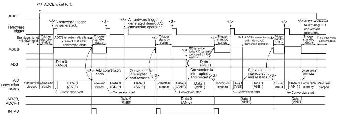
14.6.11 Hardware trigger wait mode (scan mode, sequential conversion mode)
