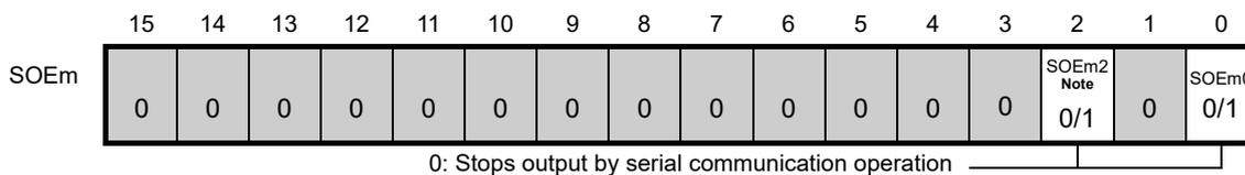
\* For channel n, whose serial output is stopped, the SOmn bit value of the SOm register can be set by software.
