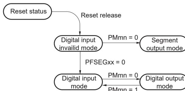
**Caution** Be sure to set the segment output mode before segment output starts (while SCOC bit of LCD mode register 1 (LCDM1) is 0).
