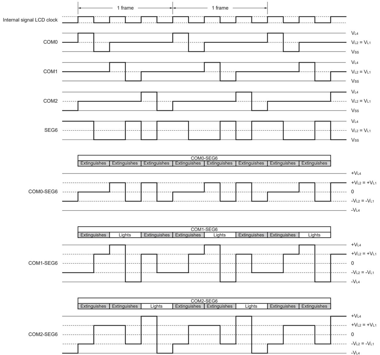
**Figure 21-34. Three-Time-Slice LCD Drive Waveform Examples Between SEG6 and Each Common Signals (1/3 Bias Method)**
