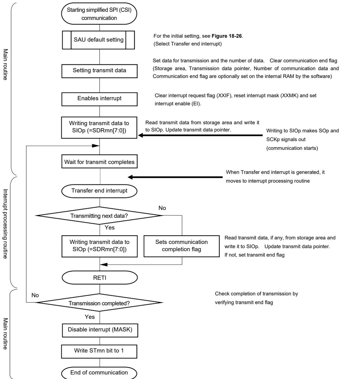
(4) Processing flow (in continuous transmission mode)
