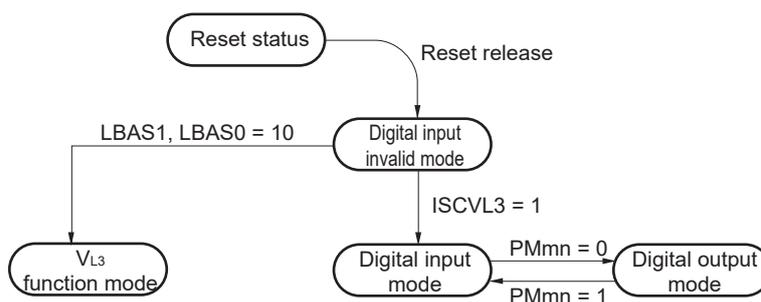
**Caution** Be sure to set the VL3 function mode before segment output starts (while SCOC of LCD mode register 1 (LCDM1) is 0).
