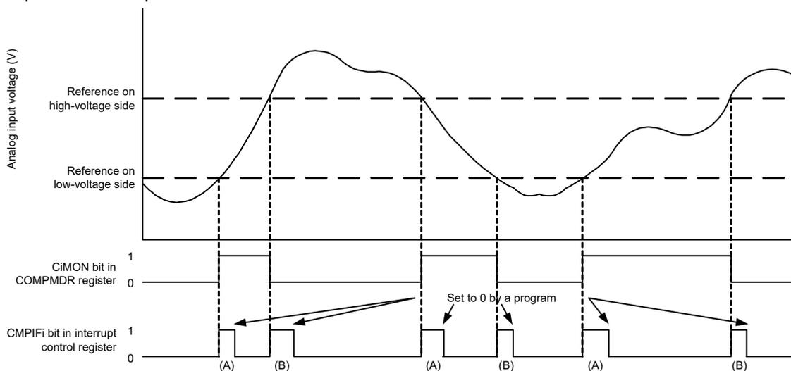
**Caution** The above diagram applies when CiFCK1 to CiFCK0 in the COMPFIR register = 00B (no filter) and CiEDG = 1 (both edges). When CiEDG = 0 and CiEPO = 0 (rising edge), CMPiFi changes as shown by (A) only. When CiEDG = 0 and CiEPO = 1 (falling edge), CMPiFi changes as shown by (B) only.
