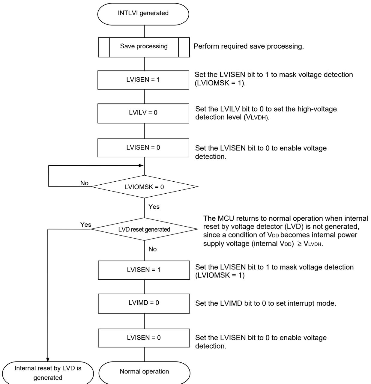
When setting an interrupt and reset mode (LVIMDS1, LVIMDS0 = 1, 0), voltage detection stabilization wait time for 400  $\mu$ s or 5 clocks of  $f_{IL}$  is necessary after LVD reset is released (LVIRF = 1). After waiting until voltage detection stabilizes, (0) clear the LVIMD bit for initialization. While voltage detection stabilization wait time is being counted and when the LVIMD bit is rewritten, set LVISEN to 1 to mask a reset or interrupt generation by LVD.
