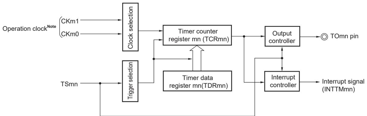
**Note** When channels 1 and 3, the clock can be selected from CKm0, CKm1, CKm2 and CKm3.
