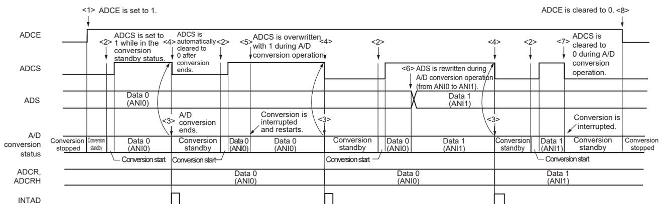
14.6.3 Software trigger mode (scan mode, sequential conversion mode)
