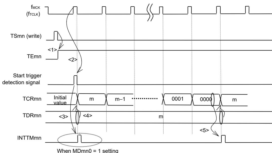
**Caution** In the first cycle operation of count clock after writing the  $TS_{mn}$  bit, an error at a maximum of one clock is generated since count start delays until count clock has been generated. When the information on count start timing is necessary, an interrupt can be generated at count start by setting  $MD_{mn0} = 1$ .
