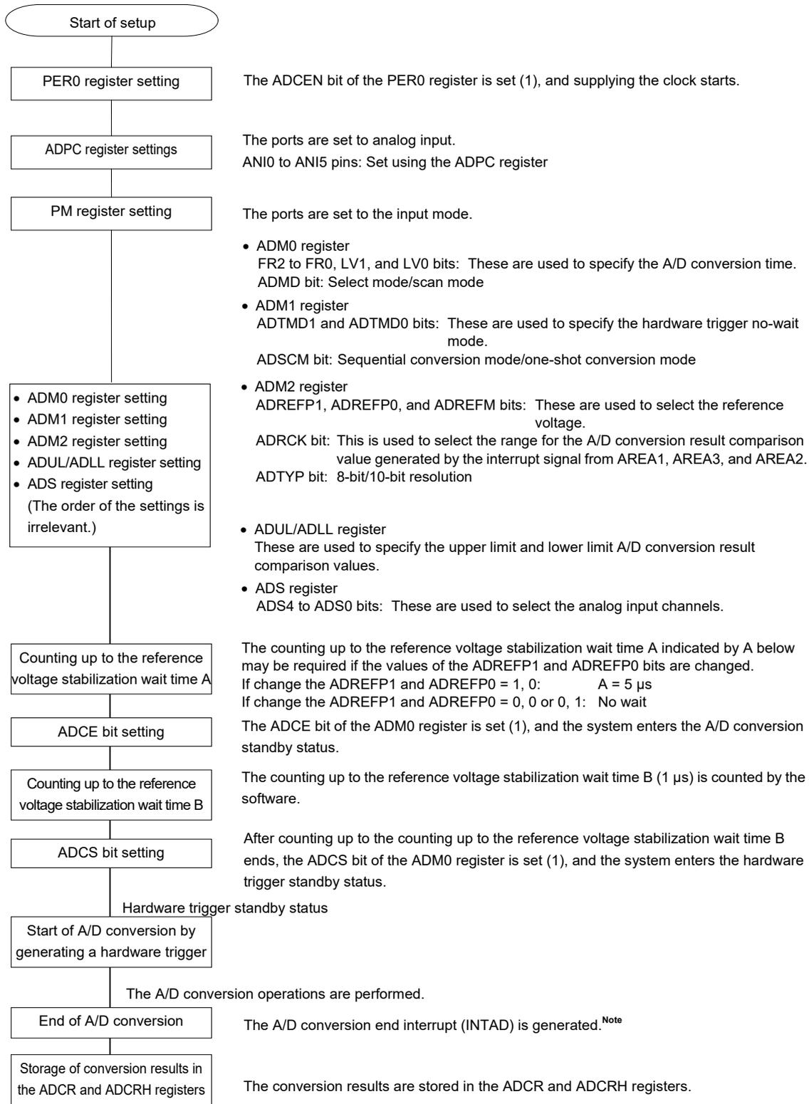
**Note** Depending on the settings of the ADRCK bit and ADUL/ADLL register, there is a possibility of no interrupt signal being generated. In this case, the results are not stored in the ADCR, ADCRH registers.
