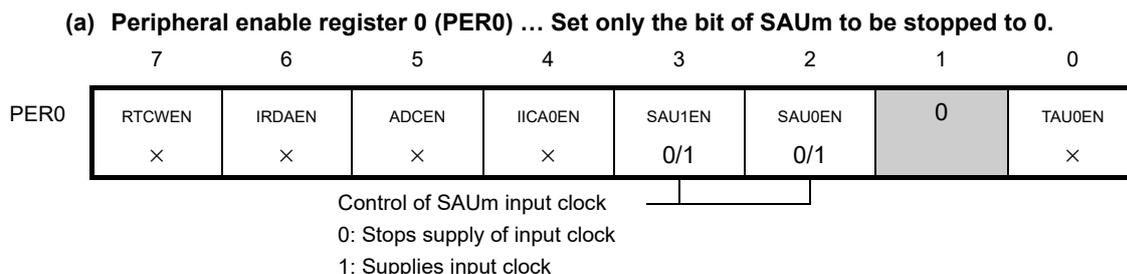
**Cautions 1.** If SAUmEN = 0, writing to a control register of serial array unit m is ignored, and, even if the register is read, only the default value is read
