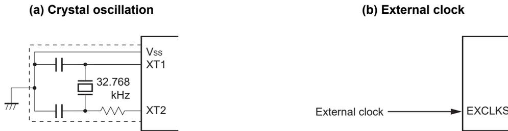
**Caution** When using the X1 oscillator and XT1 oscillator, wire as follows in the area enclosed by the broken lines in the Figures 5-12 and 5-13 to avoid an adverse effect from wiring capacitance.
