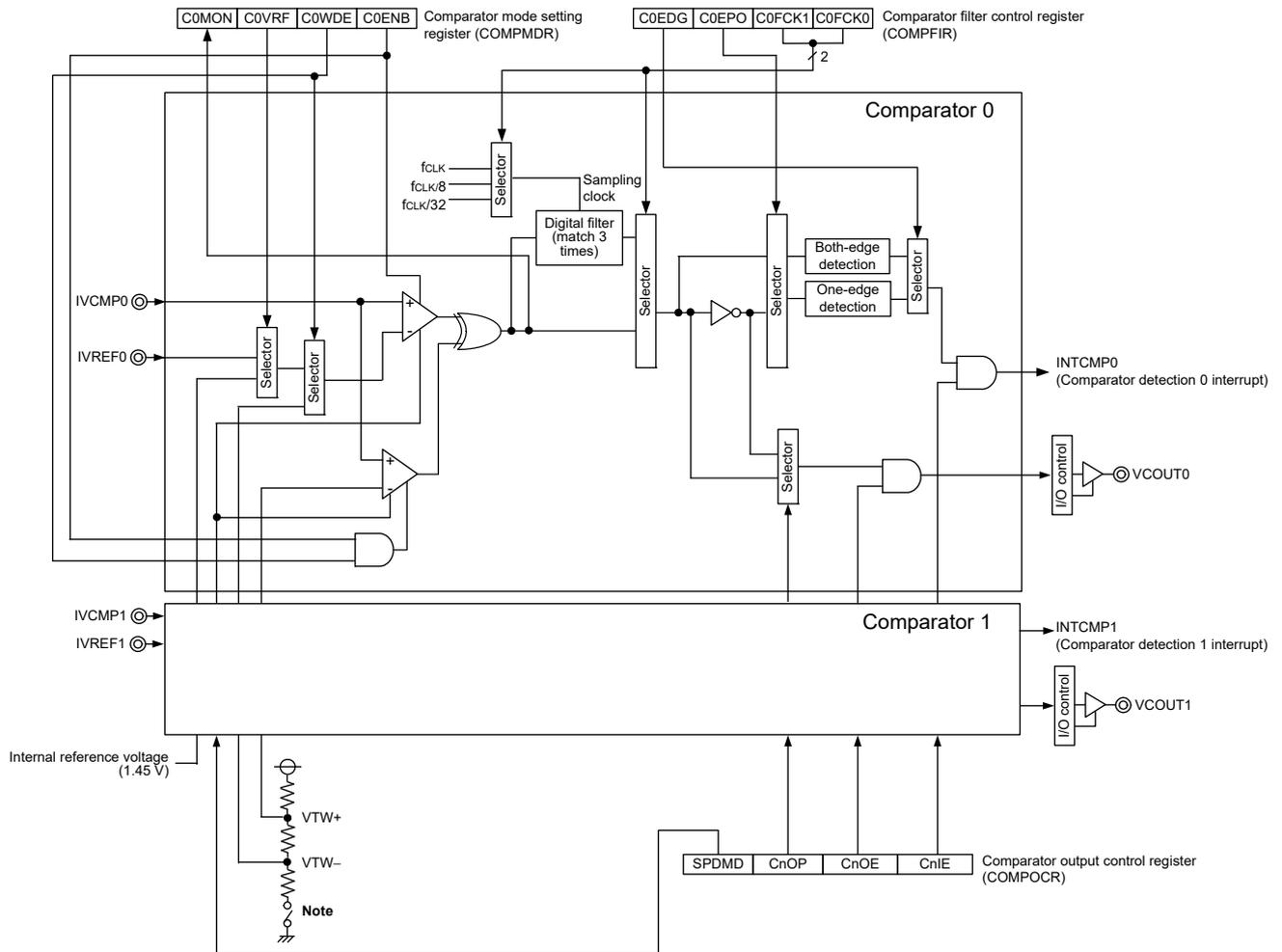
**Note** When either or both of the C0WDE and C1WDE bits are set to 1, this switch is turned on and the divider resistors for generating the comparison voltage are enabled.
