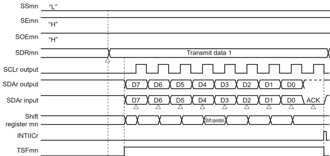
Figure 18-109. Flowchart of Simplified I<sup>2</sup>C Data Transmission
