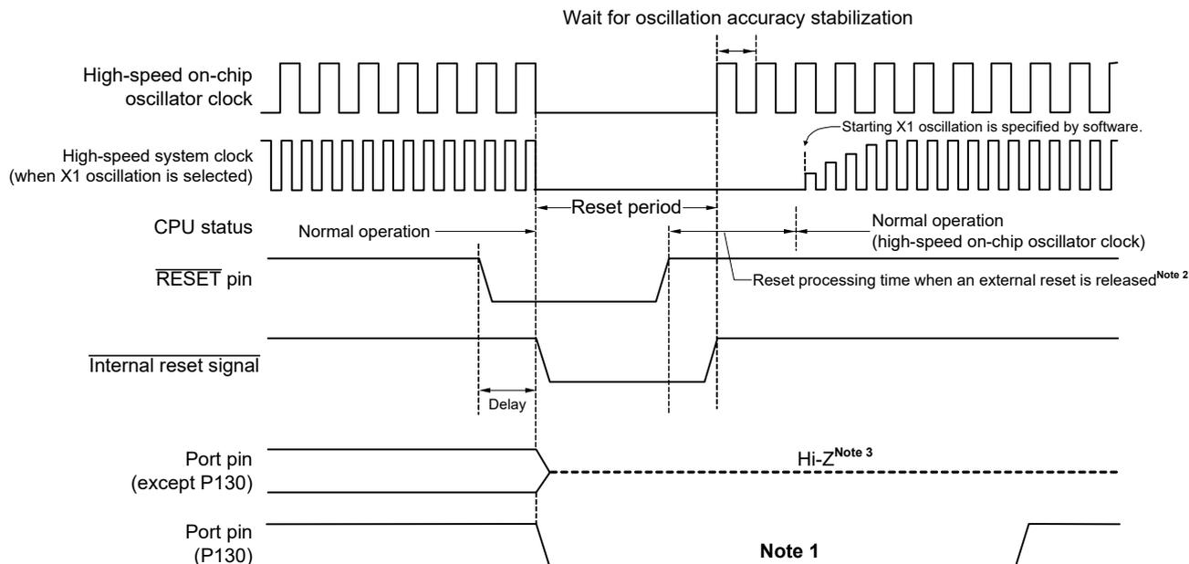
The input buffer of the  $\overline{\text{RESET}}$  pin is connected to internal  $V_{DD}$ . When using the battery backup function, input signal based on the voltage of the selected power supply source ( $V_{DD}$  pin or  $V_{BAT}$  pin).
