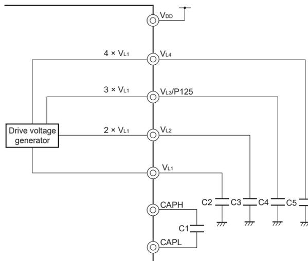
**Note**  $V_{L3}$  can be used as port (P125).
