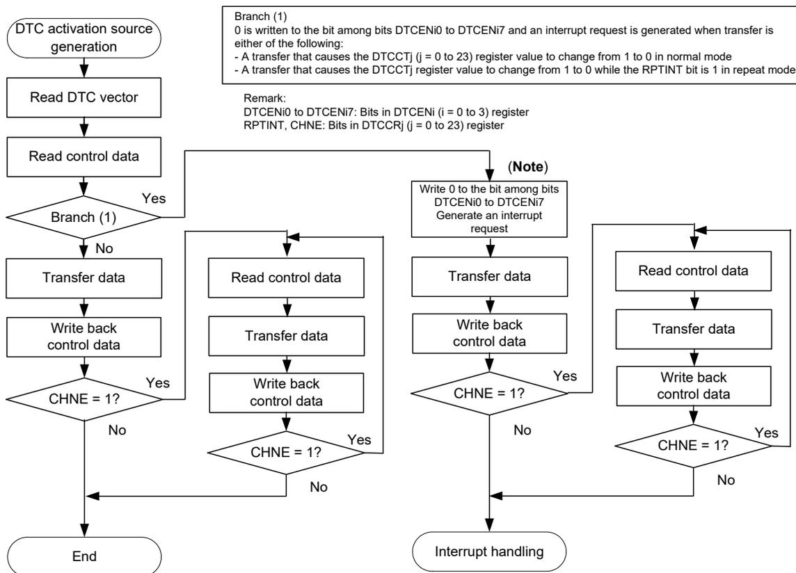
**Note** 0 is not written to the bit among bits DTCENi0 to DTCENi7 for data transfers activated by the setting to enable chain transfers (the CHNE bit is 1). Also, no interrupt request is generated.
