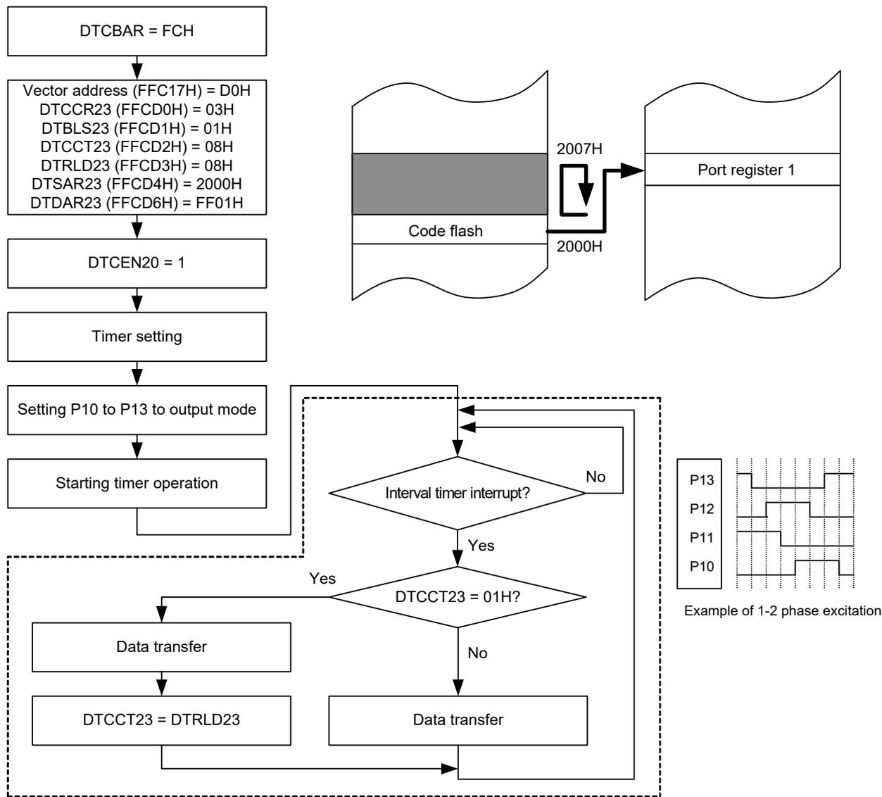
The processing shown inside the dotted line is automatically executed by the DTC.
