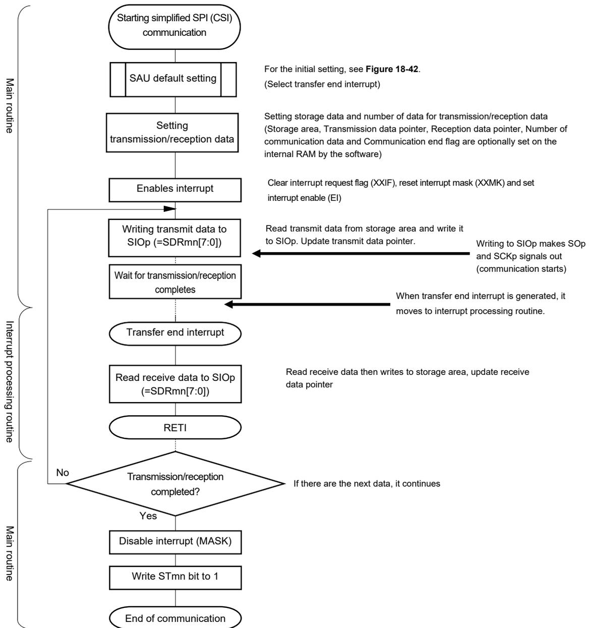
(4) Processing flow (in continuous transmission/reception mode)
