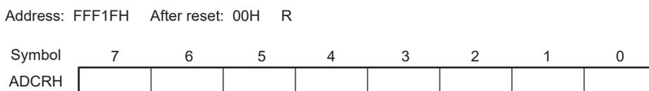
**Caution** When writing to the A/D converter mode register 0 (ADM0), analog input channel specification register (ADS), and A/D port configuration register (ADPC), the contents of the ADCRH register may become undefined. Read the conversion result following conversion completion before writing to the ADM0, ADS, and ADPC registers. Using timing other than the above may cause an incorrect conversion result to be read.
