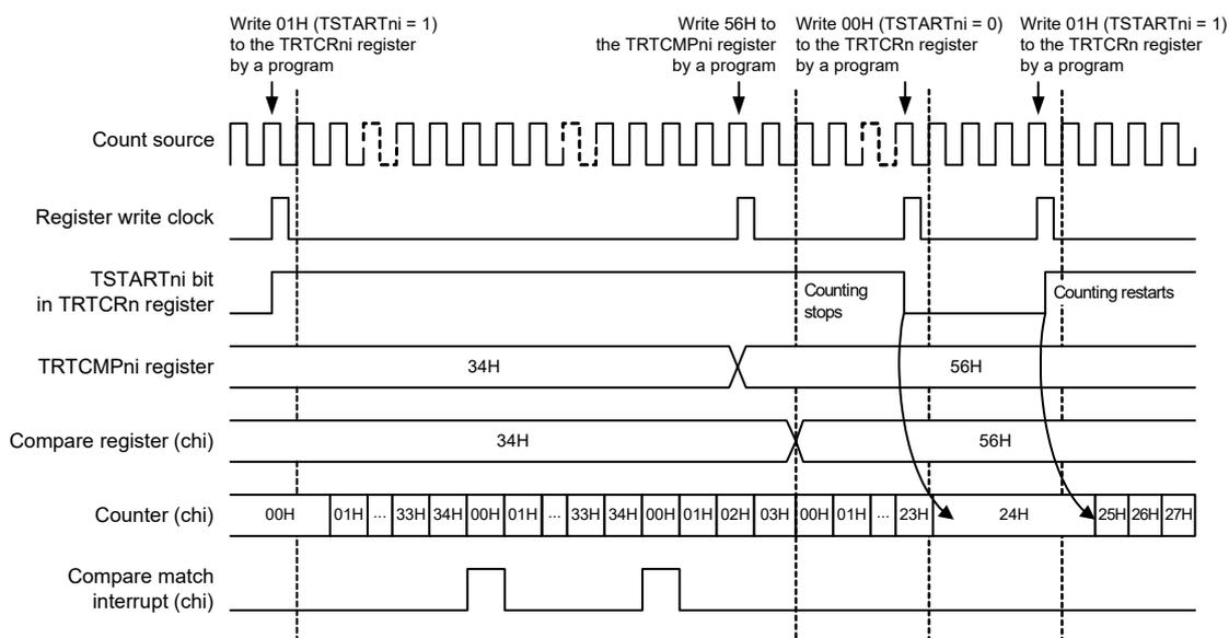
The TCSMD $_n$  bit in the TRTCR $_n$  register is set to 0 (8-bit counter operation).
