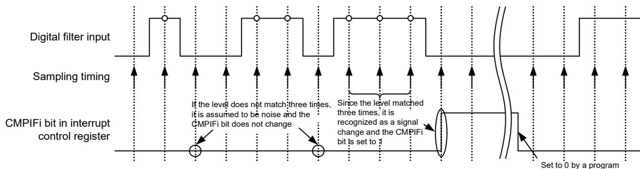
**Caution** The above operation example applies when bits CiFCK1 and CiFCK0 in the COMPFIR register is 01B, 10B, or 11B (digital filter enabled).
