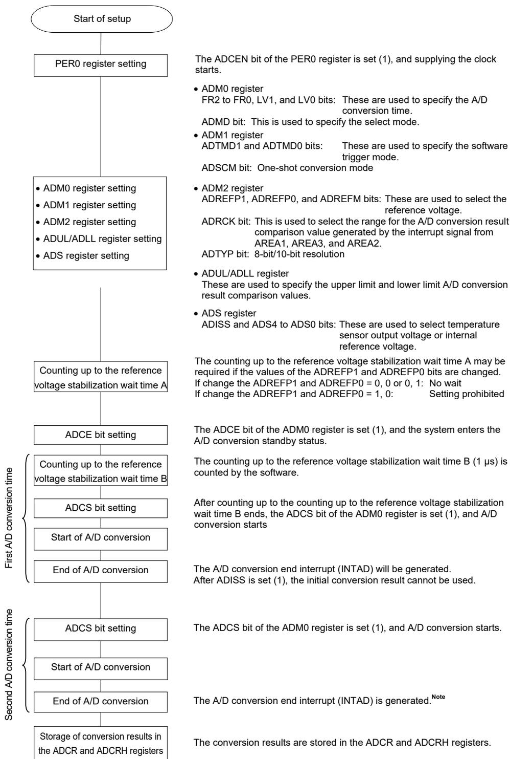
**Note** Depending on the settings of the ADRCK bit and ADUL/ADLL register, there is a possibility of no interrupt signal being generated. In this case, the results are not stored in the ADCR and ADCRH registers.
