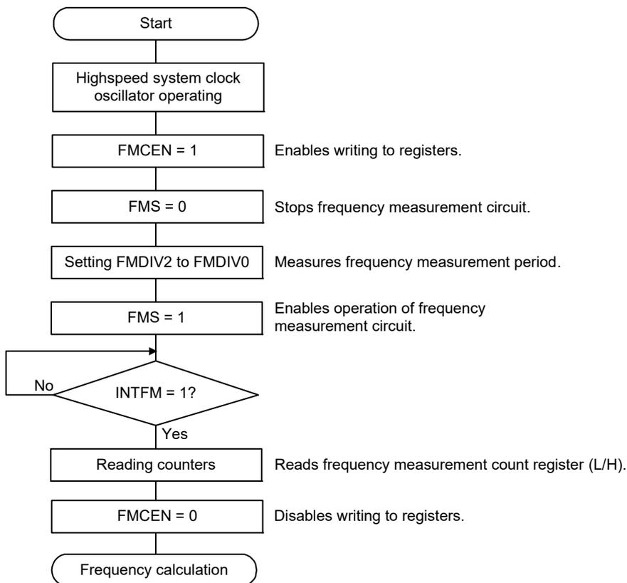
**Caution** After the frequency measurement count register (L/H) is read, be sure to set FMCEN to 0.
