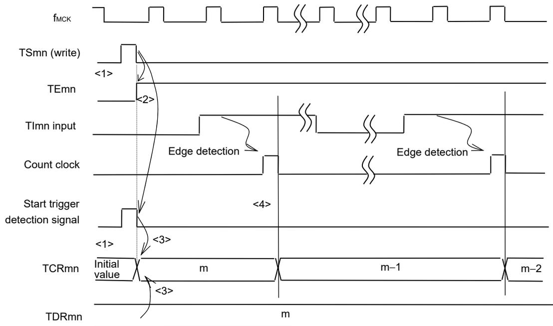
**Remark** The timing is shown in above figure indicates while the noise filter is not used. By making the noise filter on-state, the edge detection becomes 2 f<sub>MCK</sub> cycles (it sums up to 3 to 4 cycles) later than the normal cycle of TImn input. The error per one period occurs be the asynchronous between the period of the TImn input and that of the count clock (f<sub>MCK</sub>).
