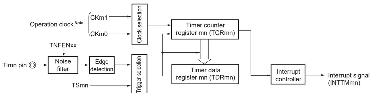
**Note** When channels 1 and 3, the clock can be selected from CK<sub>m0</sub>, CK<sub>m1</sub>, CK<sub>m2</sub> and CK<sub>m3</sub>.
