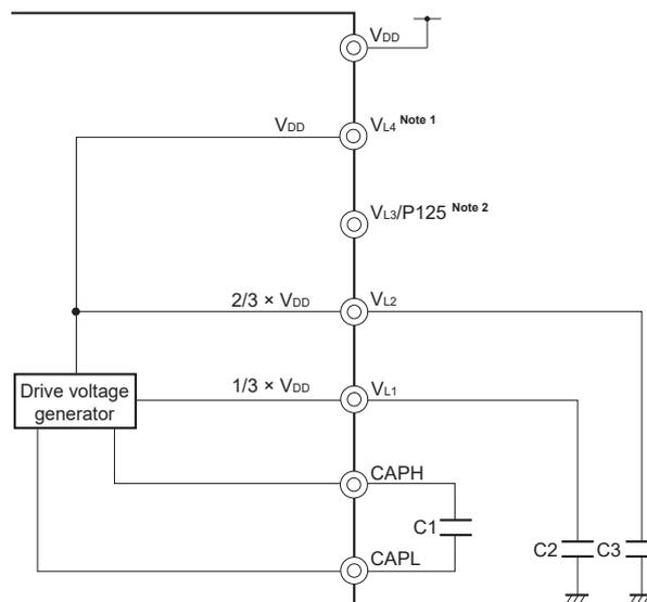
**Notes 1.** When switching to internal voltage boosting method, connect capacitor C4 as shown in Figure 21-21. Examples of LCD Drive Power Connections (Internal Voltage Boosting Method)
