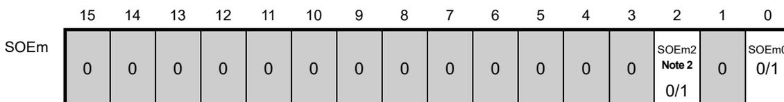
**(g) Serial channel start register m (SSm) ... Sets only the bits of the target channel to 1.**
