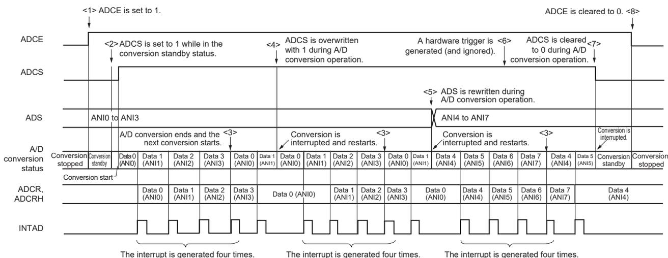
14.6.4 Software trigger mode (scan mode, one-shot conversion mode)
