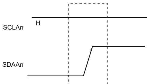
A stop condition is generated when bit 0 (SPTn) of IICA control register n0 (IICCTLn0) is set to 1. When the stop condition is detected, bit 0 (SPDn) of the IICA status register n (IICSn) is set to 1 and INTIICAn is generated when bit 4 (SPIEn) of the IICCTLn0 register is set to 1.
