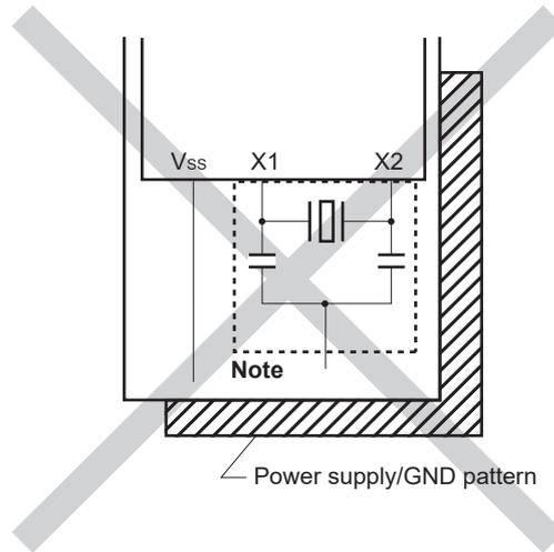
**Note** Do not place a power supply/GND pattern under the wiring section (section indicated by a broken line in the figure) of the X1 and X2 pins and the resonators in a multi-layer board or double-sided board.
