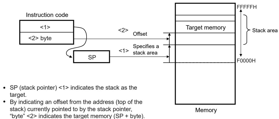
Figure 3-25. Example of [HL + byte], [DE + byte]
