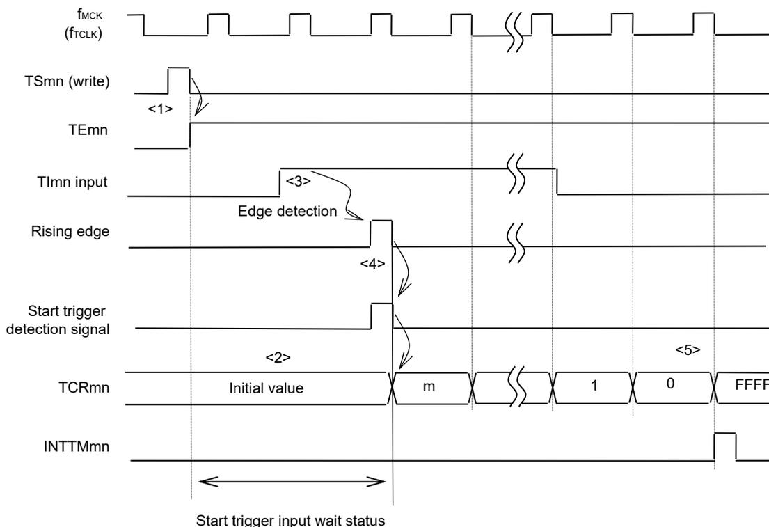
**Remark** The timing is shown in above figure indicates while the noise filter is not used. By making the noise filter on-state, the edge detection becomes 2  $f_{MCK}$  cycles (it sums up to 3 to 4 cycles) later than the normal cycle of  $TI_{mn}$  input. The error per one period occurs be the asynchronous between the period of the  $TI_{mn}$  input and that of the count clock ( $f_{MCK}$ ).
