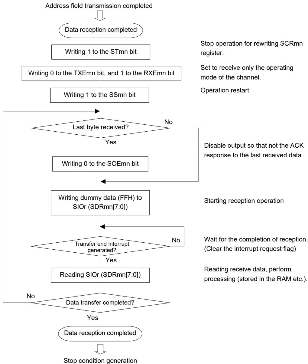
**Caution** ACK is not output when the last data is received (NACK). Communication is then completed by setting “1” to the STmn bit of serial channel stop register m (STm) to stop operation and generating a stop condition.
