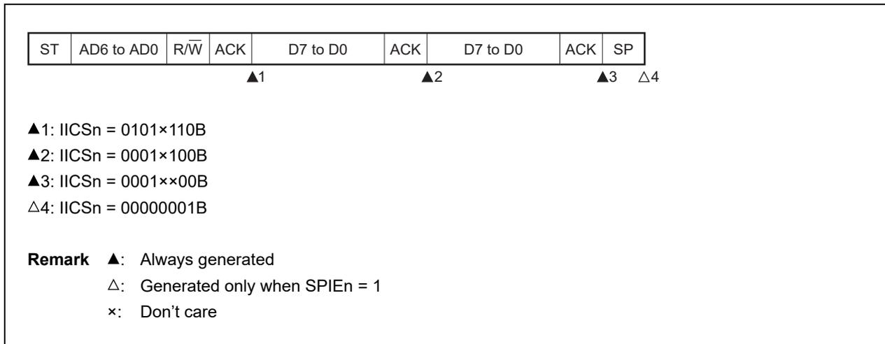
(b) When arbitration loss occurs during transmission of extension code
