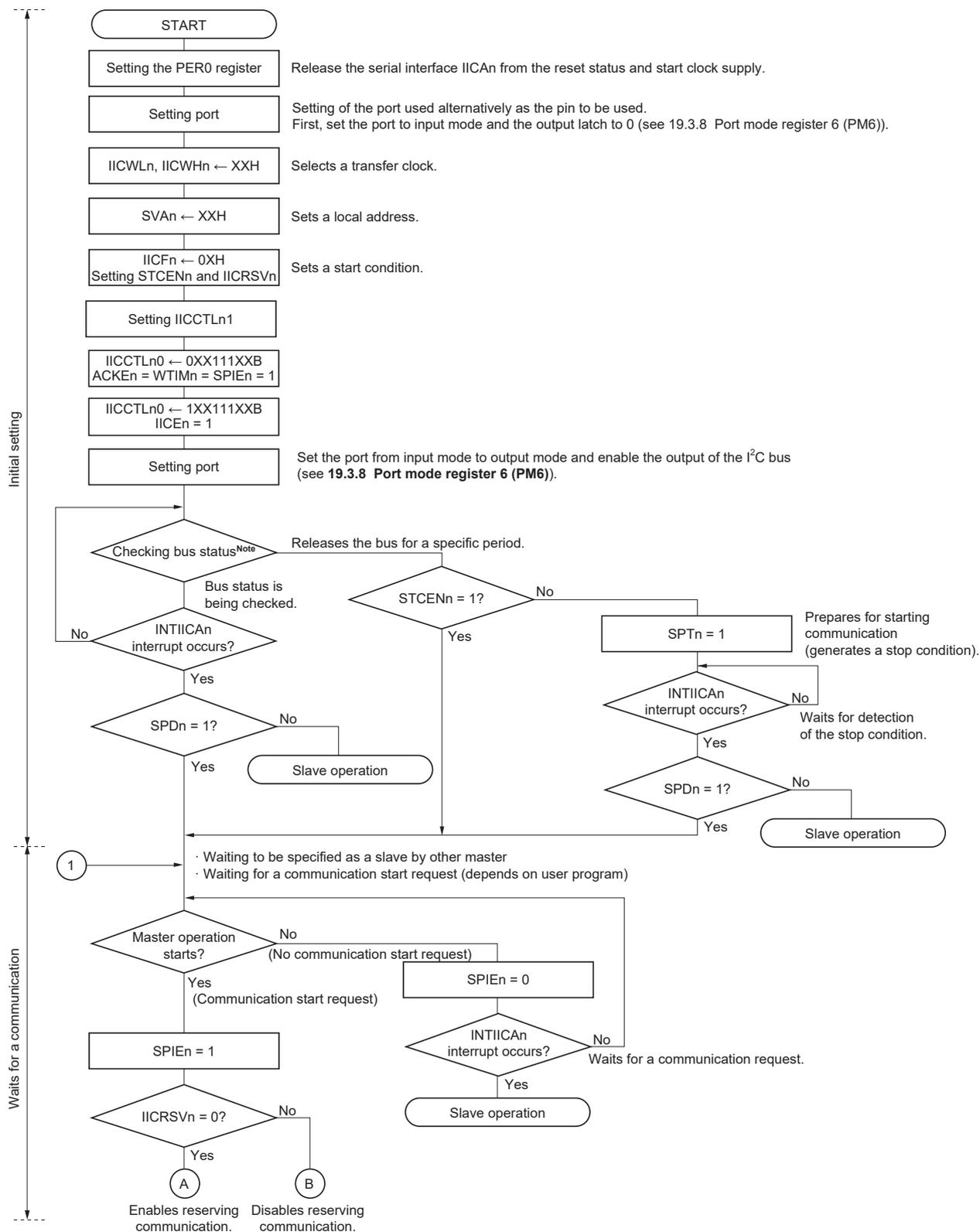
Figure 19-29. Master Operation in Multi-Master System (2/3)
