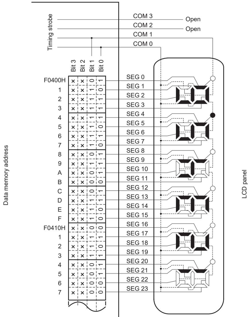
x: Can always be used to store any data because the two-time-slice mode is being used.
