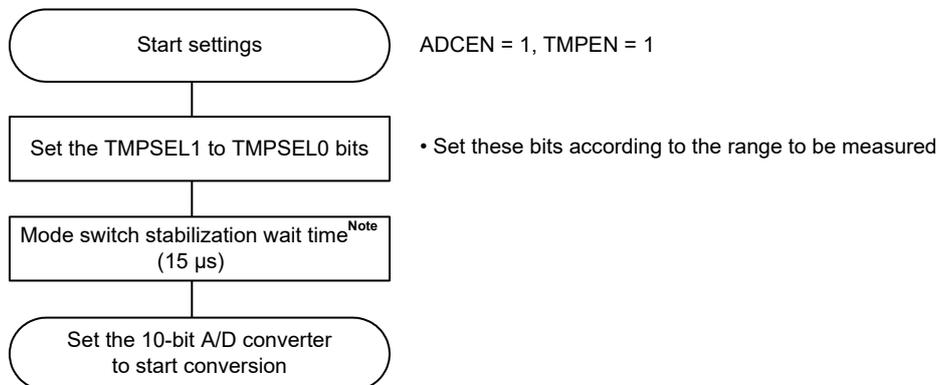
**Note** Mode switch stabilization wait time is required until the A/D converter starts conversion.
