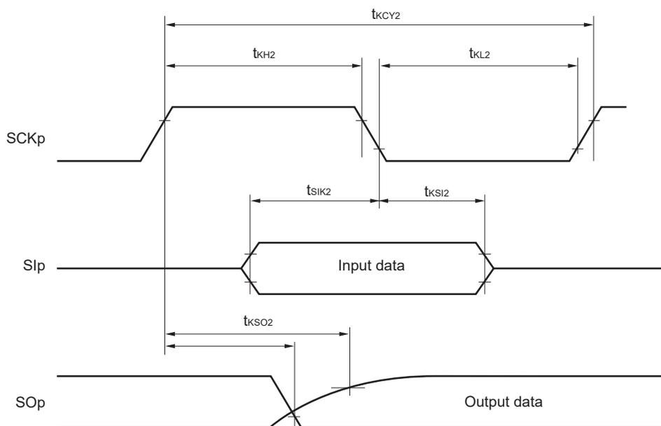
**Caution** Select the TTL input buffer for the SIp pin and SCKp pin and the N-ch open drain output ( $V_{DD}$  tolerance) mode for the SOp pin by using port input mode register g (PIMg) and port output mode register g (POMg). For  $V_{IH}$  and  $V_{IL}$ , see the DC characteristics with TTL input buffer selected.
