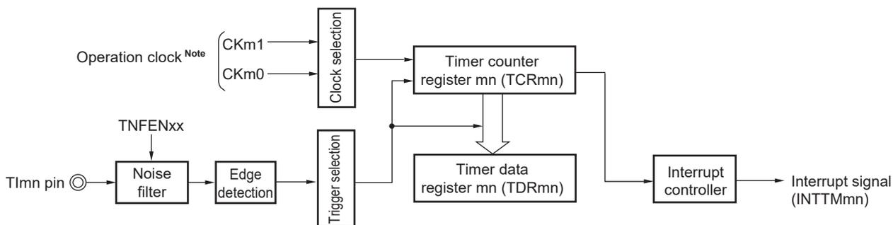
**Note** For channels 1 and 3, the clock can be selected from CKm0, CKm1, CKm2 and CKm3.
