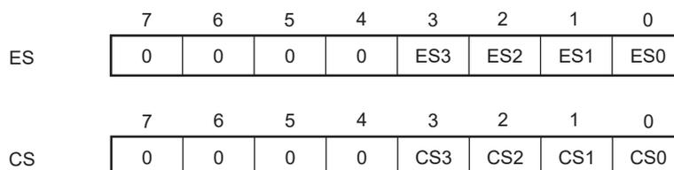
The data area that can be accessed by using 16-bit addresses is the 64 KB from F0000H to FFFFFH. By using the ES register, this area can be extended to the 1 MB from 00000H to FFFFFH.
