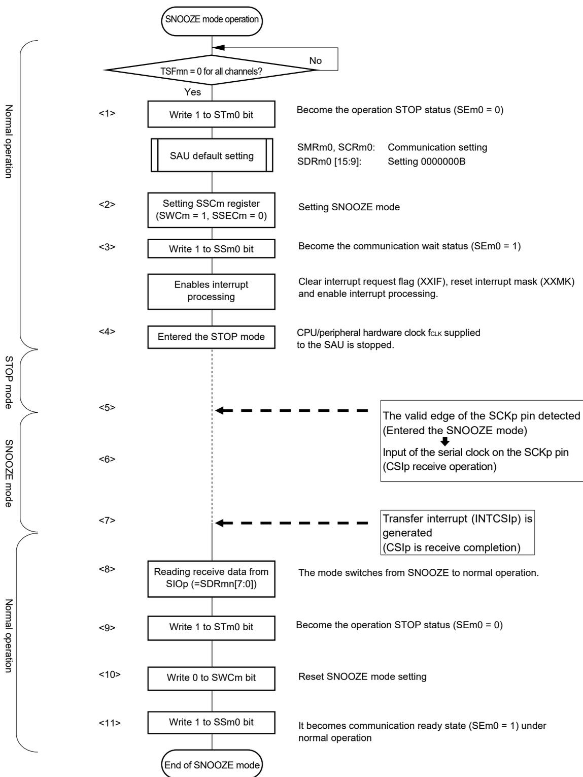
Remarks 1. <1> to <11> in the figure correspond to <1> to <11> in Figure 18-71 Timing Chart of SNOOZE Mode Operation (Once Startup).
