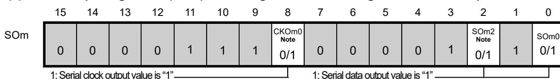
\* When using pins corresponding to each channel as port function pins, set the corresponding CKOm, SOmn bits to "1".
