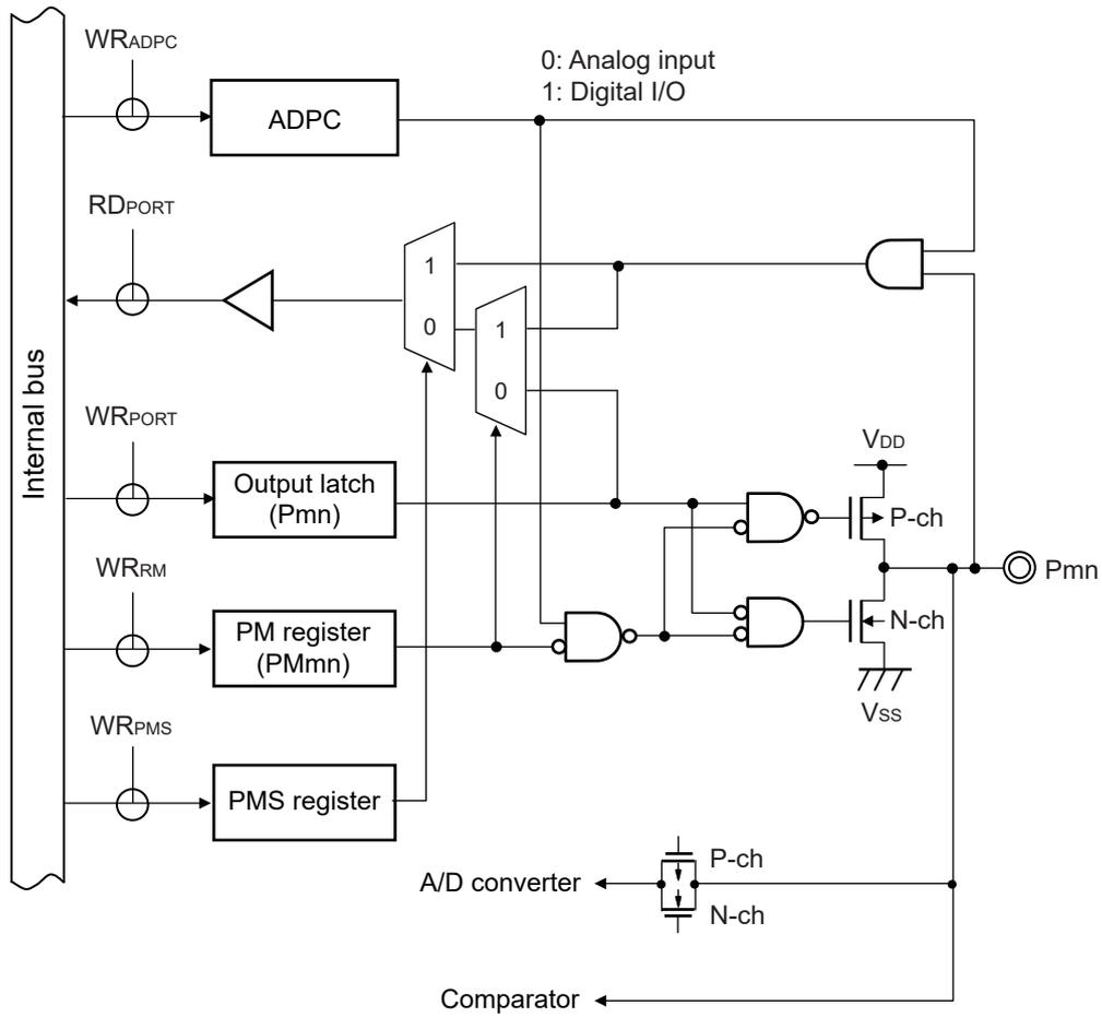
Figure 2-7. Pin Block Diagram for Pin Type 7-1-3
