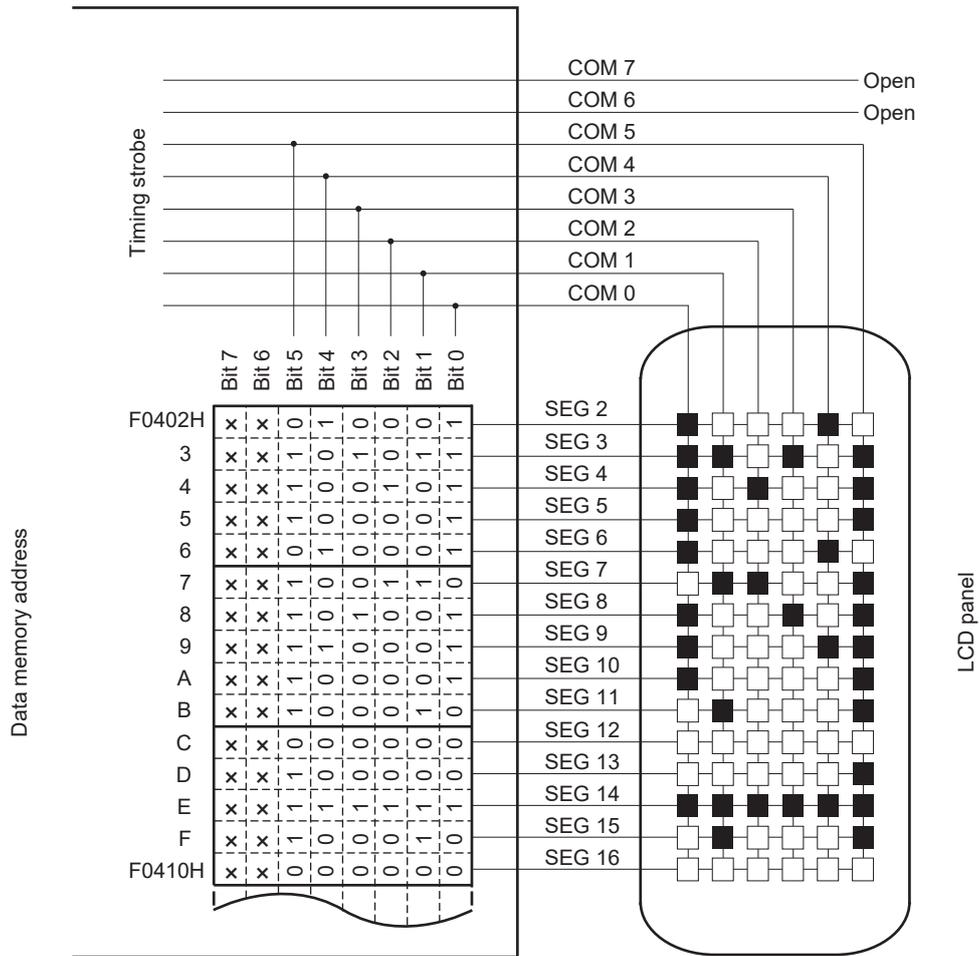
x: Can always be used to store any data because the six-time-slice mode is being used.
