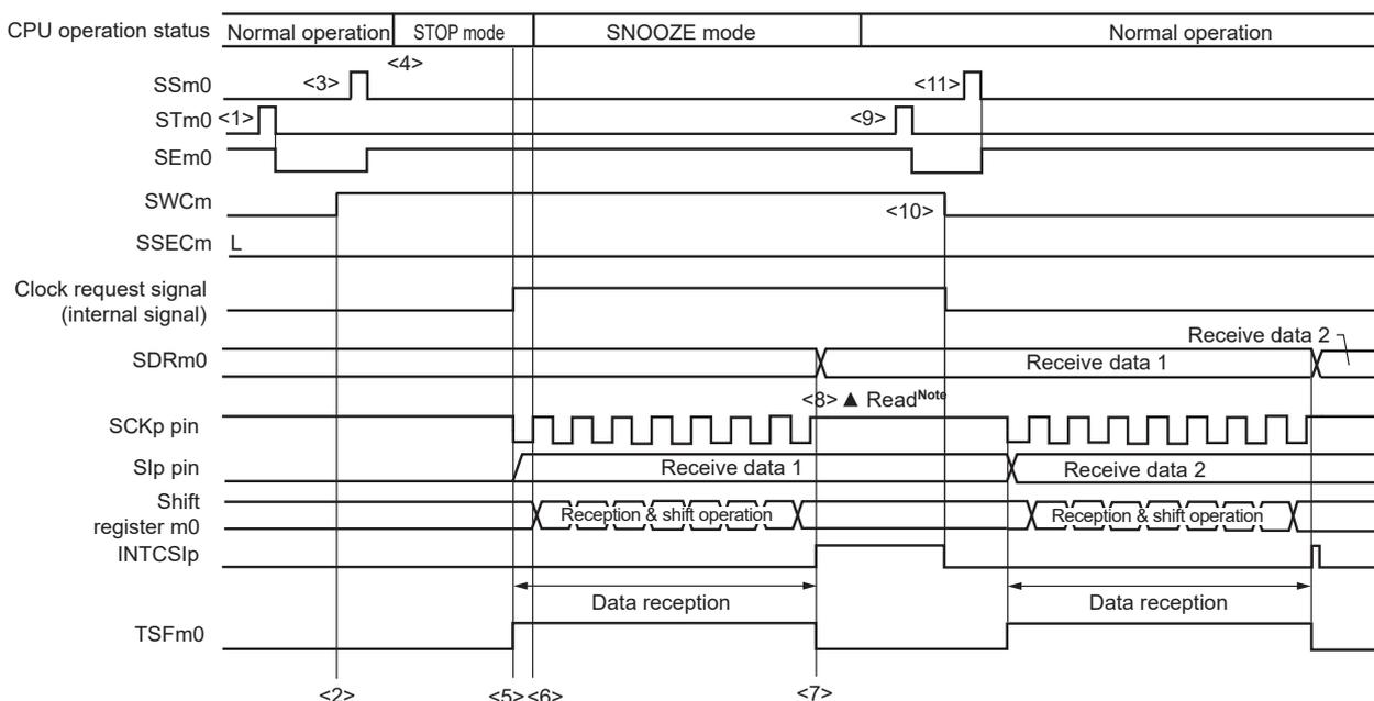
**Note** Only read received data while SWCm = 1 and before the next valid edge of the SCKp pin input is detected.
