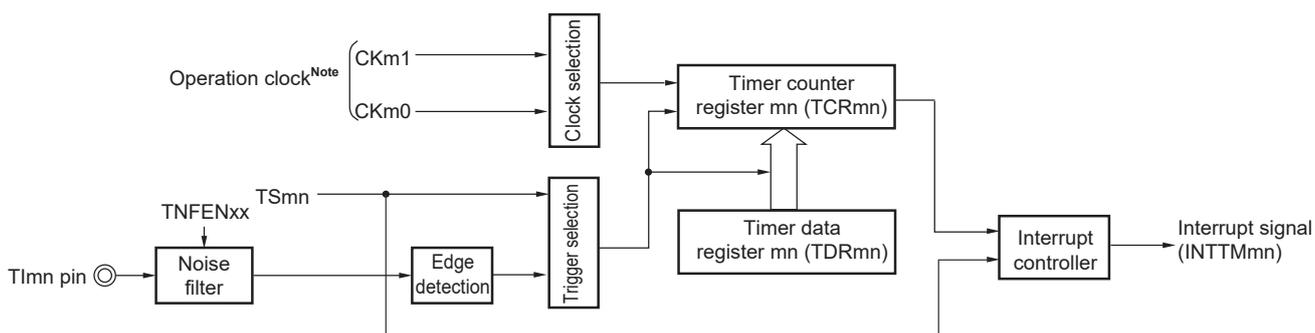
**Note** For using channels 1 and 3, the clock can be selected from CKm0, CKm1, CKm2 and CKm3.
