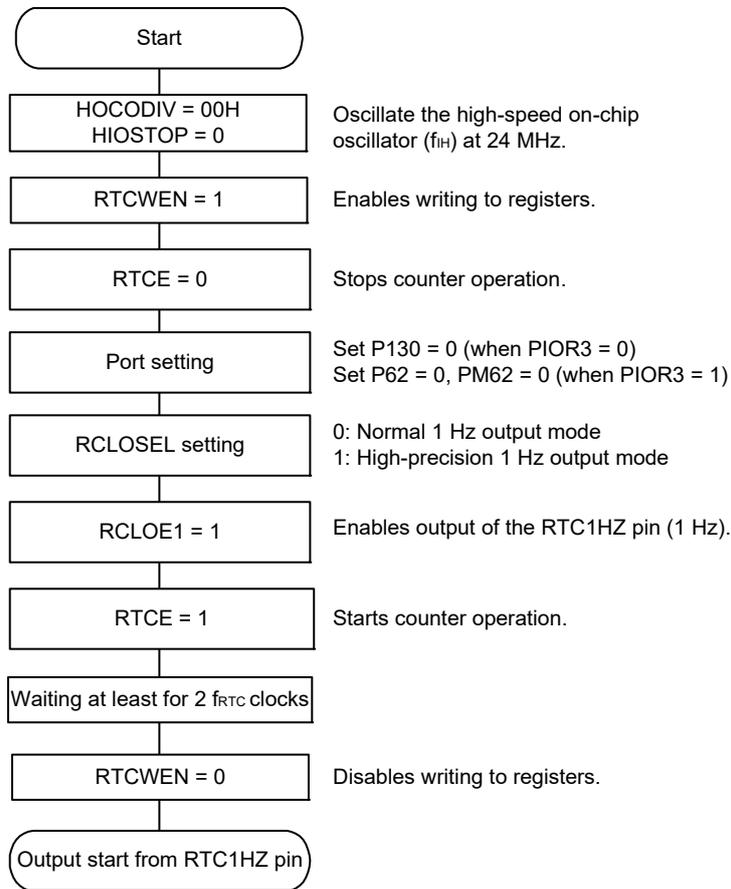
**Caution** When using a high-precision 1 Hz pin output, select 24 MHz for high-speed on-chip oscillator clock ( $f_H$ ) and operate the high-speed on-chip oscillator (HIOSTOP=0). There is no need to select it for CPU clock.
