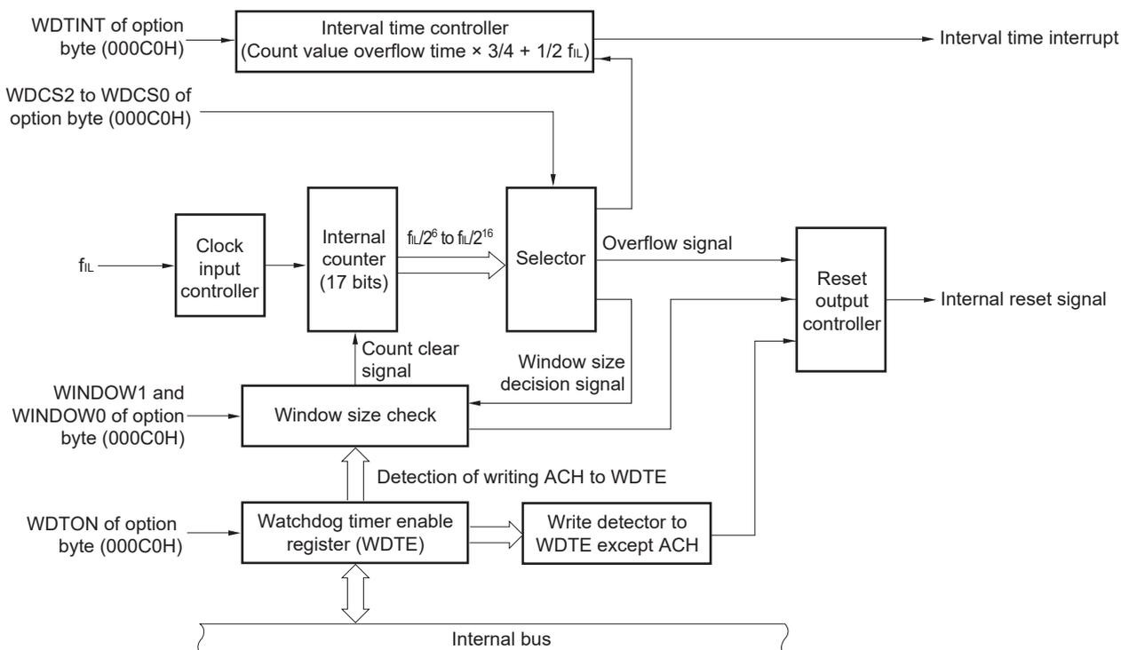
**Remark** f<sub>IL</sub>: Low-speed on-chip oscillator clock
