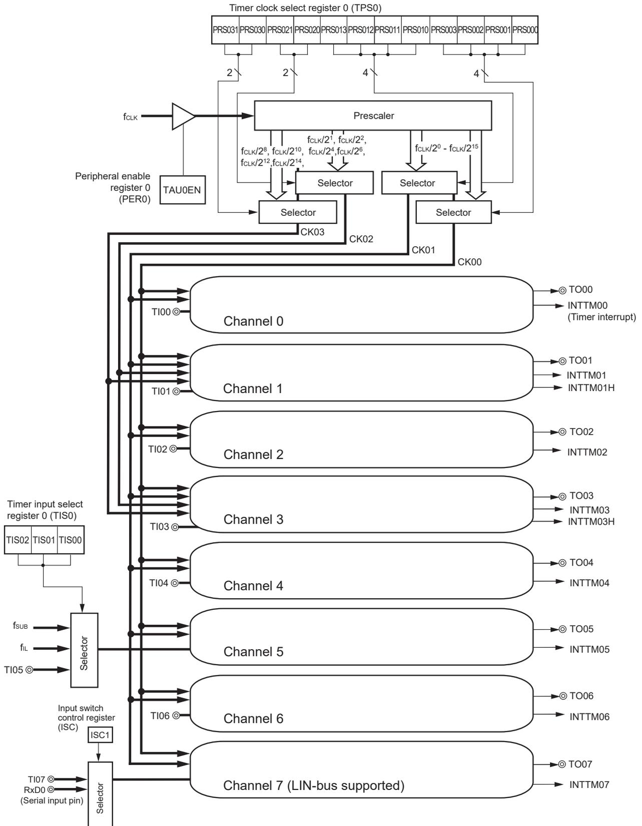
**Remark**  $f_{SUB}$ : Subsystem clock frequency
