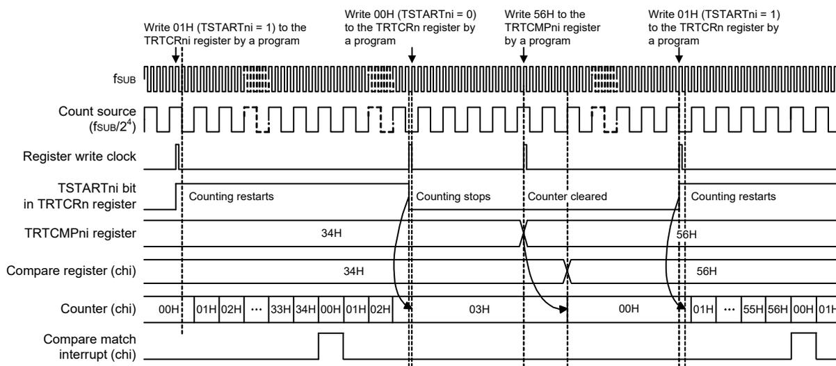
The TCSMDn bit in the TRTCRn register is set to 0 (8-bit counter operation).
