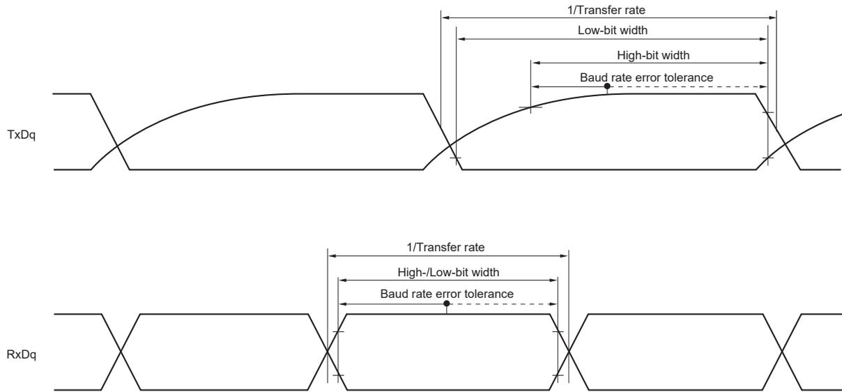
**Caution** Select the TTL input buffer for the RxDq pin and the N-ch open drain output ( $V_{DD}$  tolerance) mode for the TxDq pin by using port input mode register g (PIMg) and port output mode register g (POMg). For  $V_{IH}$  and  $V_{IL}$ , see the DC characteristics with TTL input buffer selected.
