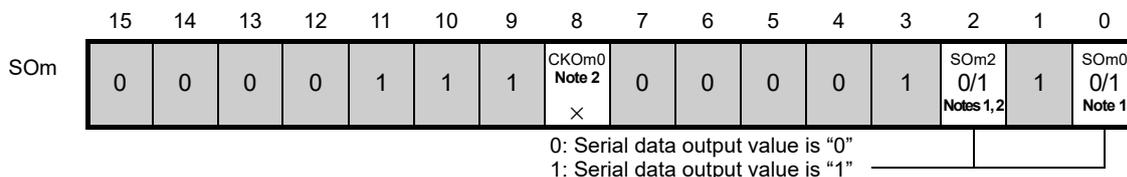
**(f) Serial output enable register m (SOEm) ... Sets only the bits of the target channel to 1.**
