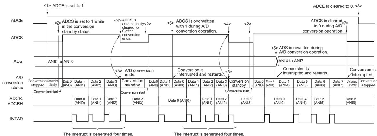
14.6.5 Hardware trigger no-wait mode (select mode, sequential conversion mode)
