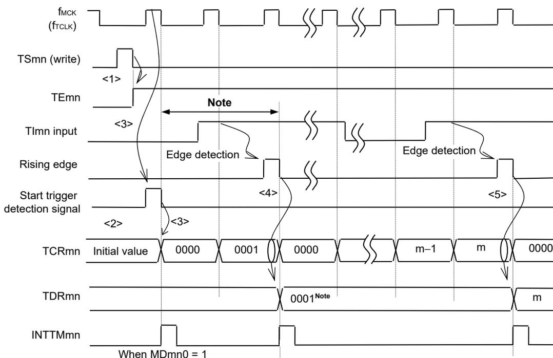
**Note** If a clock has been input to TI<sub>mn</sub> (the trigger exists) when capturing starts, counting starts when a trigger is detected, even if no edge is detected. Therefore, the first captured value (<4>) does not determine a pulse interval (in the above figure, 0001 just indicates two clock cycles but does not determine the pulse interval) and so the user can ignore it.
