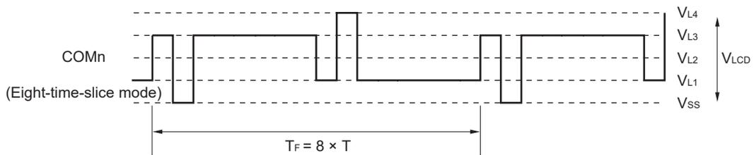
T: One LCD clock period       $T_F$ : Frame frequency
