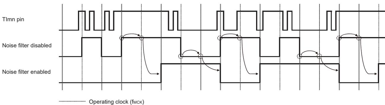
**Caution** The Tl<sub>mn</sub> pin input waveform is shown to explain the noise filter ON/OFF operation. For actual operation, refer to the high-level width/low-level width in 37.4 AC Characteristics.
