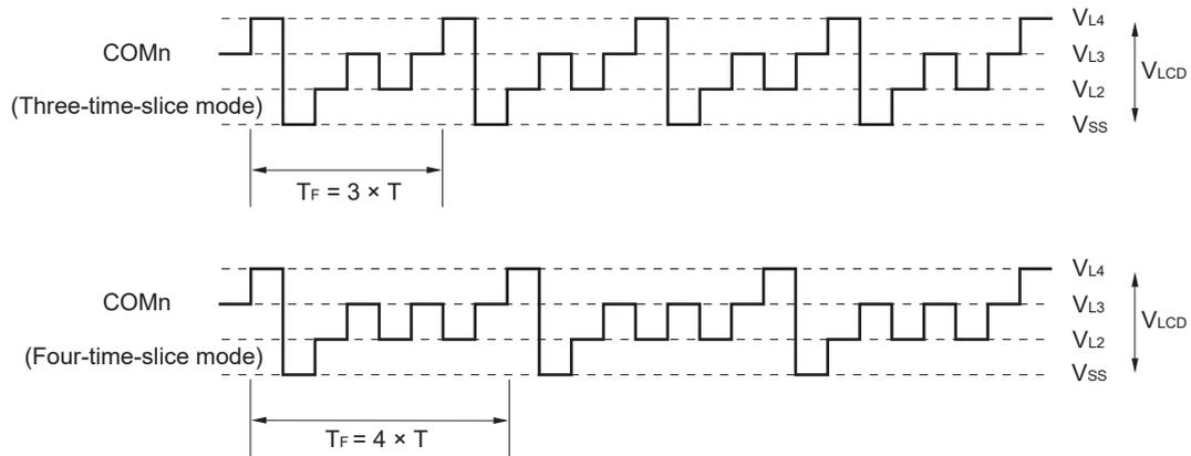
T: One LCD clock period       $T_F$ : Frame frequency
