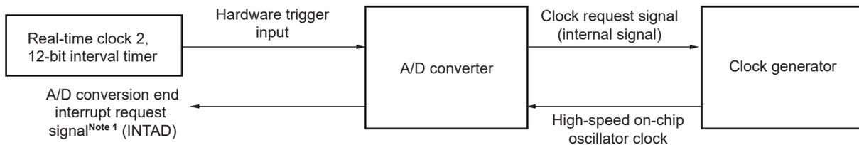
When using the SNOOZE mode function, the initial setting of each register is specified before switching to the STOP mode (for details about these settings, see **14.7.3 Setting up hardware trigger wait mode**<sup>Note 2</sup>). Just before move to STOP mode, bit 2 (AWC) of A/D converter mode register 2 (ADM2) is set to 1. After the initial settings are specified, bit 0 (ADCE) of A/D converter mode register 0 (ADM0) is set to 1.
