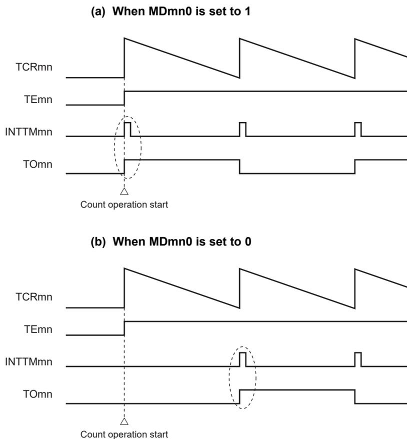
When MDmn0 is set to 1, a timer interrupt (INTTMmn) is output at count operation start, and TOMn performs a toggle operation.
