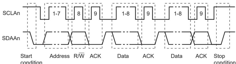
The master device generates the start condition, slave address, and stop condition. The acknowledge (ACK) can be generated by either the master or slave device (normally, it is output by the device that receives 8-bit data).
