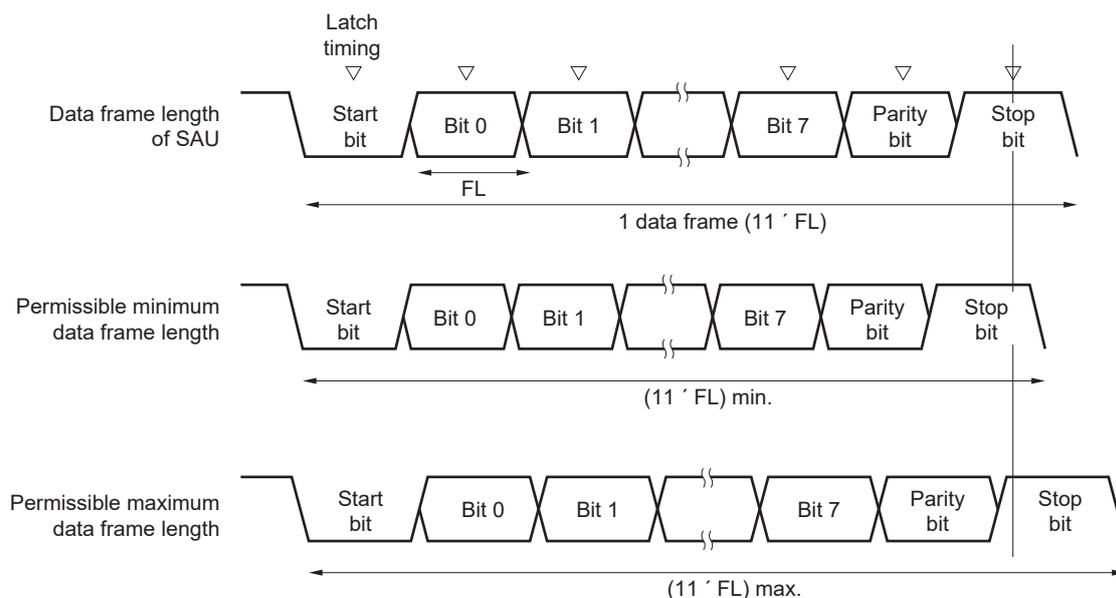
As shown in Figure 18-95, the timing of latching receive data is determined by the division ratio set by bits 15 to 9 of serial data register mn (SDRmn) after the start bit is detected. If the last data (stop bit) is received before this latch timing, the data can be correctly received.
