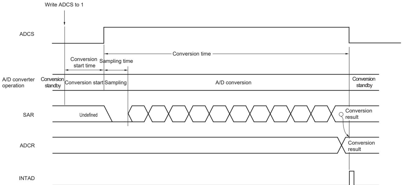
In one-shot conversion mode, the ADCS bit is automatically cleared to 0 after completion of A/D conversion.
