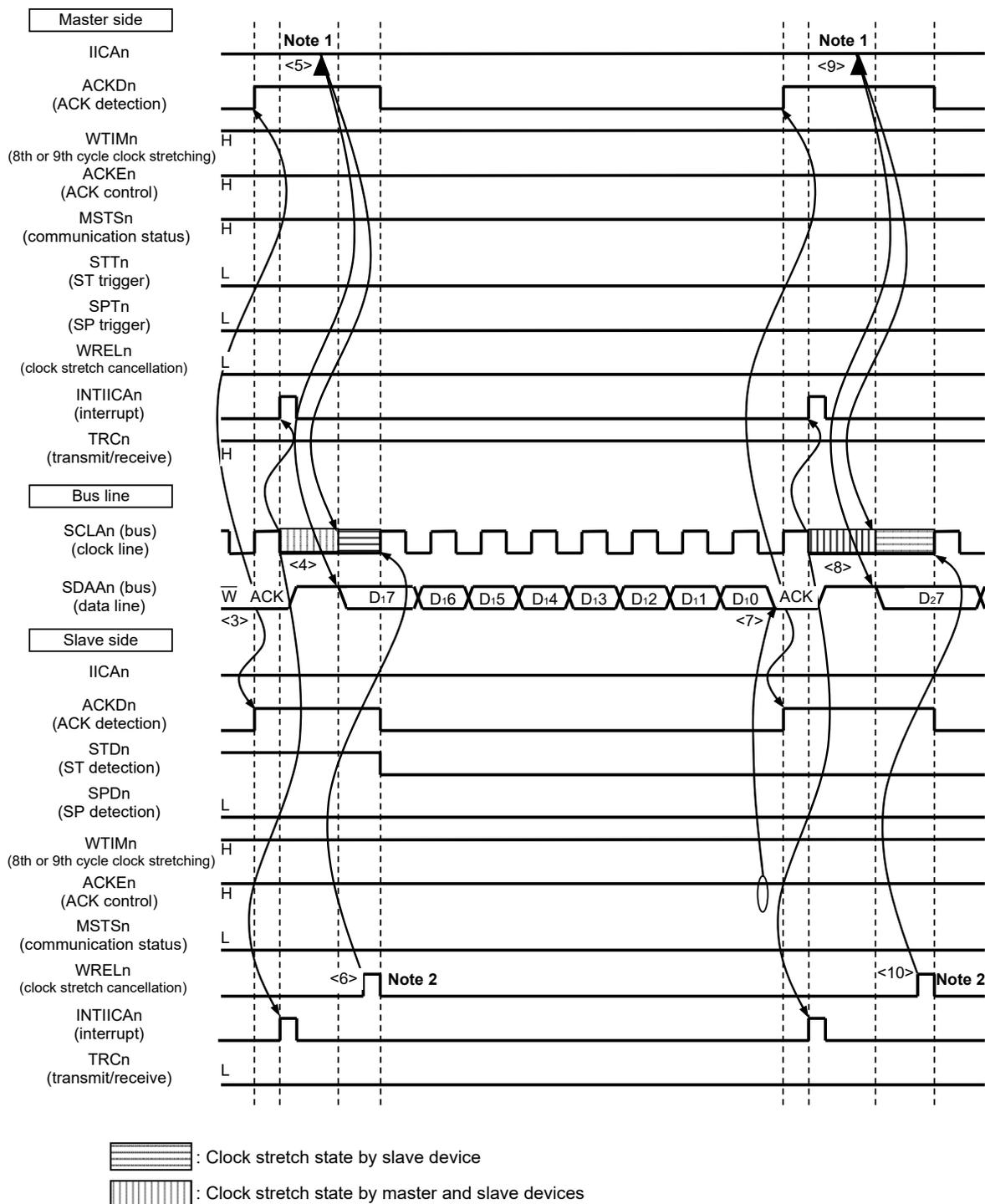
**Notes 1.** Write data to IICAn, not setting the WRELn bit, in order to cancel a clock stretch state during transmission by a master device.
