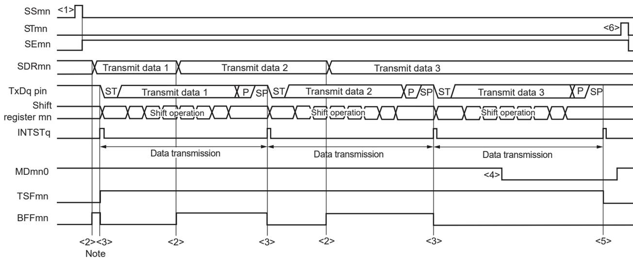
**Note** If transmit data is written to the SDRmn register while the BFFmn bit of serial status register mn (SSRmn) is 1 (valid data is stored in serial data register mn (SDRmn)), the transmit data is overwritten.
