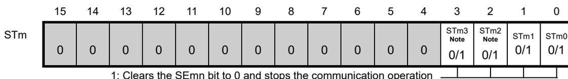
\* Because the STmn bit is a trigger bit, it is cleared immediately when SEmn = 0.
