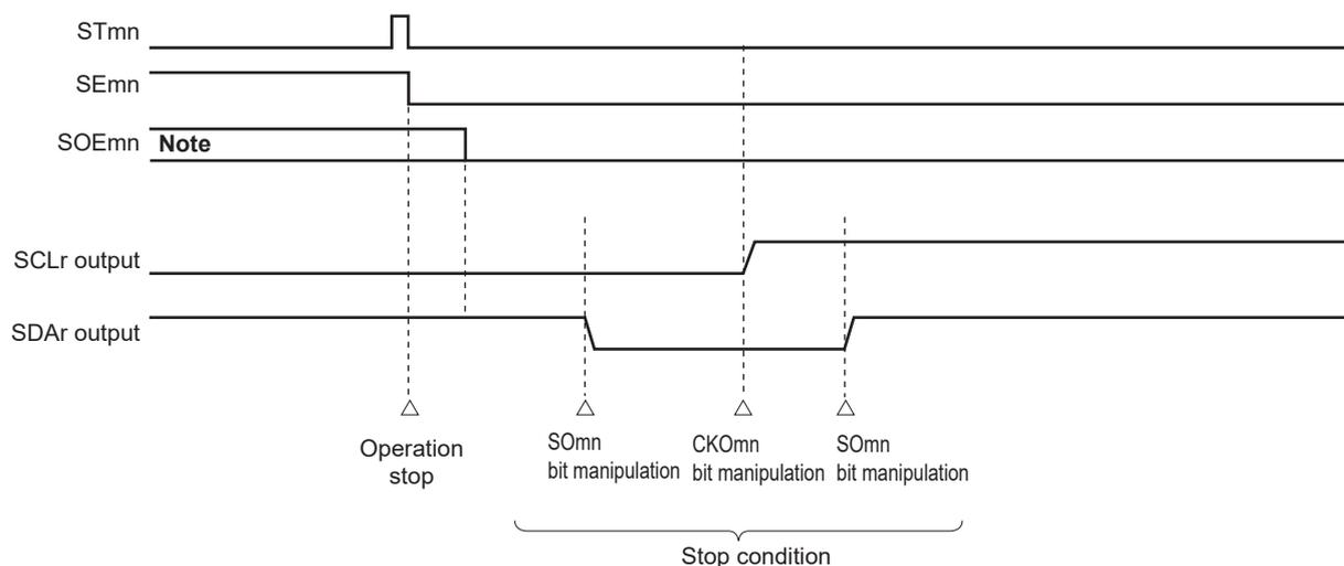
**Note** During a receive operation, the SOEmn bit of serial output enable register m (SOEm) is cleared to 0 before receiving the last data.
