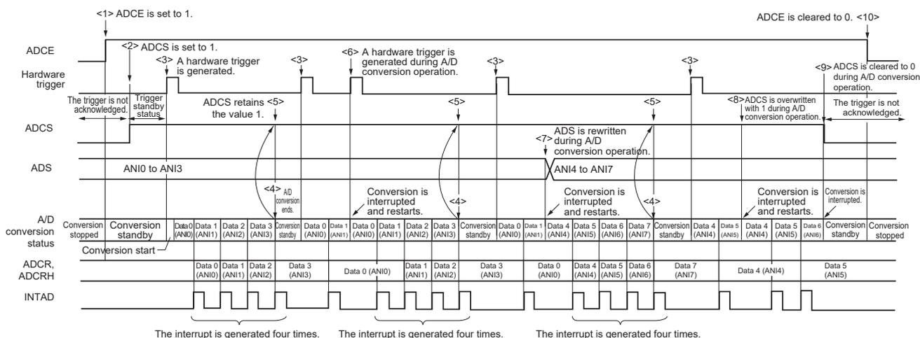
14.6.9 Hardware trigger wait mode (select mode, sequential conversion mode)
