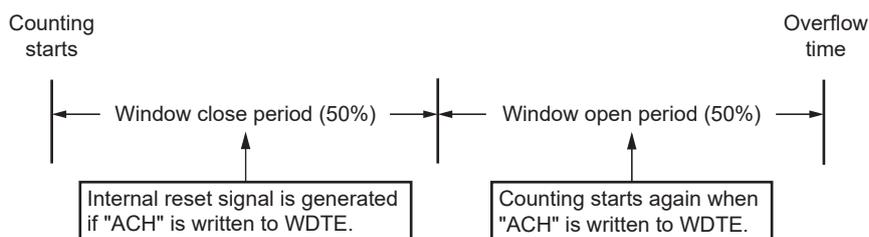
**Caution** When data is written to the WDTE register for the first time after reset release, the watchdog timer is cleared in any timing regardless of the window open time, as long as the register is written before the overflow time, and the watchdog timer starts counting again.
