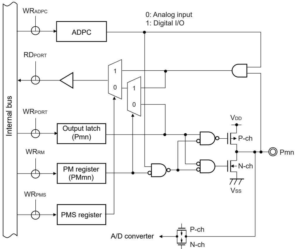
Figure 2-6. Pin Block Diagram for Pin Type 4-9-2
