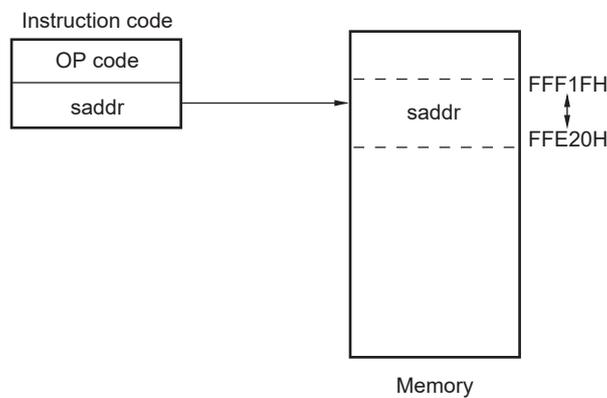
**Remark** SADDR and SADDRP are used to describe the values of addresses FE20H to FF1FH with 16-bit immediate data (higher 4 bits of actual address are omitted), and the values of addresses FFE20H to FFF1FH with 20-bit immediate data.
