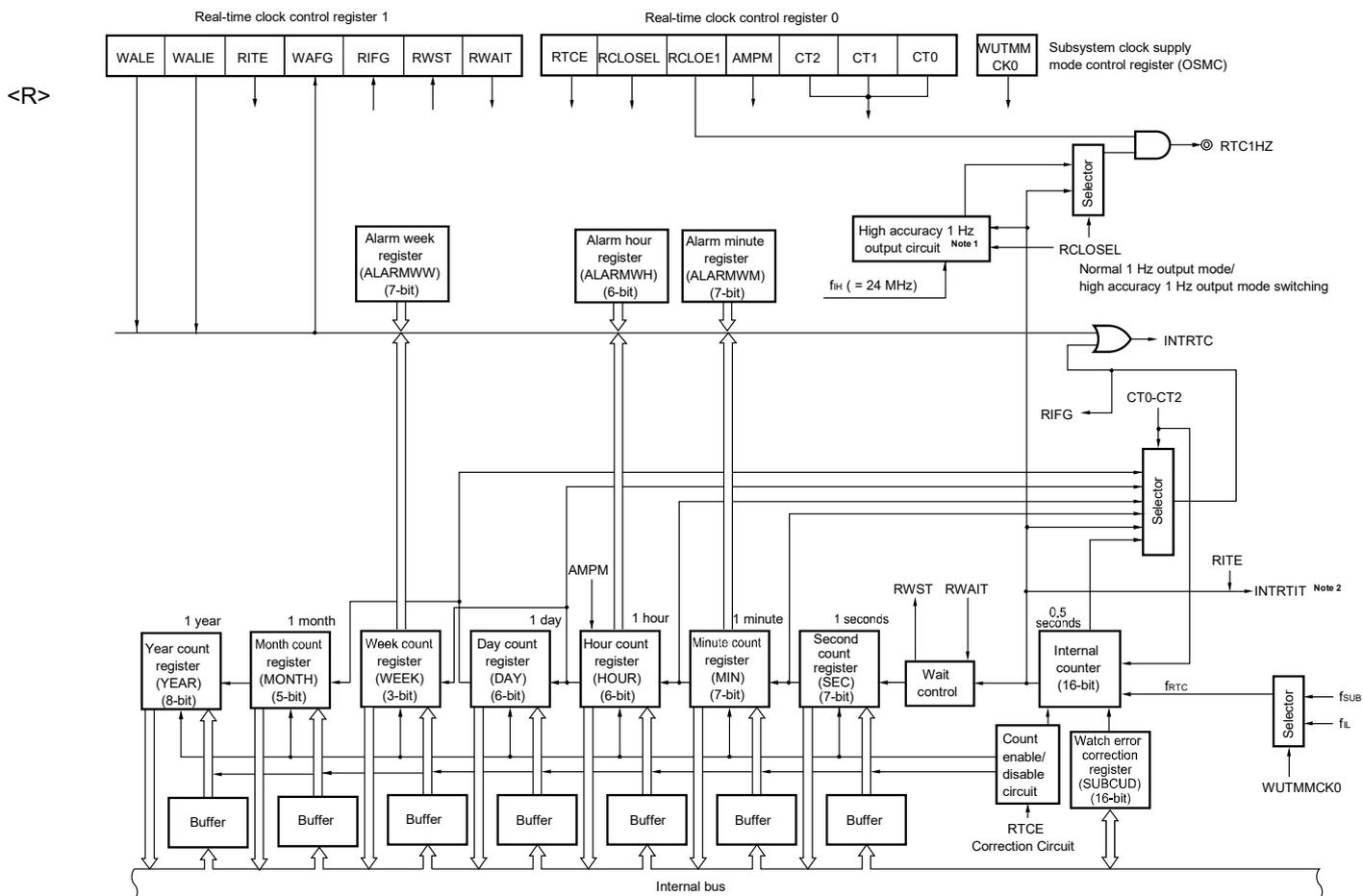
**Notes 1.** A high-speed on-chip oscillator (HOCO: 24 MHz) can be used for high precision 1 Hz output. HOCO must be set to ON in order to run in high precision 1 Hz output mode. To run in normal 1 Hz mode, there is no need to set HOCO to ON.
