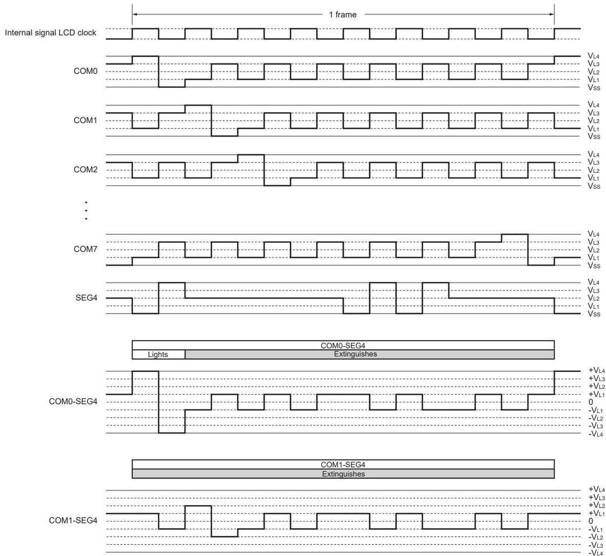
**Figure 21-43. Eight-Time-Slice LCD Drive Waveform Examples Between SEG4 and Each Common Signals (1/4 Bias Method) (2/2)**
