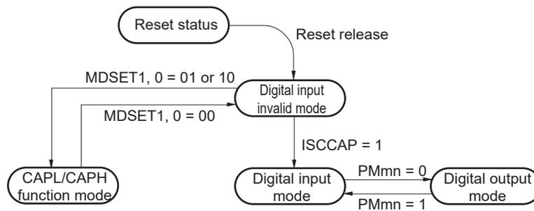
**Caution** Be sure to set the CAPL/CAPH function mode before segment output starts (while SCOC of LCD mode register 1 (LCDM1) is 0).
