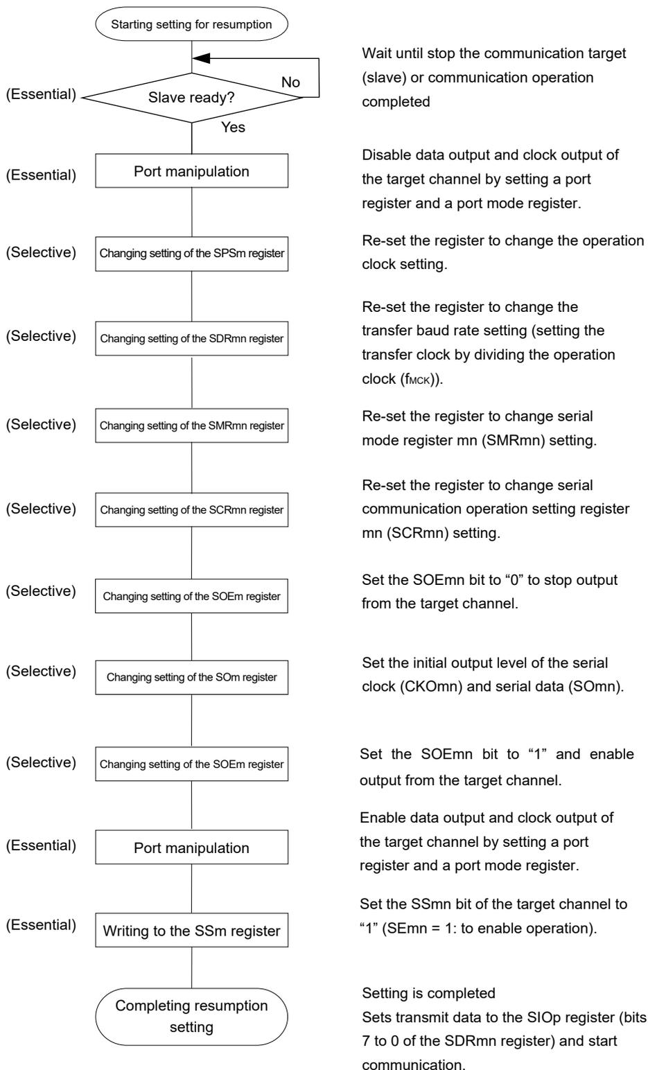
**Remark** If PER0 is rewritten while stopping the master transmission and the clock supply is stopped, wait until the transmission target (slave) stops or transmission finishes, and then perform initialization instead of restarting the transmission.
