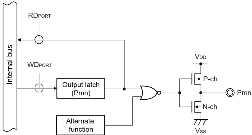
Figure 2-2. Pin Block Diagram for Pin Type 2-1-1
