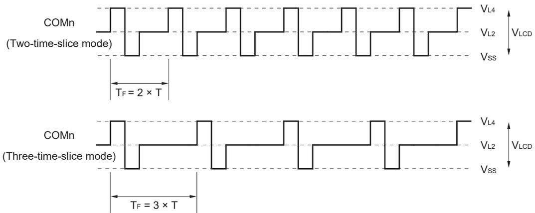
T: One LCD clock period       $T_F$ : Frame frequency
