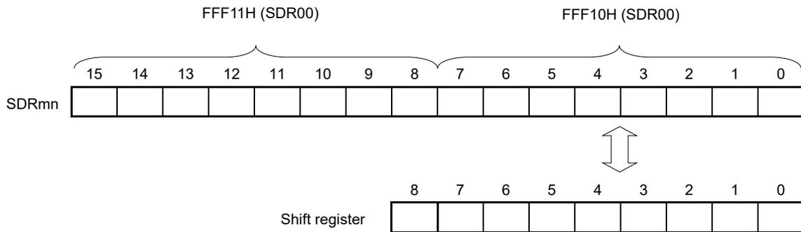
**Remark** For the function of the higher 7 bits of the SDRmn register, see **18.3 Registers Controlling Serial Array Unit**.
