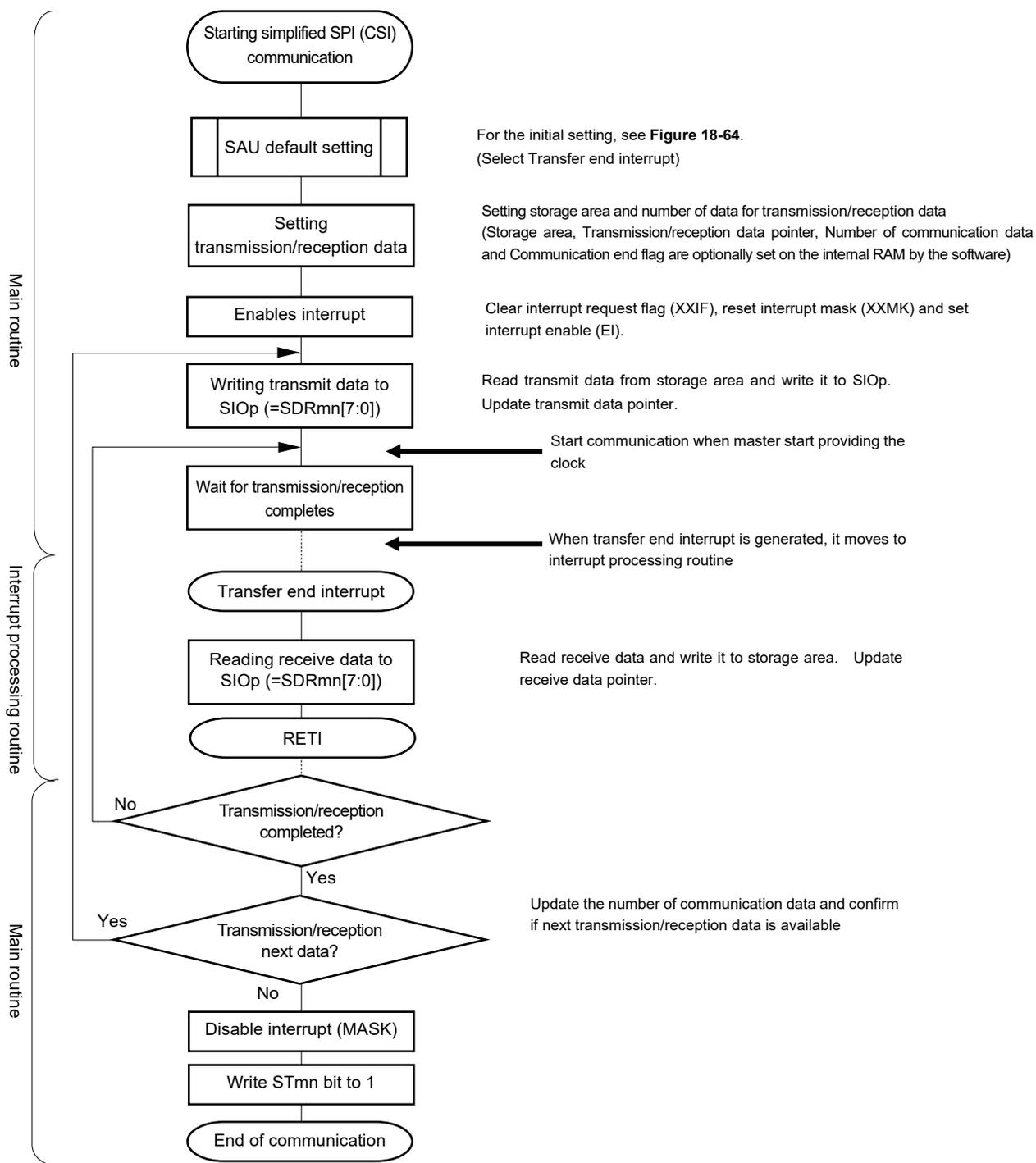
**Caution** Be sure to set transmit data to the SIOp register before the clock from the master is started.
