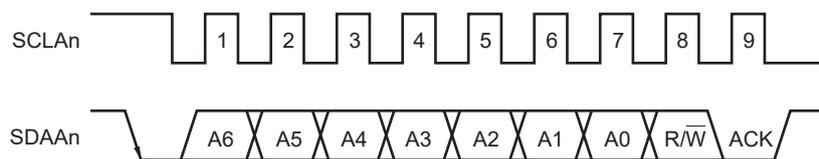
When the local address is received, ACK is automatically generated, regardless of the value of the ACKEn bit. When an address other than that of the local address is received, ACK is not generated (NACK).
