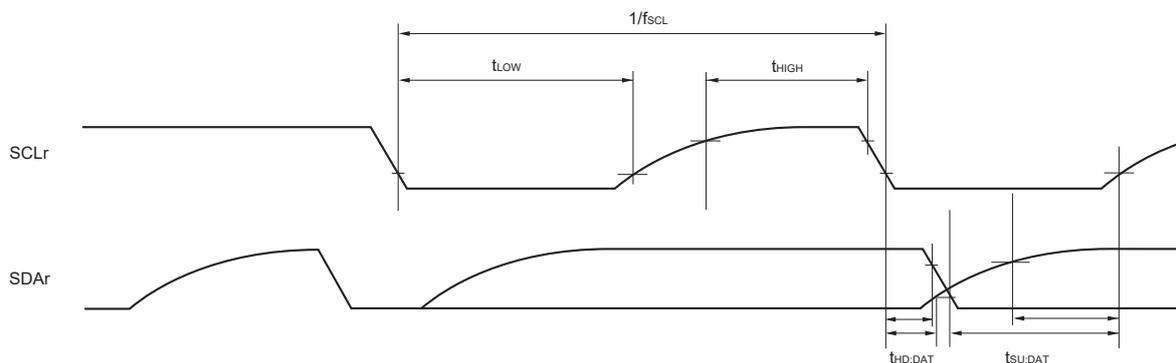
**Caution** Select the TTL input buffer and the N-ch open drain output ( $V_{DD}$  tolerance) mode for the SDAr pin and the N-ch open drain output ( $V_{DD}$  tolerance) mode for the SCLr pin by using port input mode register g (PIMg) and port output mode register g (POMg). For  $V_{IH}$  and  $V_{IL}$ , see the DC characteristics with TTL input buffer selected.
