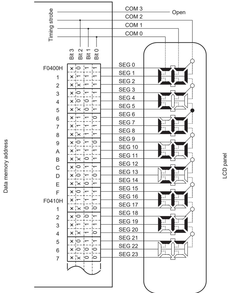
x': Can be used to store any data because there is no corresponding segment in the LCD panel.
