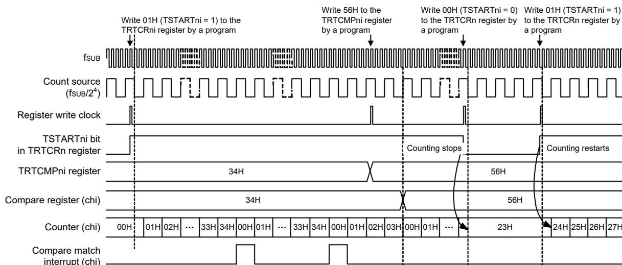
The TCSMDn bit in the TRTCRn register is set to 0 (8-bit counter operation).
