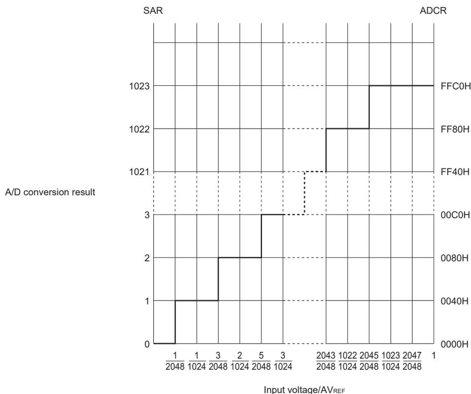
**Remark** AV<sub>REF</sub>: The + side reference voltage of the A/D converter. This can be selected from AV<sub>REFP</sub>, the internal reference voltage (1.45 V), and V<sub>DD</sub>.
