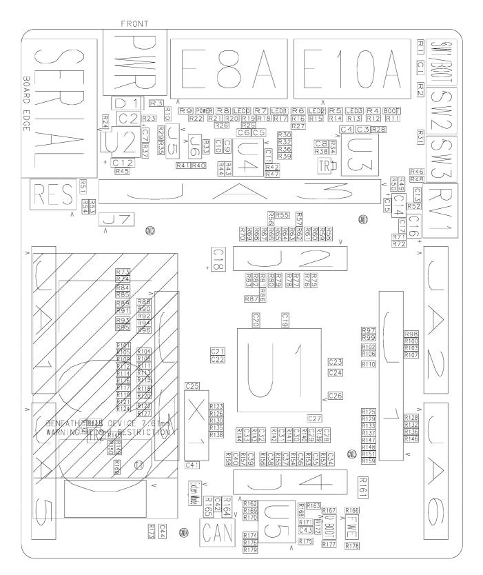
Figure 11-1: Component Placement – Front view
