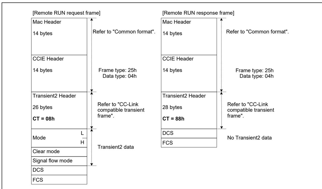
Figure 7.8 Overview of Remote RUN Frame Format
