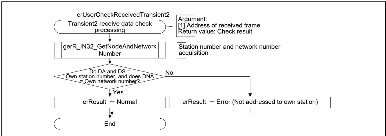
Figure 4.25 Flowchart for Transient2 Receive Data Check Processing
