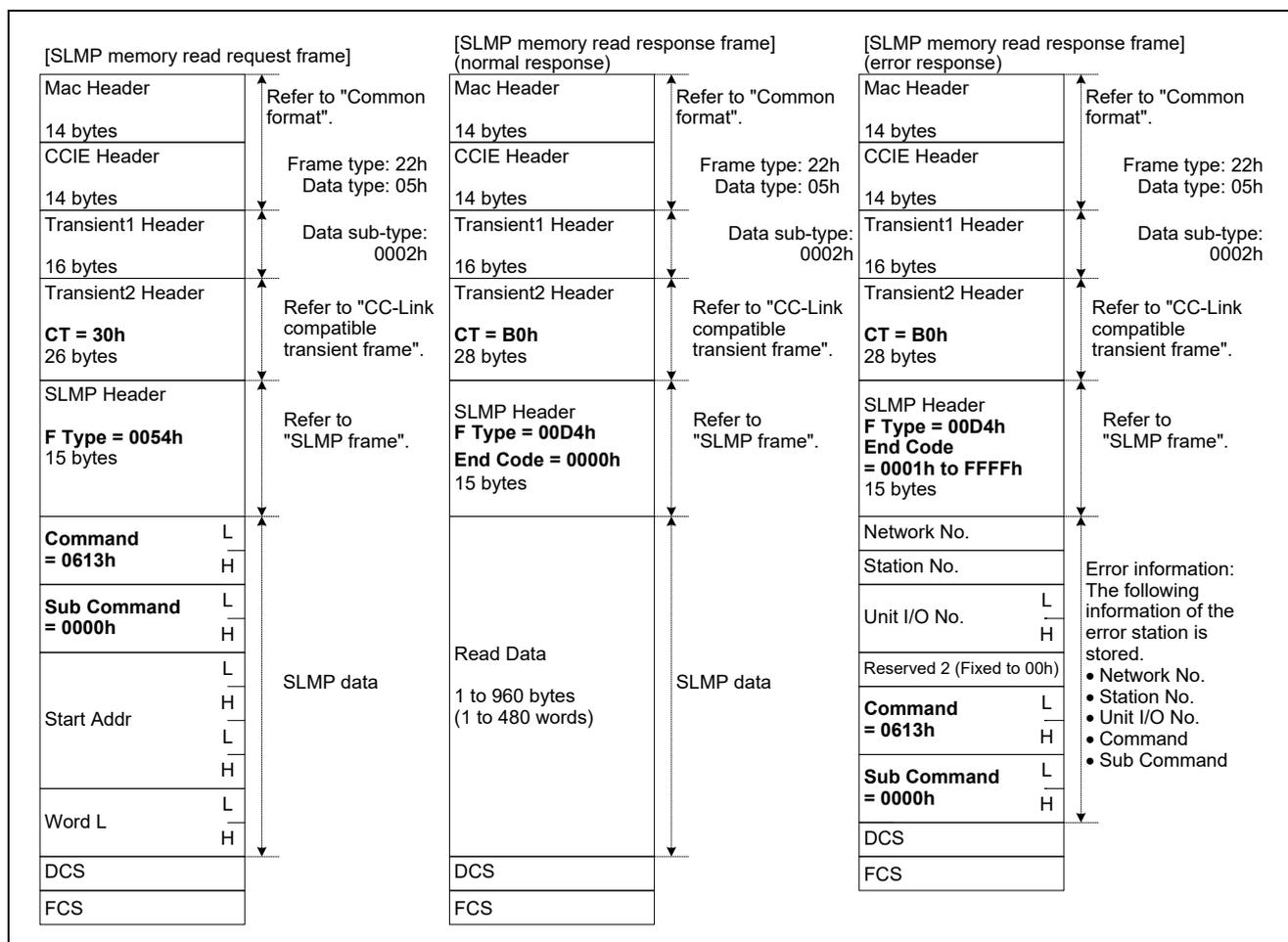
Figure 7.15 Overview of SLMP Memory Read Frame Format
