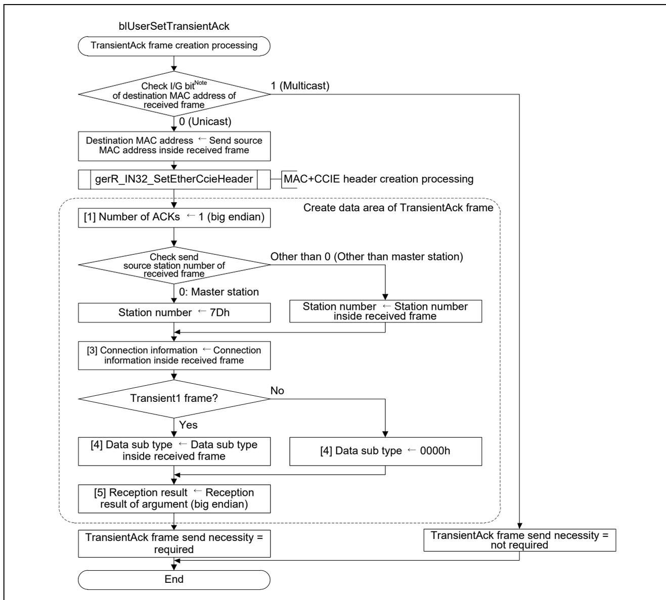
Figure 4.29Flowchart for TransientAck Frame Creation Processing
