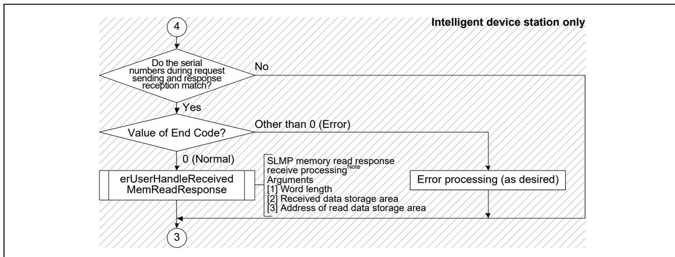
Figure 4.17 Flowchart for Transient1 Receive Data Processing (4/4)
