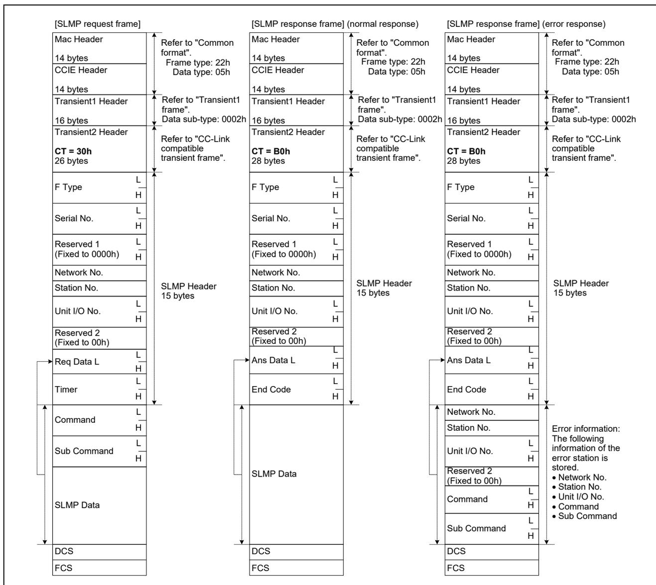
Figure 7.14 Overview of SLMP Frame Basic Format
