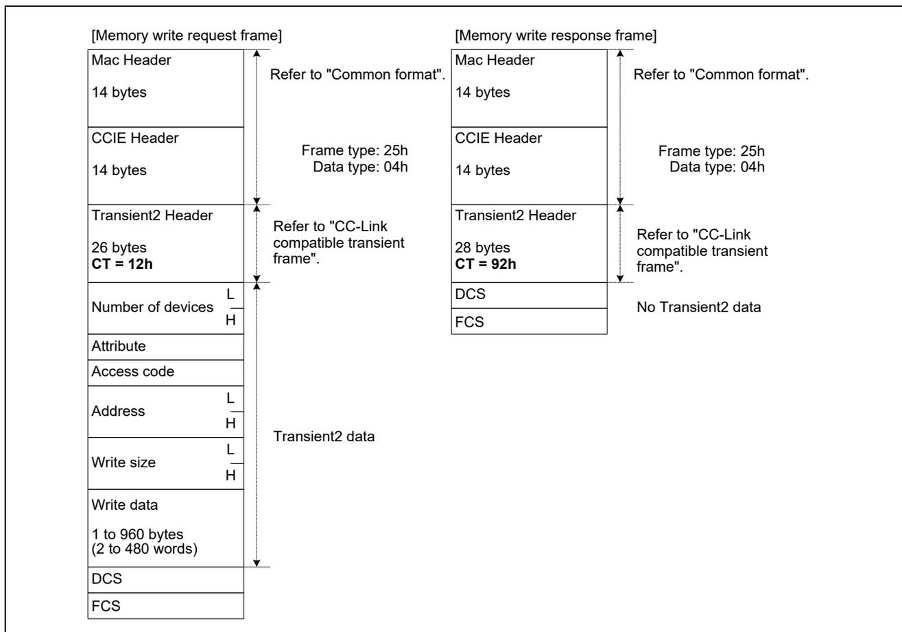
Figure 7.11 Overview of Memory Write Frame Format
