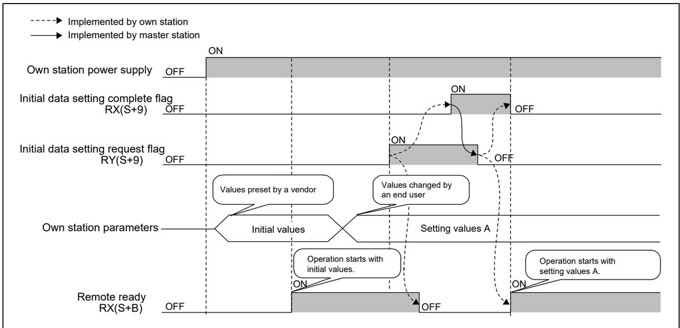
Figure 6.3 Timing Chart: Initial Data Setting Complete/Request Flag
