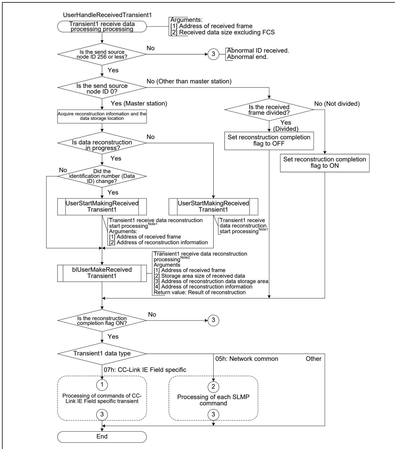
Figure 4.17 Flowchart for Transient1 Receive Data Processing (1/4)
