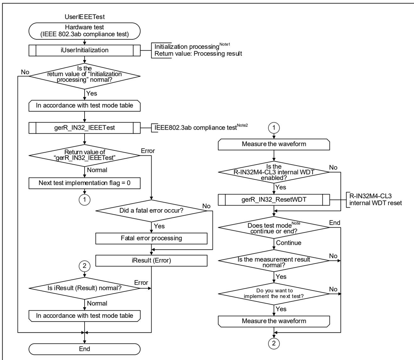
Figure 4.40 Flowchart for Hardware Test (IEEE802.3ab Compliance Test)
