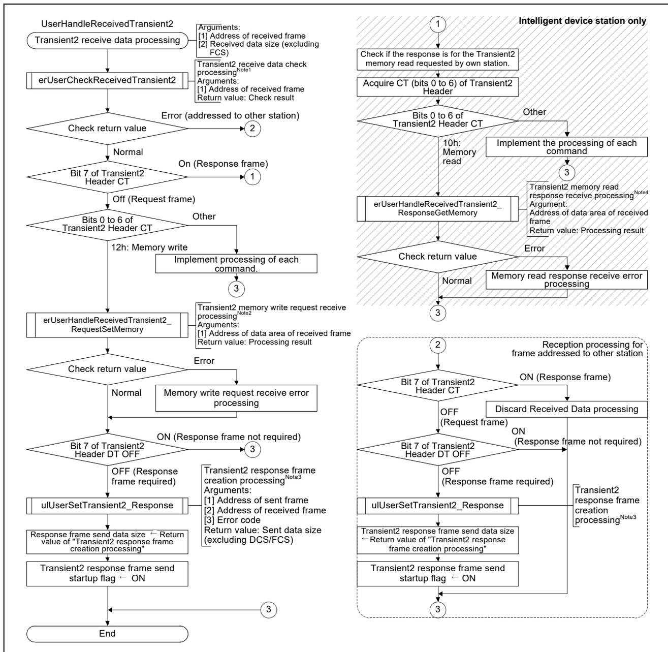
Figure 4.24 Flowchart for Transient2 Receive Data Processing
