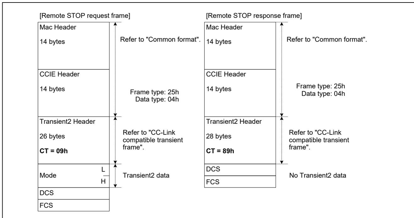
Figure 7.9 Overview of Remote STOP Frame Format
