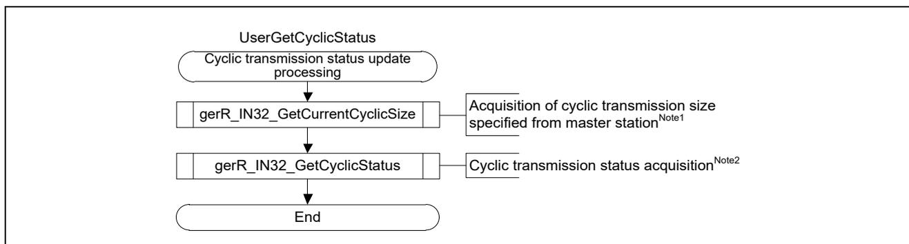
Figure 4.12 Flowchart for Cyclic Transmission Status Update Processing
