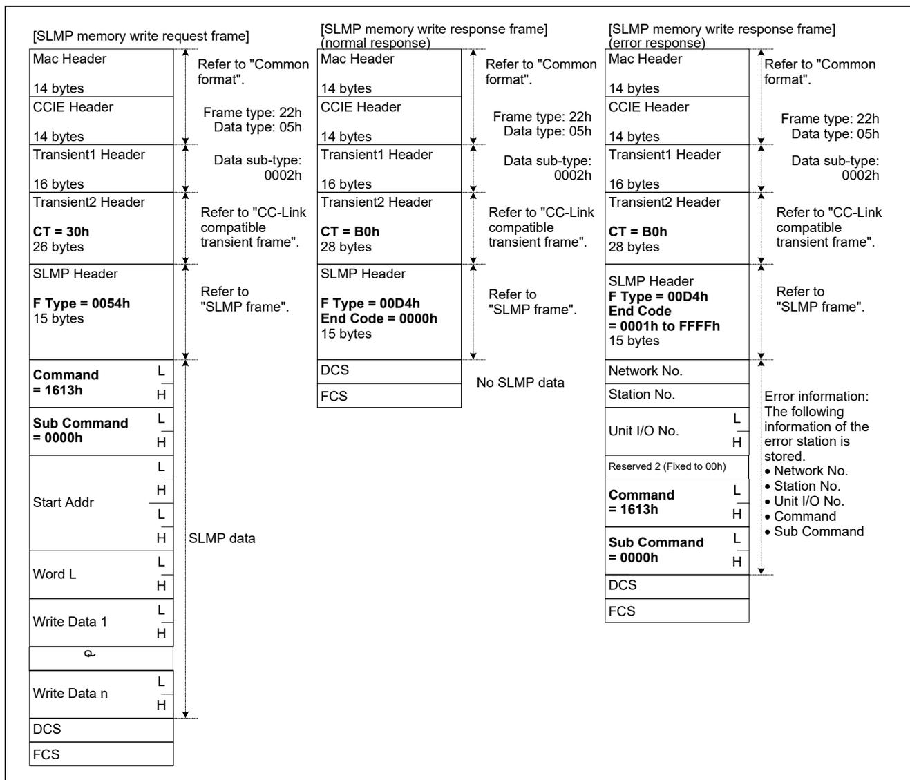
Figure 7.16 Overview of SLMP Memory Write Frame Format
