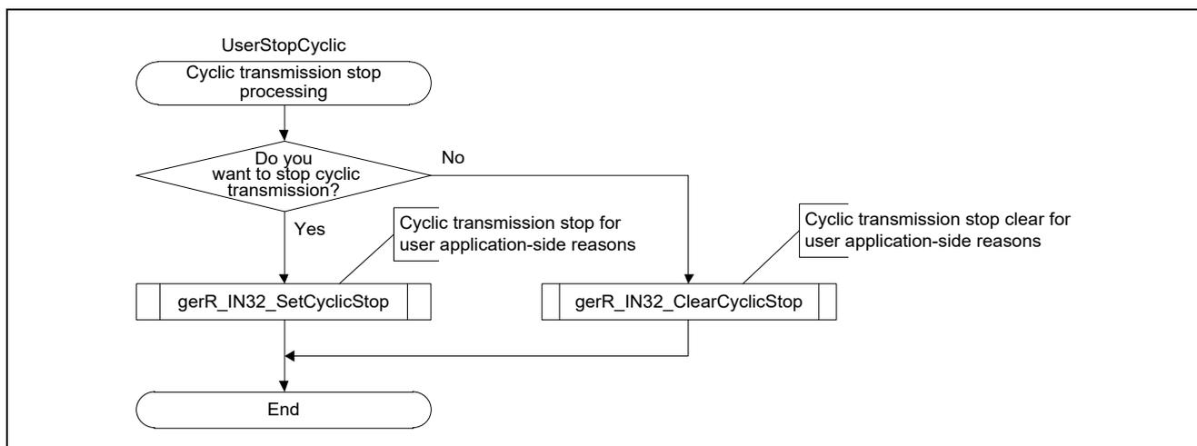
Figure 4.5 Flowchart for Cyclic Transmission Stop Processing
