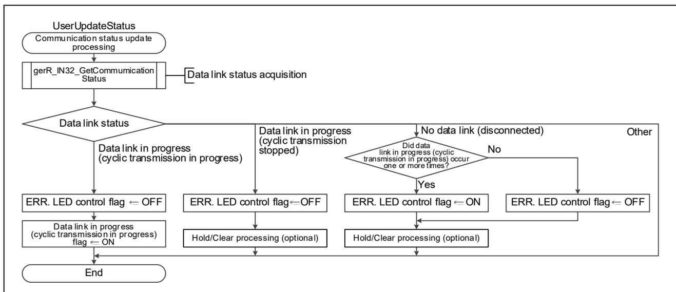
Figure 4.10 Flowchart for Communication Status Update Processing
