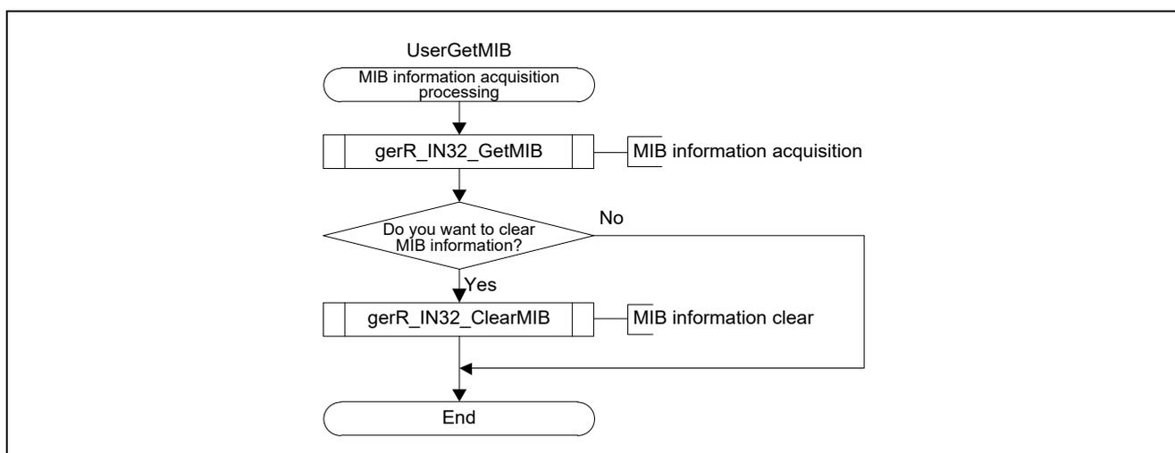
Figure 4.13 Flowchart for MIB Information Acquisition Processing
