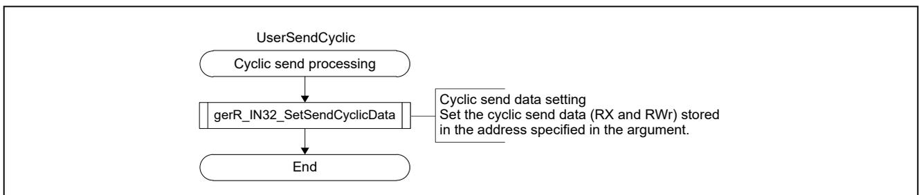
Figure 4.9 Flowchart for Cyclic Send Processing
