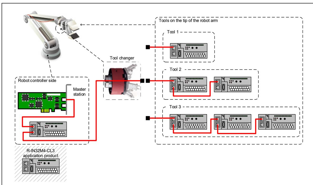
Figure 3.1 Example of Fast Linkup Usage (for an Industrial Robot Arm)
