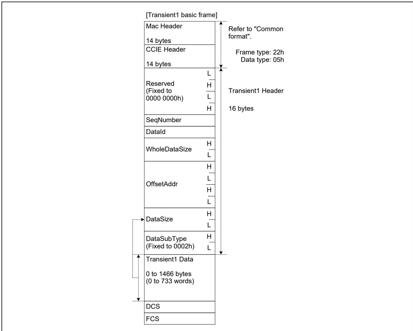
Figure 7.2 Overview of Transient1 Frame Basic Format
