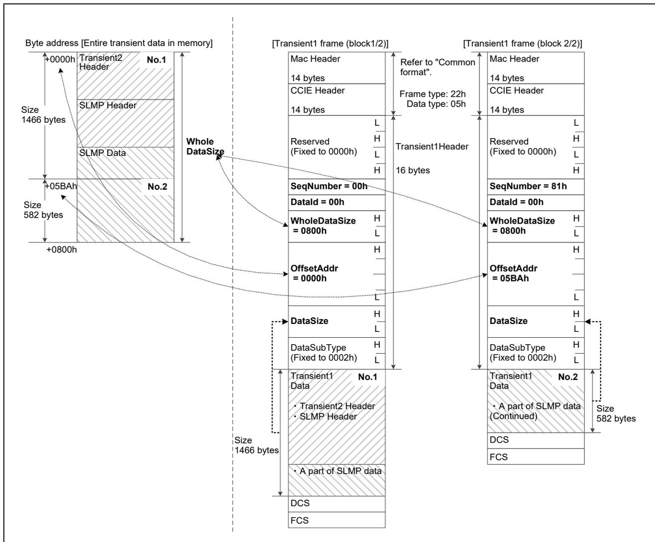
Figure 7.3 Example of Transient1 Frame Division
