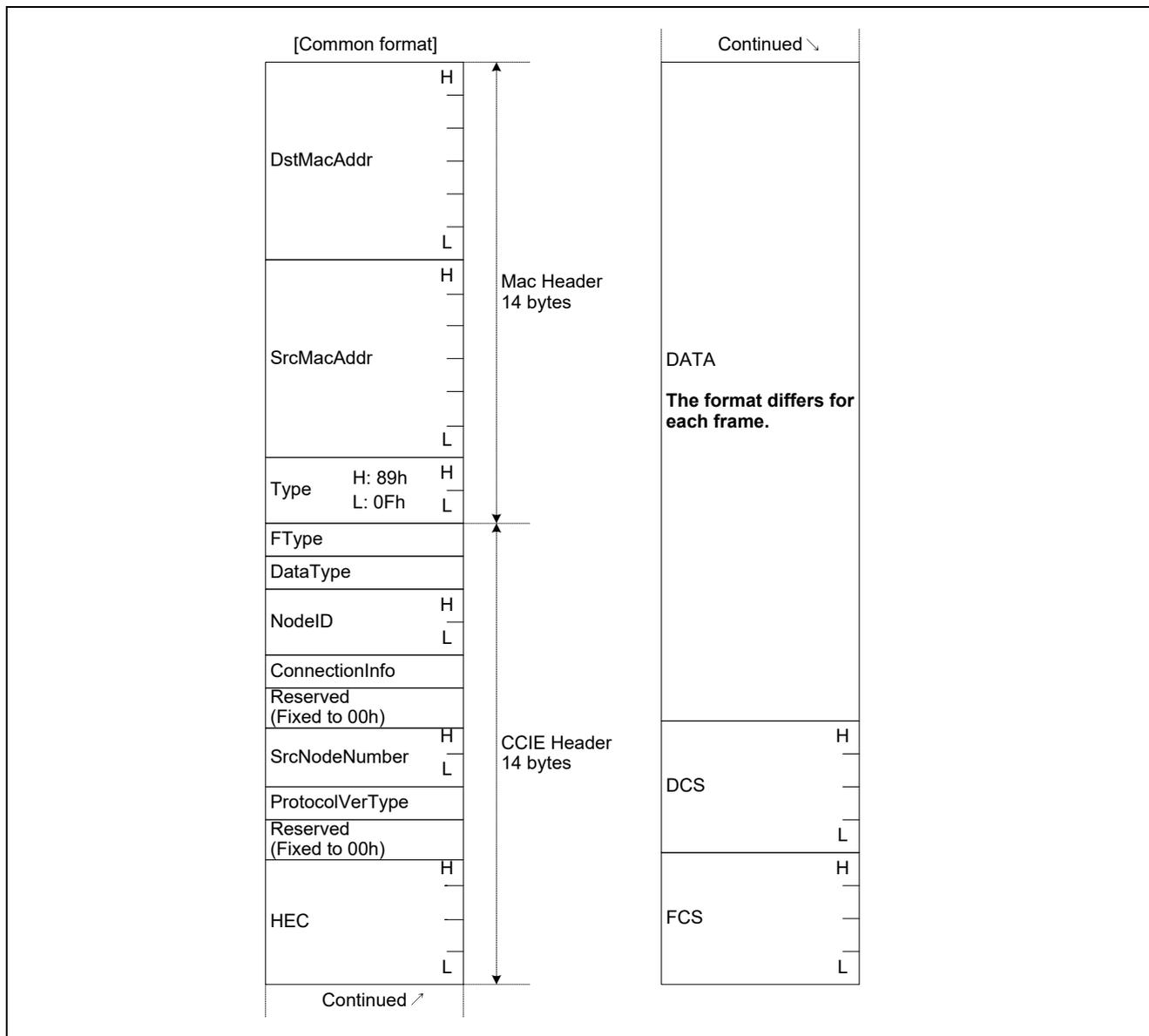
Figure 7.1 Overview of Frame Common Format
