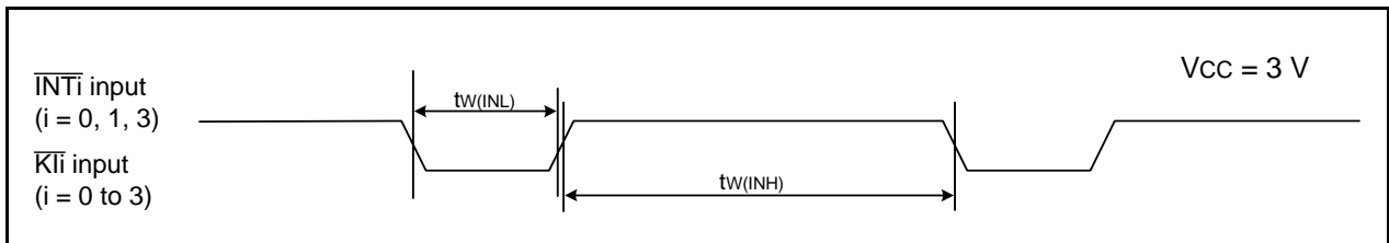
Figure 33.15 Input Timing for External Interrupt \overline{INTi} and Key Input Interrupt \overline{Kli} when Vcc = 3 V
