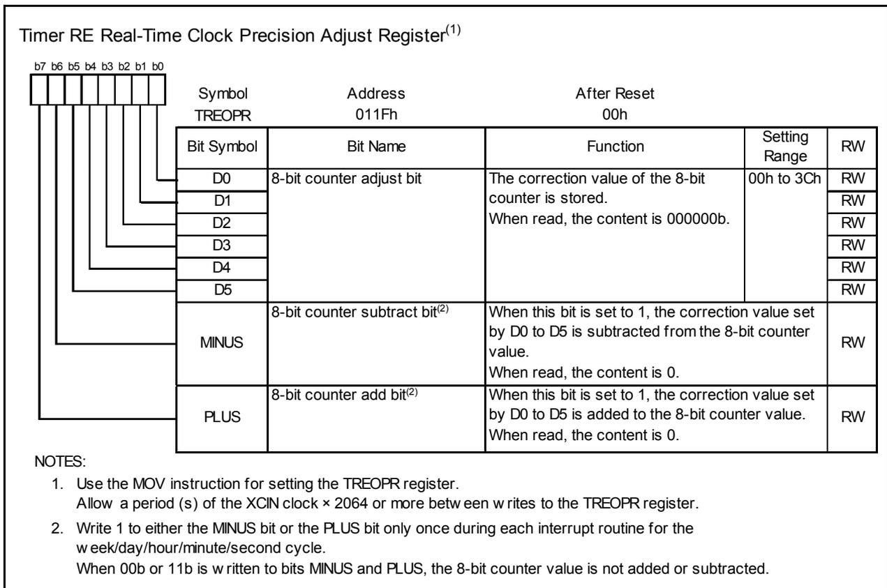
Figure 17.35 TREOPR Register in Real-Time Clock Mode
