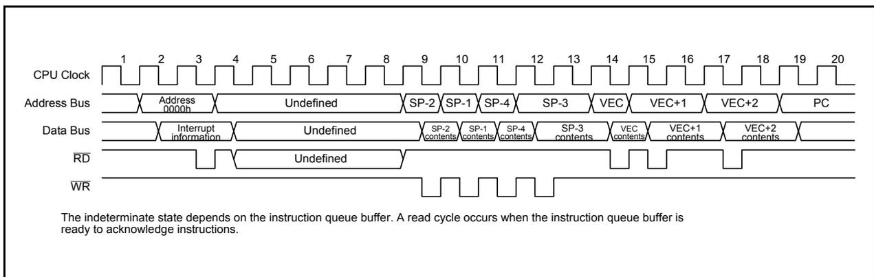
**Figure 13.5 Time Required for Executing Interrupt Sequence**
