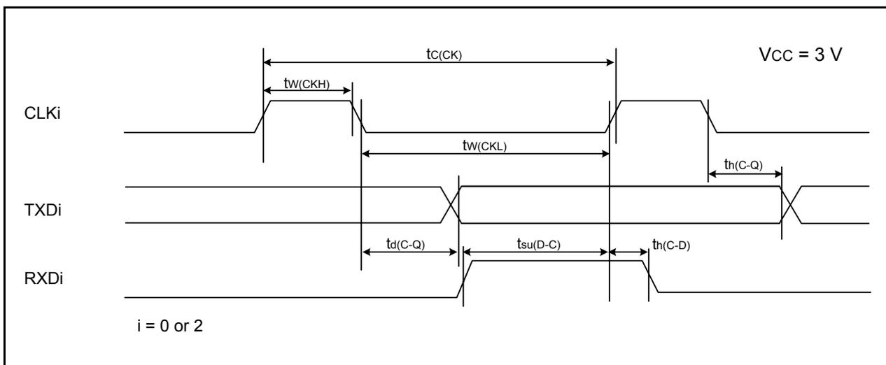
**Figure 22.9 Serial Interface Timing Diagram when Vcc = 3 V**
