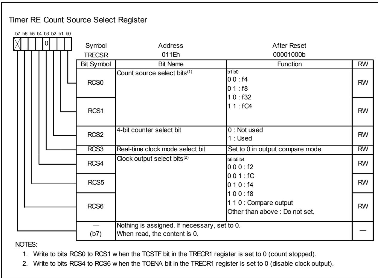
Figure 17.42 TRECSR Register in Output Compare Mode
