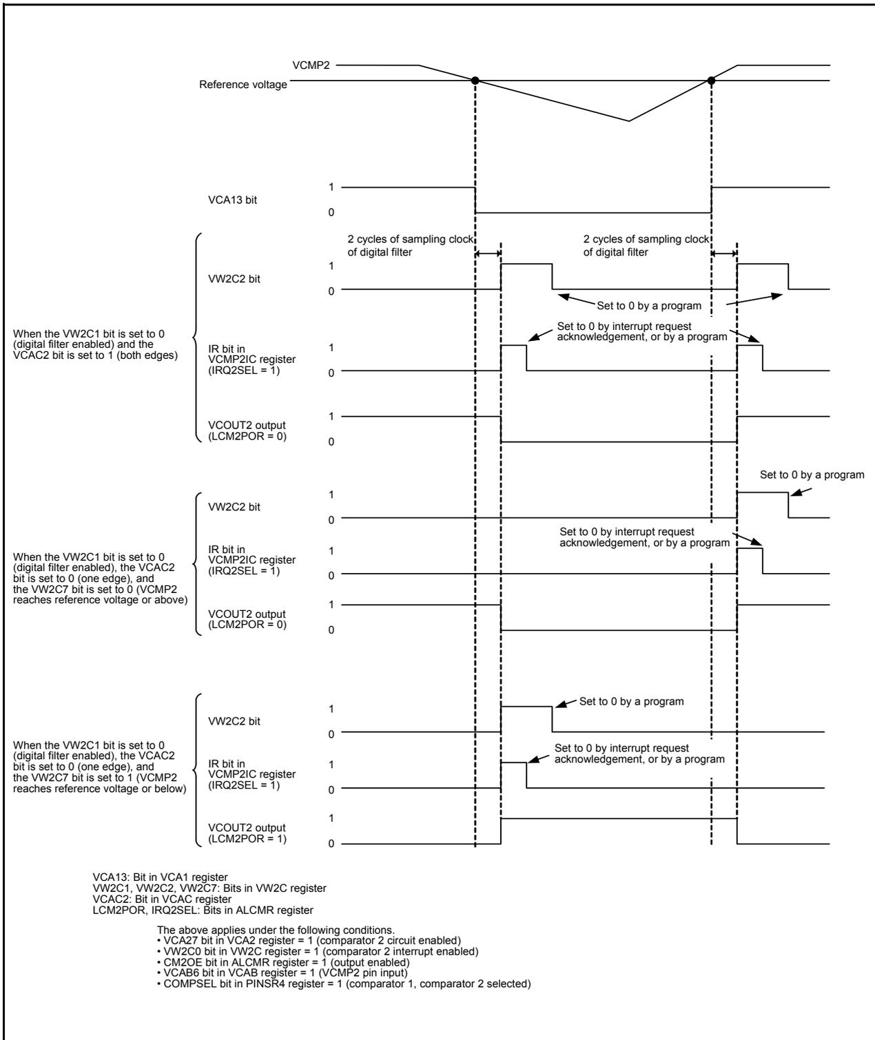
Figure 7.14 Operating Example of Comparator 2 (When Digital Filter Enabled)
