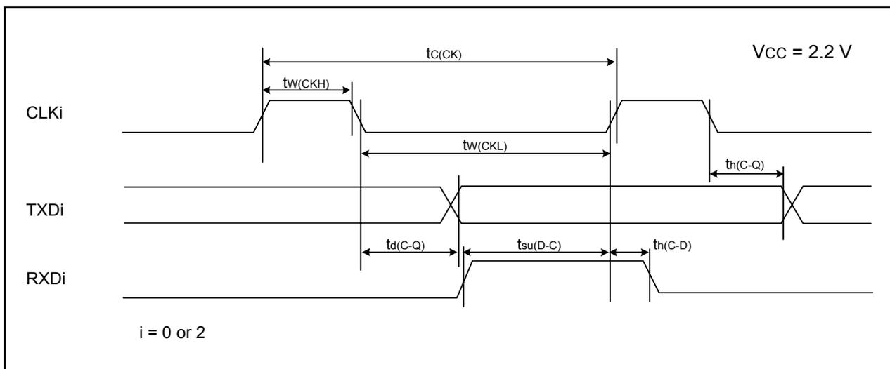
**Figure 22.13 Serial Interface Timing Diagram when  $V_{cc} = 2.2$  V**
