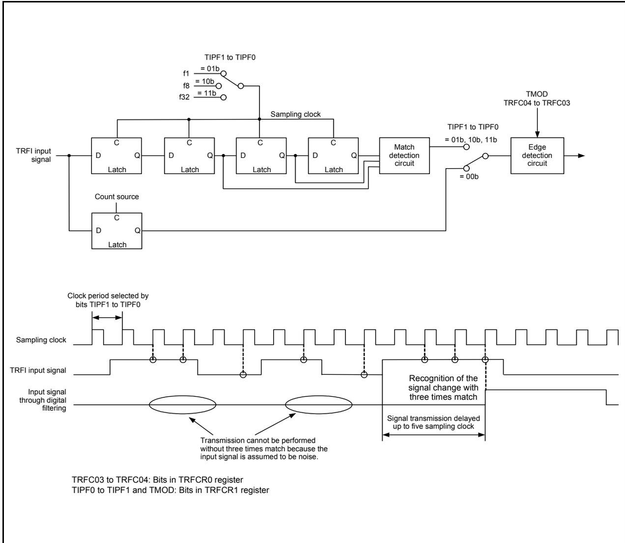
Figure 17.53 Block Diagram of Digital Filter
