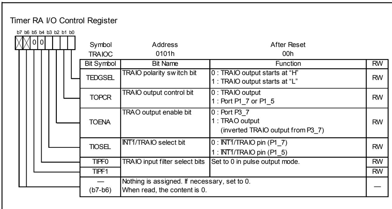
Figure 17.6 TRAIOC Register in Pulse Output Mode
