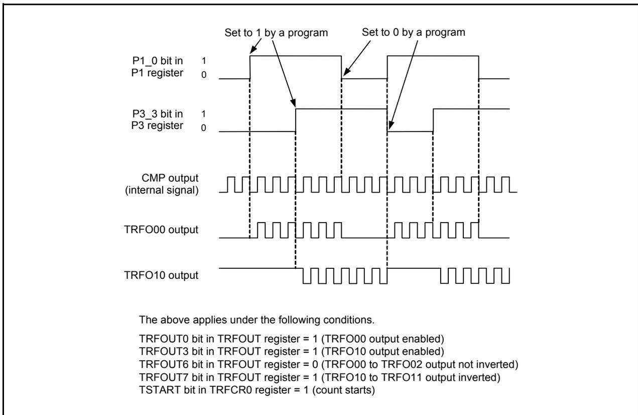
**Figure 17.55 Operating Example in Output Compare Mode (“L” and “H” Held Output in Count Stops)**
