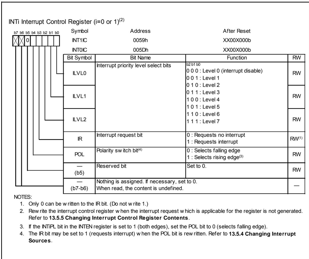
Figure 13.4 INT<sub>i</sub>IC Register (i = 0 or 1)
