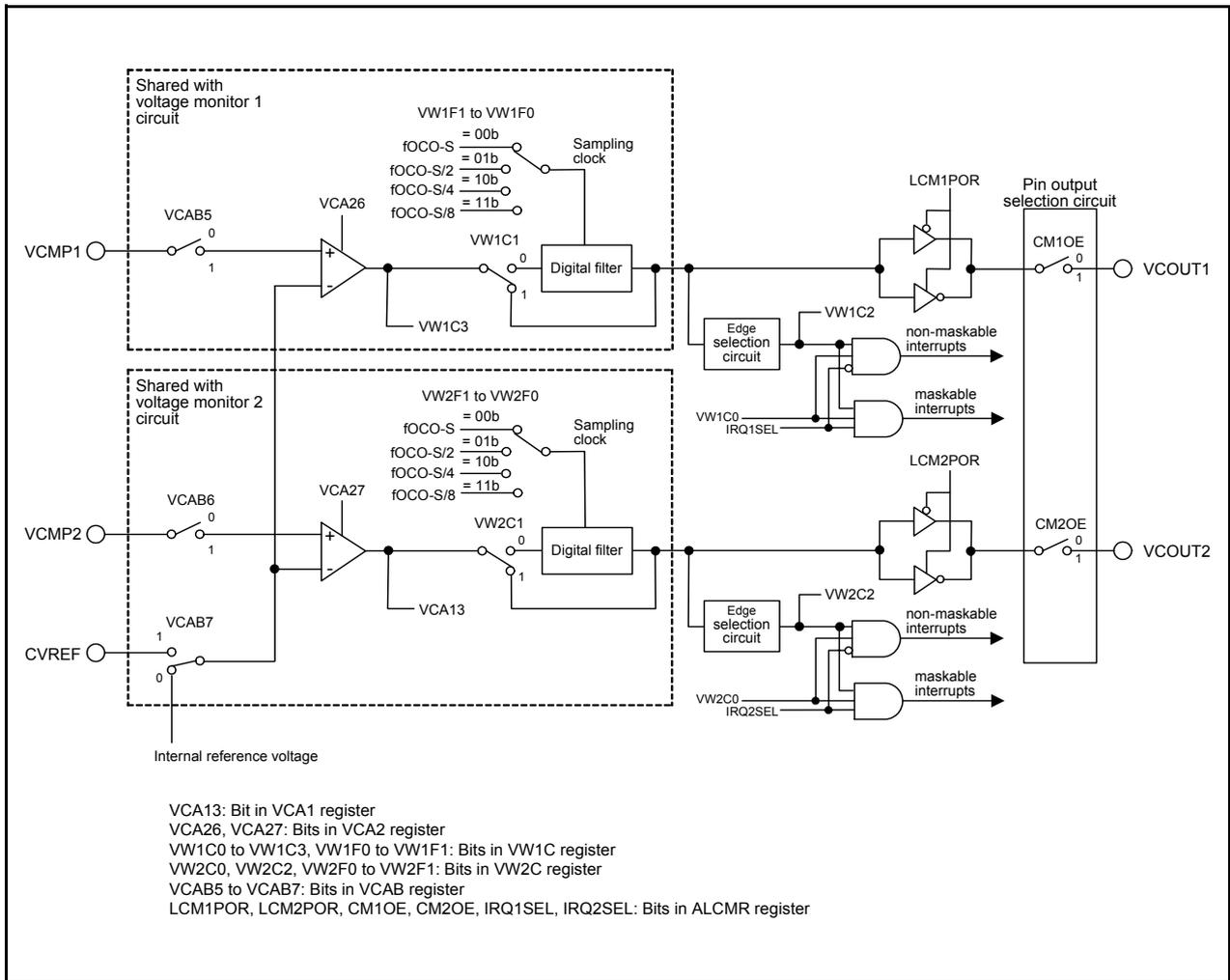
Figure 7.1 Block Diagram of Comparator
