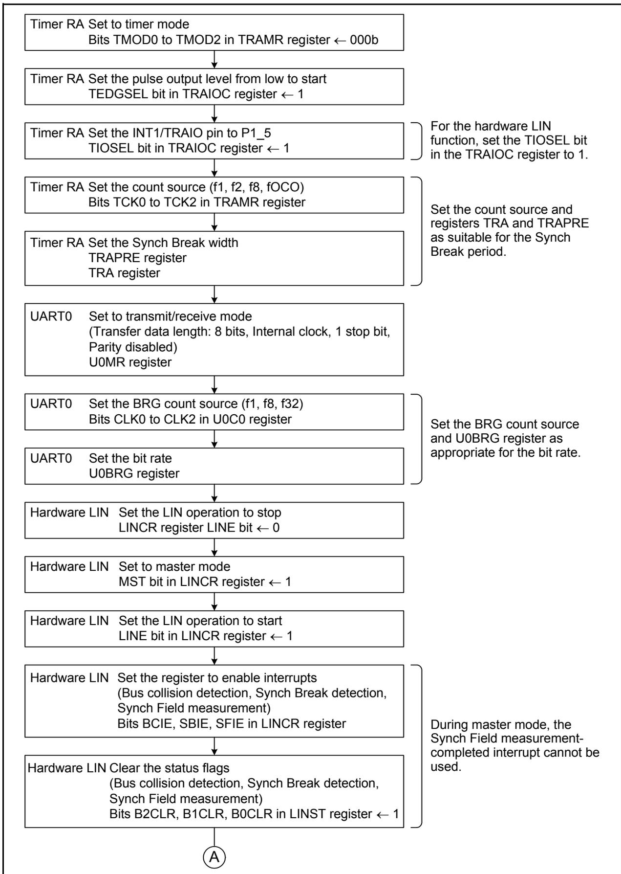
Figure 19.5 Example of Header Field Transmission Flowchart (1)
