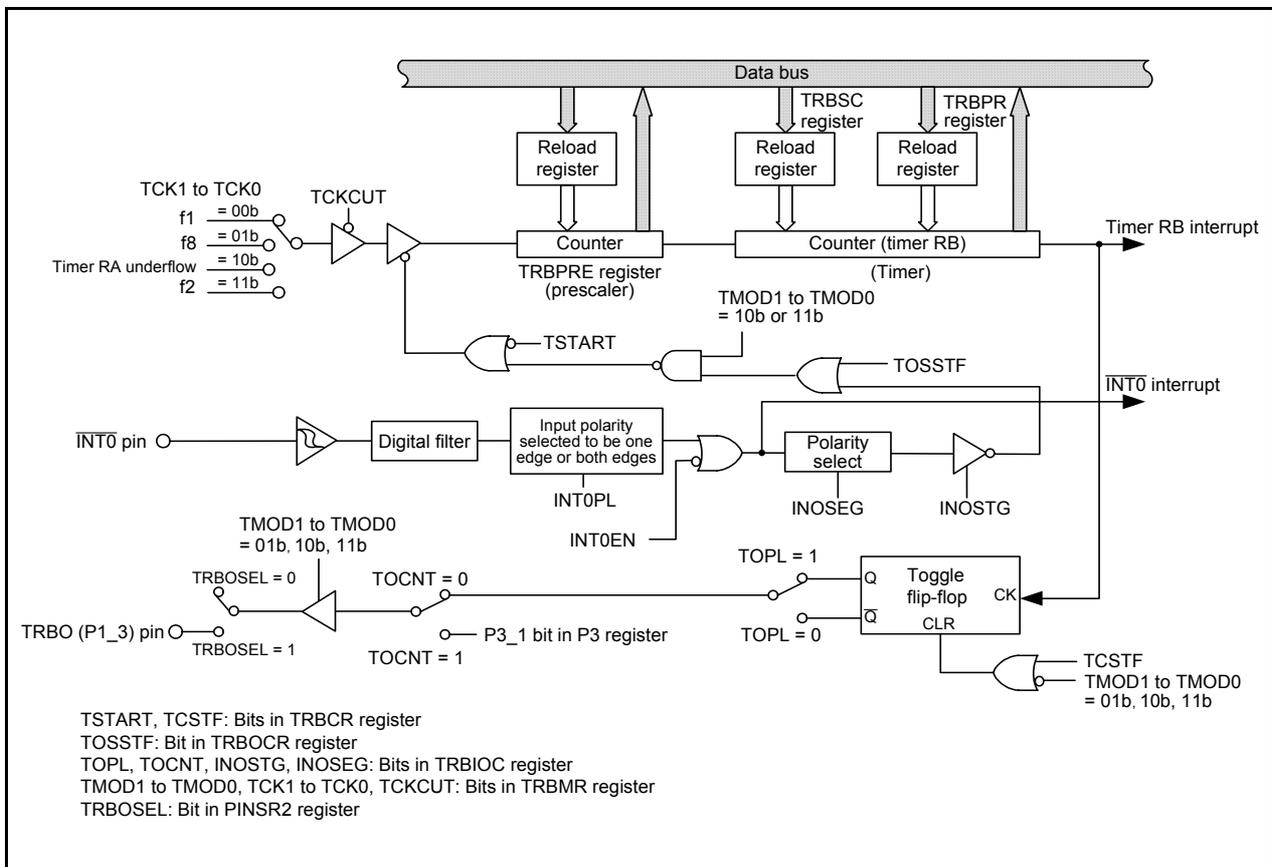
Figure 17.12 Block Diagram of Timer RB
