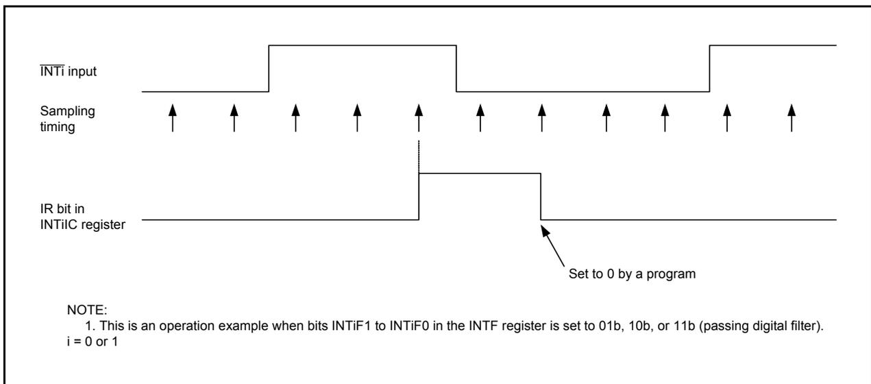
Figure 13.14 Operating Example of  $\text{INT}_i$  Input Filter
