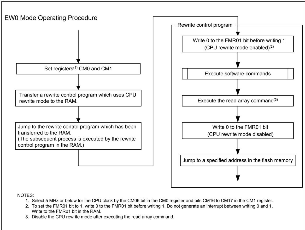
**Figure 20.7 How to Set and Exit EW0 Mode**
