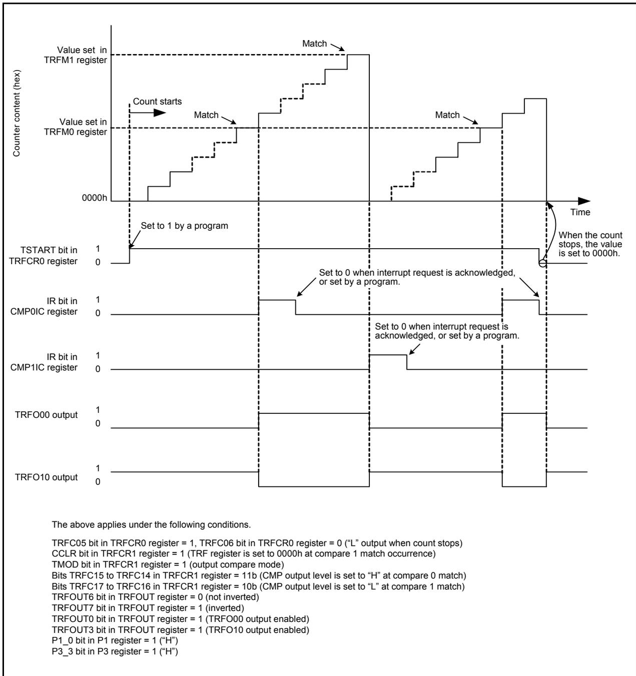
**Figure 17.54** Operating Example in Output Compare Mode
