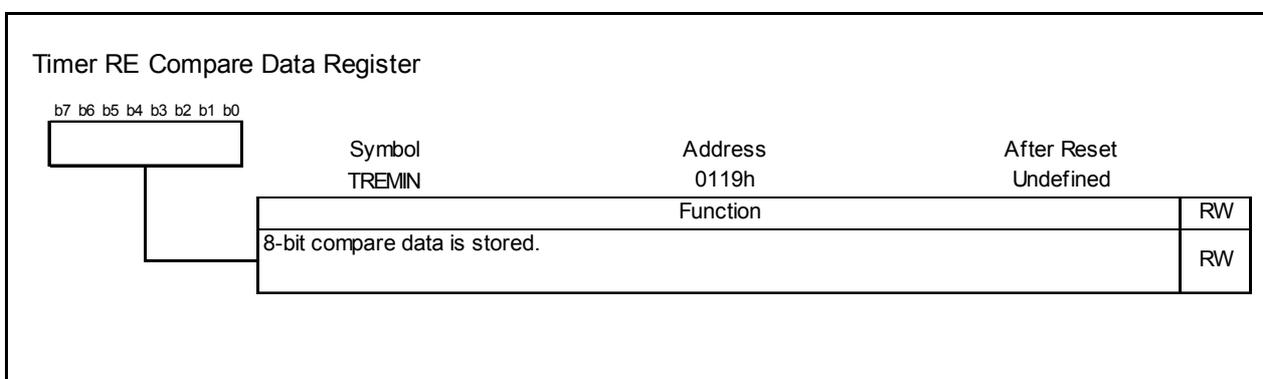
Figure 17.39 TREMINT Register in Output Compare Mode
