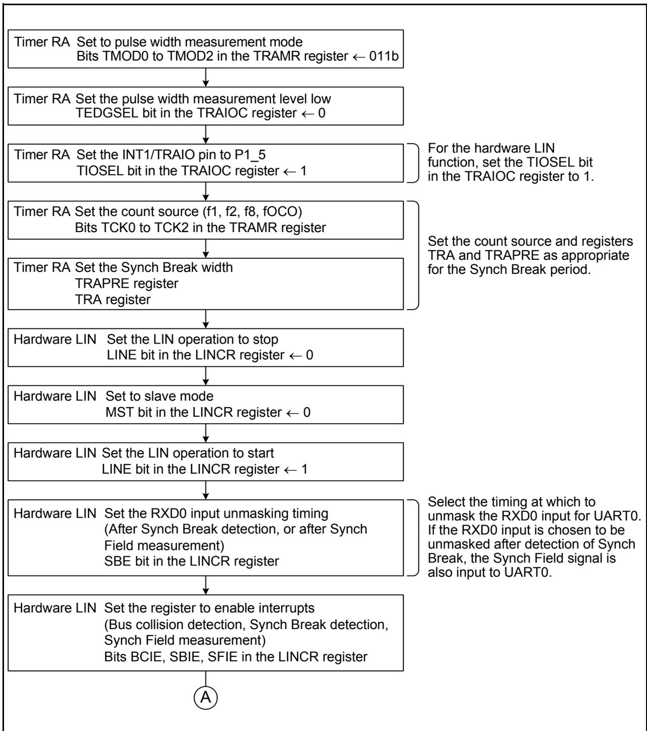
Figure 19.8 Example of Header Field Reception Flowchart (1)
