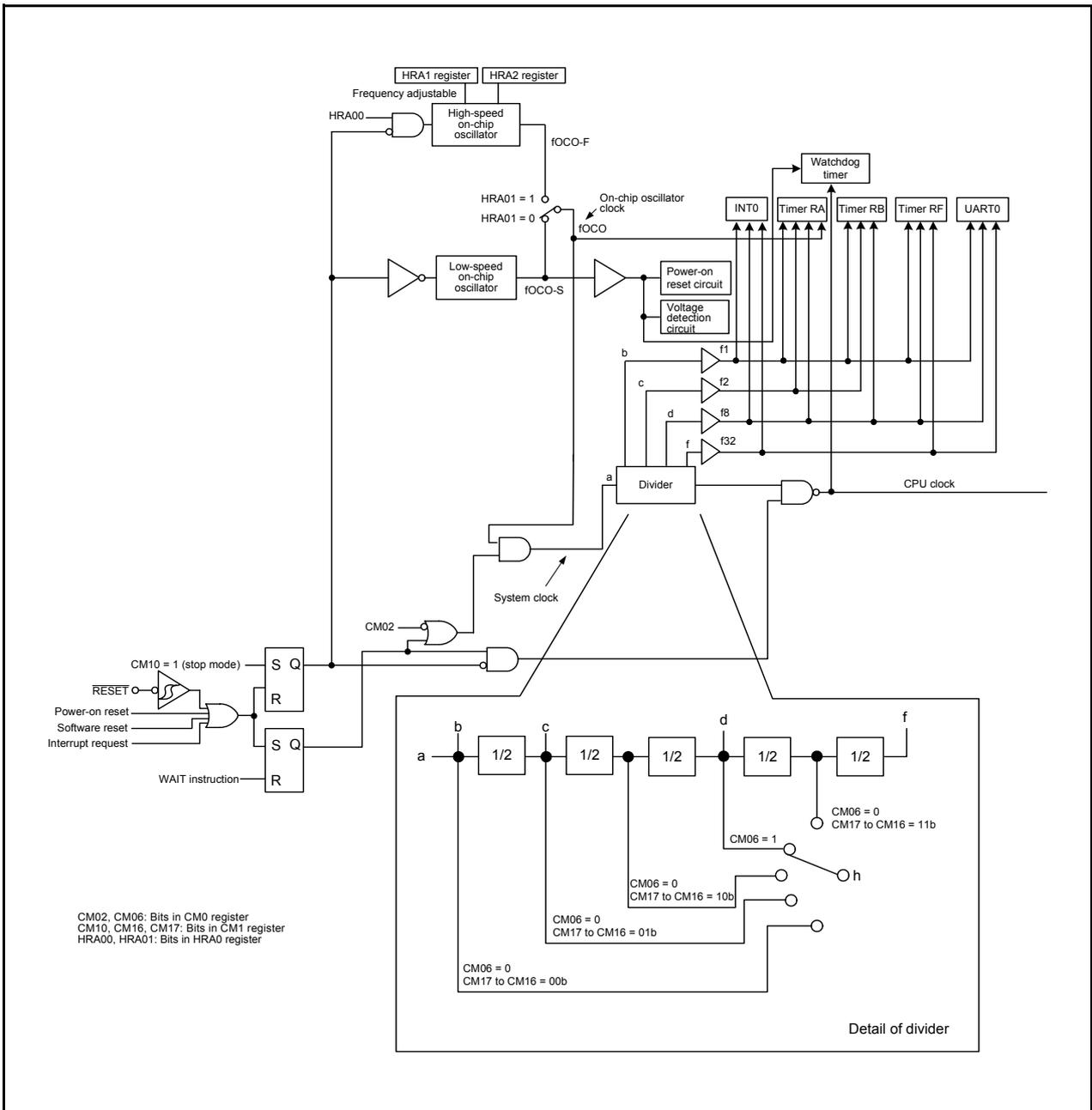
Figure 11.2 Clock Generation Circuit for R8C/2J Group
