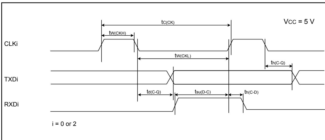
**Figure 22.5 Serial Interface Timing Diagram when Vcc = 5 V**
