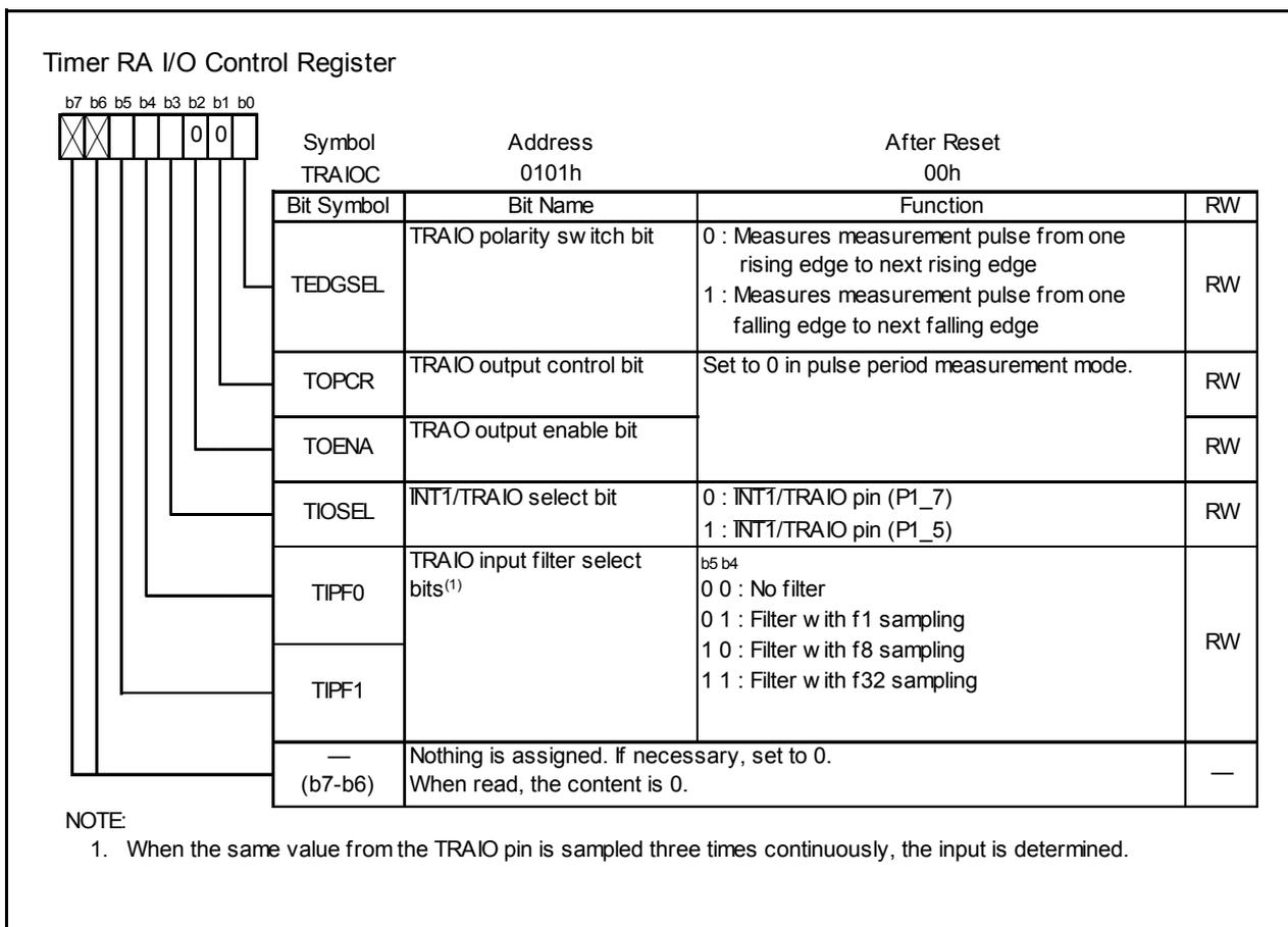
Figure 17.10 TRAI OC Register in Pulse Period Measurement Mode
