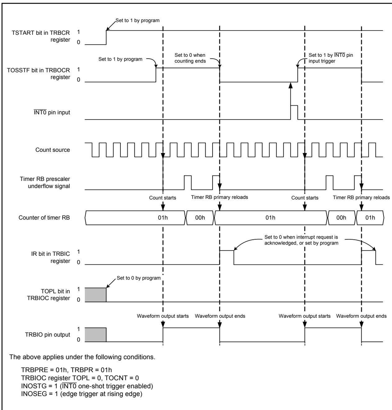
Figure 17.21 Operating Example of Programmable One-Shot Generation Mode
