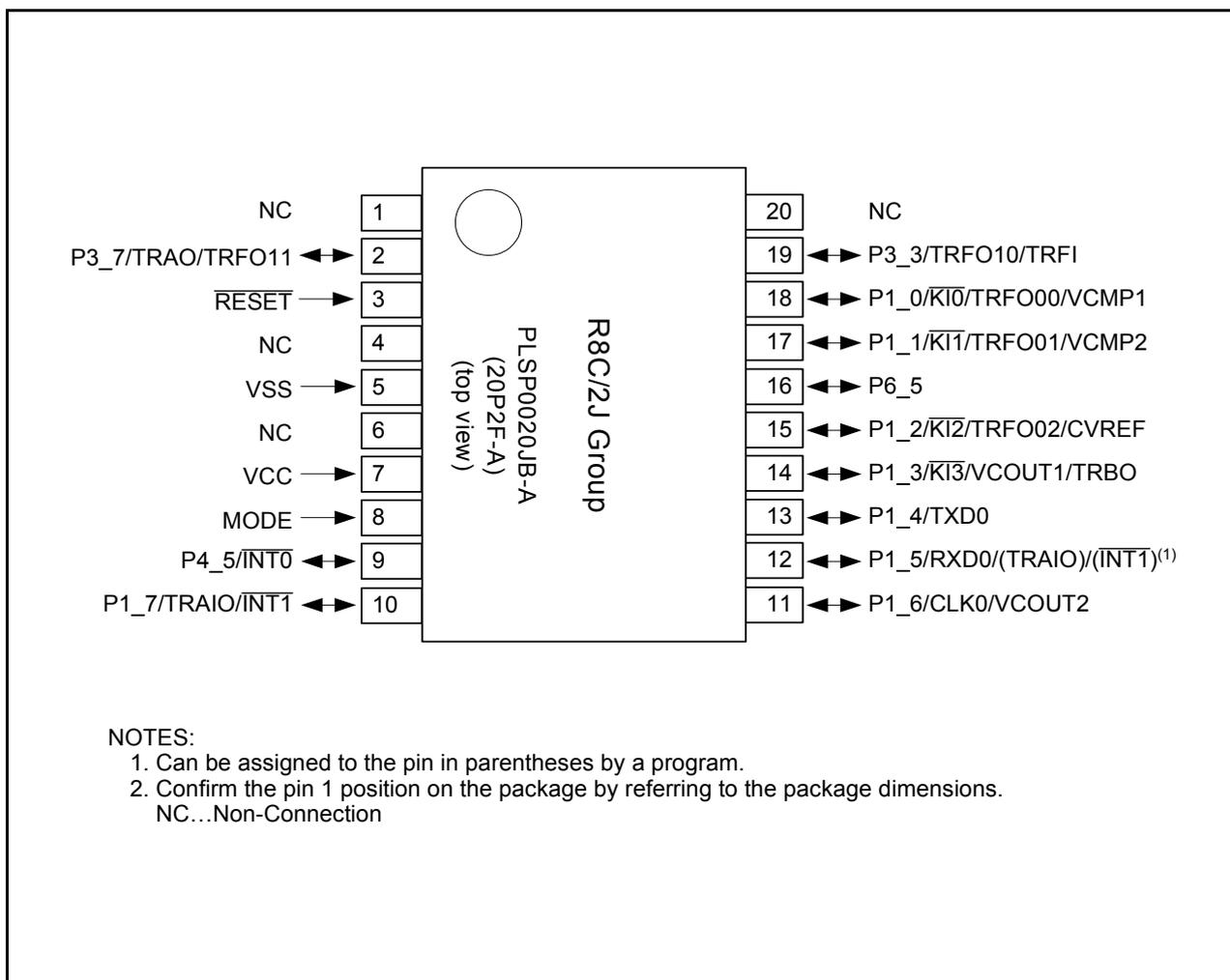
Figure 1.6 Pin Assignment (Top View) of R8C/2J Group
