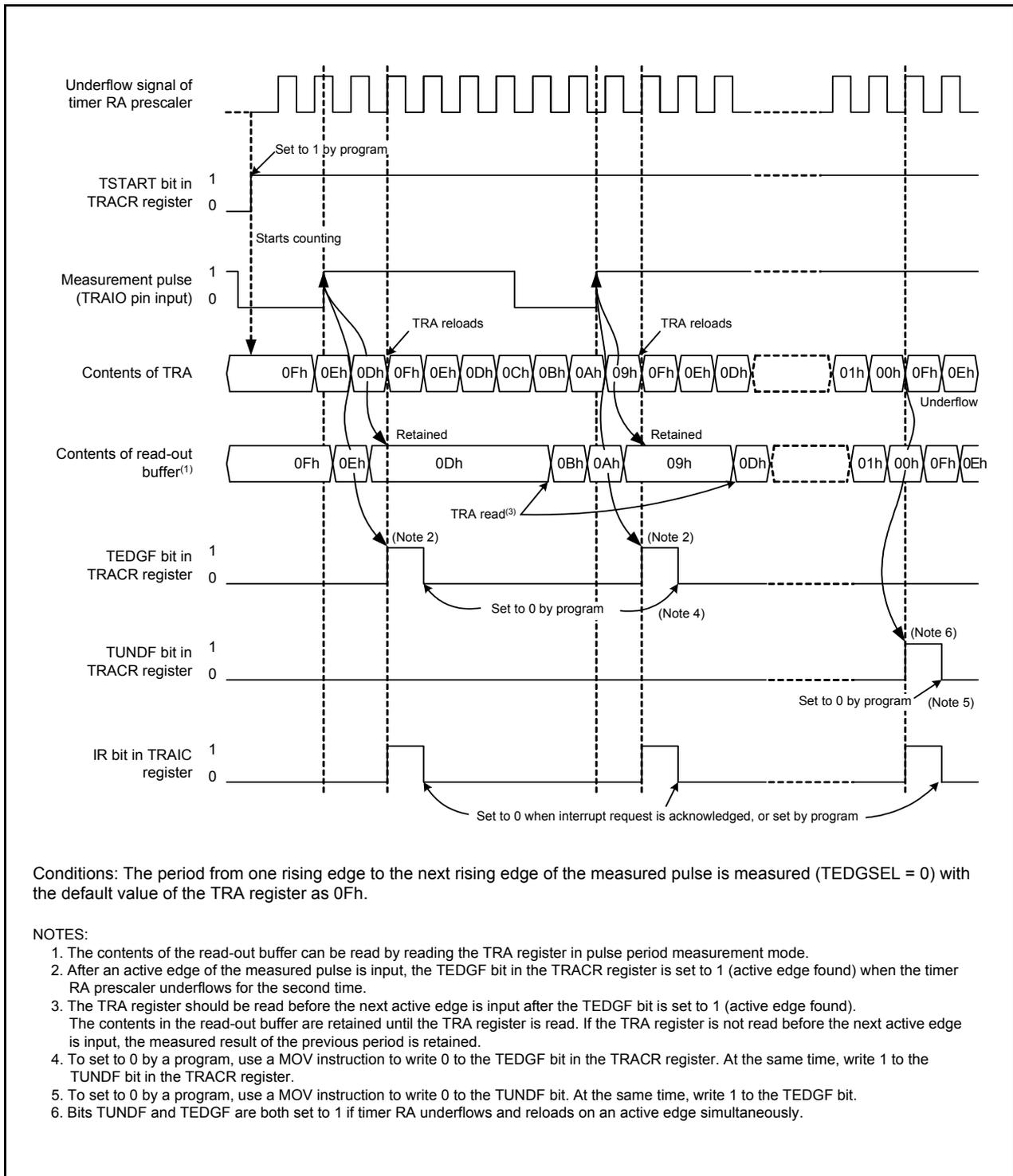
Figure 17.11 Operating Example of Pulse Period Measurement Mode
