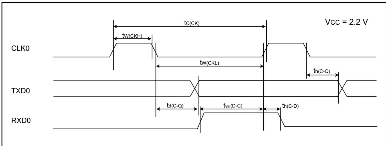
**Figure 22.24 Serial Interface Timing Diagram when Vcc = 2.2 V****Table 22.55 External Interrupt  $\overline{INTi}$  ( $i = 0$  or  $1$ ) Input**
