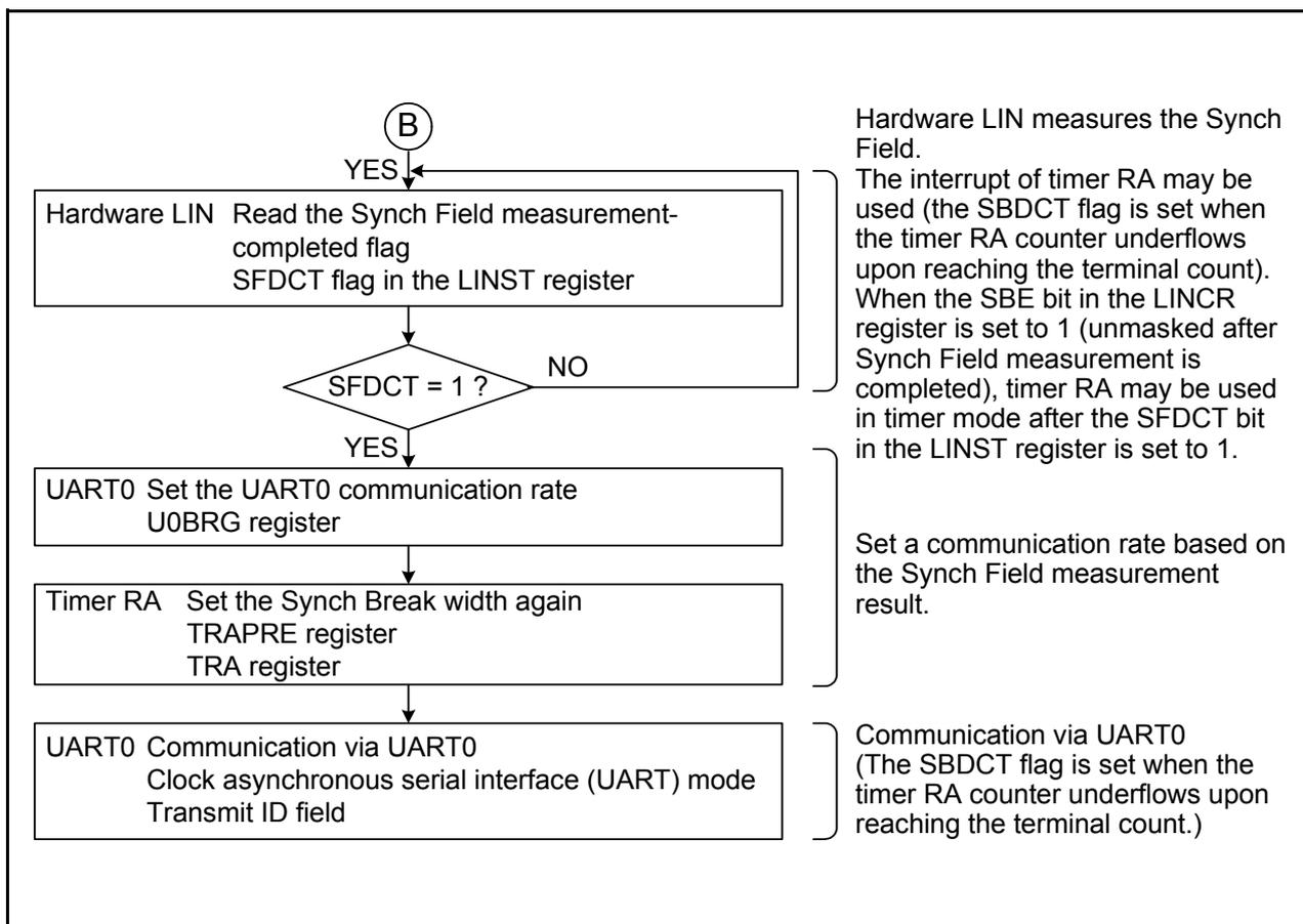
Figure 19.10 Example of Header Field Reception Flowchart (3)
