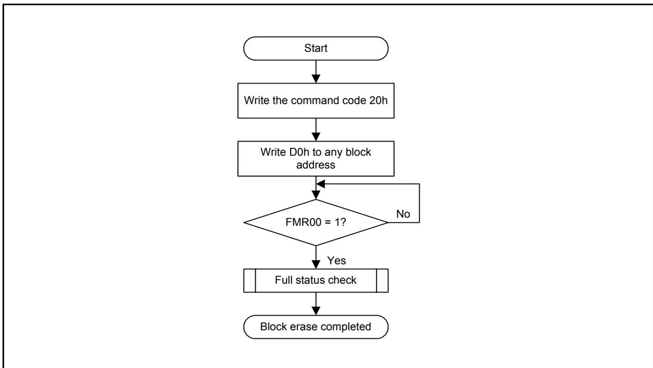
**Figure 20.11** Block Erase Command in EW0 Mode
