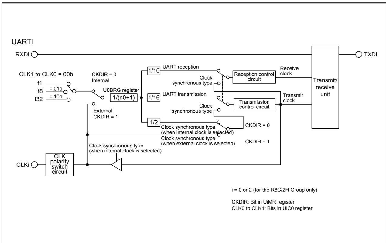
Figure 18.1 UART<sub>i</sub> (i = 0 or 2 (for R8C/2H Group only)) Block Diagram
