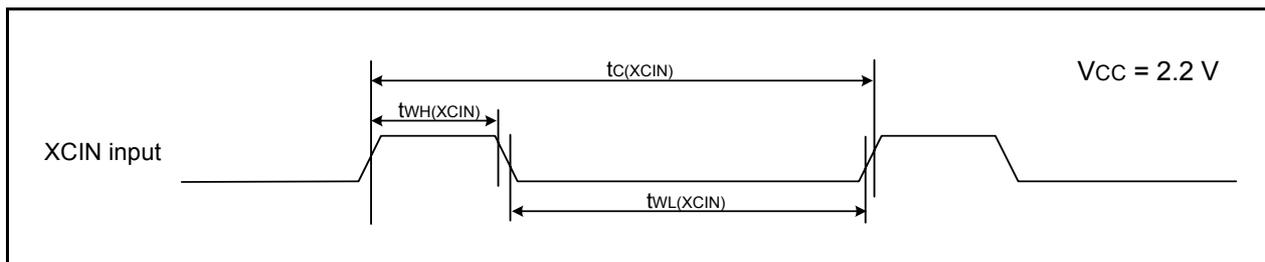
**Figure 22.11 XCIN Input Timing Diagram when  $V_{CC} = 2.2\text{ V}$** **Table 22.27 TRAI0 Input**
