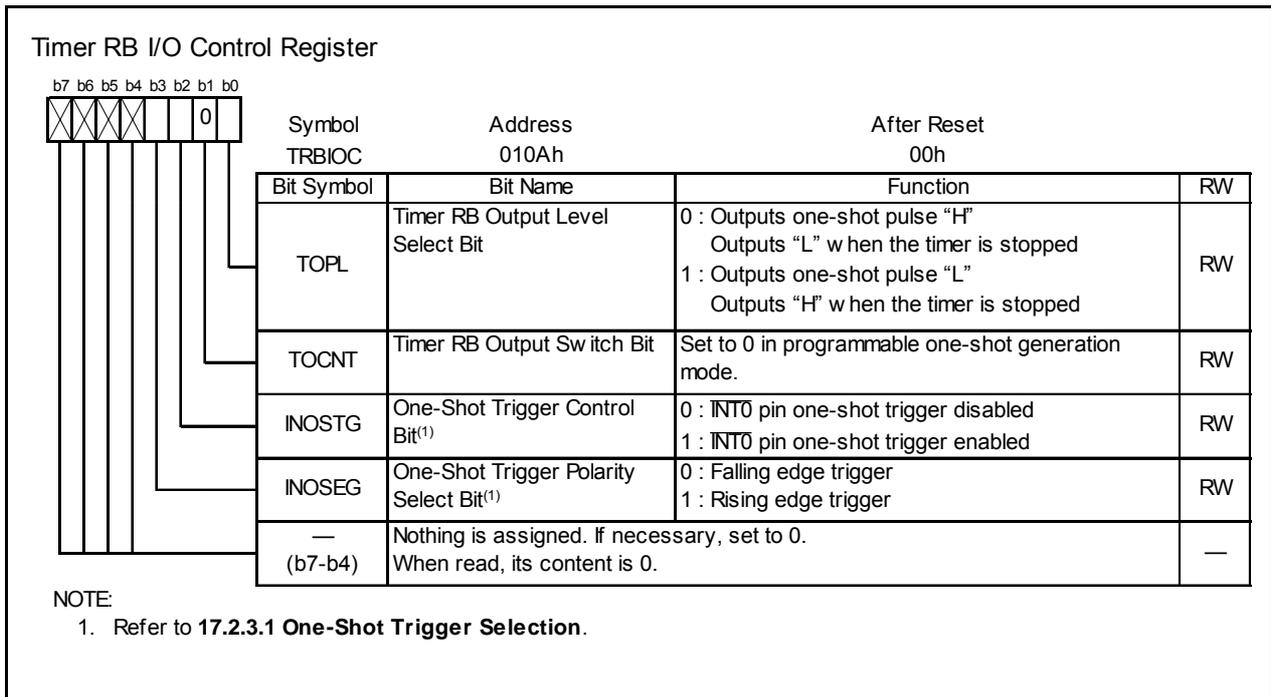
Figure 17.20 TRBIOC Register in Programmable One-Shot Generation Mode
