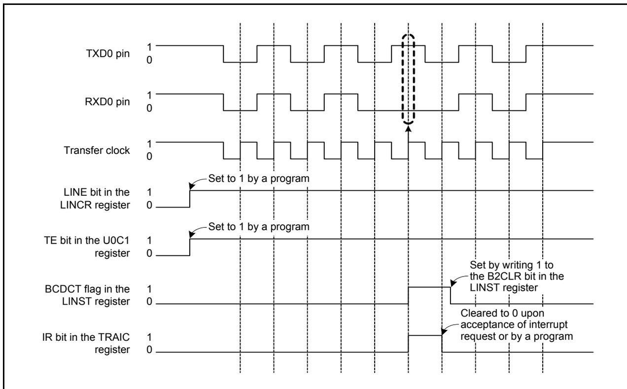
Figure 19.11 Typical Operation when a Bus Collision is Detected
