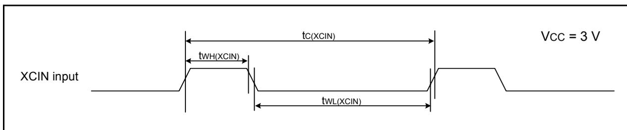
**Figure 22.7 XCIN Input Timing Diagram when  $V_{CC} = 3\text{ V}$** **Table 22.21 TRAI0 Input**
