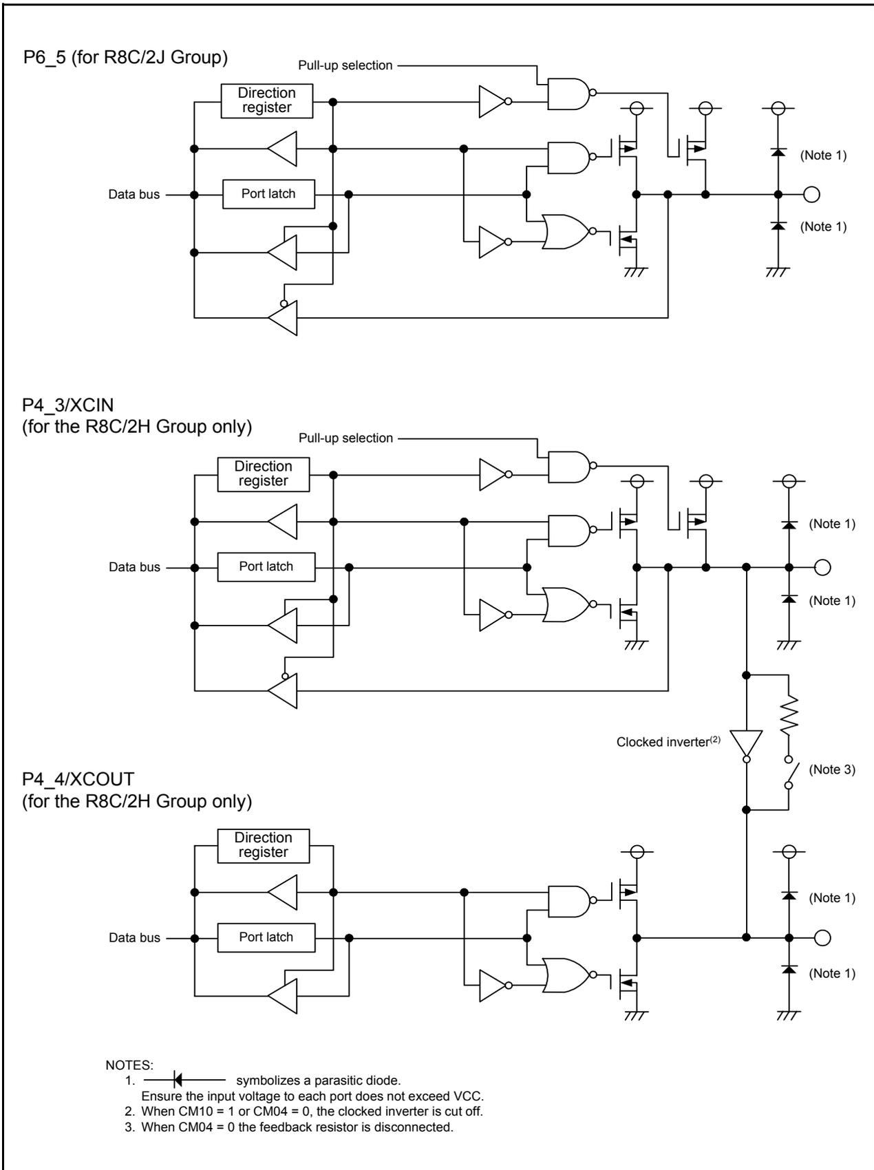
Figure 8.3 Configuration of I/O Ports (3)
