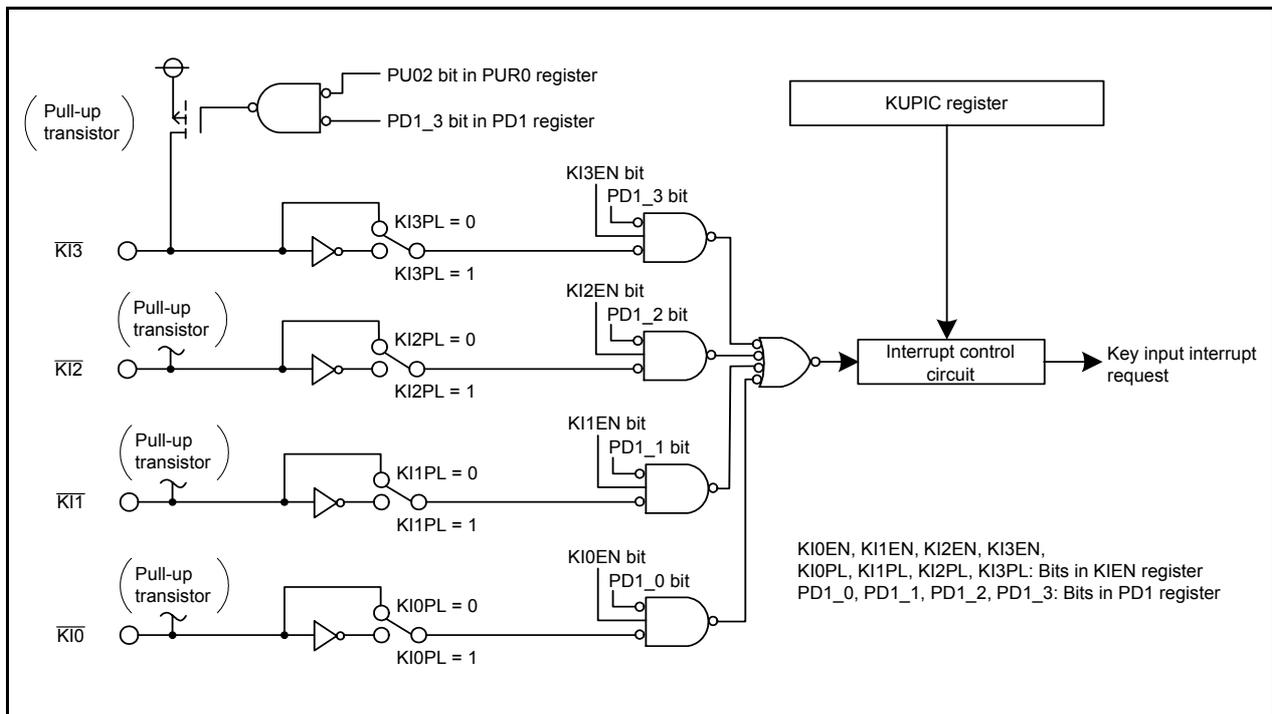
**Figure 13.15 Block Diagram of Key Input Interrupt**
