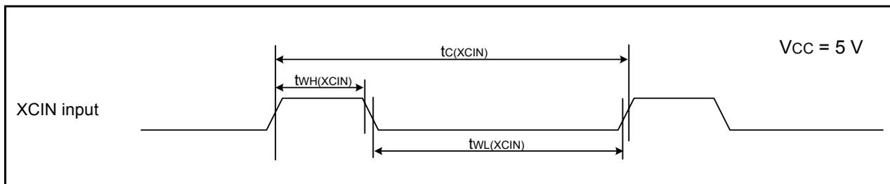
**Figure 22.3 XCIN Input Timing Diagram when  $V_{CC} = 5\text{ V}$** **Table 22.15 TRAI0 Input**
