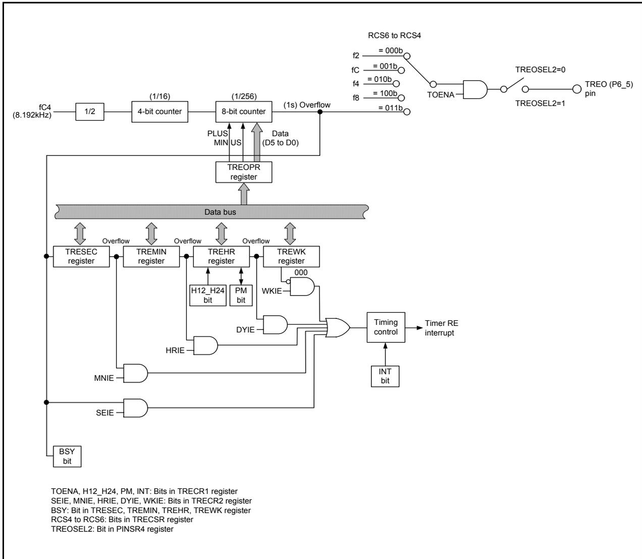
Figure 17.26 Block Diagram of Real-Time Clock Mode
