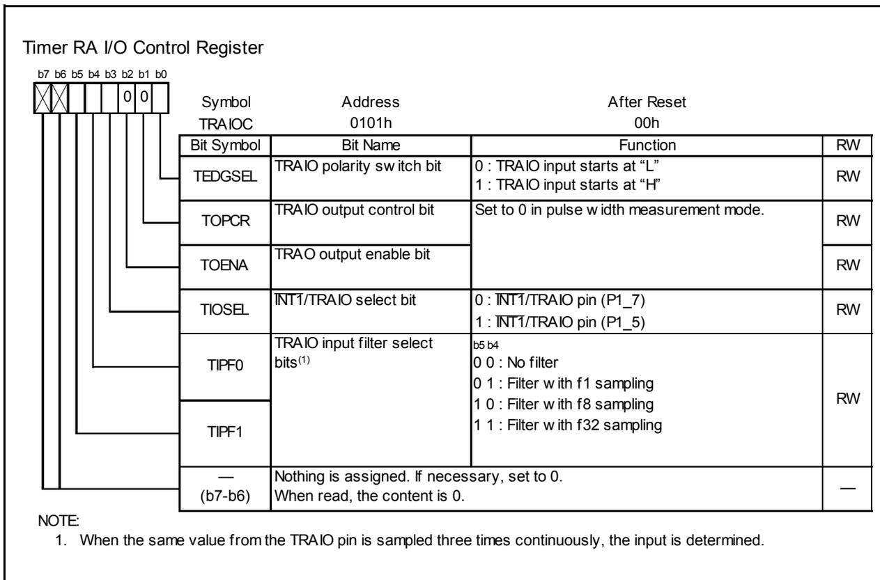
Figure 17.8 TRAI0C Register in Pulse Width Measurement Mode
