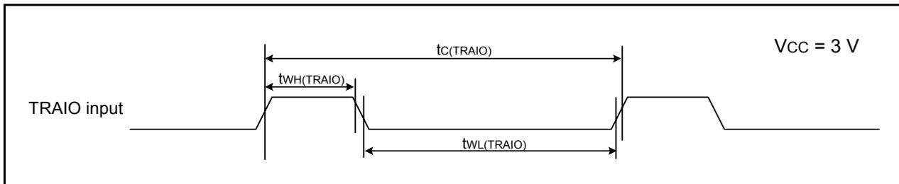
**Figure 22.20 TRAI0 Input Timing Diagram when VCC = 3 V**
