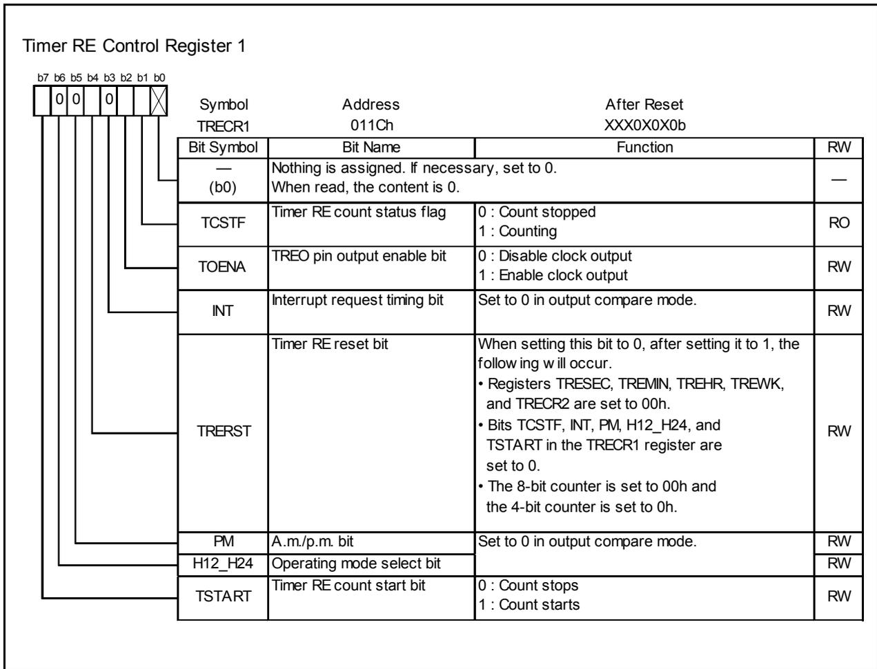
Figure 17.40 TREC1 Register in Output Compare Mode
