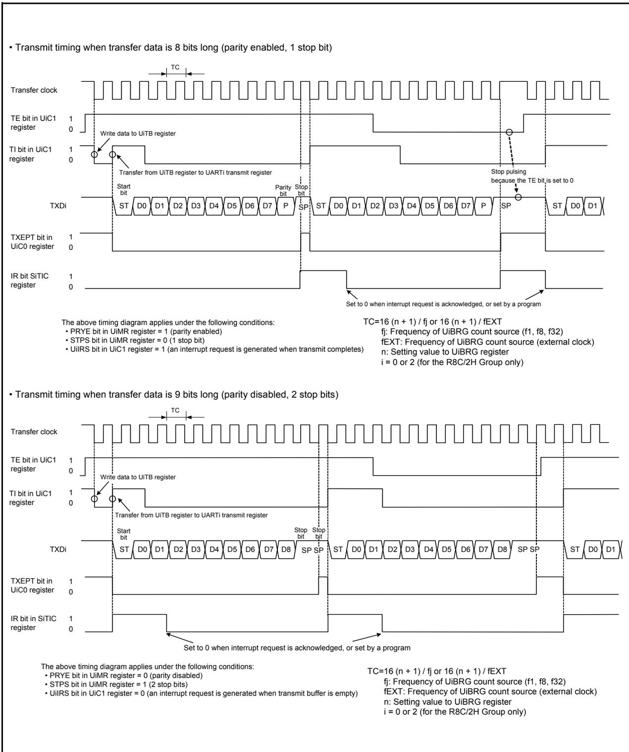
Figure 18.9 Transmit Timing in UART Mode
