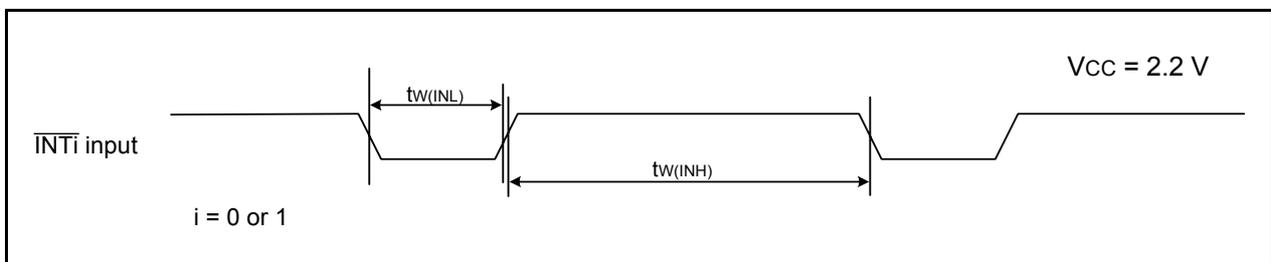
**Figure 22.25 External Interrupt  $\overline{INTi}$  Input Timing Diagram when Vcc = 2.2 V**
