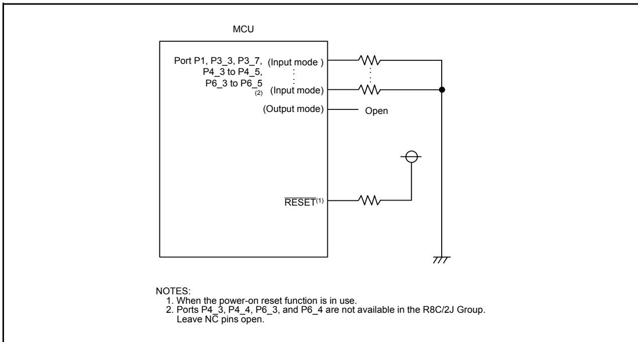
**Figure 8.12 Unassigned Pin Handling**
