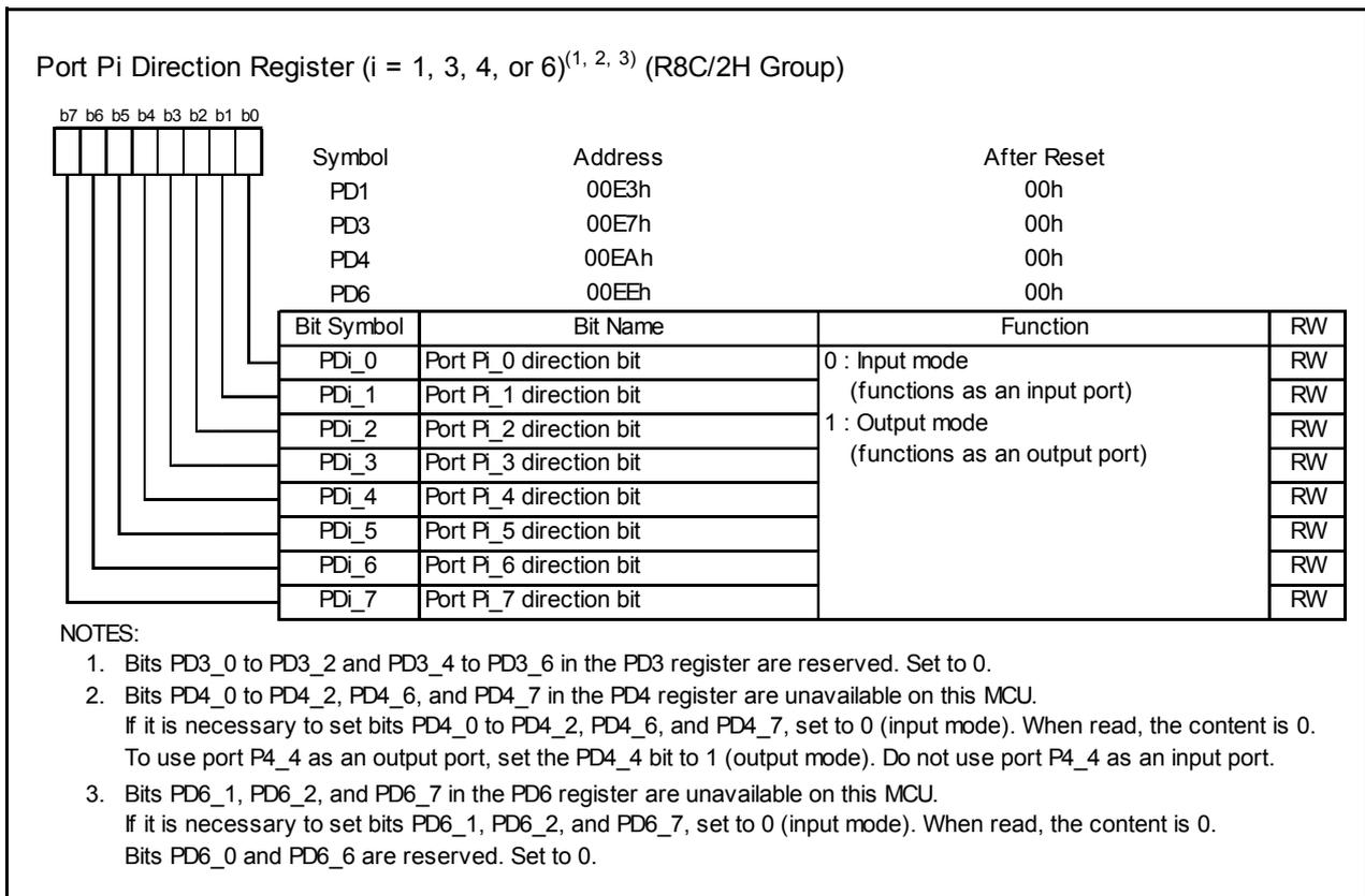
Figure 8.5 PDi ( $i = 1, 3, 4, \text{ or } 6$ ) Register (R8C/2H Group)
