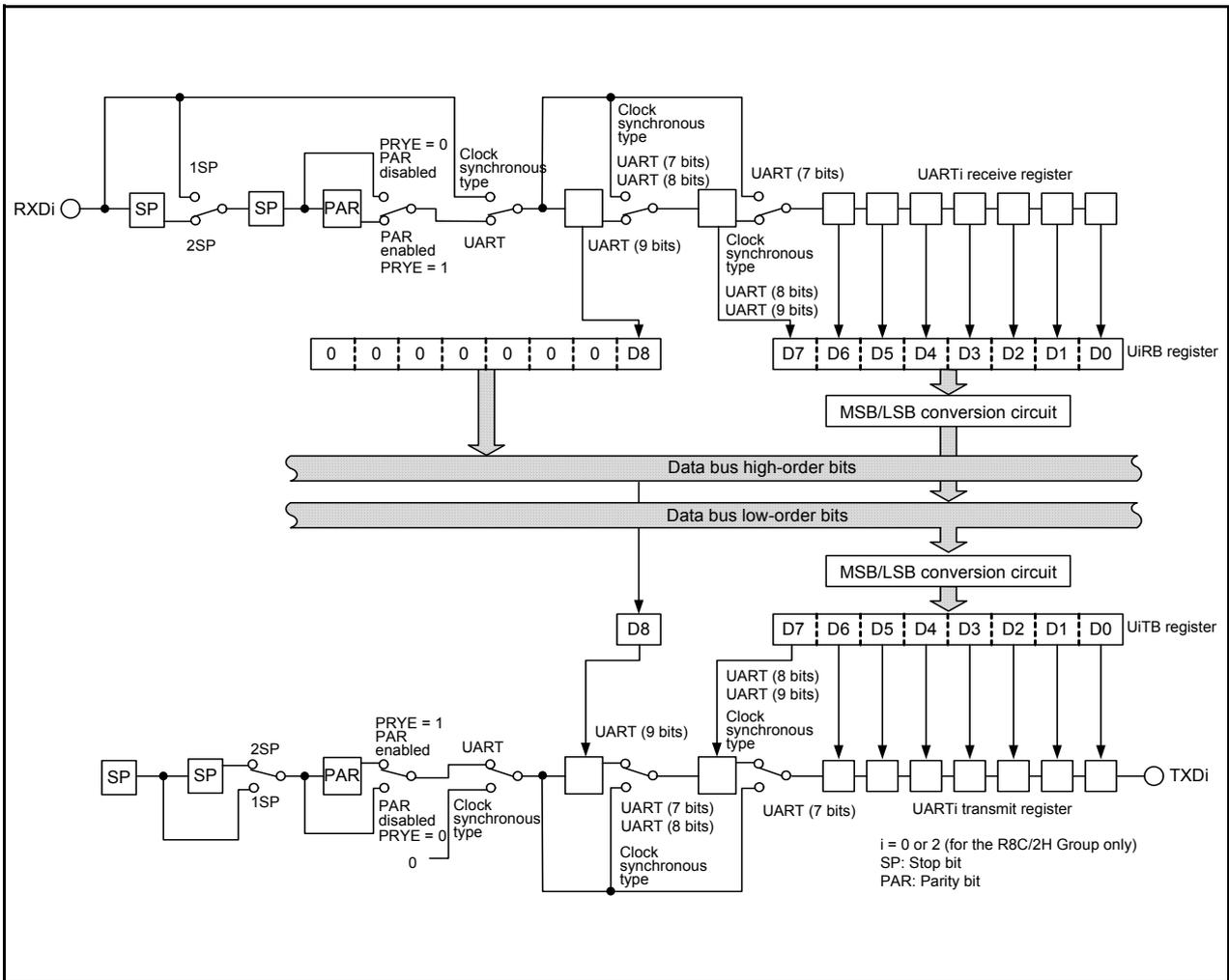
Figure 18.2 UARTi Transmit/Receive Unit
