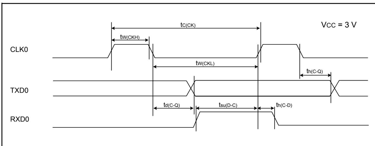
**Figure 22.21 Serial Interface Timing Diagram when Vcc = 3 V**
