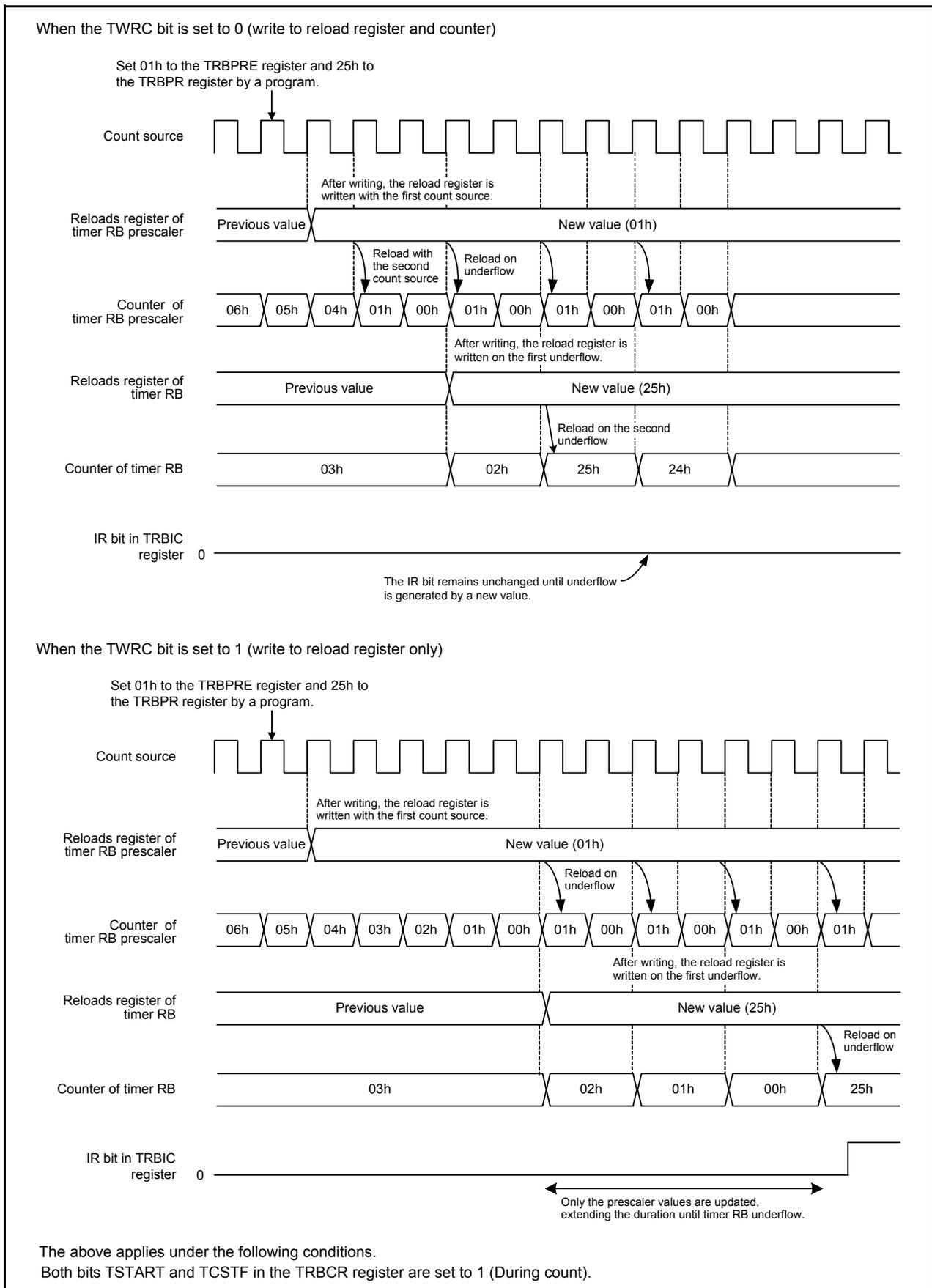
**Figure 17.17 Operating Example of Timer RB when Counter Value is Rewritten during Count Operation**
