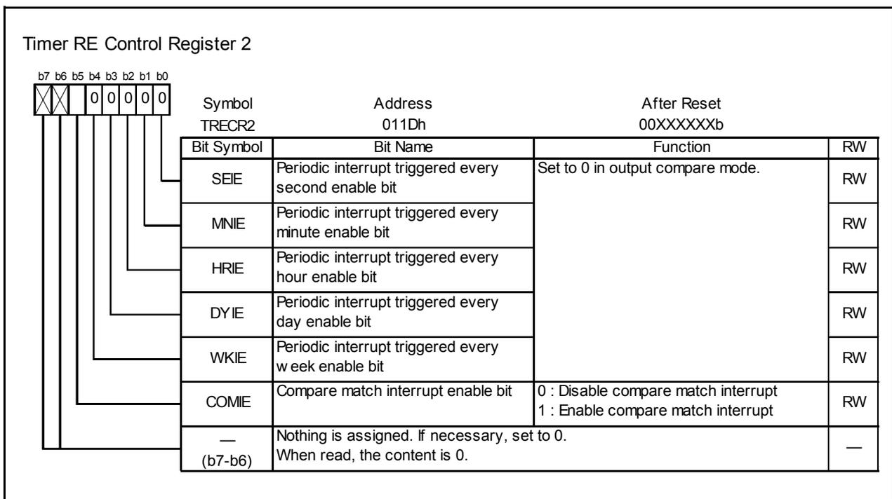
Figure 17.41 TREC2 Register in Output Compare Mode
