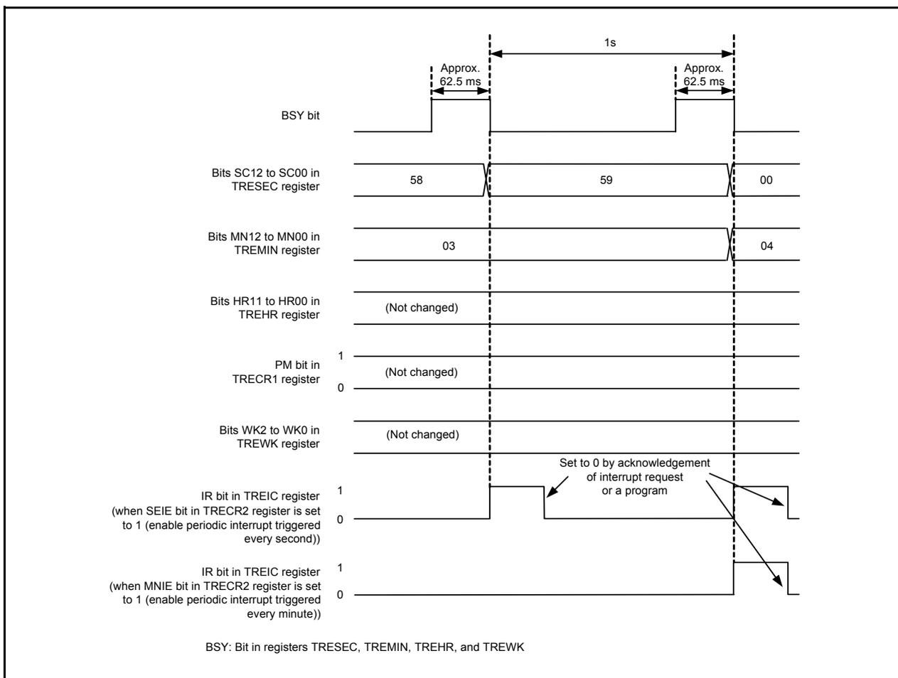
Figure 17.36 Operating Example in Real-Time Clock Mode
