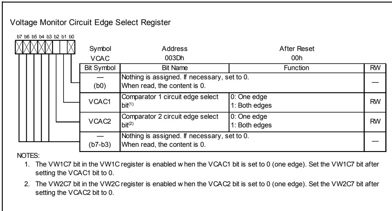
**Figure 7.8 VCAC Register**
