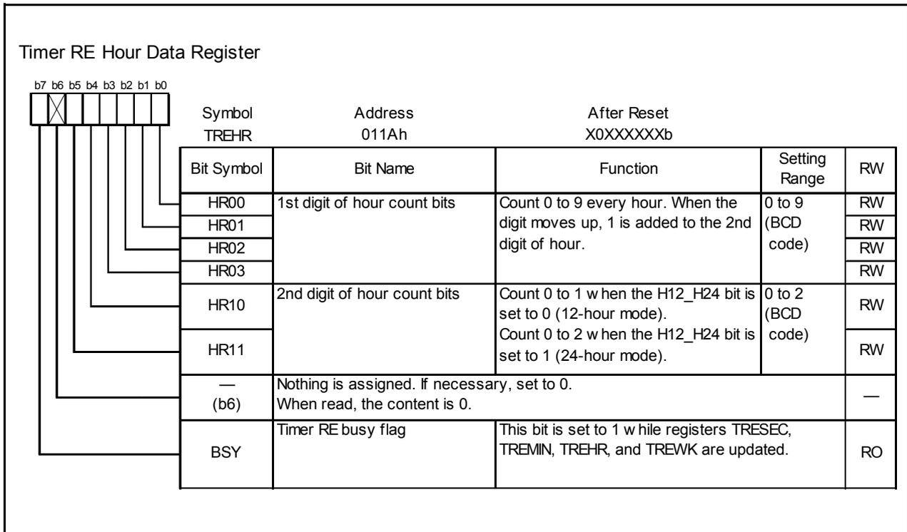
Figure 17.29 TREHR Register in Real-Time Clock Mode
