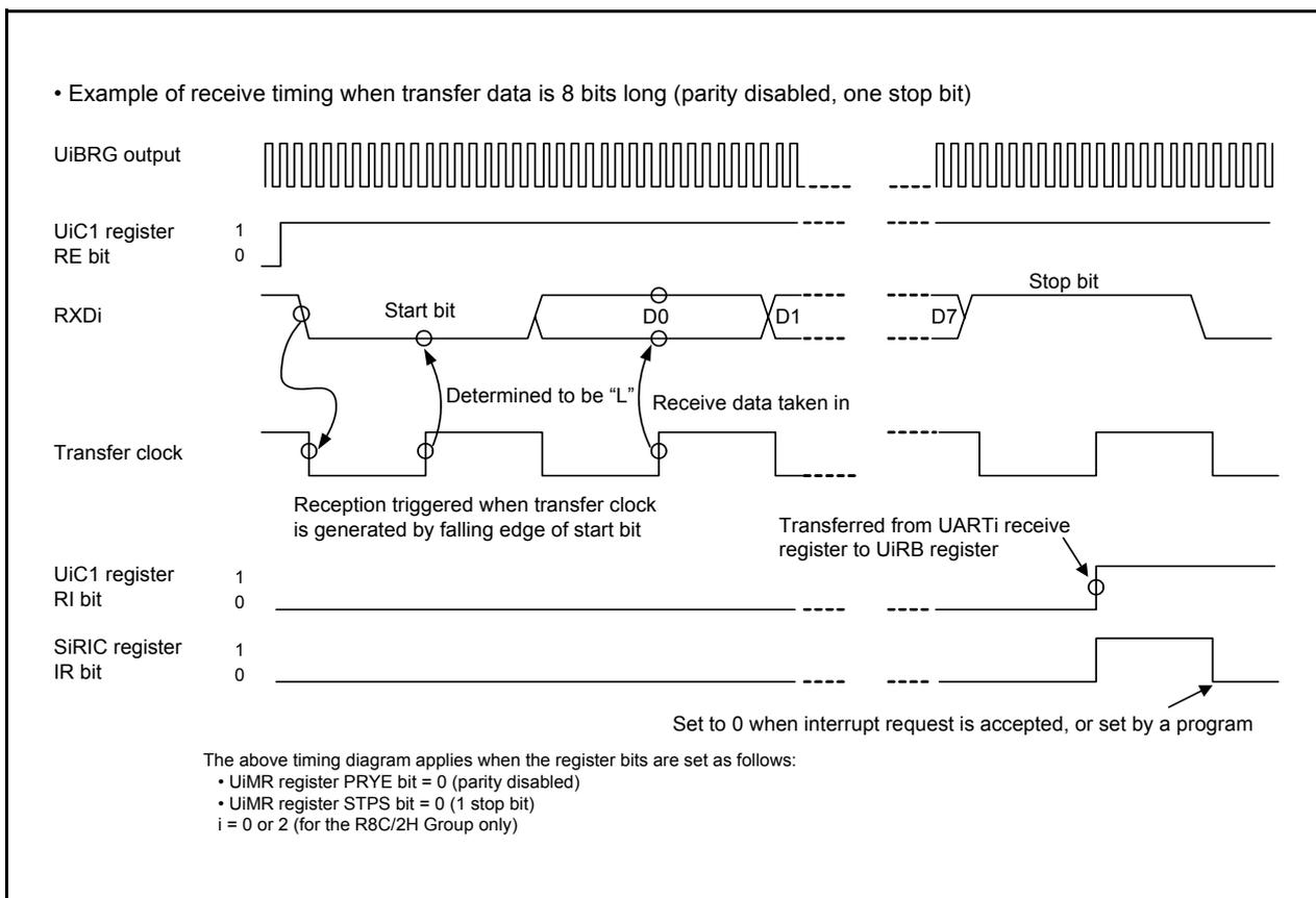
Figure 18.10 Receive Timing Example in UART Mode
