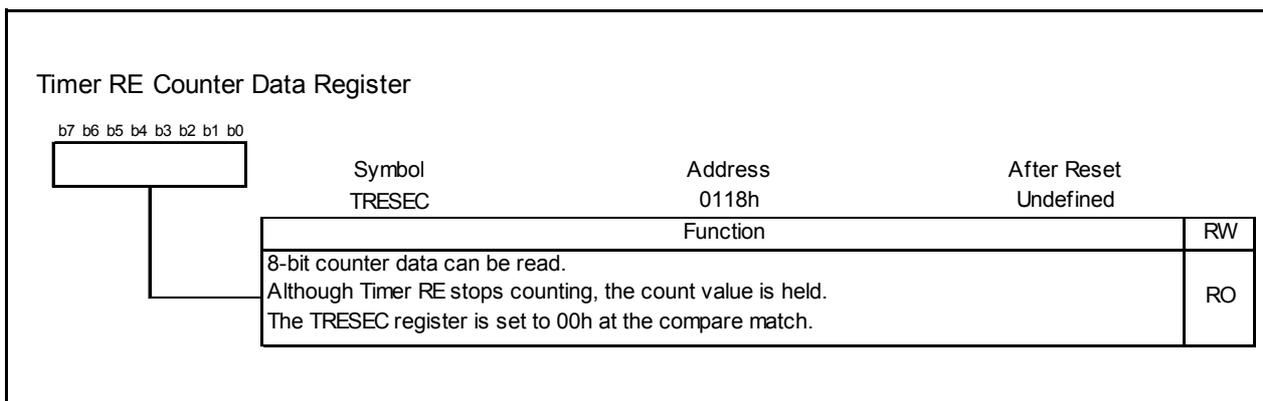
Figure 17.38 TRESEC Register in Output Compare Mode
