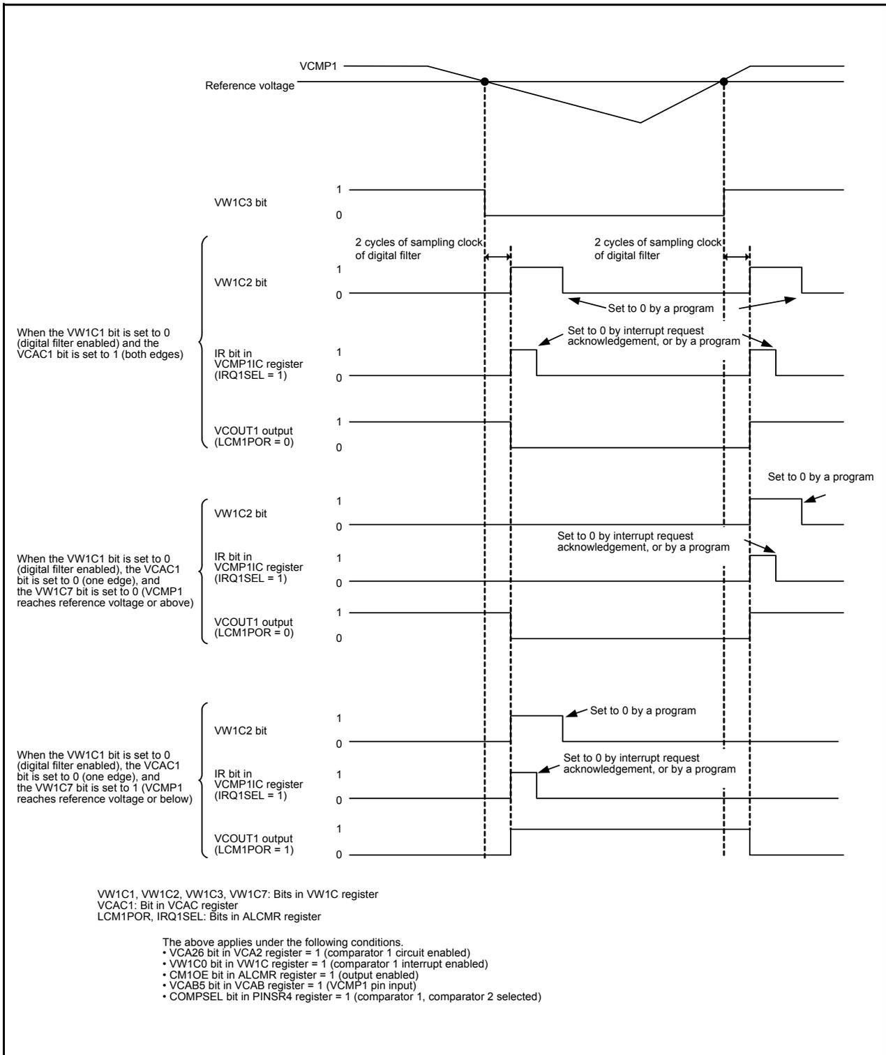
Figure 7.12 Operating Example of Comparator 1 (When Digital Filter Enabled)
