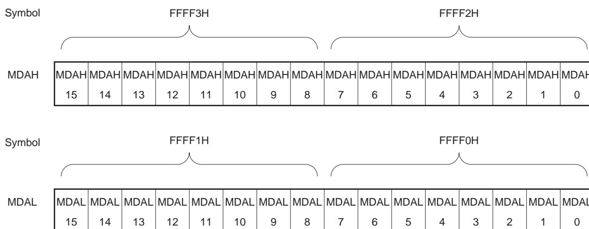
Figure 13-2. Format of Multiplication/Division Data Register A (MDAH, MDAL)
