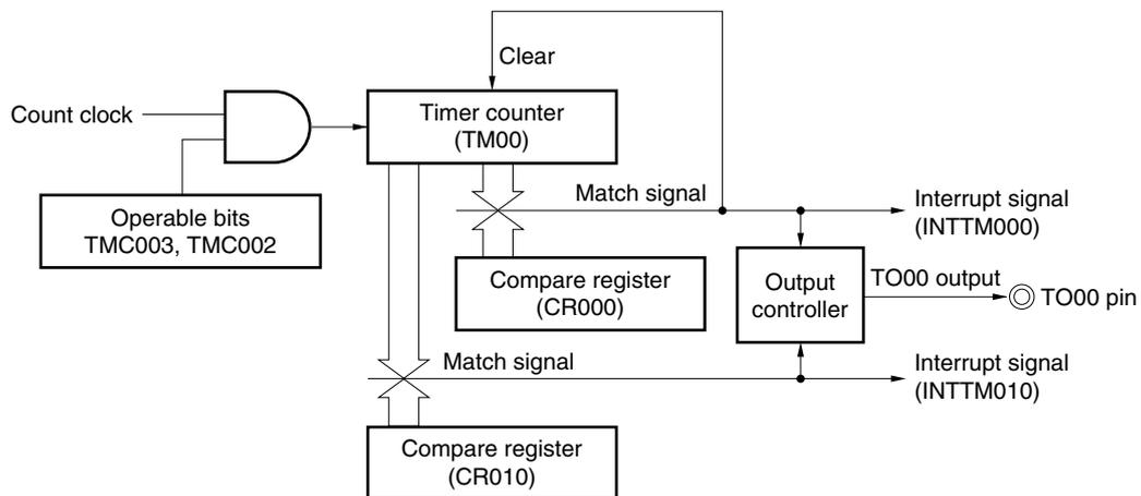
Figure 6-41. Example of Register Settings for PPG Output Operation (1/2)
