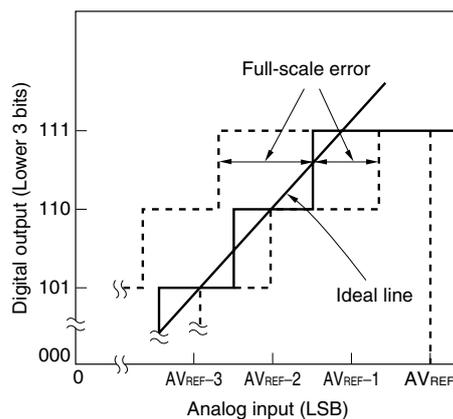
Figure 11-18. Integral Linearity Error
