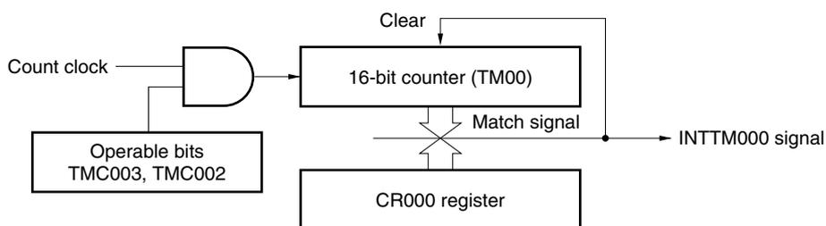
**Figure 6-12. Basic Timing Example of Interval Timer Operation**
