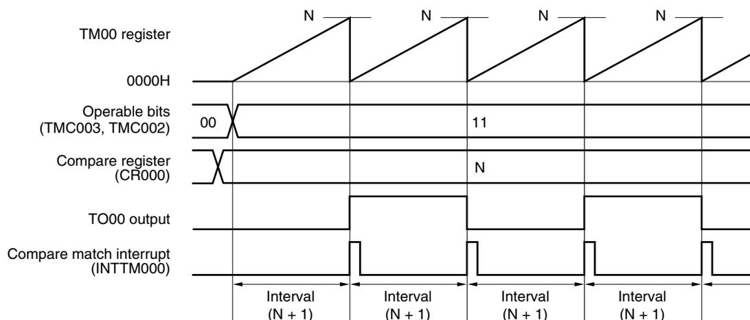
Figure 6-17. Example of Register Settings for Square-Wave Output Operation (1/2)
