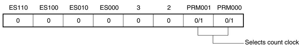
**Figure 6-41. Example of Register Settings for PPG Output Operation (2/2)****(e) 16-bit timer counter 00 (TM00)**
