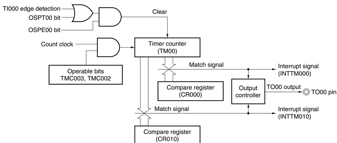
Figure 6-44. Example of Register Settings for One-Shot Pulse Output Operation (1/2)
