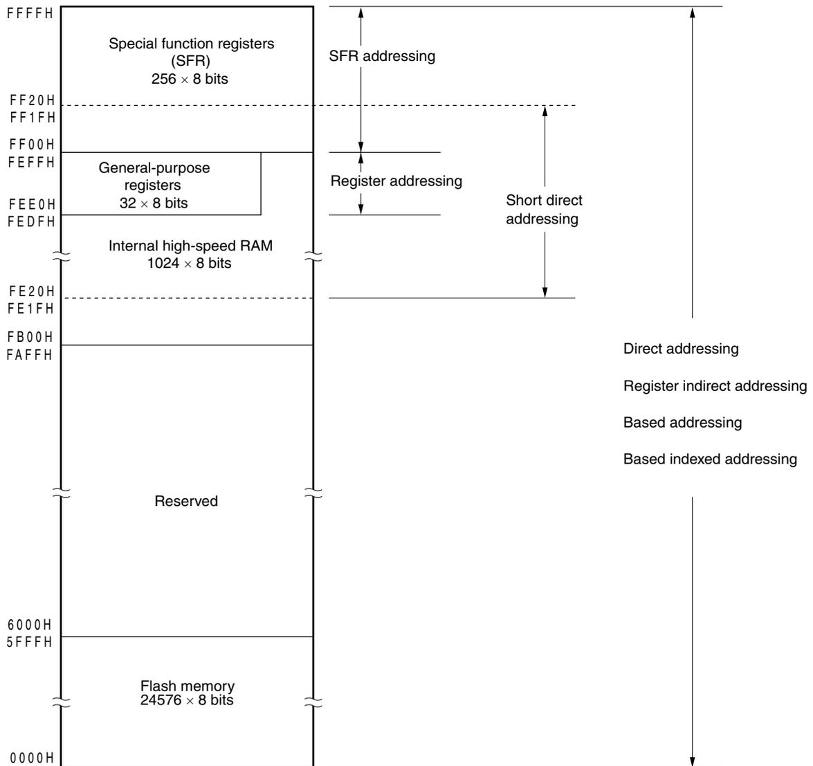
Figure 3-6. Correspondence Between Data Memory and Addressing (R7F0C013B)
