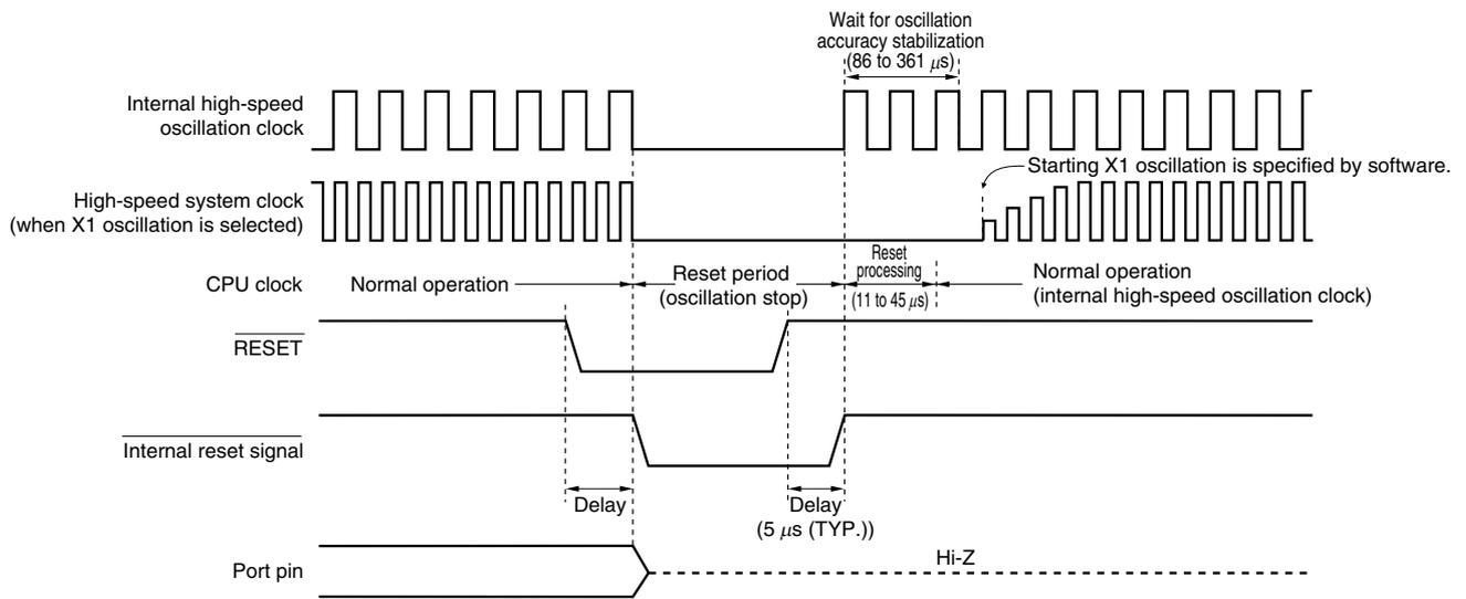
Figure 18-3. Timing of Reset Due to Watchdog Timer Overflow
