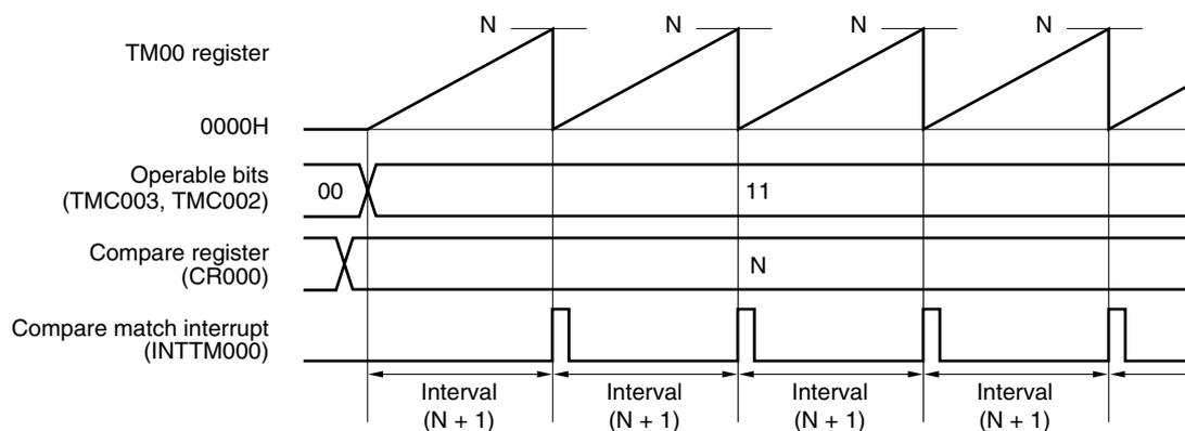
Figure 6-13. Example of Register Settings for Interval Timer Operation
