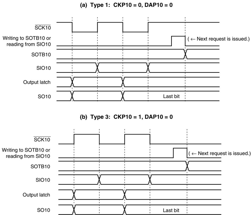
Figure 14-8. Output Value of SO10 Pin (Last Bit) (2/2)
