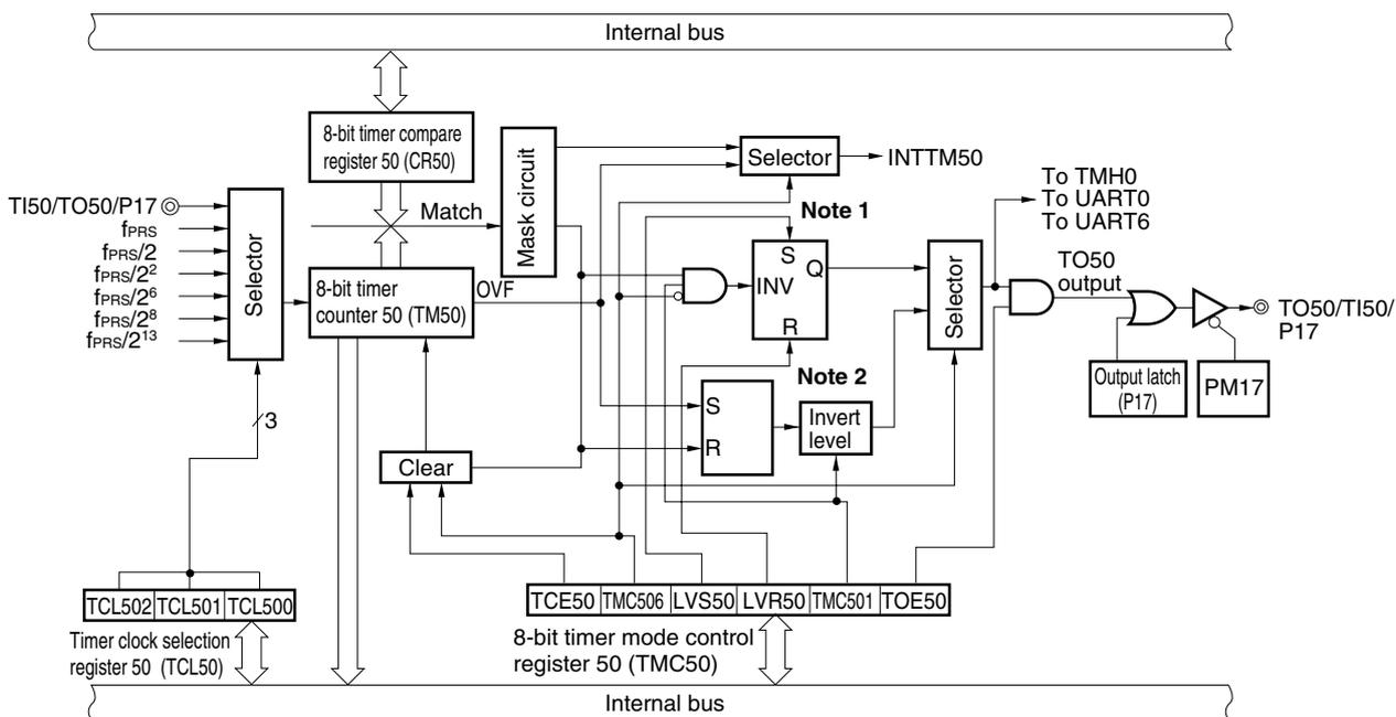
Figure 7-2. Block Diagram of 8-Bit Timer/Event Counter 51
