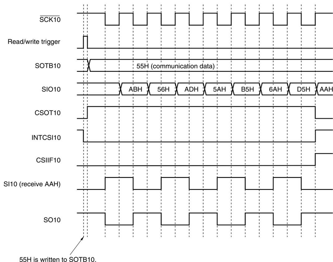
Figure 14-5. Timing in 3-Wire Serial I/O Mode (2/2)
