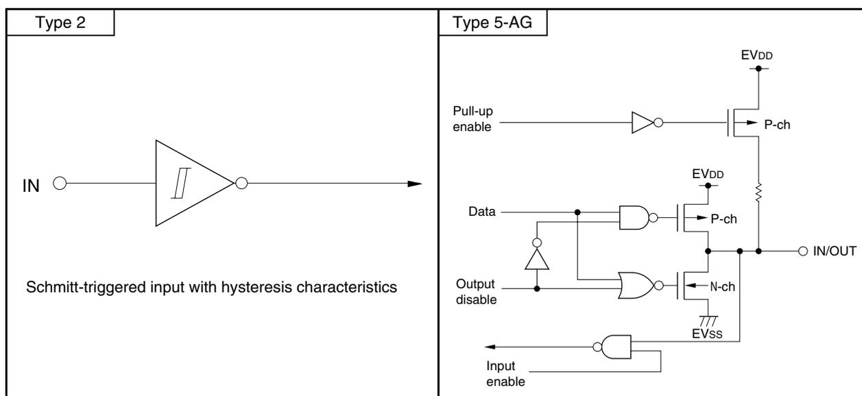
Figure 2-1. Pin I/O Circuit List (2/2)
