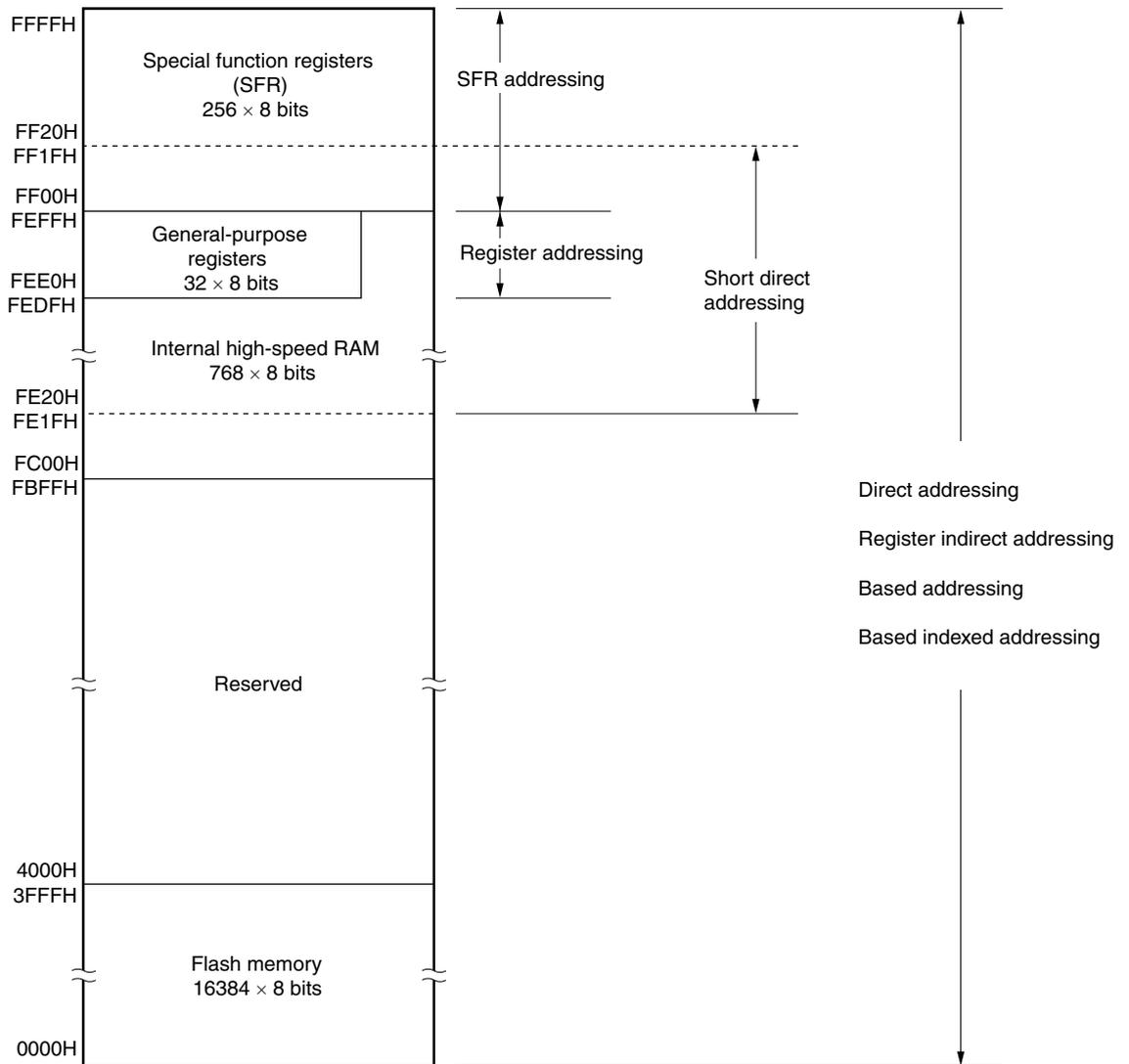
Figure 3-5. Correspondence Between Data Memory and Addressing (R7F0C012B)
