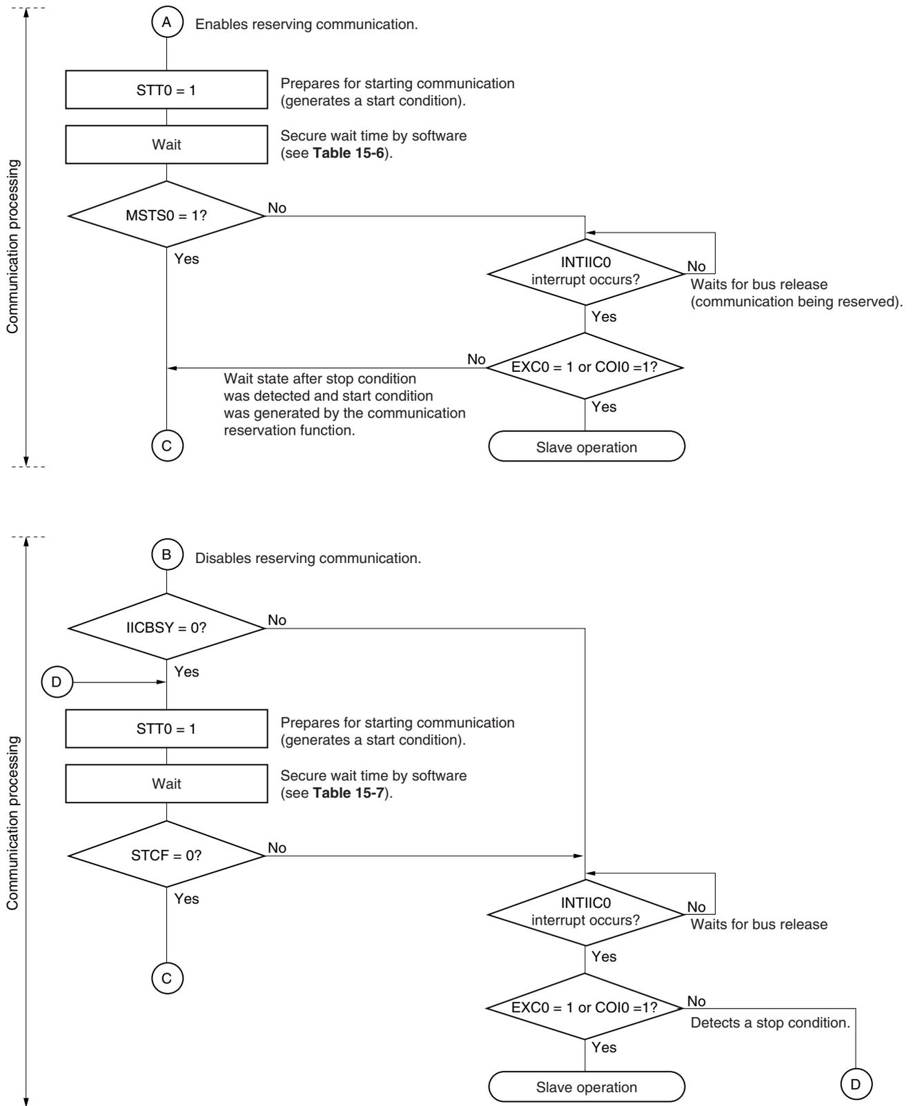
Figure 15-24. Master Operation in Multi-Master System (3/3)
