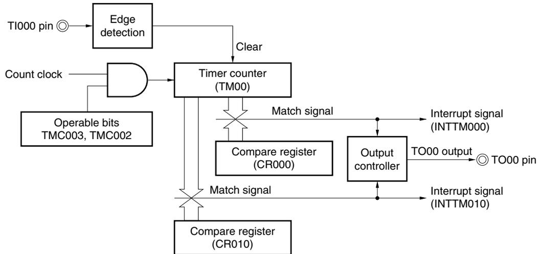
**Figure 6-23. Timing Example of Clear & Start Mode Entered by TI000 Pin Valid Edge Input
