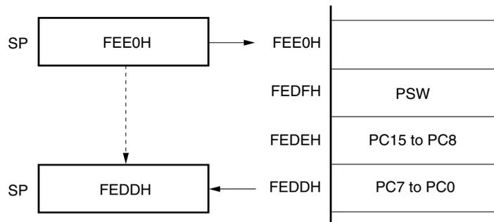
Figure 3-11. Data to Be Restored from Stack Memory
