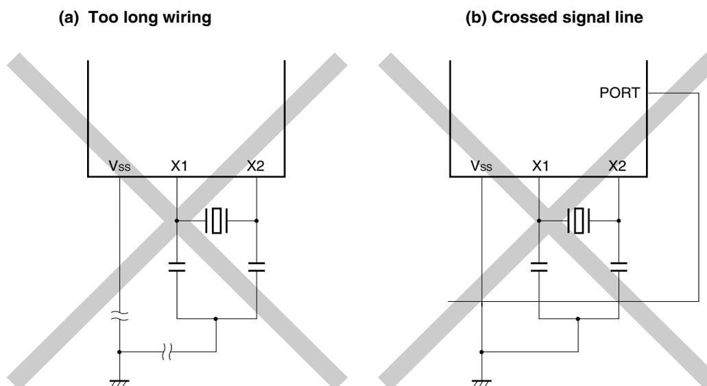
Figure 5-10. Examples of Incorrect Resonator Connection (2/2)
