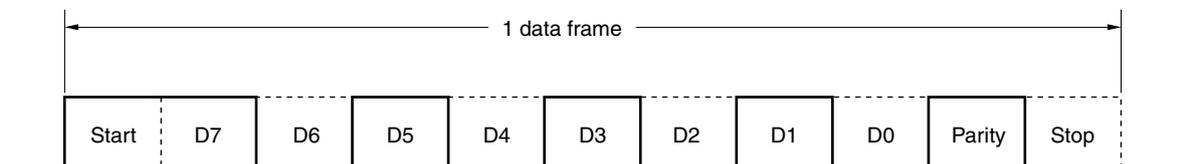
Figure 13-14. Example of Normal UART Transmit/Receive Data Waveform (2/2)
