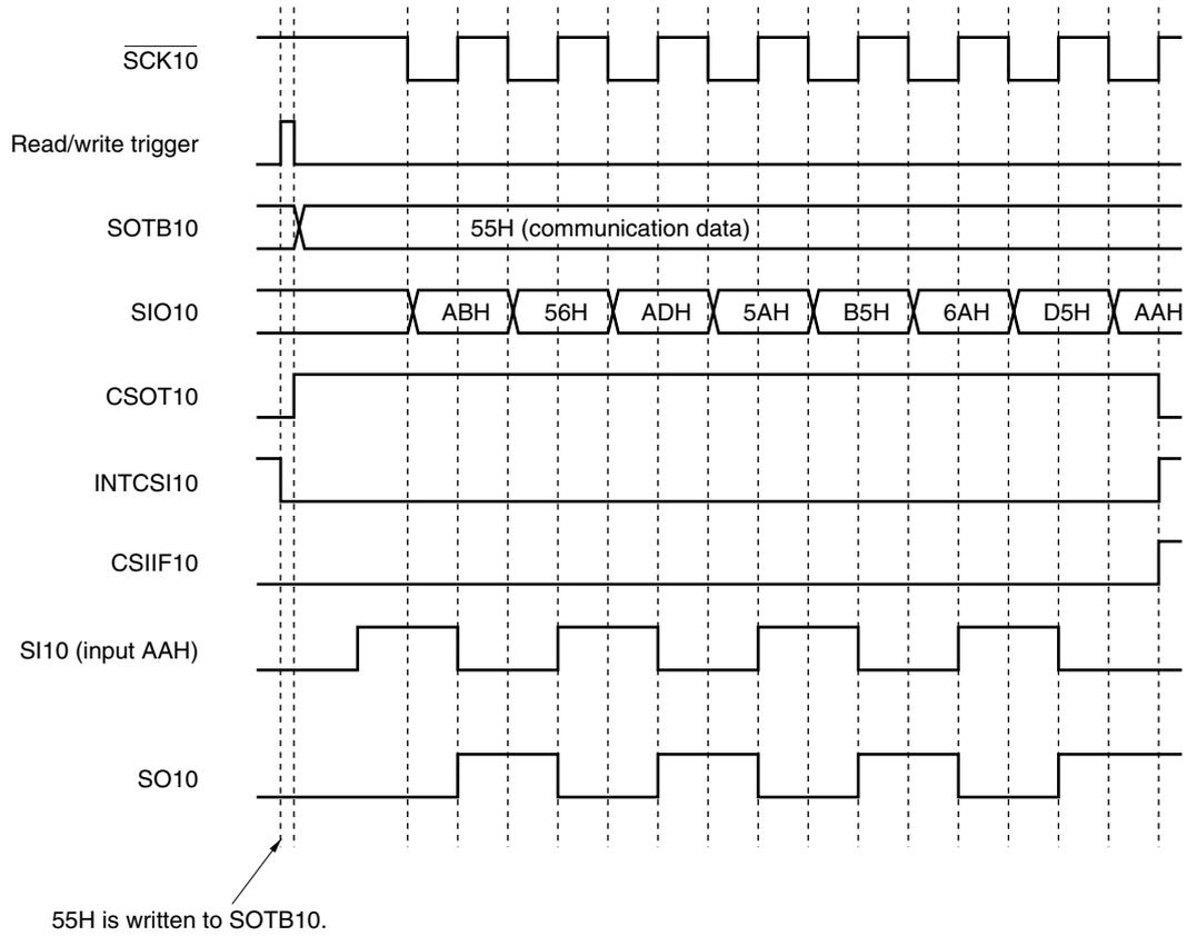
Figure 14-6. Timing of Clock/Data Phase
