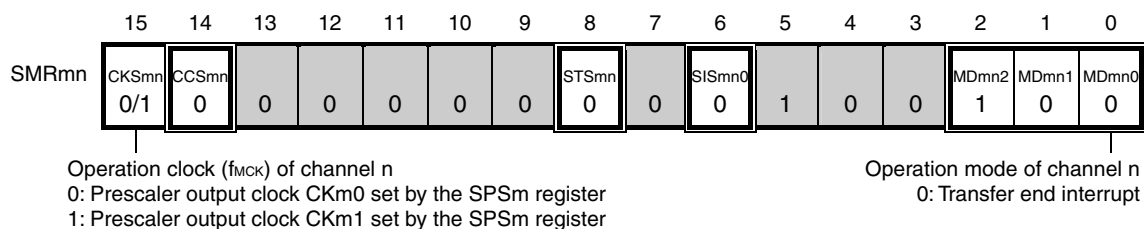
Figure 14-103. Example of Contents of Registers for Address Field Transmission of Simplified I 2 C (IIC00, IIC10) (1/2)
