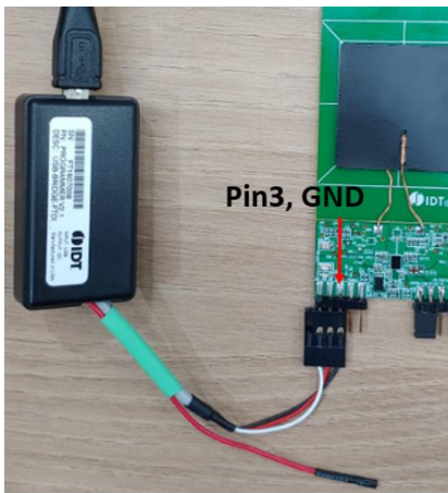
Figure 4. USB-to-I2C Dongle Connections to J12 Header
