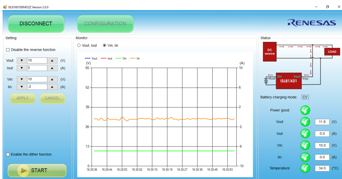
Figure 7. Precharge Complete Information in GUI
