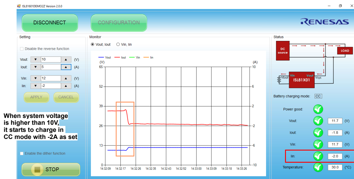
Figure 10. Mode Switching to Charging Information in GUI (Output)
