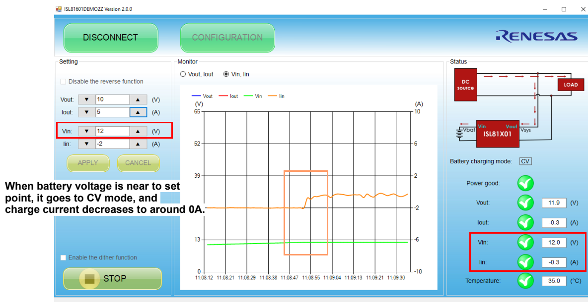
Figure 13. Fully Charging Information in GUI
