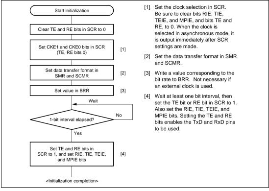
Figure 10.5 Sample SCI Initialization Flowchart
