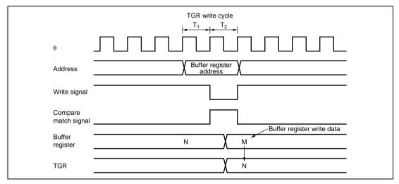
Figure 8.47 Contention between Buffer Register Write and Compare Match
