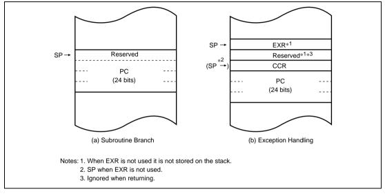
Figure 2.4 Stack Structure in Advanced Mode
