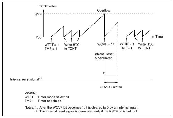
Figure 9.3 (b) WDT\_1 Operation in Watchdog Timer Mode
