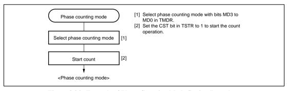
Figure 8.24 Example of Phase Counting Mode Setting Procedure
