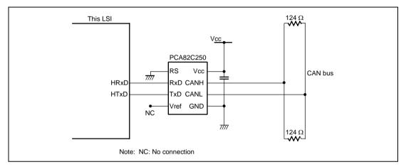
Figure 11.15 High-Speed Interface Using PCA82C250
