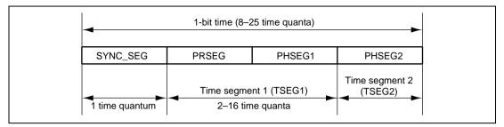
Figure 11.8 Detailed Description of One Bit
