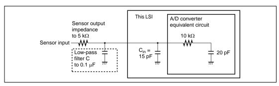
Figure 12.6 Example of Analog Input Circuit
