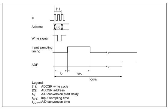
Figure 12.2 A/D Conversion Timing
