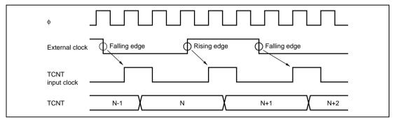
Figure 8.31 Count Timing in External Clock Operation
