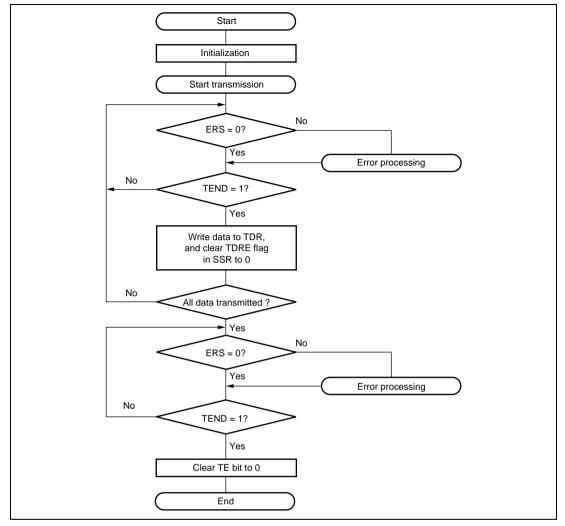
Figure 10.28 Example of Transmission Processing Flow
