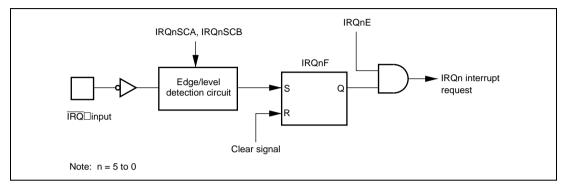
Figure 5.2 Block Diagram of Interrupts IRQ0 to IRQ5
