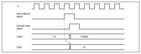
**Figure 8.35 Counter Clear Timing (Input Capture)**
