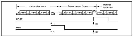
Figure 10.29 Retransfer Operation in SCI Receive Mode
