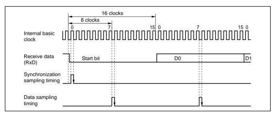
Figure 10.3 Receive Data Sampling Timing in Asynchronous Mode
