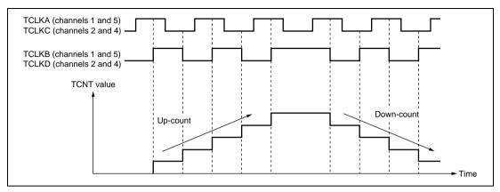
Figure 8.28 Example of Phase Counting Mode 4 Operation
