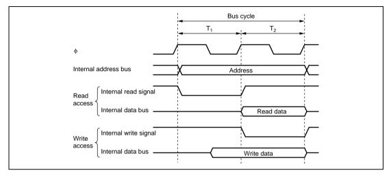
Figure 6.2 On-Chip Support Module Access Cycle
