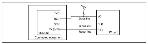
Figure 10.21 Schematic Diagram of Smart Card Interface Pin Connections
