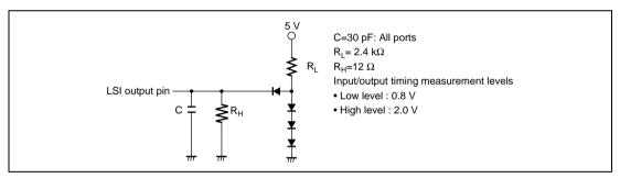
Figure 18.1 Output Load Circuit
