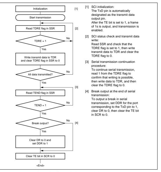
Figure 10.7 Sample Serial Transmission Flowchart
