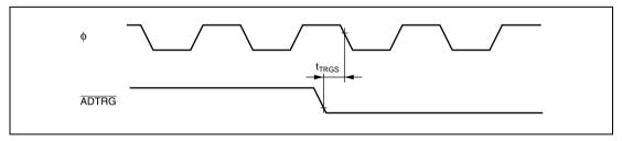
Figure 18.11 A/D Converter External Trigger Input Timing
