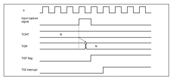
Figure 8.39 TGI Interrupt Timing (Input Capture)
