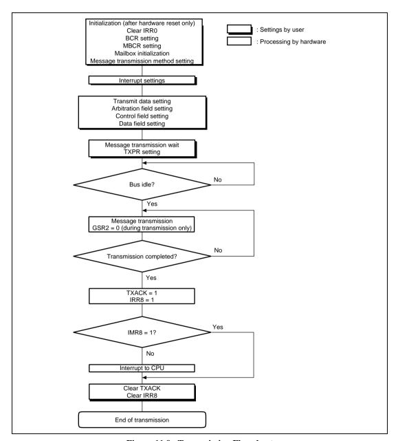
Figure 11.9 Transmission Flowchart
