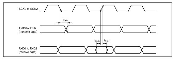
Figure 18.10 SCI Input/Output Timing (Clocked Synchronous Mode)
