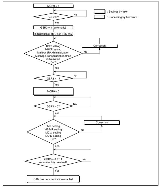
Figure 11.7 Software Reset Flowchart
