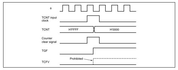
Figure 8.51 Contention between Overflow and Counter Clearing
