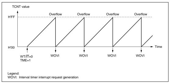
Figure 9.4 Operation in Interval Timer Mode
