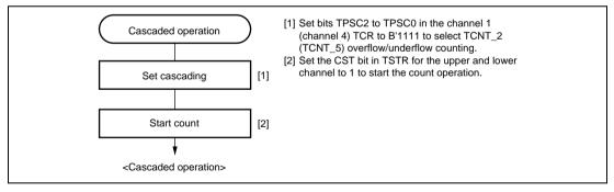
Figure 8.17 Cascaded Operation Setting Procedure
