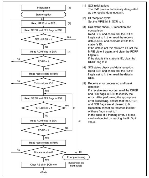
Figure 10.13 Sample Multiprocessor Serial Reception Flowchart (1)
