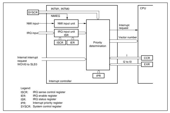
Figure 5.1 Block Diagram of Interrupt Controller
