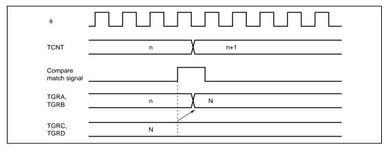
**Figure 8.36 Buffer Operation Timing (Compare Match)**
