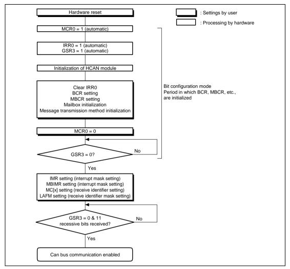
Figure 11.6 Hardware Reset Flowchart
