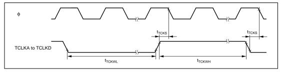
Figure 18.8 TPU Clock Input Timing
