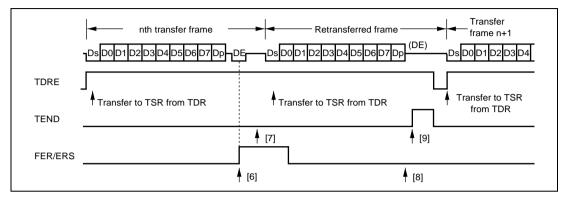
Figure 10.26 Retransfer Operation in SCI Transmit Mode
