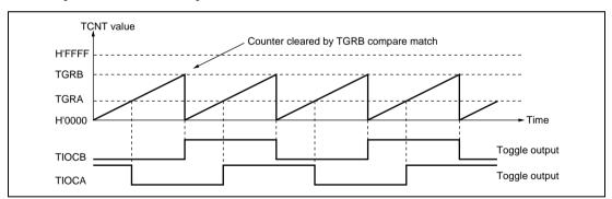
Figure 8.7 Example of Toggle Output Operation
