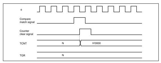
Figure 8.34 Counter Clear Timing (Compare Match)
