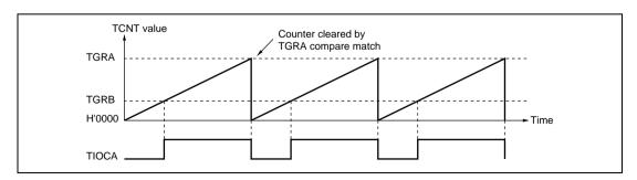
Figure 8.21 Example of PWM Mode Operation (1)
