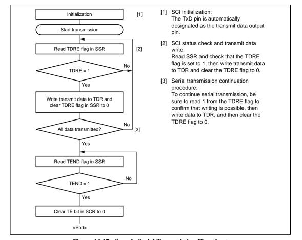
Figure 10.17 Sample Serial Transmission Flowchart
