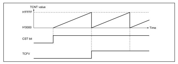
Figure 8.3 Free-Running Counter Operation
