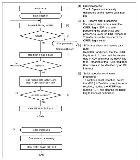
Figure 10.19 Sample Serial Reception Flowchart
