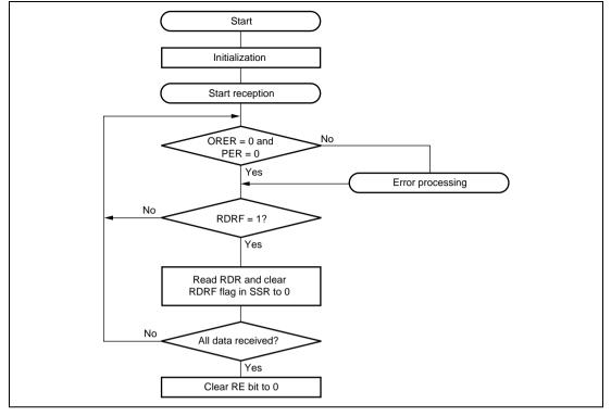
Figure 10.30 Example of Reception Processing Flow
