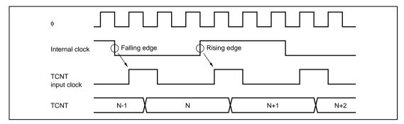
Figure 8.30 Count Timing in Internal Clock Operation
