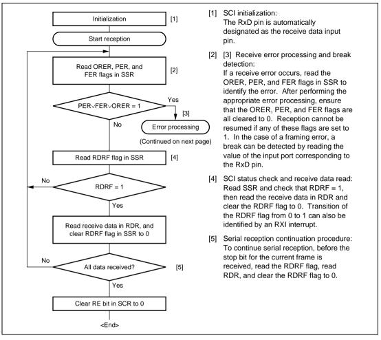
Figure 10.9 Sample Serial Reception Data Flowchart (1)
