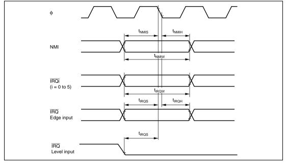
Figure 18.5 Interrupt Input Timing
