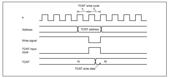
Figure 8.45 Contention between TCNT Write and Increment Operations
