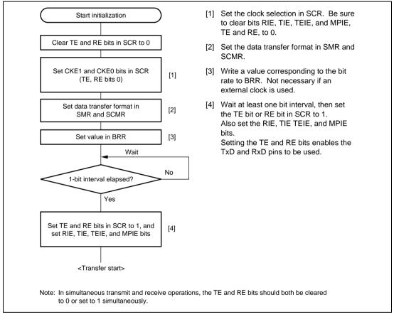
Figure 10.15 Sample SCI Initialization Flowchart
