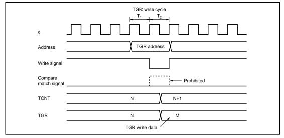
Figure 8.46 Contention between TGR Write and Compare Match
