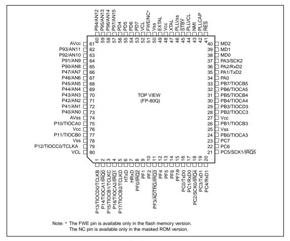
Figure 1.2 Pin Arrangement
