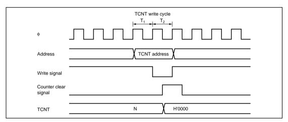
Figure 8.44 Contention between TCNT Write and Clear Operations
