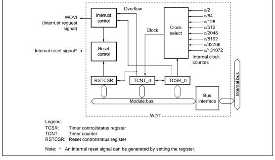
Figure 9.1 Block Diagram of WDT 0
