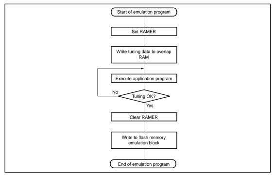
Figure 14.7 Flowchart for Flash Memory Emulation in RAM
