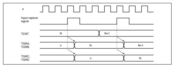
Figure 8.37 Buffer Operation Timing (Input Capture)
