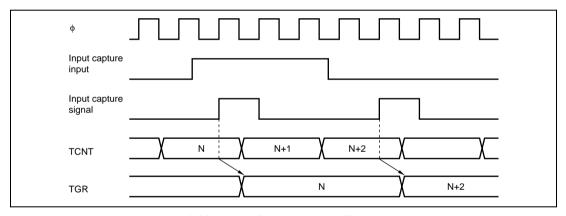
Figure 8.33 Input Capture Input Signal Timing
