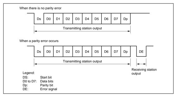
Figure 10.22 Normal Smart Card Interface Data Format
