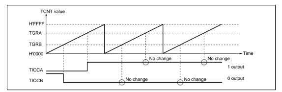
Figure 8.6 Example of 0 Output/1 Output Operation
