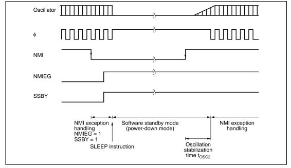
Figure 16.3 Software Standby Mode Application Example
