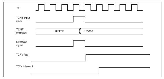
Figure 8.40 TCIV Interrupt Setting Timing
