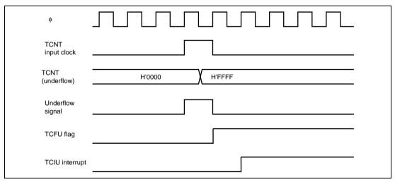
Figure 8.41 TCIU Interrupt Setting Timing
