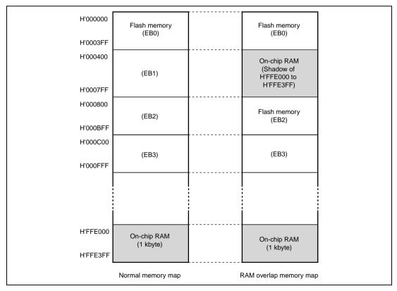
Figure 14.8 Example of RAM Overlap Operation
