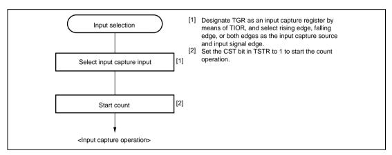
Figure 8.8 Example of Input Capture Operation Setting Procedure
