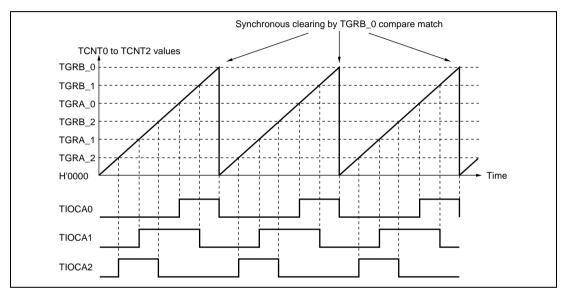
Figure 8.11 Example of Synchronous Operation
