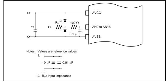
Figure 12.7 Example of Analog Input Protection Circuit
