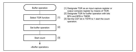
Figure 8.14 Example of Buffer Operation Setting Procedure
