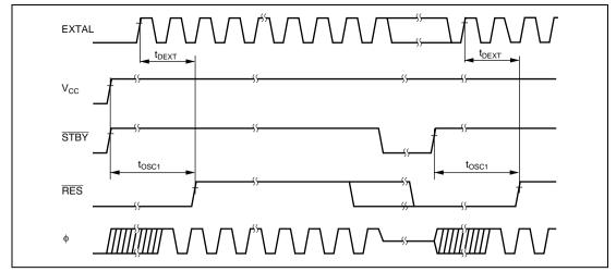
Figure 18.3 Oscillation Stabilization Timing
