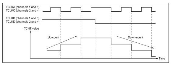
Figure 8.26 Example of Phase Counting Mode 2 Operation
