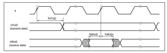
Figure 18.12 HCAN Input/Output Timing
