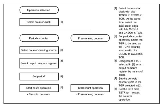
Figure 8.2 Example of Counter Operation Setting Procedure
