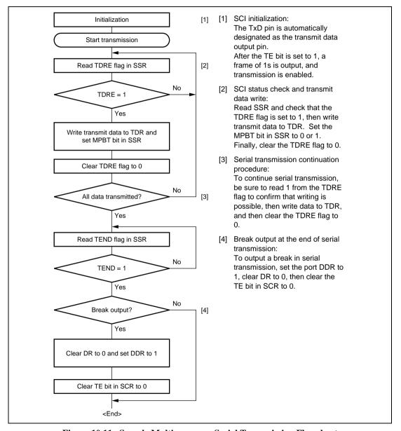
Figure 10.11 Sample Multiprocessor Serial Transmission Flowchart
