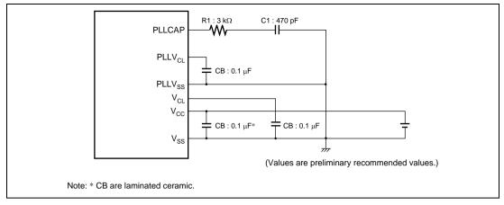
Figure 15.7 External Circuitry Recommended for PLL Circuit
