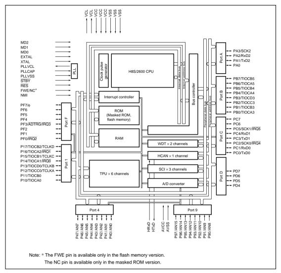
Figure 1.1 Internal Block Diagram
