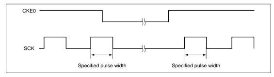
Figure 10.31 Timing for Fixing Clock Output Level
