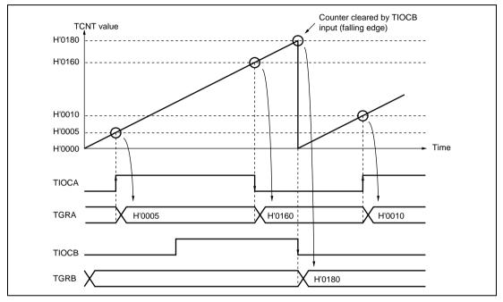
Figure 8.9 Example of Input Capture Operation
