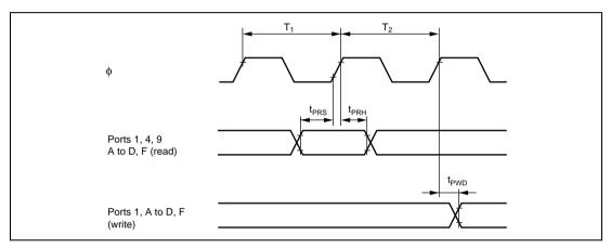
Figure 18.6 I/O Port Input/Output Timing
