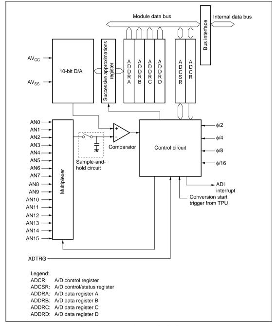
Figure 12.1 Block Diagram of A/D Converter
