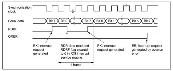
Figure 10.18 Example of SCI Operation in Reception
