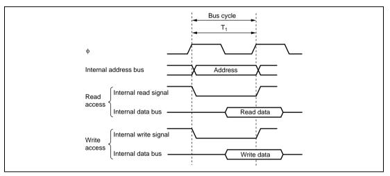
Figure 6.1 On-Chip Memory Access Cycle
