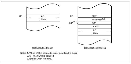
Figure 2.2 Stack Structure in Normal Mode
