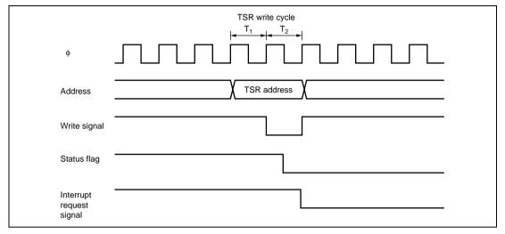
Figure 8.42 Timing for Status Flag Clearing by CPU
