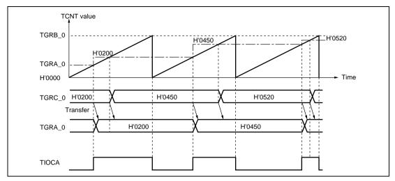
Figure 8.15 Example of Buffer Operation (1)
