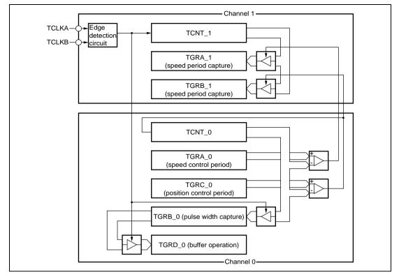
Figure 8.29 Phase Counting Mode Application Example
