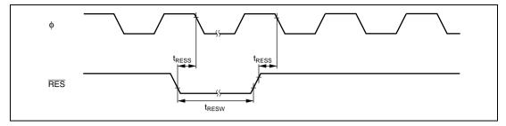
Figure 18.4 Reset Input Timing
