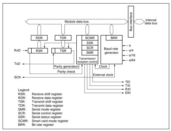
Figure 10.1 Block Diagram of SCI
