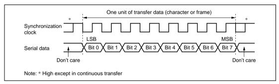
Figure 10.14 Data Format in Synchronous Communication (For LSB-First)
