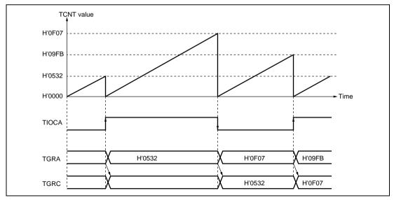
Figure 8.16 Example of Buffer Operation (2)
