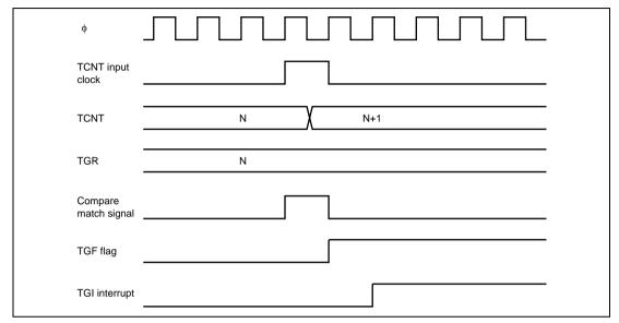
Figure 8.38 TGI Interrupt Timing (Compare Match)
