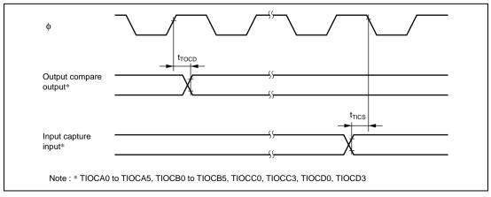
Figure 18.7 TPU Input/Output Timing
