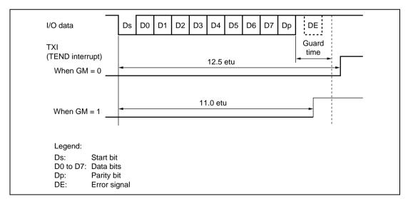
Figure 10.27 TEND Flag Generation Timing in Transmission Operation
