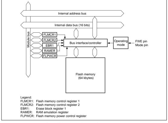
Figure 14.1 Block Diagram of Flash Memory
