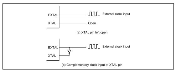
Figure 15.4 External Clock Input (Examples)
