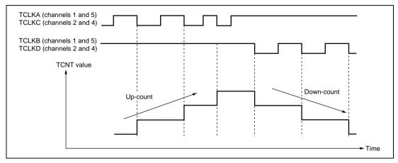
Figure 8.27 Example of Phase Counting Mode 3 Operation
