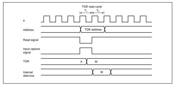
Figure 8.48 Contention between TGR Read and Input Capture
