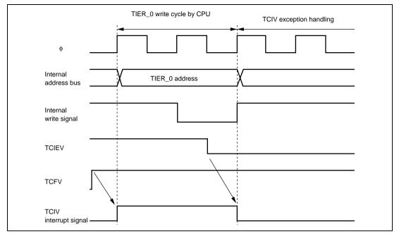
Figure 5.6 Contention between Interrupt Generation and Disabling
