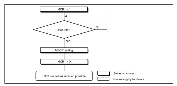
Figure 11.14 HCAN Halt Mode Flowchart
