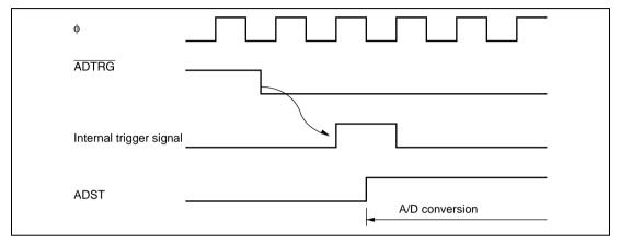
Figure 12.3 External Trigger Input Timing
