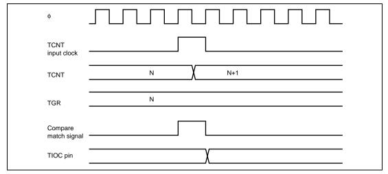
Figure 8.32 Output Compare Output Timing
