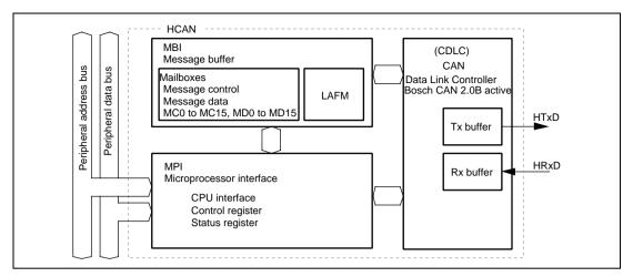
Figure 11.1 HCAN Block Diagram
