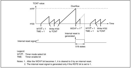
Figure 9.3 (a) WDT\_0 Operation in Watchdog Timer Mode
