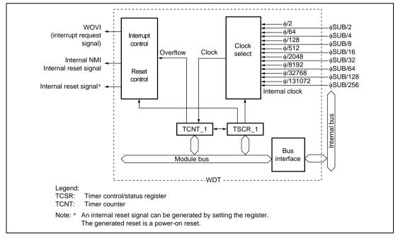
Figure 9.2 Block Diagram of WDT\_1
