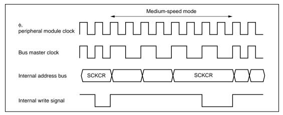
Figure 16.2 Medium-Speed Mode Transition and Clearance Timing
