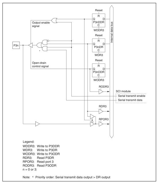
Figure C.5 Port 3 Block Diagram (Pins P30 and P33)
