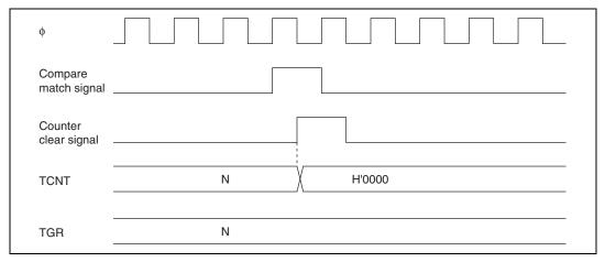
Figure 10.34 Counter Clear Timing (Compare Match)
