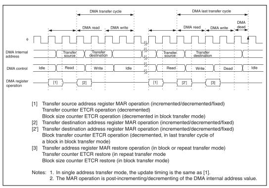
Figure 7.29 DMAC Register Update Timing
