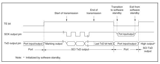
Figure 12.30 Synchronous Transmission Using Internal Clock
