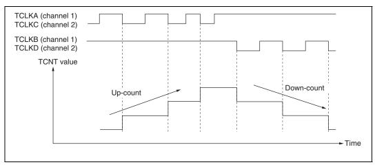
Figure 10.28 Example of Phase Counting Mode 3 Operation
