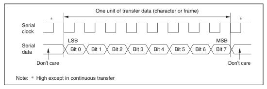
Figure 12.19 Data Format in Synchronous Communication
