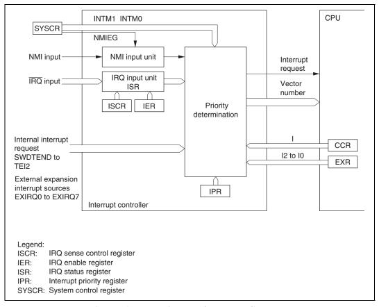
Figure 5.1 Block Diagram of Interrupt Controller
