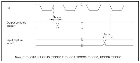
Figure 18.13 TPU Input/Output Timing
