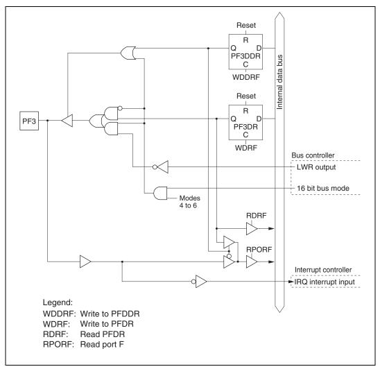
Figure C.28 Port F Block Diagram (Pin PF3)
