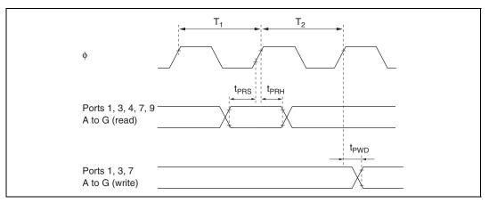
Figure 18.12 I/O Port Input/Output Timing
