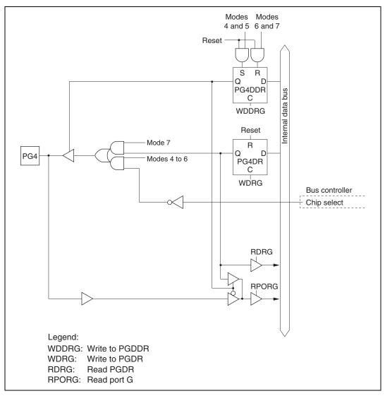
Figure C.34 Port G Block Diagram (Pin PG4)
