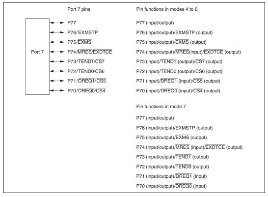
Figure 9.4 Port 7 Pin Functions
