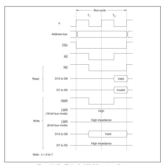
Figure 6.6 Bus Timing for 8-Bit 2-State Access Space
