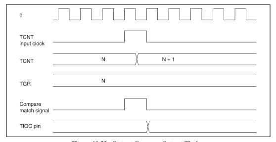
Figure 10.32 Output Compare Output Timing
