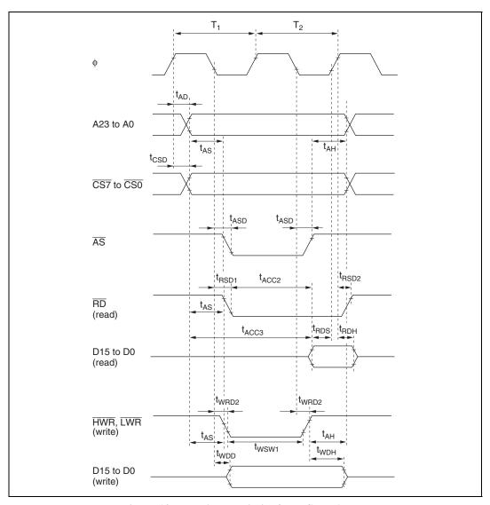
Figure 18.7 Basic Bus Timing/Two-State Access
