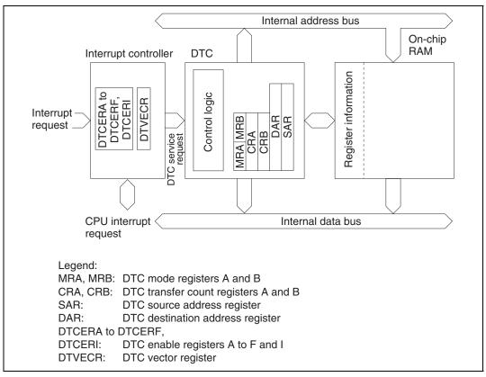
Figure 8.1 Block Diagram of DTC
