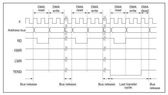
Figure 7.16 Example of Short Address Mode Transfer
