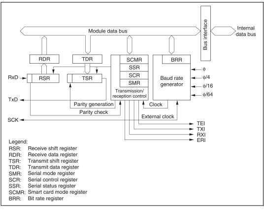
Figure 12.2 Block Diagram of SCI1 and SCI2
