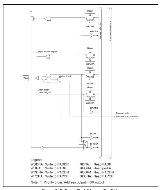
Figure C.17 Port A Block Diagram (Pin PA0)
