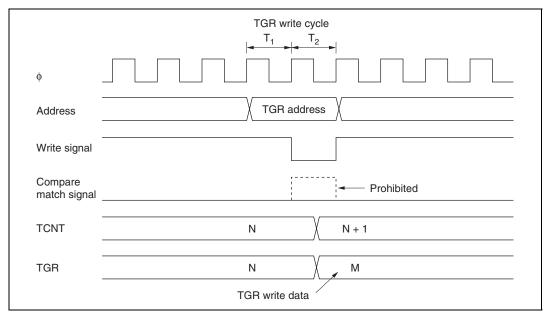
Figure 10.47 Contention between TGR Write and Compare Match
