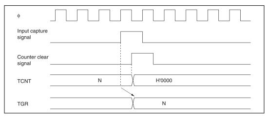
Figure 10.35 Counter Clear Timing (Input Capture)
