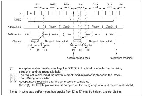
Figure 7.22 Example of DREQ Level Activated Normal Mode Transfer
