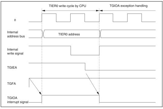
Figure 5.8 Contention between Interrupt Generation and Disabling
