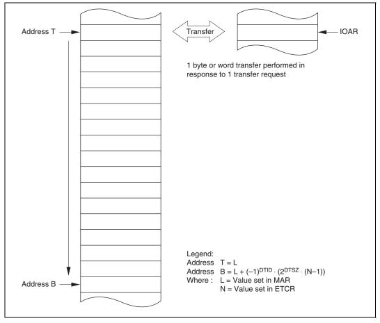
Figure 7.3 Operation in Sequential Mode
