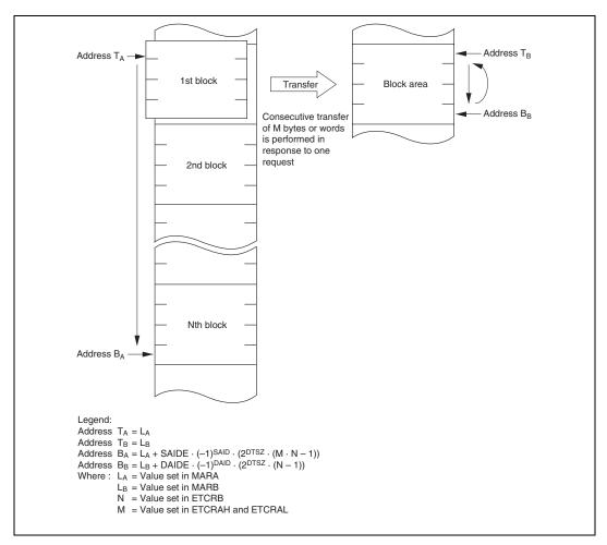
Figure 7.11 Operation in Block Transfer Mode (BLKDIR = 0)
