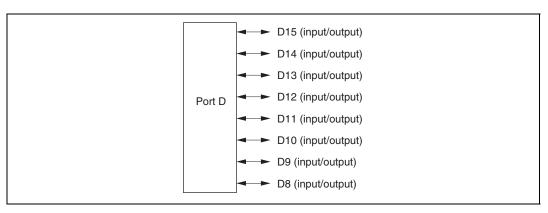
Figure 9.13 Port D Pin Functions (Modes 4 to 6)
