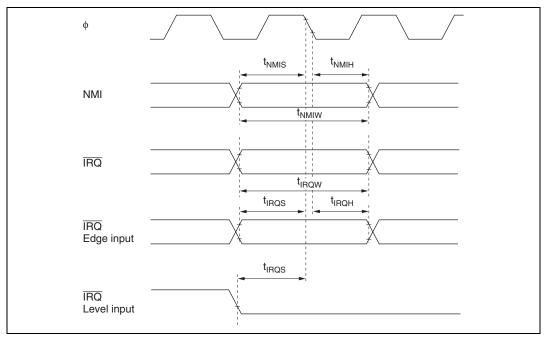
Figure 18.6 Interrupt Input Timing
