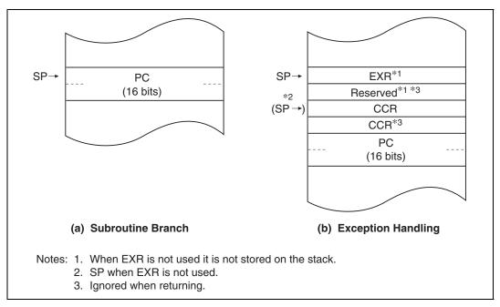
Figure 2.3 Stack Structure in Normal Mode
