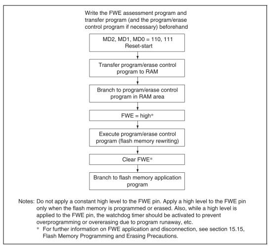
Figure 15.13 User Program Mode Execution Procedure
