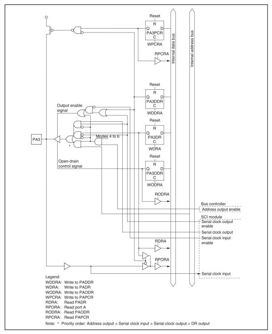
Figure C.20 Port A Block Diagram (Pin PA3)
