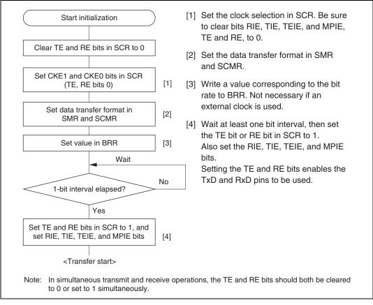
Figure 12.20 Sample SCI Initialization Flowchart
