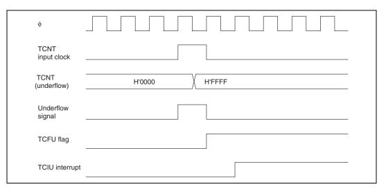
Figure 10.41 TCIU Interrupt Setting Timing
