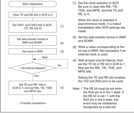
Figure 12.7 Sample SCI Initialization Flowchart
