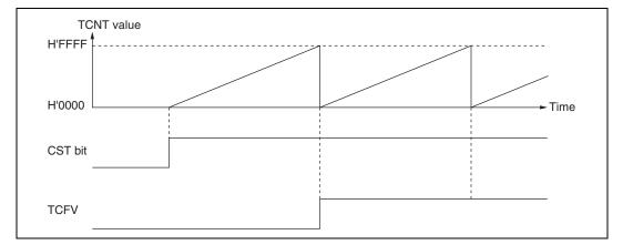
Figure 10.7 Free-Running Counter Operation
