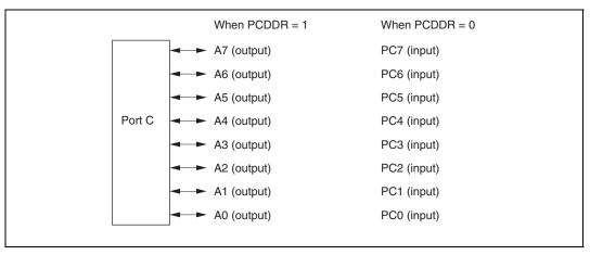
Figure 9.10 Port C Pin Functions (Mode 6)
