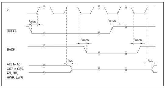
Figure 18.11 External Bus Release Timing
