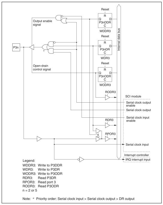
Figure C.7 Port 3 Block Diagram (Pins P32 and P35)
