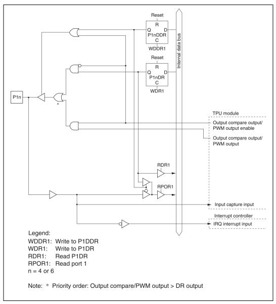
Figure C.3 Port 1 Block Diagram (Pins P14 and P16)
