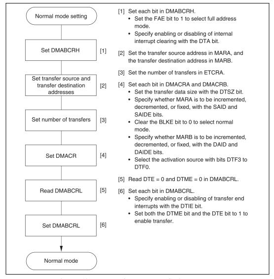
Figure 7.10 Example of Normal Mode Setting Procedure
