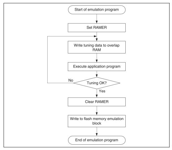
Figure 15.17 Flowchart for Flash Memory Emulation in RAM
