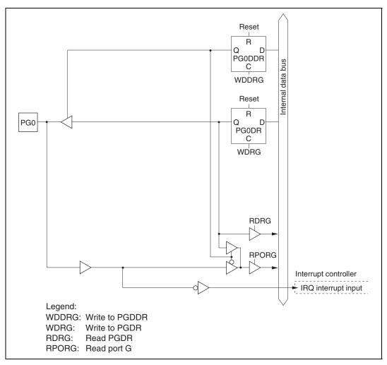
Figure C.31 Port G Block Diagram (Pin PG0)
