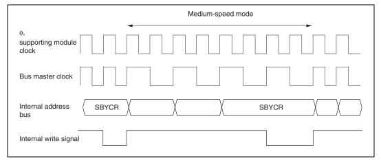
Figure 17.2 Medium-Speed Mode Transition and Clearance Timing
