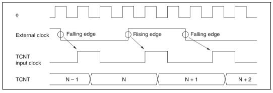
Figure 10.31 Count Timing in External Clock Operation
