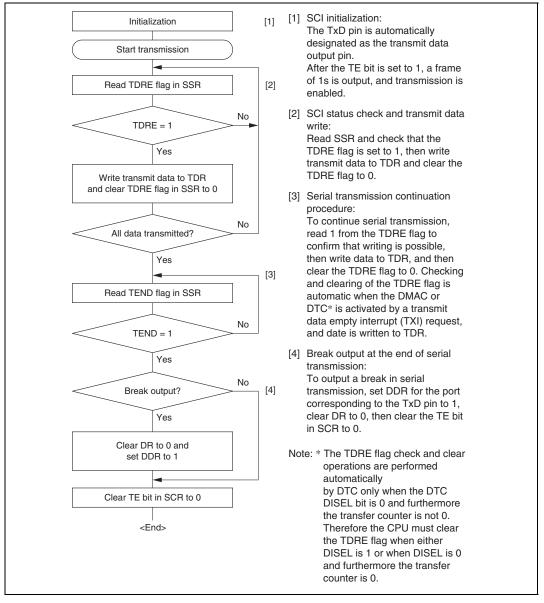
Figure 12.8 Sample Serial Transmission Flowchart
