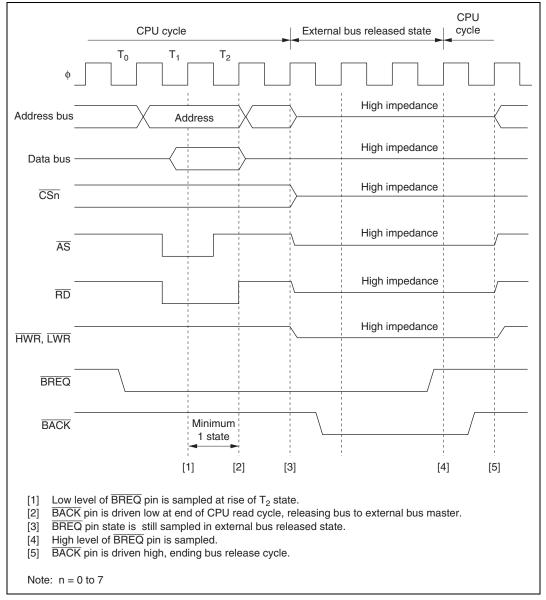
Figure 6.20 Bus-Released State Transition Timing
