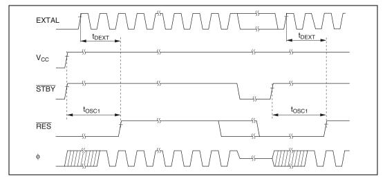
Figure 18.4 Oscillator Settling Timing
