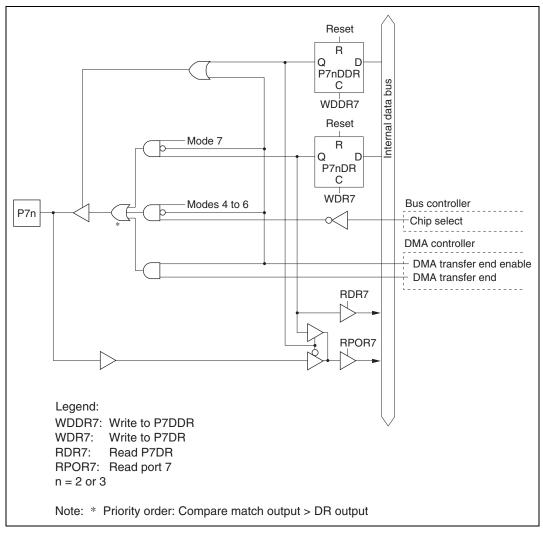
Figure C.12 Port 7 Block Diagram (Pins P72 and P73)
