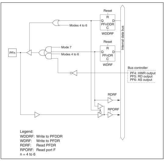
Figure C.29 Port F Block Diagram (Pins PF4 to PF6)
