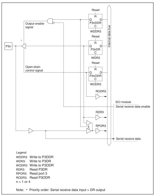
Figure C.6 Port 3 Block Diagram (Pins P31 and P34)
