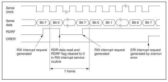
Figure 12.24 Example of SCI Operation in Reception
