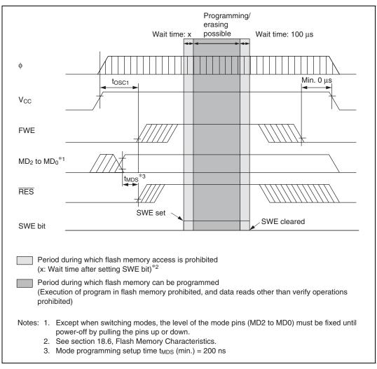
Figure 15.30 Power-On/Off Timing (User Program Mode)
