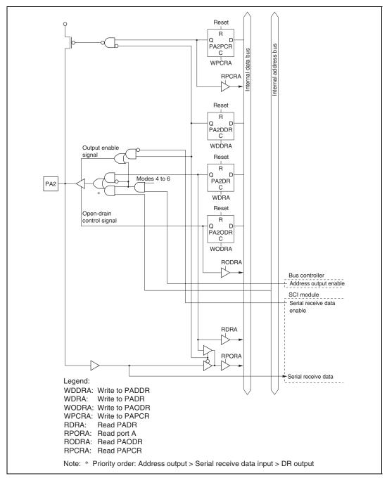
Figure C.19 Port A Block Diagram (Pin PA2)
