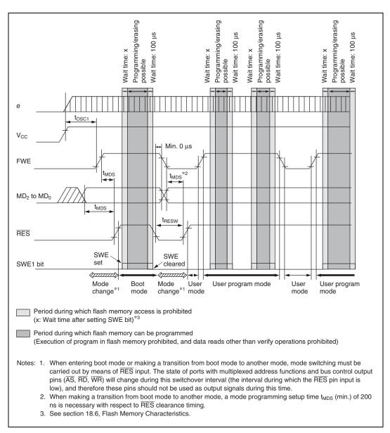
Figure 15.31 Mode Transition Timing
