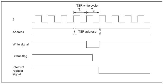
Figure 10.42 Timing for Status Flag Clearing by CPU
