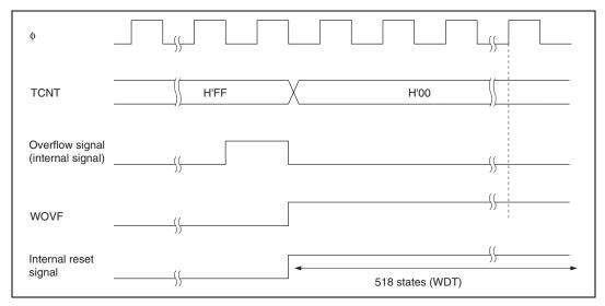
Figure 11.7 Timing of WOVF Setting
