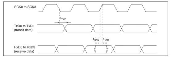
Figure 18.16 SCI Input/Output Timing/Clock Synchronous Mode
