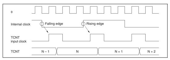
Figure 10.30 Count Timing in Internal Clock Operation
