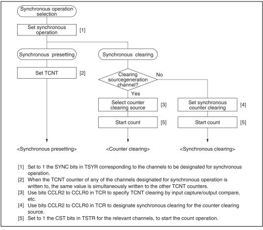
Figure 10.14 Example of Synchronous Operation Setting Procedure
