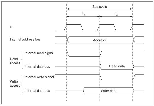
Figure 2.20 On-Chip Supporting Module Access Cycle
