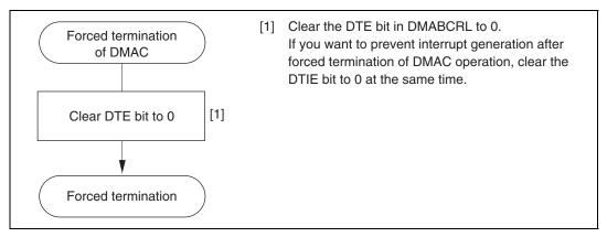
Figure 7.26 Example of Procedure for Forcibly Terminating DMAC Operation
