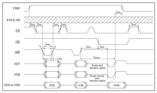
Figure 15.26 Auto-Erase Mode Timing Waveforms
