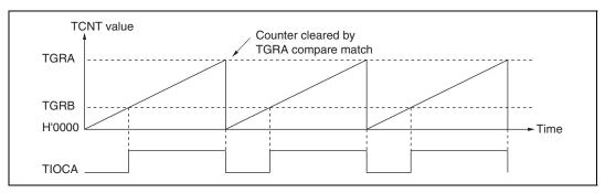
Figure 10.22 Example of PWM Mode Operation (1)
