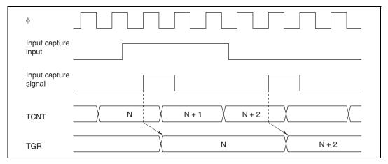
Figure 10.33 Input Capture Input Signal Timing
