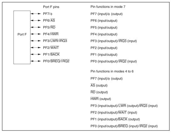
Figure 9.18 Port F Pin Functions
