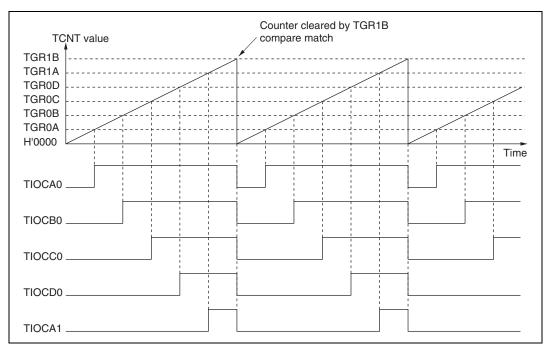
Figure 10.23 Example of PWM Mode Operation (2)
