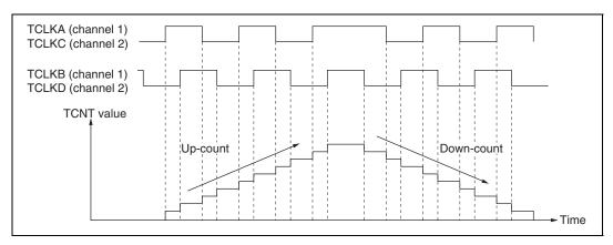
Figure 10.26 Example of Phase Counting Mode 1 Operation
