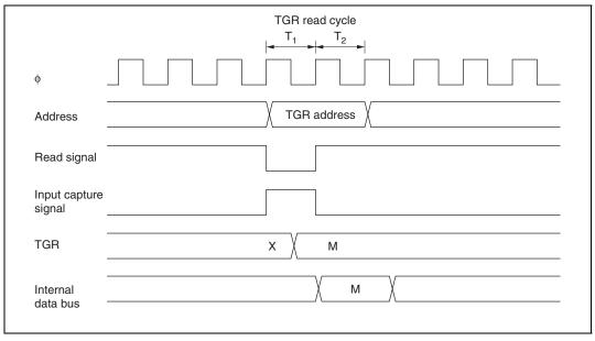
Figure 10.49 Contention between TGR Read and Input Capture
