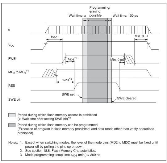
Figure 15.29 Power-On/Off Timing (Boot Mode)
