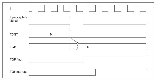
Figure 10.39 TGI Interrupt Timing (Input Capture)
