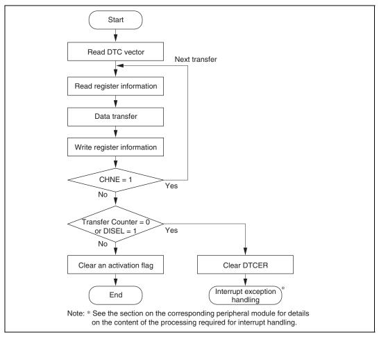
Figure 8.2 Flowchart of DTC Operation
