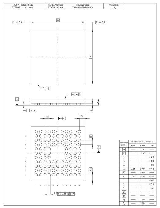
Figure G.3 TBP-112A, TBP-112AV Package Dimensions
