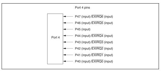
Figure 9.3 Port 4 Pin Functions
