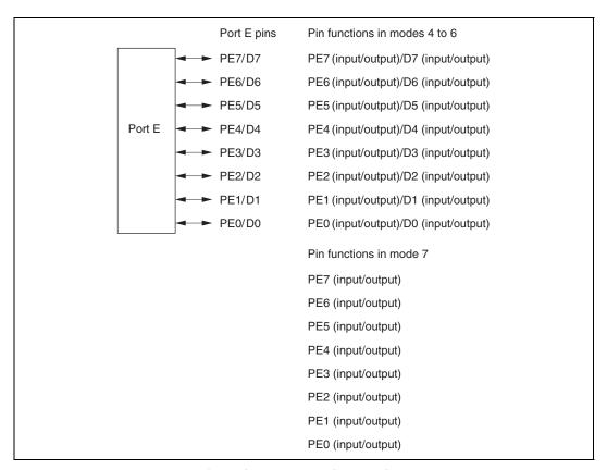
Figure 9.15 Port E Pin Functions
