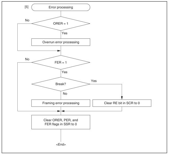
Figure 12.17 Sample Multiprocessor Serial Reception Flowchart (2)
