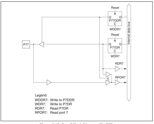
Figure C.15 Port 7 Block Diagram (Pin P77)
