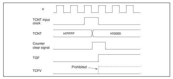
Figure 10.52 Contention between Overflow and Counter Clearing
