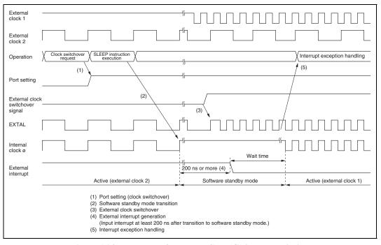
Figure 16.8 Example of External Clock Switchover Timing
