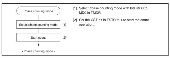
Figure 10.25 Example of Phase Counting Mode Setting Procedure
