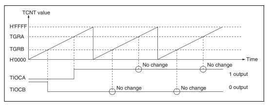
Figure 10.10 Example of 0 Output/1 Output Operation
