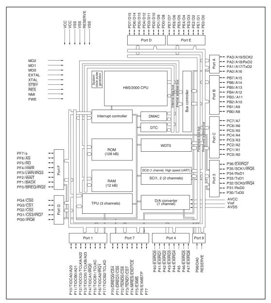
Figure 1.1 H8S/2214 Group Internal Block Diagram
