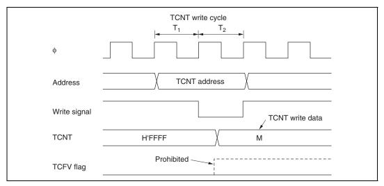
Figure 10.53 Contention between TCNT Write and Overflow
