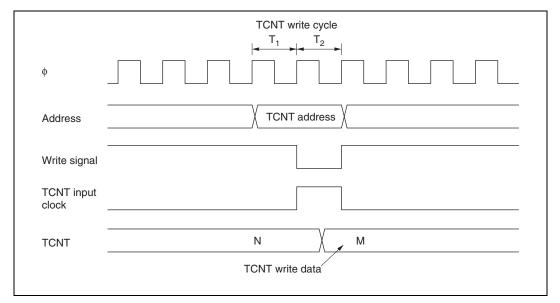
Figure 10.46 Contention between TCNT Write and Increment Operations
