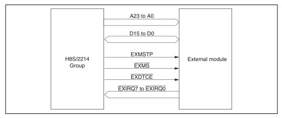
Figure 6.21 Multichip Block Diagram
