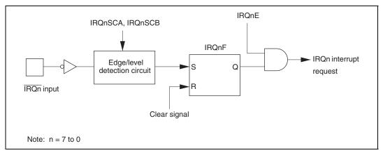
Figure 5.2 Block Diagram of Interrupts IRQn
