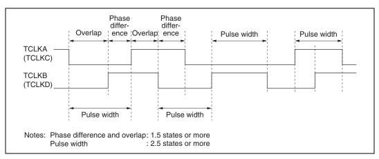
Figure 10.44 Phase Difference, Overlap, and Pulse Width in Phase Counting Mode
