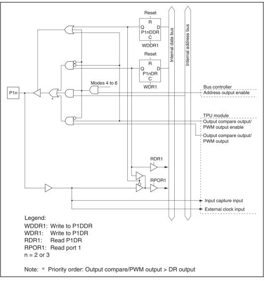
Figure C.2 Port 1 Block Diagram (Pins P12 and P13)
