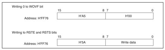
Figure 11.3 Format of Data Written to RSTCSR (Example of WDT0)
