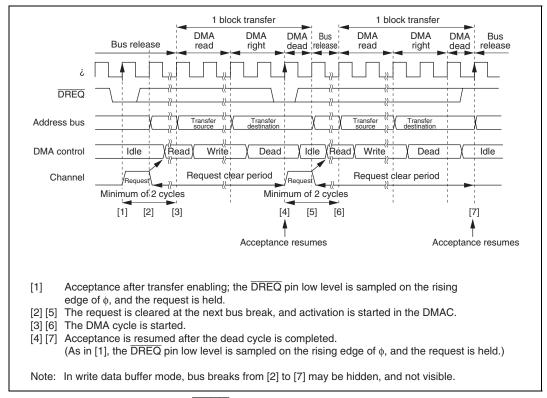
Figure 7.23 Example of DREQ Level Activated Block Transfer Mode Transfer
