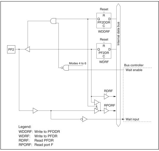
Figure C.27 Port F Block Diagram (Pin PF2)
