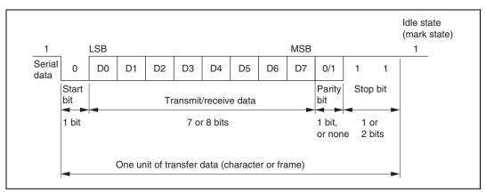
Figure 12.5 Data Format in Asynchronous Communication (Example with 8-Bit Data, Parity, Two Stop Bits)
