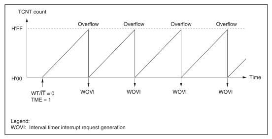
Figure 11.5 Operation in Interval Timer Mode
