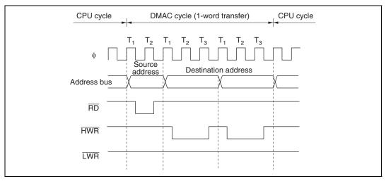
Figure 7.15 Example of DMA Transfer Bus Timing
