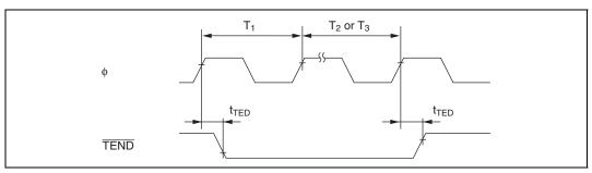
Figure 18.17 DMAC TEND Output Timing
