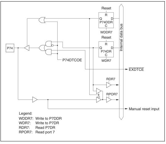
Figure C.13 Port 7 Block Diagram (Pin P74)
