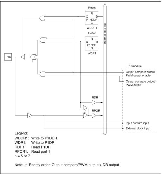
Figure C.4 Port 1 Block Diagram (Pins P15 and P17)
