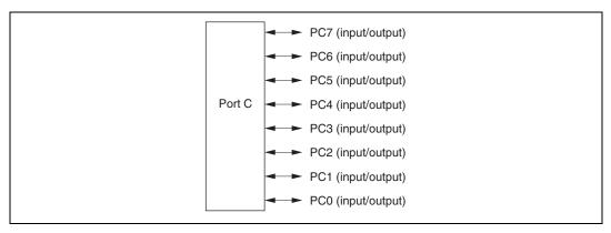
Figure 9.11 Port C Pin Functions (Mode 7)
