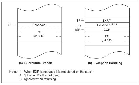
Figure 2.5 Stack Structure in Advanced Mode
