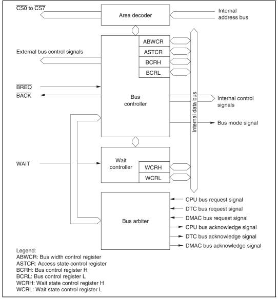
Figure 6.1 Block Diagram of Bus Controller
