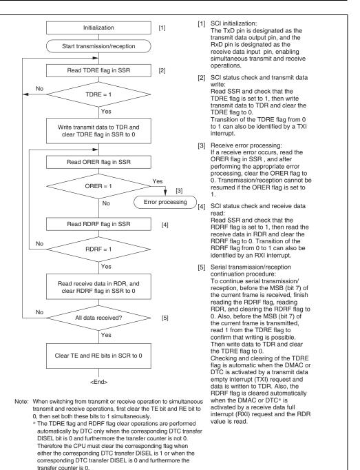
Figure 12.25 Sample Flowchart of Simultaneous Serial Transmit and Receive Operations
