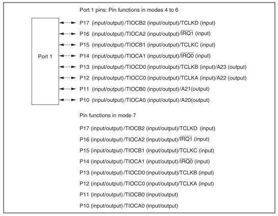
**Figure 9.1 Port 1 Pin Functions**
