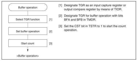
Figure 10.18 Example of Buffer Operation Setting Procedure
