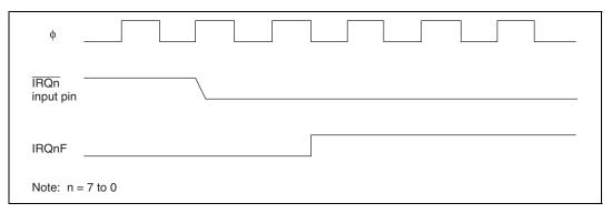
Figure 5.3 Timing of Setting IRQnF
