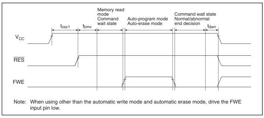
Figure 15.28 Oscillation Stabilization Time, Boot Program Transfer Time, and Power-Down Sequence
