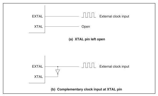
Figure 16.5 External Clock Input (Examples)
