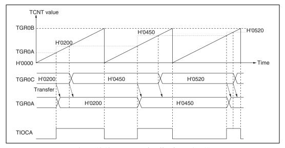
Figure 10.19 Example of Buffer Operation (1)
