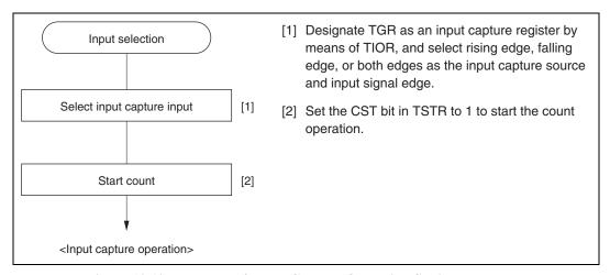
Figure 10.12 Example of Input Capture Operation Setting Procedure
