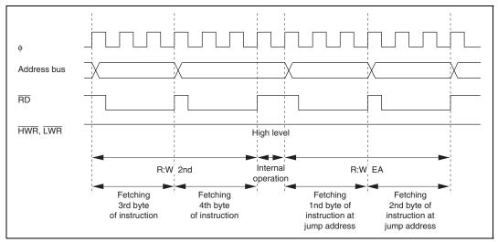
Figure A.1 Address Bus, RD, HWR, and LWR Timing (8-Bit Bus, Three-State Access, No Wait States)
