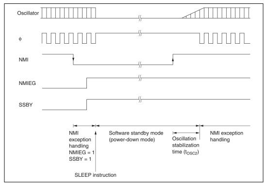
Figure 17.3 Software Standby Mode Application Example
