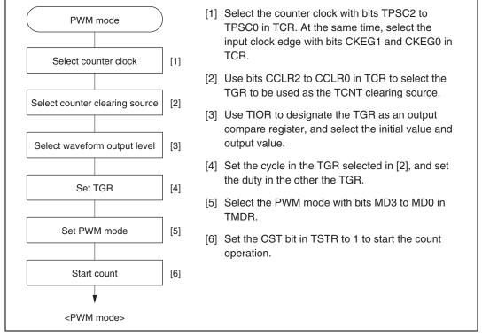
Figure 10.21 Example of PWM Mode Setting Procedure
