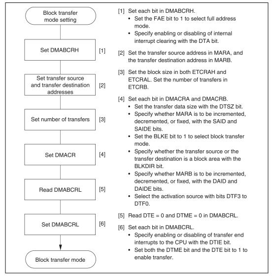
Figure 7.14 Example of Block Transfer Mode Setting Procedure
