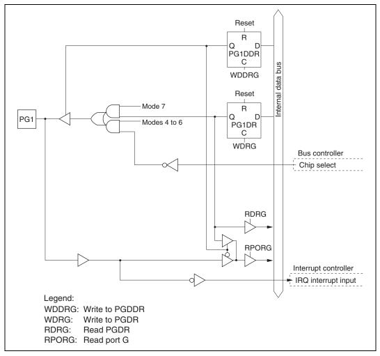
Figure C.32 Port G Block Diagram (Pin PG1)
