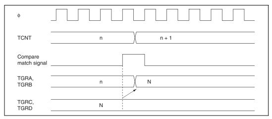
Figure 10.36 Buffer Operation Timing (Compare Match)
