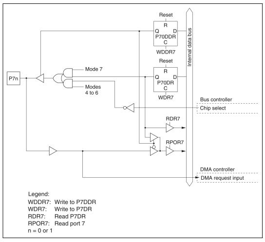
Figure C.11 Port 7 Block Diagram (Pins P70 and P71)
