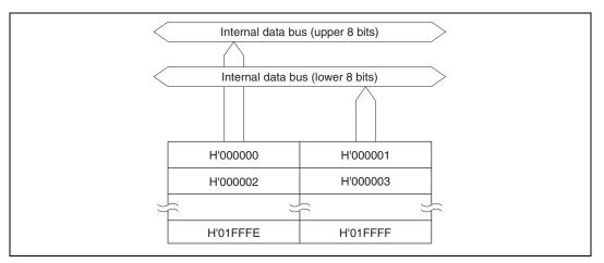
Figure 15.1 Block Diagram of ROM
