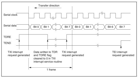
Figure 12.22 Example of SCI Operation in Transmission
