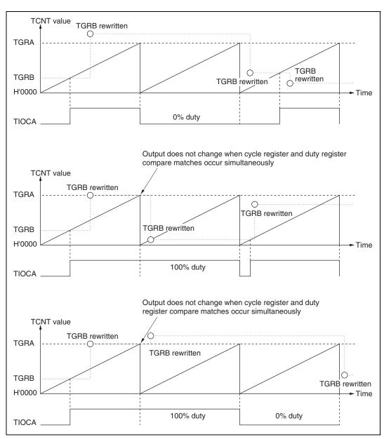
Figure 10.24 Example of PWM Mode Operation (3)
