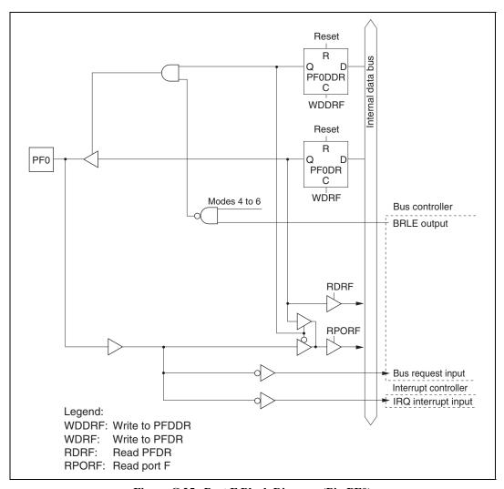
Figure C.25 Port F Block Diagram (Pin PF0)
