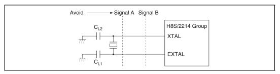
Figure 16.4 Example of Incorrect Board Design
