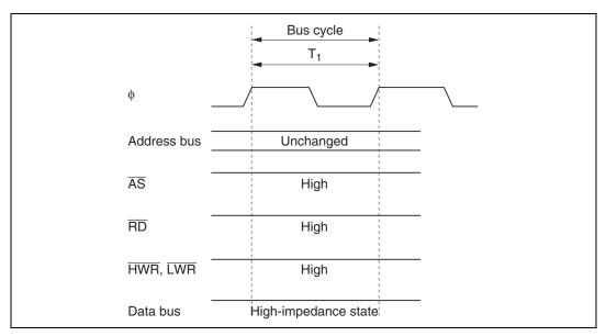
Figure 2.19 Pin States during On-Chip Memory Access
