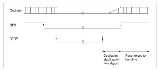
**Figure 17.4 Hardware Standby Mode Timing (Example)**
