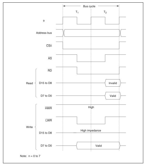
Figure 6.9 Bus Timing for 16-Bit 2-State Access Space (Odd Address Byte Access)
