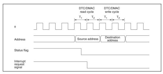
Figure 10.43 Timing for Status Flag Clearing by DTC/DMAC Activation
