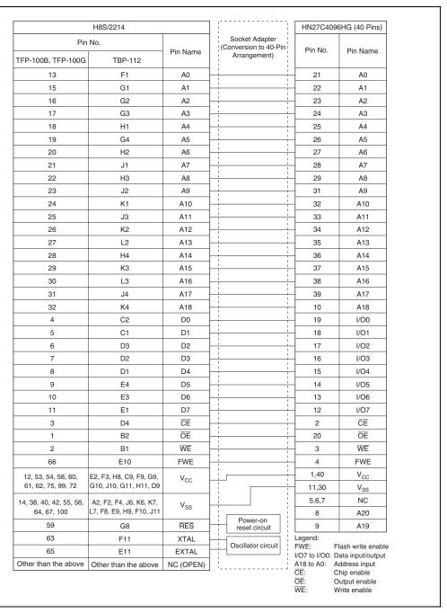
Figure 15.20 Socket Adapter Pin Correspondence Diagram
