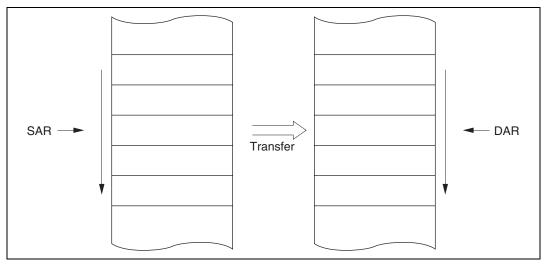
Figure 8.6 Memory Mapping in Normal Mode
