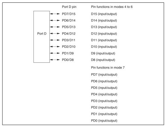
Figure 9.12 Port D Pin Functions
