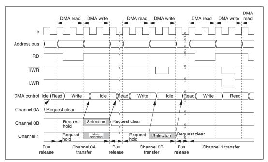
Figure 7.24 Example of Multi-Channel Transfer
