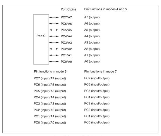
Figure 9.8 Port C Pin Functions
