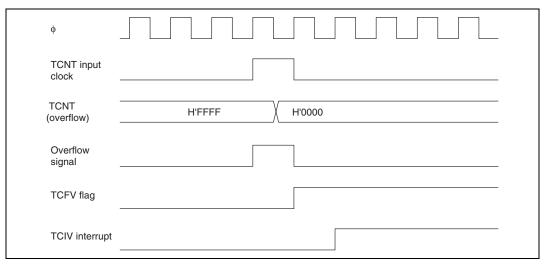
Figure 10.40 TCIV Interrupt Setting Timing
