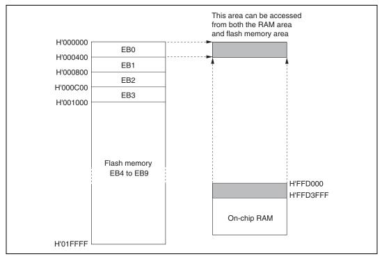
Figure 15.18 Example of RAM Overlap Operation
