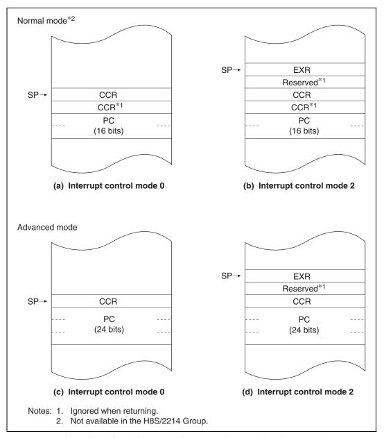
Figure 2.17 Stack Structure after Exception Handling (Examples)
