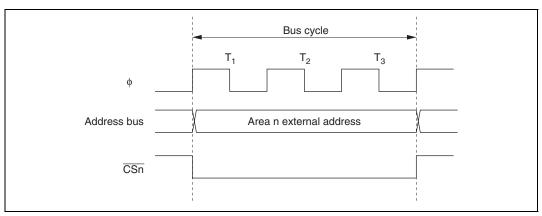
Figure 6.3  $\overline{CSn}$  Signal Output Timing (n = 0 to 7)
