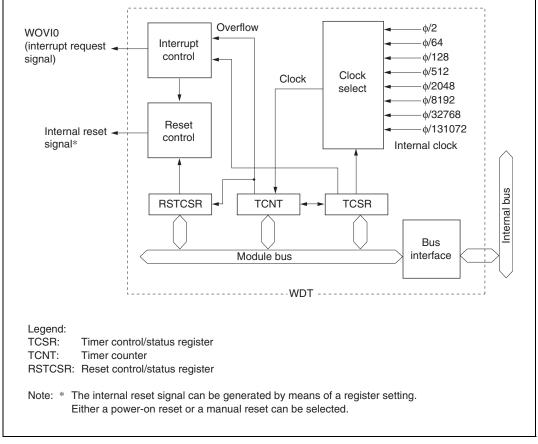
Figure 11.1 Block Diagram of WDT
