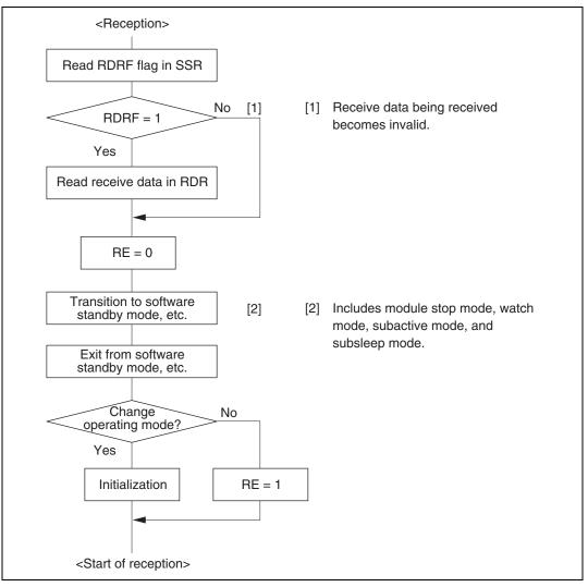
Figure 12.31 Sample Flowchart for Mode Transition during Reception
