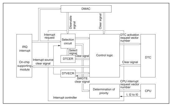
Figure 5.9 Interrupt Control for DTC and DMAC
