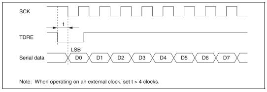
Figure 12.27 Example of Clocked Synchronous Transmission by DTC
