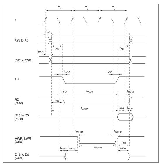
Figure 18.8 Basic Bus Timing/Three-State Access
