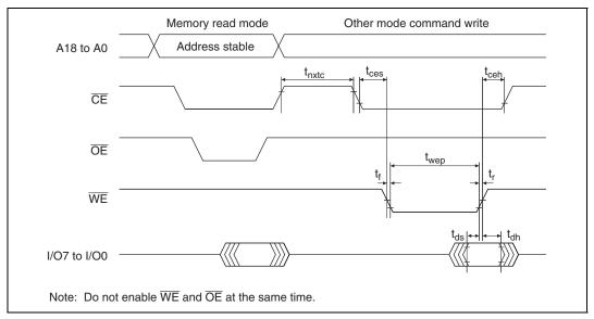
Figure 15.22 Timing Waveforms in Transition from Memory Read Mode to Another Mode
