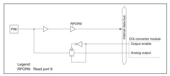
Figure C.16 Port 9 Block Diagram (Pin P96)
