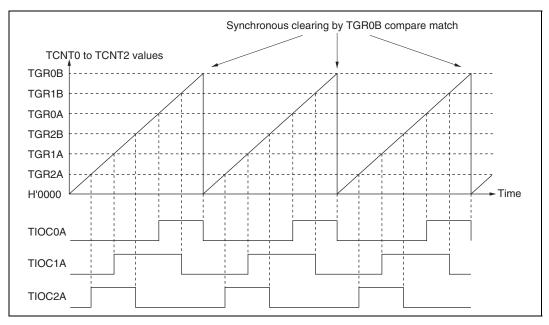
Figure 10.15 Example of Synchronous Operation
