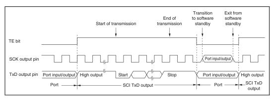
Figure 12.29 Asynchronous Transmission Using Internal Clock
