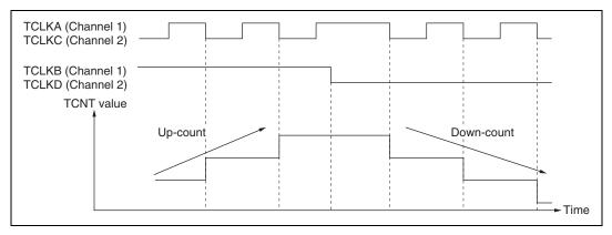
Figure 10.27 Example of Phase Counting Mode 2 Operation
