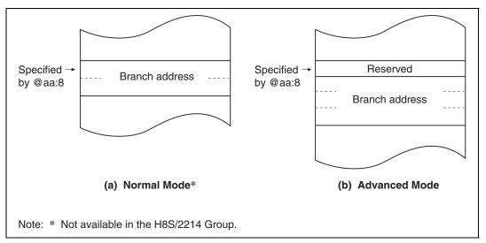
Figure 2.14 Branch Address Specification in Memory Indirect Mode
