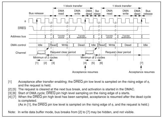
Figure 7.21 Example of DREQ Pin Falling Edge Activated Block Transfer Mode Transfer
