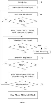
Note: When switching from transmit or receive operation to simultaneous transmit and receive operations, first clear the TE bit and RE bit to 0, then set both these bits to 1 simultaneously.
