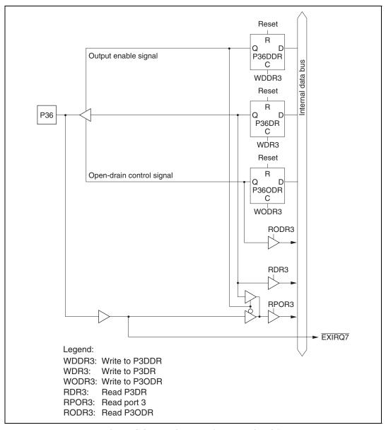
Figure C.8 Port 3 Block Diagram (Pin P36)
