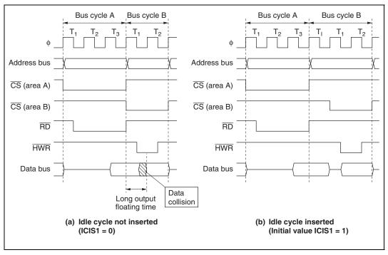
Figure 6.18 Example of Idle Cycle Operation (2)
