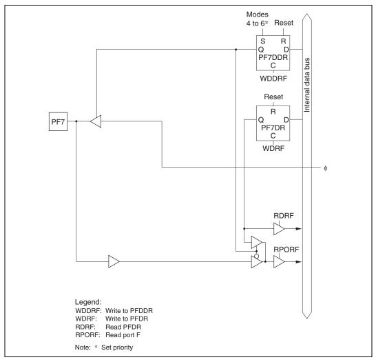
Figure C.30 Port F Block Diagram (Pin PF7)
