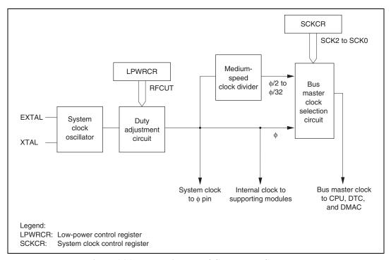
Figure 16.1 Block Diagram of Clock Pulse Generator
