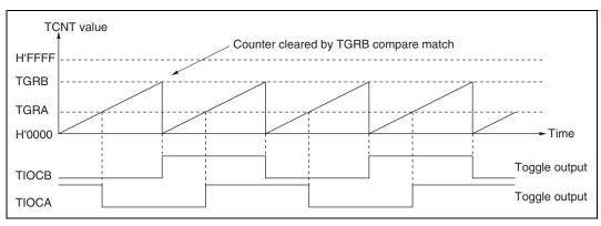
Figure 10.11 Example of Toggle Output Operation
