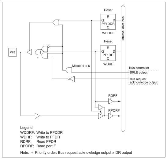
Figure C.26 Port F Block Diagram (Pin PF1)
