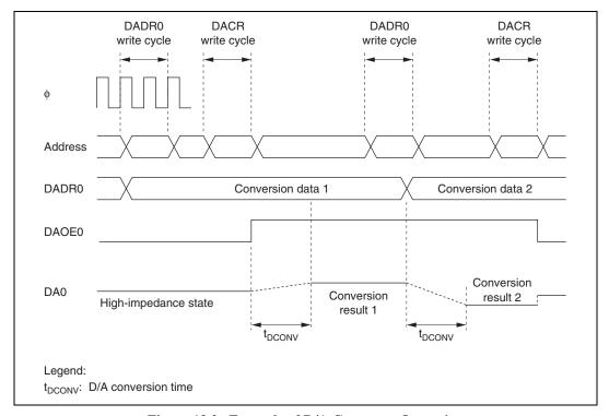
Figure 13.2 Example of D/A Converter Operation
