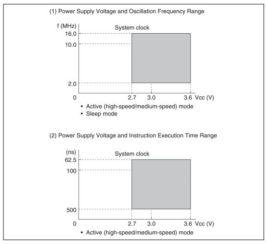
Figure 18.1 Power Supply Voltage and Operating Ranges
