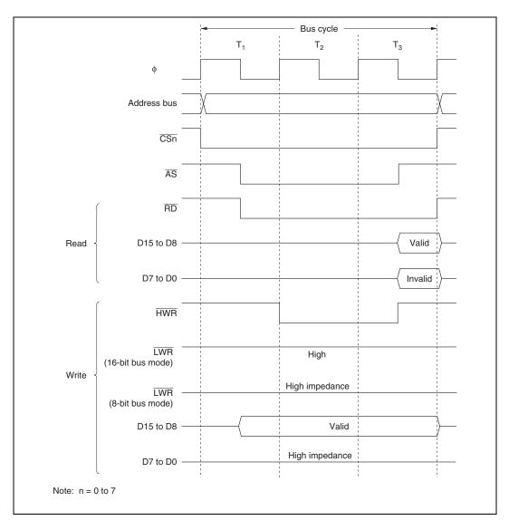
Figure 6.7 Bus Timing for 8-Bit 3-State Access Space
