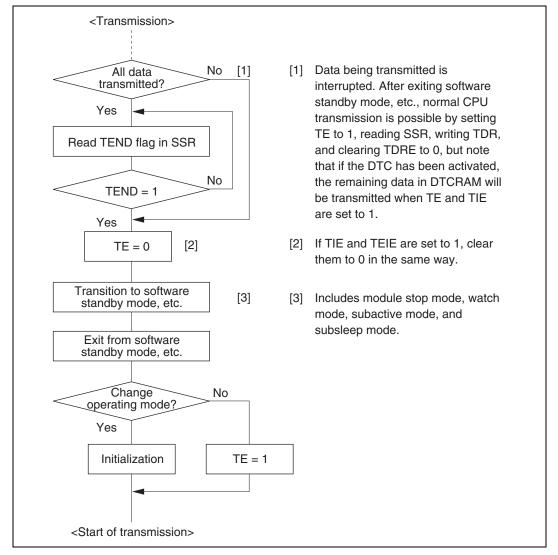
Figure 12.28 Sample Flowchart for Mode Transition during Transmission
