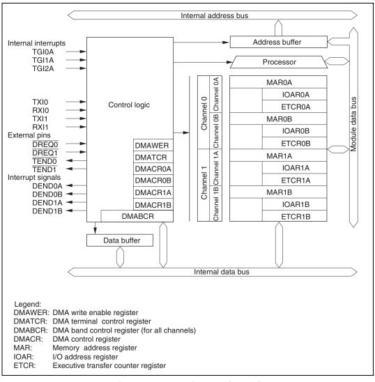
Figure 7.1 Block Diagram of DMAC
