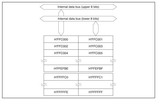
Figure 14.1 Block Diagram of RAM
