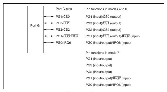
**Figure 9.19 Port G Pin Functions**
