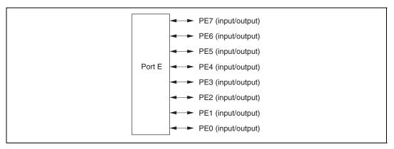
Figure 9.17 Port E Pin Functions (Mode 7)
