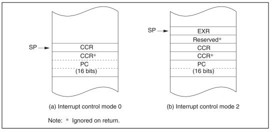
Figure 4.5 Stack Status after Exception Handling (Normal Modes: Not available in the H8S/2214)
