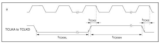
Figure 18.14 TPU Clock Input Timing
