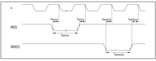
Figure 18.5 Reset Input Timing
