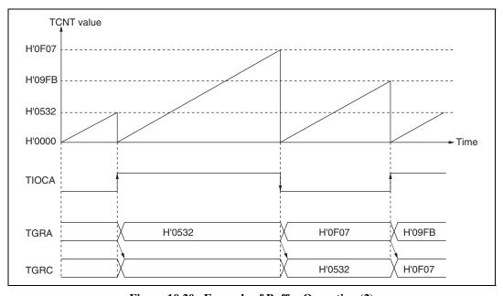
Figure 10.20 Example of Buffer Operation (2)
