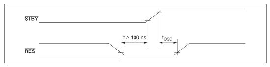
Figure E.2 Timing of Recovery from Hardware Standby Mode
