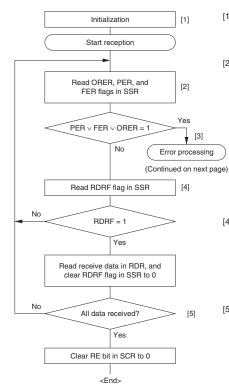
Note: \* The RDRF flag is cleared automatically by DTC only when the DTC DISEL bit is 0 and furthermore the transfer counter is not 0.
