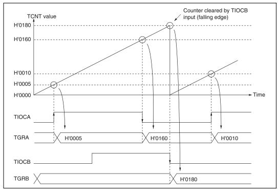
Figure 10.13 Example of Input Capture Operation
