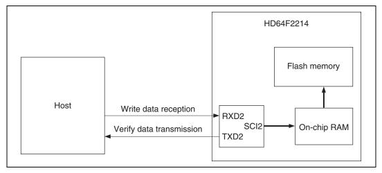
Figure 15.9 System Configuration in Boot Mode
