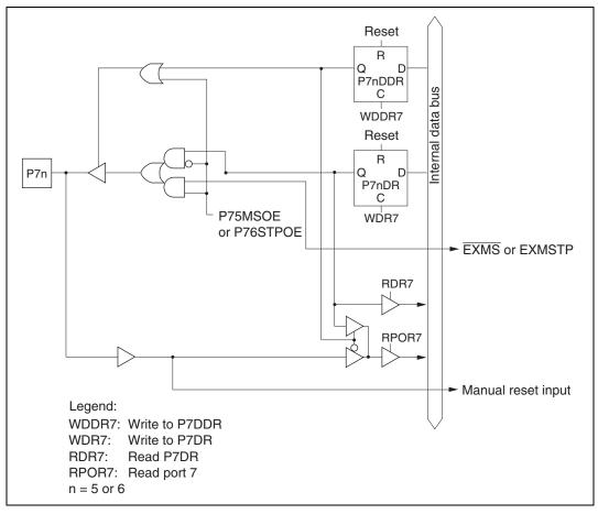
Figure C.14 Port 7 Block Diagram (Pins P75 and P76)
