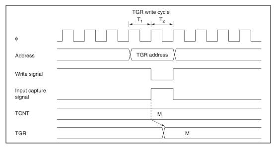
Figure 10.50 Contention between TGR Write and Input Capture
