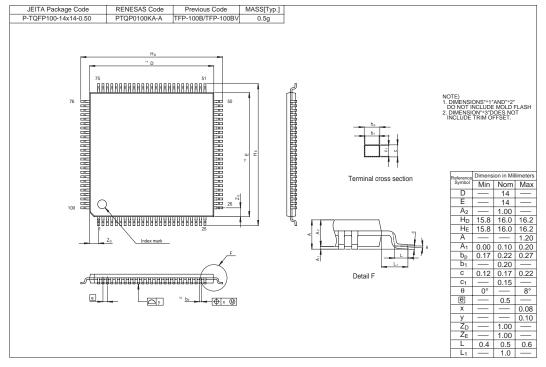
Figure G.1 TFP-100B, TFP-100BV Package Dimensions
