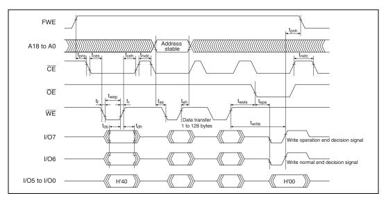
Figure 15.25 Auto-Program Mode Timing Waveforms
