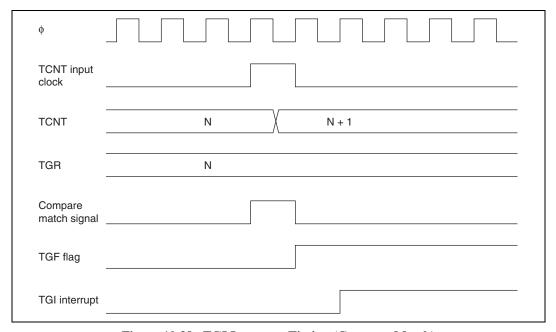
Figure 10.38 TGI Interrupt Timing (Compare Match)
