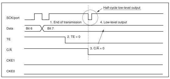
Figure 12.32 Operation when Switching from SCK Pin Function to Port Pin Function
