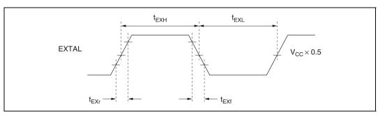
Figure 16.6 External Clock Input Timing
