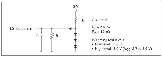
Figure 18.2 Output Load Circuit
