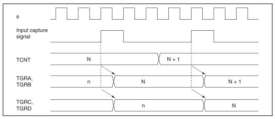
Figure 10.37 Buffer Operation Timing (Input Capture)
