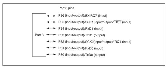
Figure 9.2 Port 3 Pin Functions
