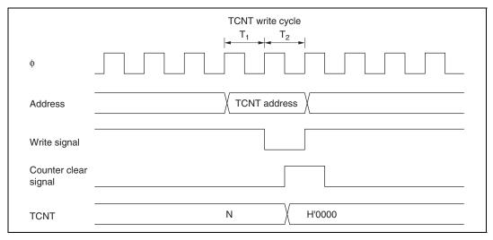
Figure 10.45 Contention between TCNT Write and Clear Operations
