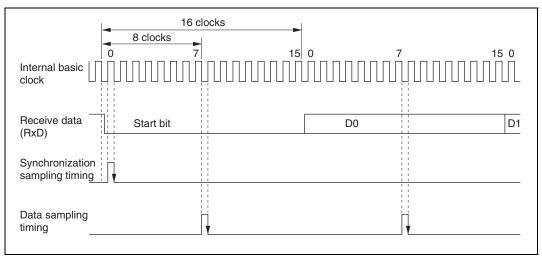
Figure 12.26 Receive Data Sampling Timing in Asynchronous Mode
