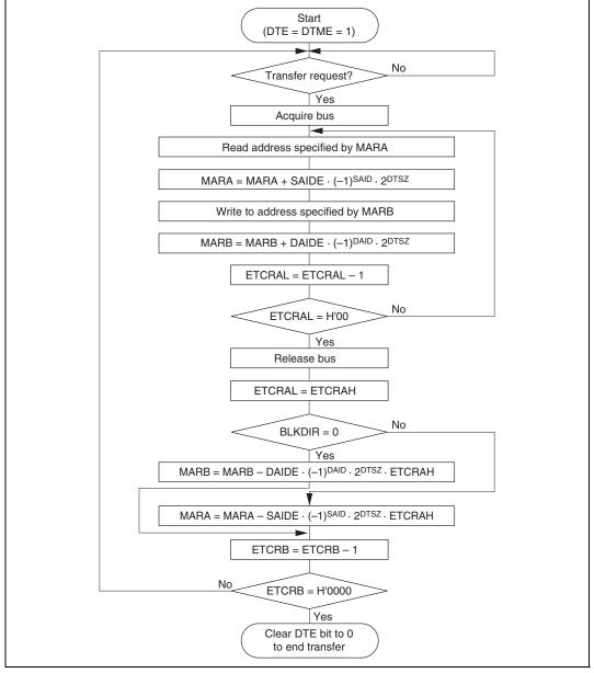
Figure 7.13 Operation Flow in Block Transfer Mode
