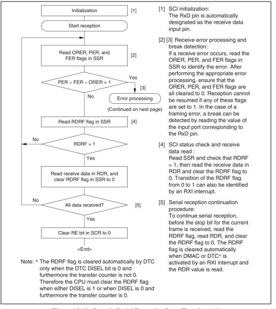
Figure 12.10 Sample Serial Reception Data Flowchart (1)
