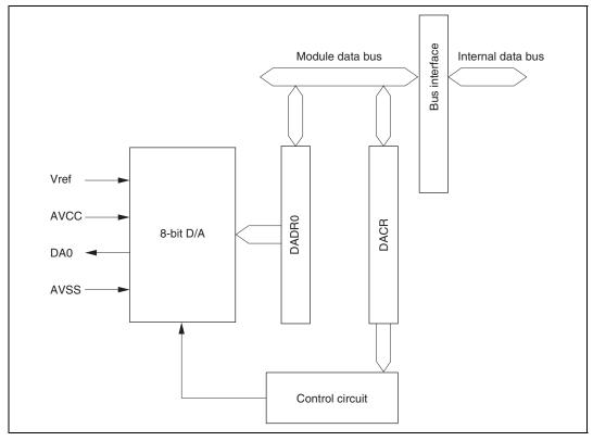
Figure 13.1 Block Diagram of D/A Converter
