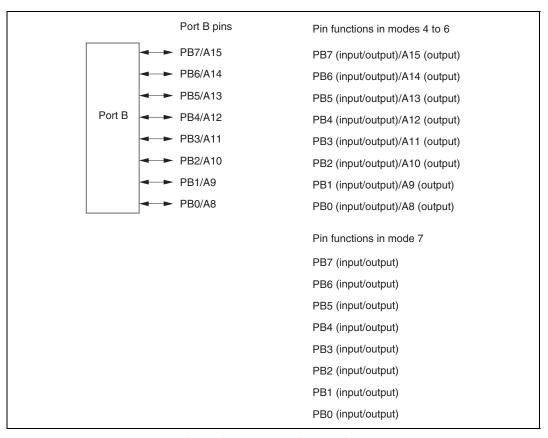
Figure 9.7 Port B Pin Functions
