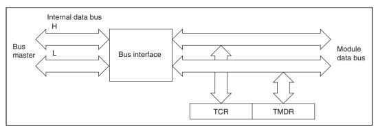
Figure 10.5 8-Bit Register Access Operation [Bus Master  $\leftrightarrow$  TCR and TMDR (16 Bits)]
