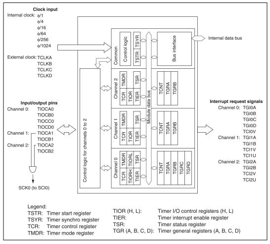
Figure 10.1 Block Diagram of TPU
