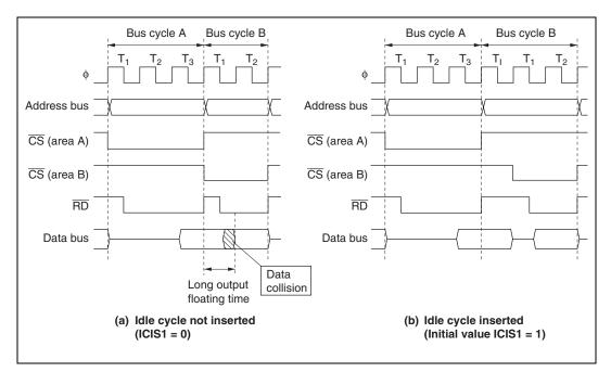
Figure 6.17 Example of Idle Cycle Operation (1)
