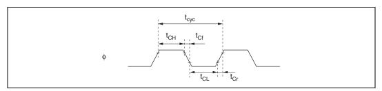
Figure 18.3 System Clock Timing
