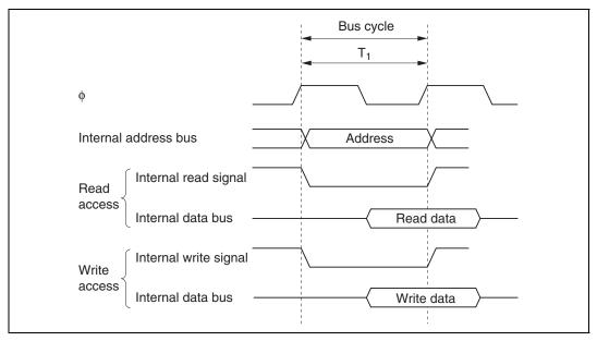
Figure 2.18 On-Chip Memory Access Cycle
