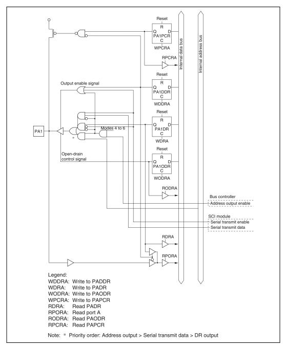
Figure C.18 Port A Block Diagram (Pin PA1)
