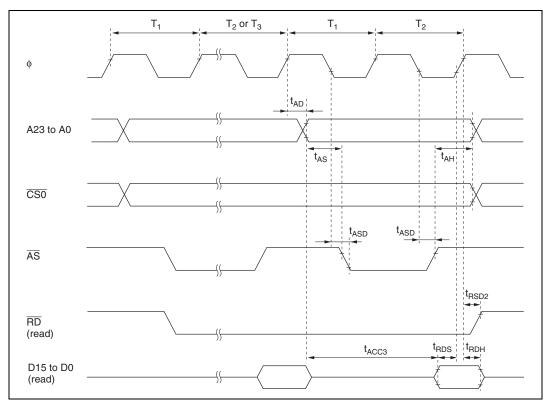
Figure 18.10 Burst ROM Access Timing/Two-State Access
