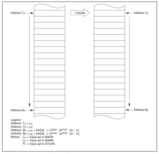
**Figure 7.9 Operation in Normal Mode**
