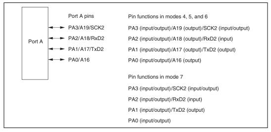
Figure 9.6 Port A Pin Functions
