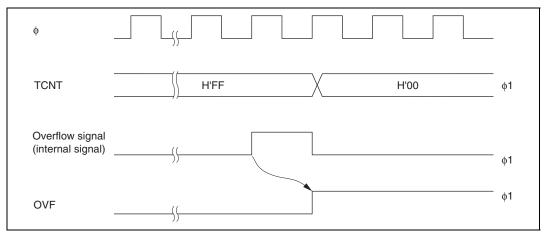
Figure 11.6 Timing of OVF Setting
