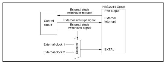
Figure 16.7 Example of External Clock Switching Circuit
