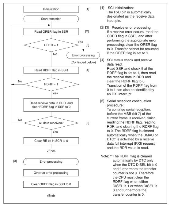
Figure 12.23 Sample Serial Reception Flowchart
