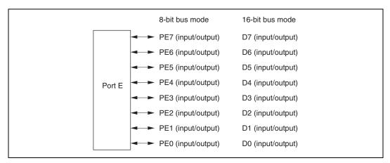
Figure 9.16 Port E Pin Functions (Modes 4 to 6)
