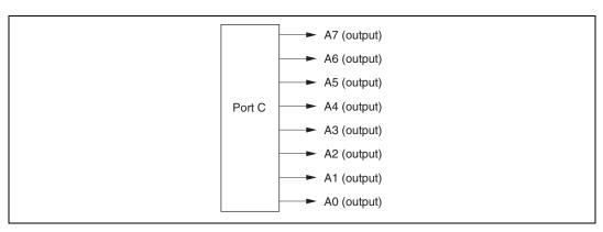
Figure 9.9 Port C Pin Functions (Modes 4 and 5)
