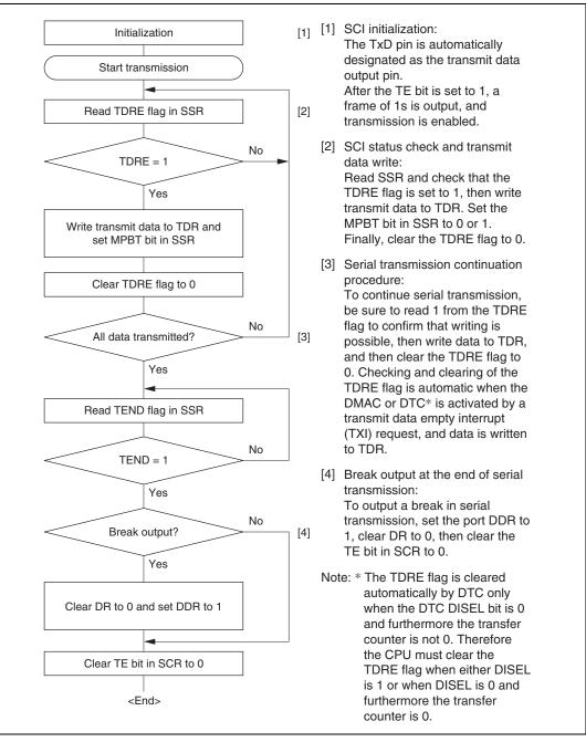
Figure 12.14 Sample Multiprocessor Serial Transmission Flowchart
