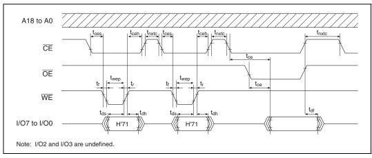
Figure 15.27 Status Read Mode Timing Waveforms
