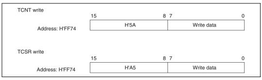
Figure 11.2 Format of Data Written to TCNT and TCSR (Example of WDT0)
