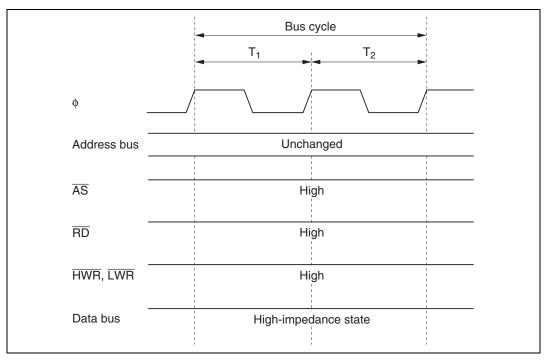
Figure 2.21 Pin States during On-Chip Supporting Module Access
