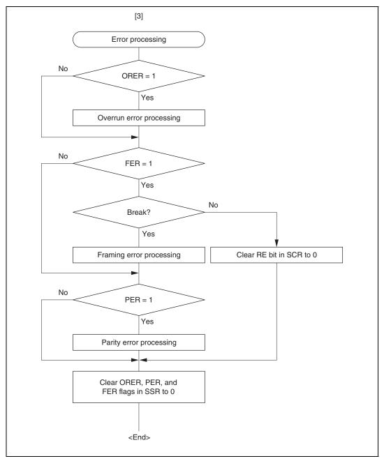
Figure 12.11 Sample Serial Reception Data Flowchart (2)
