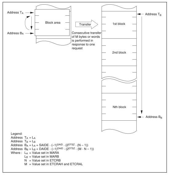
Figure 7.12 Operation in Block Transfer Mode (BLKDIR = 1)
