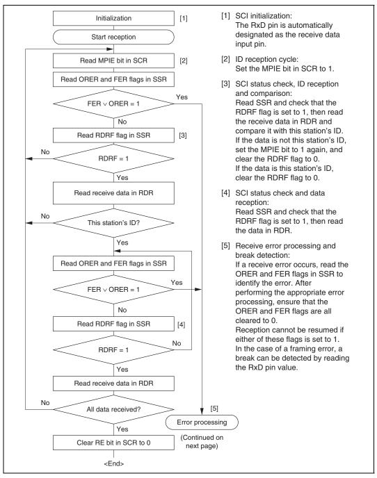
Figure 12.16 Sample Multiprocessor Serial Reception Flowchart (1)
