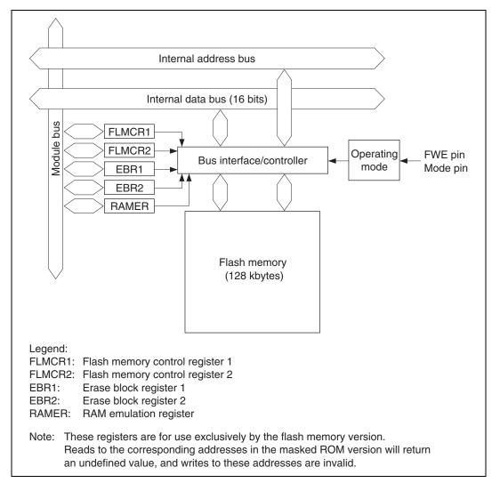
Figure 15.2 Block Diagram of Flash Memory
