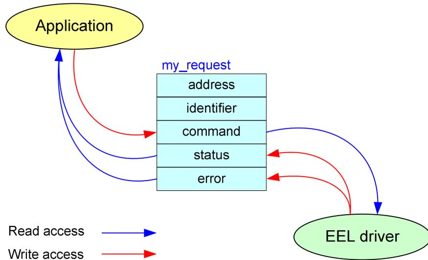
Figure 4-19 Shutdown request and feedback
