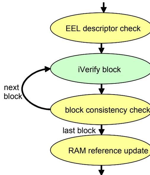
Figure 4-1 sequence of the startup command
