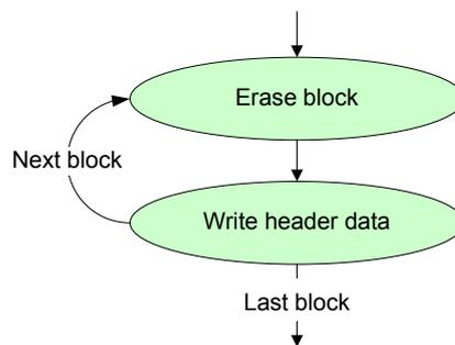
Figure 4-9 sequence of the format command
