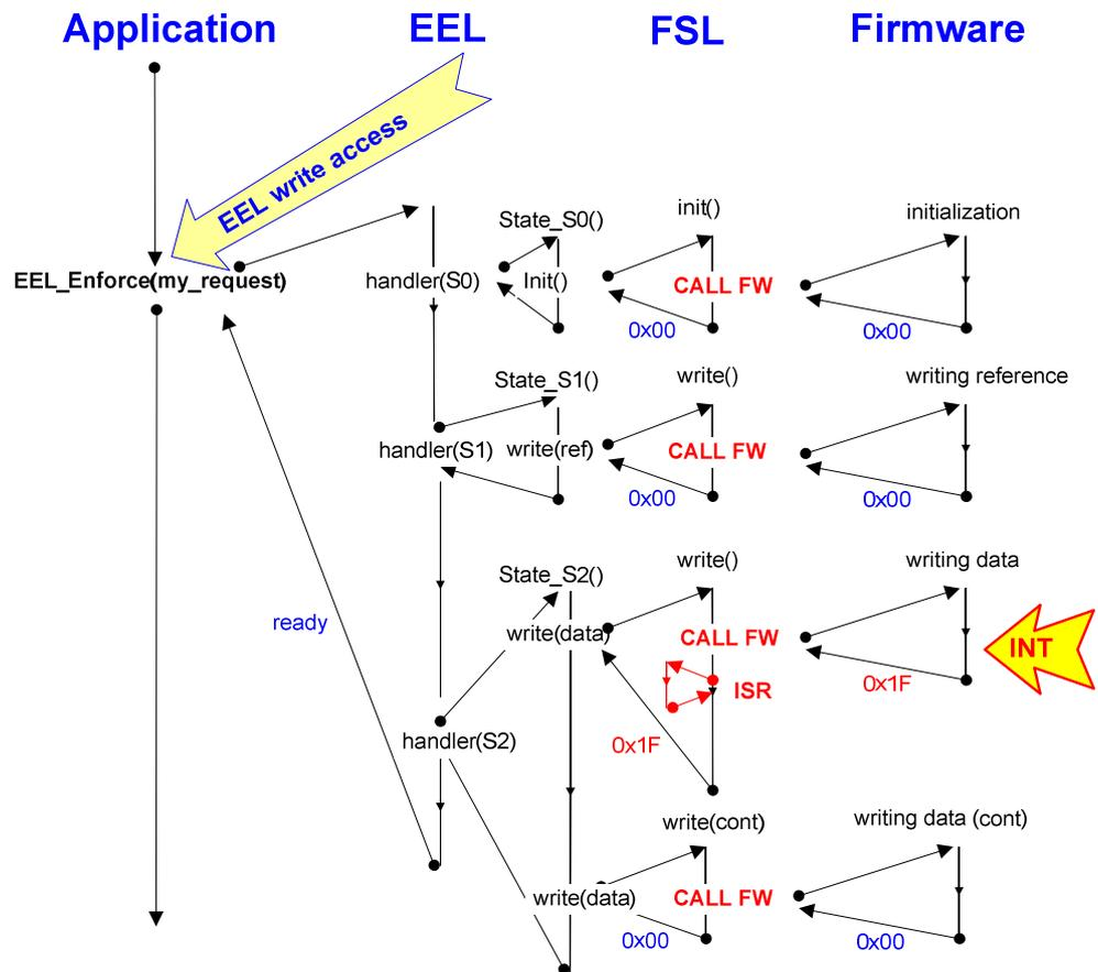
Figure 3-2 typical flow of an EEL\_Enforce function
