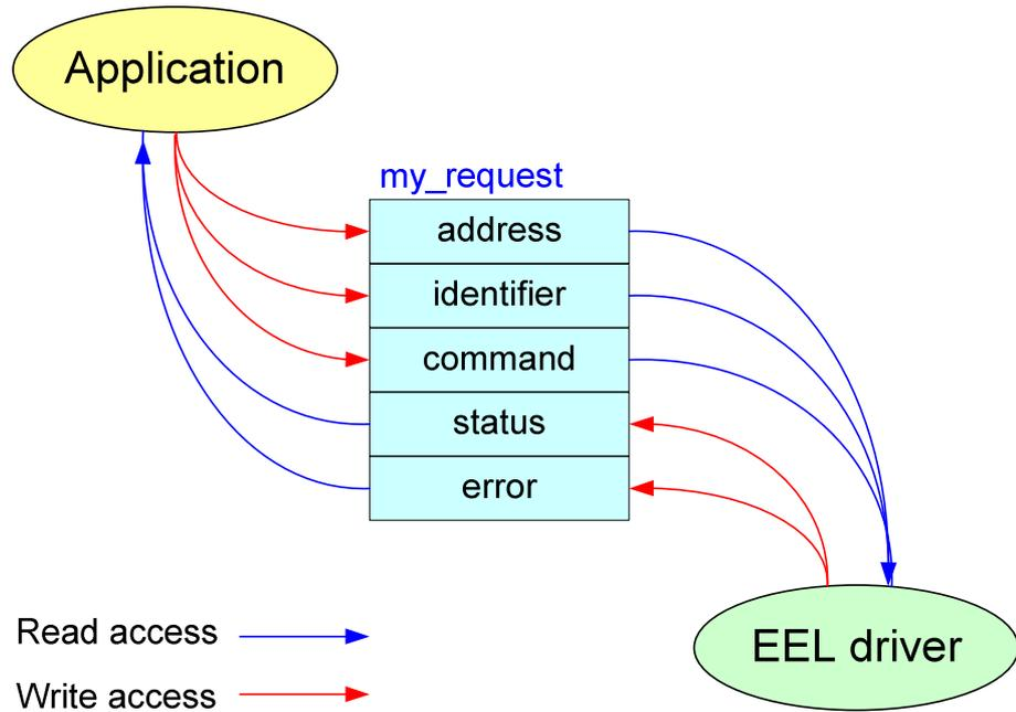
Figure 4-4 write request and feedback
