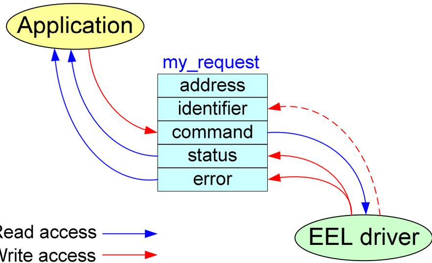
Figure 4-10 Format request and feedback
