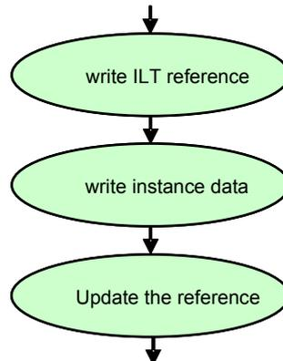
Figure 4-3 sequence of the write command
