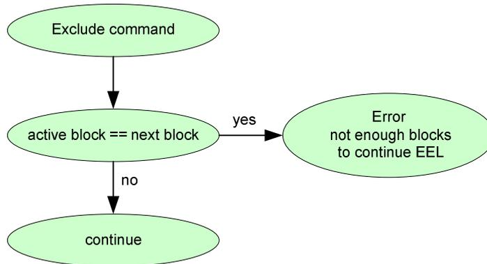
Figure 4-15 flow to use with the exclude command
