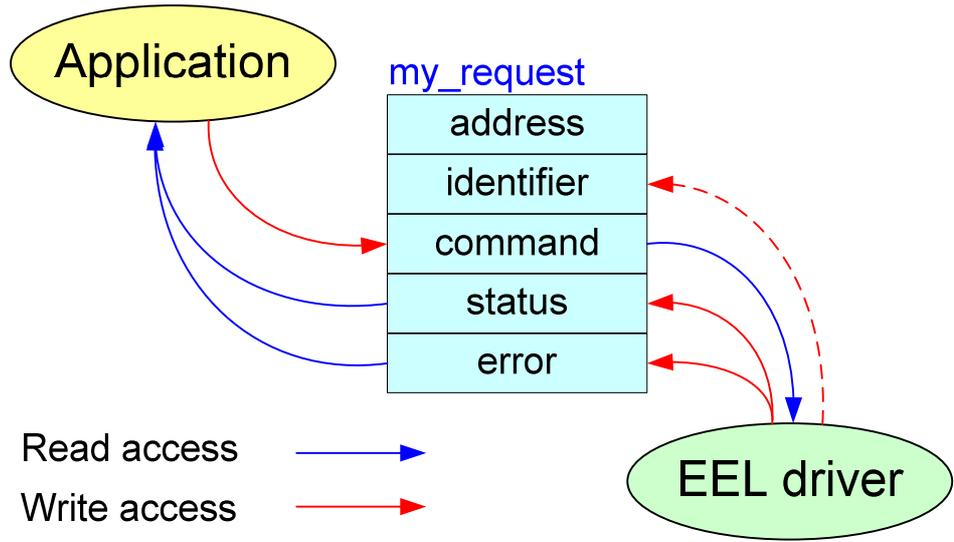
Figure 4-2 Startup request and feedback
