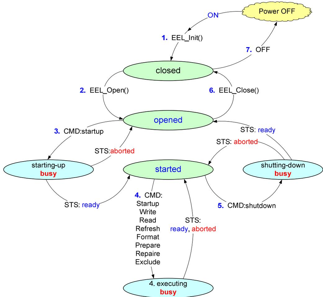
Figure 6-1 EEL driver activation and deactivation sequence
