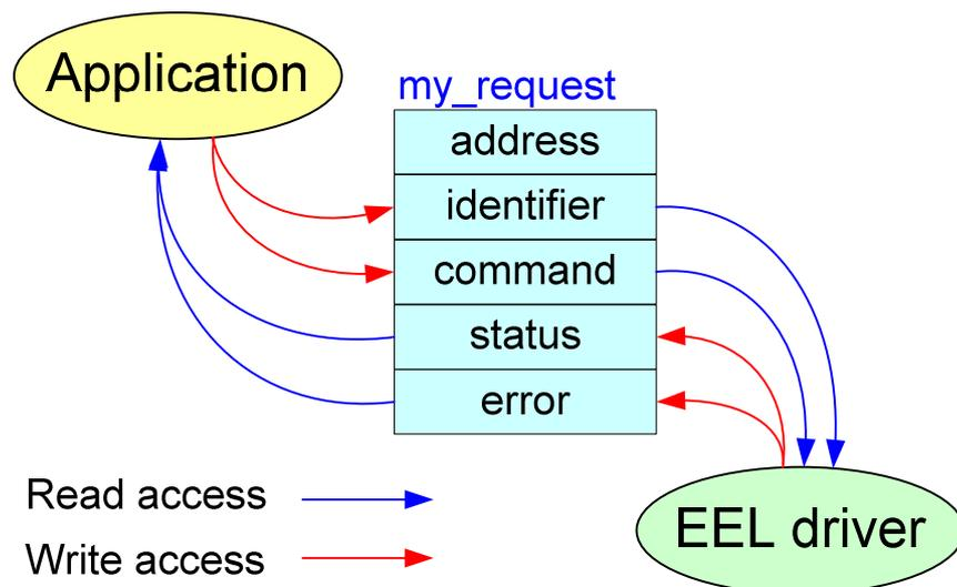
Figure 4-14 Repair request and feedback
