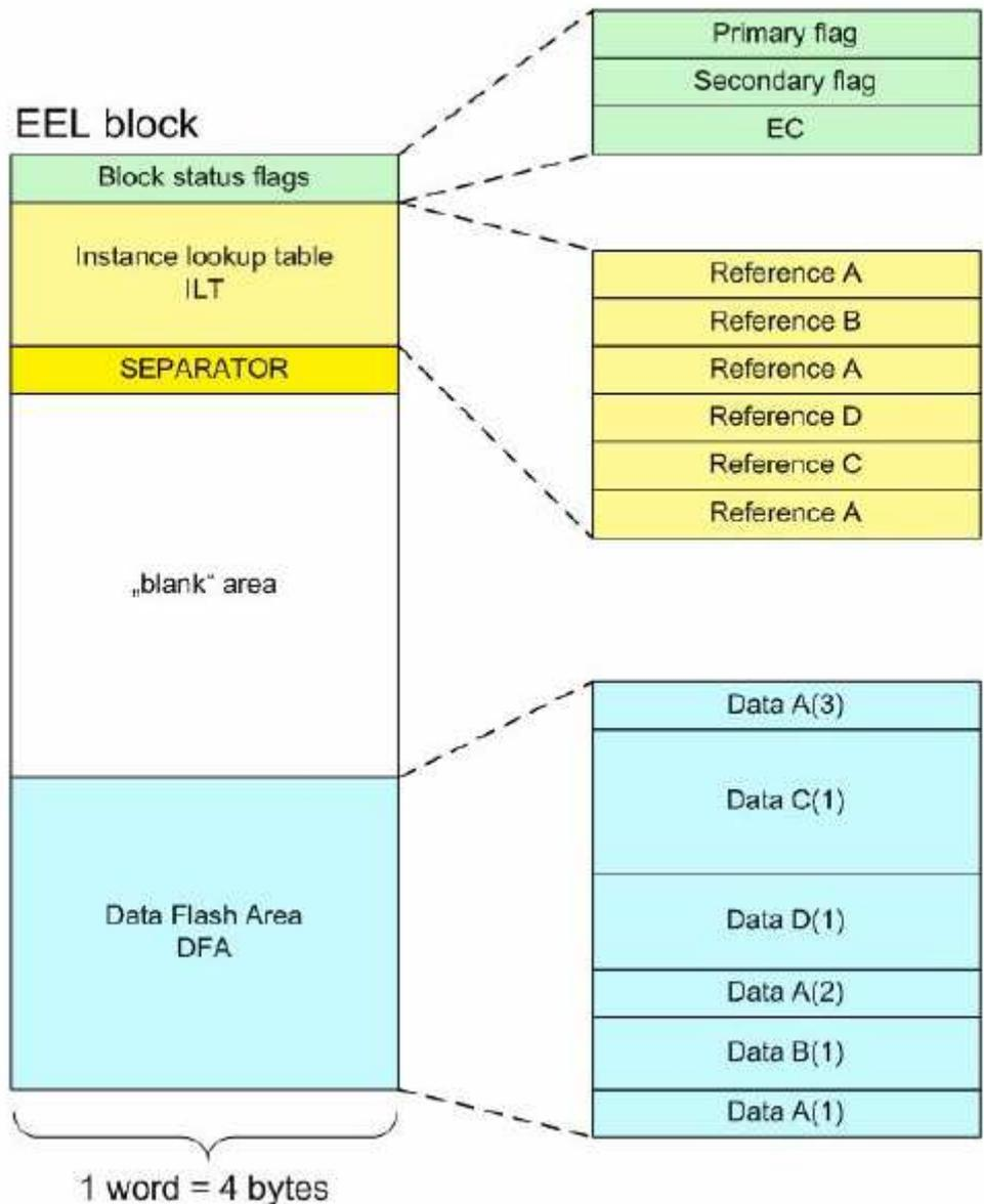
Figure 2-7 typical structure of an EEL block
