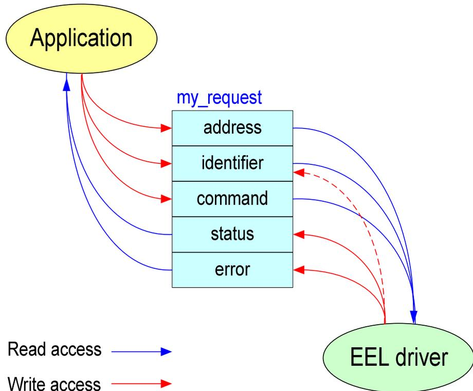
Figure 3-1 request variable synchronizing EEL and the application
