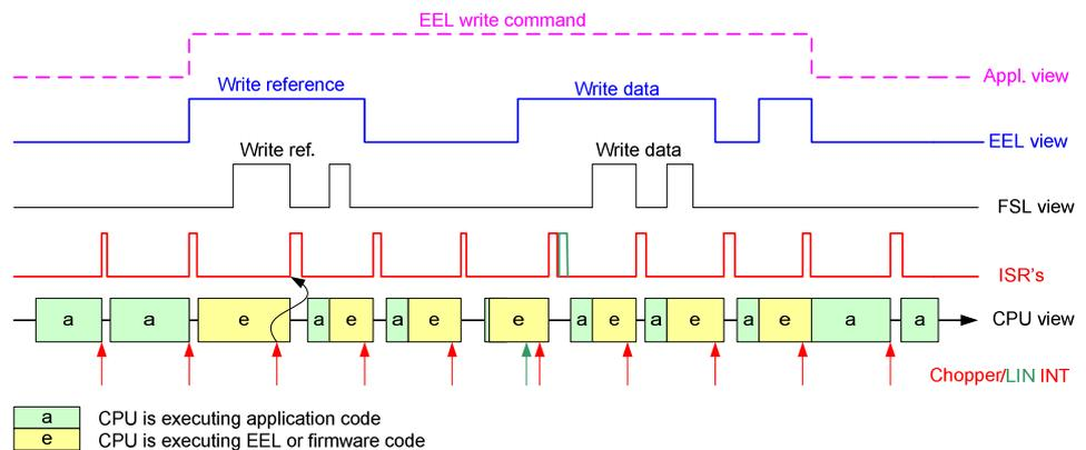
Figure 6-3 Timing example of interrupted "background" operation mode
