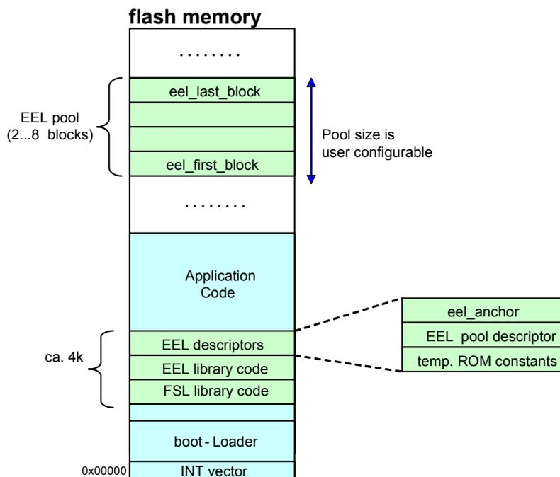
Figure 2-4 physical placement inside the device flash memory
