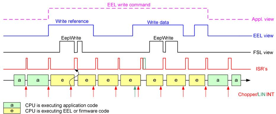
Figure 6-2 Timing example of interrupted "enforced" operation mode
