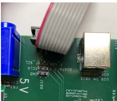
Figure 3. Connect Aardvark Adapter to J37
