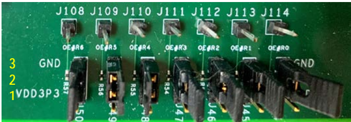
Figure 7. Output OE Pin Control
