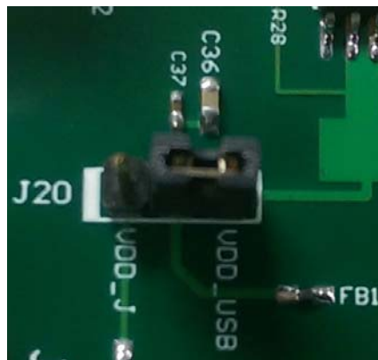
Figure 2. Connecting the jumper to VDD_J or VDD_USB. Default is to power by USB
