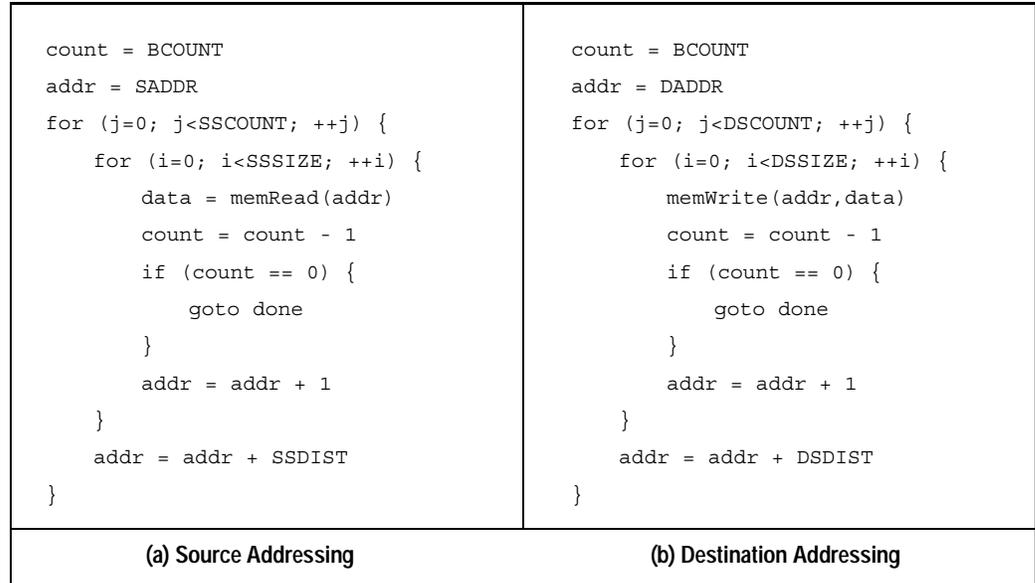
Figure 15.4 DMA Channel Addressing<sup>1</sup>
