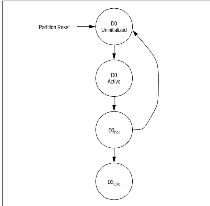
Figure 9.1 PES32NT24xG2 Power Management State Transition Diagram
