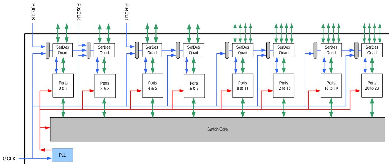
Figure 2.2 Logical Representation of PES32NT24BG2 Clocking Architecture
