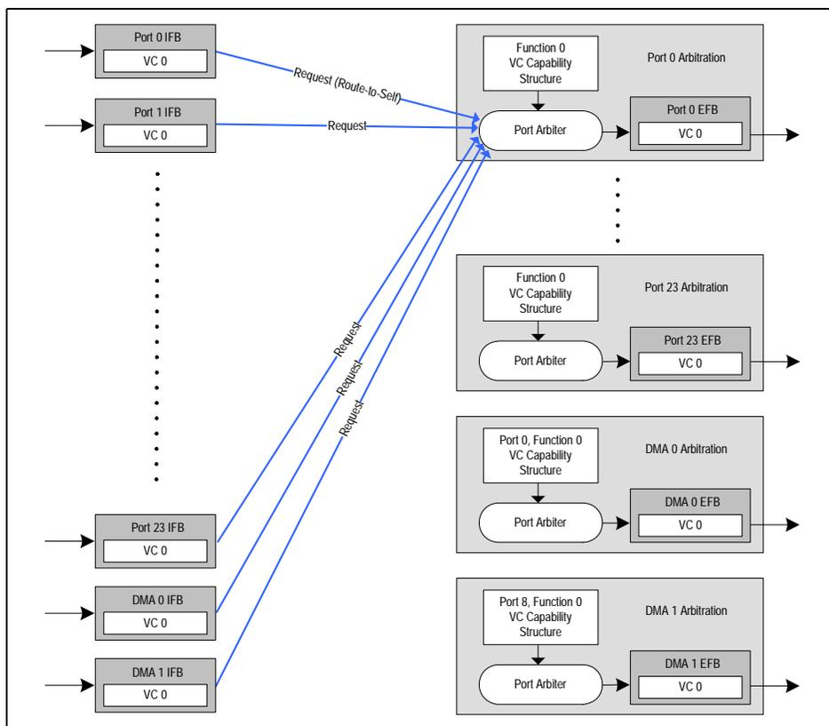
Figure 4.2 Architectural Model of Arbitration
