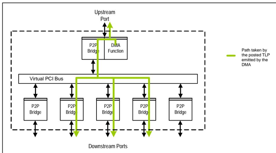
Figure 15.12 Path Taken by a TLP Emitted by the DMA When it is Multicast<sup>1</sup>
