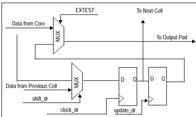
Figure 25.4 Diagram of Output Cell
