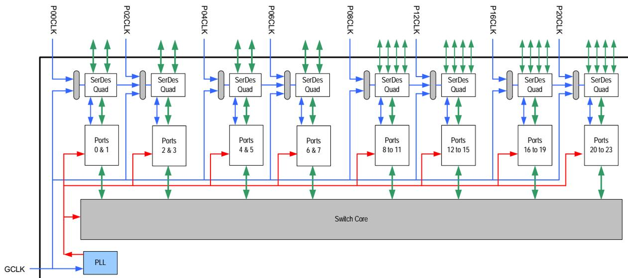
Figure 2.1 Logical Representation of PES32NT24AG2 Clocking Architecture
