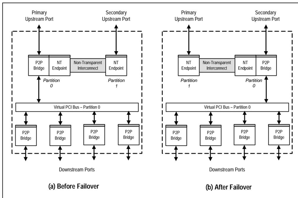
Figure 1.15 Non-Transparent Switch Failover Usage
