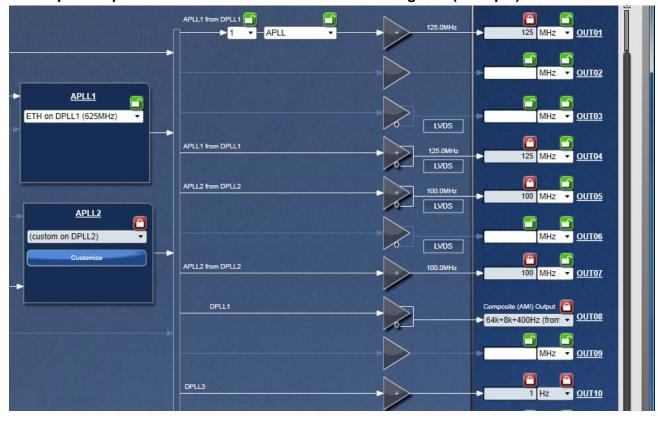
Figure 15. Output Frequencies Entered after APLL1/APLL2 Configured (example)
