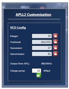
Once APLL1 and APLL2 have been configured, output frequencies can now be entered at OUT01 ~ OUT04 (APLL1), OUT05~OUT07(APLL2) and OUT08~OUT10 (DPLLs).
