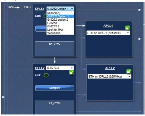
Click "Configure" button to open up configuration window for respective DPLL for additional or customized configuration. There are pull-down items for each configuration parameter. For example, in "Operation Mode" section, you can select:
