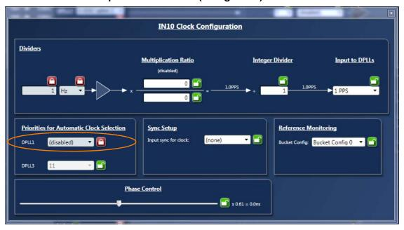
6. Each DPLL has Profile Selection and a "Configure" button. In general, the pull-down Profile Selection should be sufficient to automatically pre-configure the DPLL and reference monitor for the specific ITU-T recommendation.
