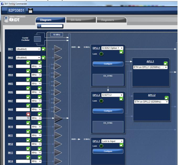
To associate an input clock (i.e., IN09) with a sync signal (such as 1PPS), click on the Input Buffer of IN09 (the triangle symbol following frequency entry box), a sub-configuration window for IN09 is shown below. In the window, IN10 is selected as sync signal.
