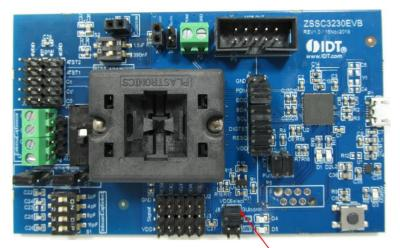
Figure 3. External Cap Sensor Connection
