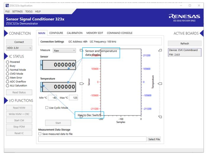
Figure 11. Sensor Readings on the "MAIN" Tab
