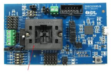
Figure 2. VDD Select Jumper Location
