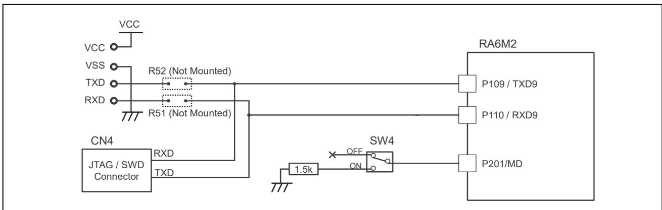
Figure 5. RA6M2 Operating Mode Setting Circuit
