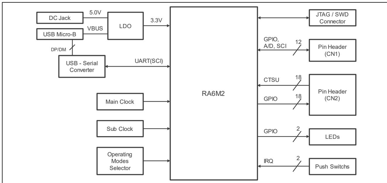
**Figure 3. RA6M2 Cap Touch CPU Board Block Diagram**
