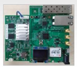
CN268 IEEE-1588 Solution for Synchronization of timing networks
