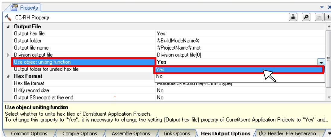
When the boot loader project is rebuilt, hex files of the boot loader project are united with hex files of the projects that have been specified as constituent application projects.
