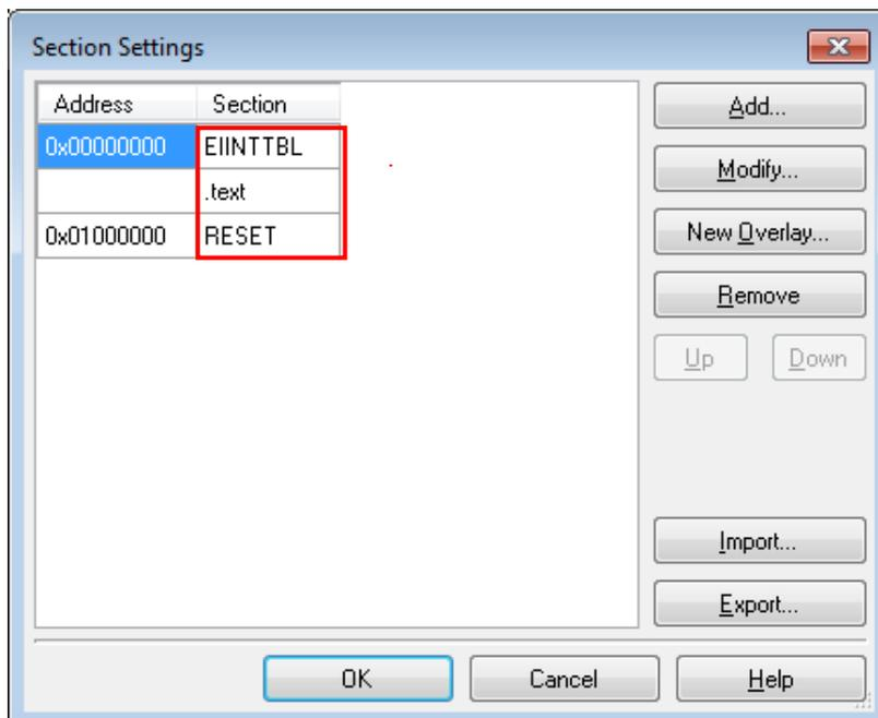
Based on this section setting, the "EIINTTBL=>.text" section is allocated from address 0x00000000 in the address ascending order and the RESET section is allocated from address 0x01000000. Customize the section settings in this dialog box so that the sections are allocated to the desired addresses.
