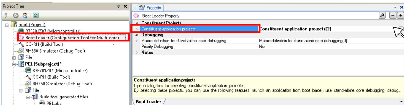
Click the [...] button at the right edge. This opens the [Select Constituent Application Projects] dialog box as shown below. Application projects "PE1" and "PE3" which have been added to boot loader project "boot" are selected, and they are registered as constituent application projects of "boot".
