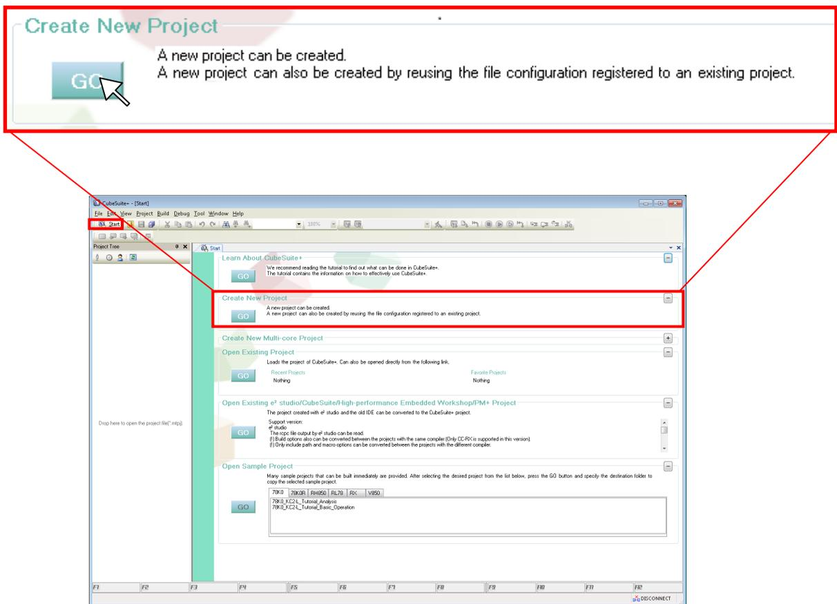
**Remarks** A project can also be created from [Create New Multi-core Project] on the Start panel. In this case, if [Create an application project with a boot loader project] is selected in the Create Project dialog box, a boot loader project and a single application project are created. The application project name becomes "Boot loader project name\_App1". The project name can be changed.
