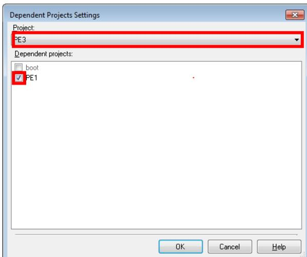
This dialog box setting specifies that PE3 is a project dependent on PE1. As a result, rebuilding takes place in the order of PE1 => PE3 => boot.
