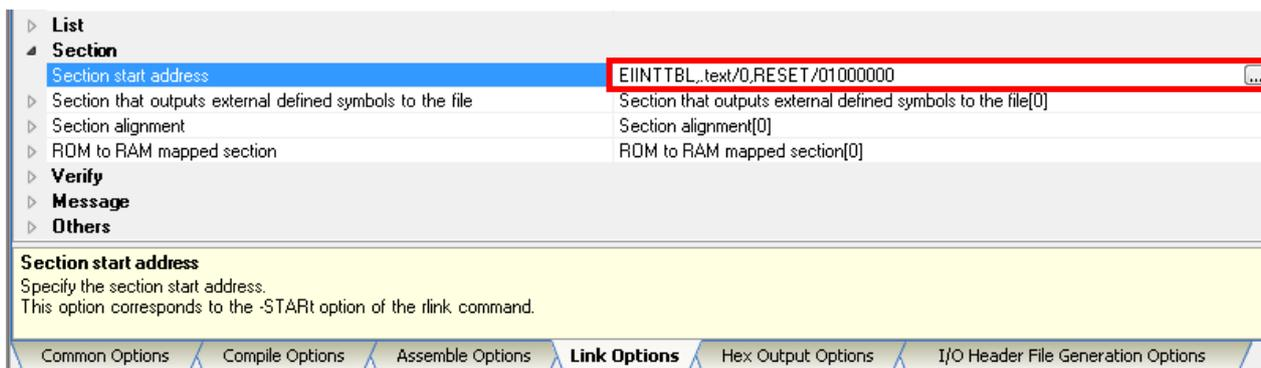
Clicking the [...] button at the right edge of the [Section start address] property opens the Section Settings dialog box as shown below. The start address of the section can also be specified from this dialog box.
