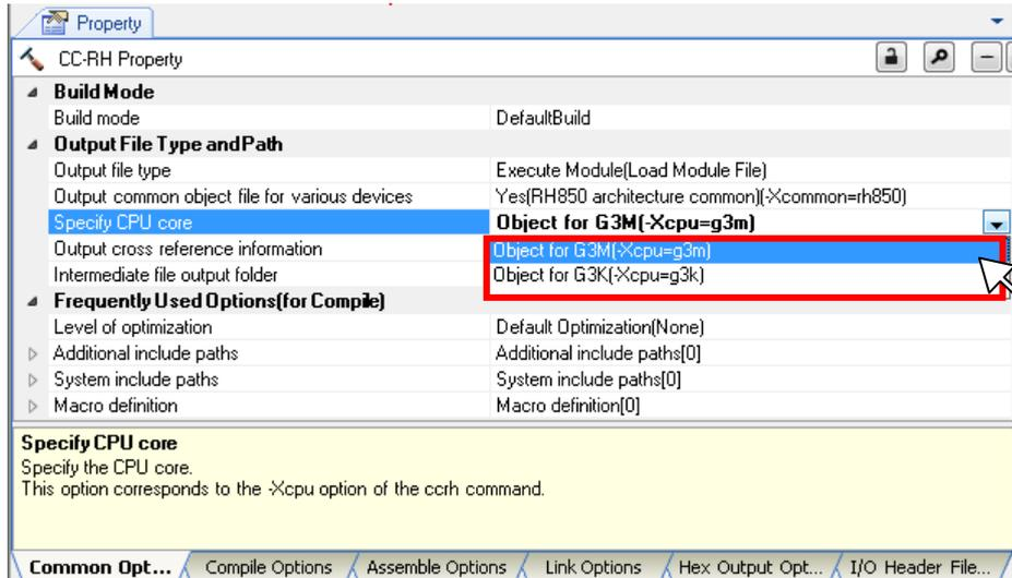
Select [Object for G3M] for a main CPU project and select [Object for G3K] for a PCU project. [Object for G3K] should be selected when compiling a file that includes functions that are executed from both the main CPU and PCU.
