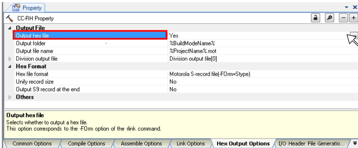
Next, select either "Intel HEX file" or "Motorola S-record file" in [Hex Output Options] tab -> [Hex Format] category -> [Hex file format]. Note that Intel HEX files and Motorola S-record files cannot be united. The hex format for the boot loader project and application projects must be the same.
