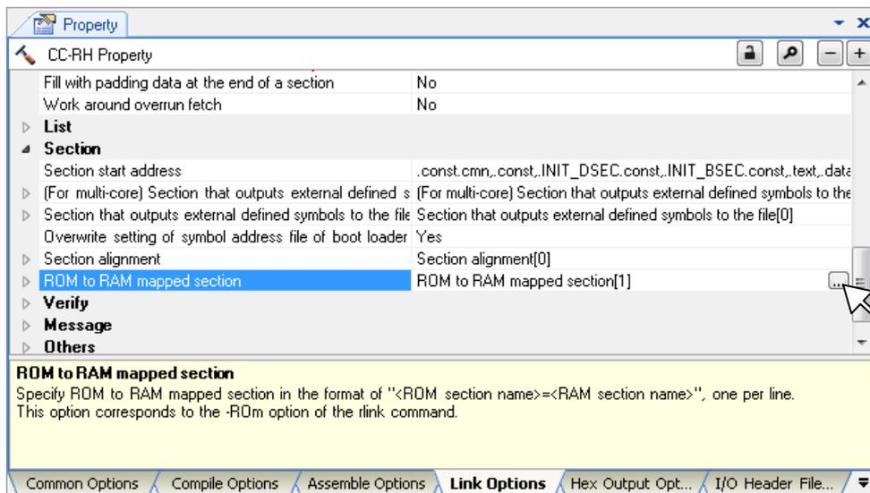
`<ROM section name>` is the section to which ROMization is to be performed. The -start option is used to specify the section set in `<ROM section name>` to be allocated to ROM and the section set in `<RAM section name>` to be allocated to RAM.
