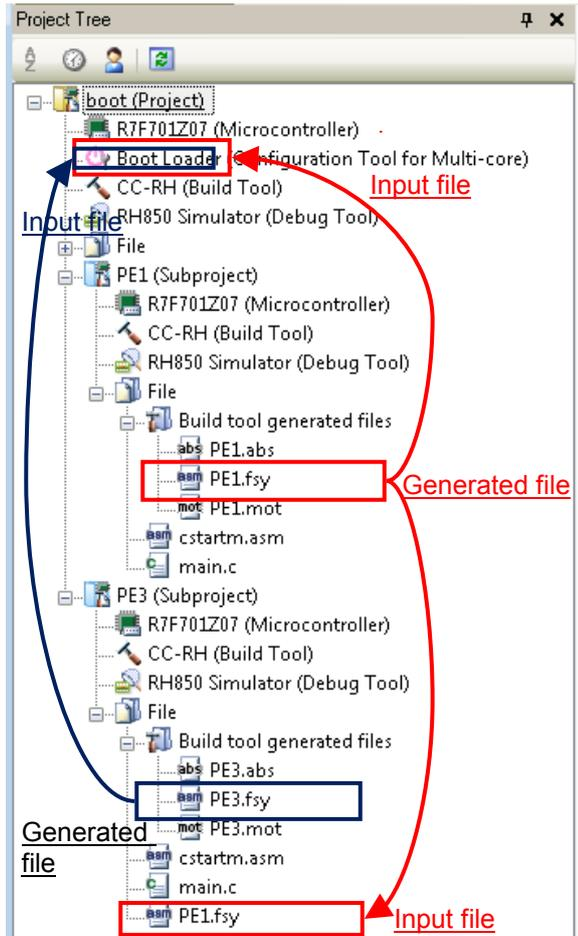
1. When the entire project is rebuilt, first the "PE1" project will be rebuilt. This generates the symbol address file (PE1.fsy) containing the located addresses of the application information table (\_pm1\_setting\_table) and shared variables and shared functions which are defined in "PE1".
