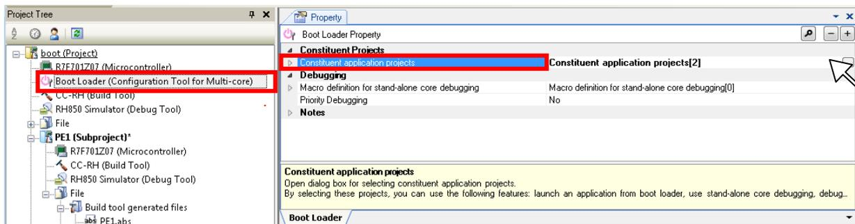
This opens the [Select Constituent Application Projects] dialog box as shown below. It can be confirmed that the application projects added to the boot loader project have been selected and the \*.fsy files that will be generated in that application project are associated.
