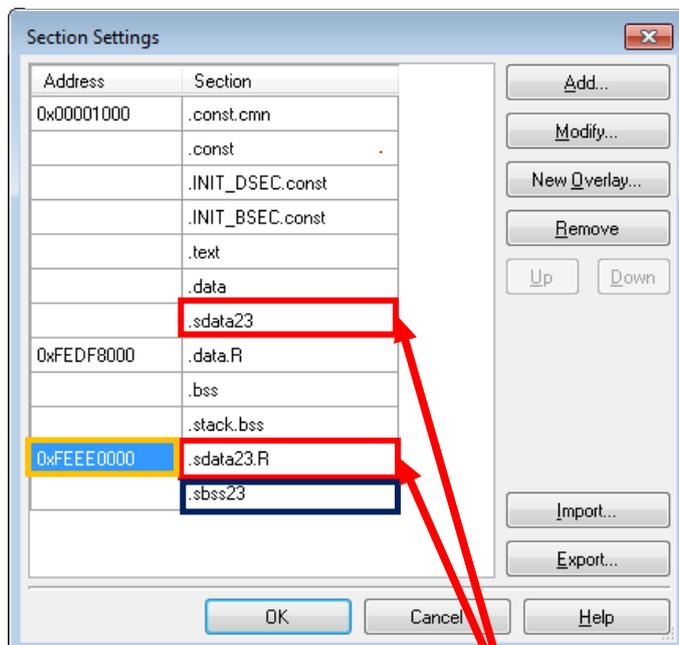
.sdata23 which is specified as the <ROM section name> parameter of the -rom option is specified to be located in the ROM area while .sdata23.R which is specified as the <RAM section name> parameter is specified to be located in the RAM area.
