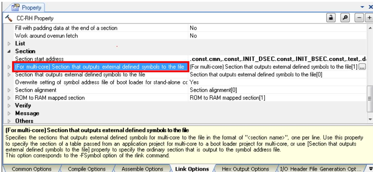
In [(For multi-core) Section that outputs external defined symbols to the file], specify a section name that includes external symbols shared between application projects or between the boot loader project and application projects.
