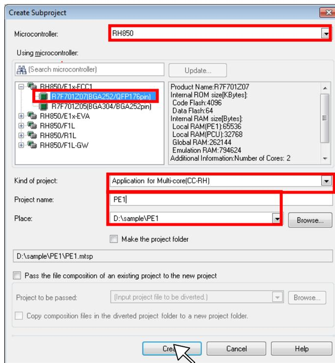
\* When a project was created from [Create New Multi-core Project] on the Start panel, in addition to the boot loader project, one application project for a multi-core will be created as a subproject.
