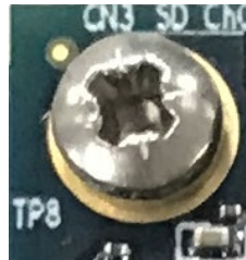
Specially shaped screw threads
