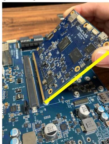
3. Insert the replacement the board diagonally, then roll the SMARC board parallel to the board and fix it with screws.
