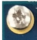
2. Remove the screw and the board will stand up at an angle. Slide it out.
