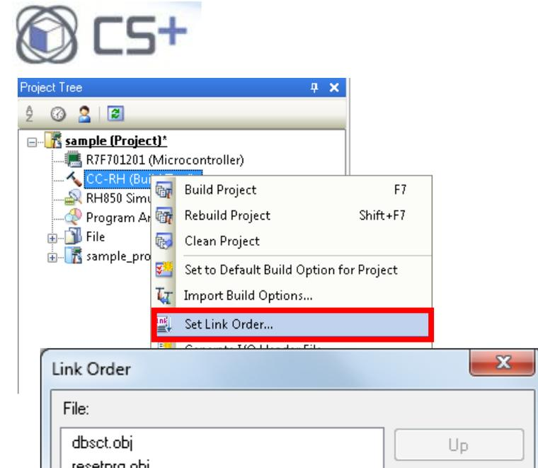
Since CS+ has an internal order of management by default, the order will require rearrangement to have the order in CS+ conform to that in the HEW environment.
