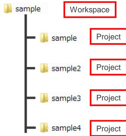
You can freely create projects in HEW. For example, \*.abs and \*.lib files can be generated for each project and parent and child relationships between projects can be set up.
