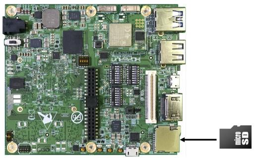
Figure 10. Set micro SD card to SMARC-EVK
