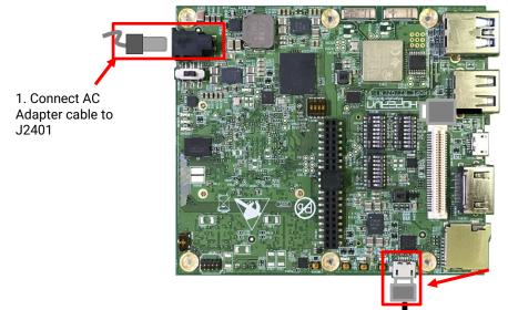
Connect USB Type-microAB cable to CN2201 for SCI download
