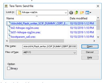
The image will be sent to the board via serial connection.
