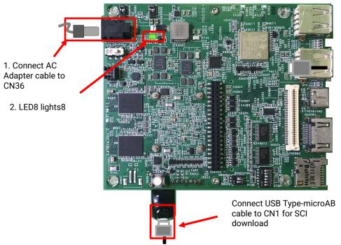
**Figure 8. Connecting Power Supply**
