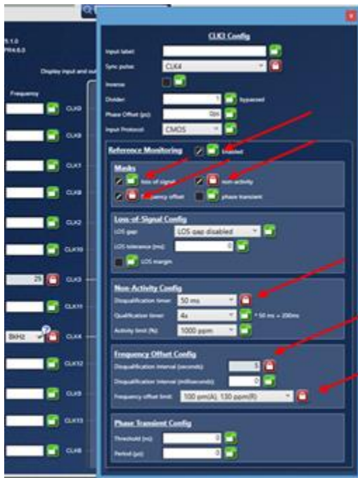
Figure 5. Timing Commander: Reference Monitors Location
